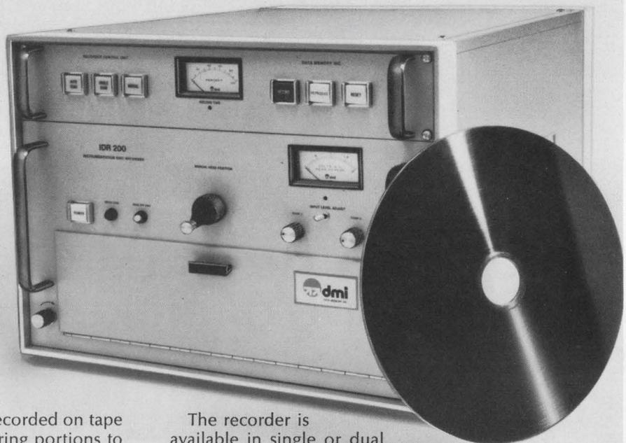
The recorder is available in single or dual channel models. The dual channel model, stores 10 seconds of data on each channel. For more information, or assistance in applying the IDR-200 to solving your particular problems, contact DMI today.
