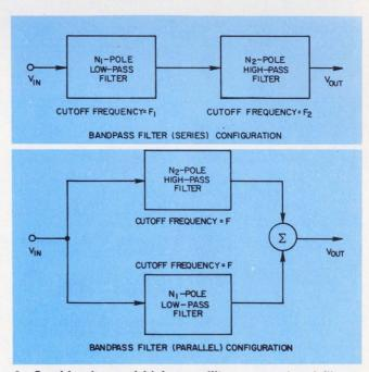
2. Combine low and high-pass filters to get band filters. If  $F_2 > F_1$ , the filter is bandpass, if  $F_1 > F_2$ , it is a band-stop filter.
