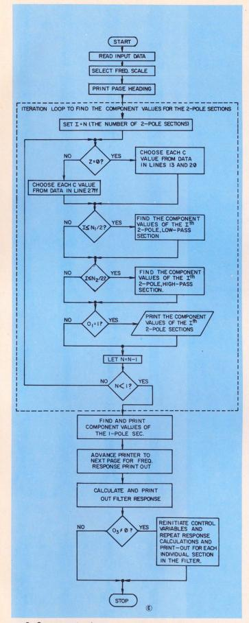
**3.** Component values are computed by this expanded **BASIC program:** (a) is the main program; (b) is a list of the subroutines used in the main program; (c) is a flow chart of the complete program.
