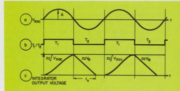
4. Integrator output (c) shows ac signal integrated during  $T_1$ , dc reference integrated during  $T_2$ .
