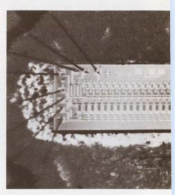
**Differential IC operational amplifiers,** which are also useful as direct-current amplifiers, can deliver output currents as large as 70 mA. p. U146.
