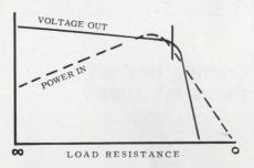
Line regulation is  $\pm$ 3%, 105-129 volts (Input 105-129 v. RMS 60 Hz). Load regulation is less than 20%, 0-5 ma., and ripple is less than 2% RMS.
