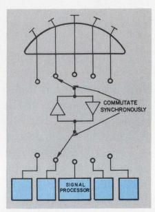
1. **Background clutter is reduced** with this phased-array setup that can scan 360° without a moving beam. A multiple-beam approach is used. Note that each radiating element in the diagram is a complete beam-forming antenna.
