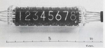
**Eight digits in one readout tube.** Nippon Electric is also demonstrating a 12-digit model.
