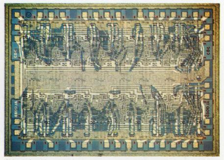
**Chip made with standard-cell** techniques marks Fairchild's entry into the field of bipolar Micromosaic. By March, the company expects to have enough cells in its library to implement 75 to 80% of all customer designs in Micromosaic, and 95% by the end of the year.
