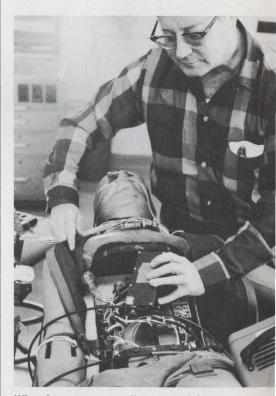
What happens to a pilot ejected from his aircraft at the speed of sound? This transducer-equipped dummy will be blasted off a rocket-propelled sled to find out.
