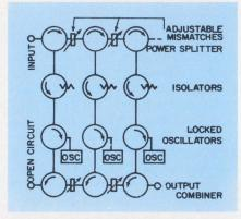
2. All paths from input to ouput have the same electrical length. Adjustable mismatches in the combiner allow for diode differences.
