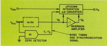
3. Integrating converter is sensitive to clock and signal frequency variations.
