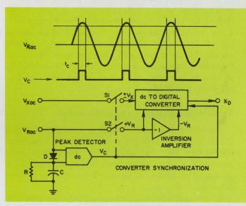
2. Single-phase sampling converter provides input signal noise rejection and high speed.
