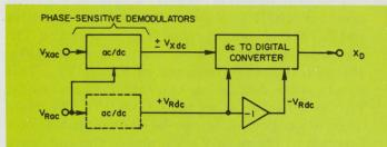
1. Asynchronous converter uses off-the-shelf hardware but is relatively slow.
