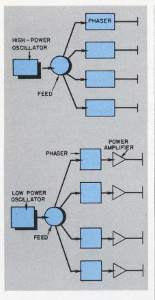
2. Two approaches for generating the power: the "big bottle" approach (top) and the individual-amplifier approach (bottom). The relative costs of high-power phasers and power amplifiers will determine the best way to go.
