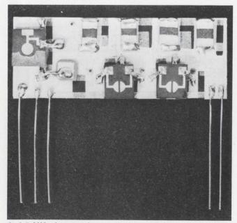
A 4.5-MHz intercarrier sound i-f module, using ceramic filters based on the energy-trapped mode, is being offered to TV manufacturers by Murata Manufacturing Co., Nagaoka. The hybrid offers 40-to-46-dB gain with more than 70-kHz bandwidth.
