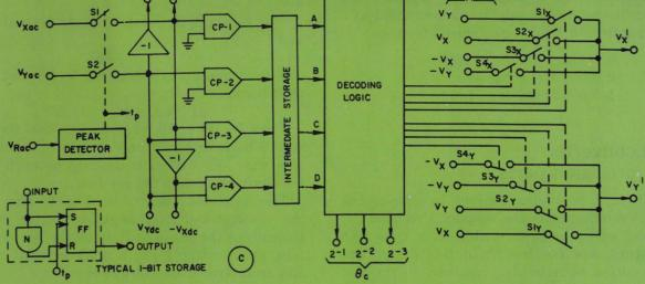
8. **Octant selection circuits** use phase-sensitive demodulators (a) for converting resolver outputs to dc. Sampling technique (b) provides octant selection with inputs applied
