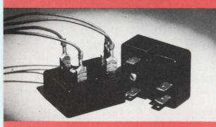
The Quick Connect thermal relays are designed to withstand the most demanding industrial applications. They reduce installation time and cost. Require only two mounting screws. Eliminates need for brackets, sockets, retainers. Features: time delays, 2 to 180 sec.; contacts, SPST, NO/NC; heater voltages, 6.3, 26, 115V AC or DC; resistive rating, 2A 115V AC or 1A 28V DC; mounts in any position.
