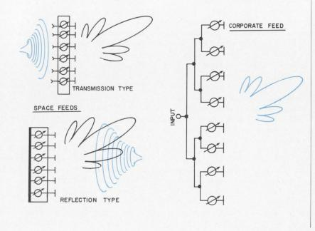
Both types of space feeds have a common problem: They take up a lot of room. Typically, optical considerations make it necessary to have the distance from the feedhorn to the aperture about equal to the aperture diameter.
