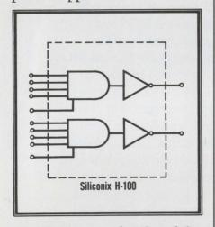
The H-100 was developed for use with noisy aircraft and marine power supplies; output drives 100 mA and sustains 90 volts. Available in TO-86 or TO-116 packages. Write or call today for the data sheet on the Siliconix H-100!
