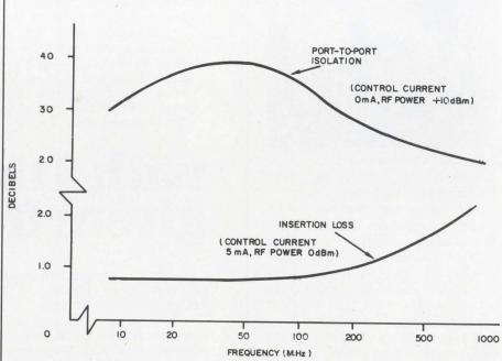
**Spanning the frequency range of 10 to 1000 MHz**, the model SB-1 low-cost miniature rf switch minimizes its insertion loss (1 dB typical) and maximizes its port-to-port isolation (over 30 dB typical).
