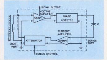
2. Impedance converter allows transformed value of C to appear across L. Two such units—one for the antenna coil, one LO—go into an a-m receiver.
