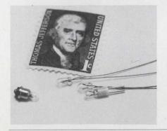
Low-voltage neon lamps generate HV internally
