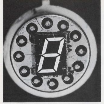
This seven-segment, solid-state GaAsP array by Hitachi requires only 85 mW per digit.
