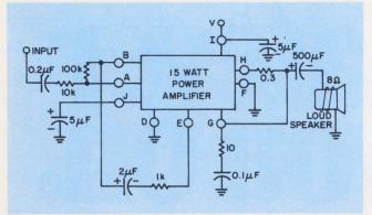
1. Typical connection using a high-power IC in an audio system. Motorola plans to market a 15-W, IC amplifier on a  $74 \times 75$ -mil chip within a year.
