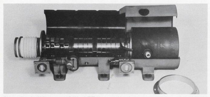
Cutaway view of a high-power, pulsed, X-band TWT by Hughes Aircraft Co. A heat pipe surrounding the tube
