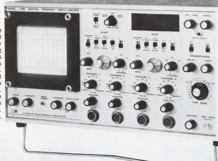
Four-channel oscilloscope with digital readout and a four-trace display allows simultaneous viewing of inputs and outputs from digital ICs or flip-flops. This new instrument also features a bandwidth of greater than 1 GHz. Waveform voltage measurements can be made on any one channel. See p. U140.
