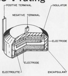
**Electrochemical capacitive device,** about the size of a poker chip, uses pressed-wafer construction to achieve capacities of 50 F at 0.5 V.
