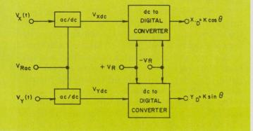
5. Elimination of octant selection circuits is the major advantage this asynchronous sin/cos converter gives.
