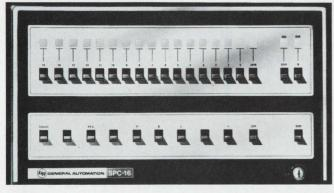
It's the SPC-16...a powerful new industrial automation computer ... 960 nanoseconds fast... expandable 4K memory.
