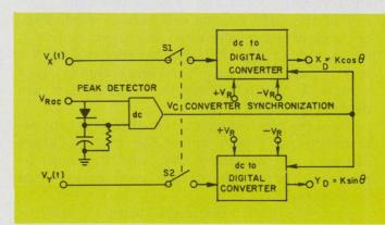
6. Sampling sine/cosine converter design allows a reduction in hardware requirements.
