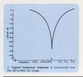
For this particular network the switching pulse length was fixed at 2.5  $\mu$ s, and the frequency adjusted over the range 10 to 200 kHz; the lowest switching frequency being more than 10 times greater than that of the highest frequency handled by the filter. The resonant frequency for the filter is given by:
