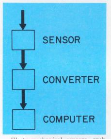
Electromechanical sensors, such as linear transformers, resolvers and synchros, are commonly used in control systems because they provide precision and economy. With the application of digital computers in control systems, simple and accurate methods for converting the ac outputs of these sensors into digital form become vital.
