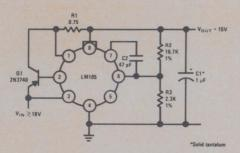
LB-10 IC REGULATORS SIMPLIFY POWER SUPPLY DESIGN Write: National Semiconductor Corp., 2900 Semiconductor Drive, Santa Clara, California 9505
