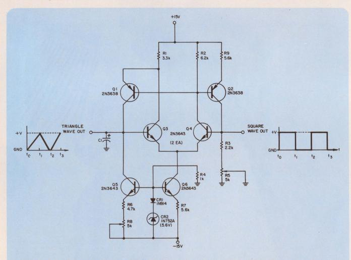
Low component count function generator simultaneously produces triangle and square waves.
