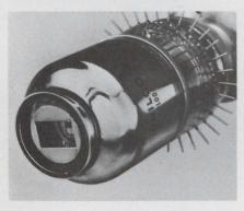
Because Philco<sup>®</sup> detectors are made entirely in-house. The whole assembly ... detector array, liquid nitrogen- or cryostat-cooled dewar with cooled filter, and matching current-mode preamp.
