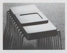
The Philco<sup>®</sup> MOS 1024-bit read-only memory has a *static* output data level. It remains valid as long as an address is present. That means you can address it as slowly as necessary to be compatible with your output device, and the extra expense of clock generators and drivers is eliminated.
