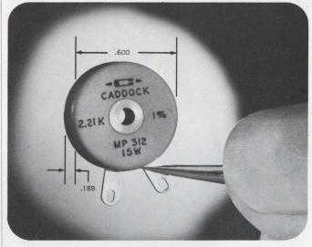
CHASSIS-MOUNT TYPE • NEW LAMINAR DESIGN • LOW PROFILE . 50% REDUCTION IN SIZE AND WEIGHT . COMPLETELY NON-INDUCTIVE . T.C.: 50 PPM/°C . **RESISTANCE TOLERANCE:** ±1%
