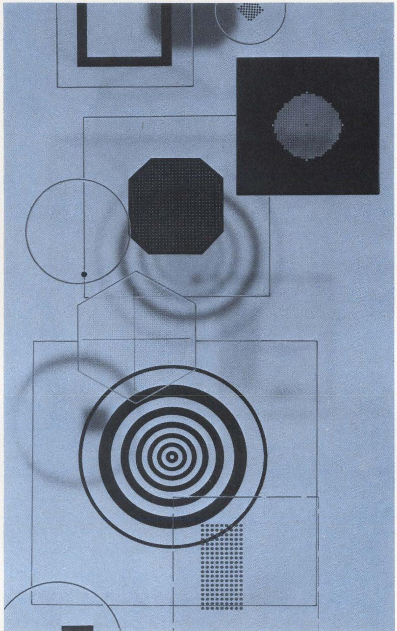
Up to now the only kind of glass master available for tooling had an emulsion coating that usually scratched after one or two uses. Costs to replace these emulsion masters were extremely high, and the production downtime to change masters was equally expensive.
