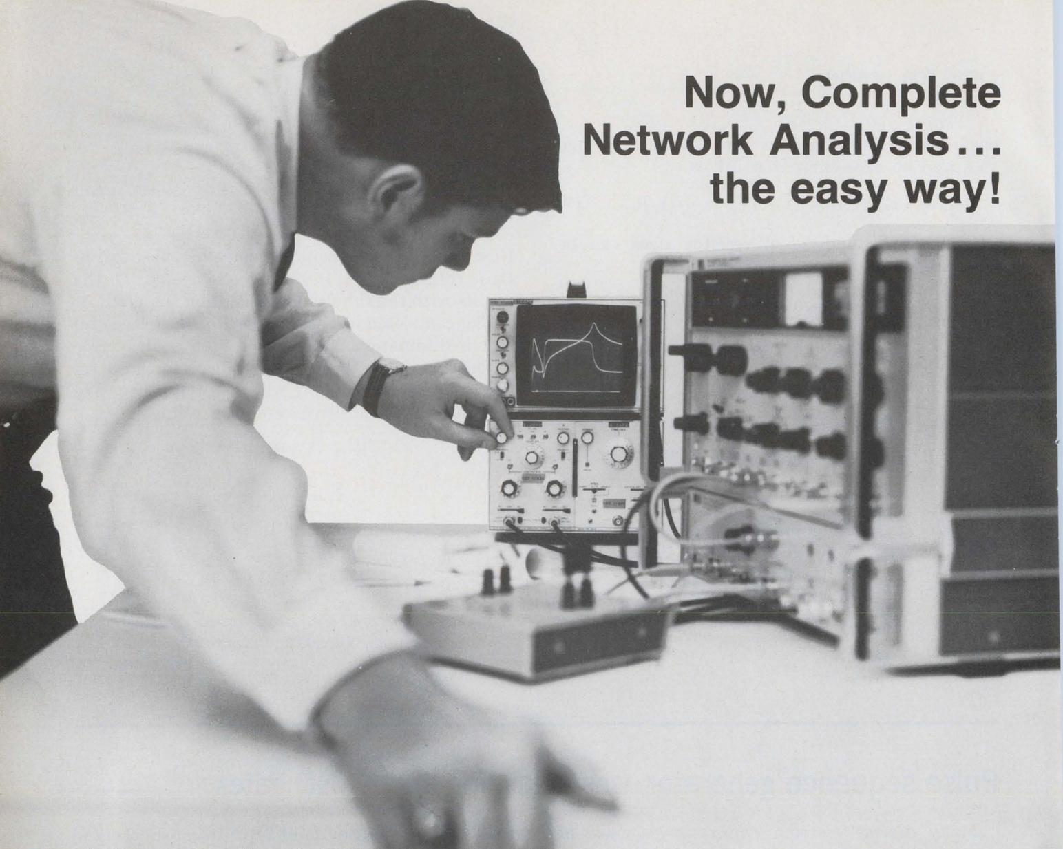
**Get amplitude, phase and complex impedance measurements on a swept basis to 32 MHz... automatically with the HP 675A/676A network analysis system.**
