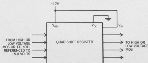
General Instrument's 4-bit byte 25-bit and 32-bit QUAD Static Shift Registers are the newest additions to the growing family of GIANTS. And, like all GIANTS, they are products of General Instrument's exclusive MTNS (Metal-Thick Oxide-Nitride-Silicon) process.
