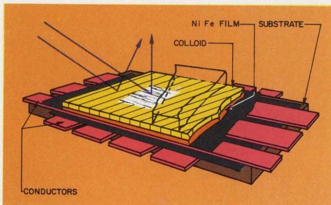
**Magneto-optic display** acts similarly to a diffraction grating. Display reflects light from external source. Magnetic particles create strain lines.
