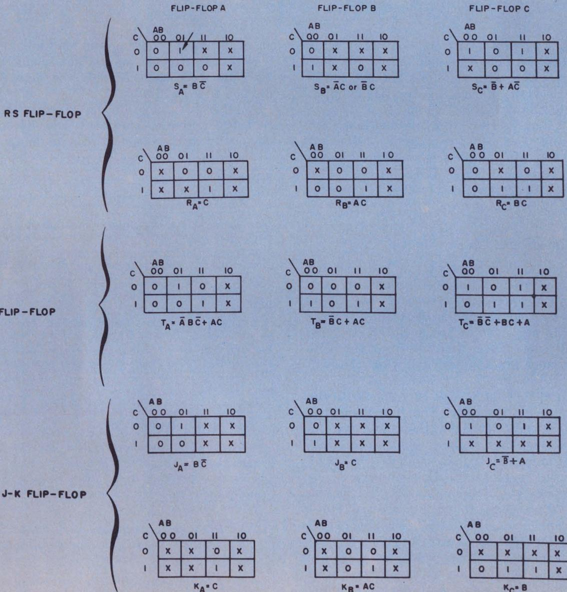
5. The three flip-flop sequential counter flow table (Fig. 3) translates into this multiple set of maps.
