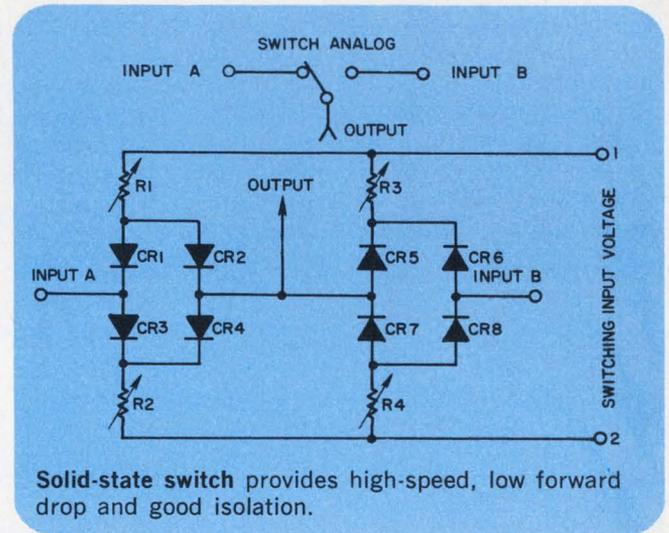
signal at input B is therefore disconnected from the output.
