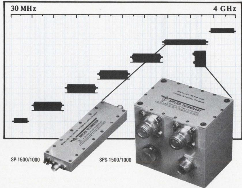
The SP-1500/1000 L-Band preamplifier is now available with an integrated power supply for direct TWTA replacement. Designated the SPS-1500/1000, the unit covers the frequency range from 1000 to 2000 Megahertz. Microstrip construction of the all solid state design permits significant reductions in size, weight, power consumption, and heat dissipation.
