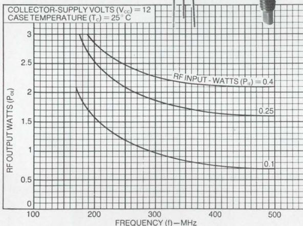
Headed for an important role in mobile and portable communications equipment, the high-gain RCA-TA7477 is now available in production quantities. This silicon n-p-n "overlay" transistor, designed for 12 V service, also is capable of 2 W minimum output at 470 MHz (7 dB gain). It is intended for Class C vhf/uhf amplifier service in CB, sonobuoy and beacon, as well as other mobile and portable applications.
