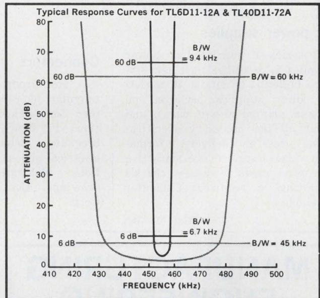
Here's the smallest (less than 0.1 cu. in.), most rugged fixed-tuned filter of its kind on the market today!
