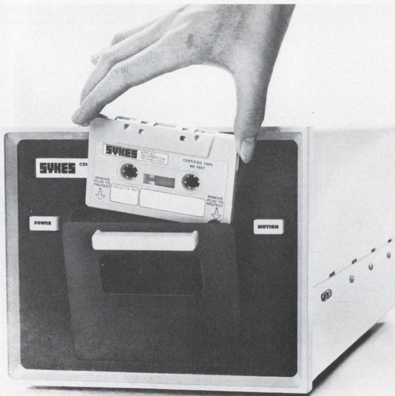
One of several cassette data recorders on view was this Compu/Corder 100. The tape is computer grade and has a preformatted address track.
