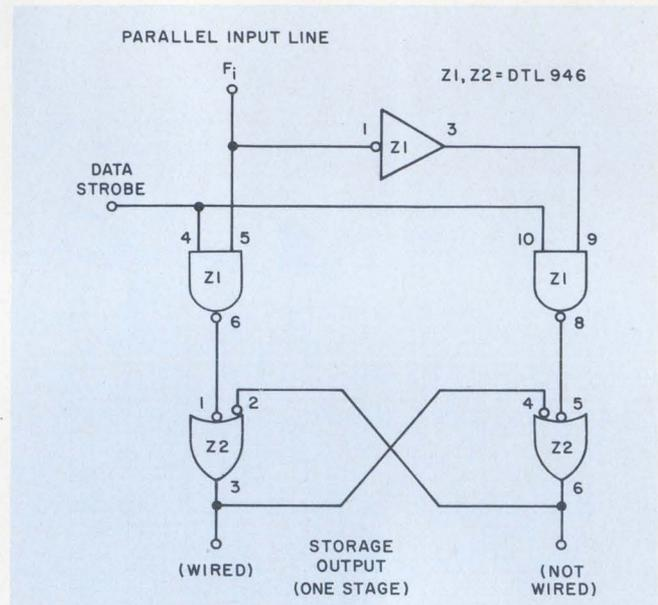
13. Two DTL 946 packages make one stage of an n-bit storage register. This is the register used in the parallel-to-serial converter of Fig. 15.
