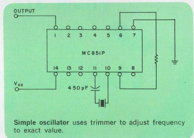
Typically, the free-running frequency without any crystal is about 1.6 MHz.
