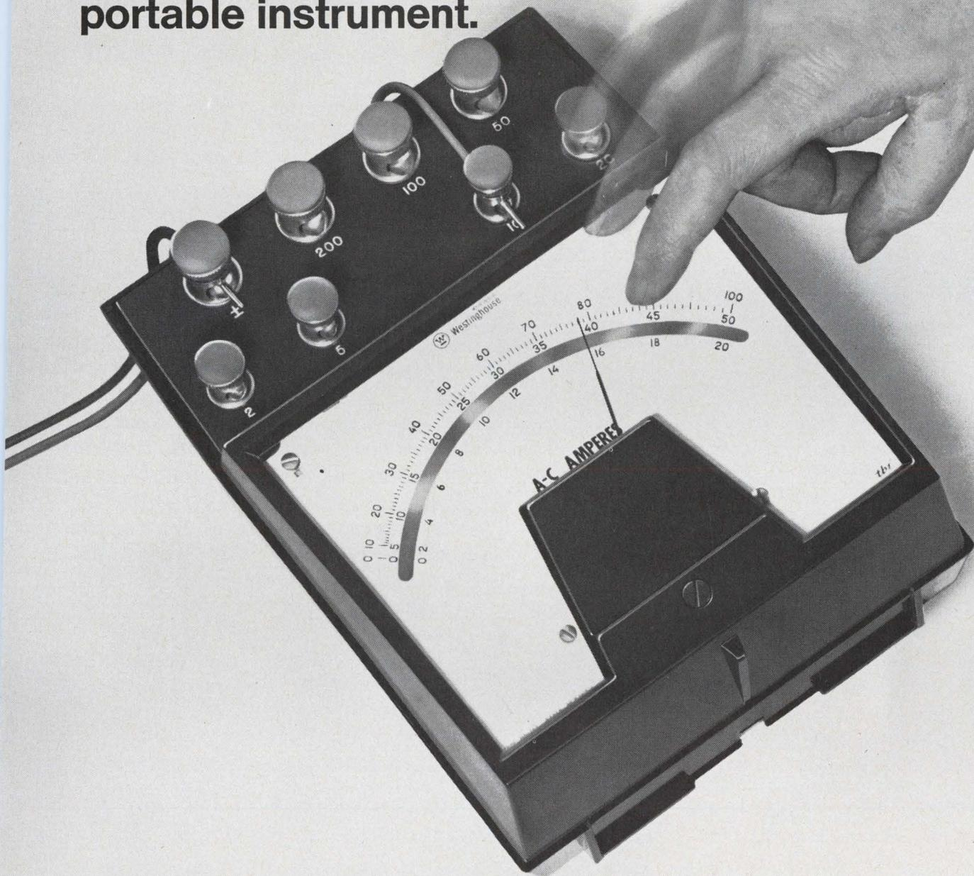
Westinghouse taut-band suspension instruments have no repeatability error because there is no pivot friction, no roll-in jewel error, and no measurable hysteresis in the taut-band materials.
