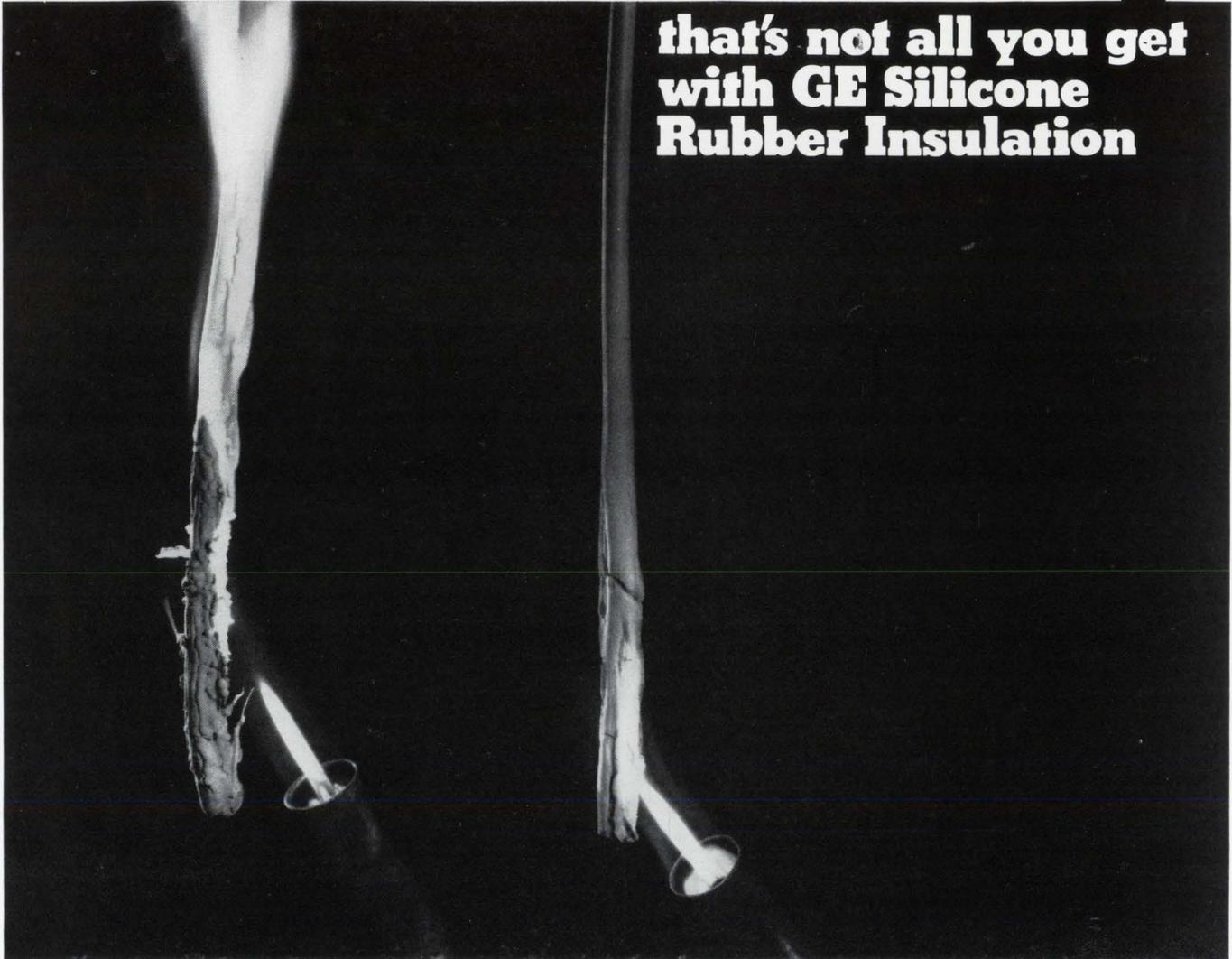
*New ultra-tough SE-9090 braidless wire and cable insulation (right) doesn't support combustion like conventional insulation. It's shown here passing the UL vertical flame test. SE-9090 has both outstanding insulation resistance and dielectric strength.*
