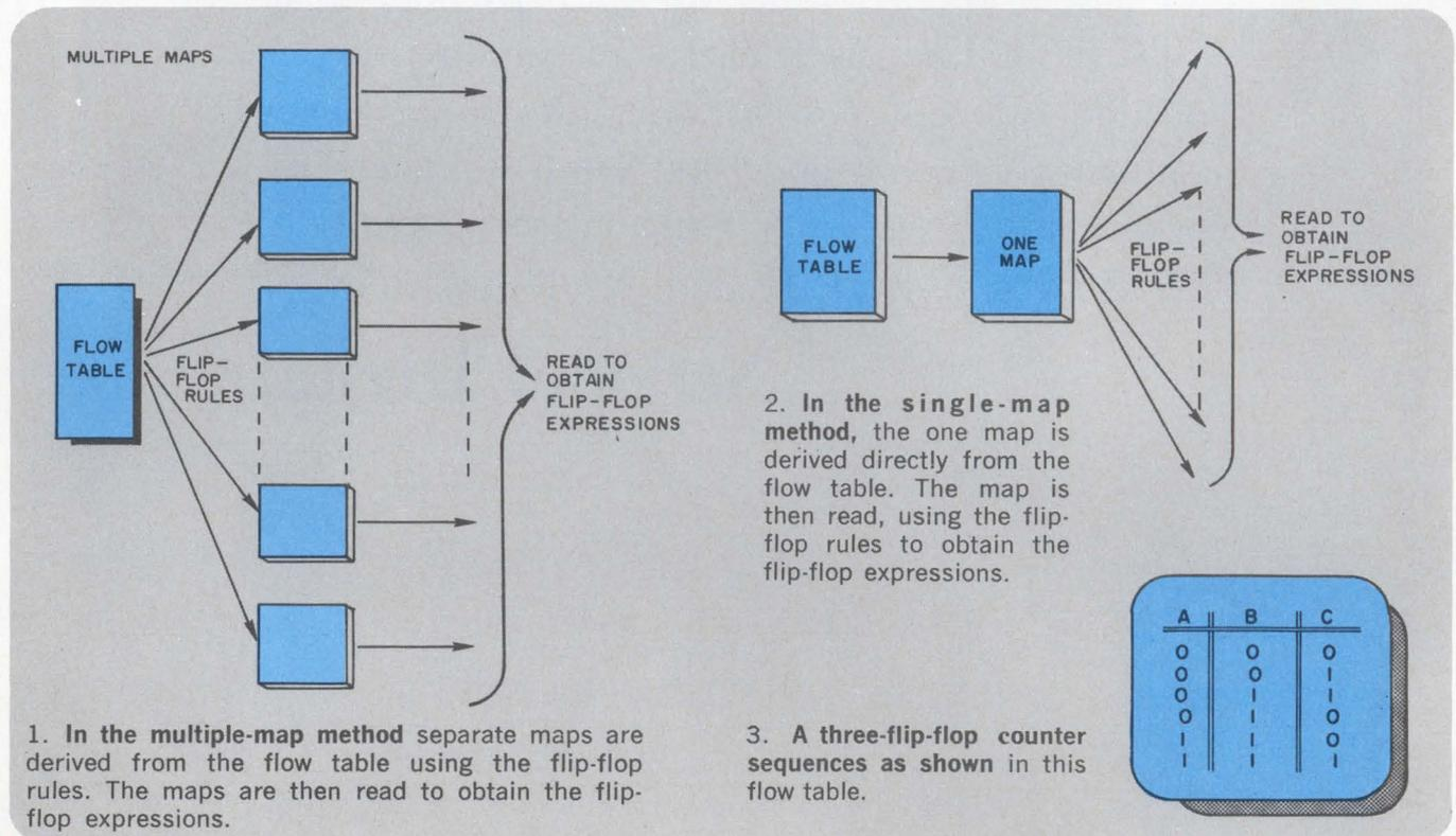
with the flip-flop rules, determine the map entry, which can be 0, 1 or X.
