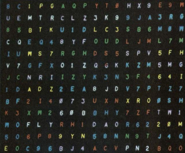
Chart used to test color and resolution of images for large-screen displays at Rome Air Development Center.
