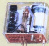
**Small, variable time delay will switch 4 PDT at 10 amperes**
