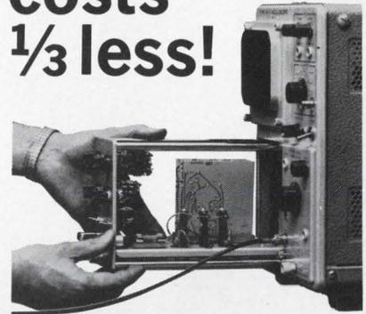
With U-Tech's plug-in and console units, any X-Y oscilloscope becomes a curve tracer displaying the dynamic characteristics of both NPN and PNP transistors, N Channel and P Channel junctions, FET's, MOS-FET's, bipolars, unijunctions, diodes, tunnel diodes and SCR's. You have curve tracer capabilities, without buying a complete curve tracer unit. In so doing you pay up to:
