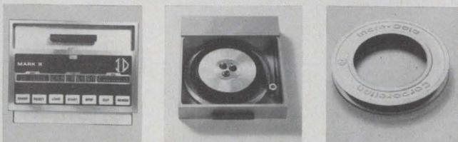
The Mark II incremental digital data acquisition system is 6¾" high, 7¾" wide, 13½" deep and weighs 29 lbs. Cartridge loading simplifies operation; computer-compatible magnetic tape speeds mission analysis. FOR INFORMATION ON MARK II contact Incre-Data Corporation, 6401 Acoma Rd., S.E., Albuquerque, New Mexico 87108. AC 505 265-9575.
