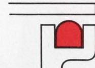
CONSIL® — "D" shaped strip gaskets seal and shield.
