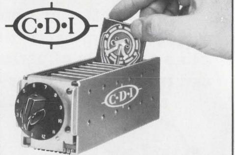
For critical reliability applications. Meet MIL-S-22710. Removable wafers permit quick changing of programs, configurations, circuits. CDI patented switches with dust covers available in sizes 2" x 2", 3" x 3" and 4" x 4" with lengths to accommodate up to 36 wafers. Operation may be manual, motor or solenoid.
