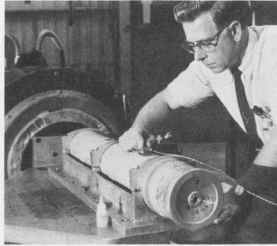
of its Mach 3 supersonic wind tunnel, and to bond piezoelectric accelerometers to test specimens made of aluminum, magnesium, steel or glass.
