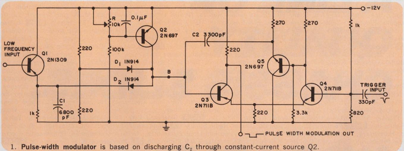
1. Pulse-width modulator is based on discharging  $C_2$  through constant-current source  $Q_2$ .
