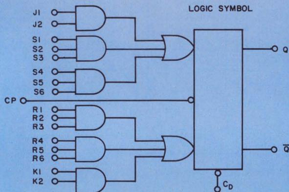
4. The multifunctional flip-flop has a more complex master latch circuit, controlled by a group of set gates and reset gates. The number of sources which control the master latch is thus greatly increased. The operation of the flip-flop is described by the truth table, which indicates that the set and reset condition may come from three sources, as controlled by the 2- and 3-input AND gates. This type of circuit is commonly used in shift-left, shift-right parallel load registers.
