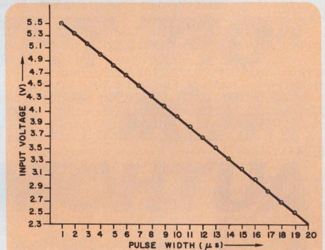
2. Linearity of output pulse width is within 2% of the maximum pulse width.
