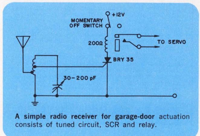
A simple radio receiver for garage-door actuation consists of tuned circuit, SCR and relay.
