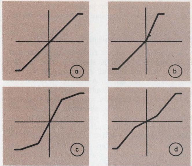
1. The dc transfer characteristics of op amps are seldom ideal, as in the linear transfer curve (a). Practical op amps have asymmetrical positive and negative gain (b), a decrease in gain near their output swing limits (c), a decrease in gain near zero output level (d), or a combination of these.
