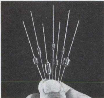
Ideal for network, filter, delay line and computer applications, 70F Series RF chokes give designers high reliability in a small package. Coils are impregnated with moisture resistant lacquer; can be fungus proofed or encapsulated on special order.
