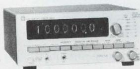
1192 COUNTER • dc to 32 MHz (to 500 MHz with scaler) • 10-mV sensitivity • crystal time base • 5, 6, or 7 digits and data output – \$575 and up.
