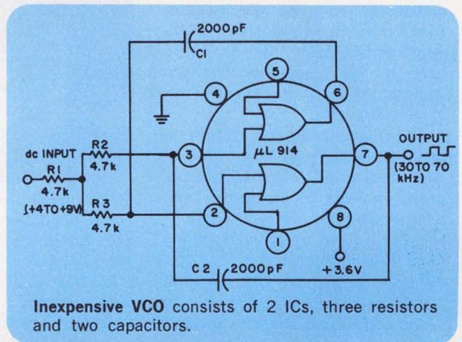
Inexpensive VCO consists of 2 ICs, three resistors and two capacitors.
