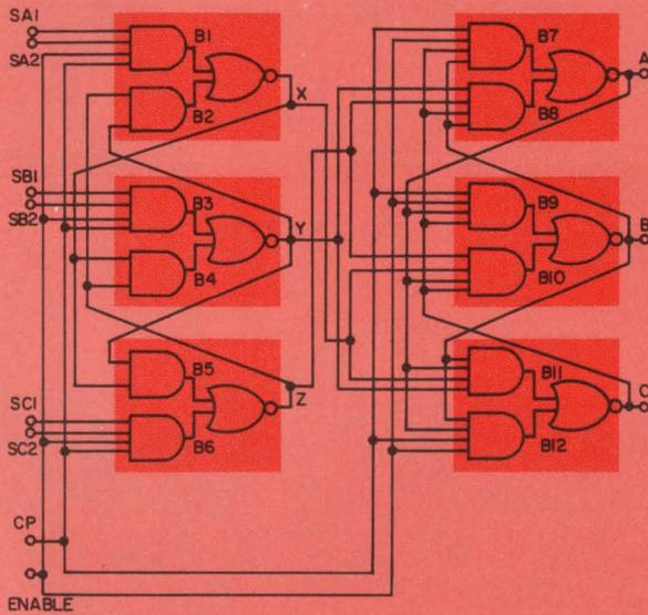
3. The tristable flip-flop is an interesting variation of the J-K flip-flop. Its three stable states result in an unconventional but potentially cost-saving design. When both inputs of an AND gate are at logic ONE, the selected state is obtained on the ONE to ZERO transition of the clock. The three stable states are 011, 101, 110; when the selected output is LOW, the other outputs are HIGH. A synchronous entry truth table and a logic symbol are derived from the sequence table.
