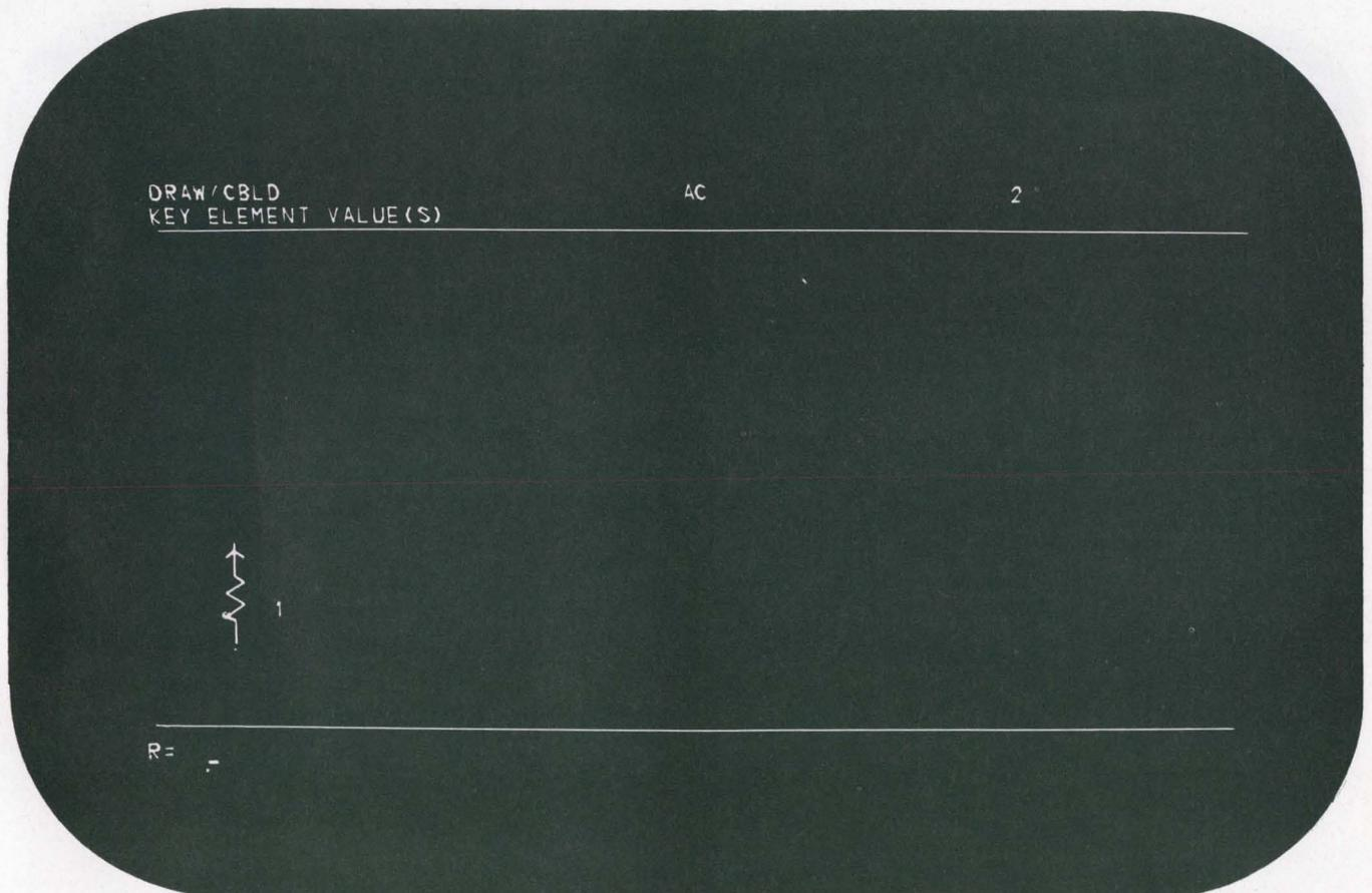
3. After a resistor is selected for branch 1, the display looks like this. The terminal requests a value for the resistor, and the user enters the value using the keyboard.
