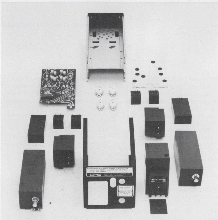
Dynamic-focus CRT supply can modulate high voltages from dc to 100 kHz. This compact unit delivers an output of 1 to 5 kV at 2 mA. It is constructed of interlocking epoxy blocks with no soldered connections.
