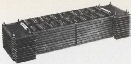
Perfect for high speed, large capacity mainframe memory systems... **NANOSTAK 3020**...technology breakthrough in 3W, 2-1/2D stacks. Stackable, compact size is an amazing 25% of competitive planar stacks and offers a significant advantage in form factor for system packaging. Extremely fast 650 nanosecond cycle time for 8K or 16K by 40, or 32K by 20 word memories.
