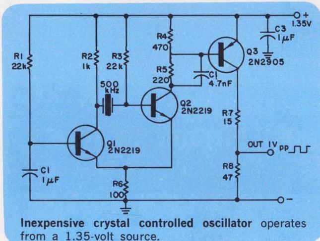
Inexpensive crystal controlled oscillator operates from a 1.35-volt source.
