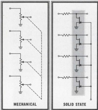
These quad VCRs are specially matched to give close tracking over the specified resistance range. Others: Single and dual voltage controlled resistors (VCR10N, VCR11N) for many applications such as multipliers, phase shift circuits, attenuators, feedback resistors in variable gain amplifiers or . . . what have you?
