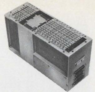
Compact, ATR compatible memory system **SEMS-6** for use in military and rugged commercial aircraft applications. Reliable performer is optimized around 8K or 16K with maximum capacities of 8K by 40 or 16K by 20. Full cycle time of 2 microseconds, with access time of 700 nanoseconds. Meets MIL-E-5400, low power consumption and lightweight.
