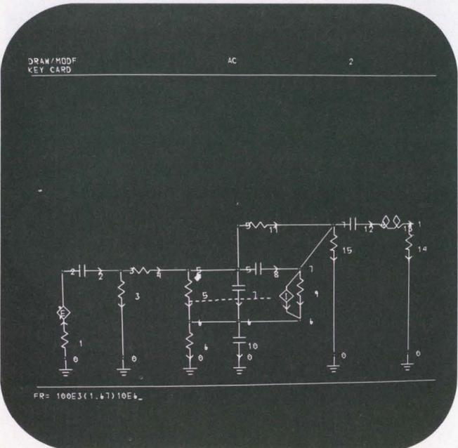
13. A frequency response plot is now requested by detecting FREQ from menu items. When values are asked for, the user keys in 100E3 (1.67) 10E6. Translated, this means a frequency response from 100 kHz to 10 MHz with each frequency in the plot 1.67 times the previous one.
