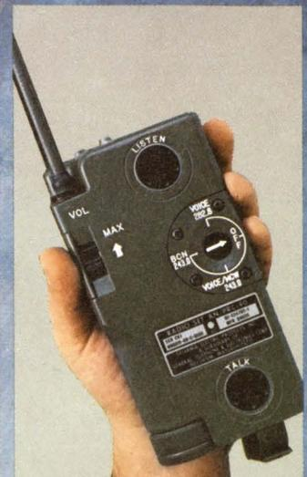
Sylvania AN/PRC-90 dual channel rescue transceiver permits two-way voice communication, the transmission of Morse code or the sending of a homing beacon.
