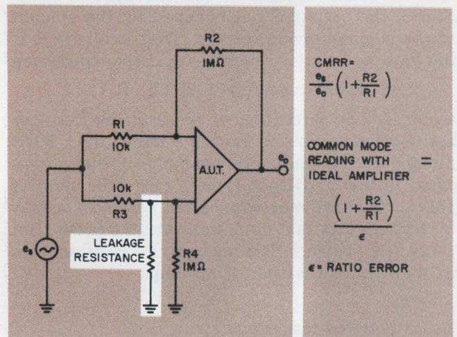
2. This CMRR test circuit requires careful matching of resistor ratios  $R_1/R_2$  and  $R_3/R_4$ , but leakage effects make close matching difficult. Matching error must be less than 0.01% for the circuit to be practical.
