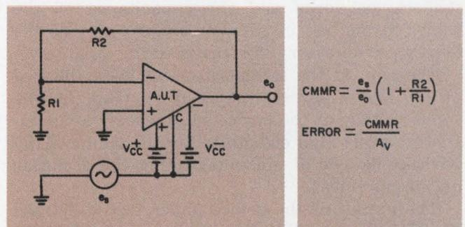
3. Error is inversely proportional to gain in this CMRR test circuit, which limits its usefulness to op amps with comparatively high gain ( $1 \times 10^6$ ) and low CMRR ( $1 \times 10^5$ ).
