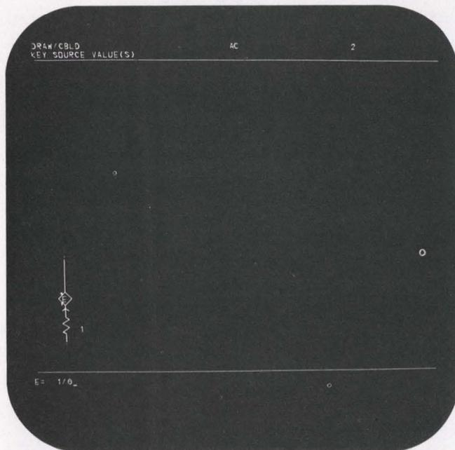
5. The computer requests the value of the voltage source, and the user keys in 1.0 V at zero phase.
