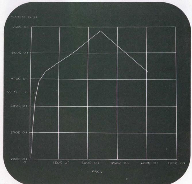
15. The computer plot of the voltage across branch 14 has approximately 14 frequency steps as a result of the choice of the frequency multiplier=1.67. The inductor of branch 13 is used as a parameter to vary the peaked frequency response. Here  $L=20 \mu\text{H}$ . The computer automatically selects the vertical and horizontal scales so the curve fills the screen.
