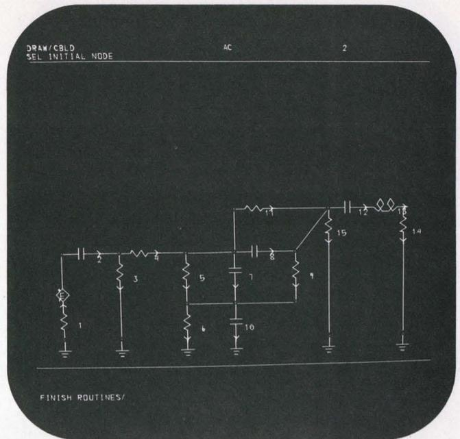
10. The passive part of the circuit is completed with the addition of the load components. The next step will be to put a current source in branch 9 dependent on branch 5.
