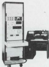
1790 LOGIC-CIRCUIT ANALYZER • tests logic circuits with as many as 96 inputs and 144 outputs • up to 4000 tests per second • GO/NO-GO or complete diagnostic testing • easy test language • autoprogramming lets the device determine proper outputs
