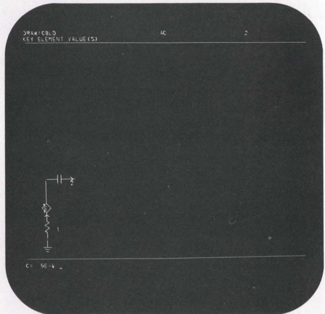
7. The next branch begins at the upper node of the first branch, and after selection of a 5  $\mu$ F capacitor the display looks like this.
