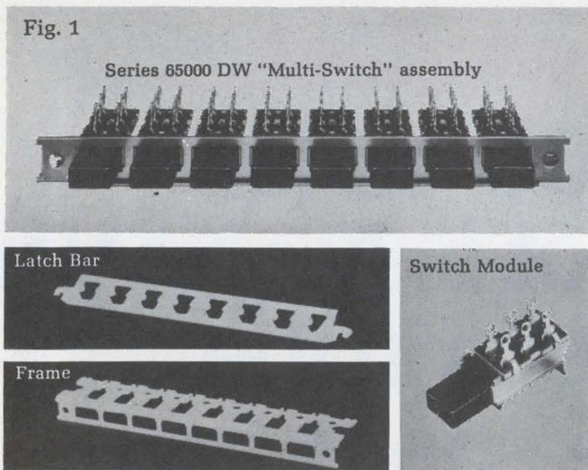
Fig. 1 shows how these elements are combined to complete the switch. The latch bar and mating actuator configuration determine the functional operation, such as: Interlock, All-lock, Non-lock, and even special functions. The push-to-lock, push-to-release function is also available and can be combined with Interlock, All-lock, Non-lock on the same switch frame without any interaction between the various functions.
