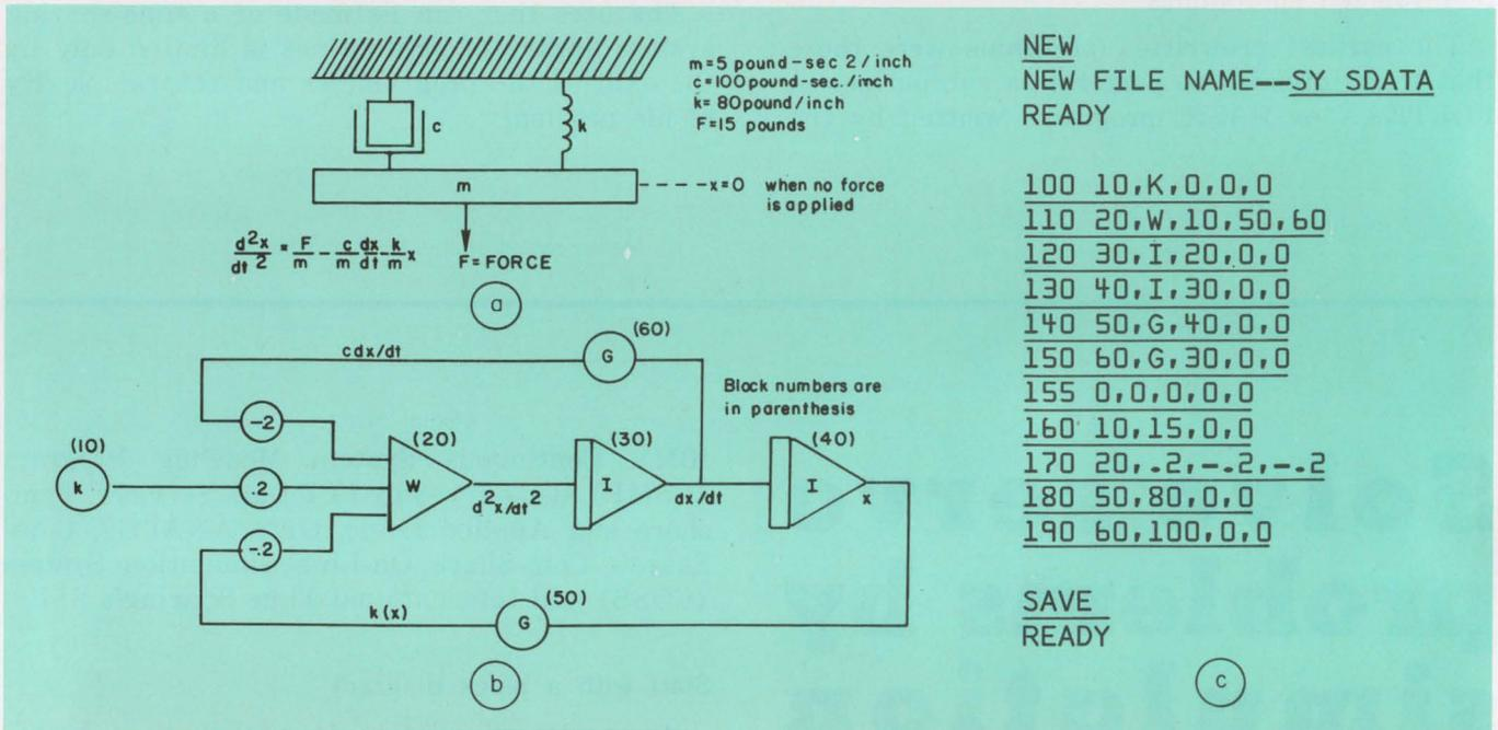
4. A simple resonant mechanical system is described in (a). A block diagram of the system is drawn in (b) as the first step in using an ANALG\$ simulation. Block K is a constant; I is an integrator; G is gain; W is a
