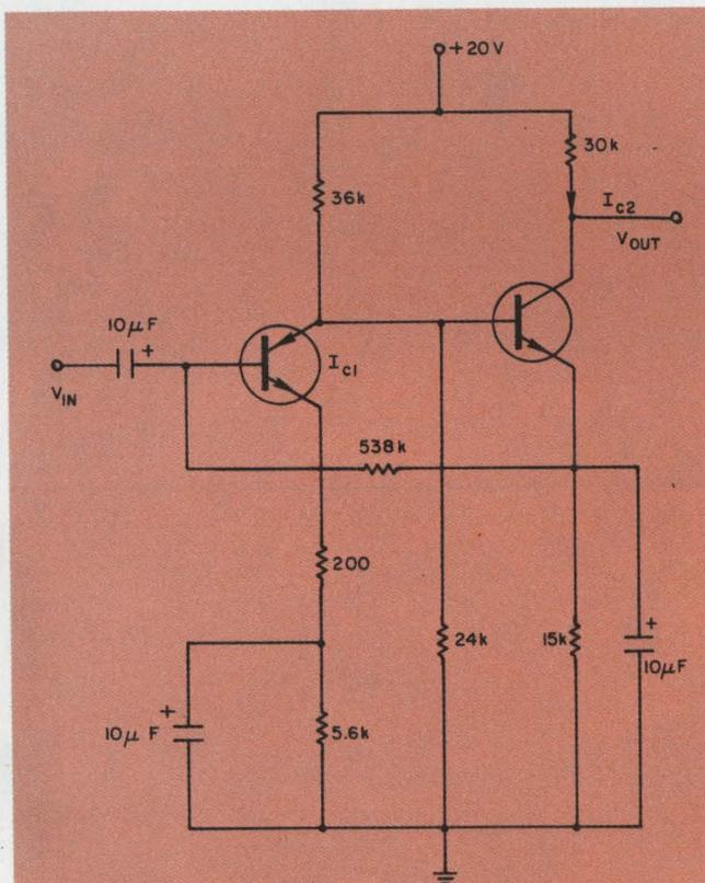
5. A current-feedback pair amplifier using a 2N2060B dual transistor has an  $I_{c2}$  drift of about 88 nA/°C, only a 4.5% change from the 250  $\mu$ A collector current from 25°C to 150°C. The kHz voltage gain is 76 dB.
