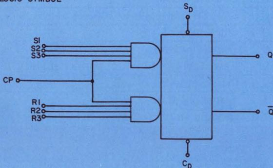
2. Two AOI gates form a gated latch. From the sequence table we note that the latch may be set when the S inputs are ONE (C<sub>P</sub> may be considered an S input) or reset when the R inputs are ONE, and that direct inputs C<sub>D</sub> and S<sub>D</sub> operate with logic ZERO levels. The truth table and logic symbol are derived from the sequence table. The gated latch is useful for general storage applications, where a full master-slave flip-flop is not required.
