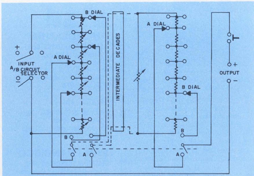
By using the same voltage divider resistor ladder for both A and B measurements, the potentiometer achieves an accuracy of 1 part in 100 million since deviations of the ladder's accuracy are kept common to both A and B.
