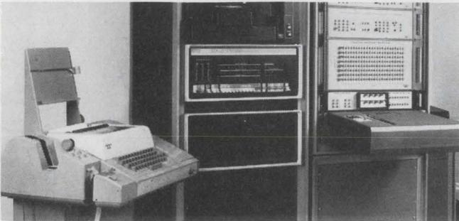
Picker uses its J259 to test circuit boards going into x-ray generators. The J259 whips through the 70 or 80 tests required on a board in a split second, automatically typing out the results of any test that is failed. Test data on a rejected board then accompanies the board to trouble-shooting, where a technician refers to his copy of the test program and keys the failed test to the bad component or connection.
