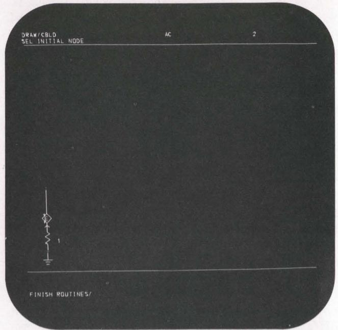
6. By detecting the bottom node with the light pen, and then GROUND from a new series of menu items (not shown here) a ground symbol appears. NEW BRANCH is then detected from the menu items, and this display then appears where the instruction, SEL INITIAL NODE at the top, calls for the initiation of a new branch.
