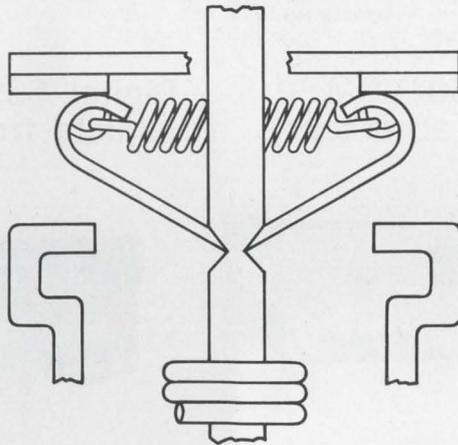
3. The contacts snap up into place and close the NO circuit. This positive snap action provides 120 grams of contact pressure and contact resistance below 10 milliohms—perfect for dry circuits.
