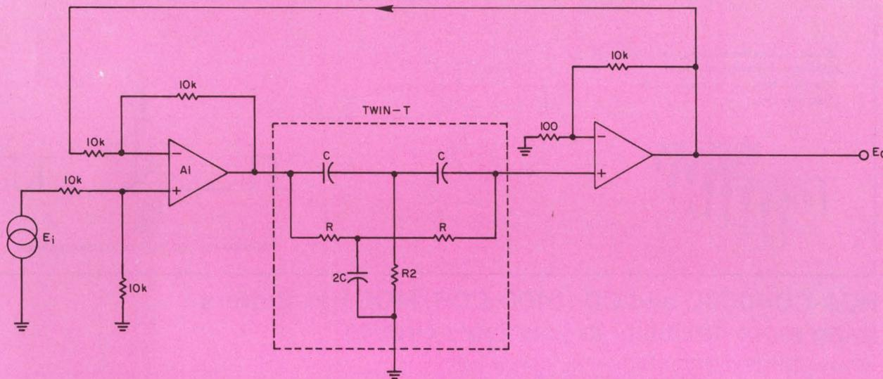
Narrow-band amplifier using twin-T requires two operational amplifiers.
