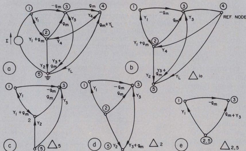
6. **The input impedance is found** by using the graph (a) to calculate the voltage at node 1. To evaluate  $\Delta_{i0}$ , the current source is open-circuited (b). The subgraphs  $\Delta_5$  (c),  $\Delta_2$  (d) and  $\Delta_{2,5}$  (e) are also shown.
