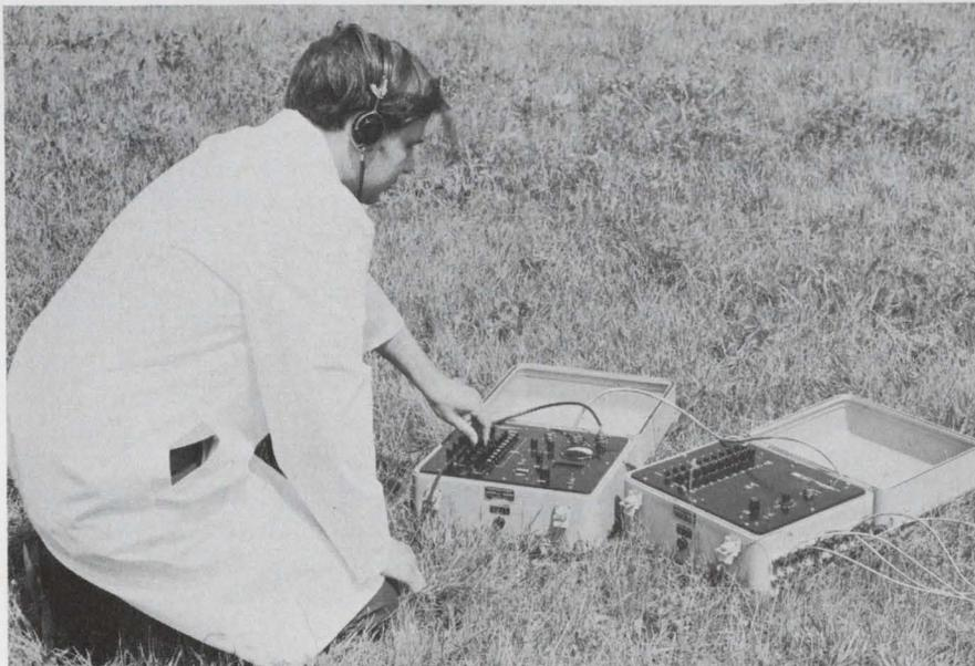
A 10-channel alarm system built by DEI Industries warns of intruders within a 3.6-million-square-foot area. Called AIDS-10, the system employs buried geophone sensors that are linked by wire to a multiplexer.
