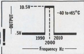
These new Go/NoGo completely solid-state Audio Switches fire whenever input frequency goes above, below or within definite frequency limits... as accurate as 1 cycle per thousand, with maximum response of 2 input cycles.
