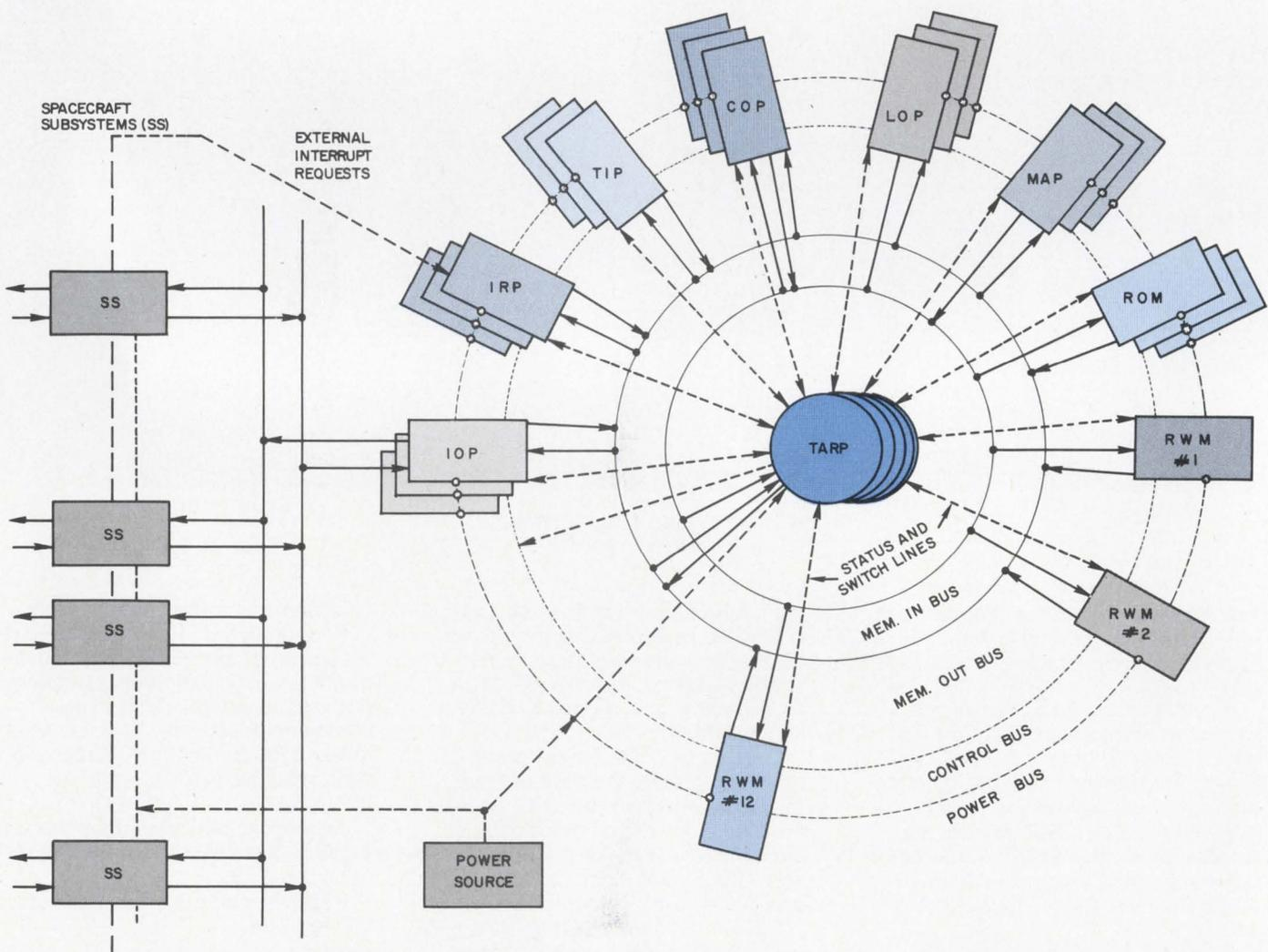
Self-testing and repairing computer (STAR) block diagram. The computer is essentially a replacement system. Test and repair processor (TARP) monitors status re-
