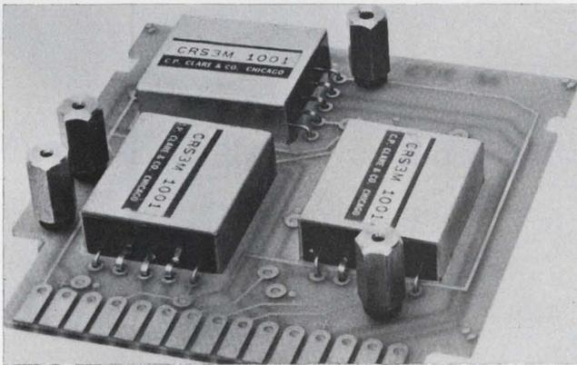
It is often necessary to coat PC board assemblies with encapsulant before final wiring is done. In such cases, there are a number of areas on the board that must be protected, or masked, from the encapsulating material to permit subsequent soldering of lead wires. Masked areas are also often necessary to permit electrical tests subsequent to encapsulation and prior to soldering of lead wires.
