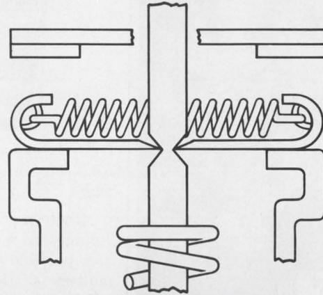
2. As the plunger is pressed down, the contact arms approach the trip position.
