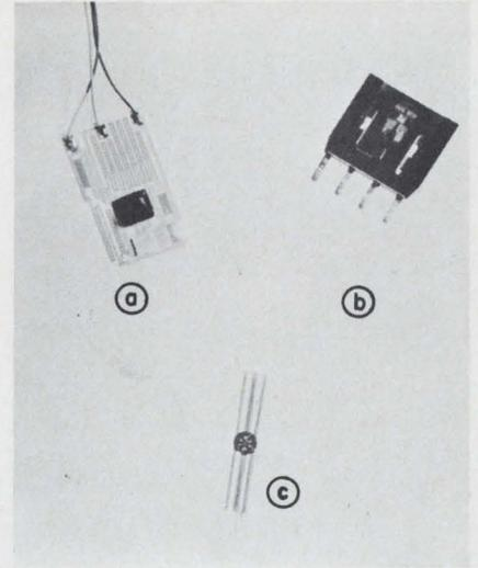
Latest magneto-sensitive devices include: (a) F. W. Bell hybrid switch assembly; (b) Honeywell Hall switching unit; (c) Hudson Magnistor.
