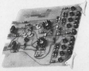
Gives on-axis linearity correction for geometric distortion occurring when a flat-faced CRT is used. Ideal for line-scan applications.
