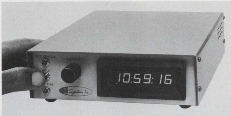
**Six-digit clock** improves display versatility with interchangeable light-emitting-film panels, p. 158.
