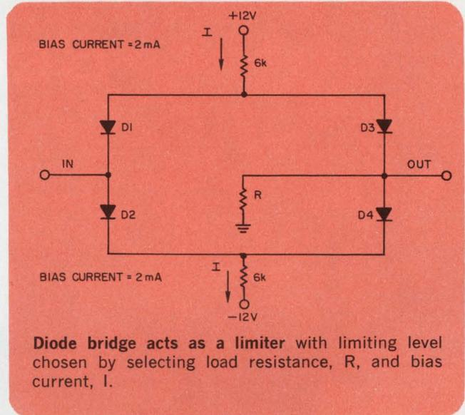
tortion below the limiting level will occur from dc to about  $1 \text{ MHz}$ . The limiting level is independent of temperature. The circuit has relatively low output and high input impedances.
