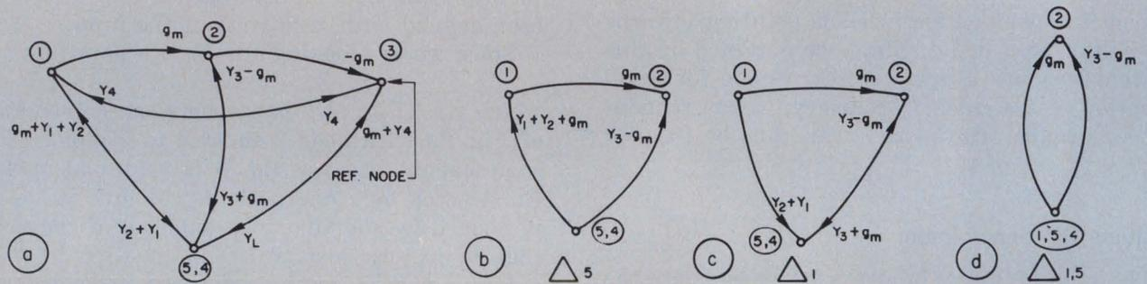
4. **To evaluate the denominator**, open-circuit all of the independent current sources and short-circuit all of the independent voltage sources. When this is done to the graph of Fig. 3a, the result is that shown in "a." The subgraphs  $\Delta_5$  (b),  $\Delta_1$  (c), and  $\Delta_{1,5}$  (d) are also shown.
