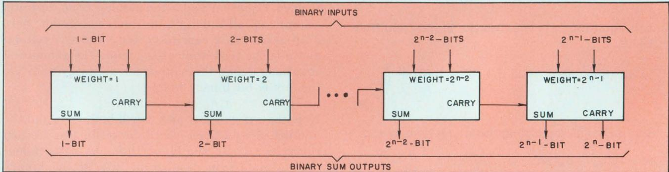
2. The standard binary  $n$ -bit adder is built from full-adder circuits. Although it offers a limited number of input lines, it can be modified to handle more inputs, if desired, simply by ganging adders.
