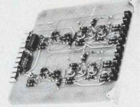
Converts X and Y deflection current samples into parabolic voltage wave forms to maintain beam focus anywhere on the CRT face.
