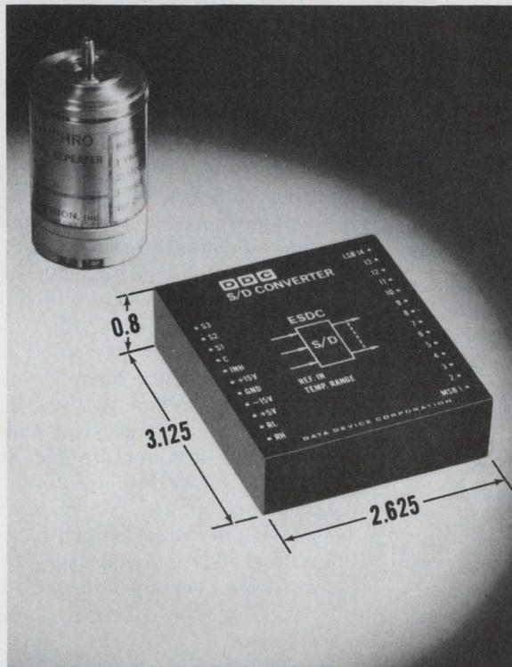
DDC has a new encapsulated module, only 6.6 cubic inches, which offers true 14-bit continuous conversion. The 8 ounce device, called the ESDC, has a specified accuracy of  $\pm 4$  minutes  $\pm 1$  LSB over the full operating temperature range. This spec takes into account all errors due to input rates to  $360^\circ/\text{second}$ , accelerations to  $20^\circ/\text{sec}^2$ , harmonic distortions to 10%, frequency variations to 10%, and amplitude variations to 10%.
