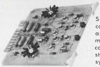
Supplies highly stable constant current to two axes of centering, alignment or static astigmatic correction coils in CRT, storage tube or vidicon systems.
