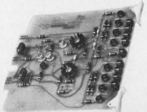
Gives on-axis linearity correction for geometric distortion occurring when a flat-faced CRT is used. Ideal for line-scan applications.
