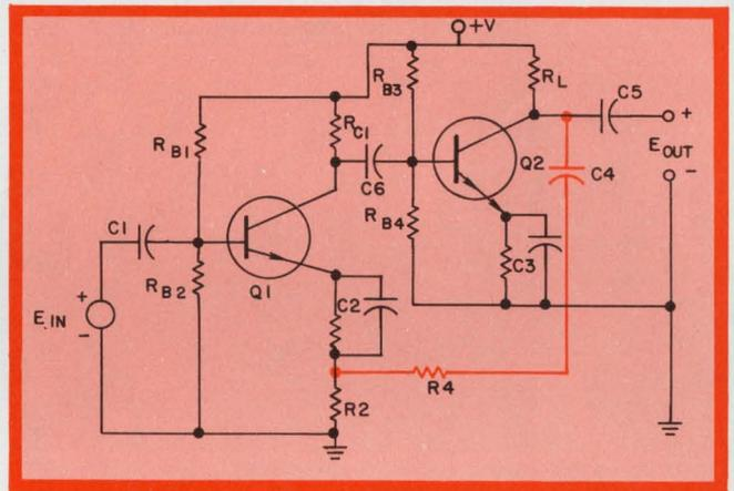
1. **Extremely stable gain**, high input impedance and low output impedance characterize this voltage-series feedback amplifier. It's called a voltage-series type because a portion of the output is fed back (via  $R_1$  and  $R_2$ ) in series with the input. When properly designed, the amplifier's gain is  $(R_2 + R_4)/R_2$ .
