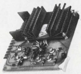
Provides a fully adjustable constant dc current supply to the static focus coil in magnetically focused systems. Low ripple, adjustable.
