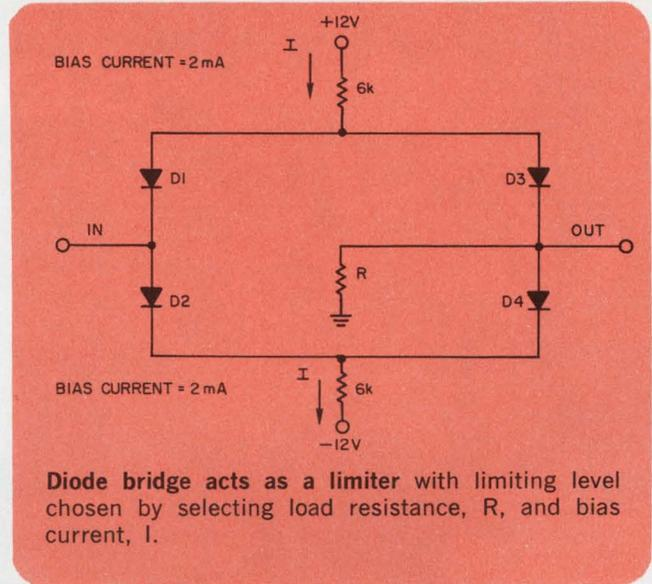
tortion below the limiting level will occur from dc to about  $1\ MHz$ . The limiting level is independent of temperature. The circuit has relatively low output and high input impedances.
