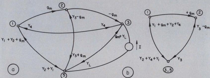
5. **The output impedance is found** from the graph of Fig. 3a by shorting node 4 to ground (a). Subgraph  $\Delta_{3S}$  (b) is also derived from Fig. 3a, but by grounding node 3.
