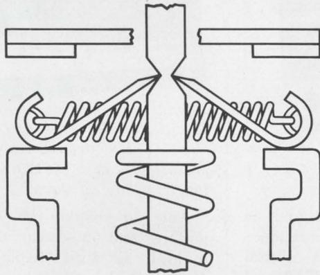
1. Let's start with the advanced switch mechanism design. In this position, the 2-circuit momentary contact switch, built to MIL-S-8805/3B, is not activated. Watch the action.
