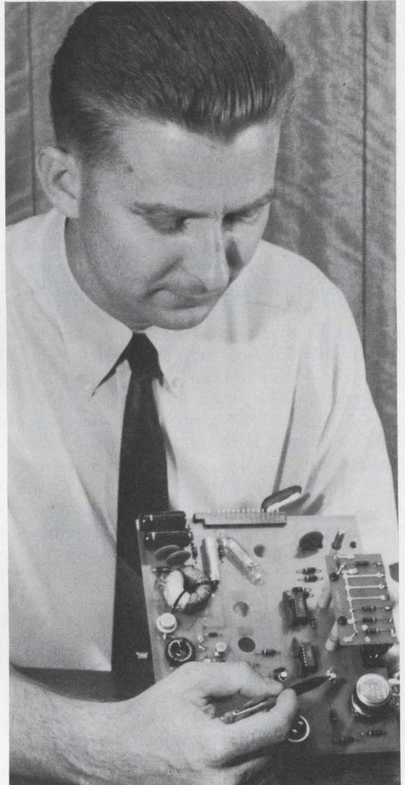
**Fred Palenschat points** to a dual JFET that provides low common-mode voltage to an IC amplifier's input. p. 86.
