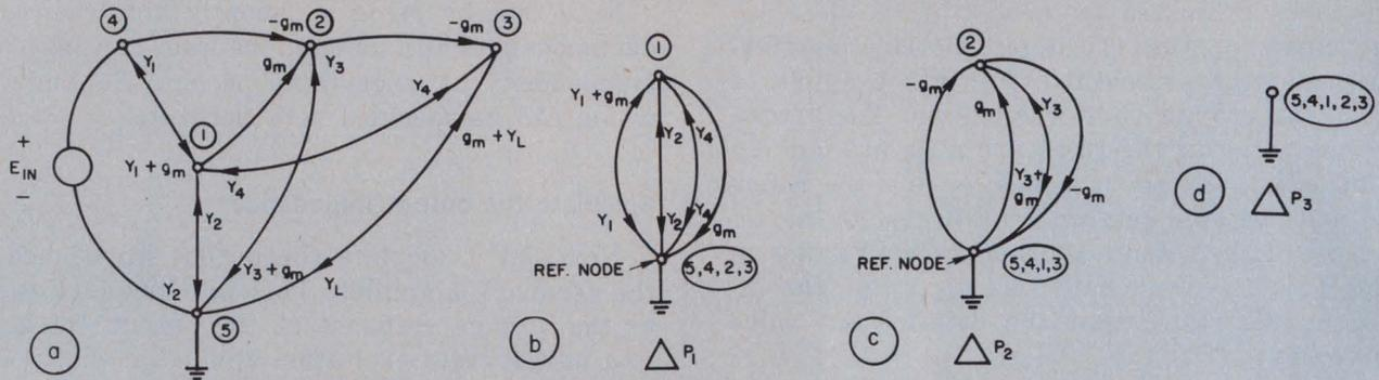
3. **Generating the network graph is the first step** in the analysis (a). The subgraphs for  $\Delta P_1$  (b),  $\Delta P_2$  (c) and  $\Delta P_3$  (d) are also shown. Note that subgraph  $\Delta P_3$  is only a single node. This has a value of unity.
