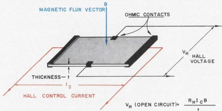
The Hall generator output is a voltage that is proportional to the product of magnetic field intensity and control current.
