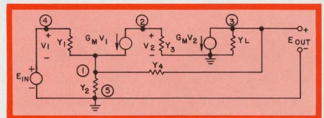
2. **This equivalent circuit** of the amplifier of Fig. 1 can be applied to other amplifiers with similar feedback and different biasing arrangements.
