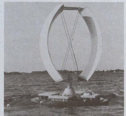
A robot sailboat developed by RCA can navigate itself unmanned by radio command to any point on the world's seas. The craft employs movable sails and rudders plus electronic navigation to proceed to a designated point. It will hold its station until commanded to move elsewhere.
