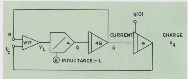
3. Converted into a block diagram for CSMP analysis, the R-L-C circuit of Fig. 2 appears in this form.
