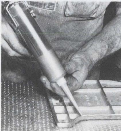
**Cheaper than gaskets.** GE RTV-109 silicone rubber seals plate assemblies of food slicer to keep juices out. Non-toxic, inert RTV-109 is applied easily, forms permanent, moisture-proof bond. Contact GE for FDA data on RTV-109.
