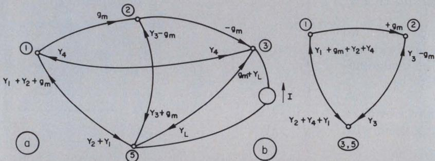
5. **The output impedance is found** from the graph of Fig. 3a by shorting node 4 to ground (a). Subgraph  $\Delta_{3,5}$  (b) is also derived from Fig. 3a, but by grounding node 3.
