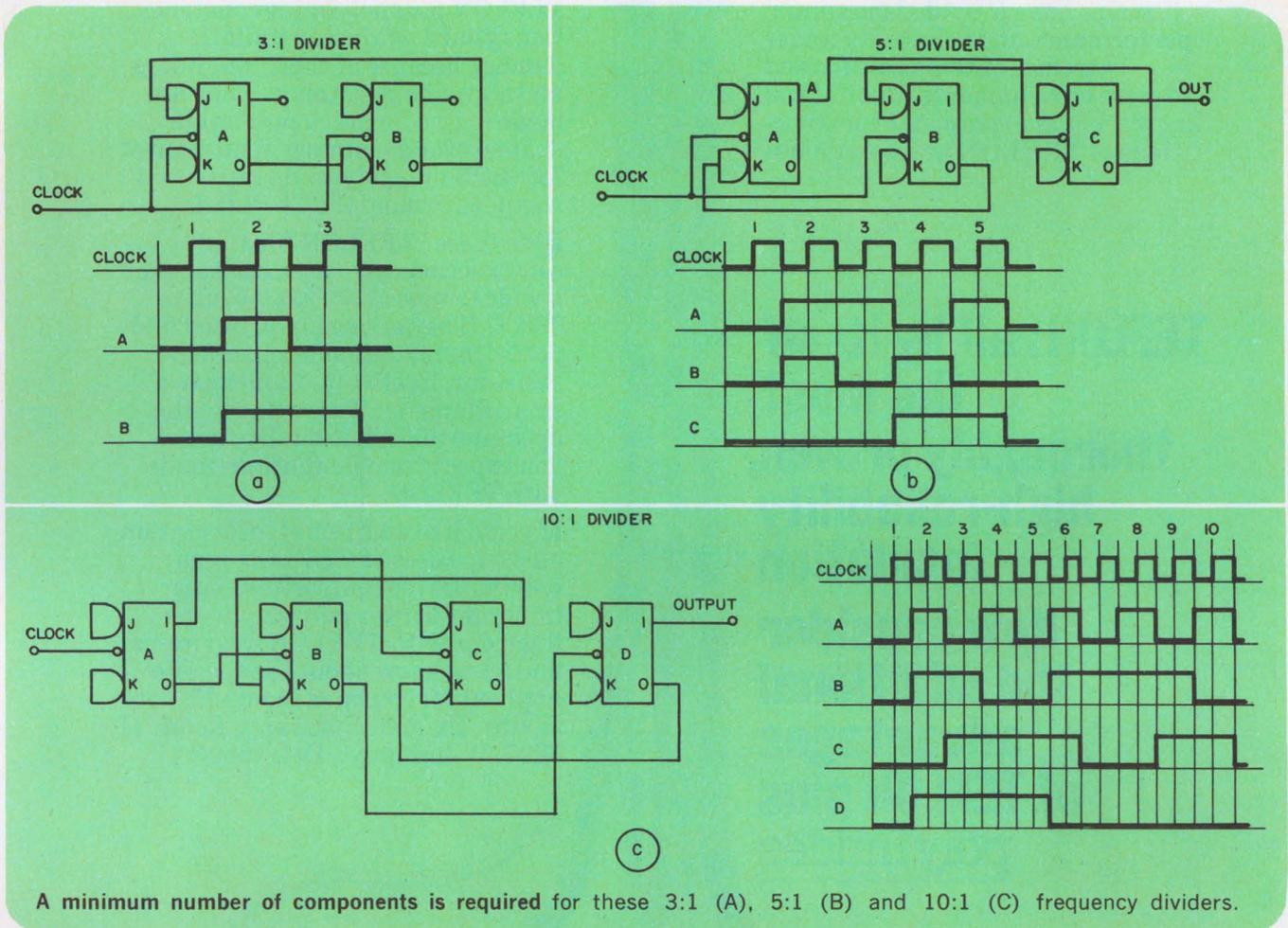
puts of J-K flip-flops. Minimum-hardware frequency dividers of this type for factors of 3, 5, and 10 are shown in the illustrations. These arrangements are suitable for either DTL or TTL
