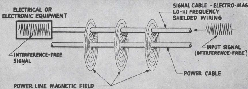
A new method of attenuating electro magnetic interference over an extremely wide frequency range 60 CPS to 10 KMC. Can be applied over power cable and assemblies to reduce noise.
