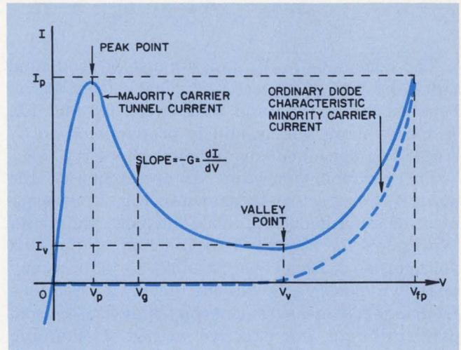
1. Static V-I characteristic of typical tunnel diode defines the curve that must be matched mathematically.
