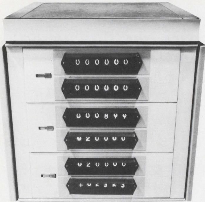
Indicator tubes—simple interfacing, limited flexibility, low in cost.
