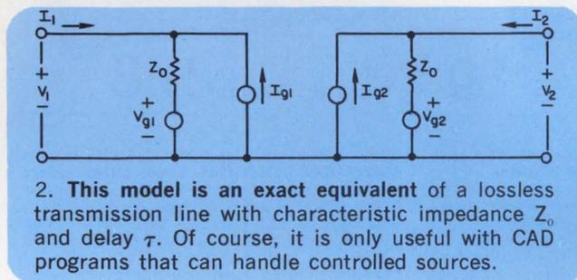
transmission line of characteristic impedance  $Z_0$  and delay  $\tau$ . The circuit is especially well-suited to steady-state analysis.
