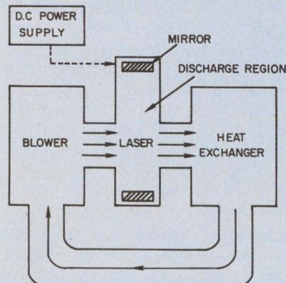
Desk-sized CO<sub>2</sub> laser contains a closed-cycle gas cooling system.
