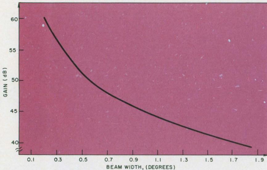
4. No freedom exists to specify the antenna gain once the coverage area is chosen. Here antenna gain is plotted against 3-dB beamwidth at a frequency of 4 GHz. The gain equation is given in Fig. 1, the formula for 3-dB beamwidth is  $\Theta = 7 \times 10^4 / fD$ , where  $f$  is the frequency in MHz,  $D$  is the antenna diameter in feet, and  $\Theta$  is expressed in degrees. (Both formulas are from ITT's "Reference Data for Radio Engineers," fourth edition, p 753).
