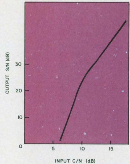
5. The price of fm improvement is the existence of a threshold. In this rather representative system, it occurs in the neighborhood of 10-dB carrier-to-noise ratio. The corresponding S/N is about 25 dB.
