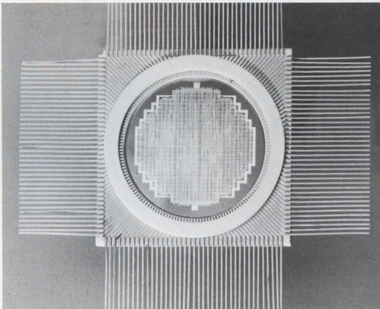
**Computer on a chip.** New digital LSI analyzer with 253 gates solves differential equations, p. 97.
