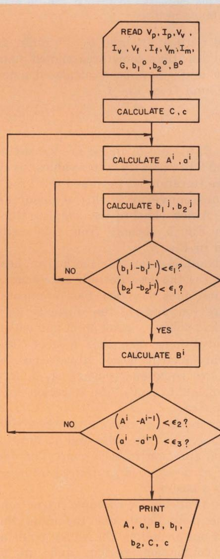
5. Flow chart of computer program shows the steps to be followed in determining parameters of the curve-fitting equation. Note the iteration steps for the  $a$ ,  $A$ , and  $B$  parameters.
