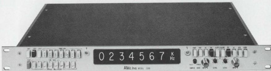
Atec's new Model 2000 offers more performance for less money than any competitive instrument. Standard features include a 1 MHz crystal-controlled time base stable to one part in  $10^8$ /day, remote programming, and 1-2-4-8 BCD output. Options include display storage, oven-stabilized crystal, and additional digits (to seven). Modular plug-in design makes it simple to add options at any time.
