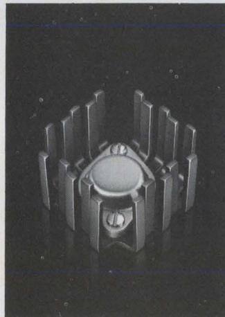
T03's, T066's, T015's and other case-mounted devices can be operated with many times more power when mounted in UP's. In still air, the staggered fingers dissipate by radiation and convection. In forced air, turbulence moves the air around each finger. Efficient in any direction. Outperforms extrusions dramatically.
