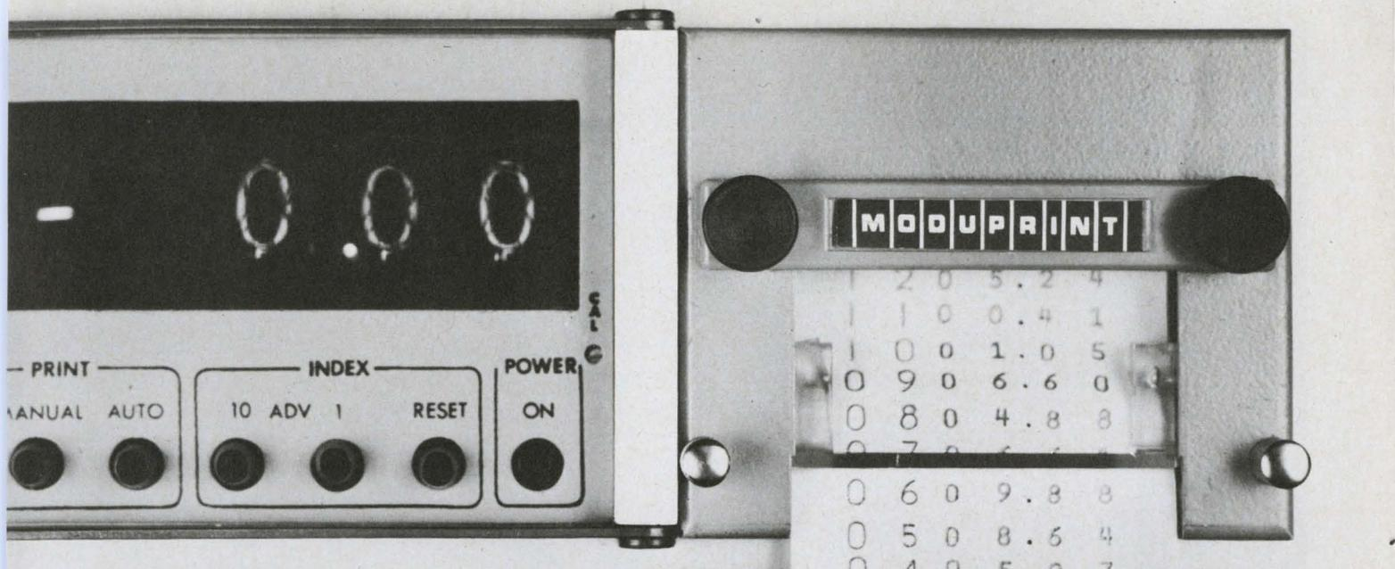
Printing digital voltmeter with 3-1/2-digit readout occupies only 3-1/2 by 8 in. of a front panel.
