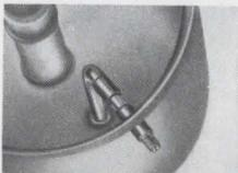
Solder one end to coupling link
