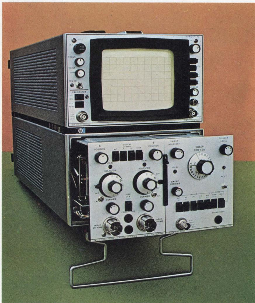
**High-performance dual-trace oscilloscope** with distributed-electrode CRT features a real-time response from dc out to 250 MHz. It can be used to analyze the short-duration fast-rise pulses of high-speed digital systems.
