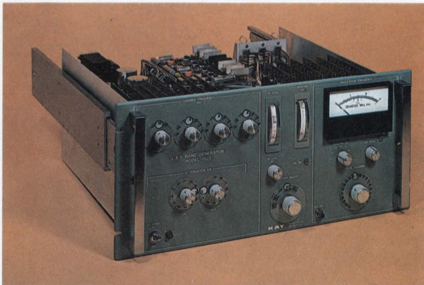
Combining the reliability of solid-state construction with the desirability of remote operation, a new L- and S-band signal generator can be programmed for rf output frequency and level, as well as subcarrier frequency.
