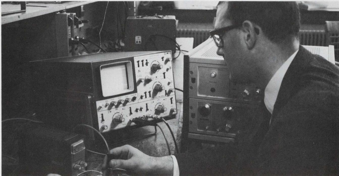
**Dual-trace oscilloscope** views dc-to-5-MHz signals with an accuracy of 200  $\mu\text{V}/\text{cm}$ . It
