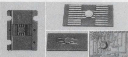
TINY-PAK™ op amps are handled and tested in standard Barnes carriers. Leads can be bent for insertion into PC boards or soldered or welded to ceramic substrates.
