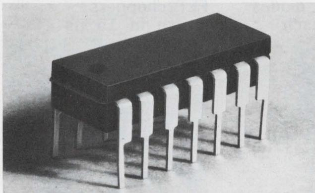
**Monolithic integrated circuit** is a complete a-m radio receiver on a single chip, p. 254.
