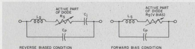
Fig. 1 Small-signal equivalent circuit of PIN diode.
