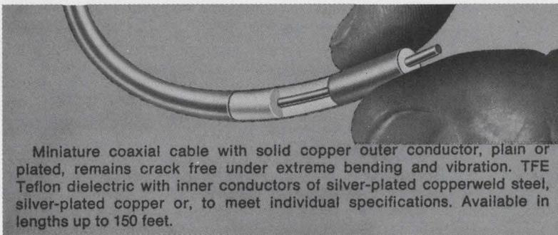
Miniature coaxial cable with solid copper outer conductor, plain or plated, remains crack free under extreme bending and vibration. TFE Teflon dielectric with inner conductors of silver-plated copperweld steel, silver-plated copper or, to meet individual specifications. Available in lengths up to 150 feet.
