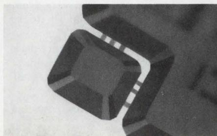
lographic planes in silicon. The solution etches perpendicular to each of these at different rates. The surface shown light, for example, etches away most rapidly. To cut out an area, a mask is applied onto the fastest—"light"—plane, with the mask edges parallel to the slowest—"dark"—planes of the crystal.
