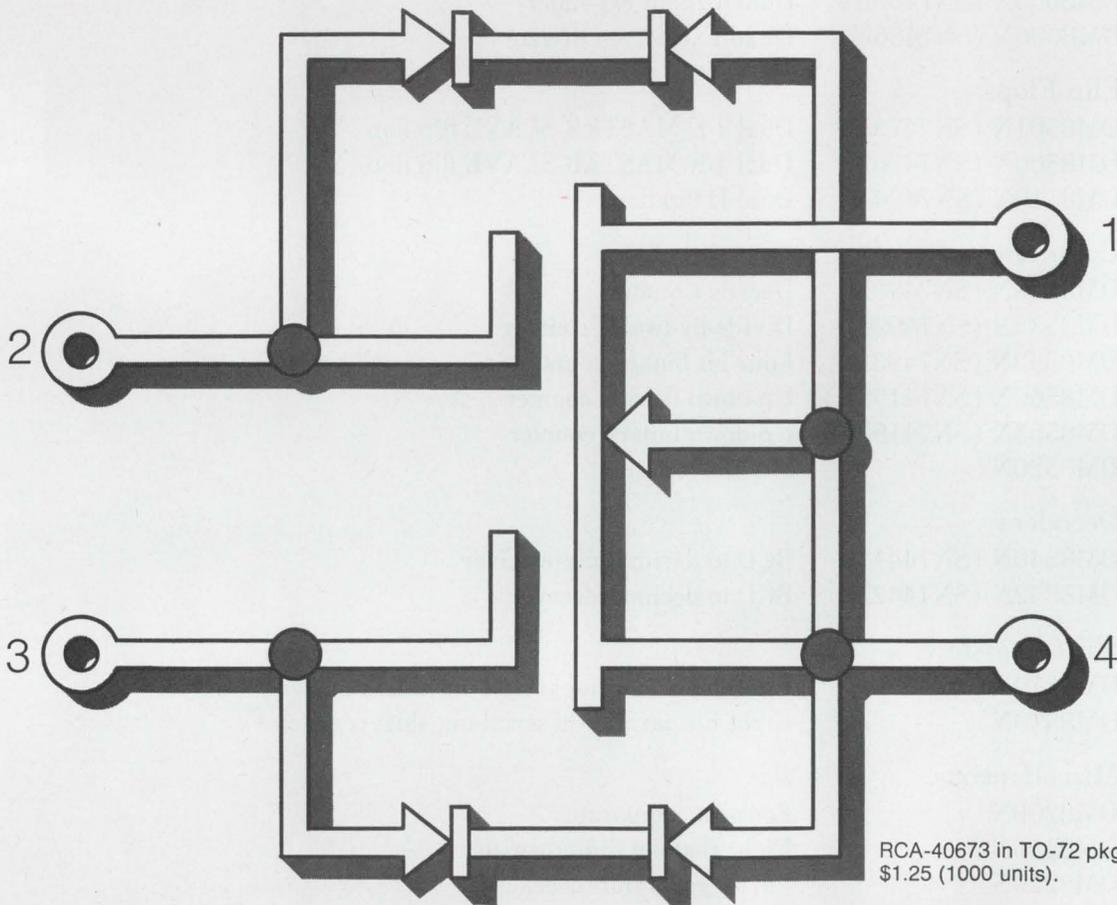
The major technical challenge associated with the development of the RCA-40673 was that gate protection must not significantly degrade the RF performance.
