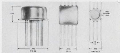
Note standard .050" spacing between .017" x .005" TINY-PAK™ leads.
