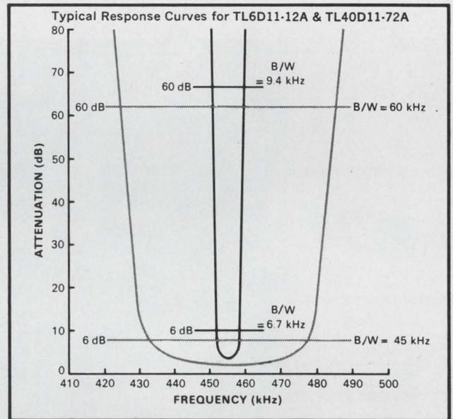
Here's the smallest (less than 0.1 cu. in.), most rugged fixed-tuned filter of its kind on the market today!
