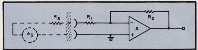
3. The conventional op amp connection is unsuitable for biological use, because the over-all gain depends on the unstable value of the source resistance,  $R_s$ . Common-mode rejection is poor. Typically,  $R_s = 2 \text{ k}\Omega$  to  $150 \text{ k}\Omega$ ,  $R_1 = 10 \text{ k}\Omega$ ,  $R_2 = 1 \text{ M}\Omega$ ,  $A_o = 30,000$ ,  $R_{in} = 10 \text{ k}\Omega$ , and the gain is 10 to 100.
