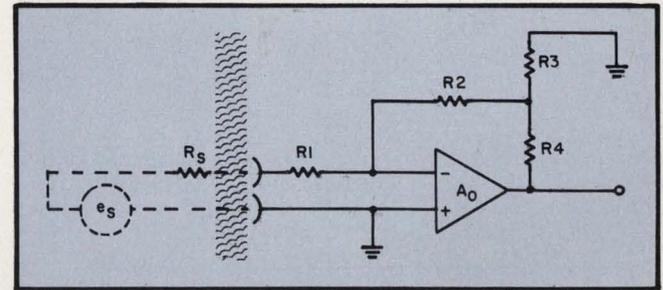
4. A further deterioration in CMRR results from this modification of the voltage divider feedback arrangement, although gain stability is improved due to increased input impedance. Typically,  $R_s = 2 \text{ k}\Omega$  to  $150 \text{ k}\Omega$ ,  $R_1 = 1 \text{ M}\Omega$ ,  $R_2 = 1 \text{ M}\Omega$ ,  $R_3 = 100 \Omega$ ,  $R_4 = 10 \text{ k}\Omega$ ,  $A_o = 30,000$ , and gain is 90 to 100.
