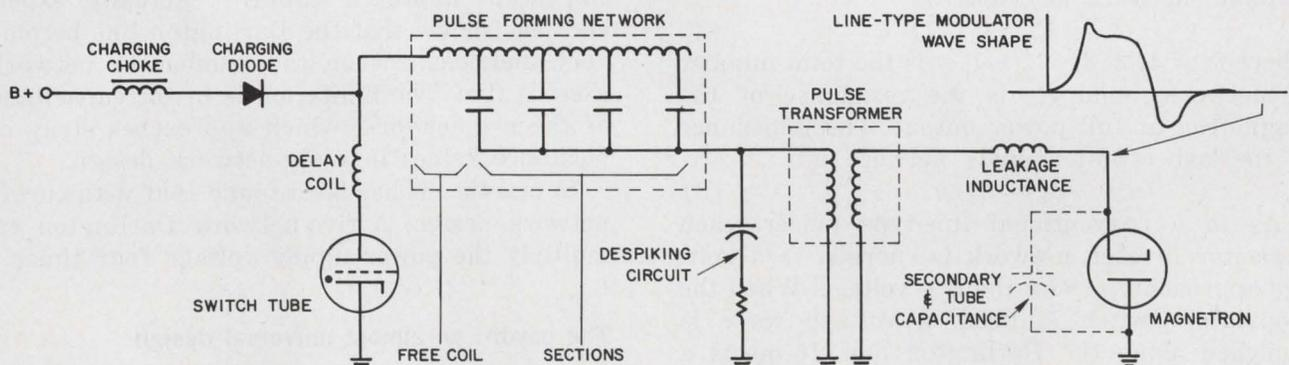
2. **Risetime limitations** make the conventional line-type pulse modulator unsuitable for the generation of very
