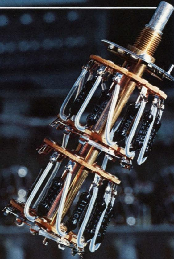
Dale Metal Film Resistors provide precise voltage attenuation in the Brush Mark 200 Recorder. This highly accurate direct writing system is now in use in the Apollo Deep Space Program.
