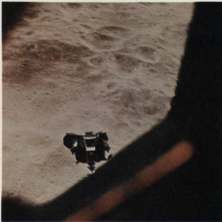
Ascent stage of the Apollo lunar module is photographed from the command module prior to docking in lunar orbit. The photo was made during the Apollo 10 mission.
