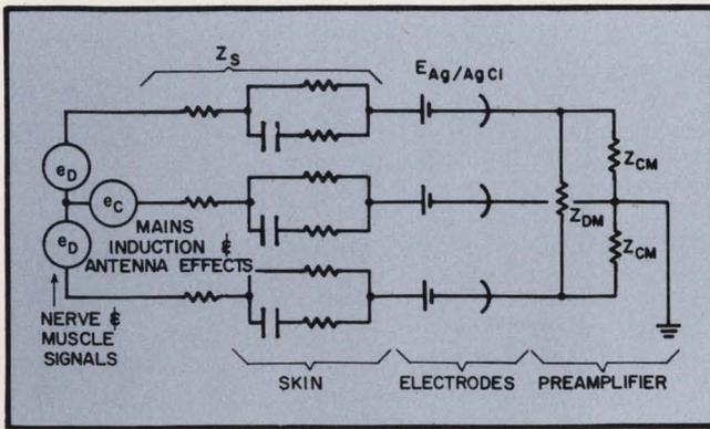
1. Biological signal sources generate millivolt signals and exhibit high output impedance. The skin layer adds series impedance, electrode-skin contacts add dc noise in the form of contact potential, and common-mode induced noise acts to swamp out the signal making detection of nerve or muscle signals difficult and high-gain op amps must be used.
