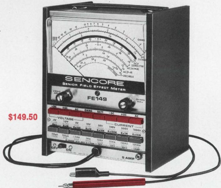
**Exclusive push-button design.** Just push two buttons for any test — top row selects function, bottom row selects range. Action is instant and automatic.
