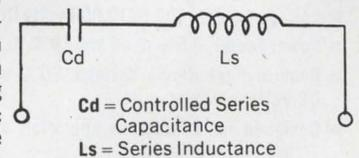
After four years of production use, Zenith says of the Series-Resonant Trap: "It saves space, saves time, works satisfactorily." Here are the basic specs:
