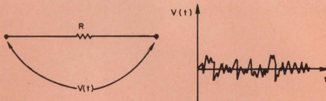
1. Noise in a resistor is caused by the random thermal motion of free electrons within it. An open-circuit voltage fluctuation is developed across its terminals.
