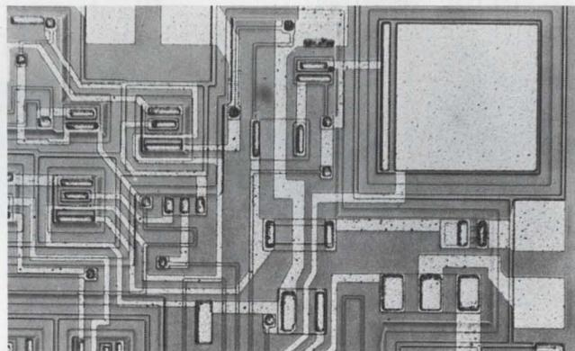
**Single-chip high-speed operational amplifier** gets settling time down to 300 ns, p. 254.
