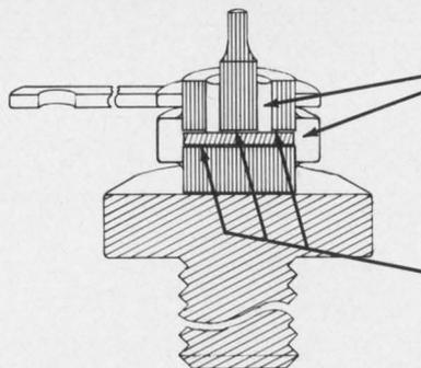
Two fused-in-glass seals melted, wetted and fused to both silicon and metal surfaces permanently protecting and stabilizing the SCR die in a voidless Unitrode package.
