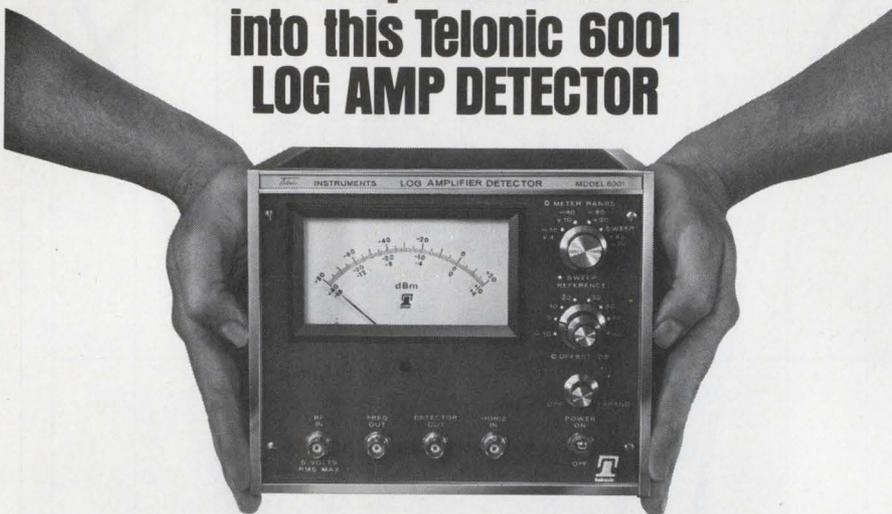
The solid state 6001 will accept RF inputs from 400 kHz to 130 MHz with voltage swings as wide as 178,000 to 1. It's calibrated over a 90 dB range (-70 to +20 dBm) and is even equipped with a range switch for closer looks at -40 to +10 dBm and -16 to +4 dBm. An offset control also allows shifting the meter range as much as 70 dB either way.
