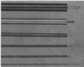
Miniature coaxial cable available in sizes from .020 inches to .325 inches. Tolerance as low as  $\pm 1/2$  ohm on characteristic impedance of 50 ohm. Minimum VSWR.
