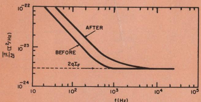
9. Surface states lead to excess noise because some carriers are trapped, and subsequently escape, many times on their way across the depletion region, causing a pseudoshot-noise effect.
