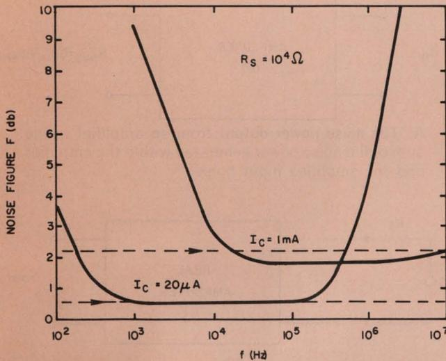
14. The measured noise figure of a planar silicon transistor corresponds to the noise figure calculated from the model only for mid-range frequencies. At low frequencies the  $1/f$  excess noise predominates, and at high frequencies the decreased current gain of the transistor leads to an increase in the noise figure.
