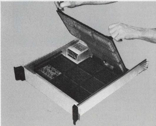
When you specify EECO 2D Hardware a computer converts your "Pin Logic List"\* into a wire plan and checks for errors and omissions before wiring begins. EECO plugs in the IC's, machine Wire-Wraps the backplanes and in days...your schematic is a drawer of working electronics with all necessary computer generated support documentation.
