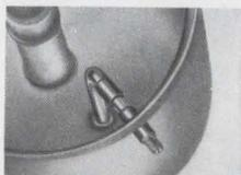
Solder one end to coupling link
