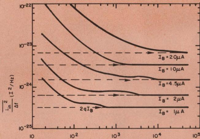
12. The noise current of a planar silicon transistor, referred to the input, closely follows Schottky noise at frequencies above a few kHz. At the lower frequencies, excess  $1/f$  noise become significant.
