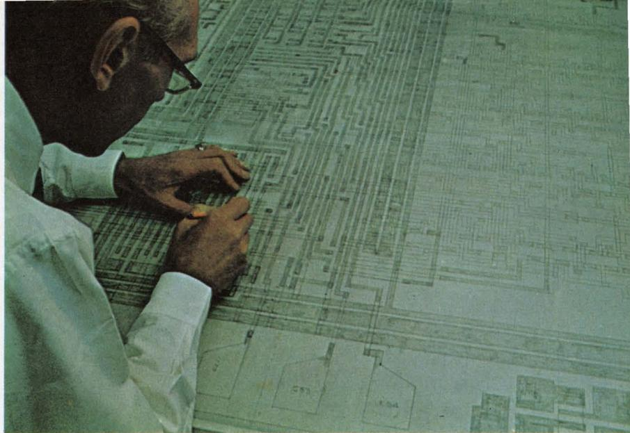
**Array systems engineer** Charles Mclean of Viatron Computer Systems Corp. is busy designing a composite layout for a complex MOS array (Paper 15/3).
