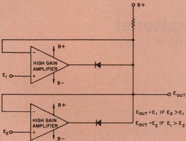
5. Operational-amplifier gate passes the more negative signal and avoids the drawbacks of simple diode and transistor gates. This operational amplifier configuration is the N gate of Figs. 7 and 8.
