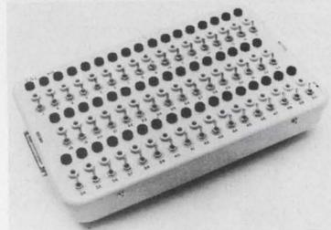
A — A Break-Out Box is designed to reduce hook-up and testing time. It offers a convenient method to measure or interrupt voltages, currents, and/or signals between any two pieces of equipment. A flip of a switch instantly opens or closes any circuit. Cumbersome shorting plugs are no longer necessary. It comes in a variety of connector configurations, is of rugged construction, low in cost, and available off-the-shelf.
