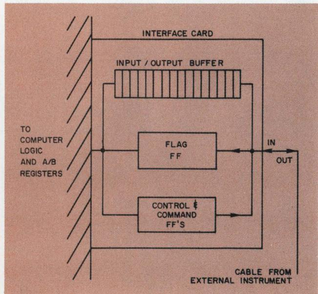
3. Typical interface card shown here contains storage and control circuitry.
