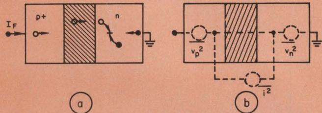
7. Current flow through a pn junction includes resistive flow of electrons and holes through the  $n$  and  $p$  regions, with associated resistance noise, and recombination in the depletion region, with associated shot noise (a). A simple model includes all of these noise sources (b).
