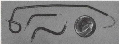
Assemblies used in LEM program. Directly soldered into circuits. Operate successfully in temperatures ranging from  $-54^{\circ}\text{C}$  to  $+140^{\circ}\text{C}$  under environmental pressure of  $10^{-6}$ .
