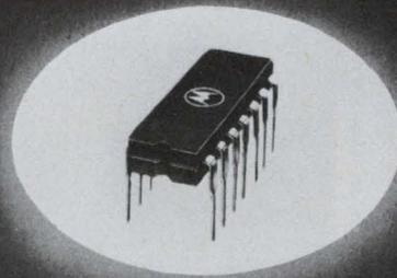
Motorola's MC1566L/1466L is a precision wide-range voltage and current regulator (Monolithic Epitaxial Passivated). This unique "floating" regulator can deliver hundreds of volts—limited only by the breakdown voltage of the external series pass transistor. Output voltage and output current are adjustable. The MC1566L/MC1466L integrated circuit voltage and current regulator is designed to give "laboratory" power-supply performance.
