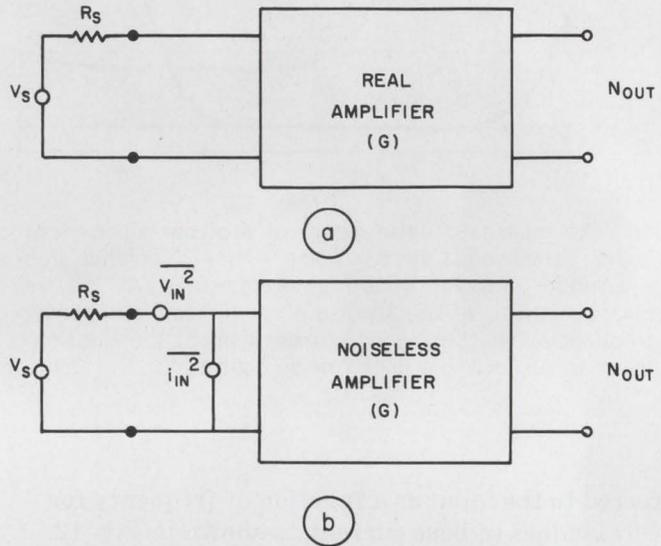
B. A circuit model of a noisy amplifier consists simply of a noiseless or ideal amplifier with noise sources  $\overline{v_{in}^2}$  and  $\overline{i_{in}^2}$  connected to its input. The noise sources represent the mean square values of the corresponding voltage and current fluctuations, and are chosen so that the resultant output noise power is equivalent to that of the real amplifier.
