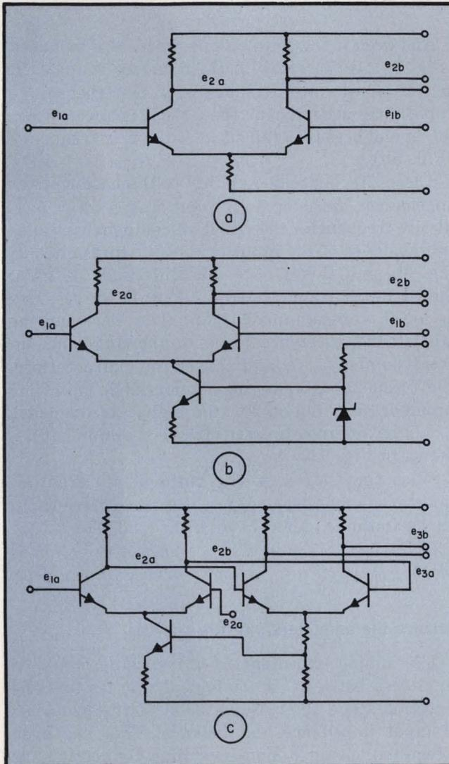
2. The differential pair is an essential part of every biological amplifier (a). For better common-mode rejection the common emitter resistor is replaced by a constant current source (b), which can be controlled by the common-mode output of a second differential stage (c).
