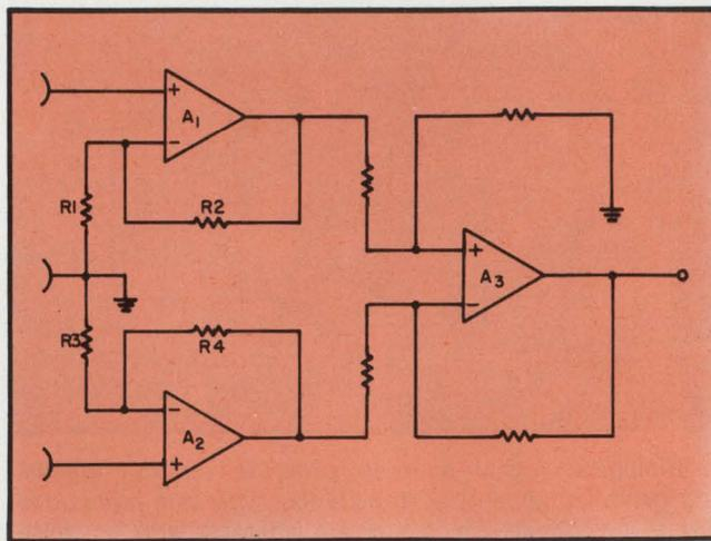
7. The compound differential circuit uses matched-gain, non-inverting preamplifiers before the common-mode rejection stage. Differences in gain between  $A_1$  and  $A_2$  lead to poor CMRR, of course, but the problems associated with the high, but variable, impedance of the biological source are avoided.
