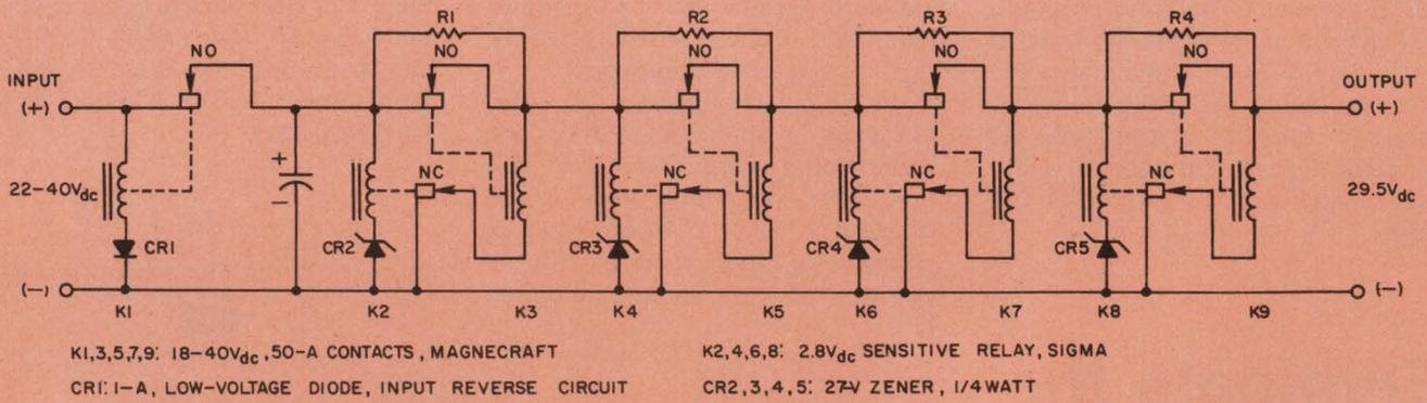
Series resistance is added to the line by the various stages of the limiter when an overvoltage
