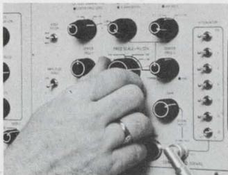
**2.** A selector knob sets the frequency scale in one of five settings from 15 Hz/division to 1.4 kHz/division. Interlocked circuit functions in the analyzer automatically optimize the display for any setting of the frequency scale.
