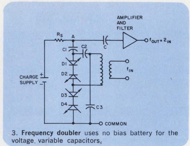
3. Frequency doubler uses no bias battery for the voltage, variable capacitors.
