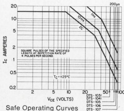
energy reliability that's needed for very tough switching jobs—resistive or inductive. The 28-volt shunt regulator above, for example, is amply handled by the DTS-103 ( $V_{CEX}$  of 80 volts). For complete data on this circuit, ask for our application note No. 42.
