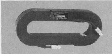
Encapsulated delay line, used between 8 and 12 Gc, exhibits 100 nanoseconds of delay. Weighs less than 8 pounds, cable is 70 feet long, .270" diameter, 50 ohm impedance.
