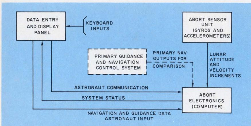
**Lunar-module abort guidance-system** is checked by comparing performance with inputs from the primary system displayed on the panel. The system was developed by TRW Inc., Redondo Beach, Calif.
