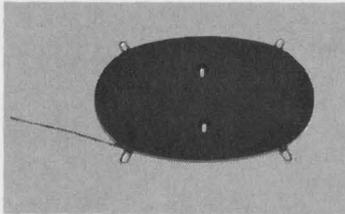
To achieve 122 nanoseconds of delay and fit tight confines, a pancake configuration measuring 11" x 7" x 3/8" containing 45 feet of .141", 50 ohm miniature semi-rigid coax was potted for use with an airborne radio altimeter.
