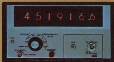
Model 8220—500MHz Direct Reading Frequency Counter. 7-digit display with memory. Price: \$1795.00. (additional specs on reverse side)
