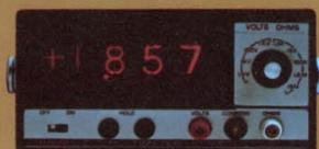
Model 7050—Dual Slope Integrating 3 $\frac{1}{2}$ -Digit Multimeter. 0.1% accuracy. Measures DC volts, ohms, current. Price: \$354.00. (additional specs on reverse side)
