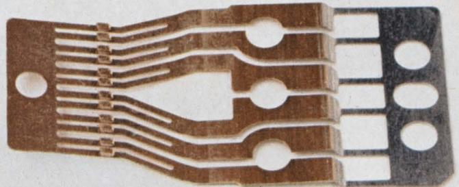
Then there are the contact springs. Ours are phosphor-bronze. Others use nickel-silver. Our lab gave this stuff a thorough check, but found nickel-silver too prone to stress-corrosion. Atmospheric conditions which cause tarnish and ultimately stress corrosion have almost no effect on phosphor-bronze.
