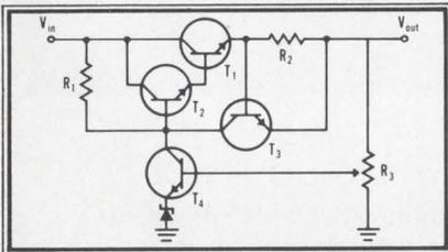
**Solution:** Replace the darlington pair with a FET and a CL diode.
