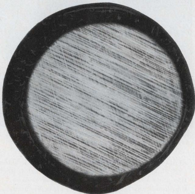
**Nay!** That's the alternative to Belden—a cross-section of conventionally insulated fine magnet wire. Note the thin spots that can quickly burn through to cause shorting. And the thick spots that cause uneven windings.
