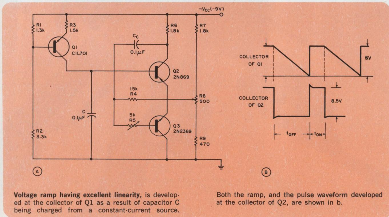
Voltage ramp having excellent linearity, is developed at the collector of Q1 as a result of capacitor C being charged from a constant-current source.
