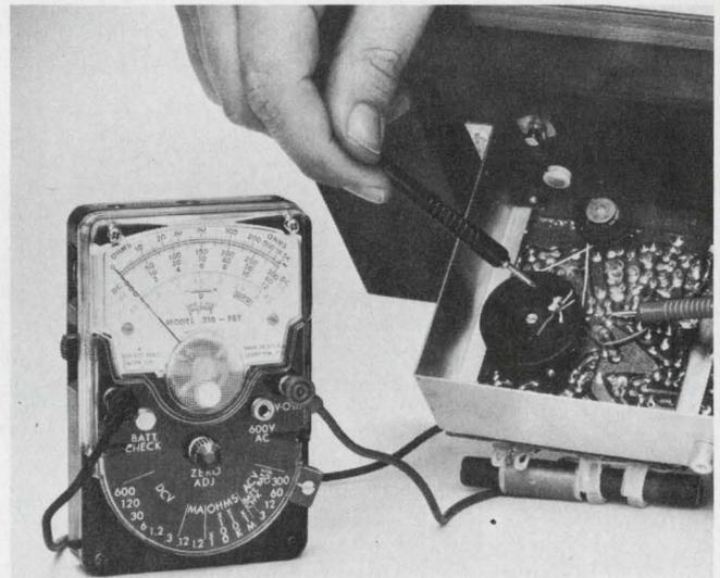
Shirt-pocket battery-operated VOM features constant 10-M  $\Omega$  FET-input, p. 168.
