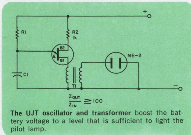
supply voltage is in the 6 to 40 volt range. For very low voltage operation, a 2N2840 should be used, which will operate with voltages as low as 1.5 V. The values of  $R_1$  and  $C_1$  will determine the frequency of oscillation.
