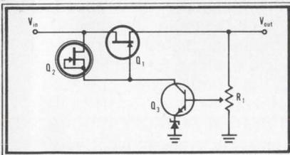
Increases in  $V_{OUT}$  are inverted and amplified by Q3. The increased  $V_{GS}$  on Q1 reduces the supply current, decreasing output voltage. Current-limiter Q2 (1) acts as a load for Q3 and (2) when the output is short circuited it limits the forward bias current of Q1, limiting short circuit output current to the  $I_{DSS}$  of Q1. The use of the FET increases circuit power gain, reducing ripple, and increasing regulation.
