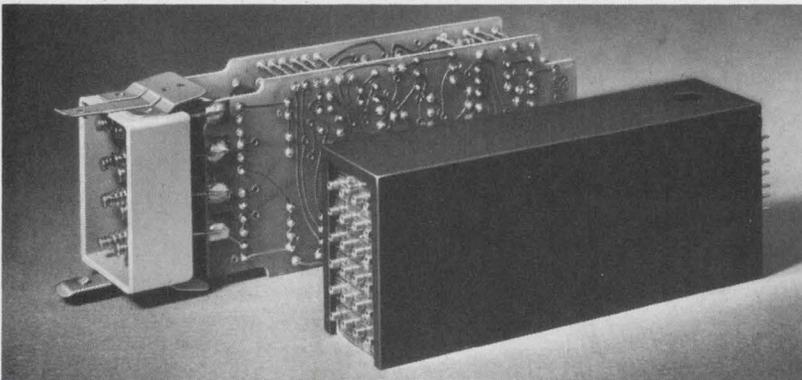
**IC Driver/Decoders**—Small, reliable units for driving IEE readout incandescent lamps ranging from 250 ma @ 6V to 40 ma @ 28V. Fully compatible with modern IC's. Accept a variety of binary codes for decimal conversion. Require normal signal V., draw less than 2 ma per data input. Internal data storage for pulsed oper.
