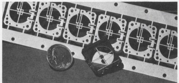
Etched lead frames for integrated circuits. Any configuration can be made adequately framed for support. Leads are flat ribbons down to 0.002 inches wide and from .002, .004, .005 and .010 inches thick. We etch kovar, nickel, alloy 42, copper, aluminum and other metals for microcircuit packaging.
