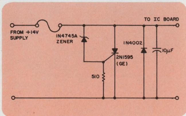
Protection against overvoltage and polarity reversals is provided by this inexpensive circuit.
