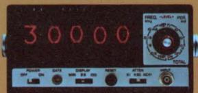
Model 8050—30MHz Frequency/period meter (with 8051 pre-scaler, capability extended to 300MHz). Also measures multiple period average and totalizes. Price: \$650.00. (additional specs on reverse side)
