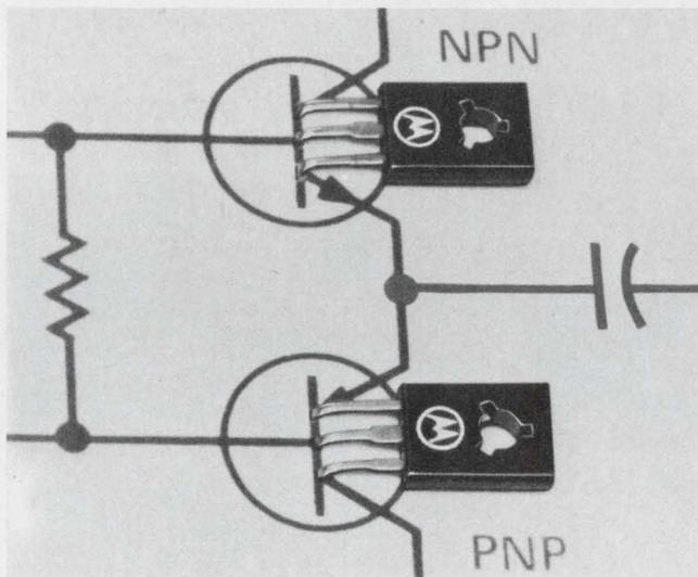
Miniature plastic npn/npn transistor pairs complement 35-W audio amplifiers, p. 158.
