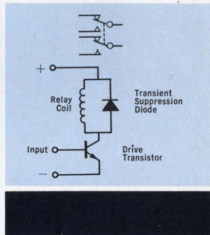
We keep our promises! Last month we promised a low-priced industrial application DPDT TO-5 case relay with an internal transistor driver. We call this new contraption "THE PILL." "THE PILL" contains a transistor driver and suppression diode, attaches externally to our DPDT industrial 712 relay to form the 712T . . . and does double duty as a transapad.
