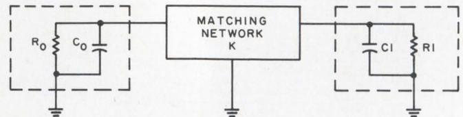
3. These are the variables that the ZMATCH program considers in computing the various suitable combinations of L and C which will make up a suitable matching network, K.
