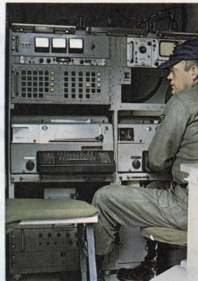
**Airborne communications van** carries long and short-haul radios and cryptographic equipment.
