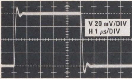
FIGURE 4. Small Signal Transient Response with Feedforward Compensation
