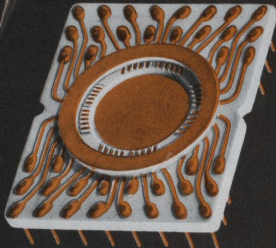
It's a 40-pin Plug-in-Package (PIP) from the Cermetron Division of National Beryllia—30% lighter, and with 8 to 10 times the thermal conductivity of similar packages using other materials, because it is made from BERLOX—Beryllium Oxide.
