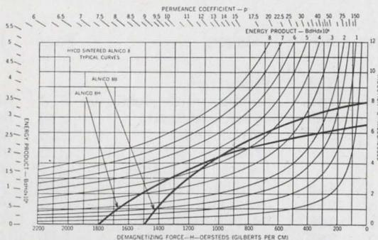
You might be able to get sintered alnico 8 somewhere else—but not like this. Our HyCo 8 has the greatest coercive force of all sintered alnicos. Typically, 1500 oersted for HyCo 8B, and 1800 oersted for 8H.
