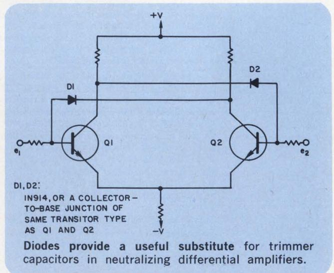
This technique is also suitable for use in linear IC amplifiers, many of which use a differential amplifier in their front end.
