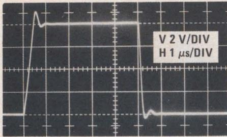
FIGURE 5. Large Signal Transient Response with Feedforward Compensation
