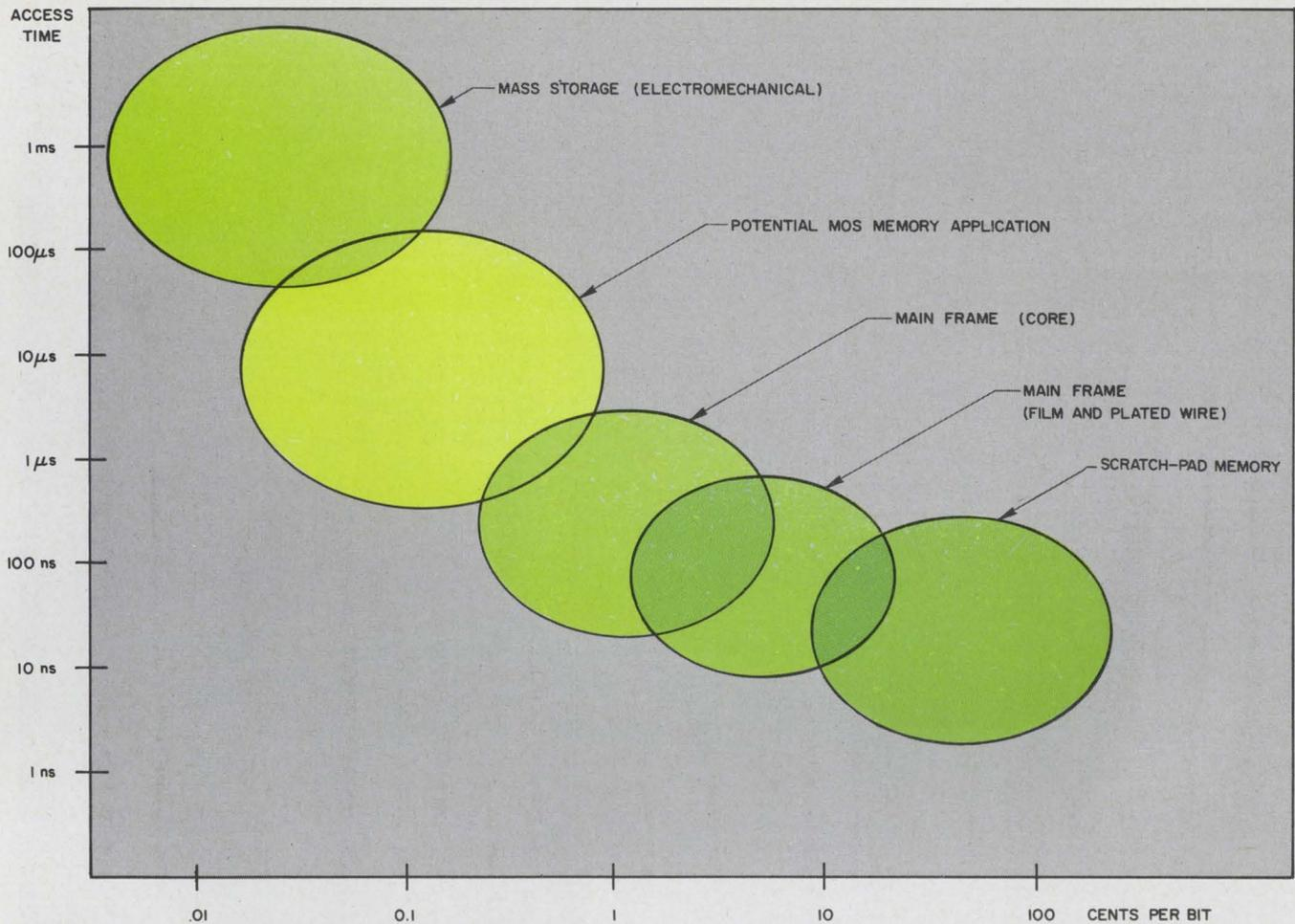
There's great potential for MOS in the memory market, according to Intel's Graham, in the area between electro-mechanical storage and main frame core memory. The MOS memory, intermediate-speed registers, for example, should have access times of 10 microseconds to offer
