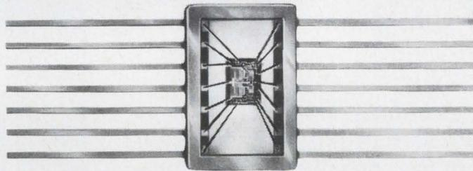
A family of 28 volt integrated circuits including dual and quad gates, expandable gates and gate expanders, set-reset flip flops, 5 volt to 28 volt converters and 28 volt to 5 volt converters, featuring:
