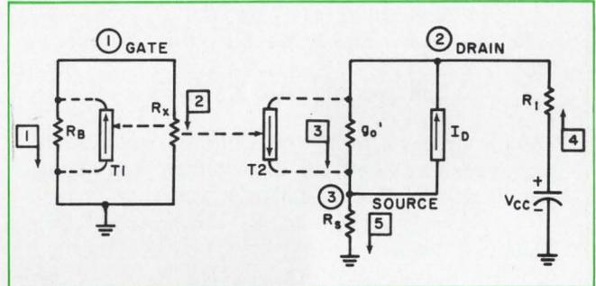
3. **Resistor stabilizes the operating point.** Selection of the proper value for stabilizing resistor  $R_s$  can be done graphically or with a curve tracer.
