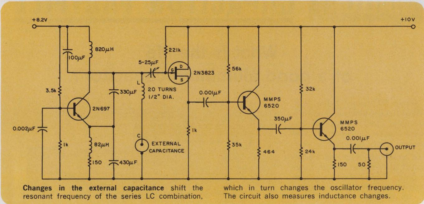
Changes in the external capacitance shift the resonant frequency of the series LC combination, which in turn changes the oscillator frequency. The circuit also measures inductance changes.
