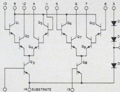
Get the feel of real design freedom with CA3050 or CA3051 for matched dual amplifiers, dual sense amplifiers, dual Schmitt triggers, doubly-balanced detectors and modulators—and anywhere you want matched device performance.
