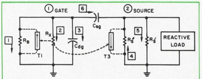
5. **Reduce current sources** by using this source follower version of the model. Only two current sources are required here, rather than four as in other versions.
