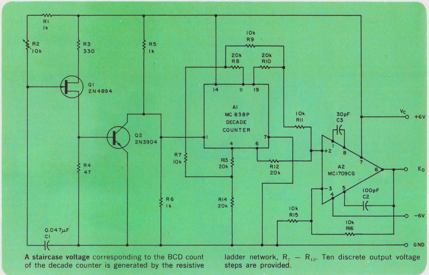
by the resistive ladder network,  $R_7$  through  $R_{13}$ . Since the BCD count changes in discrete steps, the analog output of the ladder network also changes by discrete steps that increase as the BCD count increases. The analog output voltage of the ladder network is given by the equation:
