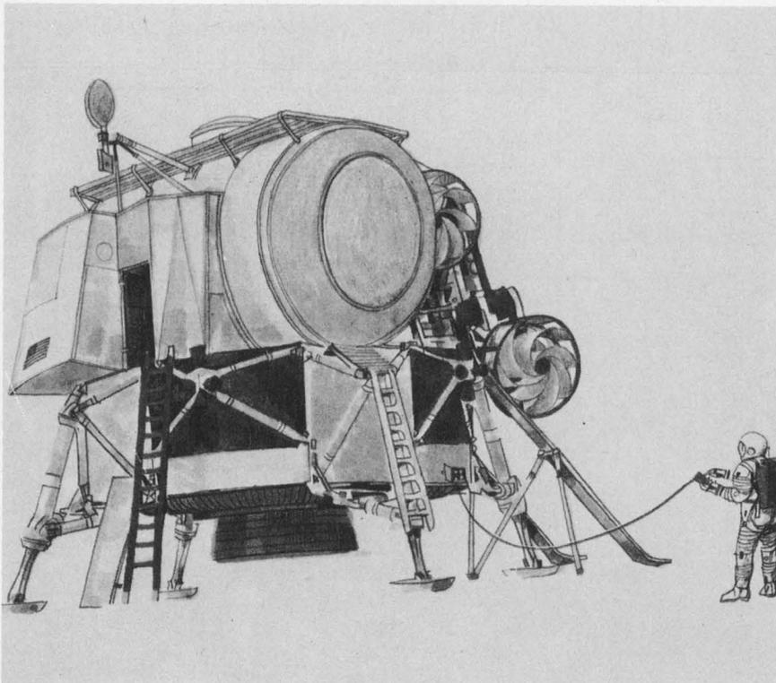
**LM truck** can transport cargo in the volume otherwise occupied by the LM ascent stage. The vacated volume, 1650 cubic feet, can be filled with 8800 pounds of payload. Living quarters here take up 760 cubic feet.
