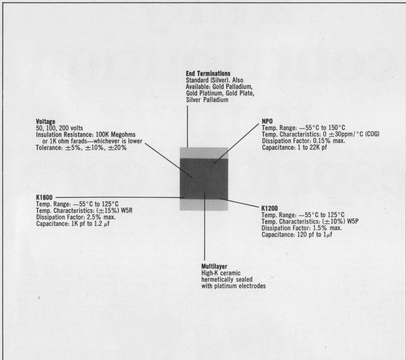
The above specs pretty well tell the story on our standard line of ceramic chip capacitors. Except that they're available in a variety of sizes in rectangular and near-square types.
