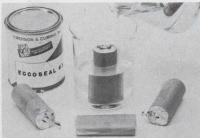
ECCOSEAL® 63 is a low-viscosity, solvent-free impregnant that cures to a rigid, low-loss crosslinked polymer. Developed specially for impregnating capacitors, filters and coils. Useful from  $-65^{\circ}\text{F}$  to  $+375^{\circ}\text{F}$ . Dielectric constant is 2.4; dissipation factor is 0.0005 at 1 MHz.
