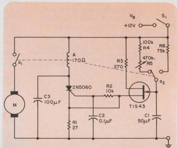
The OFF time of the motor being controlled can be varied between 5 and 35 seconds by potentiometer  $R_5$ . The motor ON time is constant at 5 seconds.
