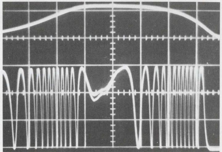
**High-voltage microsecond pulses** can be measured more accurately with Sandia's laser system. Page 34.
