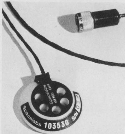
3. Relatively crude body-temperature sensor for Project Mercury, at top, compared with more recent Project Apollo skin-temperature sensor, at bottom. Rapid advance in sensor technology is evident.
