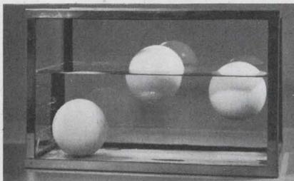
ECCOSIL® 4659 is a castable RTV silicone that cures to a resilient foam with less than half the density of conventional silicones. Photo shows buoyancy comparison of Eccosil 4659 (center) with other silicone foam (R) and conventional silicone (L). Recommended for encapsulation of delicate electronic assemblies.
