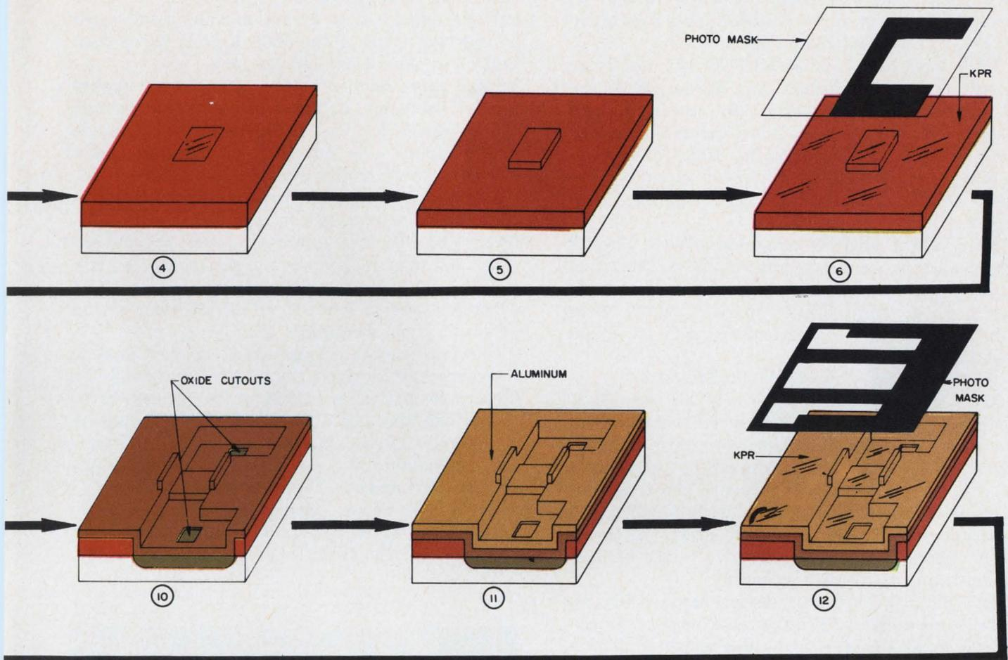
thick, is not removed because of its increased relative thickness. A p-type impurity, usually boron, is then diffused into the exposed source and drain regions, and a second protective oxide layer is grown (8). A second layer of photoresist is applied, exposed, and developed to define oxide cutouts for contacts to the source and drain diffusions, and the cutouts are made by etching (9). The photoresist is removed (10) and a layer of aluminum is applied over the entire wafer surface (11).
