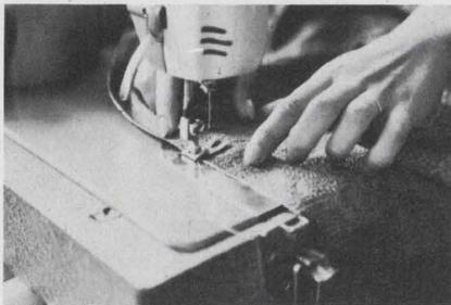
ECCOSHIELD® MNF is a series of light-weight, pliable fabrics woven from conductive fibers. It can be cut, sewn or draped to protect equipment and personnel from RF and microwave radiation. Available in two-foot widths, any length. Weight about 3 ounces per square yard.
