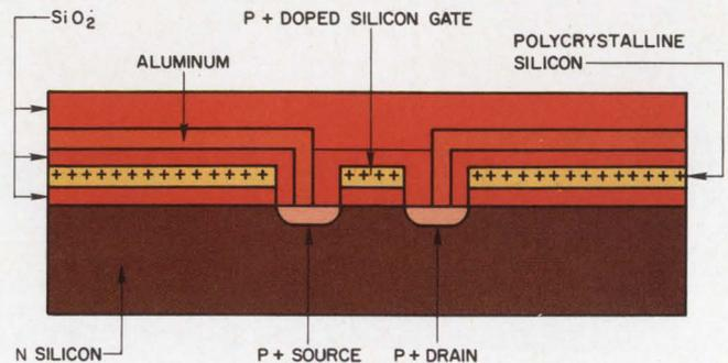
The silicon gate MOS device uses a p<sup>+</sup> doped silicon region as the gate electrode. The gate, source and drain are diffused simultaneously, and perfect alignment is automatic. Source-to-drain and gate-to-drain overlap capacitance is reduced by a factor of 5 from that of conventional devices.
