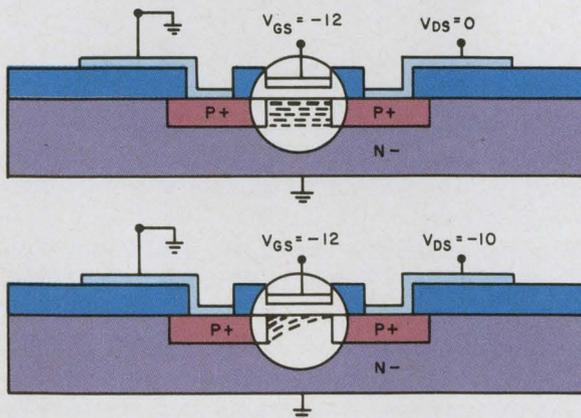
**C. The saturation phenomenon:** drain-to-source voltage effects are limited by channel pinch-off.
