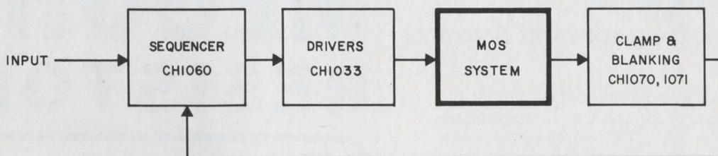
The 5 MHz Clock Driver System above uses all off-the-shelf Cermetek circuits, but you don't have to operate at 5 MHz to benefit from Cermetek's complete line of compatible MOS Clock Driver circuits. They are immediately available in a wide range of voltages and frequencies to suit your individual needs.
