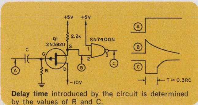
Delay time introduced by the circuit is determined by the values of R and C.
