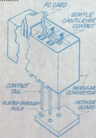
And, no, you don't give up a bit of connector reliability. The exclusive swaged single-beam design of the dual-readout contact provides optimum spring rate and deflection characteristics. A preload applied
