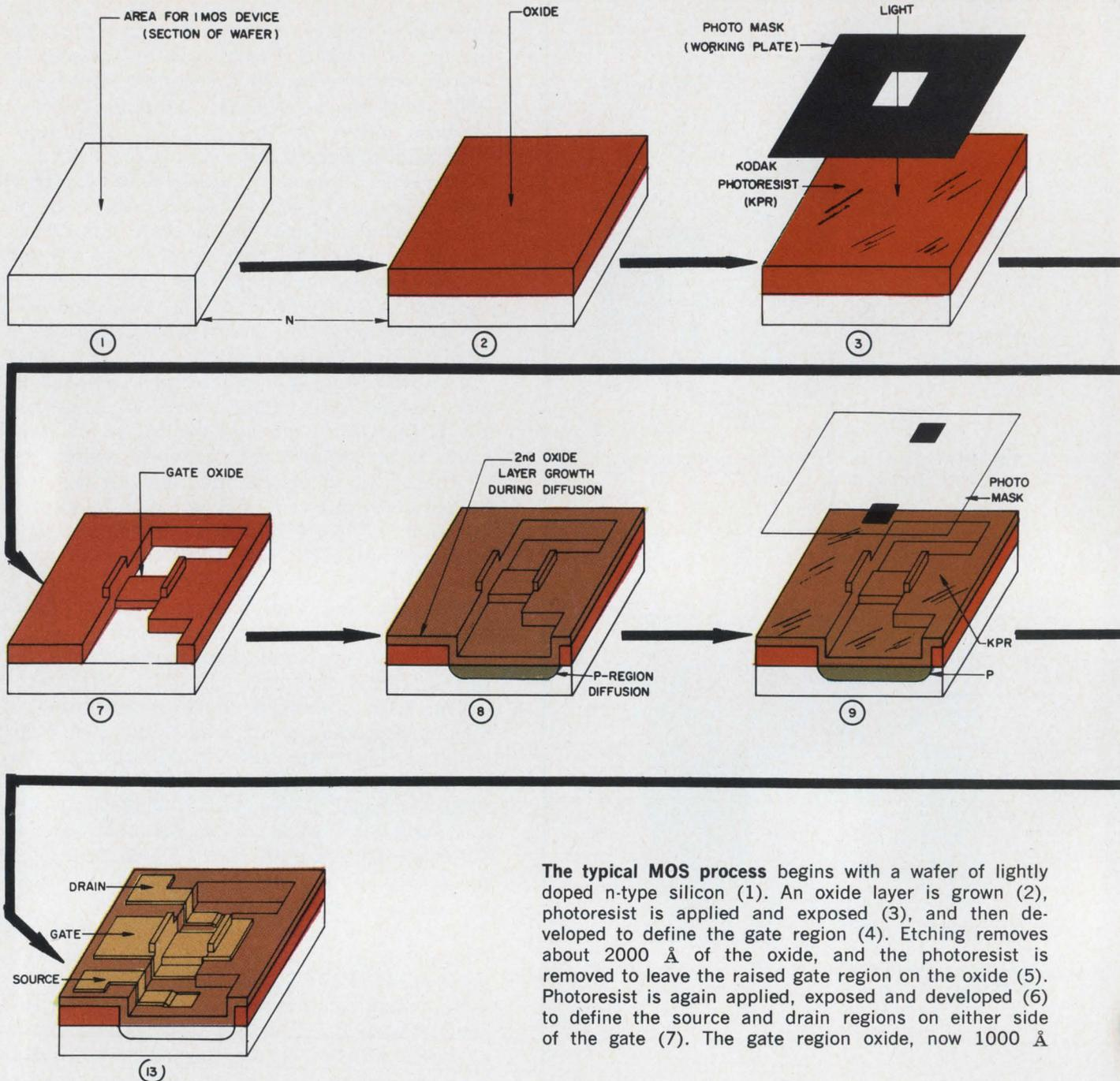
The typical MOS process begins with a wafer of lightly doped n-type silicon (1). An oxide layer is grown (2), photoresist is applied and exposed (3), and then developed to define the gate region (4). Etching removes about 2000 Å of the oxide, and the photoresist is removed to leave the raised gate region on the oxide (5). Photoresist is again applied, exposed and developed (6) to define the source and drain regions on either side of the gate (7). The gate region oxide, now 1000 Å
