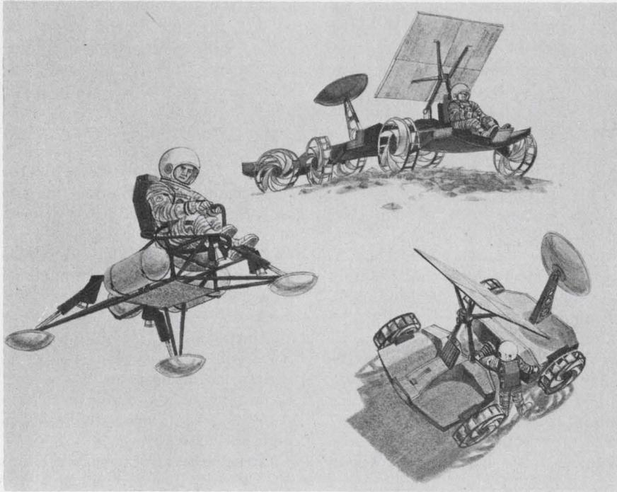
**Lunar flying vehicle** (left) carries one man with 370 pounds of gear or two men. Lunar roving vehicle (lower right) carries 500 pounds, including one man, two miles. Heavy-duty vehicle moves 500 pounds 25 miles.
