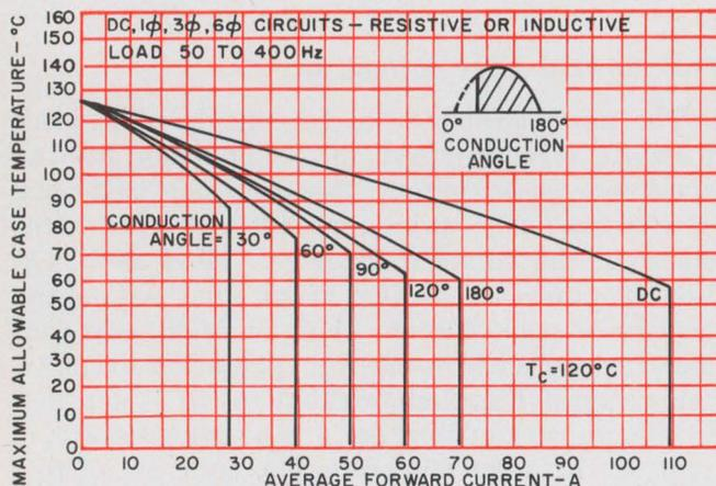
1. Power dissipation in an SCR, and therefore the allowable case temperature, is dependent on the conduction angle. The curves shown are for the G.E. series C52 SCRs, and are based on a sinusoidal current waveform.
