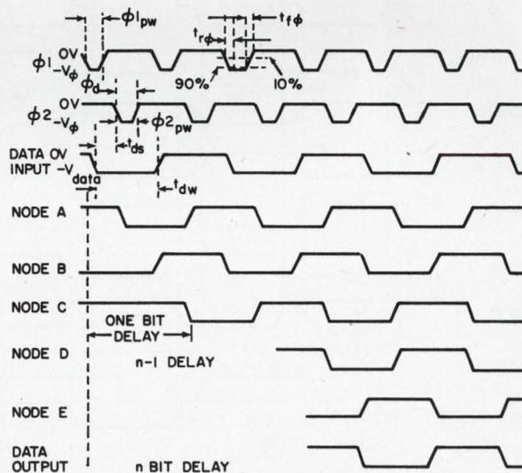
2. The dynamic shift-register cell contains six MOS transistors. Information is shifted within the cells when  $\Phi1$  goes negative (turning on devices  $Q3$ , etc.) and is shifted between cells when  $\Phi2$  goes negative (a). The data is clocked out of the register during the  $\Phi1$  clock time,  $n$ -clock-periods after data entry, where  $n$  is the size of the register in bits (b).
