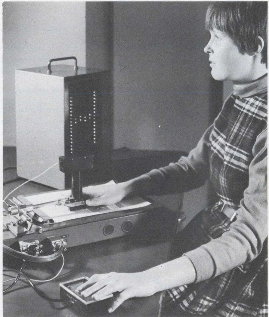
To use the Bliss-Linvill portable tactile reading aid, the operator moves the probe along the line of print and feels a bundle of stimulator pins vibrating in the shape of the letters. The light display box is used for visual troubleshooting.
