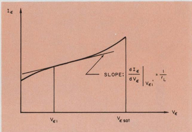
5. The incremental input resistance of the alc stage can be found from this plot of  $I_\epsilon$  vs  $V_\epsilon$ . The resistance is the reciprocal of the slope of the curve.
