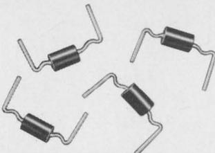
Additional savings in production time and labor costs are now possible by utilizing automatic insertion equipment to install Ceramag® ferrite beads in printed circuit boards.
