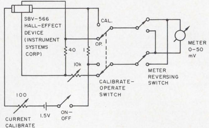
Hall-effect device produces an output voltage that is proportional to the strength of the magnetic field it is measuring.
