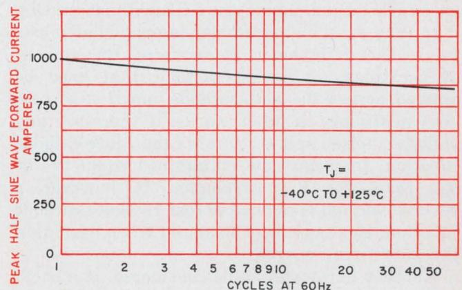
2. The peak forward surge current,  $I_{fm}$ , of an SCR must be derated if the peak current is to be conducted for more than one half-cycle.
