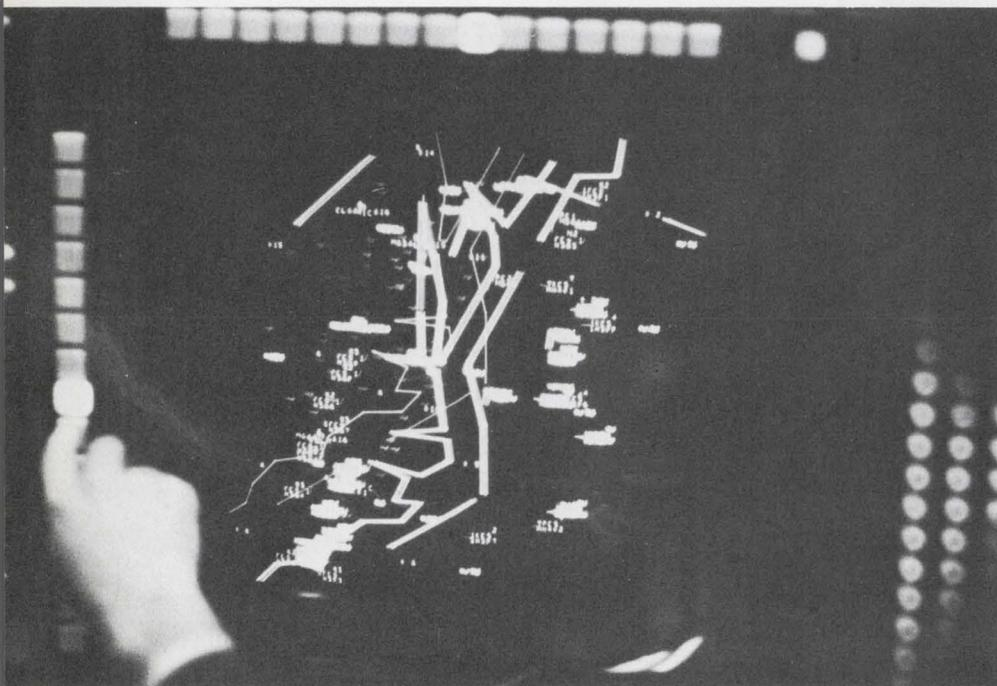
An Air Force sergeant, seated before a TV-type display, moves a small switch. Instantly, he sees a raw radar-picture of all the aircraft flying in his area. He flips another switch and these blips become aircraft symbols, processed by a digital computer that identifies each plane. A third switch brings forth data in alphanumeric form that reveal each plane's altitude, heading and speed.
