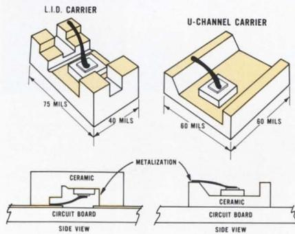
Zener diode "chips" can be supplied on metallized ceramic U-channel and L.I.D. carriers (as well as unmounted), to satisfy most any Hybrid thick or thin-film circuit mounting and fabrication requirement.
