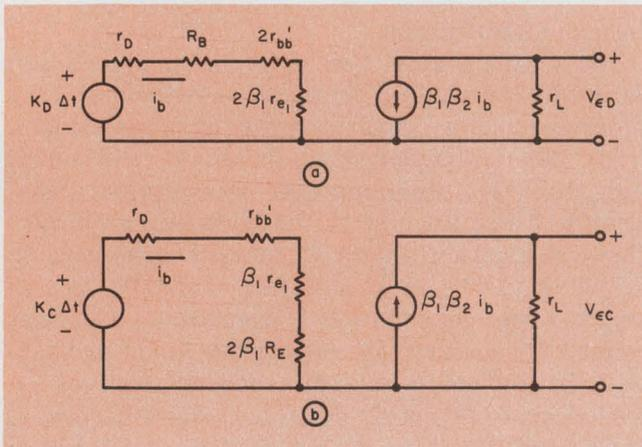
8. The linear drift behavior of the control circuitry is analyzed with these equivalent circuits. Separate models are needed for differential-mode drift (a) and common-mode drift (b).  $R_B$  is the equivalent parallel resistance of  $R_1$  and  $R_2$  of Fig. 6.
