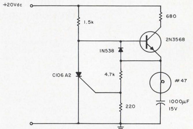
Flashing occurs each time the capacitor discharges through the turned-on SCR. When the discharge current falls below the SCR holding current, the SCR turns off, and the capacitor begins charging for another cycle.
