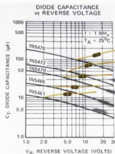
The slopes of capacitance change vs. voltage are the same for all types in the 1N5461 Epicap tuning diode series.
