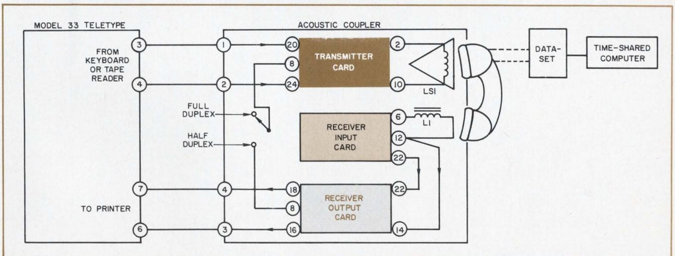
1. Acoustic coupler converts a teletypewriter into a time-shared computer terminal. The transmitter portion of the coupler converts the dc signals from the teletypewriter
