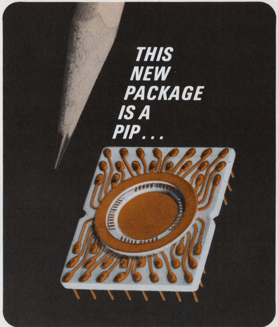
It's a 40-pin Plug-in-Package (PIP) from the Cermetron Division of National Beryllia—30% lighter, and with 8 to 10 times the thermal conductivity of similar packages using other materials, because it is made from BERLOX—Beryllium Oxide.
