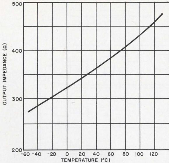
7. The output impedance of the dynamic register is typically below 500 ohms; when the output device is ON the output terminal is connected to ground through less than 500 ohms. The output impedance increases with temperature.
