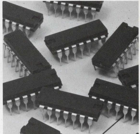
**Two up/down counter chips**, binary and decimal, rep to 30 MHz, p. 108.
