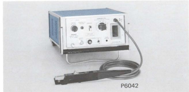
The P6042 DC-50 MHz current probe utilizes a variation of the Hall effect, offering capabilities for making both high-frequency and DC current measurements. The P6042 consists of an amplifier with built-in power supply, six-foot probe cable, and probe head. Deflection factors from 1 mA/div to 1 A/div are provided when the P6042 is used with a plug-in unit having a deflection factor of 50 mV/div.
