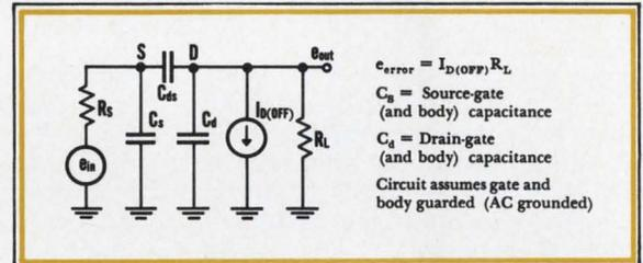
**SWITCHING:** Going from the ON condition to the OFF condition is generally the limiting case, and the important parameters are gate-to-drain capacitance, C<sub>gd</sub>, and the output load impedance R<sub>L</sub> and C<sub>L</sub>. Silicon FETs offer lower C<sub>gd</sub> for a given r<sub>DS(ON)</sub> and V<sub>P</sub>.
