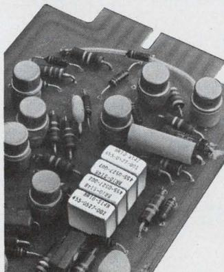
**Need 2-amp. performance?** The Model BR10 will operate dependably at 2 amps. (28 VDC), through 100,000 operations, in the temperature range  $-65^{\circ}\text{C}$  to  $+125^{\circ}\text{C}$ . Contact our Applications Engineering Group for further details.
