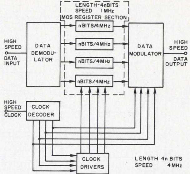
9. Clock rates can be multiplied by paralleling registers and using data modulators and demodulators. Data can enter and leave this line at 4 MHz, while individual registers are clocked at only 1 MHz. This system can be expanded.
