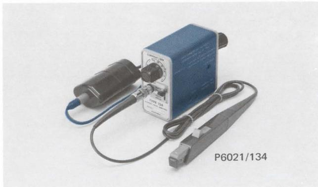
The P6021 AC Current Probe and Type 134 Amplifier provide the facility for accurate current measurements over the wide range of 12 Hz to 40 MHz without breaking the circuit under test. Used with any plug-in unit having a deflection factor of 50 mV/div, the P6021/134 provides deflection factors from 1 mA/div to 1 A/div.
