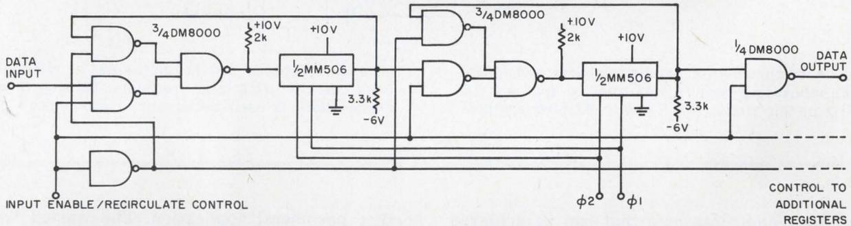
8. TTL interfaces lower register loading and improve output detection, allowing higher register
