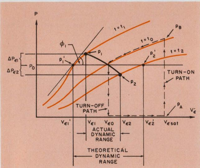
4. The effect of temperature on the output of the rf chain can easily be seen in this plot of output power vs error voltage for three different temperatures. The reference temperature is  $t_0$ ;  $t_1$  is below  $t_0$ , and  $t_2$  is above it. The dashed line shows the turn-on/turn-off locus. The solid black line is the locus of normal operation.
