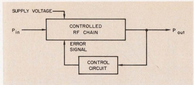
1. **Simplicity itself: the basic servo loop** consists of an rf chain and a control circuit. The chain is a series of cascaded rf amplifiers and frequency multipliers; the control circuit contains an amplifier and a stable reference voltage.
