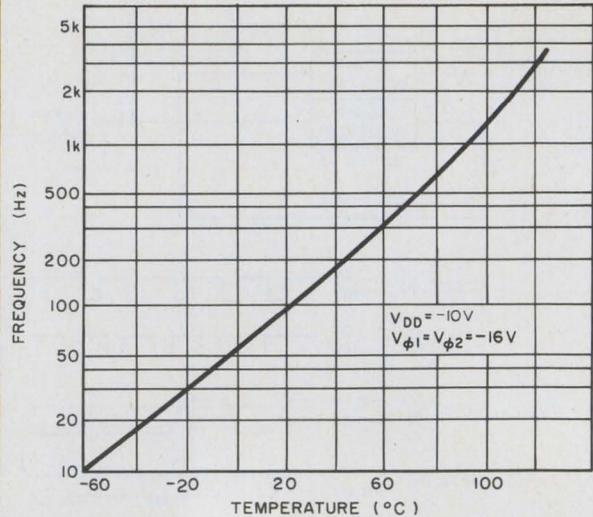
4. The minimum operating frequency of a dynamic register depends on its operating temperature. The dynamic cell does not have a feedback latch and must depend on charge-storage for retention of data. Leakage resistance, directly proportional to temperature, limits the storage time—and hence imposes a minimum operating frequency.
