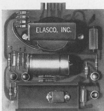
The LIC5-1A power supply is designed for mounting either on a chassis or in a 5¼" IC Basket. As many as 9 units can be mounted in a standard Elasco basket.
