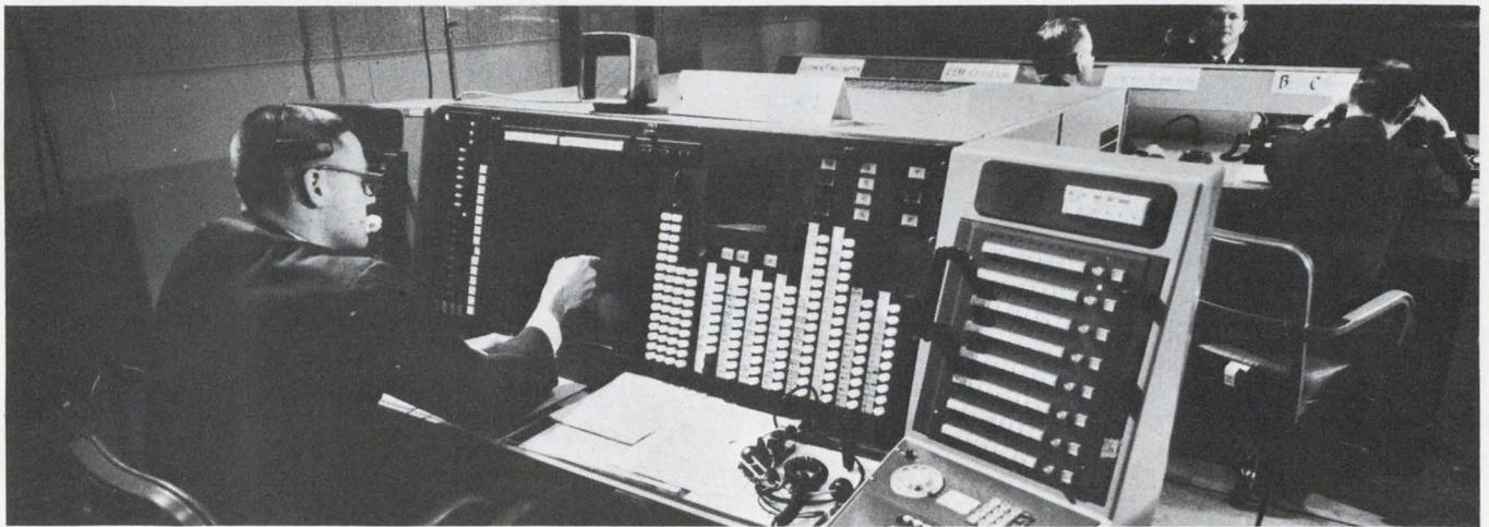
**Display for Back-Up Interceptor Center** (Buic III), which would replace a bombed-out Sage air defense network, shows twice as much
