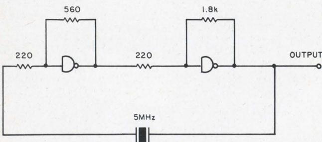
2. Highly accurate clock can be built from two linearized gates and a crystal.
