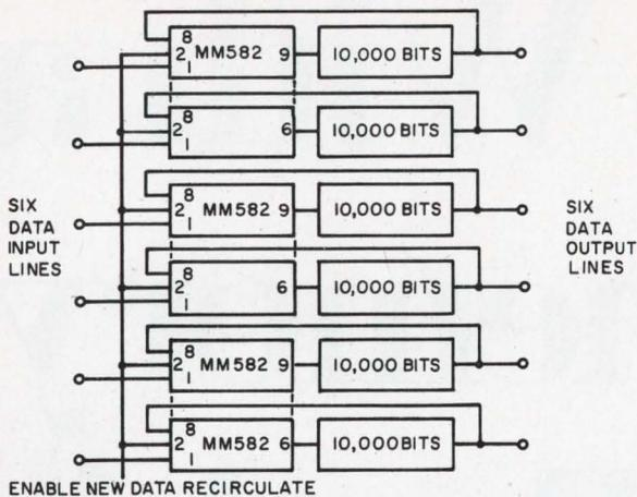
11. An MOS drum memory is a rectangular array of synchronous delay lines. This design stores 10,000 six-bit words, with MOS multiplexers handling the required input gating.
