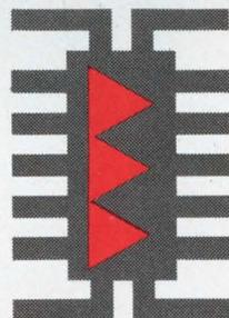
For best results, use Radiation's dielectrically isolated RA-246 at the receiving end. This 3-element buffer faithfully restores the current pulses to digital voltage pulses. The RA-246 current-to-voltage converter has built-in input terminations for balanced  $50\Omega$  lines. Outputs from each element are suitable to drive all standard saturated logic circuits (such as DTL, TTL, etc.).
