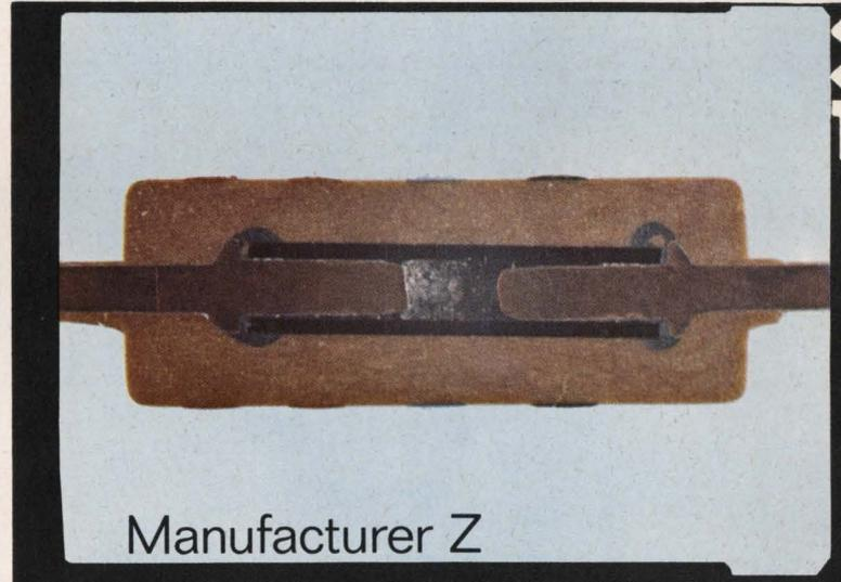
The above illustrations are from unretouched photomicrographs taken of four  $\frac{1}{2}$ -watt fixed resistors. Compare the anchoring of the leads, the seal provided by the insulating jacket at the ends, the homogeneity of the resistance material, the sharp color code bands—and decide for yourself.
