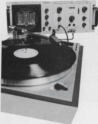
The spectrum analyzer with an **AL-2** module is often used in audio distortion measurements. Amplitudes of all frequency components in the scanned spectrum are simultaneously displayed for rapid analysis. Typical of its applications are measurement of IM distortion in transducers such as phonograph cartridges. IM products are displayed as side bands on a recorded carrier.
