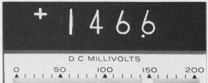
**Compact panel meters** combine digital and analog readouts in the same package. Page 110
