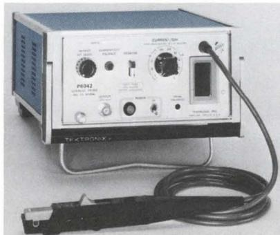
The new P6042 DC Current Probe permits measuring current flow with bandwidth from DC to 50 MHz and deflection factors to 1 mA/div.
