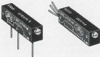
NEW Series 650. Metal Glaze resistive element built to MIL-R-22097, Characteristic C capability. ±250ppm/°C over range of 100Ω to 10K. Std. tol. ±5%.
