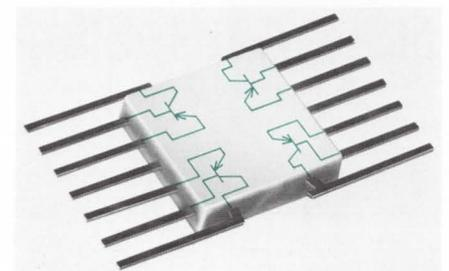
The 2N5146 "Quad," packaged in the 14-pin, TO-86 ceramic flat-pack, makes possible ultra-compact circuitry and reduces wiring requirements, to minimize lead inductance.
