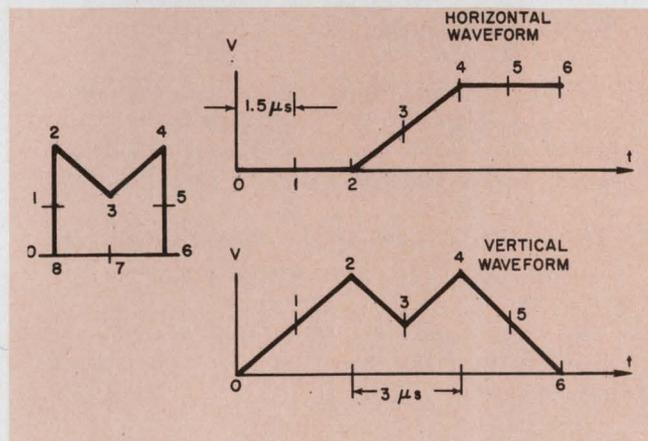
6. Straight-line approximations are used to form the characters. A maximum of 10 strokes is allowed for any symbol. For an "M" strokes 7 and 8 are blanked (return) strokes; strokes 9 and 10 are not used.
