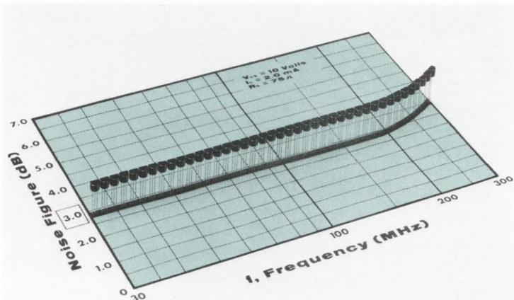
Although spec'd at 100 MHz, the 2N5208's noise figure remains typically less than 3.5 dB even out to 300 MHz—as indicated by the curve in this photo-diagram.
