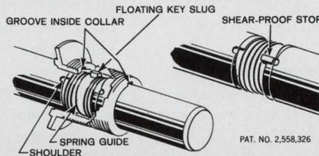
Electrical and mechanical functions of IRC metal-cased multi-turns are separate. Positive 100 oz.-in. patented stop mechanism in the shaft and bushing prevents damage to internal parts and catastrophic failure. The wiper contact assembly is relieved of stopping action. This assures setting accuracy, stability and long rotational life.
