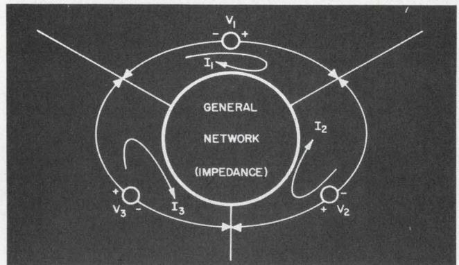
2. For a floating impedance matrix, use this network. The circuit is particularly useful for analysis of transistors and their cascaded stages.
