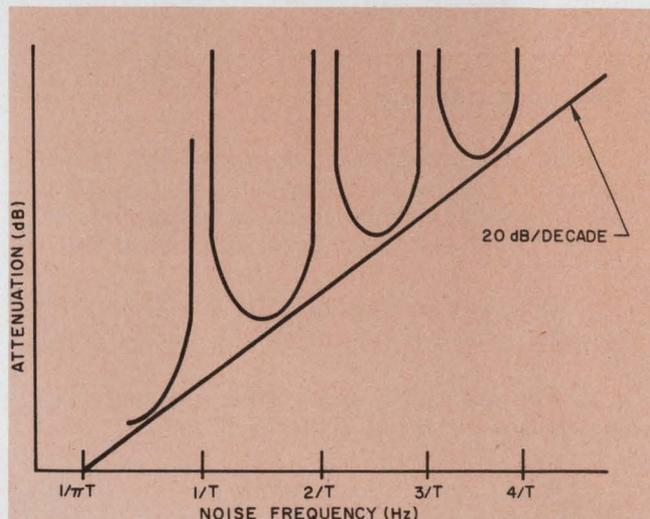
5. Infinite attenuation of noise frequencies occurs at frequencies that are multiples of the integration time.
