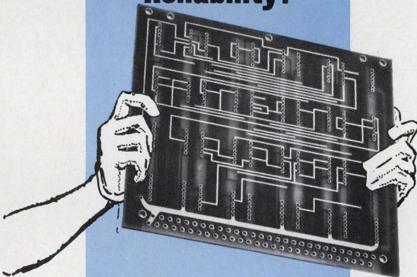
Methode's "white glove" treatment—we call it SUPER-SOLDERABILITY—on every production lot is your guarantee of printed circuit solderability. The only hands that touch a Methode board after its final cleaning operation are those of an inspector . . . with white gloves.
