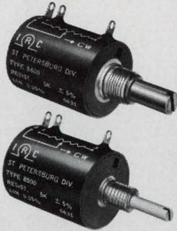
High performance and long life at lowest cost. 10 turns,  $\frac{1}{8}$ " diameter with only  $\frac{1}{16}$ " behind the panel. 2 watts @ 25°C., derates to zero @ 105°C. 100Ω to 100K, with all popular intermediate values.  $\pm 5\%$  tolerance and  $\pm 0.25\%$  linearity. Side terminals accept to #14 wire. Model 8400 has  $\frac{3}{8}$ "-32 bushing,  $\frac{1}{4}$ " shaft. Model 8500 has  $\frac{1}{4}$ "-32 bushing,  $\frac{1}{8}$ " shaft.
