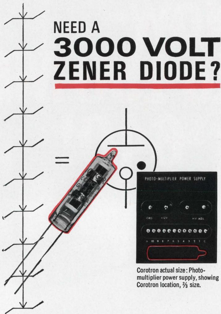
Corotron actual size: Photo-multiplier power supply, showing Corotron location, 2/3 size.
