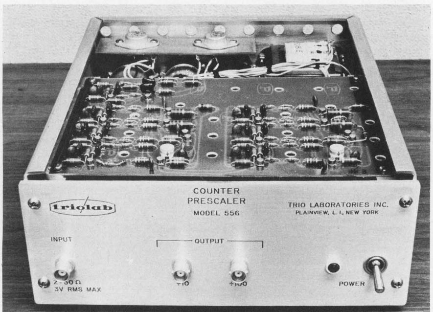
Any counter's scale can be extended 10 or 100 times higher with this
