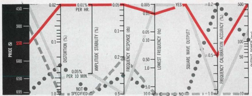
IMPORTANT OSCILLATOR PARAMETERS are plotted for four competing solid-state instruments. The plot for the K-H Model 4100 (color) is compared to other units with lower and higher price tags. Relative position of each parameter was determined by its value to the instrument user, not by its number. Thus the lowest price has
