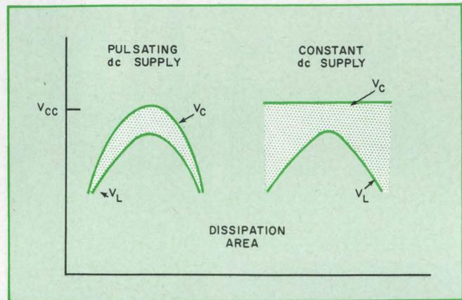
**A pulsating dc supply** may be used in Class-B circuits to reduce collector-to-emitter voltage and hence dissipation. Since the collector-to-emitter voltage equals the difference between the supply and the output voltages, it will approach zero as the output voltage increases.
