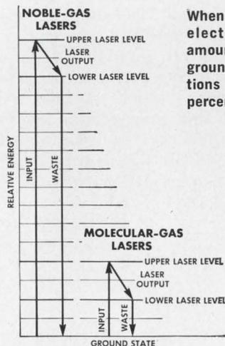
When a laser operates through energy stored in electron orbits (left), a comparatively large amount is wasted through the long return to ground state. But, when energy is stored in vibrations and rotations within a molecule (right), the percent wasted is much smaller.
