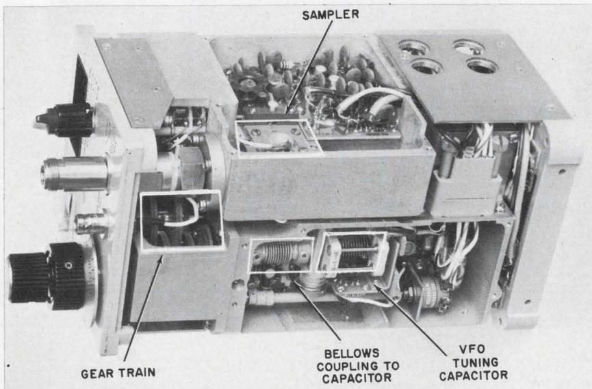
Plug-in's interior shows the cast aluminum chassis and the 636-to-1 gear train, which can position the capacitor rotor within  $1/12,000^\circ$ .
