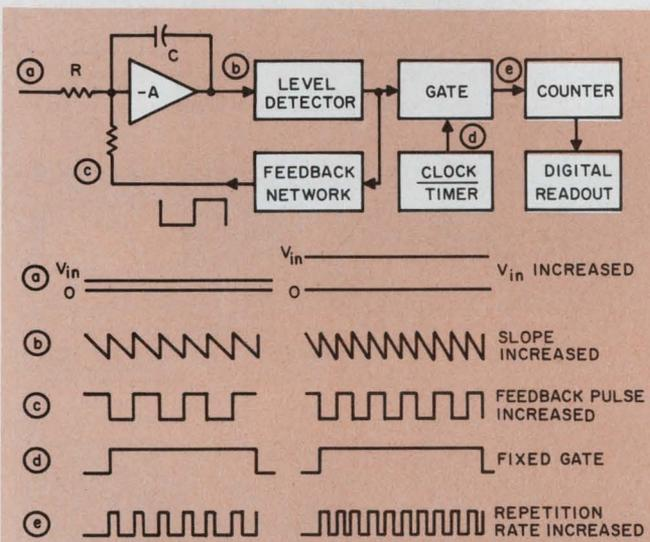
4. Voltage-to-frequency integration is fast and quiet. Accuracy, however, is a a problem for three reasons: C drifts with time and temperature, the clock frequency can shift and zero offset voltages can occur around the integrator input.
