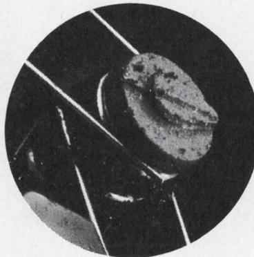
Brush assembly of conventional synchro after 1000 hours
