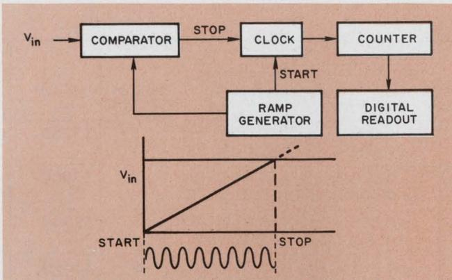
3. Ramp conversion measures the time it takes for the linear ramp to go from 0 to  $V_{in}$ . When the clock pulses stop, their duration is indicative of  $V_{in}$ .
