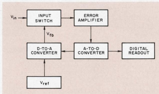
1. **Null-balance system** is susceptible to noise, since the error amplifier will sense any input noise and drive the system out of balance.
