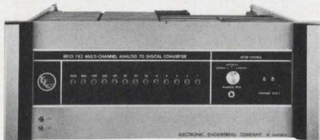
Only the EECO 762 Multi-Channel Analog-to-Digital Converter gives continuous overvoltage channel protection. You get uninterrupted operation with transient overvoltages up to 125 VRMS on any input channel.
