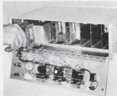
Seven plug-in circuit boards make up the diffusion furnace controller.
