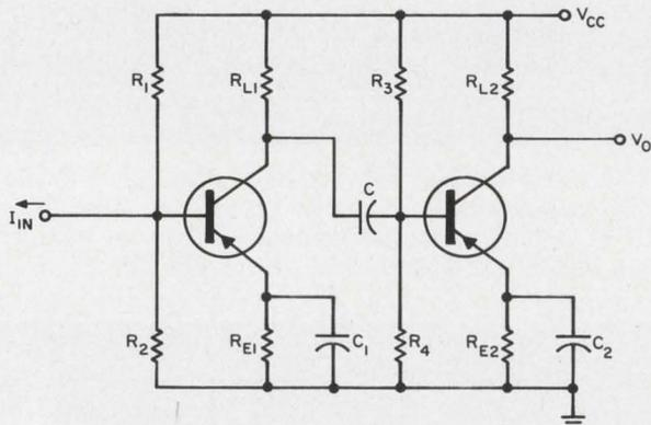
The combined cascaded network derived in connection with Fig. 6 can be applied to the analysis of this amplifier circuit. The transistor is a 2N1925, a pnp germanium, general-purpose, medium-power device. The  $h$  parameters obtained from the data sheet and typical values are:
