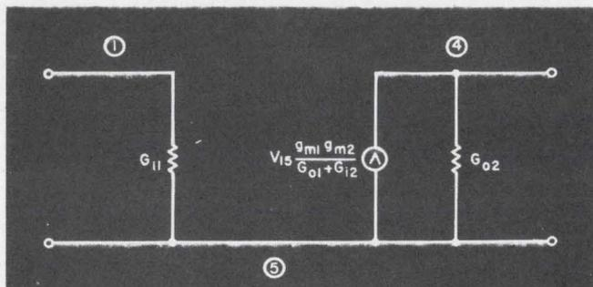
7. Equivalent circuit of a transistor amplifier. Its matrix is derived in the text with the aid of standard matrix reduction techniques.
