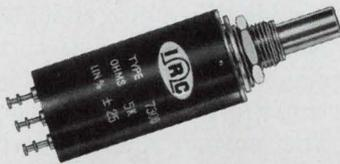
Model 7300 has 100 oz.-in. patented stop system and space-saving rear terminals. 10 turns, 2 watts @ 40°C., derates to zero @ 85°C. 100Ω to 100K.  $\pm 5\%$  tolerance,  $\pm 0.25\%$  linearity.
