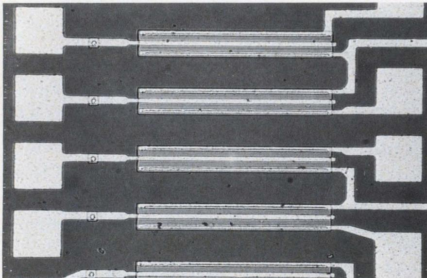
Dielectrically isolated MOS devices are used in five-channel multiplex switches fabricated on a polycrystalline silicon passive substrate by TRW Systems.
