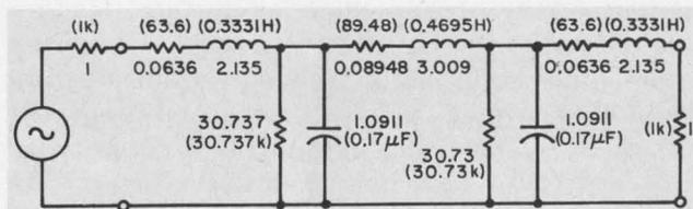
6. Chebyshev band-pass filter has a pass-band ripple of 1 dB and a bandwidth of 1020 Hz, which guarantees a 1-kHz bandwidth between the  $2\text{-dB} \pm 0.5\text{-dB}$  points. The final component values in parentheses reflect the changes from low-pass to band-pass.
