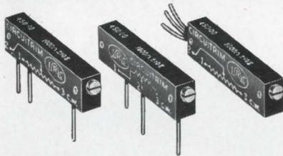
Series 450. Metal Glaze element provides essentially infinite resolution output. RJ-12 size to MIL-R-22097 requirements. Resistance values from 50Ω to 1 Meg. Standard tolerance is ±10% with 20% available for cost-saving applications.
