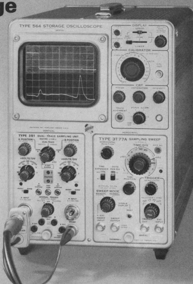
**The Tektronix Type 564** split-screen storage oscilloscope with the Type 3T77A sampling time-base and the new Type 3S1 dual-trace sampling vertical is a DC-to-1 GHz measurement system with the unique capabilities of split-screen storage.
