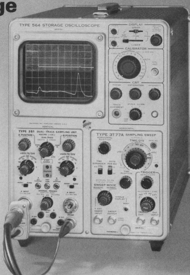
**The Tektronix Type 564** split-screen storage oscilloscope with the Type 3T77A sampling time-base and the new Type 3S1 dual-trace sampling vertical is a DC-to-1 GHz measurement system with the unique capabilities of split-screen storage.
