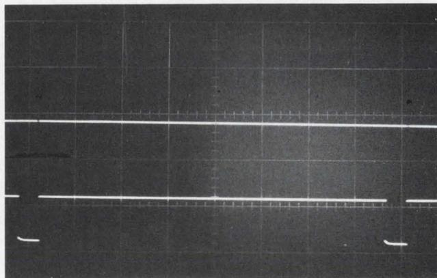
Long-duty-cycle multivibrator (top) uses only one discrete component,  $C_T$ . Upper trace (bottom) is the set pulse, lower trace is the output pulse. Horizontal scale is 500  $\mu$ /cm, vertical is 5 V/cm.
