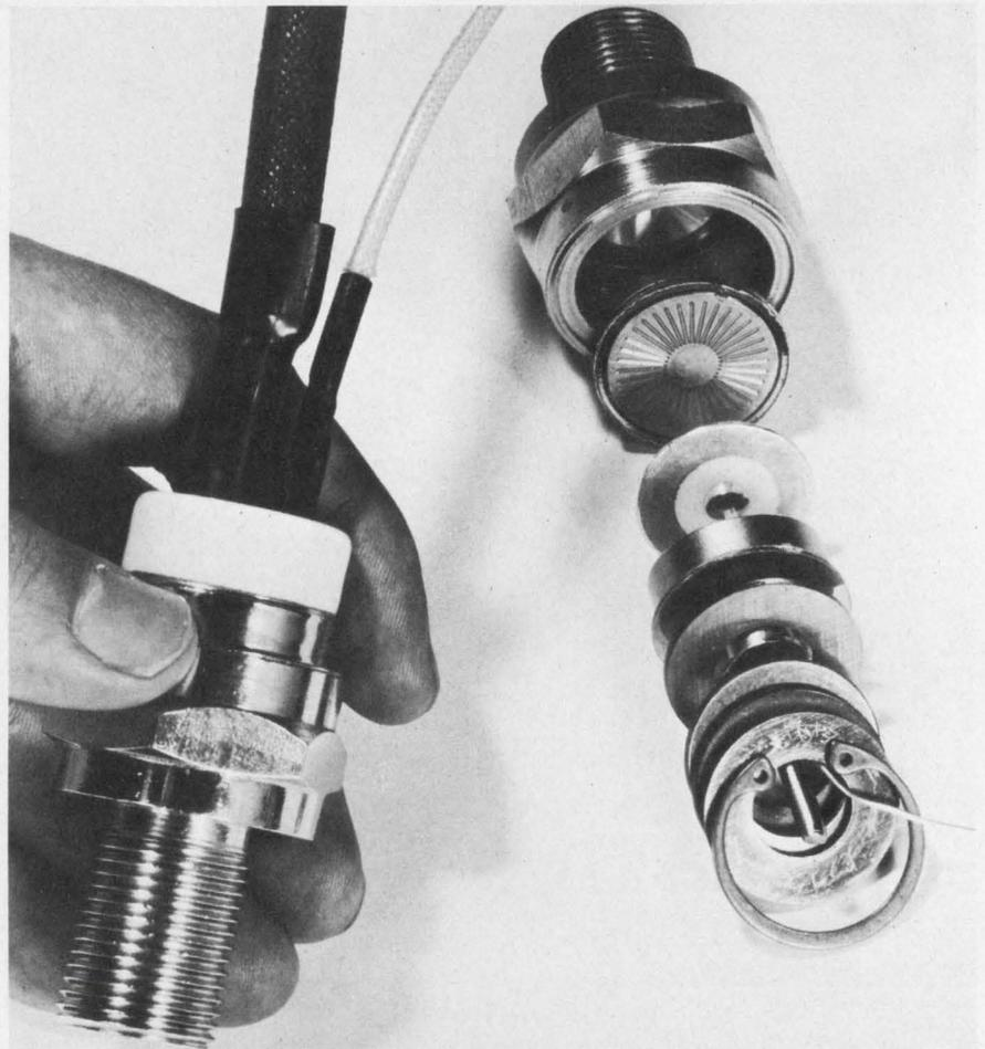
Compression-bonded encapsulation is what holds this transistor's junction in place. This technique eliminates soldering and uses spring pressure.
