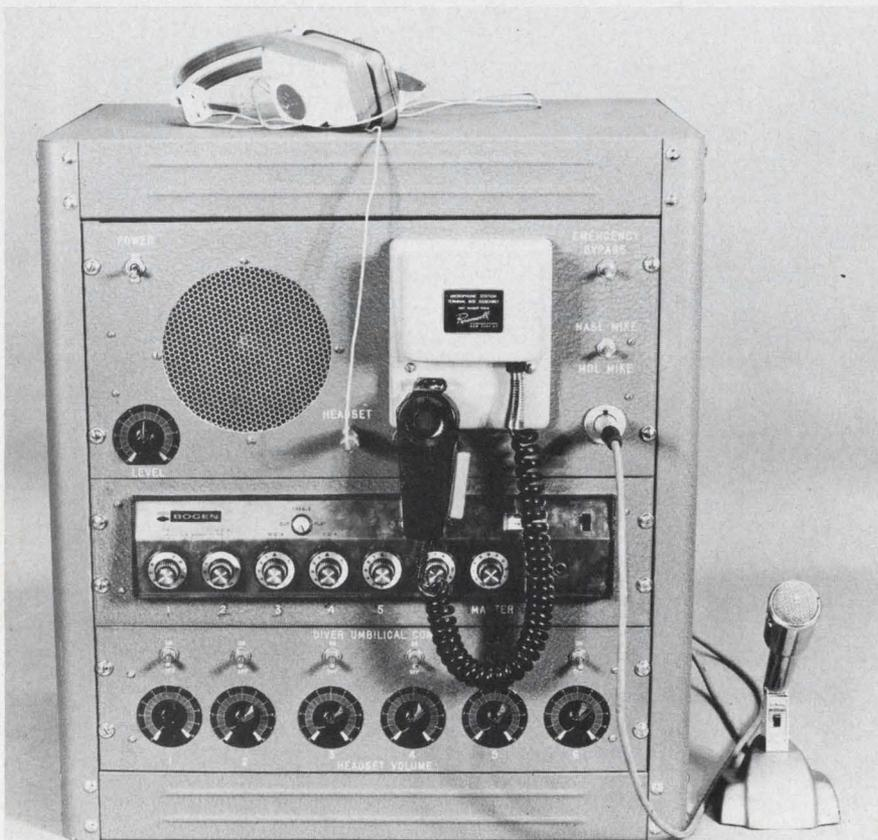
**Navy-built aquanaut phone system** accepts calls from six divers and a seabed base. Speech makes round trip to surface, where it can be corrected for helium distortion before it is returned and redistributed.
