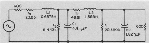
4. Low-pass Butterworth filter is designed with a bandwidth that ensures the specified response in the specified range. Resistances  $r_2$  and  $r_4$  stand for core and copper losses and  $r_1$  and  $r_3$ , for losses in the capacitors.
