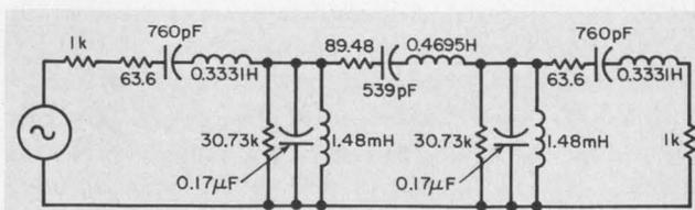
7. The resonant circuits in the Chebyshev filter are completed by adding the shunt inductances and series capacitances. The capacitors may be considered lossless. This can be closely approximated with high-quality filter capacitors.
