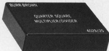
This new, low-priced, encapsulated Burr-Brown quarter-square multiplier is a precision analog function module capable of performing accurate four-quadrant multiplication, two quadrant division as well as square and square root functions. Accuracy is  $\pm 0.5\%$  max. Bandwidth at 1% abs. error is 5kHz. Rated input:  $\pm 10V$ . Rated output:  $\pm 10V$ ,  $\pm 5mA$ . Module size: 2.4" x 1.8" x .60".
