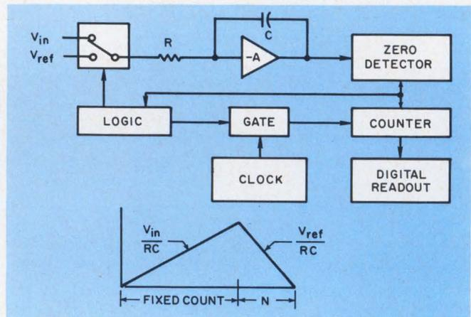
6. Dual-slope integration is accurate, fast, and quiet. Long-term accuracy is high, since shifts in  $C$  are compensated for by shifts in  $V_{ref}/RC$ . Even if the clock frequency varies, the reading will remain correct.
