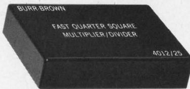
The 4012/25 is a high-speed, fully encapsulated quarter-square multiplier containing three wide-band operational amplifiers and two precision diode squaring circuits. It performs precision four-quadrant multiplication and two-quadrant division as well as square and square root functions. Accuracy is  $\pm 0.25\%$  max. Bandwidth at 1% abs. error is 40 kHz. Rated input is  $\pm 10V$ .
