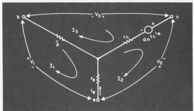
4. Low-frequency T model of a transistor is in floating form. The impedance matrix is found in the text.
