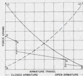
Curve CA — Balanced-Force Relay normally closed contacts.
