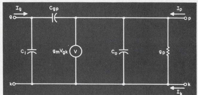
3. Equivalent circuit of a pentode helps establish the appropriate floating admittance matrix. One matrix is sufficient to describe all modes of operation.
