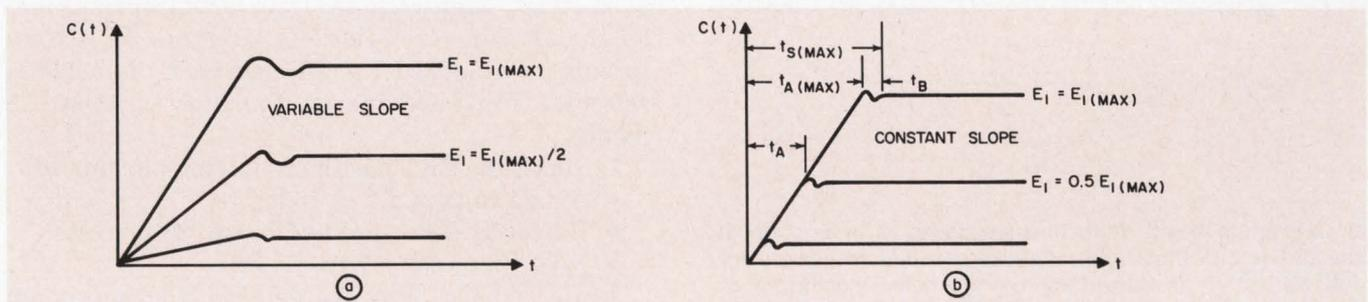
4. Both positioning time,  $t_A$ , and settling time,  $t_s$ , are functions of the yoke voltage  $E_1$ . Ideal deflection ampli-
