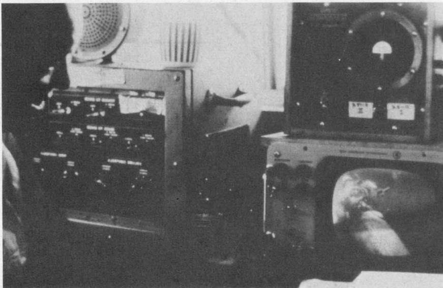
**Westinghouse surface station** has an underwater TV monitor, telephone switchboard and a terminal for each diver's oxygen sensor telemeter.
