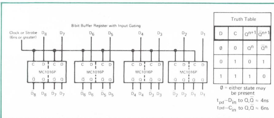
Here's an easier, less-complex and less-expensive way to construct an 8-Bit Buffer Register using just four dual-function MC1016P MECL II integrated circuits! These new dual R-S flip-flops reduce can-count (and system cost) by
