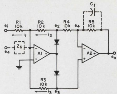
1. Ideal rectifier circuit with equal resistors really works. Design equation is Eq. 3.
