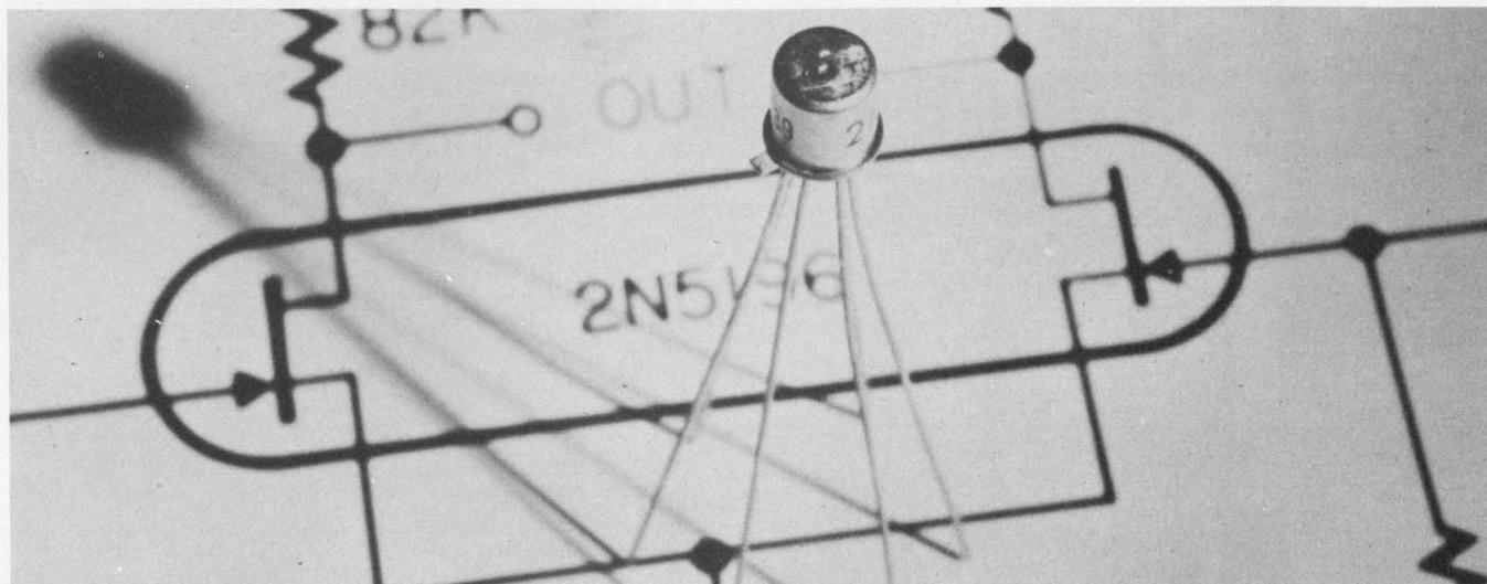
Matched FET-pairs track from  $5\mu V/^\circ C$  with an input (gate) current of 15 pA. Page 116
