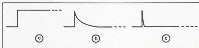
2. The input step (a) is differentiated by the circuit in Fig. 1a. Large RC products yield long trailing edges (b), small RC products have sharp skirts (c).
