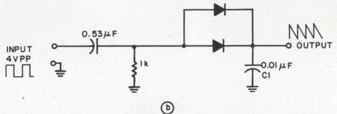
Sawtooth is obtained when a sine, square, or triangular waveform of 4-V pk-pk is applied to the input (a). For square waves the circuit reduces to (b). Two diodes are used to lower output resistance to increase rise time.
