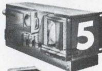
**Bina-View Readout:** Accepts binary or teletype code, decodes, and displays the proper character.
