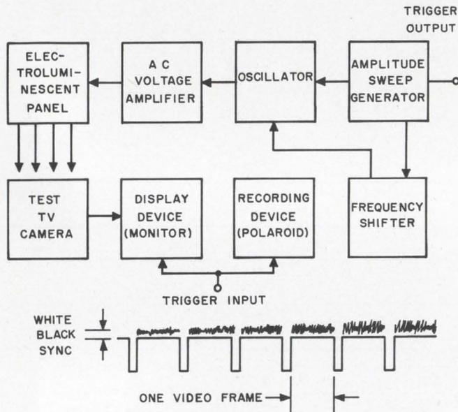
**Solution:** Measure the light from a calibrated electroluminescent panel as a function of the current output of the image sensor. The plot of current output vs the calibrated light output of the electroluminescent panel is the transfer characteristic of the vidicon.
