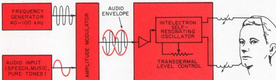
2. Device pumps rf signal into head and nerves demodulate the audio. Insulated electrodes act as plates of a capacitor, and tissues as the dielectric, in a series-resonant LC circuit. Unit handles speech as well as pure tones. Self-resonating oscillator adjusts to shifts in electrode placement.
