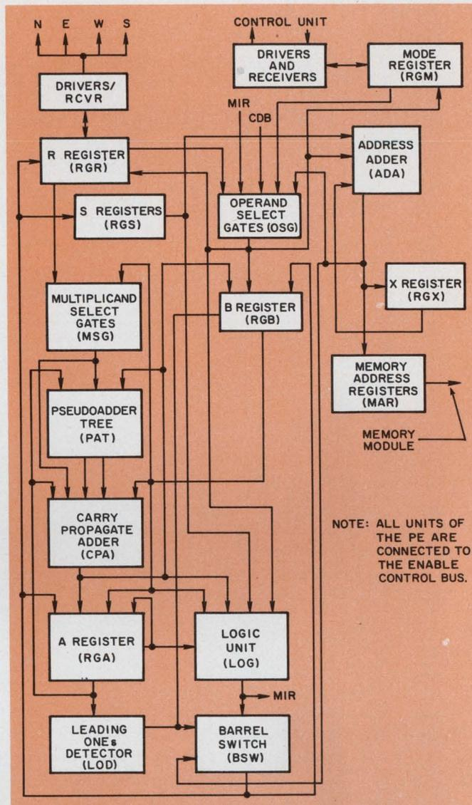
7. The processing element has three principal registers. It will be built from 64-pin ECL logic packages. Instruction execution times are typically 200 ns for floating point add and 400 ns for floating point multiply.
