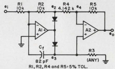
2. Degenerate form of ideal rectifier uses only four precision resistors.
