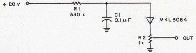
Fast pulses are obtained from a circuit that can be built in about 10 minutes.
