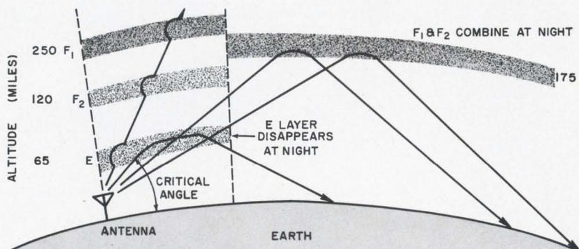
Three ionospheric layers are generally available in the daytime for bouncing high-frequency radio signals down over the horizon to missile sites. At night, the lowest layer, the E region, disappears, and the two layers (F<sub>1</sub> and F<sub>2</sub>) of the upper F region combine to form one. If the angle of transmission is greater than the critical angle, the signal will pass right through the ionosphere and not be returned.
