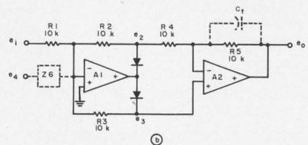
Full-wave rectifier amplifies equally with the value of  $R_3$  shown here.
