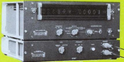
General Radio Type 1680 Bridge automatically measures capacitance and loss simultaneously, generates coded digital output data, and displays measured values in about one-half second. The basic accuracy is  $\pm 0.1\%$  and the range is from 0.01 pF to 1000  $\mu\text{F}$ .
