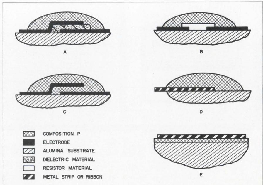
Elastic ceramic material serves as a hermetic encapsulant for printed thick-film capacitors (a) and resistors (b), a dielectric for printed capacitors (c), an elastic clamp for joining a metal ribbon to a ceramic substrate (d), or a bonding cement for a metal-to-ceramic seal (e).
