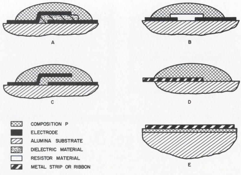
Elastic ceramic material serves as a hermetic encapsulant for printed thick-film capacitors (a) and resistors (b), a dielectric for printed capacitors (c), an elastic clamp for joining a metal ribbon to a ceramic substrate (d), or a bonding cement for a metal-to-ceramic seal (e).
