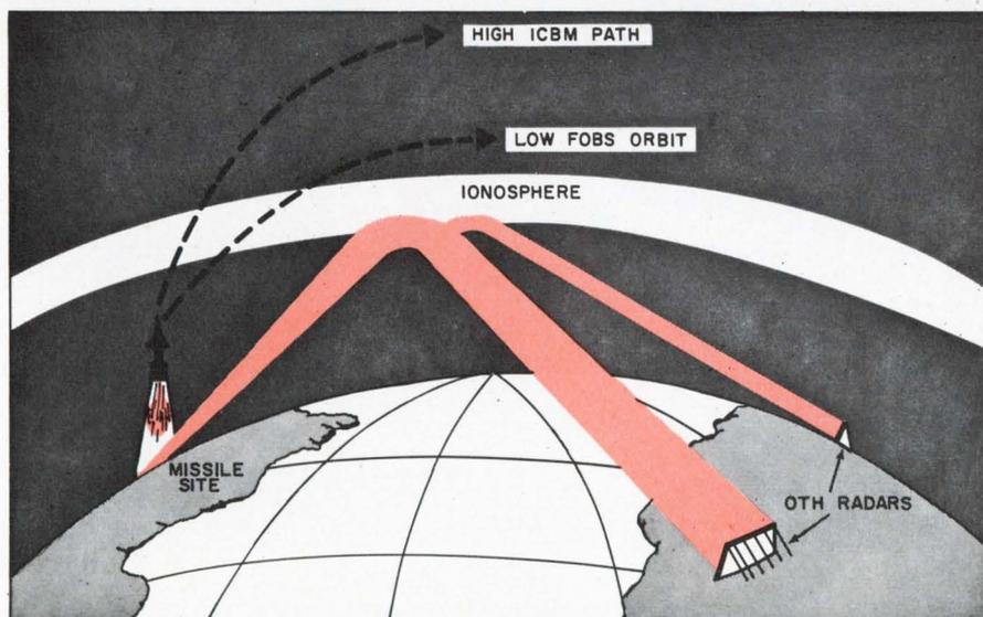
Over-the-horizon radar avoids line-of-sight restrictions by bouncing off the ionosphere to detect launchings of ICBMs and FOBSs alike at the site. A signal that bounces off the horizon only once can reach a target as much as 2000 miles away. Those that zigzag up and down twice or more reach much farther.
