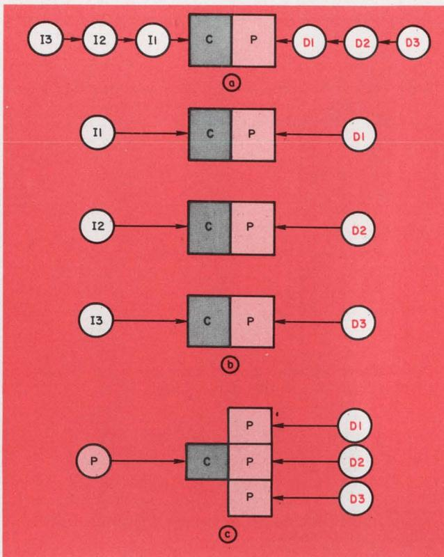
1. **Development of parallelism** began with the aim of improving the throughput of the pipeline computer (a). Simply paralled identical processors (b) executing the same program could have common control logic (c).
