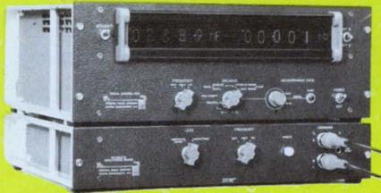
General Radio Type 1680 Bridge automatically measures capacitance and loss simultaneously, generates coded digital output data, and displays measured values in about one-half second. The basic accuracy is  $\pm 0.1\%$  and the range is from 0.01 pF to 1000  $\mu$ F.
