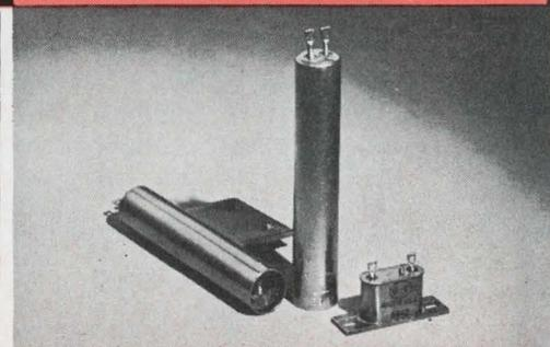
**Cartridge Type:** Series C8 hermetically sealed and still adjustable. Contact rating up to 5 amps. **Crystal Can Size:** Series VE-2 hermetically sealed. Contact rating up to 3 amps. **Features:** Rapid rate of response; minimal differential; operating range,  $-65^{\circ}$  to  $+300^{\circ}\text{F}$ ; vibration to 2000 Hz; shock to 50g.
