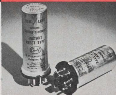
Instant reset during or after timing is available, by combining G-V's unique instant reset timing element with a magnetic relay. Widely used in communication systems and data processing equipment. **Features:** Delay time, 2 sec. to 5 min.; ambient operating temp., 32°F to 185°F.
