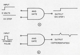
1. Noise feedthrough in ICs measured by dc testing (a) is not adequately determined; it must be established by dynamic pulse means (b) so that output truly reflects filtering action of the circuit.
