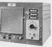
The NA Series of AC Power Supplies are exceptionally flexible sources of audio power. Each power supply consists of a Regulated Audio Power Amplifier with interchangeable fixed or variable Plug-In Oscillators for a wide range of precision AC power applications. The Amplifier has a full power range of 45-6,000 cycles. With the incorporation of a CML Plug-In Oscillator precise fixed or adjustable output frequencies are available anywhere within this range. For complete information, write today.
