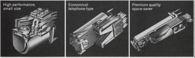
CLASS E RELAY. A lightweight space-saver with most of the features of the Class B. Life exceeds 200 million operations. Industry's widest terminal options: taper pin, integral socket, conventional solder, taper-tab, solderless wrap and printed circuit terminals.
