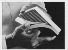
Tough, flexible G-E RTV silicone for moldmaking reproduces detail accurately and minimizes tooling costs.
