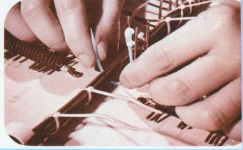
**Position Clamps and Identifying Straps** directly on the harness for further time saving and reliability. As the harness is being fabricated, the *T&B TY-RAP* clamp/tie can be installed. It serves two functions — as a tie and as a clamp. By pre-positioning the clamp, the installation of the harness in the equipment is made quicker and easier.
