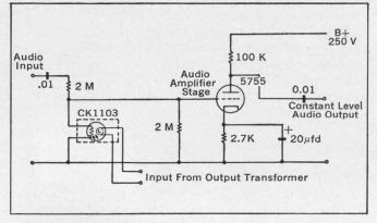
**1. Use the Raysistor**<sup>®</sup> as a simple remote or automatic volume control in SSB suppressed carrier receivers. Feeding part of the audio output into the control light source varies the resistance of the Raysistor's photocell, making it usable in place of a normal volume control.
