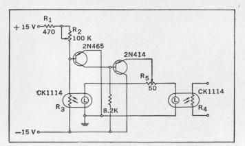
2. As a remotely controlled linear potentiometer. The Raysistor can be used as a remotely controlled linear potentiometer when used in the circuit shown above. Here the Raysistor forms a voltage divider between the positive and negative voltages.
