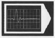
Typical Photograph of Crosscorrelation Function of Input and Output Signals of Complex Passive Network Driven by White Noise.
