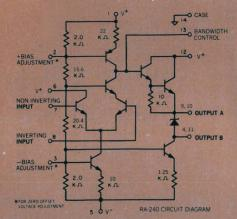
Radiation's dielectric isolation and thin film technology, in conjunction with a virtually ideal circuit, permits design of high Q active filters with high initial attenuation. The Radiation RA-240 IC Amplifier has an extremely high internal feedback impedance, and allows wide flexibility in the choice of external filter components without regard to the active element of the circuit.
