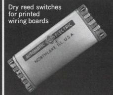
PRINTED CIRCUIT CORREEDS.\* Strong, moisture-resistant, compact. Unstressed contact leads provide firm, positive connections. Glassfilled plastic bobbins prevent moisture absorption. Low profiles and magnetic shielding permit high density within standard PC terminal spacing (multiples of 0.200 inches). Available with 1, 2, 3 and 5 capsules and magnetic latching. Contact forms A, B, & C.
