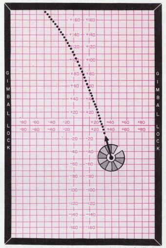
5. All attitudes are shown at once on the attitude display. The display uses a map of yaw and pitch projected on a plane instead of on a ball.
