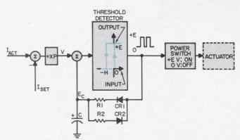
2. **Proportional amplifier output is fed to a detector,** where it is converted to a variable-width pulse. This pulse controls a solid-state switch that, in turn, activates the actuating relay.
