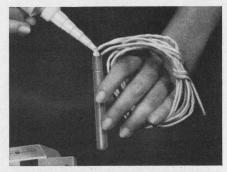
G-E RTV is ideal for high temperature moisture sealing of heating elements. It withstands temperatures as high as  $600^{\circ}$ F, as low as  $-75^{\circ}$ F.
