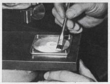
G-E two-part RTV, available in a range of viscosities, seals filament condenser plate in dielectric heater. Also protects against vibration.
