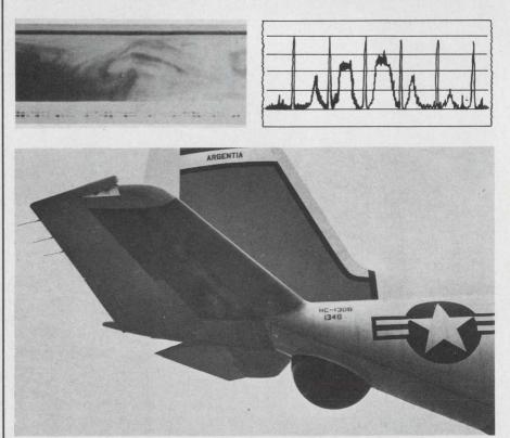
**Iceberg shows up** as a dark shadow on a graphic display (above left) and as a temperature-analog plot on a recorder (above right) in Sperry's airborne microwave radiometric search system. The black dome under the tail of the Coast Guard HC-130 aircraft contains three parabolic antennas that rotate perpendicularly to the flight path.
