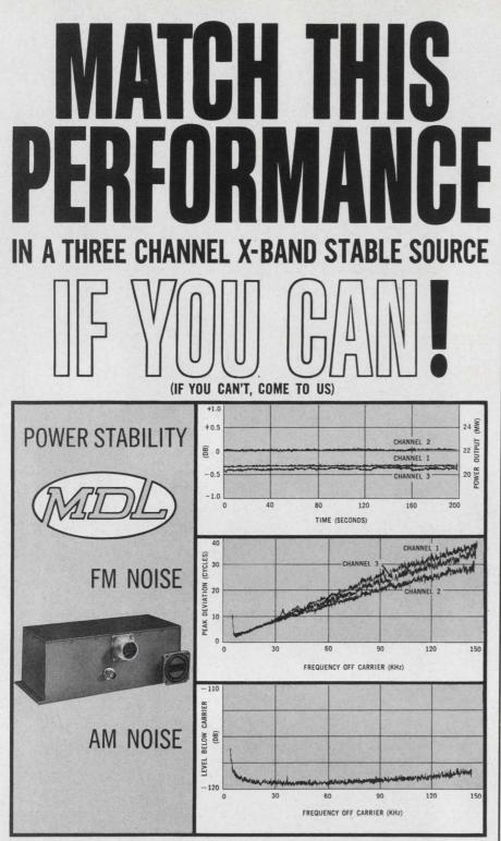
**OUTPUT POWER:** 20 MW  $\pm$  0.5 db at any of three discrete frequencies in a 150 MC bandwidth factory adjustable 8-12GC.
