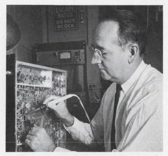
Breadboard model of composite filter, tested by author Noble, is designed for a 20-MHz flow meter.
