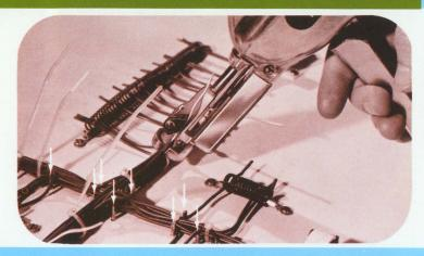
**Drop Nails and Apply Ties** to complete the harness with maximum convenience. This feature of the *T&B TY-RAP* harness board increases the ease and speed of applying and tying the cable ties. Further speed and convenience is gained with the new *T&B TY-RAP* pistol-tool WT-295. One squeeze of the trigger and the tying is completed.
