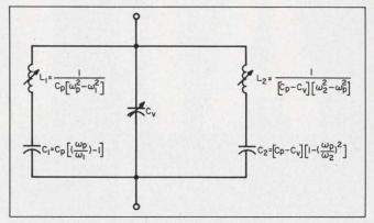
1. Simple filter replaces a cascade of resonant circuits at the output of mixers and frequency multipliers. It effectively suppresses unwanted pairs of frequencies at the opposite sides of the selected frequency,  $\omega_{n}$ .
