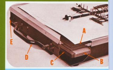
NEW Mechanized Harness Board allows further cost reductions and increased production. The board controls the height of the wire routing nails. It consists of (A) a stationary perforated metal surface over (B) a wooden backing board which is (C, carried in a movable metal frame controlled by (D) handles located on each side. Unlock the handles and the board (anc nails) lower to (E) a preset level. It's an entirely new way of harnessing.
