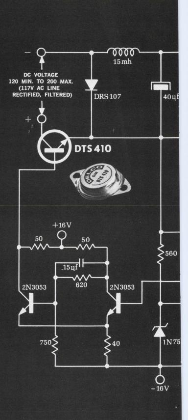
Application of Delco high voltage silicon power transistor
