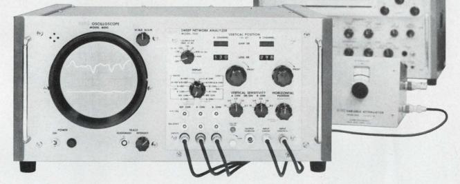
Now, with one totally new instrument, measure gain, loss, absolute or relative power levels, VSWR, and impedance magnitude (reflection coefficient). The new Alfred 8000/7051 system speeds and simplifies rf and microwave measurements.
