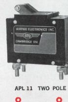
COMPLETELY MAGNETIC TIME DELAY AND TRIP. CONTAINS NO HEATING ELEMENTS. AVAILABLE 50 MA TO 50 AMPERES AC OR DC. 50, 60 AND 400 CYCLES.
