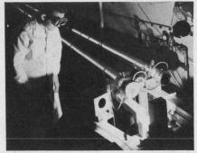
A doubled-barreled Raytheon carbon dioxide laser is said to be the mightiest in existence. It produces more than one kilowatt of output power.
