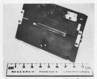
millipounds of thrust and consumes 33 W. The linearstrip engine at right produces a thrust of about one-half millipound with about 100 W input power.
