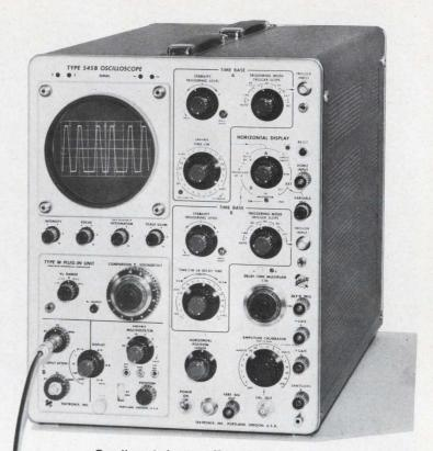
Small spot size – uniform focus The waveform demonstrates the small spot size and uniform focus which provides fine trace definition.
