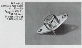
RCA brings you a new generation of control devices! Each of these 6-amp Triacs can provide the same full-wave function as two SCRs... with the option of using either positive or negative gate-trigger signals. Hermetically sealed in an allwelded TO-66 package, RCA 40429 and 40430 can simplify your control circuits ... reduce costs ... add reliability and efficiency.
