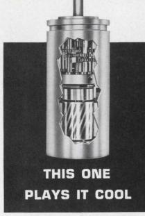
One continuous stainless steel case houses both motor and gearhead in Harowe integral-geared servo motors. There are no joints to block heat flow; no dissimilar metals to expand unevenly. Result is cooler motor operation and excellent thermal stability.
