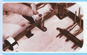
**Set Up Harness Board Aids** to suit your present fabrication. Shown here are smooth, molded, nylon corner posts, plastic chutes and bundle retainers. These simplify wire routing and hold harness above board for easy tying. The new *T&B TY-RAP* bundle shaper-retainer has a slotted foam center which expands to accept the wires as they are positioned for harnessing.
