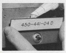
Screws and drilling are eliminated by adhering identification plates with RTV adhesive sealant. It won't harden, soften, crack or shrink.
