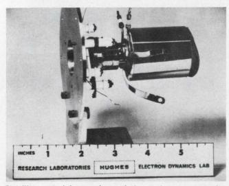
Satellite-control ion engines of the cesium contact type are under development at Hughes. The variable thruster at left can be deflected in two directions. It produces 0.1
