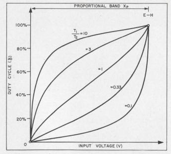
4. Different ratios of charge-discharge times alter controller linearity. Adjusting R1 and R2 in the charging and discharging circuits alters any nonlinear input and makes it almost perfectly linear.
