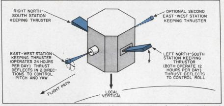
A proposed synchronous satellite would use ion engines for north-south and east-west station keeping and for three-axis attitude control. The 1000-pound Hughes satellite would have a 50-pound propulsion system including solar cells capable of furnishing about 80 W.
