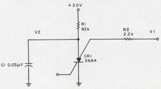
1. Key to the operation of the relaxation oscillator is the value of R1. Its value must be high enough to keep the ON current of the SCS below its holding current.
