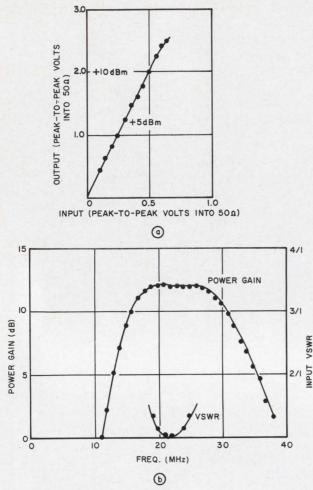
3. Linearity (a) and power gain and input vswr vs frequency curves (b) show performance achieved in the resulting circuit.
