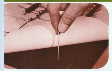
**Insert Routing Nails** through wiring diagram into perforated holes and screw down. While routing hardware is necessary and desirable during the wire layout stage, it is cumbersome and tends to slow tying operations. The *T&B TY-RAP* "Pop-UP" Board eliminates the problem. It allows routing pins to be adjusted to optimum height for all harnessing operations — they can be dropped level with the board's surface for tying.
