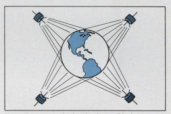
**Extremely accurate timekeeping is possible** for everyone through satellite-transmitted standard time signals. The satellites beam the signals world-wide, allowing them to synchronize all electronic or electromechanical watches capable of receiving and processing them.
