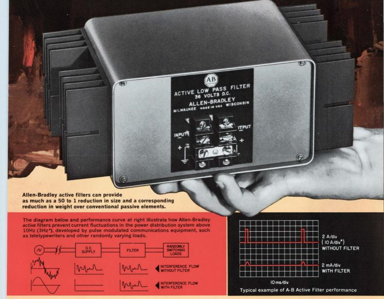
■ Directly as the result of some new ideas applied to the field of ElectroMagnetic Compatibility, Allen-Bradley has been able to produce a new *active* low pass filter that provides an attenuation of greater than 60 db over the range of 10Hz (3Hz\*) to 100KHz. The maximum dc component of the load current is 5 amperes.
