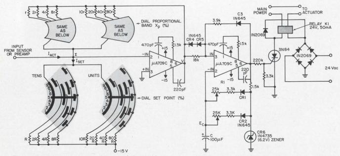
5. Time-proportional control uses binary-coded switching to select the reference signal (I $_{\rm set}$ ) and the proportional
