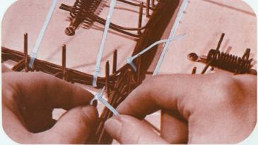
**Form Harness** by strategically positioning *TY-RAP* ties wherever bundle separates or turns. The new friction grip head allows *T&B TY-RAP* cable ties to hold bundle without being completely tied. The advantage of forming the harness is mainly ease in handling for increased speed in complete tying.
