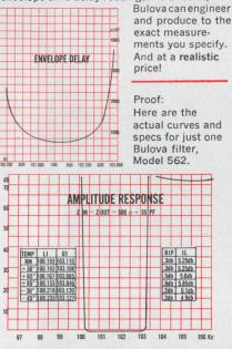
Bandwidth (1db) 100.255 to 103.035 Kc Bandwidth (60 db) 99.990 to 103.260 Kc Carrier frequency — is 100 Kc Loss at carrier — 55 db min. Ultimate attenuation — 70 db Max. insertion loss — 6 db Max. ripple — 1 db max. Operating temperature —  $-40^{\circ}$  to  $+65^{\circ}$ C Impedance —  $500^{\circ}$  (in and out) Differential envelope time delay —  $500 \ \mu$ sec max. over 80% of pass band
