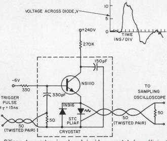
Silicon transistor is placed inside cryostat for efficient pumping of gallium-arsenide laser diode.
