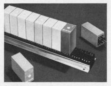
G-E RTV provides attractive, protective packaging for components. Each unit is encapsulated in a different color RTV for easy identification.
