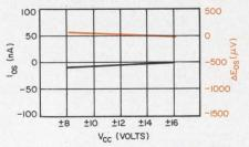
1. Virtual immunity from power supply variations is evident as offset voltage and current remain nearly linear as the supply varies from  $\pm 8$  to  $\pm 16$  V.
