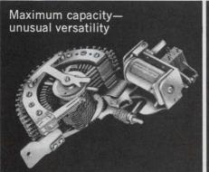
TYPE 45 ROTARY STEPPING SWITCH. Larger CLASS V MERCURY-WETTED RELAY. For comcapacity: up to twelve 25-point levels, eight 50-point levels. For any DC voltage up to 110, or 115 volts AC with rectifier. Can be impulsecontrolled or self-interrupted. Available with normally open or normally closed circuits (Type 45NC). Also available as prewired, hermetically sealed units.
