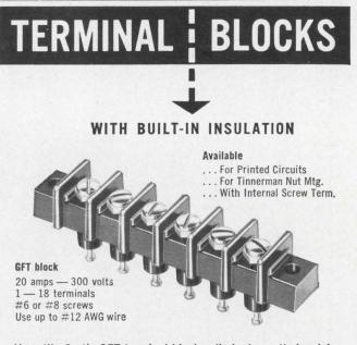
Versatile Curtis GFT terminal blocks eliminate costly insulating and mounting procedures, when complying with UL and CSA requirements. Fully insulated, GFT blocks give you ¼" solder terminal to ground clearance on ¼" thick chassis. Excellent conductivity. Terminals are bright tin plated.
