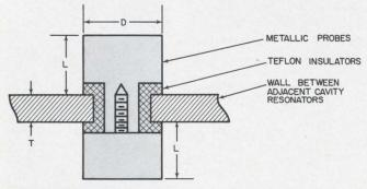
1. **Capacitive probe mechanism** can increase or decrease the interstage coupling of microwave cavity-type filters. The probe's length, L, changes the air gap between the center conductor of the resonator and the metallic partition separating the cavities.
