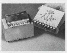
Impregnation of transformer coils with G-E RTV provides electrical insulation and environmental protection at high temperatures.
