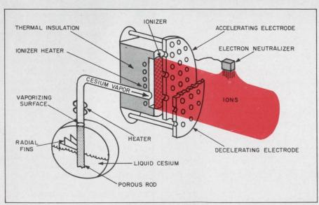
**The contact ion engine,** one of two important electrostatic thrusters (the other is the electron-bombardment type). The essential components of both types are an ionizer, a high-potential grid, or electrode, and a beam-neutralizing electron source.
