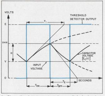
3. Since the detector output is a switched signal, it introduces noise spikes in the system. To prevent this interference, the pulse, at a 50% duty cycle, should have a frequency outside the pass-band of the op-amp.
