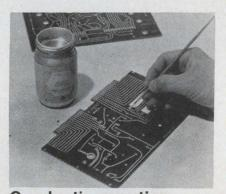
Conductive coating contains Ag particles Acheson Colloids Co., Port Huron,
