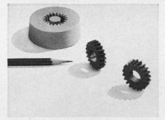
For prototypes or short-run parts production, G-E RTV is an excellent flexible moldmaking material. And it needs no release agent.
