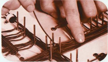
**Routing Wires for a Complex Harness** is convenient with the adjustable nails. With the *TY-RAP* harness board, the nails can be set at maximum height when the operator begins or they can be raised as the bundle increases. *T&B TY-RAP* harnessing aids mounted on the board add to routing convenience and efficiency. A variety of *T&B TY-RAP* tools, ties, clamps and harnessing aids allow fabricators to pick and choose the most efficient ways to simplify their harnessing work.
