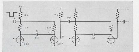
Here's just one excellent example of how you can put the SUS' unique characteristics to work. This twostage frequency divider (or binary counter) circuit uses two SUS' per stage for precise frequency division.
