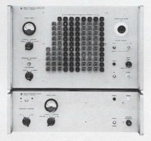
The new Hewlett-Packard 5105A Frequency Synthesizer generates spectrally pure frequencies from 0.1 MHz to 500 MHz in 0.1 Hz steps—a frequency range 10 times higher than previously available by direct synthesis.
