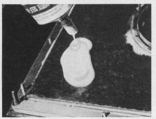
Laminated layers of mica sheeting are securely bonded with G-E RTV silicone sealant. Ready to use, it bonds to most materials, forming heat-resistant rubber.
