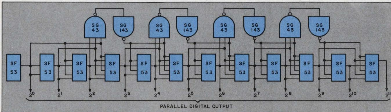
2. Binary digital outputs from this master counter drive the D/A converter which generates the sawtooth voltage
