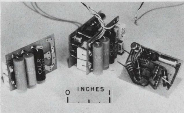
1. Stable RC oscillator (center) consists of two major stages: The twin-T network is at the left and the amplifier is at the right. The volume of the potted unit is slightly more than 1 cubic inch.
