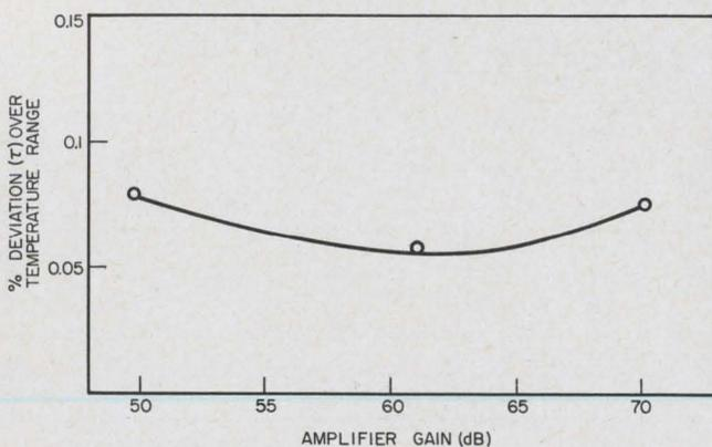
**3. Amplifier's gain should be around 60** for stable oscillation. At this point the gain of the amplifier becomes equal to the loss of the twin-T circuit, which results in an over-all gain of unity.
