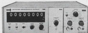
The **Model 800** has 8 decade readout, memory standard. Gate times: 1 μsec to 100 sec in decades. Oscillator stability: ±3 parts in 10<sup>9</sup> per day.
