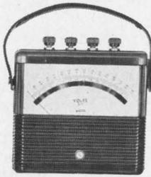
**MODEL 904 AC SERIES:**  $\frac{1}{2}\%$  accuracy with shielded radial vane, moving iron mechanism. Multi-range voltmeter available with self-contained ranges 750 | 300 | 150 | 75 | 30 | 15 | 7.5 | 3 Volts full scale. Multi-range ammeter self-contained with ranges 200 | 100 | 50 | 20 | 10 | 5 | 2 amperes full scale. Other ranges and sensitivities available from stock.
