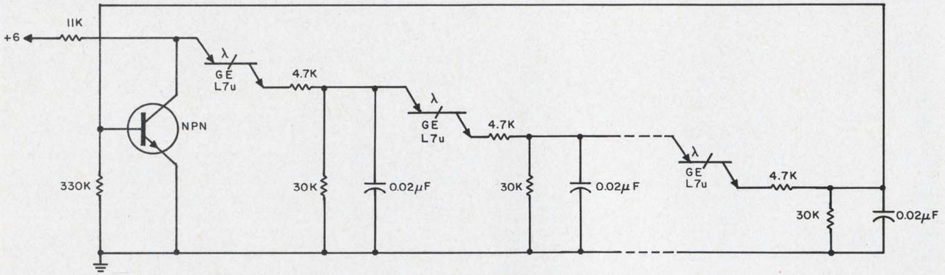
Light pulses replace voltage pulses as triggers for this stepping counter.
