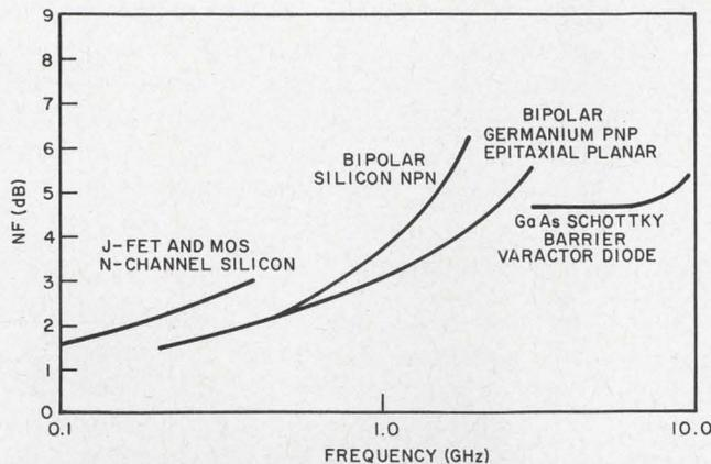
1. Noise figures of devices capable of microwave amplification indicate optimum performance for each type. The data were taken with bias currents and source immittances that yield the best results for each device.
