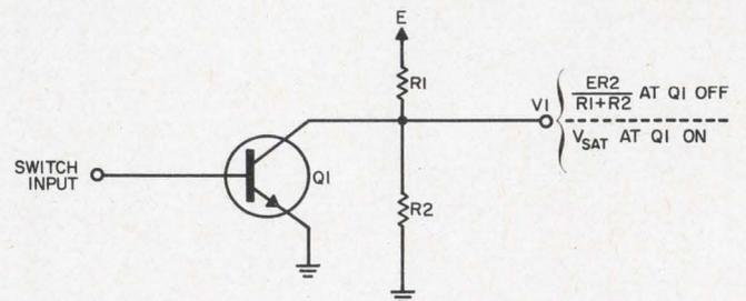
**1. Basic shunt switch** is used in many applications to produce a voltage level,  $V_1$ , and then switch the output to zero. However, in practice the zero level is not reached because of the saturation voltage of the transistor.
