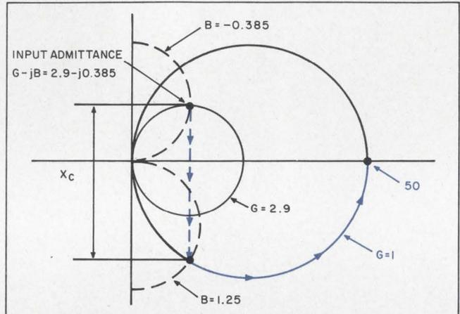
13. In the design of the input circuit the admittance chart is again used. Here one unit is equal to 50 ohms, or 0.02 mmhos. The starting point is the input admittance and the procedure is similar to that used in Fig. 9.
