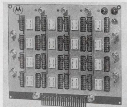
**IC breadboard accepts 14-pin dual in-lines**
