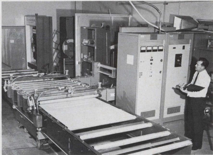
**Continuous microwave processing system** dries the protective coatings on plywood sheets without scorching the wood surface. The prototype 25-kW, 915-MHz system, shown above, was developed by Eimac Div. of Varian Associates. The system uses a slotted waveguide in a serpentine configuration as the microwave applicator.
