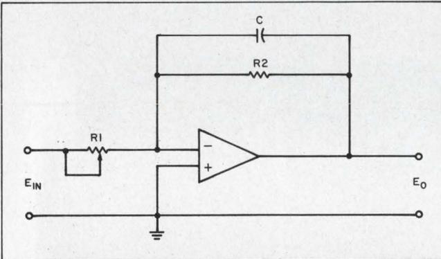
1. Conventional operational amplifier achieves attenuation rate of 20 dB/decade. Rheostat R1 is a gain adjustment.
