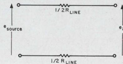
5. Equivalent circuit of line resistance between power source and series regulator. This resistance is included in the line regulation equation.
