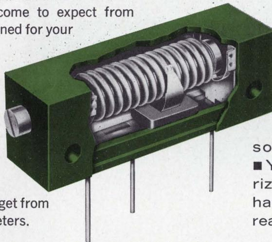
**SPECIFICATIONS:** Mechanical Travel: 12 turns approximate; ■ Effective travel: 11 turns ( $\pm 1/4$ ); ■ Resistance Range: 100 ohms to 20,000 ohms; ■ Resistance Tolerance:  $\pm 5\%$ ; ■ Power Rating: .75 watts @ 85°C. derated linearly to zero power @ 150°C. ■ Available with printed circuit or solder lug terminations. ■ Your local Clarostat Authorized Industrial Distributor has the Series 76 in stock ready for immediate delivery.
