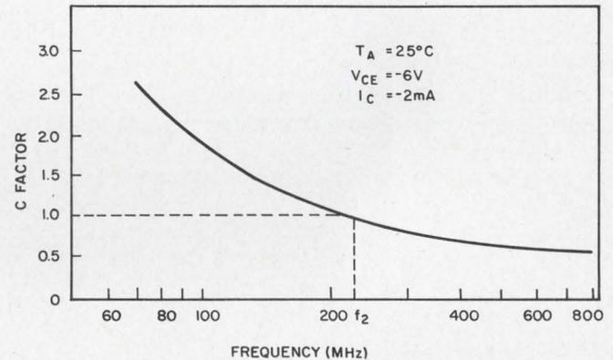
7. Common-emitter germanium transistors reach  $f_2$  somewhat above 200 MHz and are unconditionally stable above this frequency.
