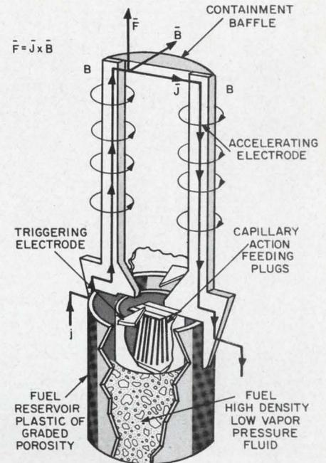
**Pulsed plasma engine** proposed by General Electric scientist, Dr. Aldo LaRocca, weighs only 1.5 pounds and develops 100 micropounds of thrust. The engine can theoretically operate on one ounce of fuel for up to two years.
