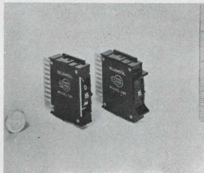
**Rotary thumbwheel indexes 16 positions**
