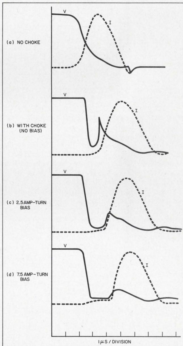
4. Curves show SCR voltage and current waveforms during turn-on. In (a) no choke is used to delay the current. In (b) a saturable choke is used, but the voltage tends to rise again when the current builds up. In (c) and (d) bias turns are used on the choke for the purpose of increasing the current delay.
