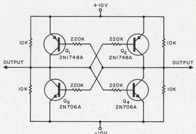
Low output impedance is maintained by the double flip-flop regardless of its state.
