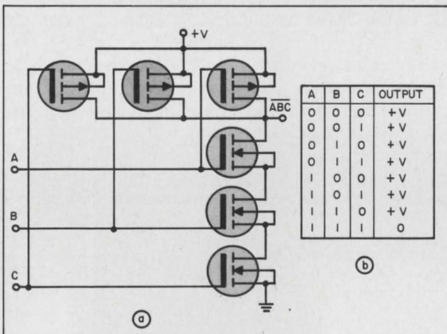
7. Three-input NAND gate using MOS-FETs (a) has p-channel units in parallel and n-channel devices in series. Truth table (b) shows that output is always high (at +V) except for the condition of  $A=B=C=1$ .
