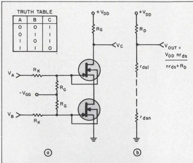
1. **NAND gate** is formed by connecting two J-FET inverters in series (a). If the truth table definitions of logical 1 and 0 were reversed, a NOR gate would result. Equivalent circuit for ON state of NAND gate appears in (b).
