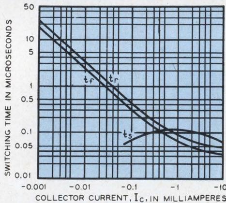
Fastest switching transistor available in the 1 to 100  $\mu A$  range.
