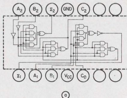
Two-bit numbers are added in this Dual Adder (a) just announced by Texas Instruments. Entire circuit is monolithically integrated (b).
