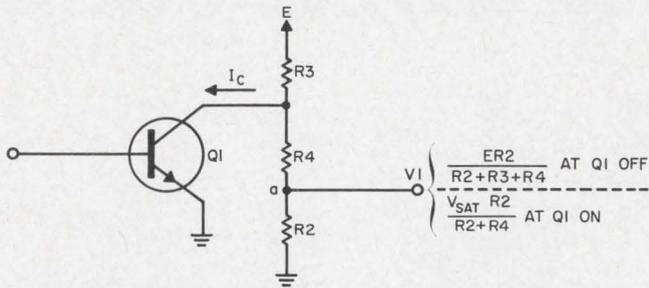
2. A resistor, **R4**, attenuates the saturation voltage. The amount of attenuation is limited by the ratio of **E** and **V1** (OFF).
