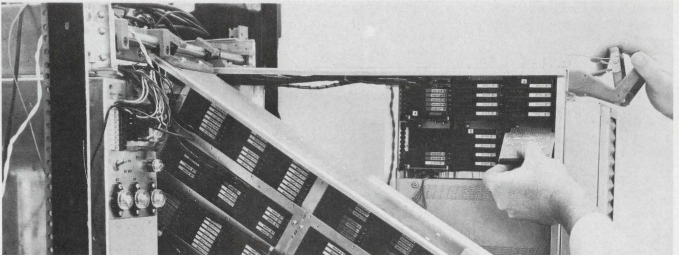
**IC logic modules** in tilt-out racks, are used exclusively in a new 16-bit, 960-ns computer. It
