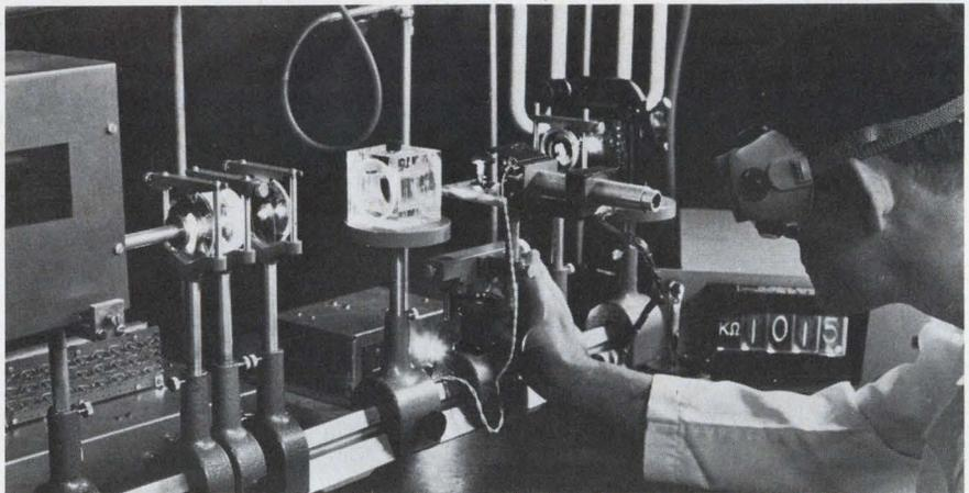
Adjustment of resistivity is achieved when light from a ruby laser (left) is aimed at the resistor on a one-eighth-inch-square hybrid circuit, mounted at the right of the apparatus. By precision regulation of the beam, Univac researchers can predict and control subtle changes in the electrical values of the resistor, to meet the strict electrical requirements of a given circuit.
