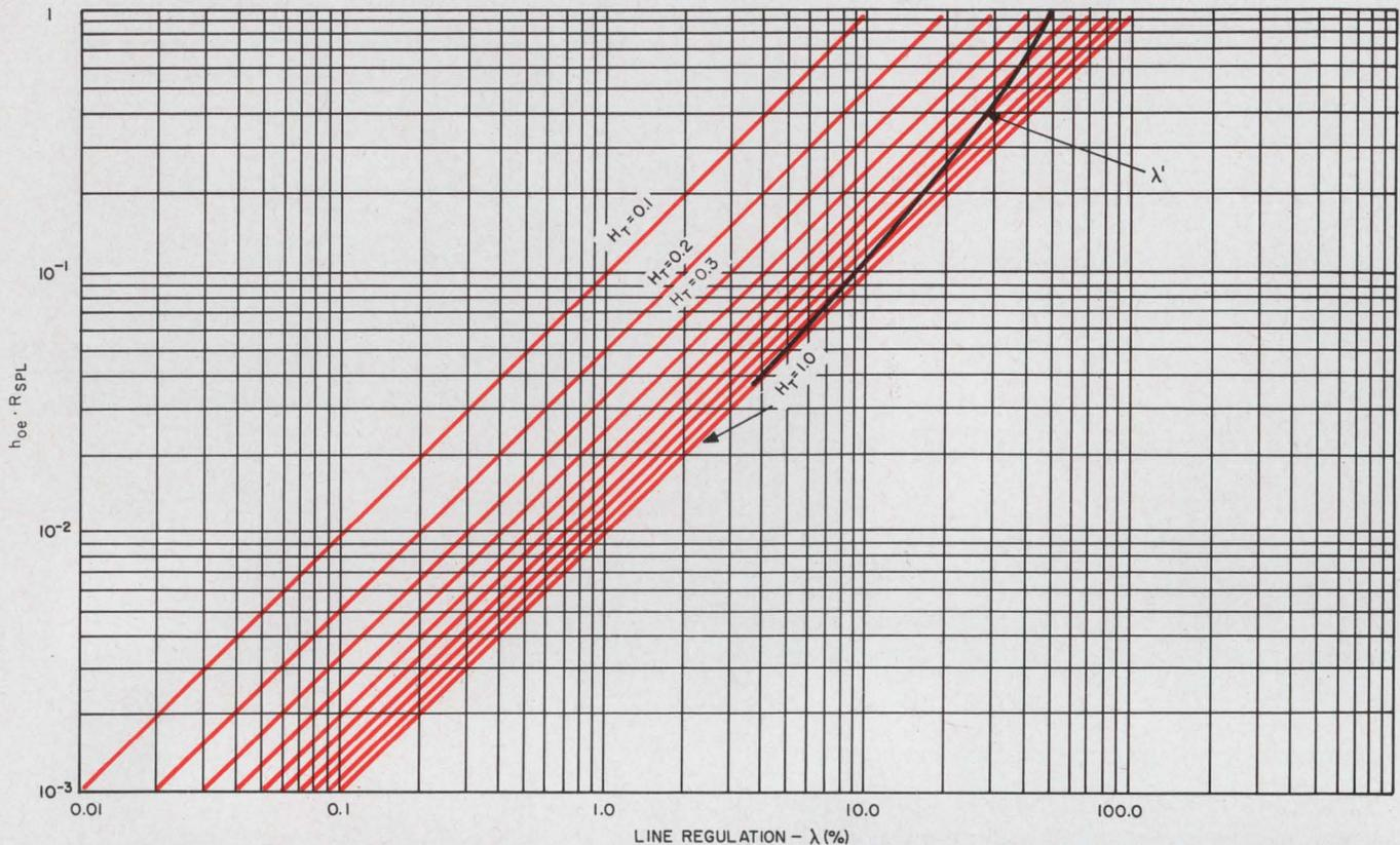
4. Line regulation as a function of the parameters and for various values of  $H_T$ . For any given regulation the best
