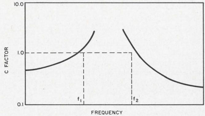
6. The inherent safety factor,  $C$ , crosses unity at two frequencies,  $f_1$  and  $f_2$ , for common-emitter connection of bipolar transistors. The frequency region between these two is potentially unstable.
