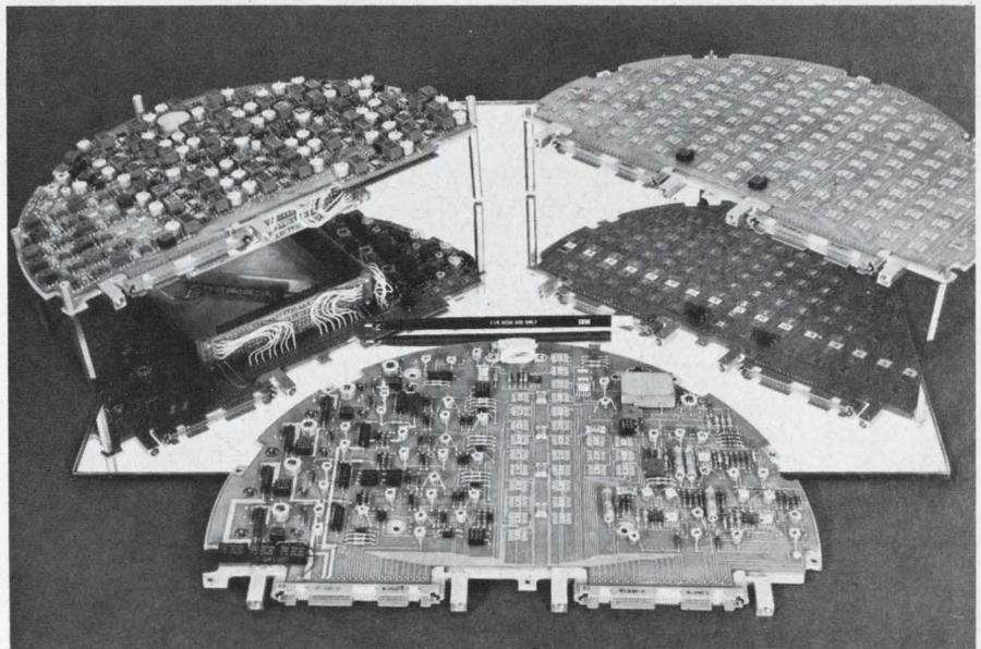
**Ready for use in a tactical missile**, the TC version of the 4 Pi consists of three major subassemblies: (from left) memory, input/output and central processor. Each subassembly consists of 13.25-inch-diameter assemblies of two multilayer interconnection boards and supporting aluminum plate. Mirror shows bottom side of assemblies.
