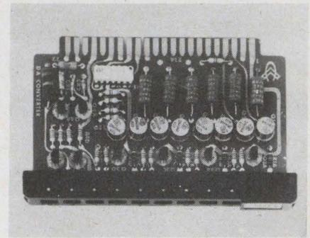
**D/A converter cards supply 0 to 10 V**
