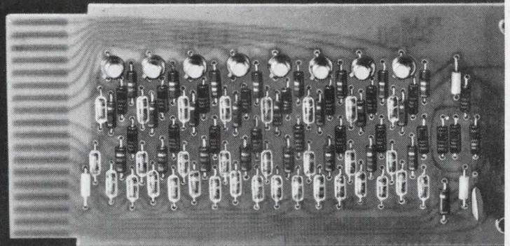
**FLIP CHIP T.M. Modules**—The Digital Equipment Corporation trademark for a new kind of digital system module uses Allen-Bradley hot molded resistors exclusively.
