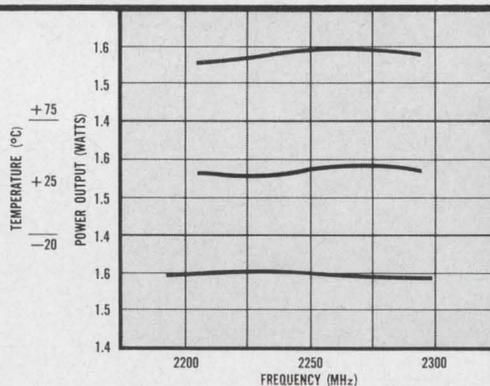
**Typical Results:** 1.5 watts from our X8 Multiplier at 2250 MC. Spurious signals down at least 30db-mid-band efficiency typically 25%.
