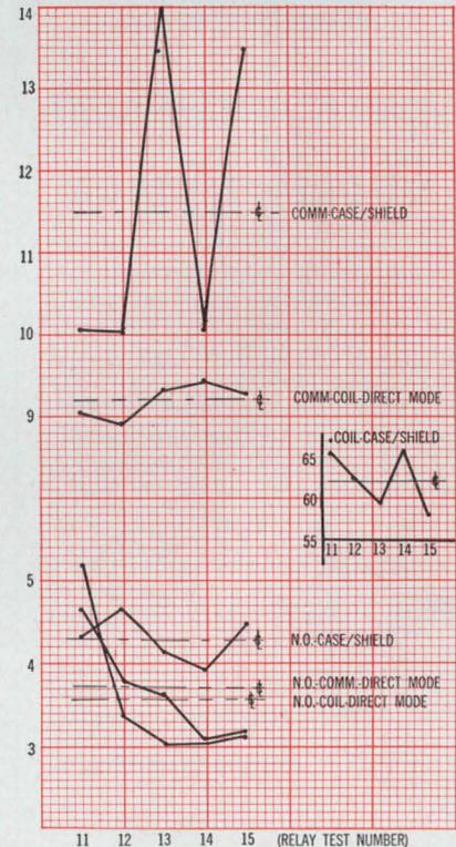
Data was obtained using a Bonton Electronics Corporation Capacitance Bridge, Model 75-A-S8 at 1MHz.
