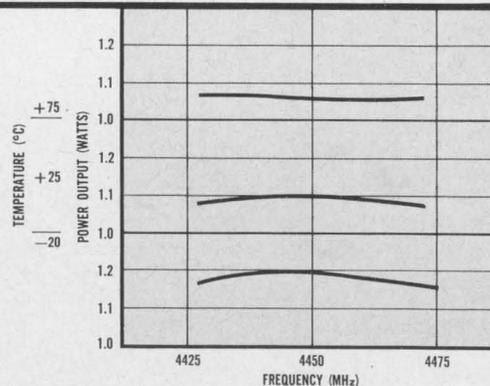
**Typical Results:** Our C Band unit gives 1 watt output, X12 mid-band efficiency typically 16%
