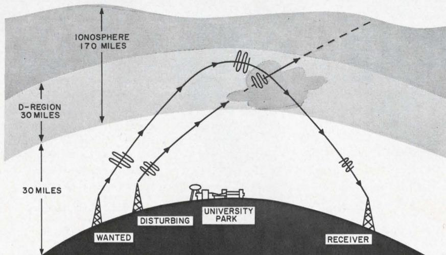
**Ionospheric-disturbance experiment** is conducted by Penn State engineers with high-frequency radio signals. One signal, beamed into the ionosphere, causes a change in phase of a second signal, by heating the electrons in the ionosphere at the intersection point.
