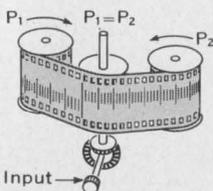
When used as a printed metal readout scale, both ends are curled on bushings of equal size. Since the opposing forces (coils) are always in balance, the span between is held taut.
