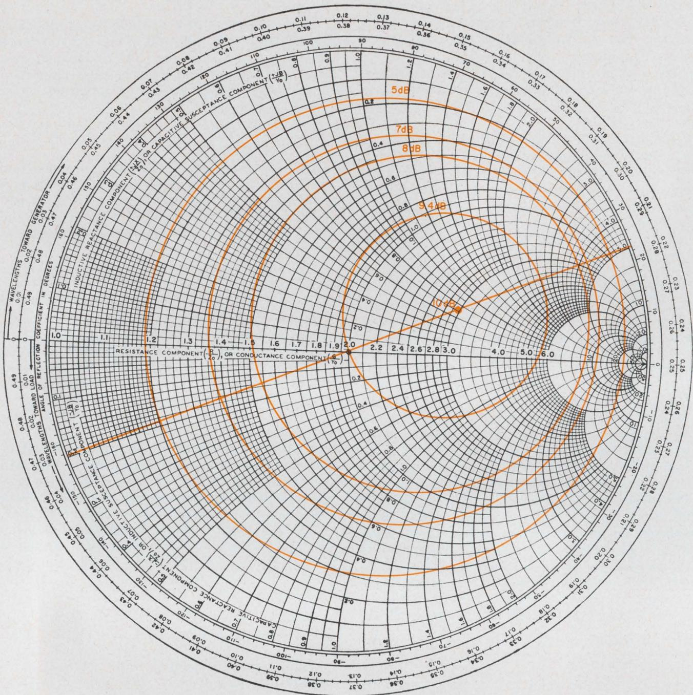
4. Linvill chart is a set of constant-gain circles superimposed on a Smith chart. The centers of the circles lie on the straight line. The maximum available gain (10 dB) is
