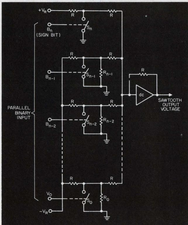
3. Combined with the counter of Fig. 2, this digital-to-analog converter generates the sawtooth voltage, which is actually a staircase voltage with 4096 steps per cycle.
