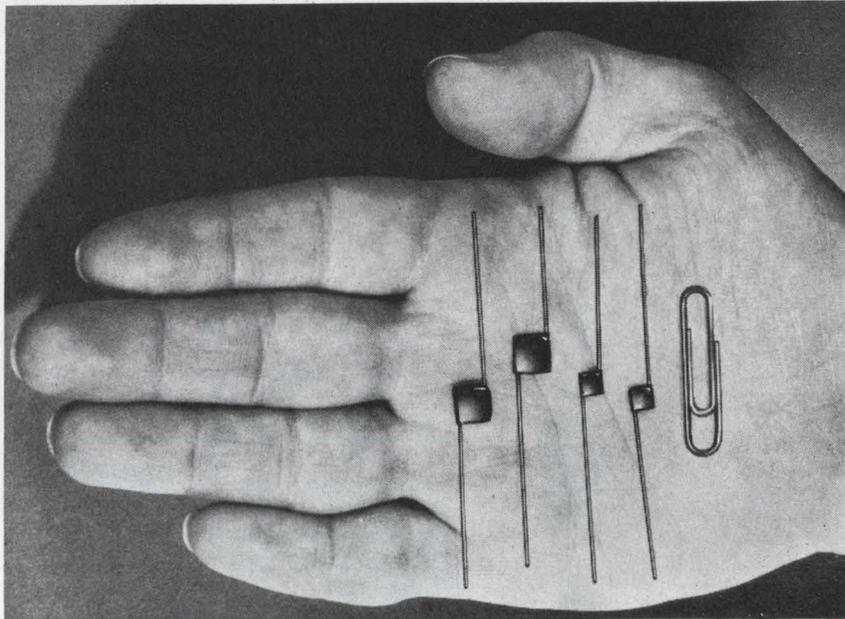
The Mallory TUR is a miniature solid electrolyte tantalum capacitor designed for use with integrated circuits, thin film and other micro-electronic circuits. It is supplied un-encapsulated to provide extremely small size per rating. It is intended for use with microcircuits where it will be encapsulated after assembly.
