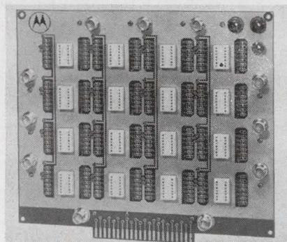
**IC breadboard accepts 14-pin dual in-lines**
