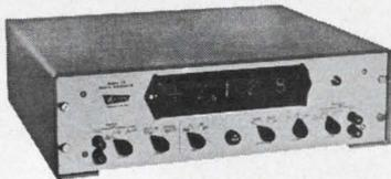
**PRECISION DIGITAL PHASE METER 331.** Large, four-digit presentation provides direct reading 0°-360° to accuracy of  $\pm 0.5^\circ$ . Frequency range, 30cps-40kc. Provisions available for printer output, AC and/or DC outputs for voltmeter reading. Inputs directly usable, 0.2-150 volts. Solid state throughout.
