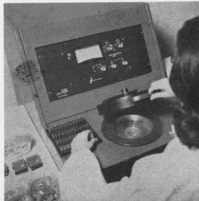
**Leak detector offers fast component testing**
