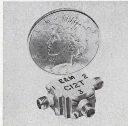
With a 50% reduction in size and weight, these coaxial circulators have customer-selected frequencies. An 8% bandwidth is offered from 1.6 to 1.9 GHz as well as 10% bandwidths from 1.9 to 12 GHz. All units have 20-dB isolation and 1.25 vswr. Insertion loss is 0.4 dB in the low frequency units and 0.3 dB above 1.9 GHz. Units from 5.4 to 12 GHz are 1/2 in. on each side and weigh 20 grams.
