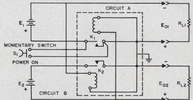
2. Equivalent circuit representation of regulator uses relays in place of the transistor elements. The interconnections here demonstrate the switching, regulating and feedback functions. Relay  $K_1$  represents  $Q_1$  and  $K_2$  is the  $Q_2$  element. Loads  $R_{L1}$  and  $R_{L2}$  depict the oscillator and dc-to-dc converter respectively (see Fig. 1).
