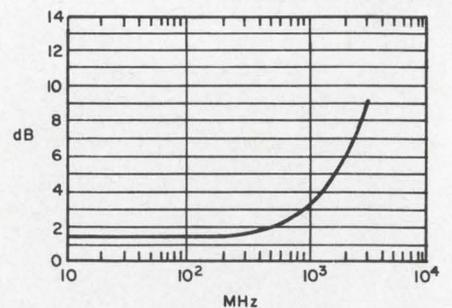
Power gain and common emitter noise figure as a function of frequency of 25°C.
