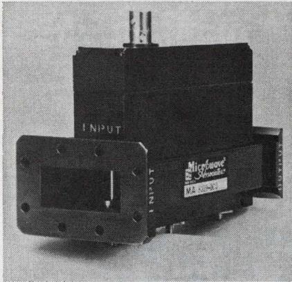
The MA-8319-1C3 switch is used for hot-standby operation in which two RF transmitters, tuned to the same frequency, are switched into a single transmit antenna. When one fails, operation is switched to the standby transmitter. The unit can switch up to 7 W cw in 500 ns. Bias power is 1/4 W and isolation is 90 dB. Insertion loss is 1 dB and vswr is 1.15 in the 6.5- to 7.2-GHz frequency range.
