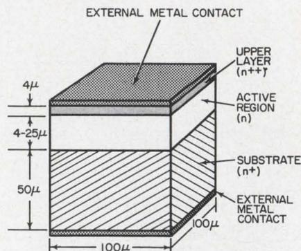
**Sandwich Gunn-effect oscillator devices** are grown epitaxially from gallium arsenide of varying resistivity to different thicknesses. Bell Laboratory scientists report improved cw power over a wide frequency range. Resistivity in the active  $n$  region is  $0.3 \Omega/\text{cm}$ ; in the  $n^+$  region,  $0.001 \Omega/\text{cm}$ ; and in the  $n^{++}$  region,  $0.0001 \Omega/\text{cm}$ .
