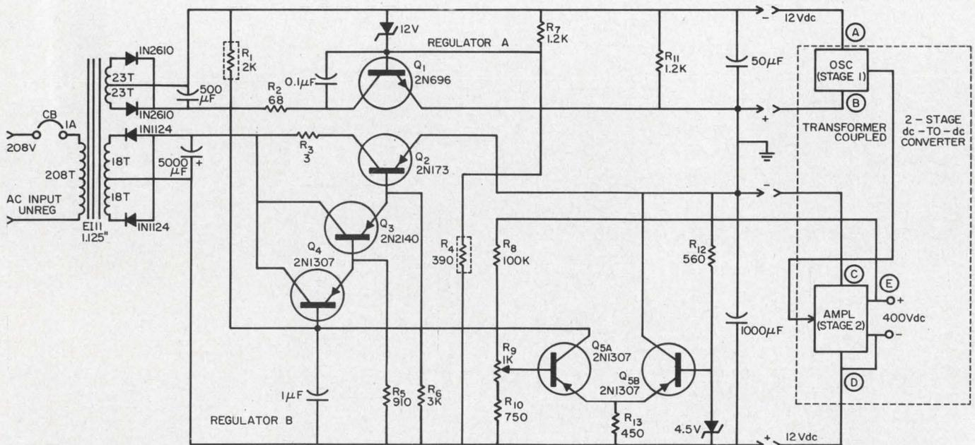
1. Fuseless high-speed shut-off dc regulator features two regulators in a complementary configuration. Resistors  $R_1$  and  $R_4$  provide feedback between the regulators—each
