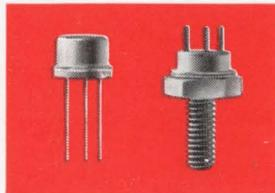
one second. Both AM aircraft and FM mobile types are designed specifically to withstand load mismatch conditions. This capability means simpler design of the final stage and no need for protective circuits. In addition, types for AM aircraft display excellent modulation capability as well as high-voltage breakdown characteristics.
