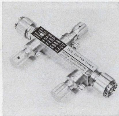
This matching tuner is a section of coax with three lockable screws to tune out small reflections in low-vswr measuring instruments. Frequency range is 0.25 to 2.5 GHz. The vswr matching range is 1.02 min at 0.4 GHz and 1.05 min from 1 to 2.5 GHz. Vswr resettability is better than 1.001 and connection is repeatable to within a vswr of 1.0005.
