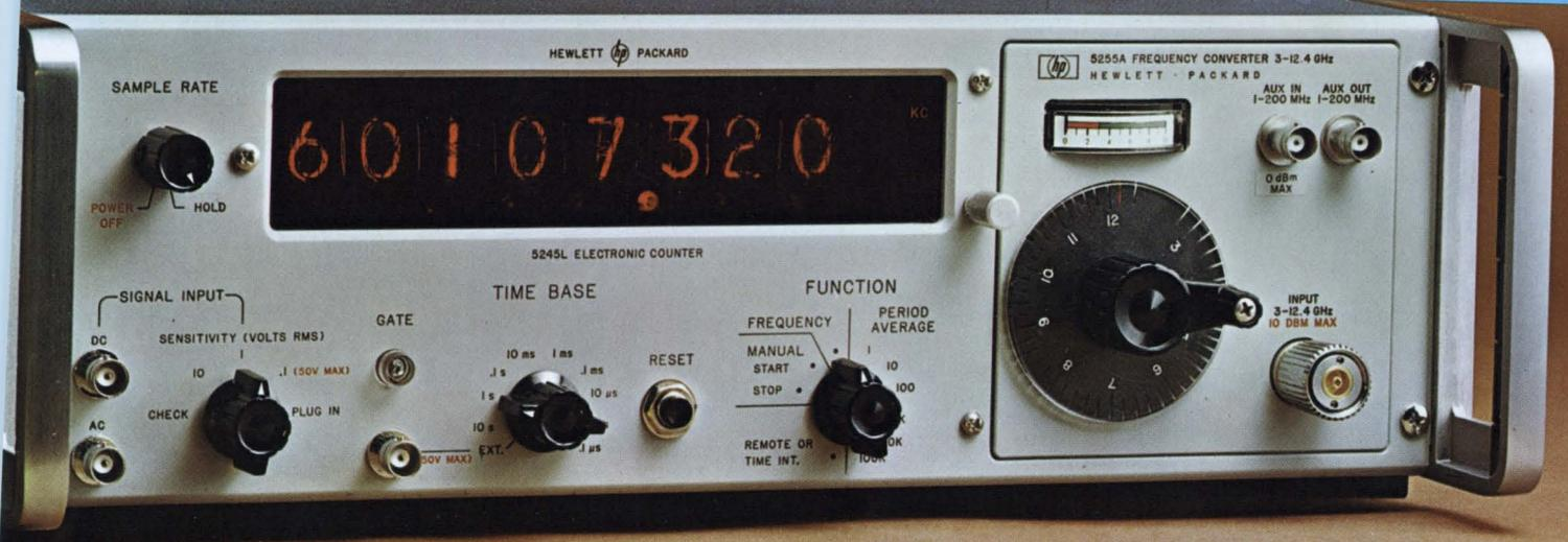
Model 5245L Electronic Counter with new 3-12.4 GHz Plug-in Heterodyne Converter
