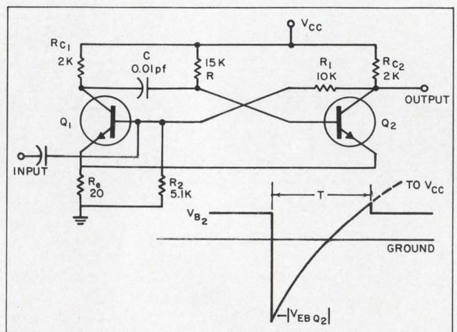
2. One-shot built with component values shown is used to measure the accuracy of the period-calculation method described in the test. The waveshape of the base voltage of  $Q_2$  is used to derive an expression for the period.
