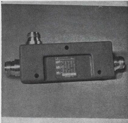
A 50% weight and size reduction is a feature of this series of 27 stripline directional couplers. The units have flat coupling of 10 to 20  $\pm 0.8$  dB, 20-dB directivity and a 1.2 vswr in both primary and secondary lines. Insertion loss is 0.2 dB max and calibration accuracy is  $\pm 0.2$  dB. Impedance is 50  $\Omega$  and ambient temperature range is  $-50$  to 250°F.
