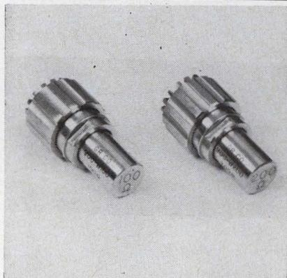
Two resistive terminations are the 100-Ω type 900-W100 and the 200-Ω type 900-W200. The 100-Ω termination has a resistance within ±1.5% to 1 GHz and within ±5% to 8.5 GHz. The 200-Ω unit holds its resistance within ±1.5% to 1 GHz and within ±10% to 8.5 GHz. The position of pure resistance is 4 cm from the reference plane of the connector.
