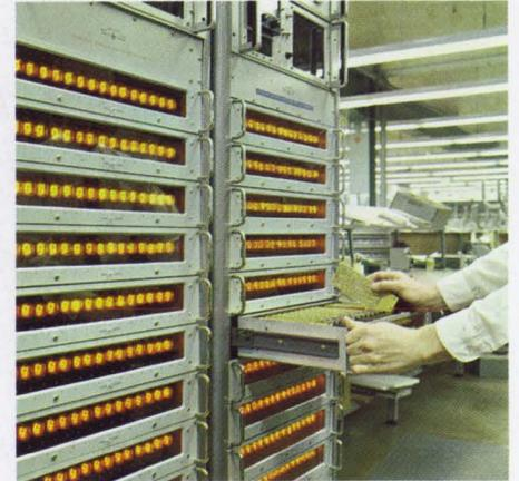
Decade counting assemblies for all solid-state counters undergo a temperature of 80° C for 2 hours to force failure of any marginal components. Despite this torture, the failure rate of decades is less than 0.5%. The assemblies are also operated for 22 hours at room temperature.
