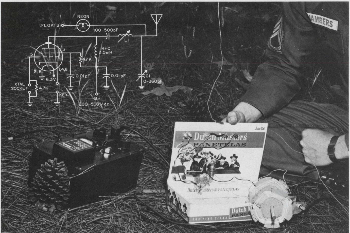
What does a Green Beret do about a damaged transmitter? Here Sgt. 1st Class Buddy Chambers demonstrates a cigar box transmitter made from a few parts salvaged from an inoperative T-784 transmitter used with the GRC-109 set. The floating neon bulb tells when the "designer" has achieved success. L1 is two sections of hand-wound coil (foreground). Mounting on a stick allows inductance
