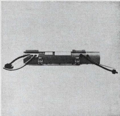
Pulse-position modulated and delivering 100 W in S through C band, the ppm-focused TWT operates from 2.5 to 5.2 GHz. Coaxially coupled, it operates with depressed collector in MIL-E-5400 Class II environments and performs with heat sink temperatures up to 100°C. The vacuum envelope is metal-ceramic and the focusing assembly is magnetically shielded.
