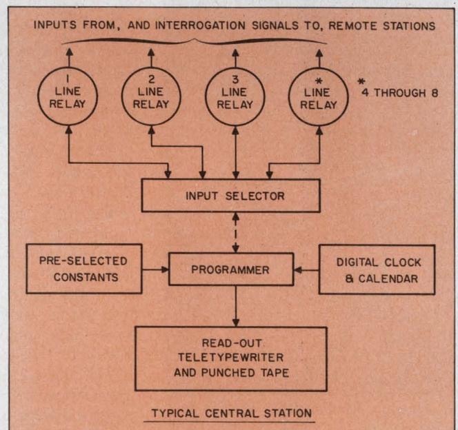
1. Typical air-quality monitoring system of the type recently installed in Chicago by Datex Corp. consists of eight remote data collection stations. Each station automatically measures air pollution content and meteorological data, digitizes the information and transmits it to a central computer station by means of telephone or teletype lines.
