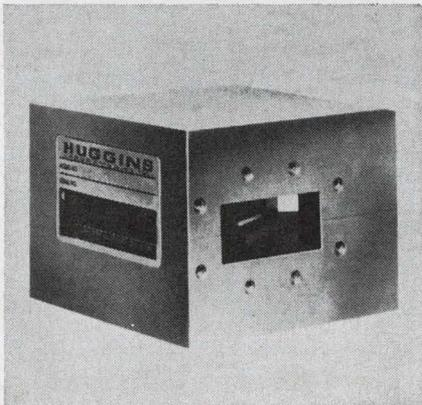
With a 7.05- to 10-GHz range, this 3-port waveguide circulator and flange offers a 20-dB min isolation, 0.3-dB insertion loss and 1.2 max vswr. Power ratings are 10 k-W peak and 20 W average. Custom models are available with 10% bandwidth or less for insertion losses down to 0.1 dB and vswr reduced to 1.05.
