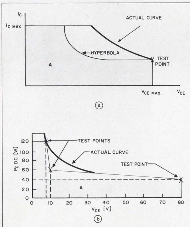
1. Safe operation of power transistor in dc mode is established by hyperbola relating  $I_C$  to  $V_{CE}$ . (a). As  $V_{CE}$  increases, the device's dissipation capability diminishes, and a derating curve must be used (b).
