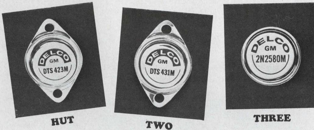
They're designed for high efficiency inverters, voltage and current regulators, control and switching circuits and high-power communications where extreme reliability is required.
