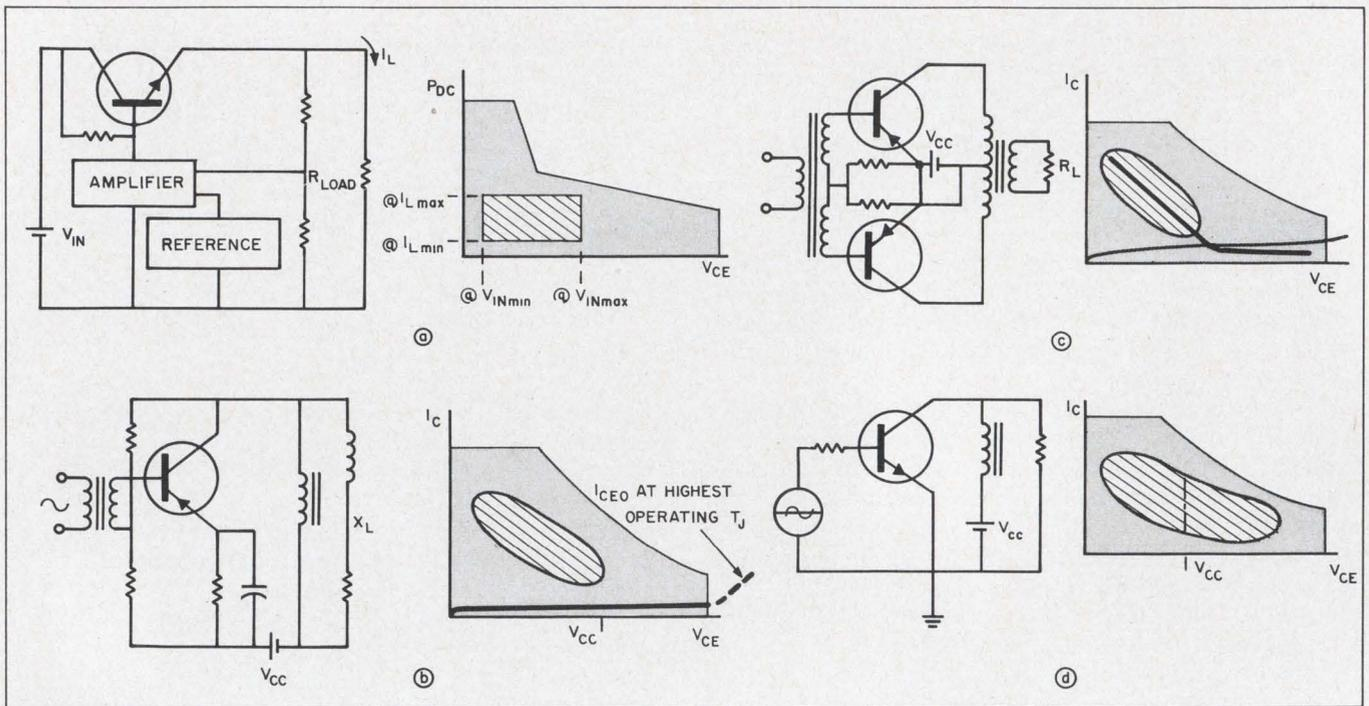
3. Safe operating area (Soar) for power transistor applications is designated by the crosshatched portions on the  $I_C-V_{CE}$  characteristic. Shown are a series dc regulator (a), a Class-A amplifier (b), a Class-B amplifier (c) and an
