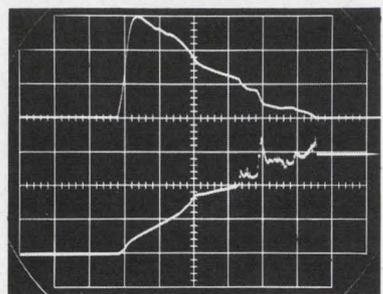
**Simultaneous Single-Shot Displays.** Current versus voltage display of a .75 ampere, fast-blow fuse during destructive overload. Both beams are driven by B Time-Base at 50  $\mu$ s/cm which is delayed by pre-triggered A Time-Base to provide base reference lines before and after the event. The upper beam shows the current waveform at 30 A/cm while the lower beam shows the corresponding voltage across the fuse at 100 V/cm.
