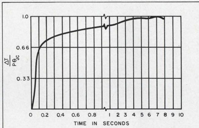
7. **Normalized junction temperature response vs time** plot is used to make safe-operating-area calculations for pulse widths in excess of 1.0 ms. Here  $\theta_{JC}$  refers to the thermal resistance, junction-to-case.
