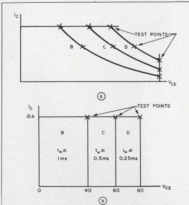
5. **Safe operating area** is a function of pulse width. The  $I_C-V_{CE}$  curve is broken into three distinct regions (B, C and D), each bounded by a hyperbola (a). When a specific transistor type is involved (b), straight-line approximations may be used to save test procedure down time.
