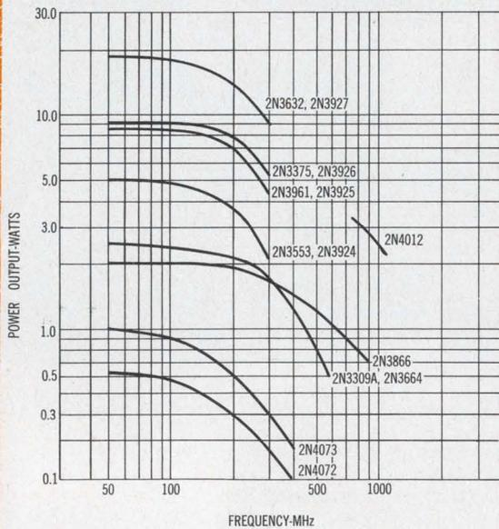
The power-frequency curves indicated here, cover only the EIA-registered device numbers available within Motorola's broad RF Power Transistor line. They are intended to help you narrow the range of possible choices for your specific application.
