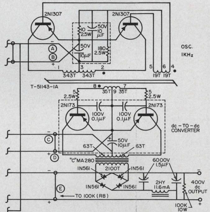
3. In this 2-stage, dc-to-dc converter (the load for the regulator of Fig. 1), a 1-kHz saturating-transformer oscillator (stage 1) drives a high-power amplifier (stage 2).
