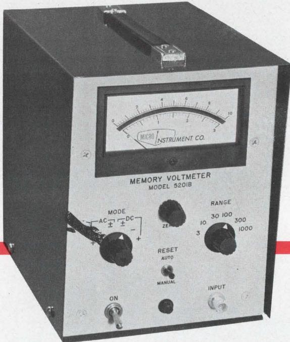
The Model 5201 memory voltmeter is a dc to 20 mc instrument which measures and stores indefinitely the maximum peak voltage applied, including continuous or one shot pulses as short as 50 nanoseconds. A memory reset-switch on the front panel allows the 5201 to monitor peak values of a varying waveform, either positive or negative going.
