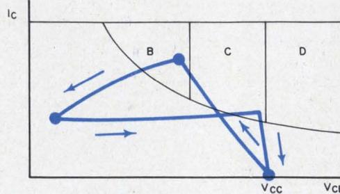
8. Each type of pulse application has its own Soar. Indicated by the heavy lines (in color) on the  $I_C-V_{CE}$  curve, it shows just how far to stress a transistor used in a switch-
