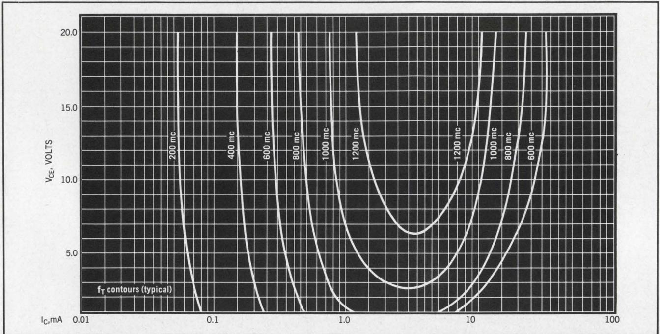
**High performance complement to the 2N918.** Now you can get PNP high frequency transistors for your VHF-UHF amplifiers, oscillators, and non-saturating switch requirements. Raytheon's 2N4080 is designed to deliver a minimum of 15db in 200 Mc class A amplifier circuits or switch in less than 10 nanoseconds turn-on time in non-saturated switching circuits. The 2N4080 is the high performance complement to the 2N 918 NPN amplifier.
