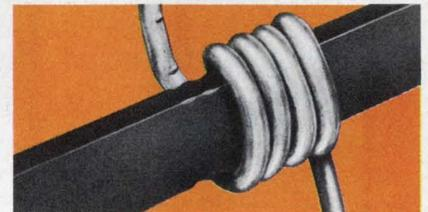
Solderless wrapped connections remain gastight even when exposed to severe changes of temperature and humidity . . . so they're not affected by atmospheric corrosion.
