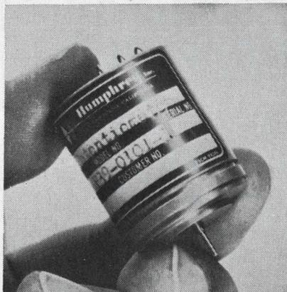
A low torque circulator potentiometer may be used as a sensing element in instrumentation systems, or as a pickoff device for oceanographic current direction sensors and magnetic compass devices. The standard model CP39 has a 10 MΩ resistance element with continuous mechanical rotation and  $355^\circ$  minimum electrical travel. Starting and running torque is 1 gm-cm max. Independent linearity is  $\pm 0.5\%$ .
