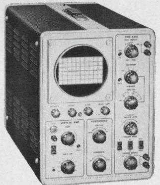
A 5" DC scope with calibrated time base & 5X sweep magnifier. For 115/230 volt, 50-60 cycle operation.
