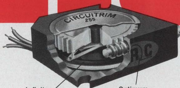
Infinite resolution Metal Glaze® element
