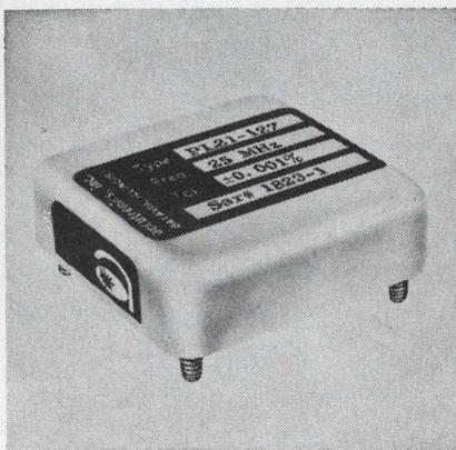
Frequency tolerances of  $\pm 0.001\%$  can be met over the 5- to 100-MHz range of this crystal oscillator. Available supply voltages of 5 to 28 Vdc suggest uses as an IC frequency source. Output voltages of 3 V p-p square wave with 20-ns rise time and 2 V rms sine wave with 10% distortion into a 1-k $\Omega$  load are typical.
