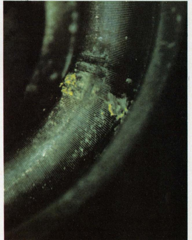
The entry of chemical agents caused a small section of the element to deteriorate. The resultant chemical action caused noisy performance.
