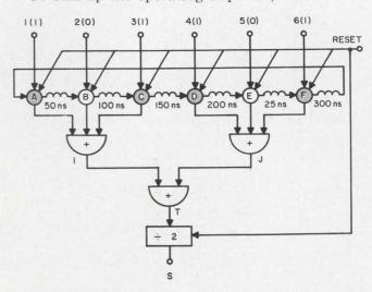
1. Parity generator, based upon threshold logic, uses neurons to simplify circuitry and cut the cost of hardware. Circuits from A to F are neurons, I, J and T are OR gates. The output at S is the parity indication.
