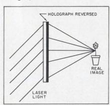
3. Holograph can reconstruct real image (just like that of a slide projector) if it is reversed in its holder after it is developed. Images always appear on emulsion side of film. For the best resolution, holographs should be made on very slow spectroscopy plates with argon laser light.
