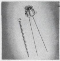
A silicon photodiode in a TO-18 package is designed to operate with bias conditions required by low cost silicon transistors. Typical reverse dark current at 55°C with −1.0 V is 0.4 µA. Typical short circuit current output at 500 foot candles is 180 µA. Spectral response peak is at 0.85 microns and speed of response is 1
