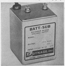
Model 100-2 constant voltage supplies replace dry cell batteries, standard cells and standardizing mechanisms in self-balancing potentiometric type chart recorders. Ratings are 10, 6, 5, 3 and 1 mA with a 1.03-Vdc output. Voltage line regulation is  $\pm 0.0016\%$  over 94 to 140 Vac. Isolation is 6 mVac rms across a 1  $\mathrm{M}\Omega$  resistor from output to ground.
