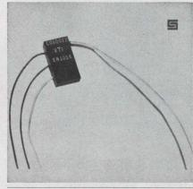
A miniature cold junction compensator for Chromel-Alumel thermocouples eliminates the need for ice baths, boiling water or transitional salts to achieve a constant temperature reference in which to embed the cold junction. With an input of 400 mV into 3.7 k $\Omega$   $\pm 1\%$ , the output of the compensator is 11 mV  $\pm 3\%$  at 25°C. Tracking ability is within 80  $\mu$ V from -65 to +125°C.
