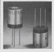
This trimming potentiometer is a 1/4-in. diameter, single-turn unit with pins spaced on a 0.1-in. grid. Pin length is 3/16-in. Standard resistances available are 10  $\Omega$  to 1 M $\Omega$ . The cermet element offers a power rating of 0.5 W at 85°C, derating to 0 at 150°C. The 0.75-gram unit is available in continuous rotation or stop configurations.
