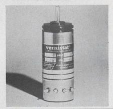
Series 7 ac potentiometers are size 11 20-turn units. Typically, output impedance is 20  $\Omega$  and absolute linearity is  $\pm 0.01\%$ . Input impedance is 100 k $\Omega$  and input voltage is 30 V max, 400 Hz. Output current is 25 mA max. The pots are designed for servo and control systems and meet MIL-specs.
