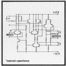
Figure 8. Circuit diagram of SN725 differential amplifier.
