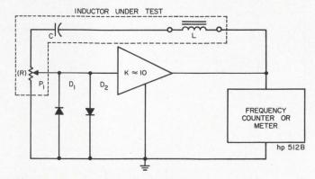
Phase-shift oscillator arrangement provides very accurate measurements of inductance. Feedback loop is formed by RLC phase network.
