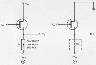
3. In low-drift, single-ended FET amplifiers, either a constant-current source (a) or a large  $R_{\rm s}$  returned to a high-valued  $V_{\rm ss}$  supply (b) may be used for the current bias. Low-drift operation is obtained by biasing at or near the zero temperature coefficient point.
