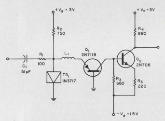
6. Divide-by-two circuit isolates the input and output. It operates at a rate that is the inverse of the minimum delay period.
