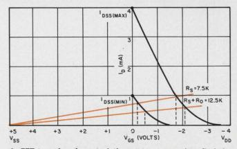
2. **FET** transfer characteristic curves are used to find the value of source resistance ( $R_{\rm S}$ ) for a simple voltmeter application (see Fig. 3a). Intersections of the proposed resistive load lines with the  $I_{\rm D}-V_{\rm GS}$  curve of both min and max units are necessary. The load lines must pass beneath  $I_{\rm DSS(MIN)}$  point to allow for temperature changes in that parameter.
