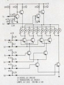
Fig. 2. Binary-to-decimal decoder drivers
