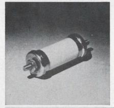
Glass-cased capacitors are suitable in high-voltage applications from -55 to  $+125^{\circ}\text{C}$  with no voltage derating. The paper-plastic film dielectric, the high dielectric strength of the impregnant, and the thermal glass tubing provide size and weight reductions.
