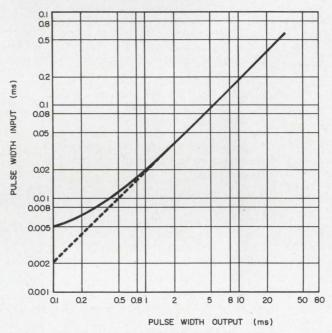
Linearity over a major portion of the input range is another feature of the PWM system. A different multiplying factor can be used in the non-linear portion to provide over-all accuracy.
