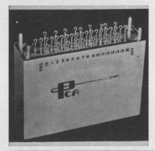
Featuring a built-in pulse equalization network, a multiple tap delay line is designed for pulse encoders and decoders. The pulse network provides an output amplitude at each tap within  $\pm 1$  dB on the nominal pulse amplitude at the end of the line. The hermetically sealed units measure  $3-1/8- \times 4-1/2- \times 1-1/4-in$ .
