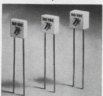
Radial porcelain capacitors with a  $\pm 25$  ppm/°C temperature coefficient, 0.2-in. lead spacing and ratings to 200 Vdc are offered. The VY03 line consists of 13 standard values in a 5.1- to 1000-pF range. Dissipation factor is 0.001 at 25°C and 0.002 at 125°C. They operate from -55 to +125°C without voltage derating.
