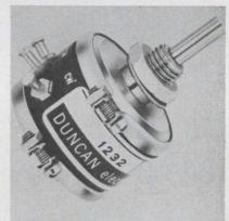
A 7/8-in. bushing mount potentiometer, model 1232, is available in single and multi-cup configurations. Resistance range is 100  $\Omega$  to 20 k $\Omega$ . Resistance tolerance is  $\pm 5\%$  and linearity tolerance is  $\pm 0.5\%$ . Life expectancy is 2  $\times$  10° revolutions and power rating is 1.25 W at 40°C. Up to 9 taps and 6 cups can be accommodated.
