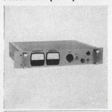
A continuously variable output of 200 to 1800 Vdc in two ranges at 0 to 10 mA is designed to power photomultiplier tubes. Line regulation of model PM-1K-01A is  $\pm 0.001\%$  for a 10% change and load regulation is 0.001% from no-load to full load. Ripple is 2 mV p-p and stability is 0.01%/hour. Output voltage and current are monitored by a pair of 2%-accuracy front panel meters.
