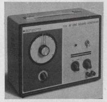
Sine and square wave signals from 20 Hz to 200 kHz are generated by model 636. For the sine wave output, frequency response is flat within  $\pm 1.5$  dB with accuracy of  $\pm 5\%$  and distortion of less than 0.25%. Output is 0 to 10 V rms across a 600  $\Omega$  load. For the square wave output, rise time is 0.15  $\mu$ s. Output is 0 to 10 V p-p into 600  $\Omega$  load.
