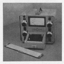
A portable test console measures electrical characteristics of all 1- to 14-lead ICs. The unit contains 6 power supplies, four of which are individually front-panel adjusted over 0 to ±15 V. Readout is on the front panel meter or on an external DVM. Accuracy is 1% full-scale with panel meter, and 0.1% with a DVM. Voltages to 30 V and currents of 1 nA can be measured.
