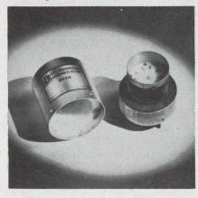
Up to 11 plug-in crystals may be installed in the low-power model 900-0153 oven. Power consumption is 6.6 W at turn-on and 1.5 W average at 25°C. Standard operating temperatures are 65, 75 and 85°C. Standard operating voltages are 12 Vdc, 24 Vac or 115 Vac. The ovens are suited for battery-powered mobile communications.
