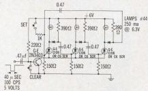
Fig. 3. High current ring counter
