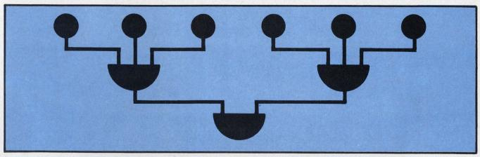
Threshold logic using tunnel diodes can serve to generate parity in a digital system. The cir-
