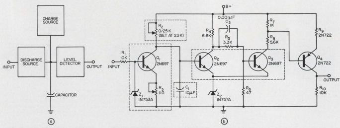
1. Pulse-width-multiplier system broadens the operating range and improves the low-level accuracy of force transducers. In the block diagram (a), input pulses are stretched so that output signals are within the response-
