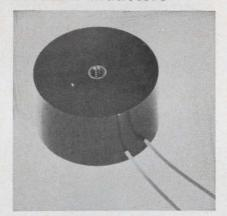
Series L toroidal inductors provide 1 to 40,000 mH from 100 Hz to 100 kHz. Inductance is stable to within  $\pm 2\%$  from -55 to  $+85^{\circ}$ C. Due to the closed field, magnetic shielding is not required. The units have 5-in. teflon leads. Adjacent stacking results in a minimum of mutual coupling.
