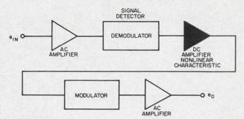
4. Nonlinear gain characteristics in an ac system can be achieved with the nonlinear dc amplifier. The dc type is employed as a stage between the demodulator and modulator circuits in this ac cascade.
