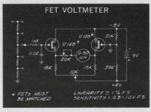
Here is a DC voltmeter with an input impedance that competes with any good VTVM, full scale sensitivity of 0.5 volts max. Add a diode and recalibrate for AC.
