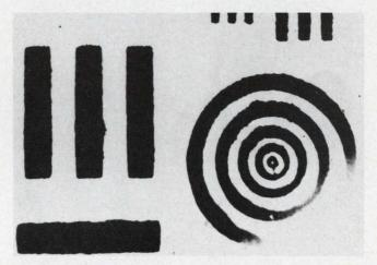
Laser holograms to print semiconductor etching patterns at reduced cost. Page 17
