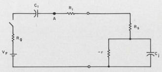
7. The equivalent circuit of the tunnel-diode and differentiating circuit,  $C_1 \, R_1$ , in Fig. 5. It helps to find the charging time constant and parameter values.
