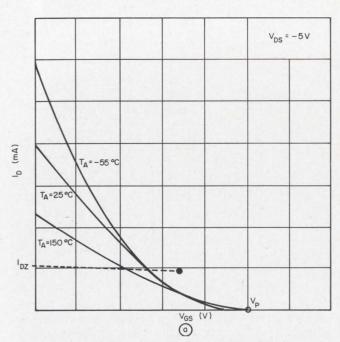
4. The zero temperature coefficient current bias ( $I_{\rm DZ}$ ) may be found in the transfer characteristic (a). Plots of  $I_{\rm D}$  vs  $V_{\rm GS}$  at different temperatures are made; their common intercept is the zero tc point. Drift as a function of temperature coefficient current bias ( $I_{\rm DZ}$ ) may be found in the zero tc point.
