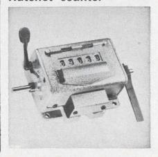
The wheels of this subtracting type predetermining ratchet counter may be preset to any figure up to 99,999. In operation, the counter subtracts from the pre-set number to 00,000. At the passage of 00,000 an spdt switch is actuated. Maximum counting speed is 500 strokes/minute. Angle of throw is 36 to 60°. The 5-digit unit is rated at 5 A, 220 Vac.
