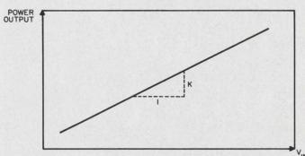
1. Voltage-power characteristics, although linear, are met by a nonlinear feedback amplifier that uses Zener diodes in the feedback loop.
