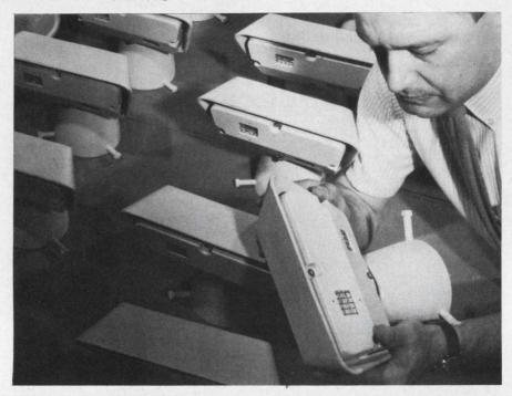
Antenna portion of ultrasonic detector is inspected by Sperry engineer.
