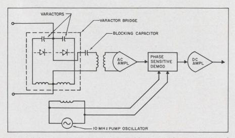
Varactor bridge has stored charge modulated by input and pump signals and provides 43 dB power gain. Noise-free output of this stage is proportional to the bridge unbalance or input error signal.
