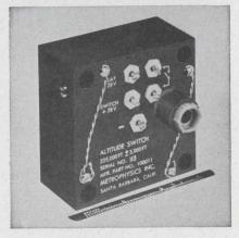
Switching over a pressure range of 30 to 0.04 mmHg (70,000 to 230,-000 feet) is accomplished by this high-altitude pressure switch. The switch withstands 20 G vibration, 150 G linear acceleration and has an operating range of -20 to +165 °F. A temperature-controlled thermocouple pressure sensor a constant-voltage source, a dc amplifier and flip-flop switching are used.
