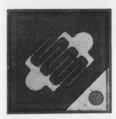
Transistor geometry features interdigitated construction.
