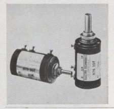
Models 875 and 876 7/8-in. potentiometers are available in 3, 5 and 10 turns, 1/8 or 14-in. shaft, with standard bushing or servo mounting. Resistance range is 25  $\Omega$  to 250 k $\Omega$  with a linearity tolerance of  $\pm 0.25\%$ . These 1-oz pots have a 3-W power rating at 40°C ambient. Life expectancy is 2  $\times$  106 shaft revolutions.
