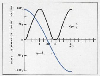
4. The output voltage is a function of the phase difference between the incoming and the reference signals (color). It also depends on the ratio of the two signals' frequencies.
