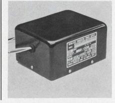
A 115-Vrms, 400-Hz sine wave inverter is rated at 100 W. The inverter operates from an input of 24 to 30 Vdc. Output power is rated at 100 VA at 50°C or 80 VA at 71°C. The wave shape is sinusoidal with 4% max harmonic distortion at full load.
