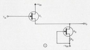
perature is plotted (b) for a low-drift single-ended FET amplifier (see Fig. 5b). Note the very small drift from  $0^{\circ}$  to  $125^{\circ}$ C. A second FET, operating at its zero tc, as a current source (c) provides even more stable operation.
