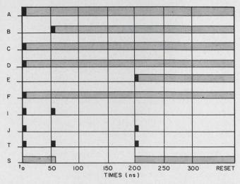
2. Timing circuit assumes that A,C,D and F are in the high state at  $t=t_o$ . Within the total delay period of 300 ns, B and E will be switched to the high state to yield outputs at  $t_{50}$  and  $t_{200}$ .
