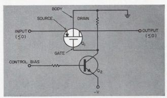
Because the input and output signals are less than or equal to zero, the body of  $Q_1$  is grounded and the source and drain junction leakage is kept in the nanoampere range. Body junctions can withstand voltages up to 25 volts without excessive leakage or breakdown, thus permitting a wide range of input voltages. Crosstalk is minimized by a source-to-drain capacitance of less than 1 pF.
