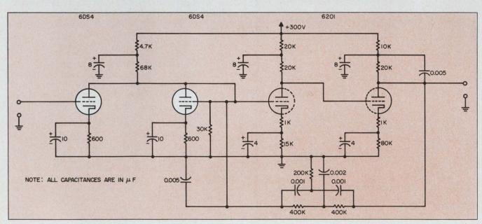
3. Low-noise, narrow-band amplifiers in detector use nuvistors in the input stages. The circuit may be used at
