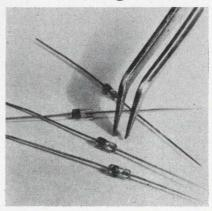
Fast switching microwave silicon diodes are designed for low loss switch applications at frequencies up to and including Ku band. Model MO 2800A of the 2800 series features a forward switching time of 1.0 ns max, total capacitance of 0.1 pF max, voltage breakdown of 80 V min and dynamic forward impedance of 3  $\Omega$  max.
