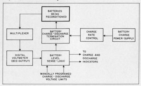
Automatic battery charging system compares individual cell voltages to preset limits. As each cell reaches the programed level, its charge or discharge cycle is terminated.
