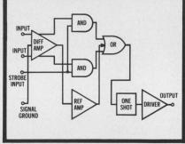
Figure 3. Functional block diagram of SN7500
