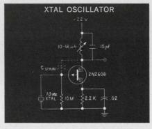
The high impedance of a crystal works hand-in-hand with the high-Z FET.
