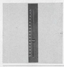
A new 1-in.-wide vertical or slide attenuator has either 20 or 30 steps in a balanced or unbalanced ladder, T or potentiometer circuit. Impedance ranges are 30 to 600  $\Omega$  on ladders or T's and up to 1  $M\Omega$  on potentiometers. Standard dB per step is 1.5. All contacts and wipers are solid silver alloy and terminals are located at the upper back end.
