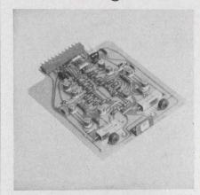
Two highly stable and linear gated sawtooth generators are combined to form the SG415. Each is do coupled, and screwdriver adjustable pots provide a  $\pm 50\%$  width adjustment. Nominal sawtooth widths can be specified from 6 ns to 500 ms. Provisions are made for the connection of external timing capacitors.
