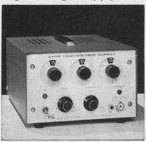
Model 240A has an output voltage from 0 to  $\pm$  1200 Vdc, front-panel selectable in calibrated 1-V steps. A pot permits interpolation with better than 5-mV resolution. Output current is 10 mA max. Line and load regulation are both  $\pm 0.005\%$   $\pm 2$  mV. Accuracy is  $\pm 1\%$  of the dial setting for all outputs. Ripple and noise are 1 mV rms max.
