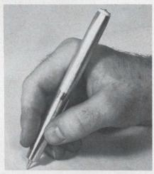
It looks like a pen, but don't expect it to write. This RF noise generator will effectively jam the output of any nearby bugging transmitter.
