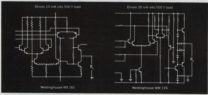
You can drive sizable inductive, capacitive, or resistive loads directly with either of these two IC op amps. They're unmatched for "muscle". Using them, you can omit an intermediate driver stage or power amplifier in many applications.
