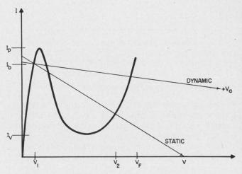
4. Dynamic and static load lines, voltages and currents of neuron circuits are valid for tunnel-diode types.
