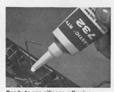
Ready-to-use silicone adhesive encapsulates, seals, bonds. Silastic® 732 RTV rubber is a tough, squeeze-on adhesive/sealant that bonds metal, glass, plastics, rubber and most other materials. It cures at room temperature in 24 hours to a solid rubber...stays flexible from -85 to 500 F. Also recommended as adhesive for Silastic® brand heat shrinkable tubing. (Circle No. 852)
