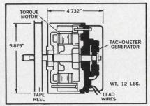
turned from conventional tape transport designs and developed a unique militarized system capable of optimum tape handling without damage or distortion. This modern, miniaturized design provides rapid reversal (less than 6 milliseconds) so programming is not restricted, high controlled acceleration and deceleration, (empty reel: 570 rad/sec², full reel: 270 rad/sec²), wide dynamic speed ranges (1000/1).
