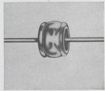
A miniature spark gap has a striking voltage of 90 Vdc. It is a radioactive isotope prompted gas-filled surge voltage protector. Current carrying capacity is 5000A for a 10to 20-us waveform. Capacitance is 2 pF and insulation resistance under unignited condition is  $10^{10} \Omega$ . The protector measures 0.38-inch in diameter and 1/4-inch in length.
