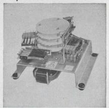
This 80-circuit motor-driven sequence cam switch has a 106 cycle life. Up to 80 spdt contacts can be operated at speeds of 1 through 35 cycles/minute. A maximum of 20 notches on each cam can be obtained. Four notched or unnotched cams are maximum for standard unit. The switch is designed for repeat cycle control.
