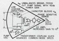
Amplifier input, ein, varies varactor capacitance, unbalances bridge, and develops pump voltage output proportional to bridge unbalance. After low-noise AC amplifica-tion, pump voltage is phase-sensitively demodulated to restore correct polarity, then further boosted by DC amplifier. Final output is a replica of original input, amplified one million times.
