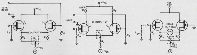
1. Matching minimizes the differences of FET pairs in differential amplifiers. Shown are a source-follower pair for impedance-matching (a), a source-coupled circuit for
