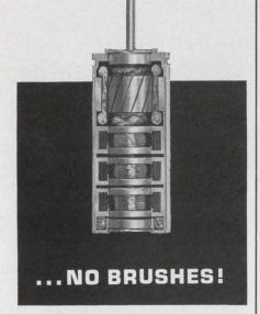
Rotary transformers couple power into rotors without contact, eliminating the numberone cause of early synchro failure. Without brushes, synchro life depends on bearing life alone-normally at least 5 or 6 times average brush life.
