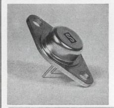
Series MHT 7901 through 7904 transistors are 10-A planar npn devices featuring sustaining voltages from 200 to 300 V. The transistors are offered in a TO-66 package with a power rating of 25 W at  $100^{\circ}$ C case temperature.  $I_{CBO}$  is 1  $\mu$ A max,  $V_{CE/SAT}$  is 0.5 V max at 5 A and  $h_{FE}$  is 50 MHz.
