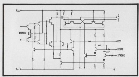
Figure 1. Circuit diagram of the SN7501 sense amplifier.
