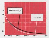
Compare charging current-time traces, reproduced from oscilloscope photographs. Sweep speed: 20 millisec/div. Vertical sensitivity:  $3\frac{1}{2}$   $\mu$ a/div.
