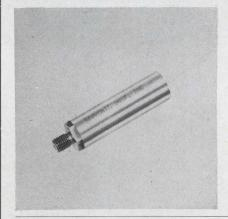
A potentiometer-type pressure transducer with a 0.655-in. diameter has accuracy exceeding 1%. Absolute or gage pressure ranges are 0 to 350 to 0 to 20,000 psi. Resistances are 2, 5, 7.5 and 10 kΩ  $\pm 5\%$ . The ac or dc output can be used for telemetry, control or actuating systems without amplification.
