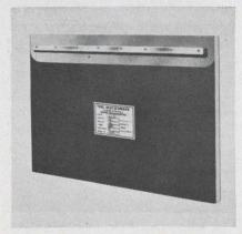
For an energy-storage capacity of 312 J at 25 kV, model ESC-259 parallel-plate capacitors have 0.5 nH self-inductance. Q in excess of 250 at 5 MHz results from the use of impregnated mica-paper as dielectric. Capacitors are available from 500 pF to 10  $\mu$ F at voltage ratings to 25 kV.
