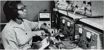
100% testing for 450 Mc/s gain and noise figure
