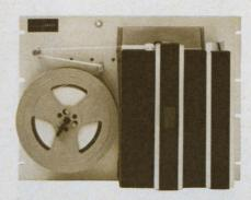
interrogation during a punching cycle and before the tape is advanced to the next character. If an incorrect parity code is sensed, (1) tape advance is inhibited, (2) the code in error is overpunched with an all-hole delete code, (3) tape is advanced and the same character punched again. Clean accurate tapes are a virtual certainty.
