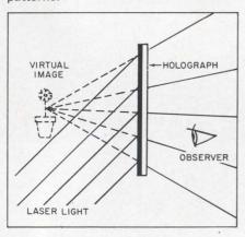
2. An observer sees a virtual image of the object when the holograph is illuminated with laser light that strikes it at the same angle as it did during exposure.
