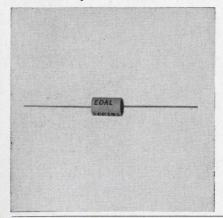
Connected across an inductive circuit element, series R selenium contact protectors suppress voltage surges from switching and offer protection against arcing. The devices can handle coil voltages from 26 to 250 V and currents from 150 mA to 1.2 A. The protectors are suitable for ac and dc applications and custom epoxy packages and spring clips are available.
