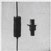
Two silicon planar epitaxial tuning varactors for vhf and uhf use are encased in a coaxial or TO-7 package. Any capacitance value from 6 to 25 pF for type MC301 and 26 to 47 pF for MC302 may be specified. Both have a PIV of 40 V and an operating range of -65 to +175 °C. They dissipate 500 mW derating at 1.67 mW/°C from 25°C.
