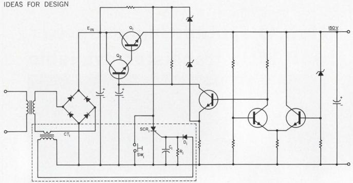
Current transformer and SCR circuit protect voltage regulator from overload damage.
