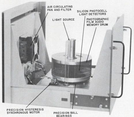
The Speechmaker's narrow light beam is modulated as it shines through the film on the drum. Photocells inside the drum detect the light.
