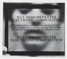
Videocomp system produces electronically generated characters such as these.
