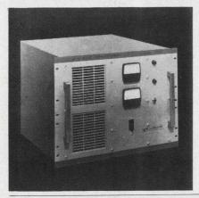
Series 3000 ac line conditioner offers complete isolation from power lines. With response time of  $50~\mu s$  max, input/output isolation of 10~dB, output distortion of 0.25% max and regulation of  $\pm 0.05\%$ , the units provide 2-1/2 kVA transient-free ac power. Models are available to operate at 47 to 53, 57 to 63 and 380 to 420 Hz.
