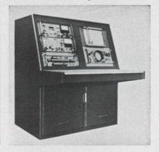
Model DS12 synchronization system provides speed/phase and indexing control of a magnetic storage drum. An unlimited number of drums may be synchronized with a time displacement error between drums of less than 200 ns. The system couples drums using an external reference frequency which becomes the clock frequency for the computer or display system.
