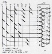
Fig. 1. Binary-to-decimal converter with drivers
