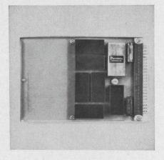
This analog-to-digital converter card uses integrated circuits. Input range is  $\pm 5$  V and conversion time is 1  $\mu s$ /bit max. Output format is 10 parallel binary bit data. Conversion frequencies exceed 100 kHz with internal or remote clock command. Resolution is 10 bits and linearity is 0.05% or 1/2 bit.
