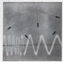
Types 1N5139 to 48 and 1N5139-A to 48A voltage-variable capacitance diodes are designed for RF tuning in the vhf band and above. Reverse leakage current is 20 nA max. Minimum Q is 200 to 350 at 50 MHz and 4 Vdc bias. Tuning ratio is typically 2.9 to 3.4. The "Epicaps" are available in ten types with capacitances of 6.8 to 47 pF at 4 V. Tolerances are 5 and 10%.
