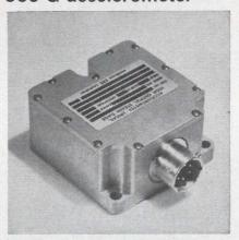
This strain gage accelerometer has a built-in amplifier capable of directly driving magnetic tape or oscillograph recorders. Output of the type 4-290 is amplified by an integral stable differential dc amplifier to  $\pm 5$  Vdc. Acceleration range is  $\pm 5$  to  $\pm 500$  G. Operable temperature range is -65 to  $+250^{\circ}$ F, and weight is less than 7 oz. The unit measures acceleration perpendicular to the mounting surface.
