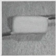
Standard resistance range of this 0.0015-in.<sup>3</sup> resistor is 50 to 200 k $\Omega$ . Applications include amplifiers and preamps, wave shaping networks and logic modules. Model 4200 offers a cermet element, an alumina substrate and weldable and solderable leads. Power rating is 70 mW at 100°C, temperature range is − 65 to + 150°C and resistance tolerances available are 1, 5 or 10%.
