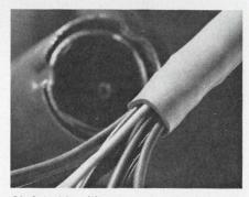
Shrinkable silicone rubber tubing can be the answer where wiring harness and electronic devices or components must be protected. Silastic® brand heat shrinkable tubing simplifies processing—reduces cost—where quick, easy fabrication of a close-fitting insulating covering for splices, leads, or components is required. Shrinks to ½ dia. when heated to 300 F or higher ... in length less than 5%. (Circle No. 853)
