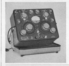
This capacitance bridge has a range of 1 pF to 1.1 farads and incorporates a 120-Hz generator, detector and adjustable dc polarizing supply. Three-, four- and five-terminal measurements can be made with the type 1617-A bridge. The built-in bias supply has six ranges to 600 V. External bias up to 800 V can be applied. The bridge measures dissipation factors up to 10.
