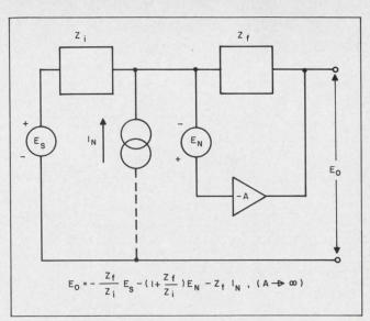
1. Generalized equivalent circuit of noise in an operational amplifier, and the transfer equation, including noise voltage generator,  $E_{\rm N}$ , and noise current generator,  $I_{\rm N}$ .
