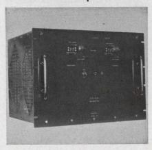
This deflection amplifier is a  $\pm 40$  V driver with regulated power supplies and safety current limiting. The all-silicon unit provides a 12-A change in less than 9  $\mu$ s with a linearity of 0.02%. Requiring 115 Vac, the amplifier handles from dc to pulses. This unit is compatible with single-ended yokes and needs no synthesizing networks.
