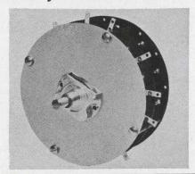
A line of magnetic reed rotary switches consists of eight models. They are available with form A or C contacts, or in combination. The rhodium contacts are isolated so that each stack handles up to 12 individual circuits. Models are available handling 1000 V max, 15 A inrush and 3 A steady.
