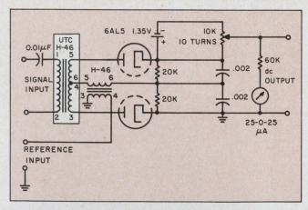
2. Pulse transformers replace special high-frequency coils in phase-lock detectors operating at 2 MHz. Their low capacitive coupling from the primary to the secondary side makes the change possible.
