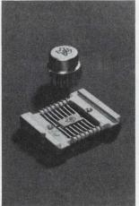
Figure 6. Package types for TI linear integrated circuits.
