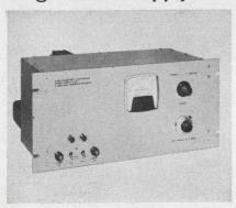
A fully programable, amplifier-type power supply has an output voltage of 0 to 3000 V. Programing voltage is +85 V. Line regulation is 0.001%, load regulation is 0.0007% and ripple is 5 mV rms. Model V-302 is available as a rack-mount or in a remote version. Input is 105 to 125 Vac.
