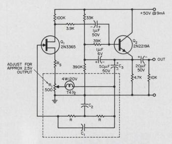
N-channel FET and emitter-follower are employed in this oscillator circuit. Notch network and lamp form degenerative and regenerative feedback loops, respectively. The latter feedback is used for output stability.
