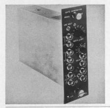
The GG200 gate generator has 6 outputs including system logic and gate signals and their complements. Delayed positive and negative trigger signals at the end of each cycle permit use as a delay generator. Gating time range is 100 ns to 11 s in 8 overlapping ranges. The cycle may be started and stopped by  $\pm 5$ -to  $\pm 50$ -V pulses as well as logic signals. All outputs drive 50- $\Omega$  loads.
