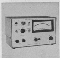
Model 624 A peak holding charge amplifier with 10-turn potentiometer and 7-step range switch accepts inputs from 50 to 1000 pC. A continuously adjustable automatic reset has periods ranging from 10 to 30 s. Input impedance is  $10^{14} \Omega$  for calibration and  $10^{11} \Omega$  in operation. Sensitivity can be adjusted from 0.1 to 100 mV/psi, G or lb.
