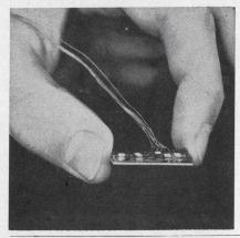
A hybrid microelectronic dc amplifier, TMS 1301, occupies less than 0.1-in.3. The amplifier operates from a power supply voltage of ±12 V and has a minimum dynamic range of ±8 V. Bandwidth is 1 MHz, gain is nominally 1000 and offset at the input is 4 mV. Packaging arrangements are available to special order.
