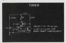
This basic circuit can be used for an enlarger timer, metronome, or other timing
