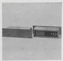
Model LRJR49 thermocouple reference junction provides a precise  $150^{\circ}\text{F}$  reference for up to 12 measurement channels. Designed for 105 to 125 Vac operation, the unit has stability and uniformity of  $\pm 0.1^{\circ}\text{F}$ , channel-to-channel, over an ambient range of 20 to  $120^{\circ}\text{F}$ . Power consumption is 30 W max and warmup time is 15 minutes.
