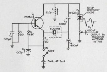
**Crystal oscillator** and step-recovery diode combine to form an RF calibrator. Battery operated, the harmonic-rich circuit draws only 2 mA.
