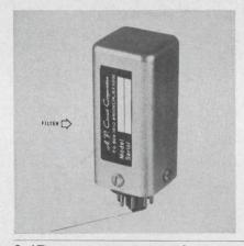
Model APN-60 is an active notch-filter which eliminates the 60-Hz frequency without signal distortion. Rejection bandwidth of this filter can be narrowed to 2 Hz without a phase shift in the pass band. Pass band is dc to 25 kHz with a max insertion loss of 0.5 dB. Power required is a regulated  $\pm 12$  V at 2.5 mA. Input impedance is 1 M $\Omega$ .
