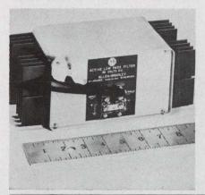
This low-pass active filter offers 60-dB min attenuation from 3 Hz to 100 kHz and handles 5 A dc. It is designed to prevent noise generated by a randomly fluctuating load from being reflected through the power supply and into the distribution system. Typically, a 30-A spike drawn by the load will be attenuated to 3 mA at the power supply. Custom units are available.
