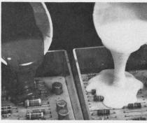
Dow Corning® 3110 RTV encapsulant can be readily color coded by mixing in master batch pigments. It is a low viscosity, deep section curing compound that cures at room temperature and is designed for potting, encapsulating and embedding of electronic circuit and components. It flows readily into place and cures to form a tough, resilient solid. (Circle No. 851)
