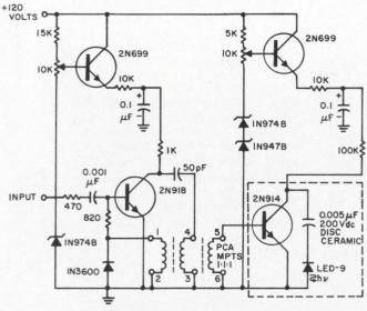
2. The basic light-pulse generator may be converted into a voltage generator. Here an avalanche blocking oscillator is driving the LED relaxation\*circuit.
