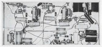
5. A 400-Hz detector, designed with conventional components, has a 1-Hz bandwidth and a 60-Hz rejection of 100 dB. The least detectable signal is 60 nV with a signal to noise ratio of 6 dB.
