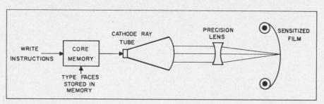
When brought from memory, characters are written on the face of the CRT and then projected through a lens on to sensitized film. Each character is stored in the form of many bits.
