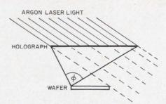
4. Holographs resolve best when the angle they subtend at the wafer,  $\phi$ , is large. But residual light from the laser beam (broken lines) must not fall on photoresist.
