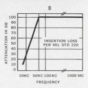
Graphs A and B show typical characteristics of Potter signal line filters. These filters are used on systems which must meet Defense Communications Agency criteria and provide maximum attenuation above the pass band with less than ½ db attenuation in the pass band.
