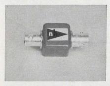
Housed in a sealed metal container, type JA transformer provides a 50- to  $75-\Omega$  unbalanced impedance match from 0.1 to 250 MHz for the 3-dB down points. It is rated at 5 W from 1 to 250 MHz.
