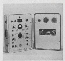
Automatic field tests to NASA specs are made with QC 275 cable tester. Resistance testing is performed with simulated load currents from 40 mA to 1 A. Leakage resistance is measurable to 5000 M $\Omega$  with go no-go settings at 50, 100, 150 and 200 M $\Omega$ . Total capacity is 75 circuits with adjustable dwell time from 0.5 to 15 s.
