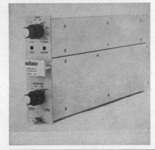
An all-silicon solid state differential dc amplifier features  $\pm 300~V$  common-mode voltage capability and gains from 1 to 2500, with 100  $M\Omega$  input impedance. Output is  $\pm 10~V\text{-}$  at  $\pm 100~mA$ . Common mode rejection is 160 dB at dc. Switch-selected bandwidth filters have standard values of 10 kHz, 1 kHz, 100 Hz and 10 Hz. Settling time is 100 ms max.
