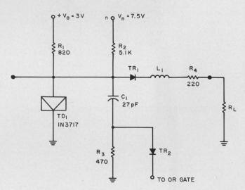
3. Basic neuron circuit is used in propagating chain and in circuits that couple to OR gates.
