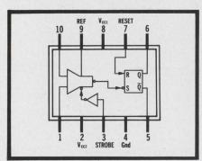
Figure 4. SN7501 incorporates flip-flop
