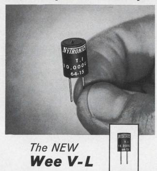
Adjustable Inductance range  $0.15\mu h$  to  $100,000\mu h$  in 0.300'' by 0.400'' molded case with 0.200'' grid spacing.
