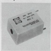
A new passive band pass filter is designed to eliminate saturation and third harmonic distortion problems. The output signal is typically phase-adjustable to  $\pm 10^{\circ}$  ( $\pm 5^{\circ}$  min). Insertion loss is 3 dB.
