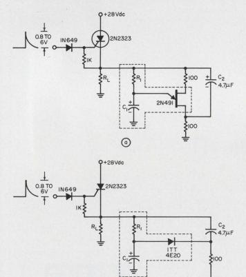
1. Remote-control time delay is formed by SCR-UJT combination (a). For higher load currents, a 4-layer diode is substituted for the UJT (b). No shut-off signal is required in either case. Delay duration is set by R<sub>1</sub>C<sub>1</sub> in both circuits.
