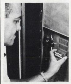
Ten transistors in a plug holder are placed in thermostat-controlled aging chamber.
