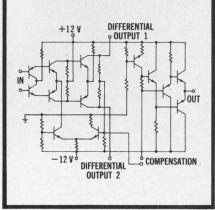
Figure 9. Circuit diagram of SN726 operational amplifier.
