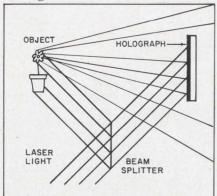
1. Holographs are exposed when an uninterrupted laser beam strikes the photosensitive surface at the same time as the laser light that diffuses from the surface of the object. Unlike photographs, which record amplitude patterns, holographs record both amplitude and phase in interference patterns.
