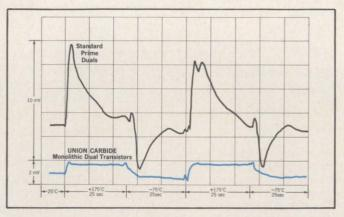
Comparative thermal transient response of standard prime duals and UCE Monolithic Dual Transistors.
