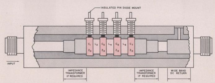
3. Construction of switch or limiter may include two or more impedance transformers. Some parasitic capacitance results from the abrupt change in the diameter of the line between a diode package and the inductive transmission-line segments. The low-pass filter structure is built with seven elements, as in Fig. 1. bias voltage to the center conductor and, if the diodes are matched, each will be equally biased.
