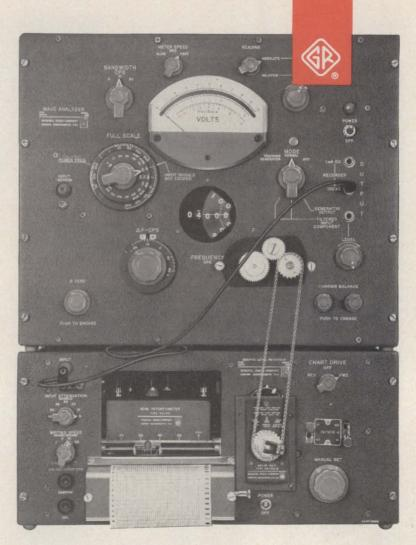
A Choice of BANDWIDTHS: 3, 10, and 50 c/s Bandwidth skirts are better than 80-dB down at  $\pm 25$  c/s,  $\pm 80$  c/s, and ±500 c/s for 3-, 10-, and 50-cycle bandwidths, respectively.
