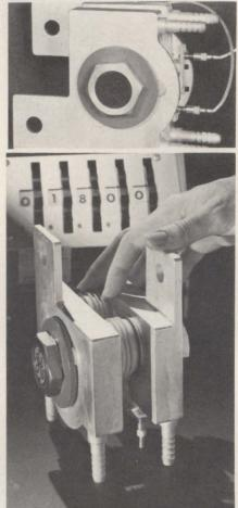
Direct operation from 480-volt distribution lines is the featured capability of a series of SCRs for industrial applications. The watercooled units have a power-handling capability of 1200 amps rms and a blocking rating of 1800 volts. This permits switching of 1.5-megawatt loads.
