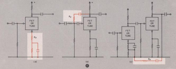
1. **Distortion in amplifying devices** is measured by this test circuit (a). Comparing the test results for a 12AT7 tube and a DNL-Q-A FET (b), it is evident that the FET shows less harmonic distortion. Feedback arrangements
