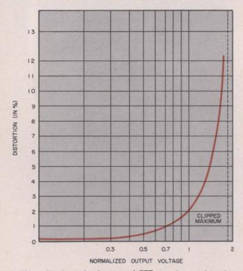
2. Normalized overload curve of FET may be used to determine output signal for a given distortion level. Unity output voltage (normalized) occurs for 2% distortion. Note that clipping of the output occurs at 1.8 volts. of additional collector distortion occurs. The relatively high distortion is unavoidable because of the inherently nonlinear input characteristic of the transistor. It is due to the forward-biased diode operated in a current mode and associated with a small load resistance.
