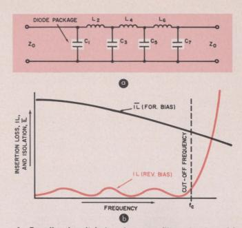
**1. Broadband switch** has low-pass filter structure (a). When diodes are reverse-biased, the structure acts as a low-pass filter and the insertion loss is small (b). During forward bias, the diodes appear as inductive elements, and because the matched condition is destroyed, the signal will be greatly attenuated.
