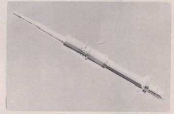
**5.** Radial mounting of diodes in a microwave switch or limiter increases the device's power-handling capability. This coaxial switch covers the frequency range of from 1 to 4.5 GHz and can switch 30 kW peak and 30 watts average power in 200 ns.
