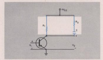
2. Complex-load network consisting of RC pair replaces ordinary load,  $R_L$ . This modification makes the frequency response of the amplifier independent of variations in the transistor parameters.
