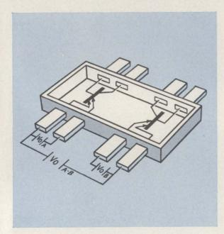
Sprague leads again with two dual-emitter chopper transistors in one flat-pack case, with tight V<sub>OFF</sub> matching of both devices
