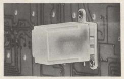
**Enclosed** type relay plugs into receptacle that is mounted directly to printed circuit board.
