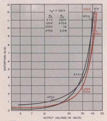
4. **FET overload characteristics** as a function of load resistance show that  $100k\Omega$  is the optimum drain resistance for combined, optimum gain-distortion. Larger loads yield increased gain at the expense of bandwidth.
