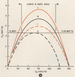
**High-voltage video-amplifier stages** (a) are rapidly designed by a five-step, power-oriented procedure. The technique, which is based upon the collector dissipation curves (b), helps the designer to choose from a number of transistors and determines the maximum achievable output.
