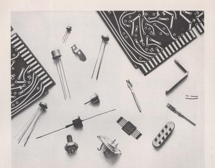
Gold-plated components conduct better, solder easier, reflect heat. and resist wear, corrosion, oxidation, galling.
