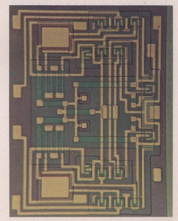
Typical of IC sophistication is the Motorola MC308. This high-speed JK flip-flop contains 16 transistors, two capacitors and many resistors.
