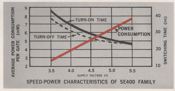
This family of four full MIL range integrated circuits features a dual 5 Mc Binary element operating on less than 9 mW per flip-flop. Like the other members of the family, it was designed for maximum speed consistent with low power operation. The family is intended for use in applications where high density packaging and the ability to drive high capacitances associated with multilayer printed circuit boards are important considerations. For complete data and specifications, write today.
