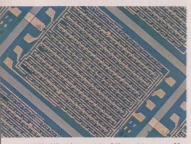
**90-bit shift register** contains 540 transistors on an 80- x 58-mil chip, deposited with MOS techniques.
