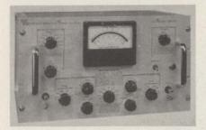
Featuring an accuracy of  $\pm 0.004$ degree of full scale at any range from 50 Hz to 20 kHz, the off-theshelf Type 203 Vectorlyzer is described by its manufacturer as the most accurate phase measuring instrument commercially available at a moderate price. In addition, it has a full scale range of 0.1 degree.
