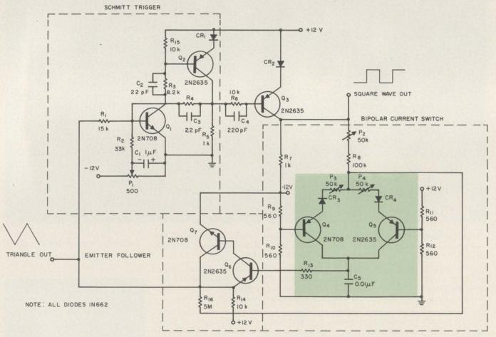
1. **Bipolar current sources** (color) are used in the charging network of a triangle generator. The output has constant amplitude over a 250:1 frequency range, since the Schmitt trigger's hysteresis is constant.
