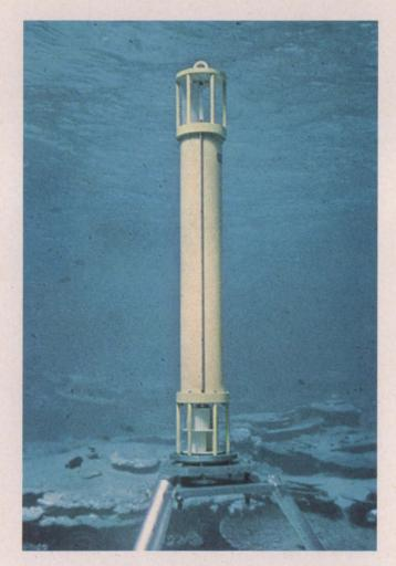
**Instrument package** developed by Bissett-Berman Corp. for measuring salinity and temperature at various depths.
