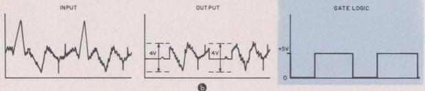
Pulse logic applied to the gating transistor,  $Q_a$ , of this video signal processor (a) determines which portions of
