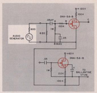
9. Frequency response in FET amplifiers is similar to results obtained with triodes. Circuit-capacitance test set-up is used to measure interelectrode capacitances and their
