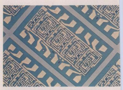
**Up-down counter** has four stages. Its 115 transistors are placed on a chip of 76- x 48-mil dimensions.
