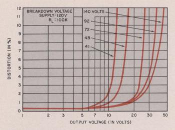
6. **Output voltage in FETs** as a function of breakdown ( $BV_{\rm DS}$ ) shows that for a specified output, harmonic distortion is larger in the lower breakdown units. The breakdown itself produces a clamping effect.
