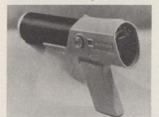
A new, low-cost infrared thermometer measures temperatures from  $150^{\circ}$  to  $3000^{\circ}$ F. The Rayner is a self-contained, light-weight pistol which is battery operated. When aimed at a surface, temperature is indicated on the calibrated meter housed in the rear of the instrument.
