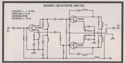
Figure 2: Wideband low-distortion amplifier employs 2N3995 transistors
