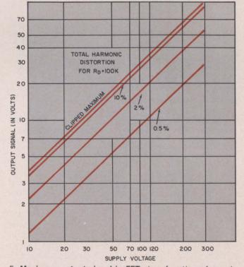
5. **Maximum output signal in FETs** is a function of supply voltage. For FETs with breakdown voltages in excess of the supply, the amplifier is supply-limited, rather than breakdown-limited. Note the excellent linearity.
