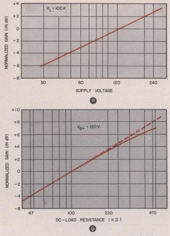
8. Gain is a function of both supply voltage and load resistance. Normalized gain vs supply-voltage curve (a) shows a 3-dB increase in gain with a doubling of the supply, because of the 3/2 FET power law. As a function of load (b), the gain increases by 3.5 dB for each doubling of the load resistance. Note that the ac-coupled load is five times the dc load resistance.
