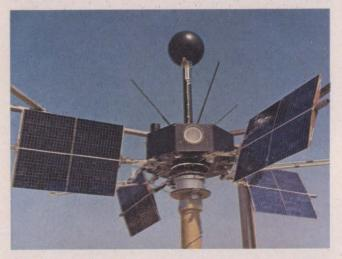
Now it's hardware and being checked out at the instrumentation site. IMP-C will measure magnetic fields, cosmic rays and solar wind.
