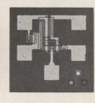
MEM590 Series Shunt Chopper. Zero offset voltage
