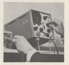
A new tester measures small signal parameters of transistors (including FETs) and junction leakage currents down to 1 namp. Gain measurements are made in a 1000 Hz bridge and leakage is tested through a MOS FET operation amplifier input.
