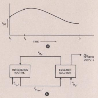
Fig. 3. **Transient programs** solve for network quantities in a series of individual time steps. For each step the initial circuit conditions are updated, and then an integration routne is carried out.
