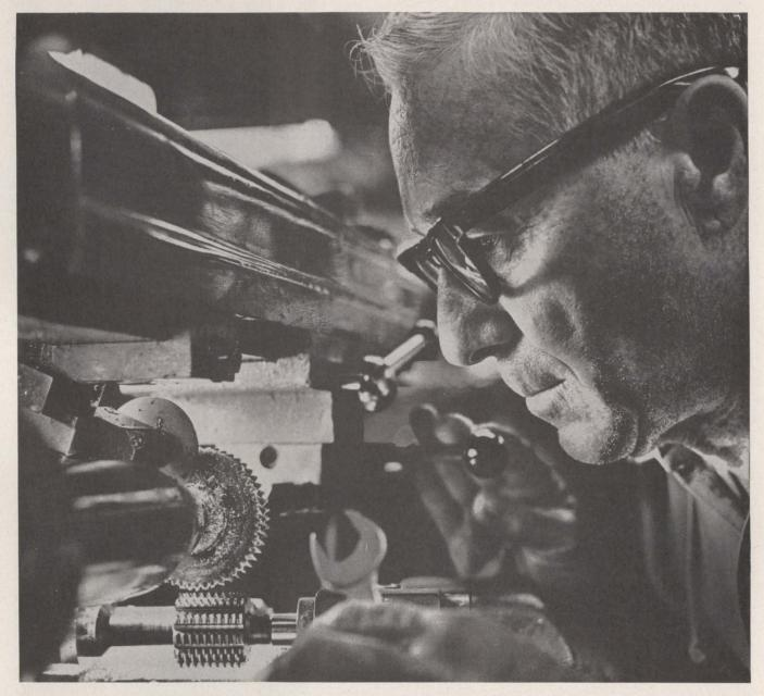
To attain consistent performance and long life in Bodine motors, we design and hob our gears to very close mechanical tolerances. By means of check points at all stages of gear manufacture, we can be sure these tolerances are kept.
