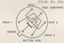
A six-lead device, the 2N4066-67 is an integrated dual-MOST.
