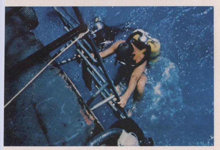
Diver in scuba gear goes over the side to implant instrument package on the ocean floor at depths of 30 to 40 feet. At greater depths, mechanized techniques are used to deposit instruments on ocean floor.
