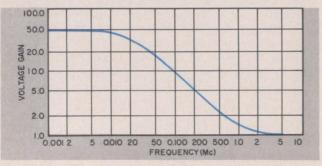
5. Single-order RC-type cutoff characteristic to beyond 1 MHz is exhibited by the amplifier in Fig. 4.
