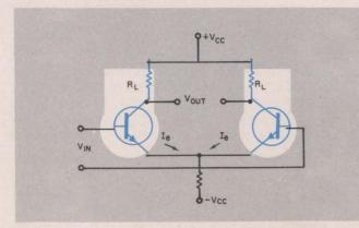
3. Differential amplifier-stage gain ( $G_v = -R_L/r_e$ ) can also be designed to be independent of transistor beta variations. Each stage's collector resistance ( $R_L$ ) is replaced by the appropriate RC network.
