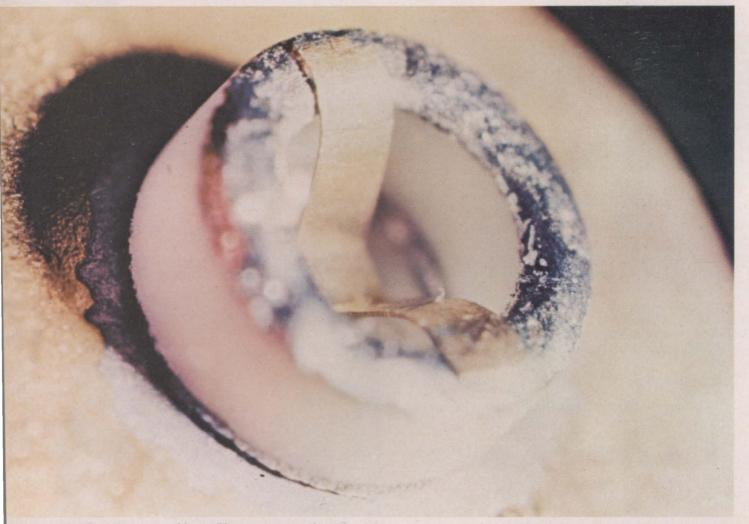
Simple gallium arsenide oscillator consists of a thin slab of gallium arsenide mounted on a copper heat sink. The top contact is insulated by an alumina washer from the heat sink, which is the bottom contact. Its operation is a manifestation of the Gunn effect. (Courtesy of IBM, T. J. Watson Research Center, N. Y.
