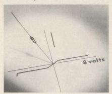
A line of two-terminal bistable switches change from the high-resistance "OFF state to a low-resistance ON state when the applied voltage exceeds a specified voltage. Voltage ratings from 8 to 12 v are available in the line with typical turn-on time at 50 ns and turn-off at 100 ns. Holding current is 4 mA and forward voltage drop is 1 V.
