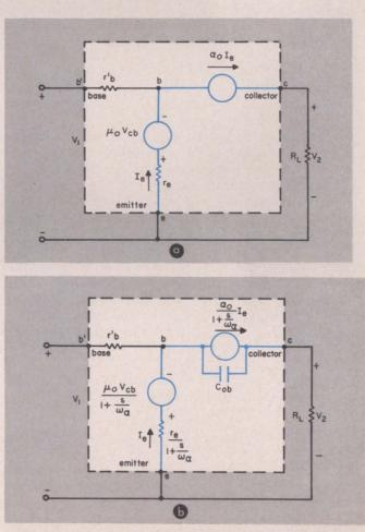
1. Simple T-type equivalent circuit for a low-frequency transistor-amplifier stage (a) is used to develop the gain and frequency response. The frequency-dependent parameters of transfer current, transfer voltage and diffusion resistance must be modified by the  $(1 + s/\omega\alpha)$  for frequencies approaching cutoff (b).
