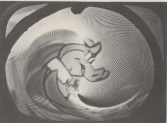
**Toroidal electromagnet** distorts TV for optical art. When line current ceases, giant spark lights the room.
