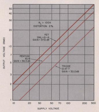
3. Maximum output voltage for FETs and tubes as a function of supply voltage shows that the FET provides more gain when the distortion level for all amplifying devices is normalized at 2%.
