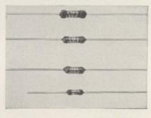
Power ratings from 1/20-watt to 1/8-watt are offered in the capped and conformally coated C Series resistors. The components cover a resistance range of 24.9 ohms to 500k in tolerances down to  $\pm 0.1\%$ . Stability and mechanical strength are well above the requirements of MIL R-10509.
