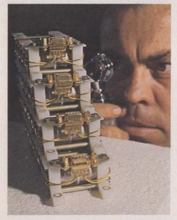
**Gold-plated wiring harness** connectors shown mounted on nickel-cadmium batteries carried in the Syncom communications satellite. Similar installation was used in the Early Bird satellite, and advanced version of Syncom.
