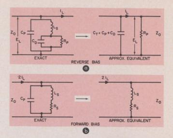
**4. Exact equivalent circuits** of the diode shunting the transmission line are needed to find the power-handling capacity during forward and reverse bias.
