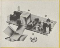
Higher density packaging . . . minimum magnetic interaction . . . no critical orientation . . . by enclosing magnetically sensitive components A, B, & C in Netic or Co-Netic. Saves Space, Time, Money, Weight Cuts easily to any outline . . . saving valuable time and weight, minimizing waste and tooling costs. Ideal for shielding hard-to-get-at components. Thicknesses from .002".
