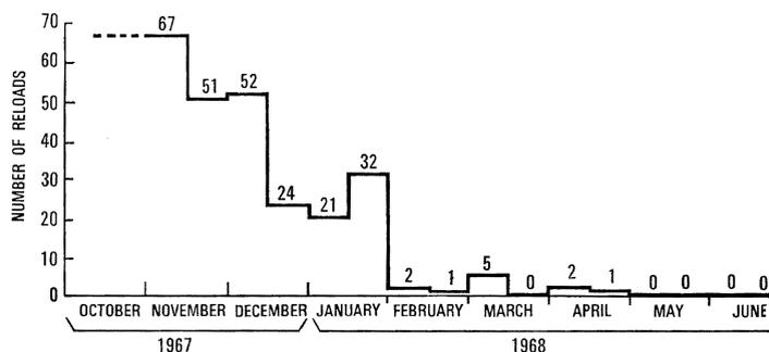
Figure 7 - Processor reloads caused by initial program faults.
