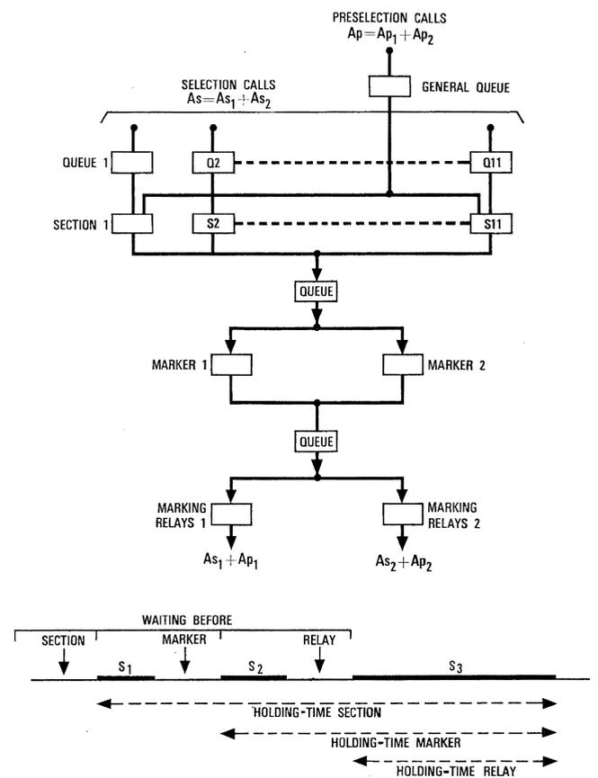
Figure 10 - Model of the control circuit.
