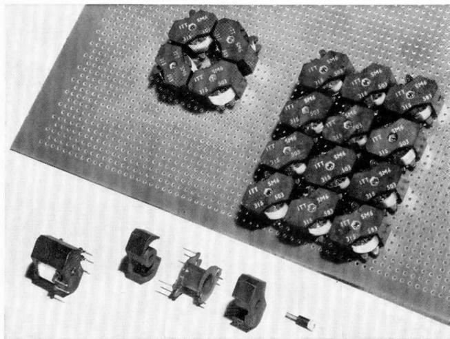
The new ferrite pot cores plug into printed-circuit boards and give a high packaging density.
