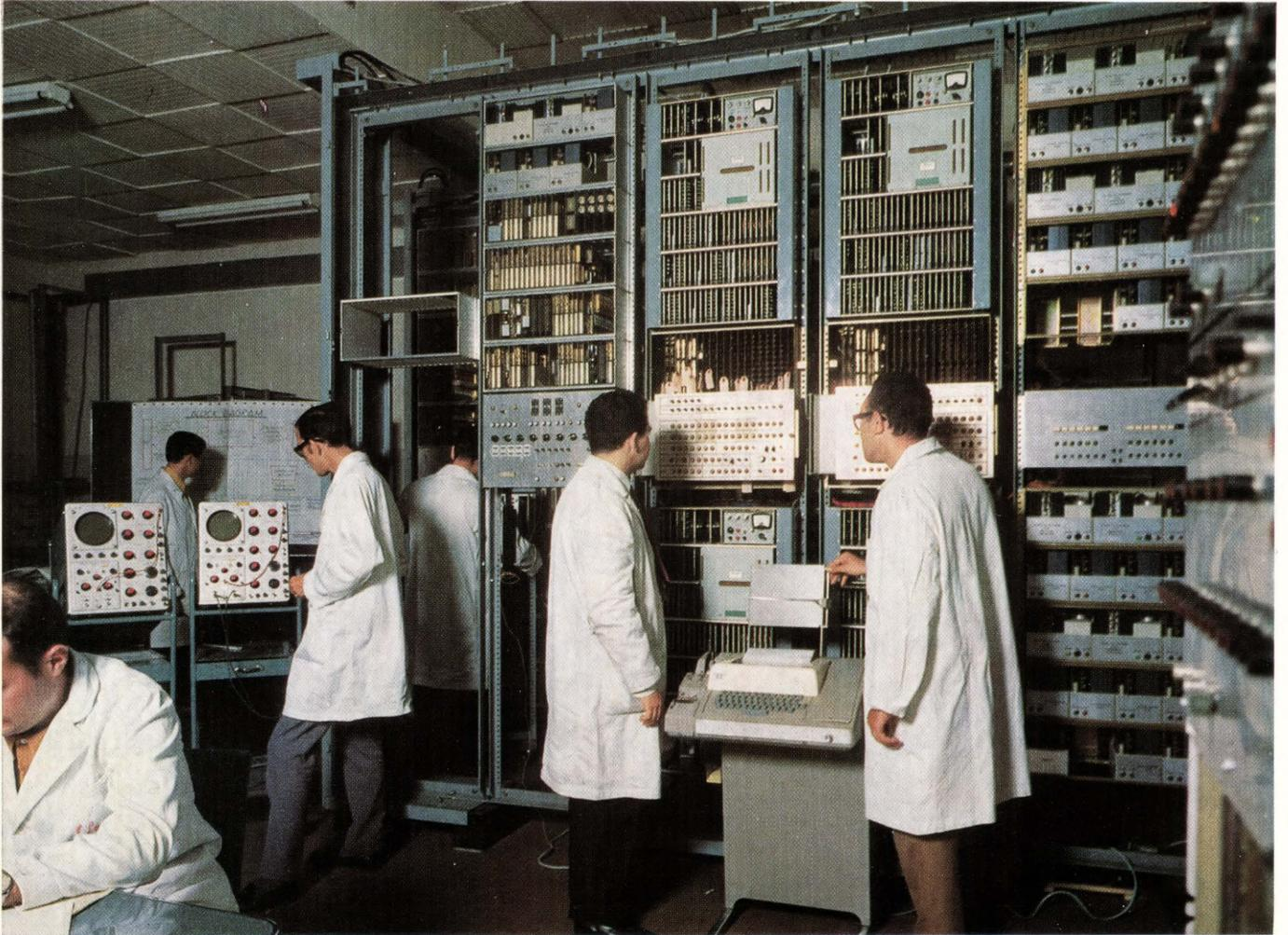
Figure 1 - Spanlab researchers have gained a capability and generated ideas that will contribute to ITT's next mainline electronic switching system. The photograph shows engineers running tests on equipment in the Semi-Electronic Switching Development Laboratory.
