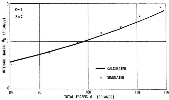
Figure 4 - Comparison of calculated and simulated interaid traffic.
