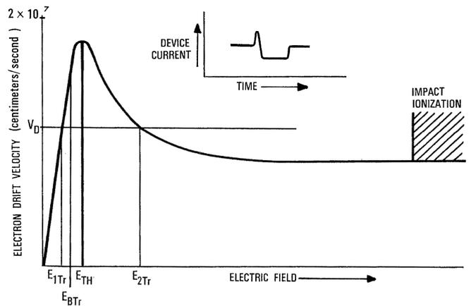
Figure 3 - The triggered-mode operation. Field distribution and one cycle of current waveform are shown in the inset.
