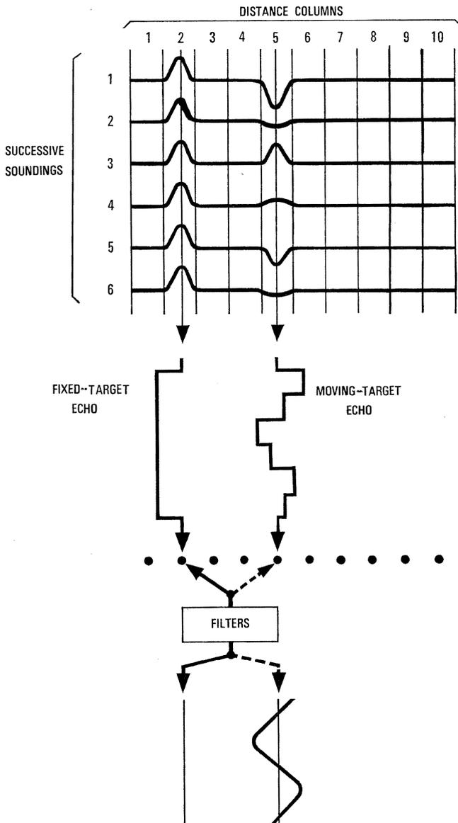
Figure 5 - Principle of the new system.
