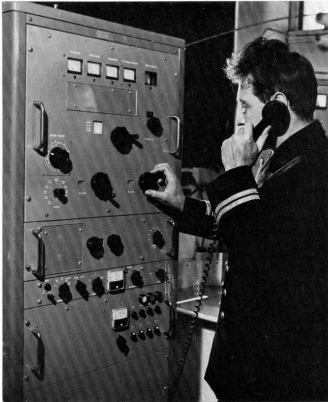
A radio officer operates a 1.5-kilowatt *ST 1400* transmitter similar to the one to be installed on the *Queen Elizabeth 2*.
