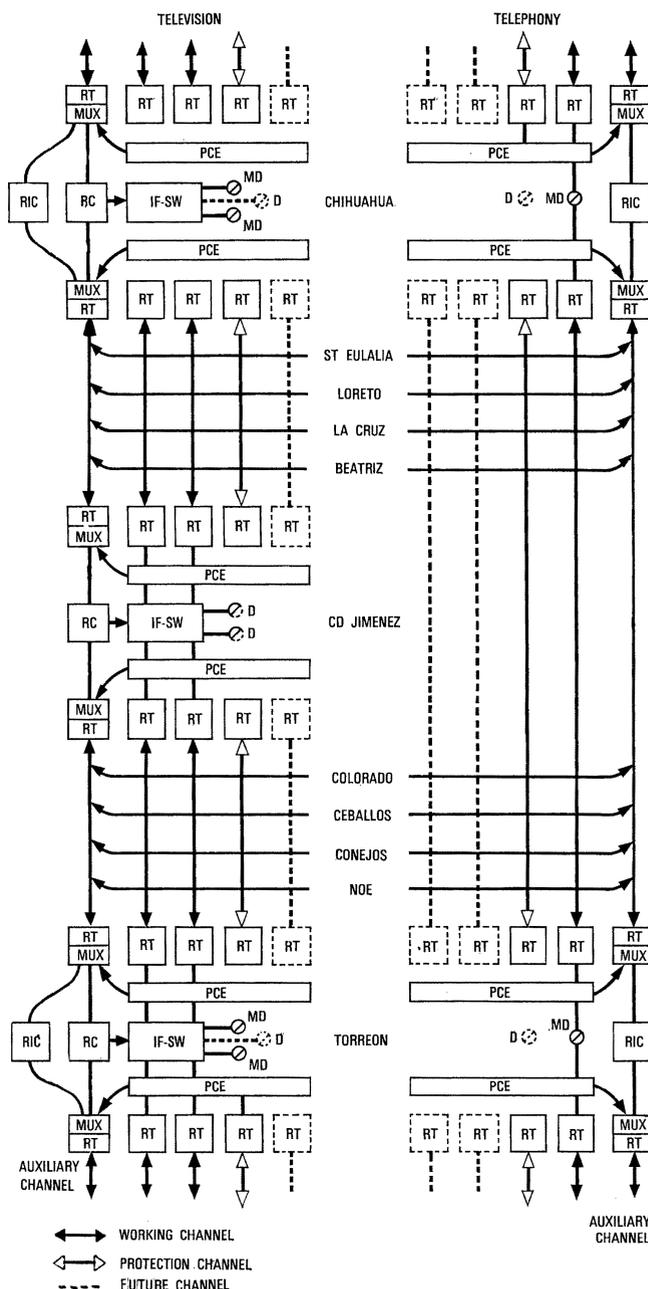
Figure 3 - Typical modulation section of the 6-gigahertz network in Mexico.
