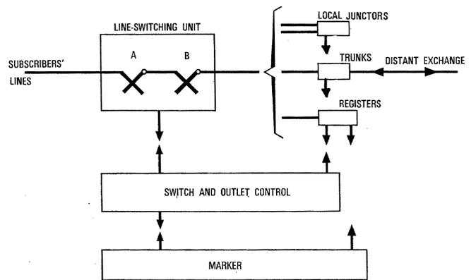
Figure 6 - The marking principle for a 2-stage exchange.
