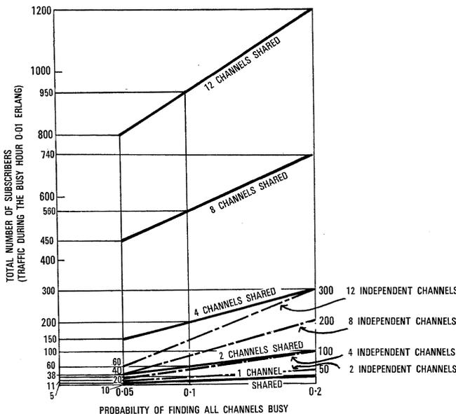
Figure 3 - Efficacy of channel sharing as opposed to independent channels.
