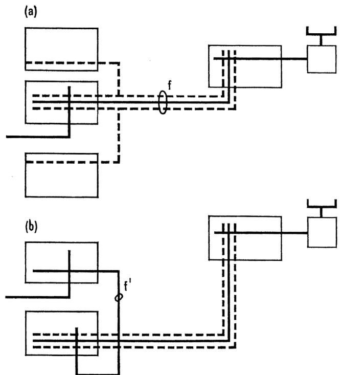
Figure 3 - Line selection through (a) 2 stages, and (b) 3 stages using interaid.
