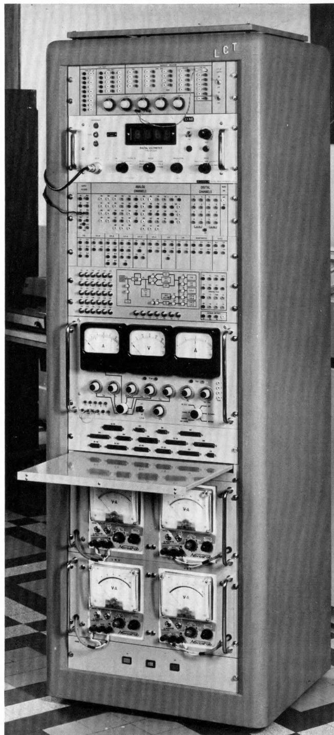
Flight equipment of the housekeeping system for the ESRO 1 satellite.
