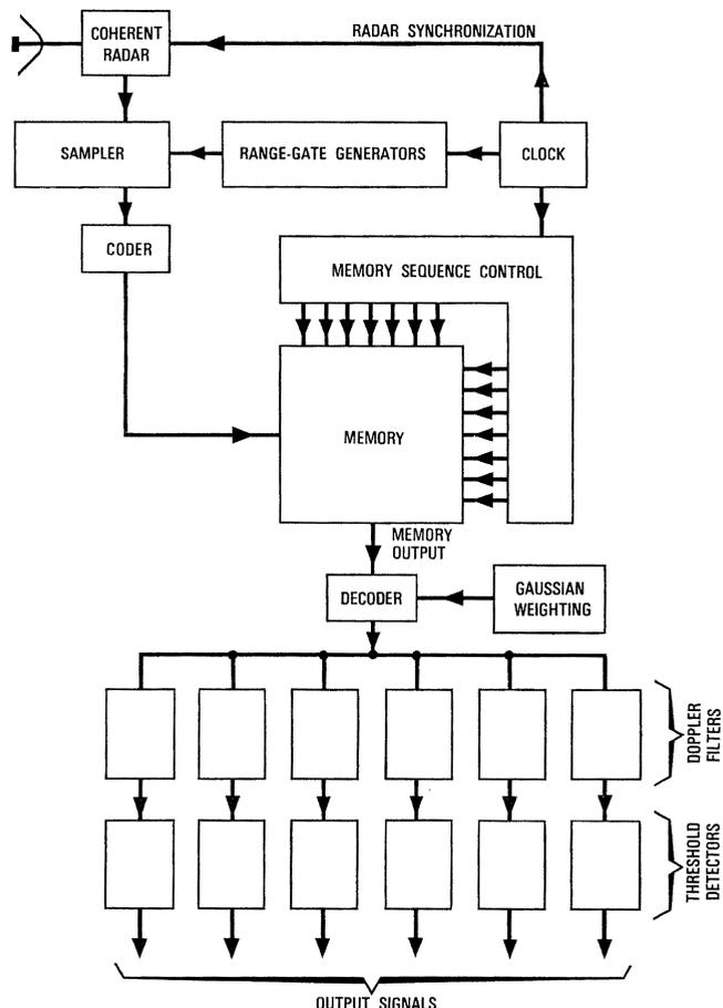
Figure 8 - General block diagram of the system.
