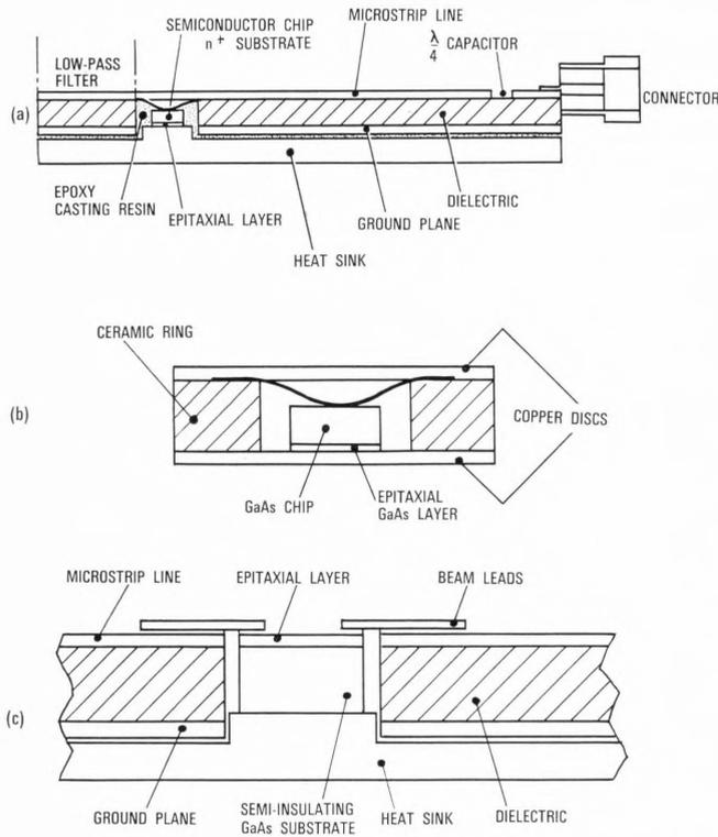
Figure 8 - Sectional drawings of devices mounted in microstrip circuit.
