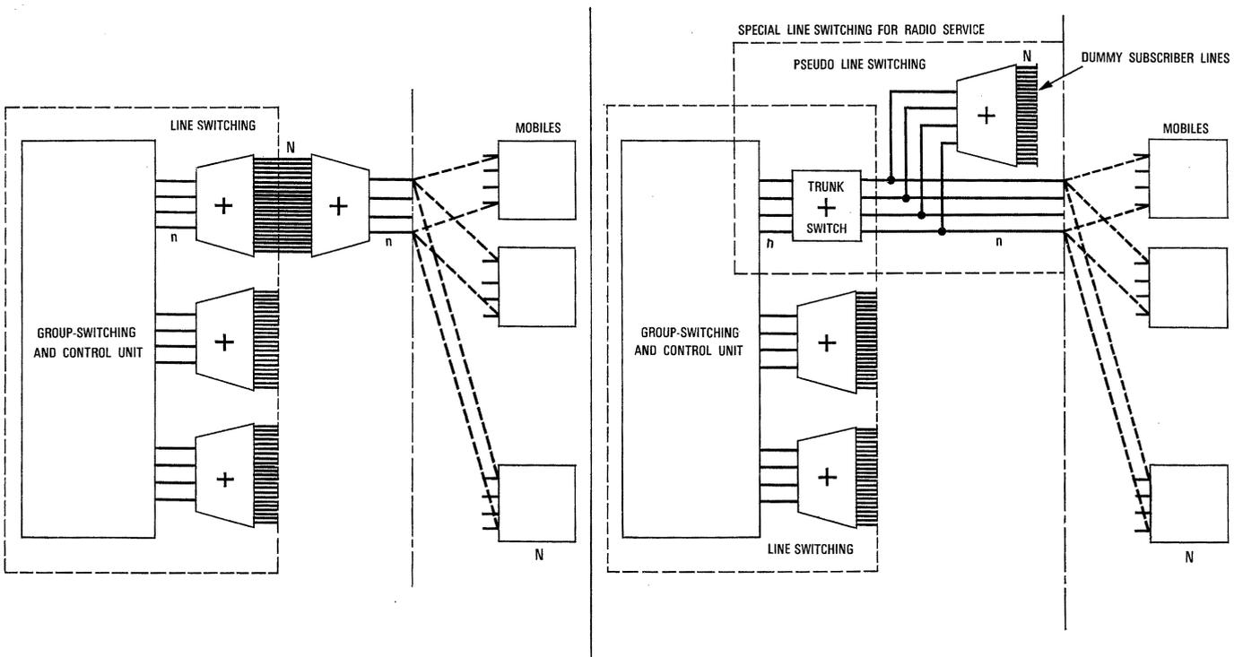
Figure 2 - Switching equipment, on the left the *IMTS* approach, and on the right, the *STAMP* approach.
