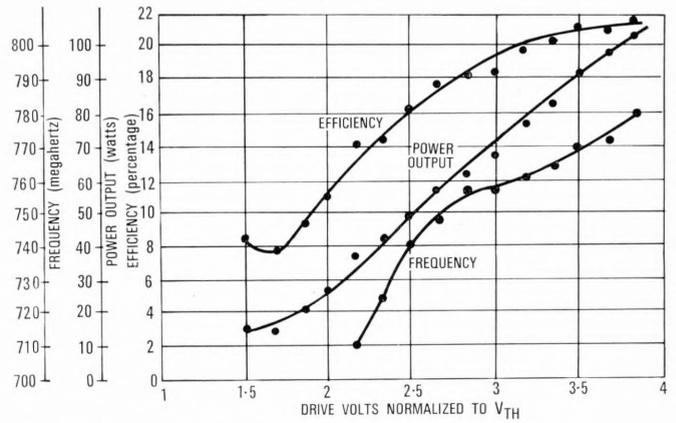
Figure 11 - Power, efficiency, and frequency for bulk device in lumped-element circuit.
