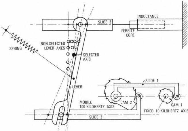
Figure 4 - Digital/analog mechanical principle.
