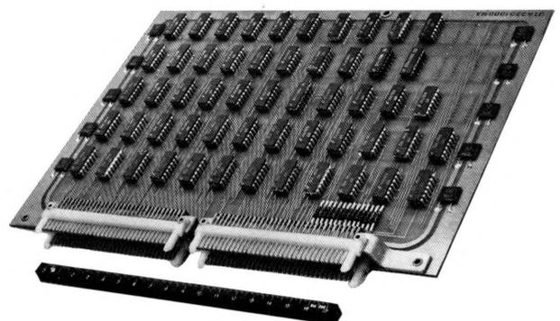
Figure 5 - Plug-in unit of the central processor.
