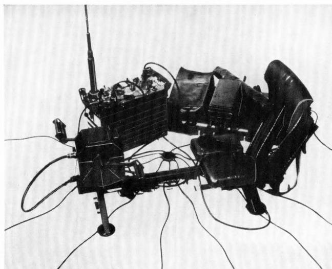
Figure 1 - Portable equipment with generator and buffer battery.
