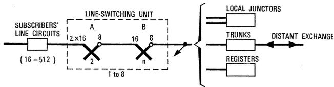
Figure 3 - A 2-stage exchange: 16 to 512 subscribers' lines.
