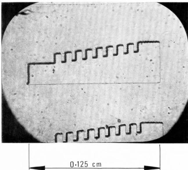
Figure 16 - A DOFIC fabricated in epitaxial gallium arsenide on a semi-insulating substrate.
