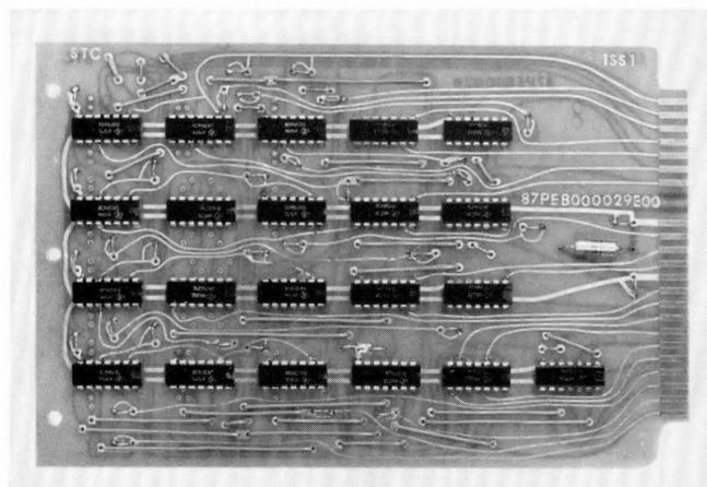
Figure 3 - A typical double-sided, plug-in, printed-circuit board.
