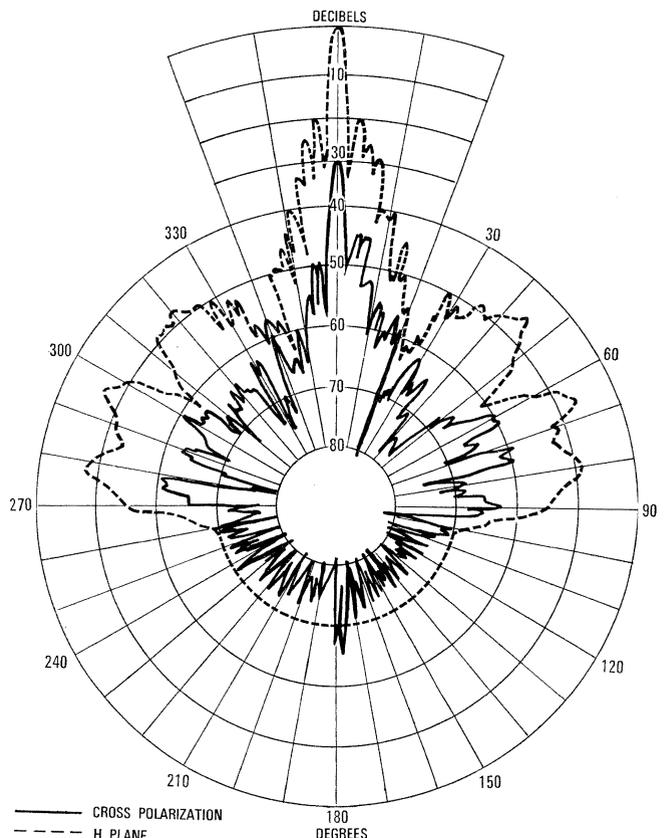
Figure 5 - Radiation patterns at 6.175 gigahertz of a 3-meter (10-foot) diameter Cassegrain antenna suitable for operation from 5.925 to 6.925 gigahertz.
