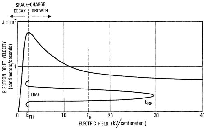
Figure 4 - Primary transferred-electron characteristic for gallium arsenide showing applied bias and radio-frequency amplitude for *LSA* operation.
