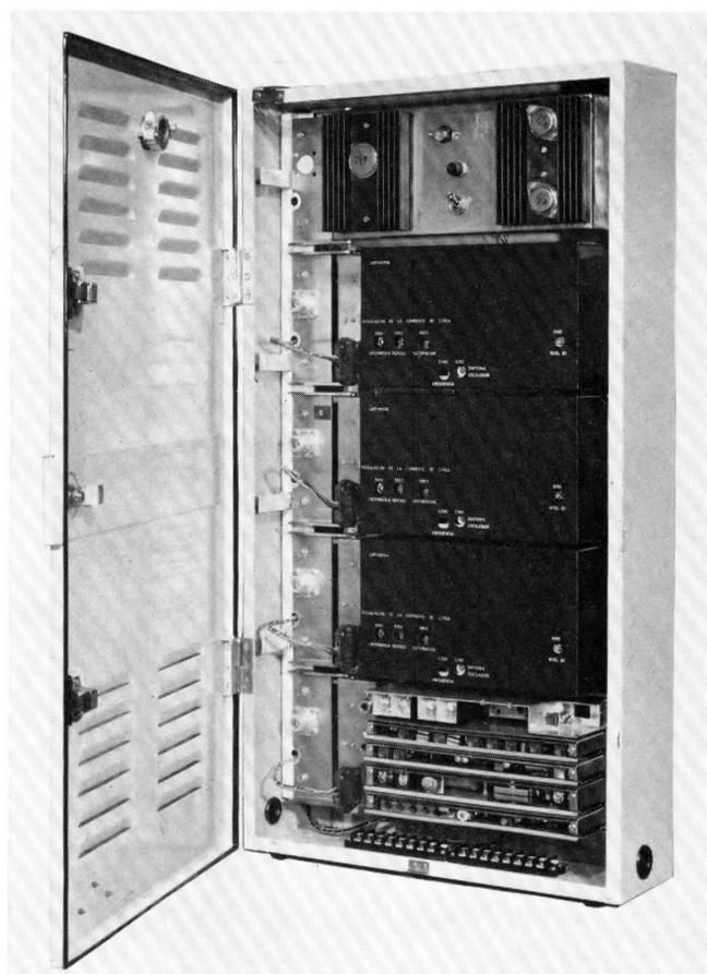
Figure 9 - Receiver cabinet in a 4-channel system.
