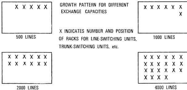
Figure 10 - Floor layouts up to 4000 lines.
