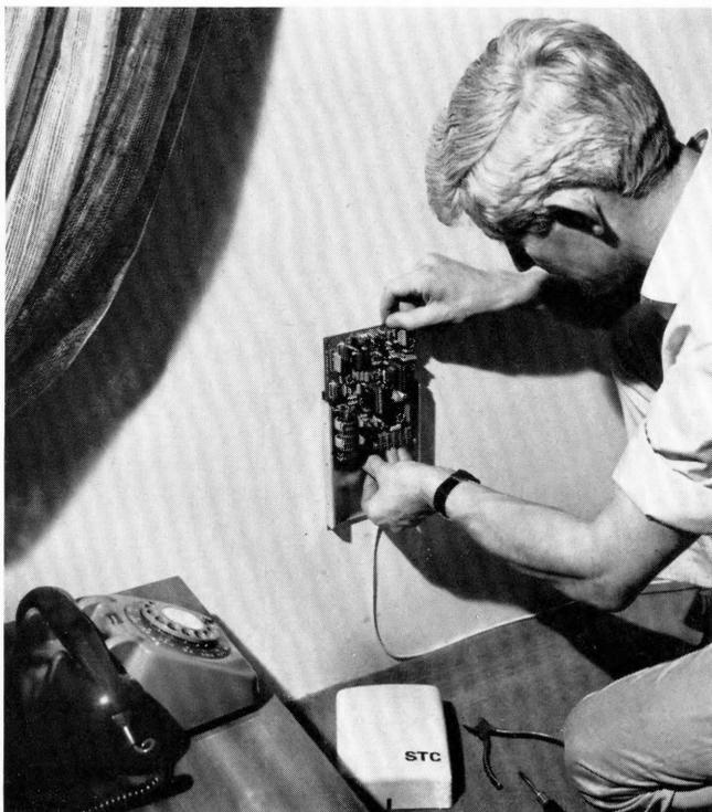
The *SUB-1A* subscriber carrier system compared with a standard telephone set.
