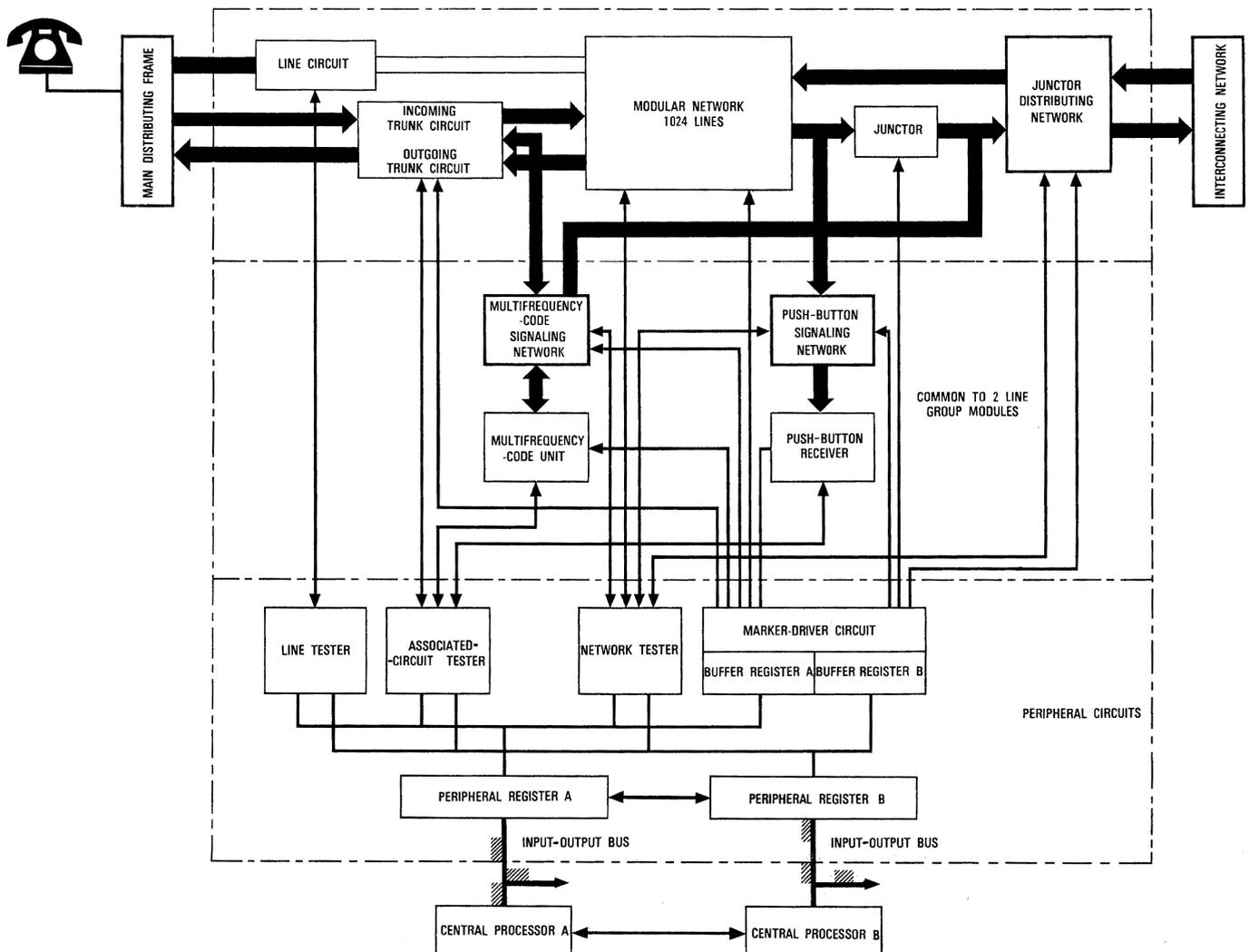
Figure 1 - The 10C peripheral package.
