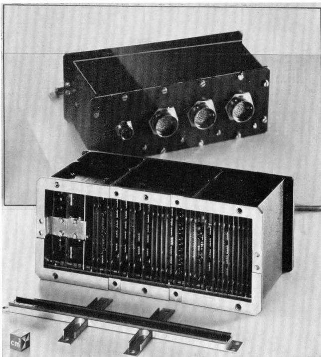
Figure 7 - PCM telemetry and command unit.
