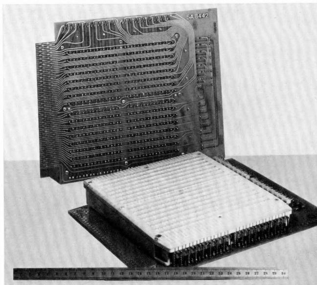
Figure 2 - The switch unit.
