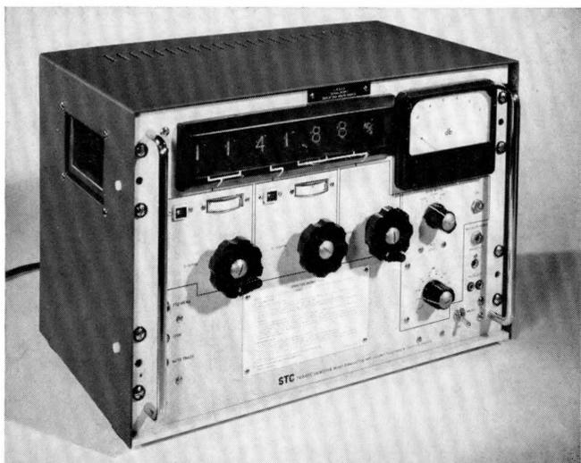
The 74314 frequency-selective level-measuring set has a digital readout of frequency updated at 0.2-second intervals.
