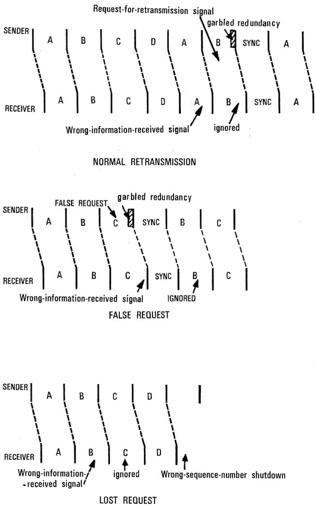
Figure 1 - Three simple cases of error control.
