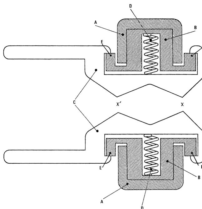
Figure 6 - Construction of the dual-face-type connector (transverse cross section).
