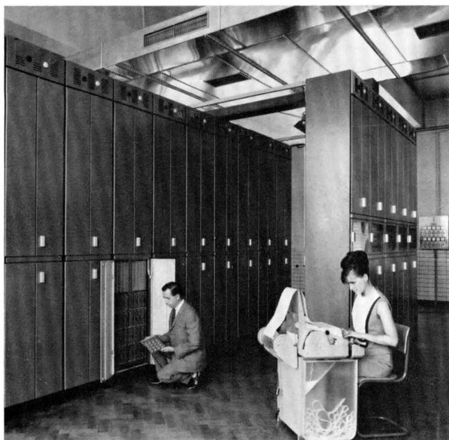
Figure 2 - The 10C exchange. On the left, a line-group module of 1000 lines. On the right, the central-control unit.
