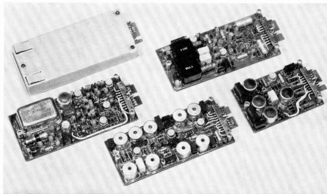
Figure 11 - Five printed-circuit cards with four of the covers removed.
