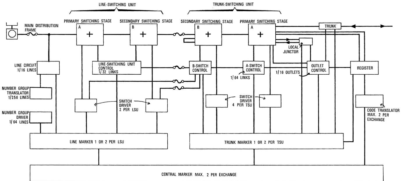
Figure 7 - Block diagram for a 4-stage exchange.
