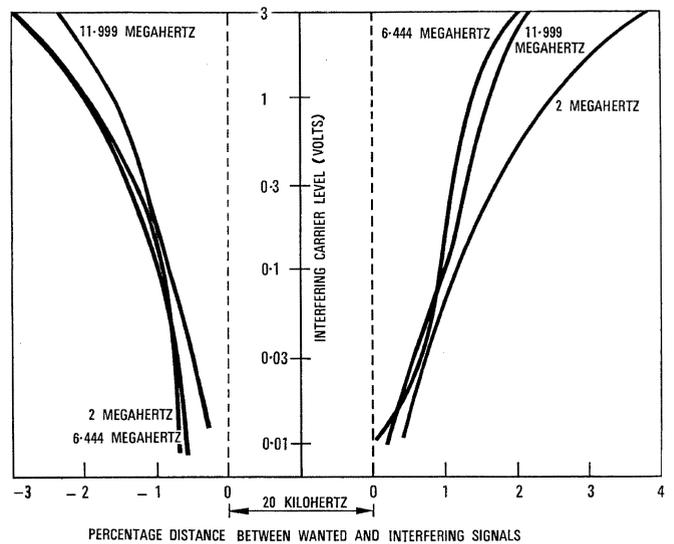
Figure 14 - Receiver cross-modulation limits.
