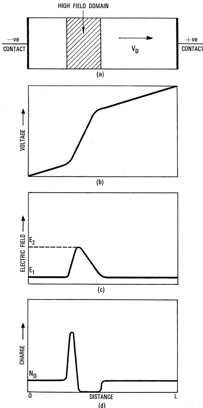
Figure 2 - (a) Representation of Gunn-effect oscillator, (b) Voltage distribution through the device, (c) Electric-field distribution, (d) Charge distribution.
