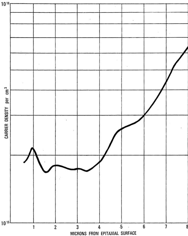
Figure 5 - Carrier-density profile through thickness of epitaxial gallium arsenide layer as derived from a Schottky barrier diode measurement.
