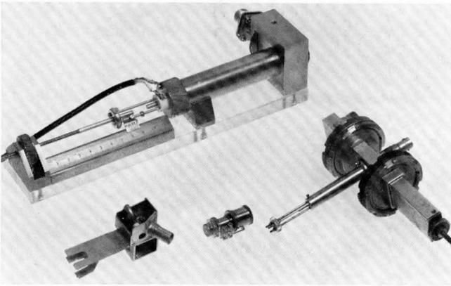
Figure 10 - Top - Wide range 3-to-12-gigahertz coaxial cavity with vernier tuning and adjustable output coupling.
