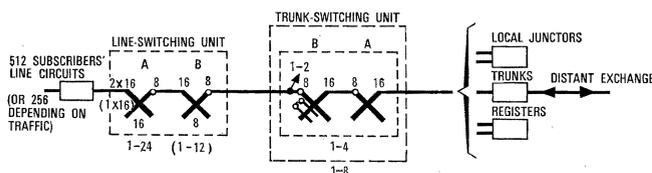
Figure 4 - A 4-stage exchange: 96 to 12 288 subscribers' lines.
