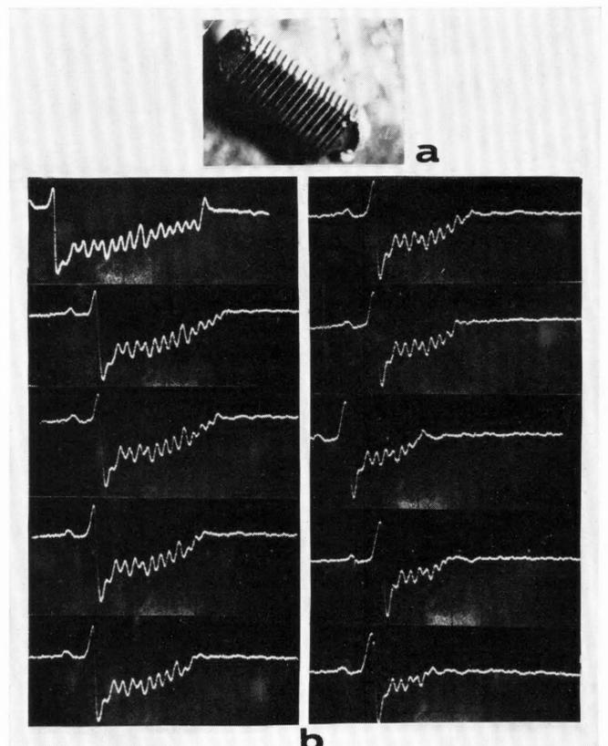
Figure 15 - (a) Geometrically coded device with 16 levels, (b) Current waveforms as a function of time for different domain transit distances.
