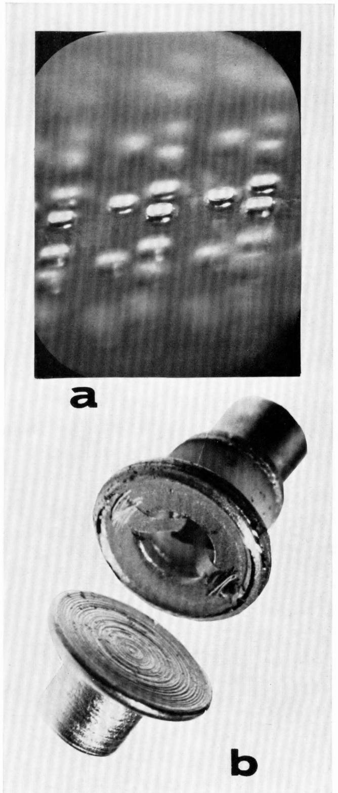
Figure 7 - (a) Continuous-wave epitaxial mesa devices with 0.004-inch (0.1 millimeter) diameter silver-tin evaporated contacts in groups of three on an  $n^+$  gallium-arsenide substrate.
