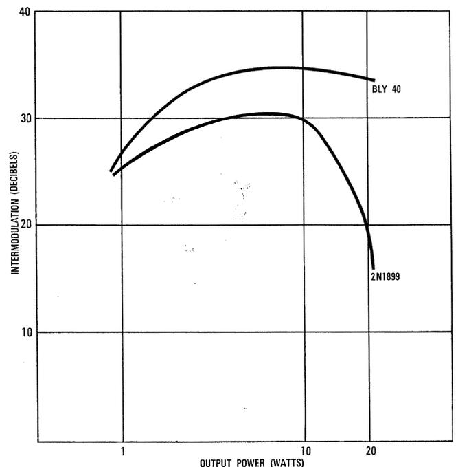
Figure 15 - Typical intermodulation curves plotted against output power for two transistors used in equipment. The CCIR 2-tone test was applied.
