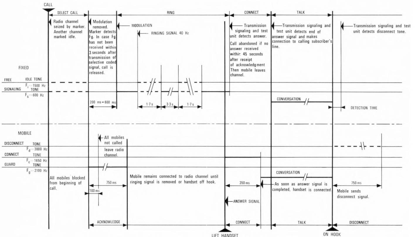
Figure 14 - Signaling sequence for a call from a fixed to a mobile subscriber.
