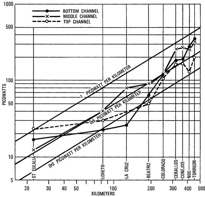
Figure 7 - Intermodulation noise, Chihuahua—Torreón, 446.5 kilometers (277 miles), 1800-channel loading.
