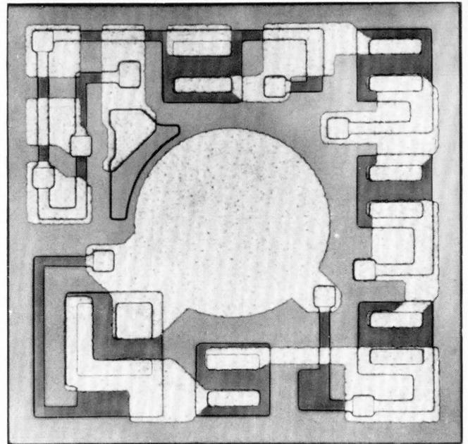
Geometry of the ZTK 33 zener diode that is well compensated for temperature coefficient of zener voltage output. The actual size is 0.5 by 0.5 millimeter (0.02 by 0.02 inch).
