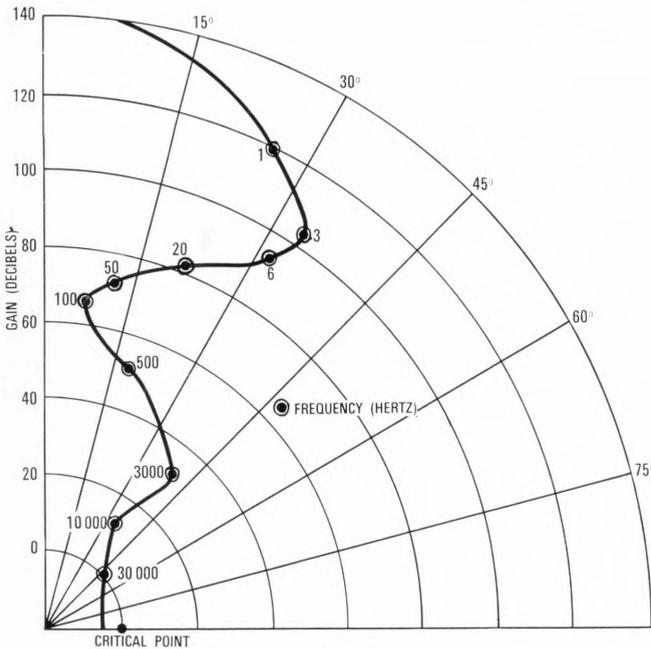
Figure 7 - Nyquist diagram for control loop.
