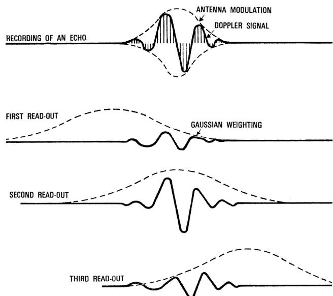
Figure 7 - Signal smoothing using multiplication by a Gaussian function.
