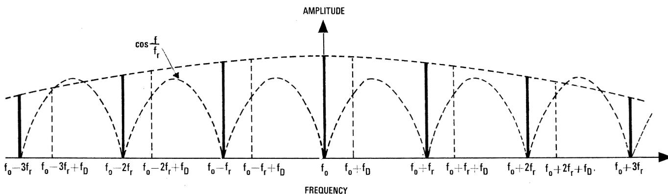
Figure 2 - Echo spectra for a fixed antenna. The solid lines are echoes from a fixed target and the vertical dotted lines are from a moving target.
