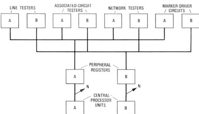
Figure 4 - The duplicated part of a 10C exchange.
