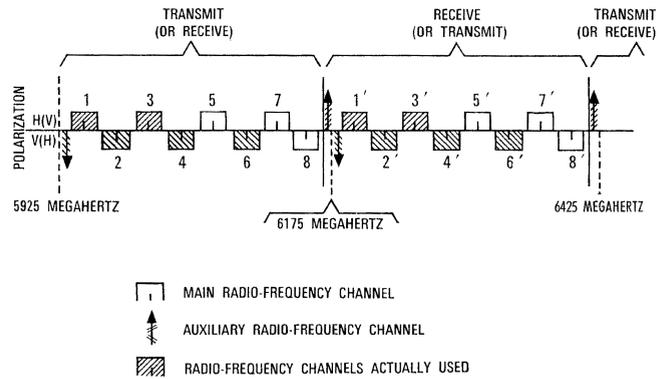
Figure 4 - Radio-frequency channel arrangement in the 6-gigahertz band for the Mexican radio-relay network. As many as 14 transmit and receive frequencies are accommodated on a single antenna, with a possible maximum of 20 frequencies.
