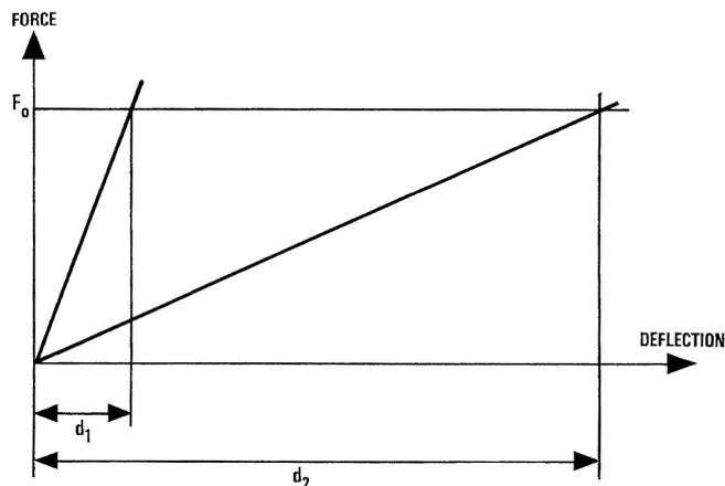
Figure 1 - Force versus deflection relationship for various types of springs.
