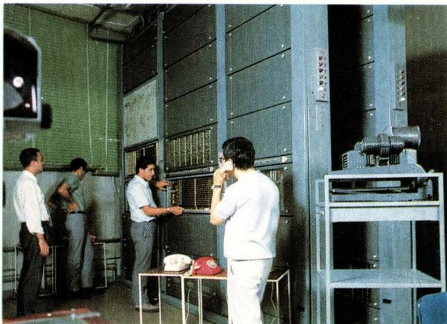
Figure 2 - The Pentaconta Switching System Trainer used for teaching engineers and technicians from the ITT system.
