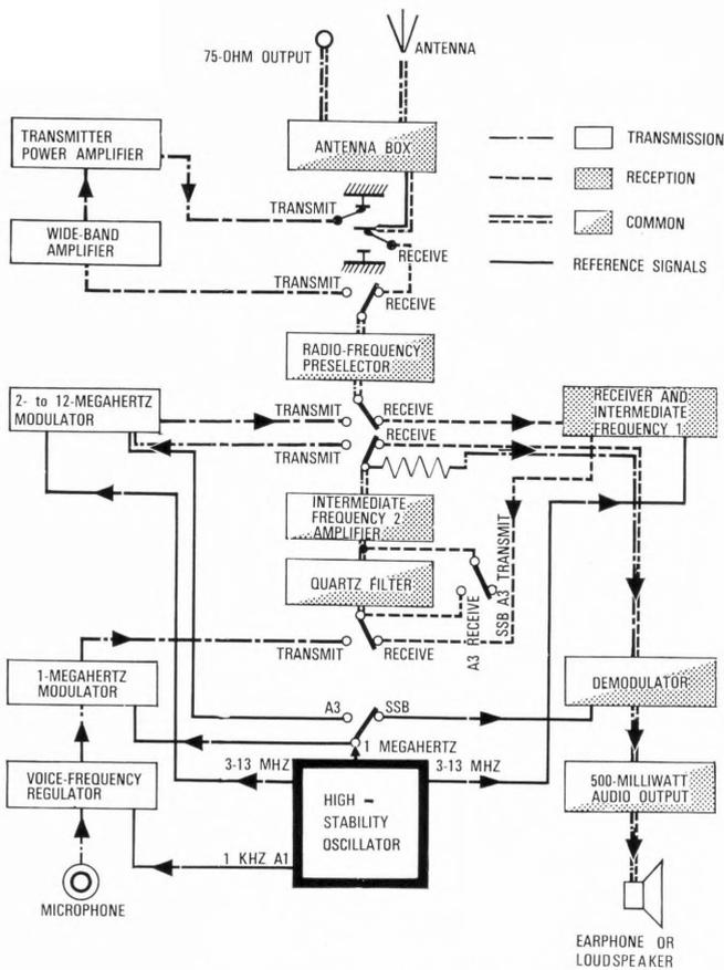
Figure 9 - TR-TM 4 block diagram. The oven for the high-stability oscillator and the transmitter power amplifier operate from a 24-volt source while all other units are fed 16 volts through a regulator.
