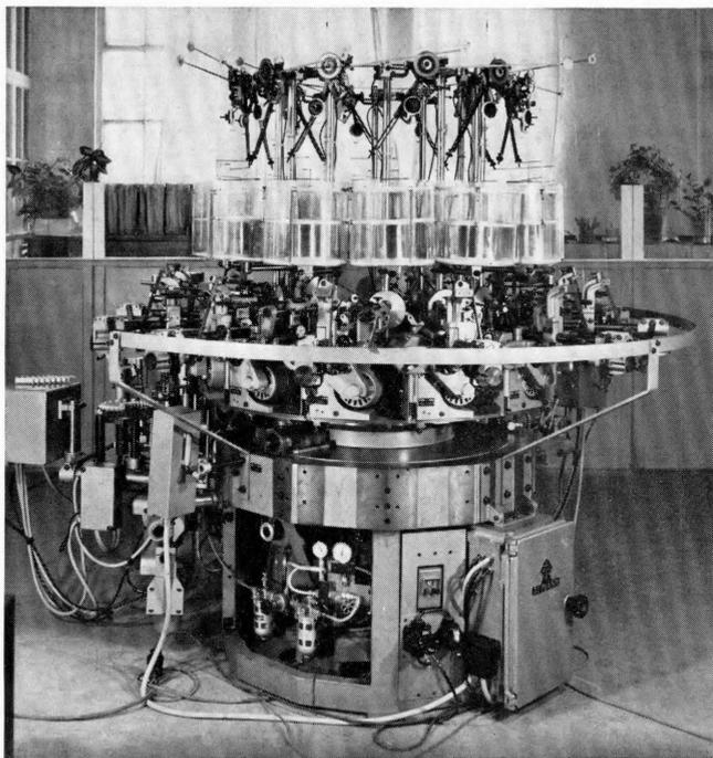
Automatic winding of relay coils.
