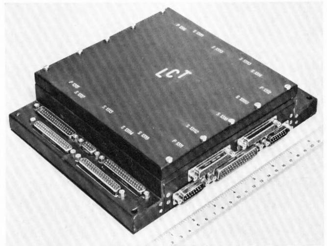
Checkout console (first type) of the housekeeping system of the *ESRO 1* satellite.
