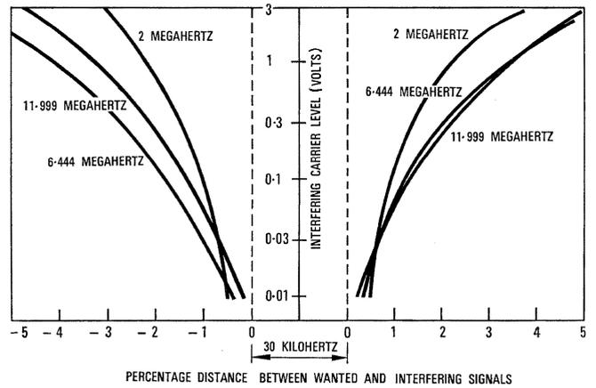
Figure 13 - Receiver desensitization limits.
