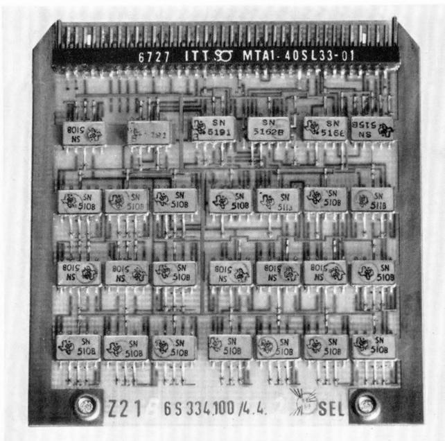
Figure 6 - Printed card of the plug-in type.
