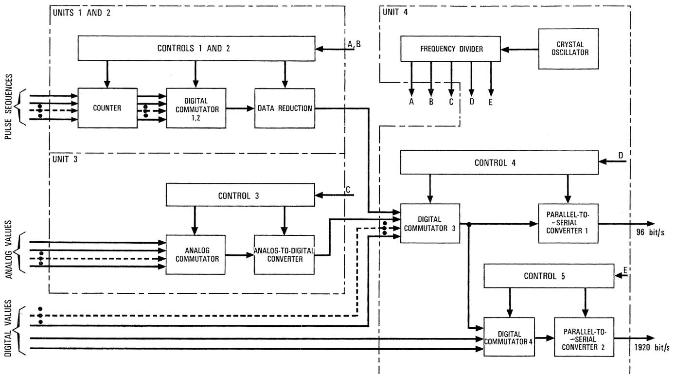
Figure 1 - Block diagram for *PCM* telemetry system *AZUR*.
