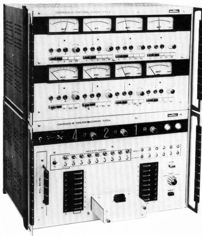
*TX 935 A* set for testing logic integrated circuits.
