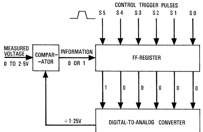
Figure 4 - Principle of analog-to-digital conversion.
