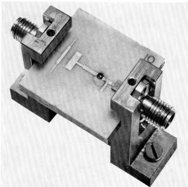
Figure 9 - Photograph of X-band microstrip oscillator circuit mounted in bench test jig.
