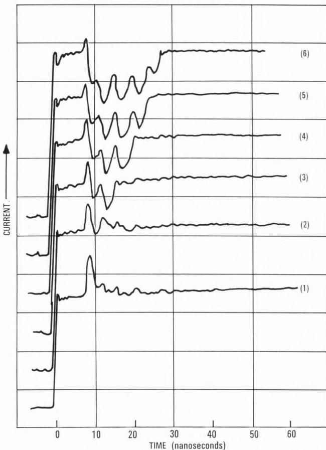
Figure 14 - Current waveforms for analog-to-digital converter with bias voltage increasing from traces 1 to 6.
