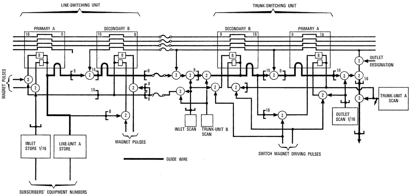
Figure 8 - The path-search and connection equipment.
