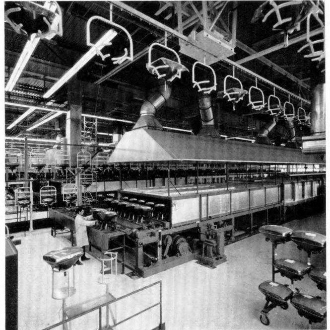
Sintering furnace in the Esslingen color-picture tube factory.
