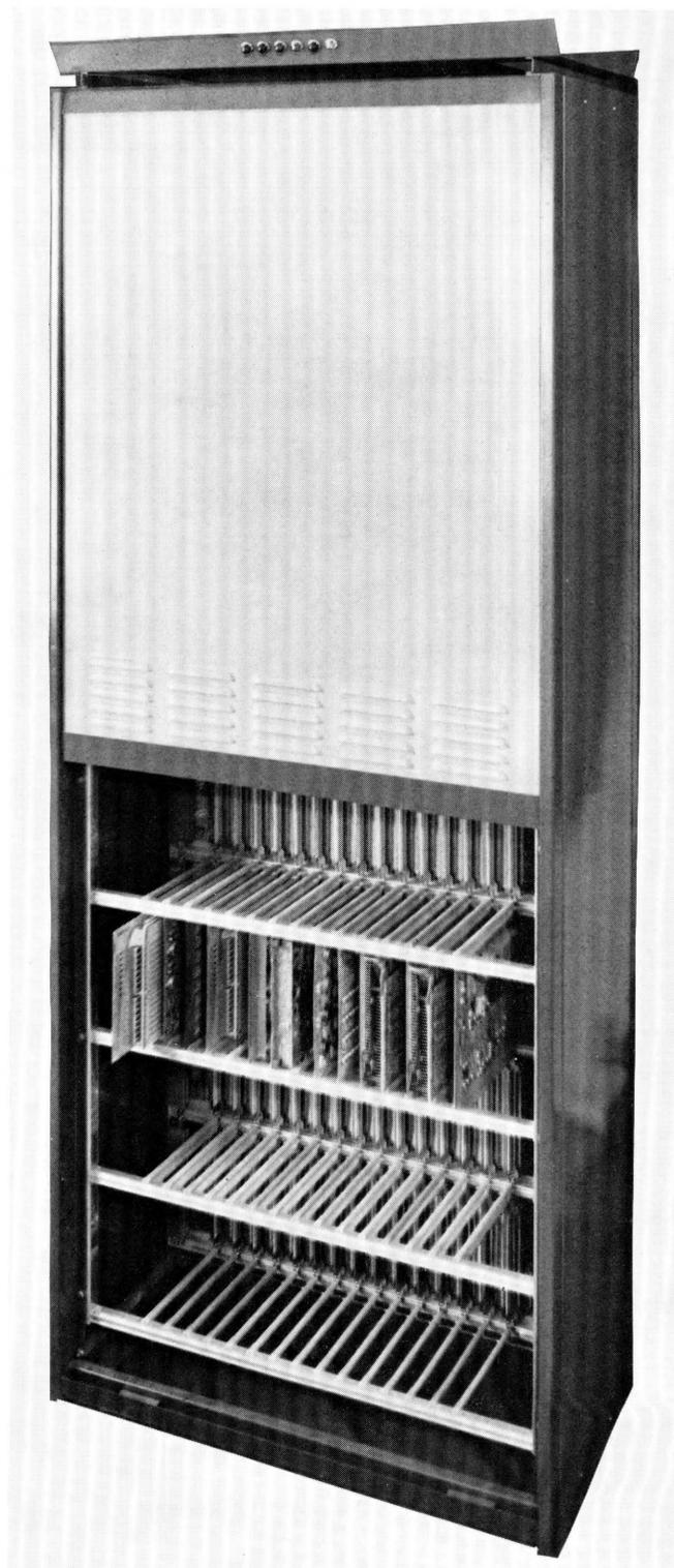
Figure 9 - A complete 11B rack constructed in accordance with ISEP standards.
