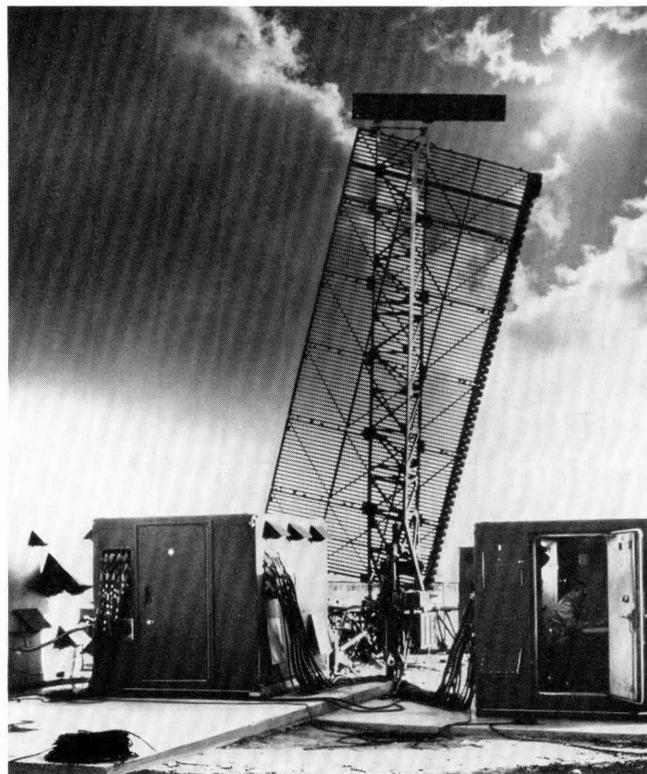
*AN/TPS-32* provides target information in data form directly to a tactical data system.
