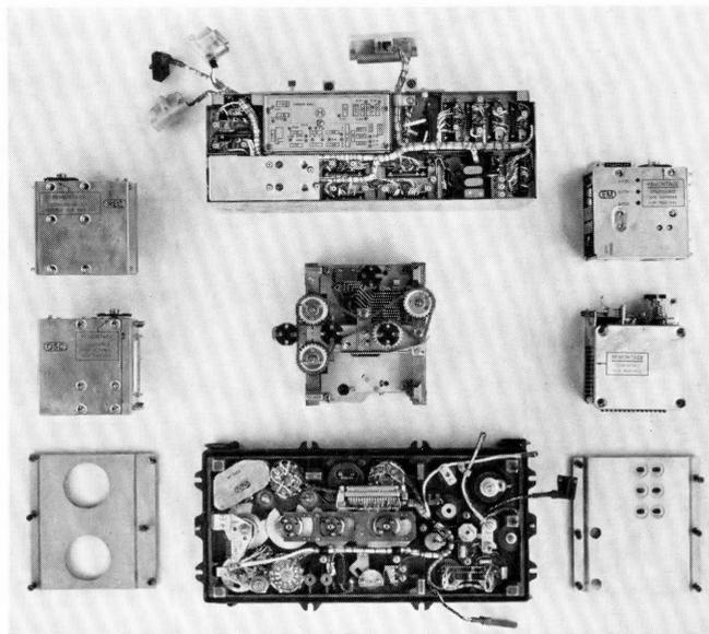
Figure 12 - Set exploded to show main units.
