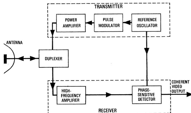
Figure 1 - Basic block diagram of a coherent pulsed radar.
