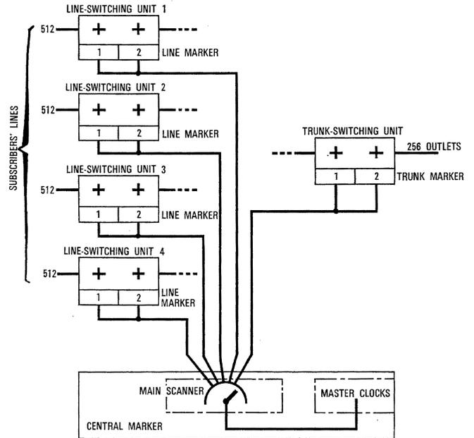
Figure 5 - Marking principle for a 4-stage exchange.
