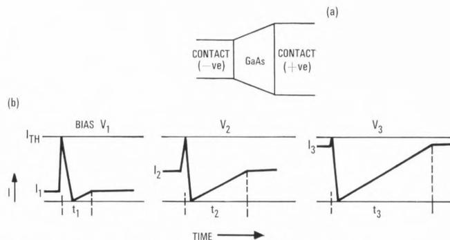
Figure 13 - The principle of analog conversion (that is, bias voltage to domain transit time) in a "wedge" shaped device in triggered mode.
