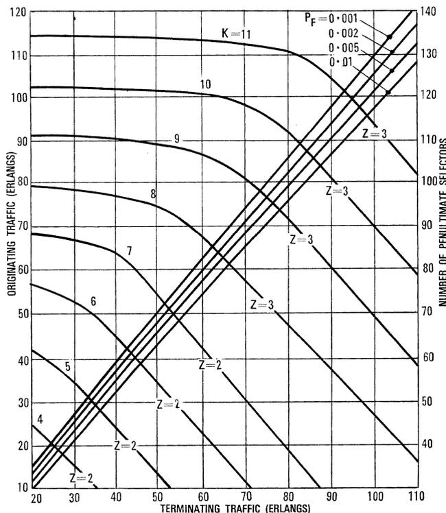
Figure 5 - Dimensioning of line-selection elements for loss probabilities in line selection and in preselection of 0.01
