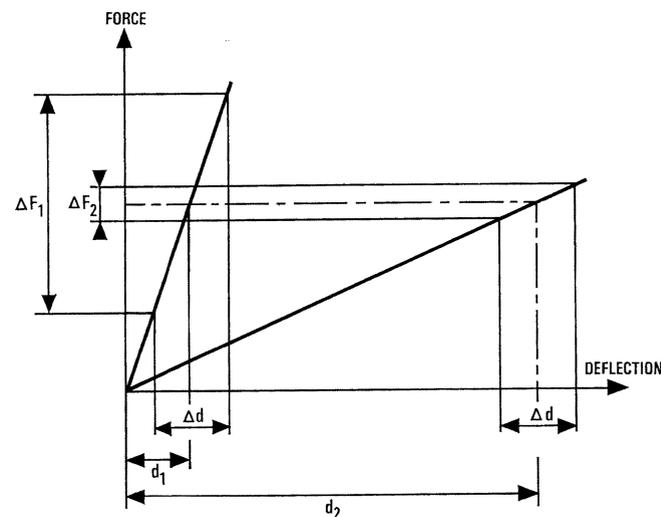
Figure 2 - Force spread versus deflection spread for various types of springs.
