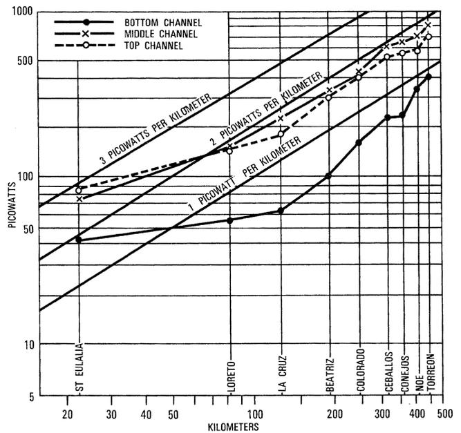
Figure 6 - Total noise, Chihuahua—Torreón, 446.5 kilometers (277 miles), 1800-channel loading.
