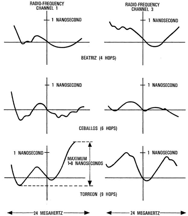
Figure 8 - Time-delay distortion, Chihuahua—Torreón.
