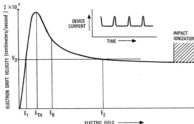
Figure 1 - Transferred-electron characteristic for gallium arsenide illustrating domain field distribution and, inset, the device current.
