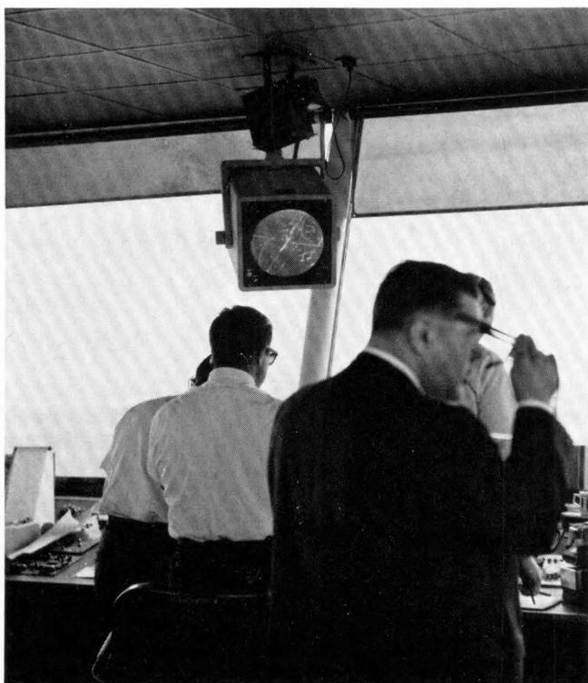
*BRITE* radar display in an airport control tower can be viewed without the conventional hood or other means of reducing the high ambient light.
