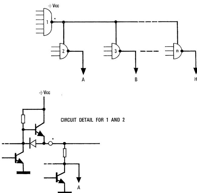
Figure 5 - *NAND*-configuration which reduces the number of integrated circuits.
