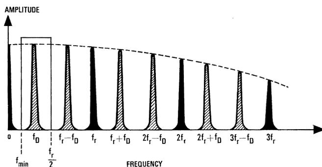
Figure 3 - Echo spectrum for a rotating antenna.
