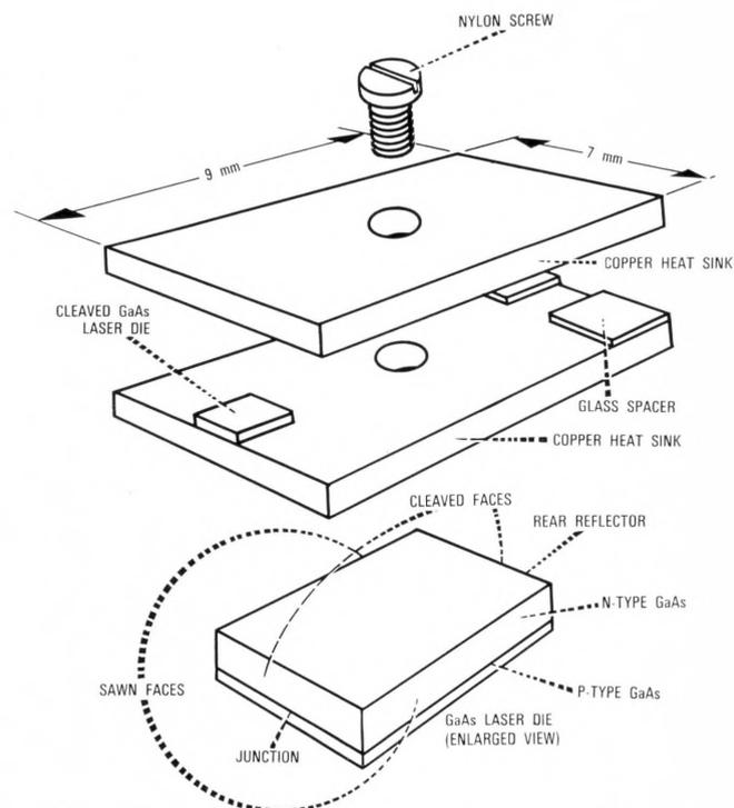
The gallium-arsenide laser junction at the bottom is clamped between the heat-sink plates at the top.
