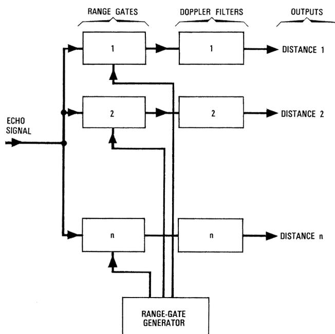
Figure 4 - Principle of echo detection with fixed range gates.
