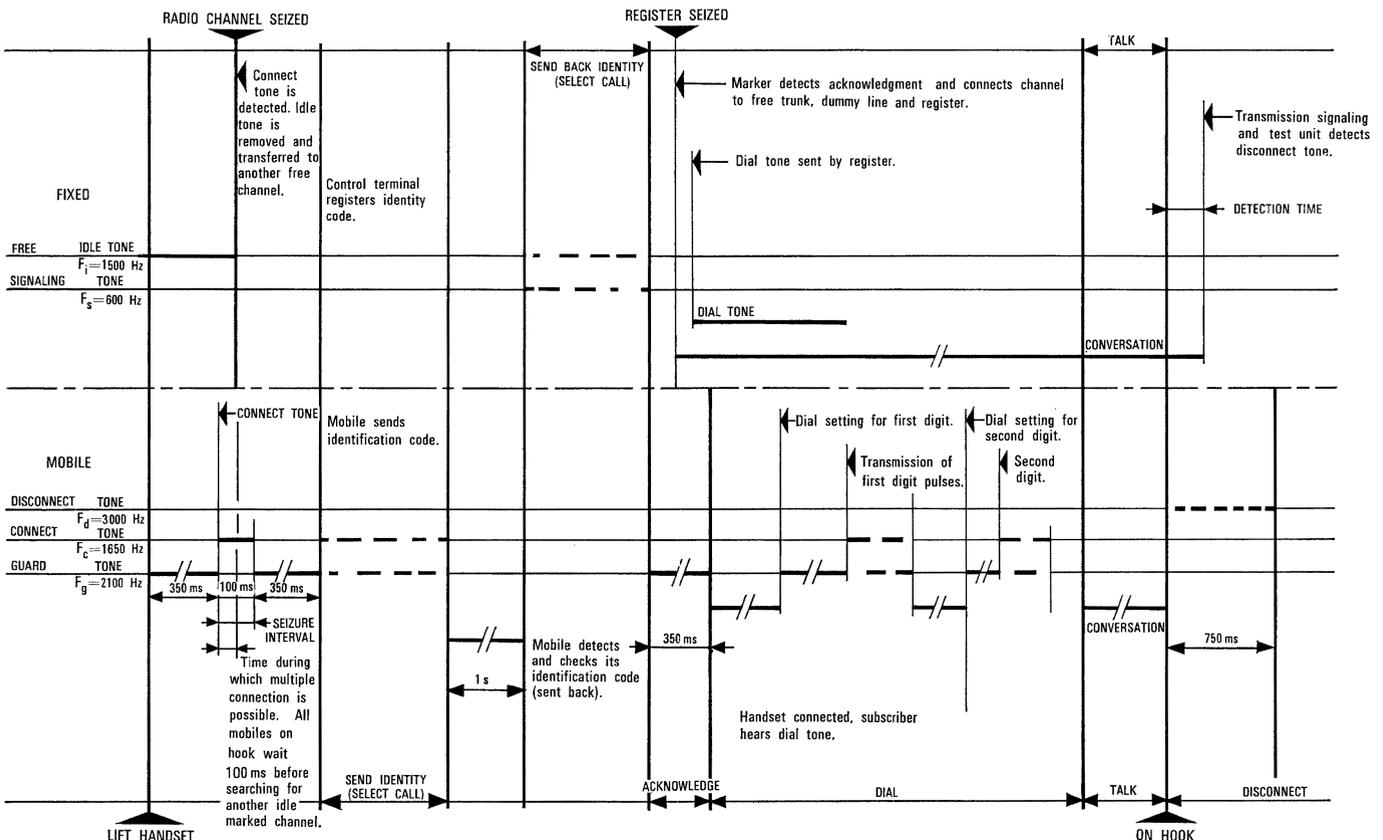
Figure 15 - Signaling sequence for a call from a mobile to a fixed subscriber.
