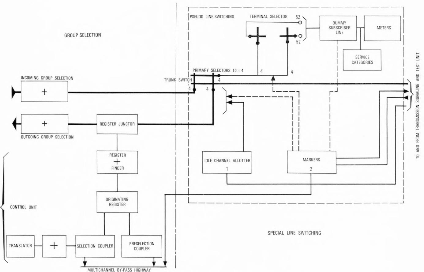
Figure 11 - Control and switching equipment.
