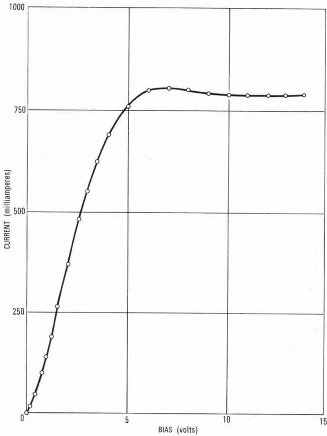
Figure 6 - Typical bias current *versus* voltage characteristic for a Gunn-effect oscillator.
