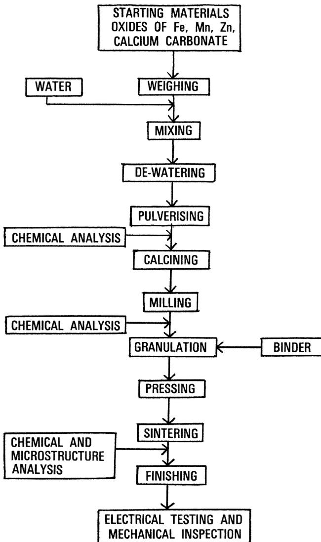
Figure 1 - Flow diagram showing the principal stages in the manufacture of manganese-zinc ferrite.
