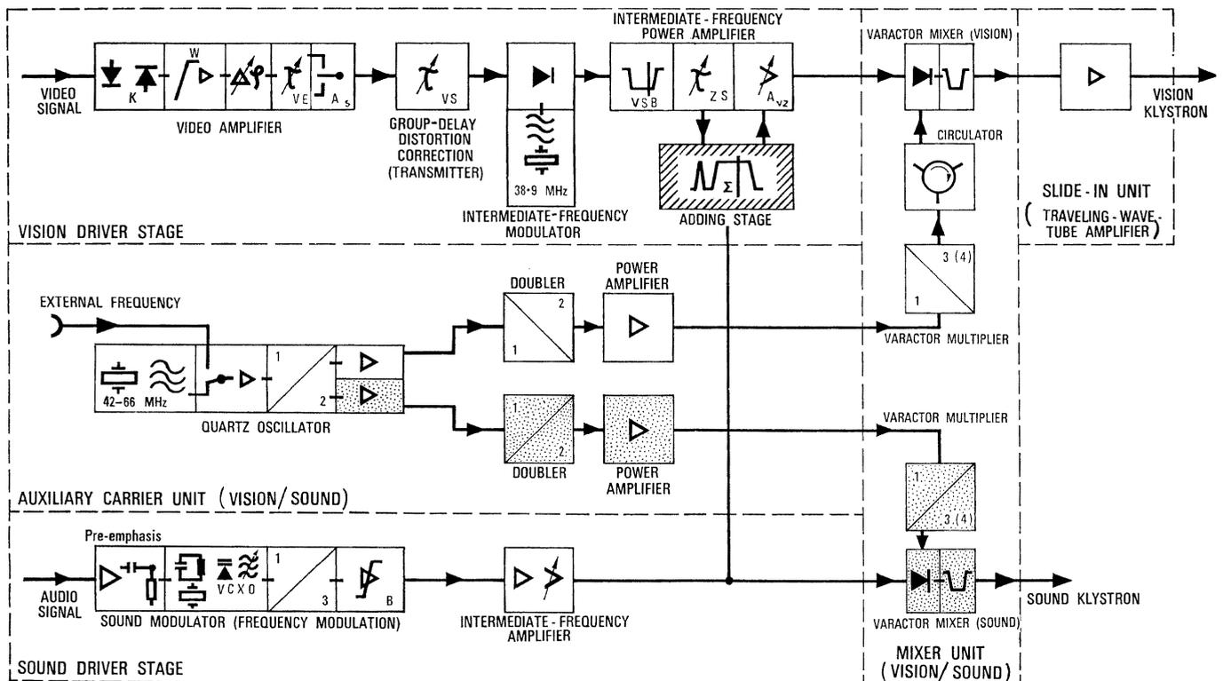
Figure 3 - Block diagram of the vision/sound driver stage.
