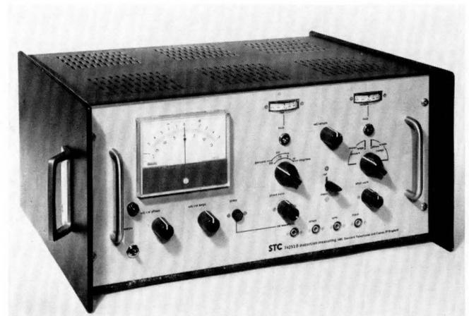
Test equipment for making differential measurements of phase and amplitude of color-television links.
