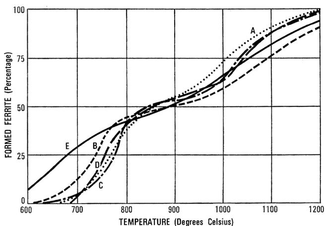
Figure 5 - Influence of iron oxide on the kinetics of formation for mixed manganese-zinc ferrites.
