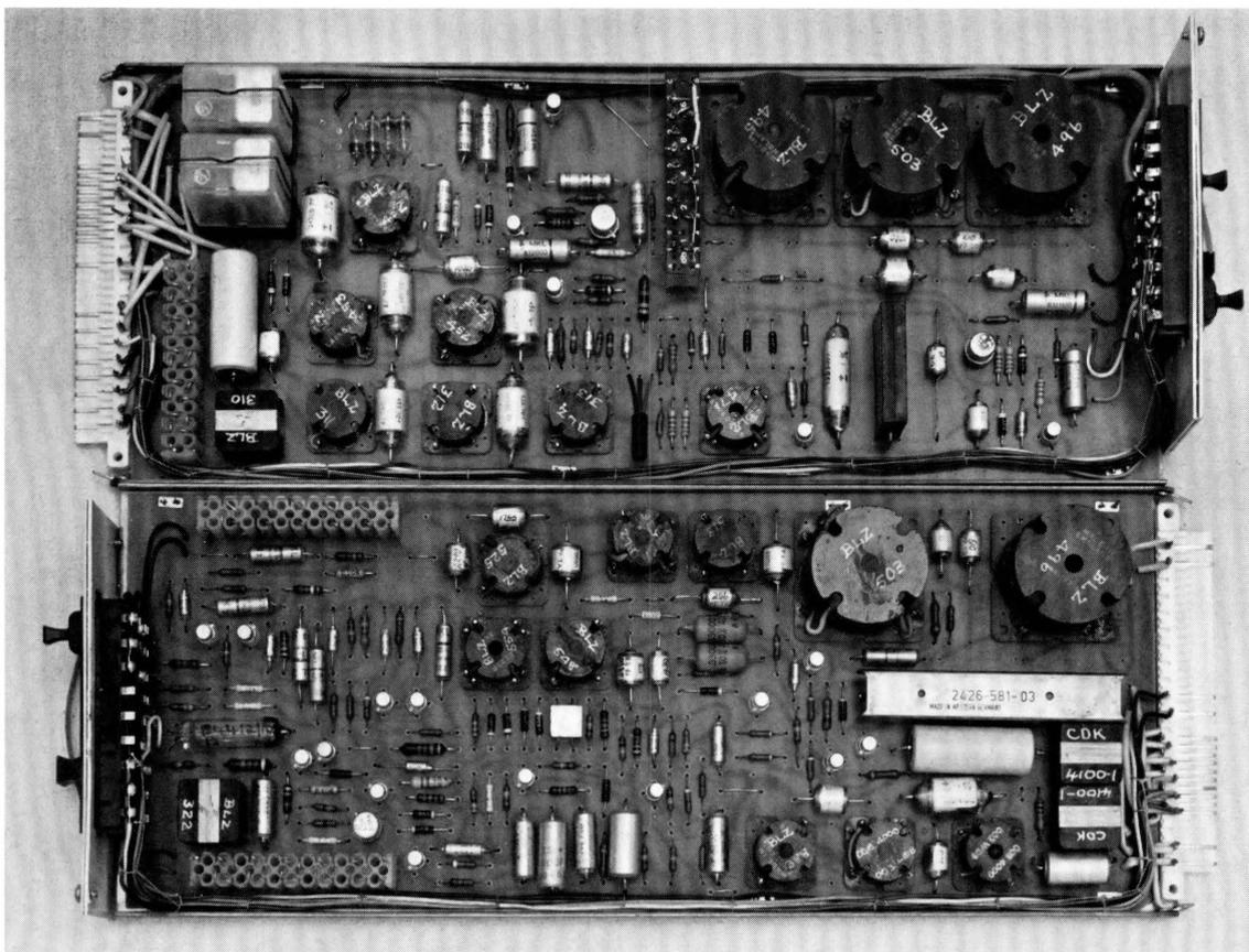
ference with shaped white-noise loading is better than 300 microvolts psophometrically weighted at zero relative level whilst send-to-receive within-channel crosstalk has a worst value of  $-45$  dBm0. All results refer to uncompandored channels.
