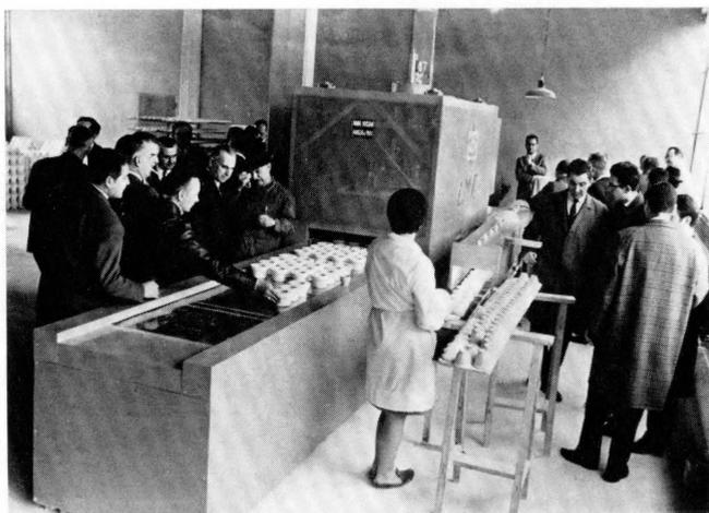
Microwave oven for rapid predrying of china dishes after molding.
