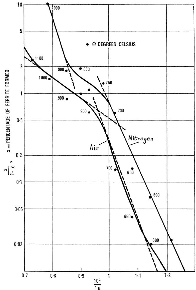
Figure 2 - Arrhenius' relationship between temperature and formed ferrite.
