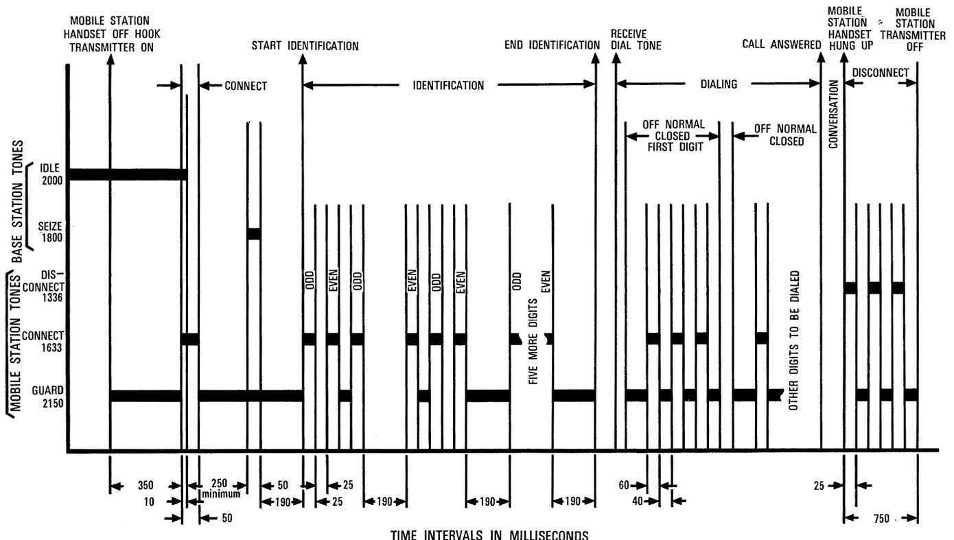
Figure 1 - Sequence of tone signals from mobile subscriber set to the base station.
