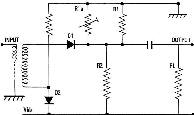
Figure 4 - Square-law detector with a suitably modified characteristic to reduce forward-voltage drop and maintain correct characteristic over working temperature range.
