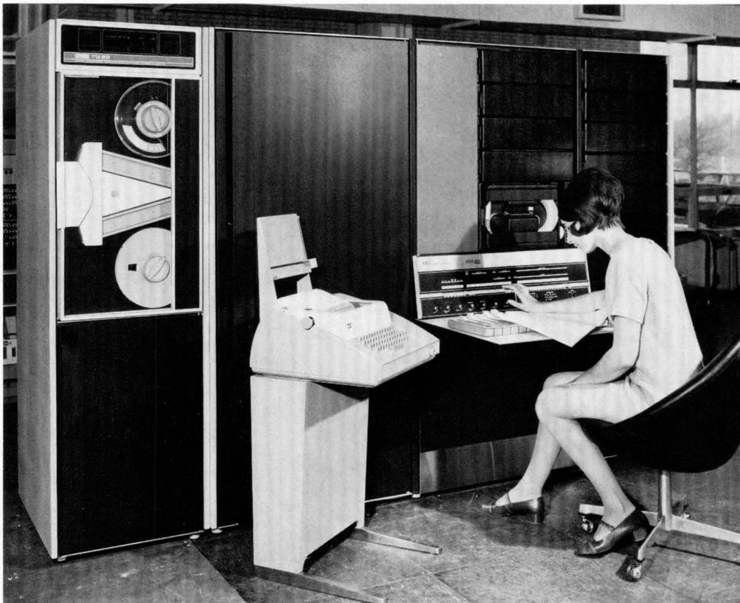
Control processor for *ADX* data switching equipment.
