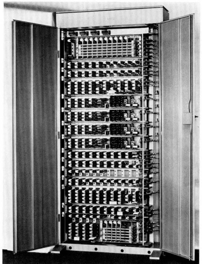
Figure 3 - Cabinet-mounted exchange extensible from 20 to 100 extensions with up to six cord circuits and complete facility program.
