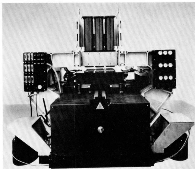
This machine for making masks for integrated circuits is operated from a computer. The  $XY$  coordinate positions of a stone table which carries the photographic plate that becomes the mask are measured by interferometers using laser beams.
