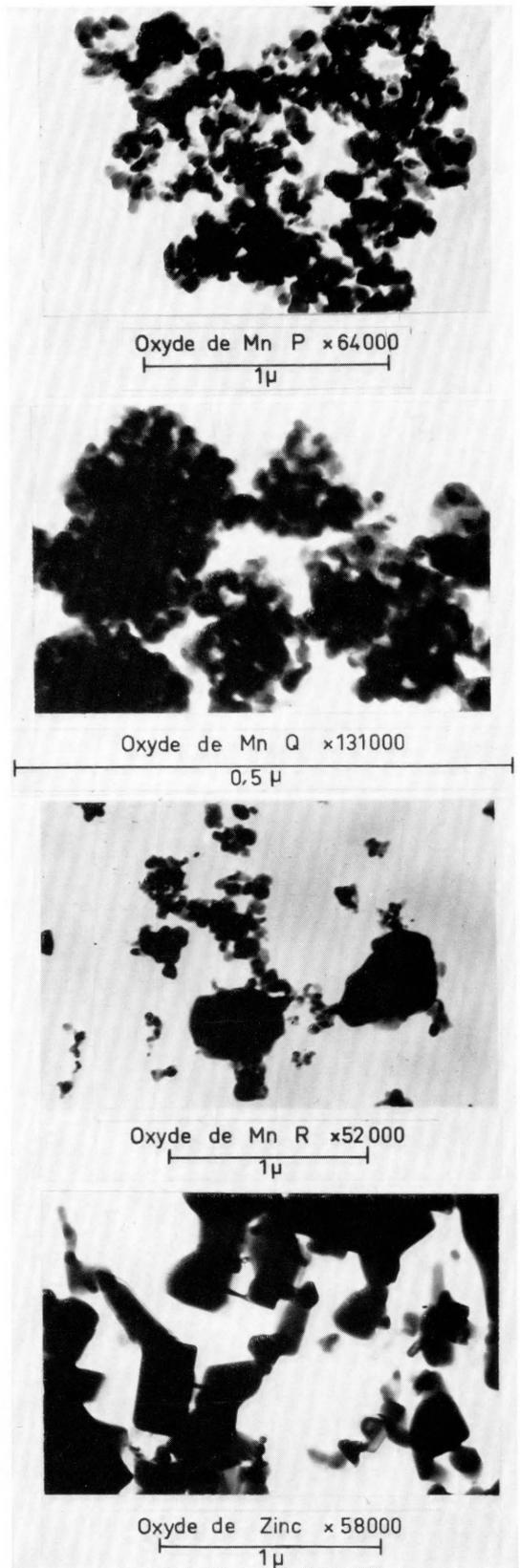
Figure 4 - Electron-microscope photographs showing manganese oxides, P, Q, and R (see Table 4), and zinc oxide.
