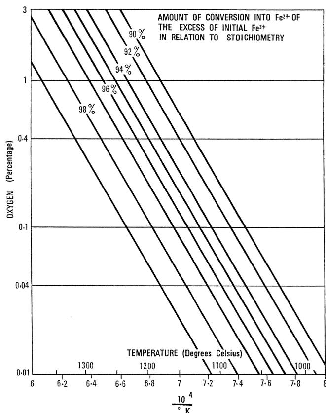
Figure 8 - Atmosphere/temperature curves showing the phase rule according to E. D. Macklen [21].
