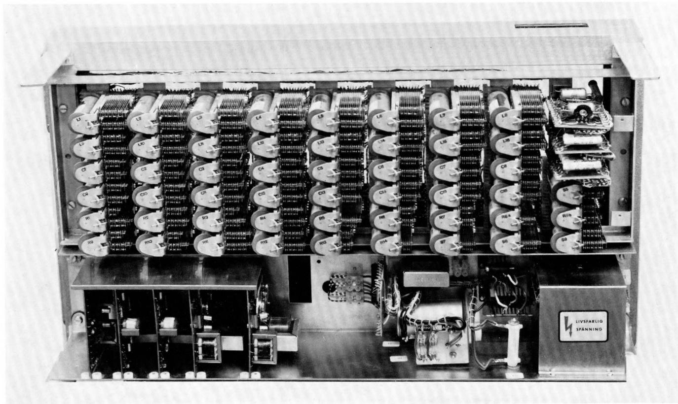
Figure 1 - A 16-line wall-mounted exchange with one cord circuit. Executive priority for one extension is included as a standard feature.
