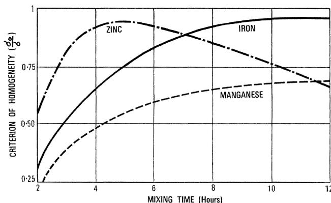
Figure 7 - Homogeneity as a function of time.
