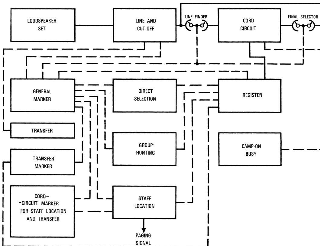
Figure 10 - Traffic lay-out 20-100 line exchange.
