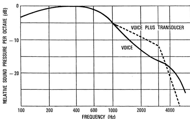
Figure 1 - Speech spectrum over a relatively long time period.
