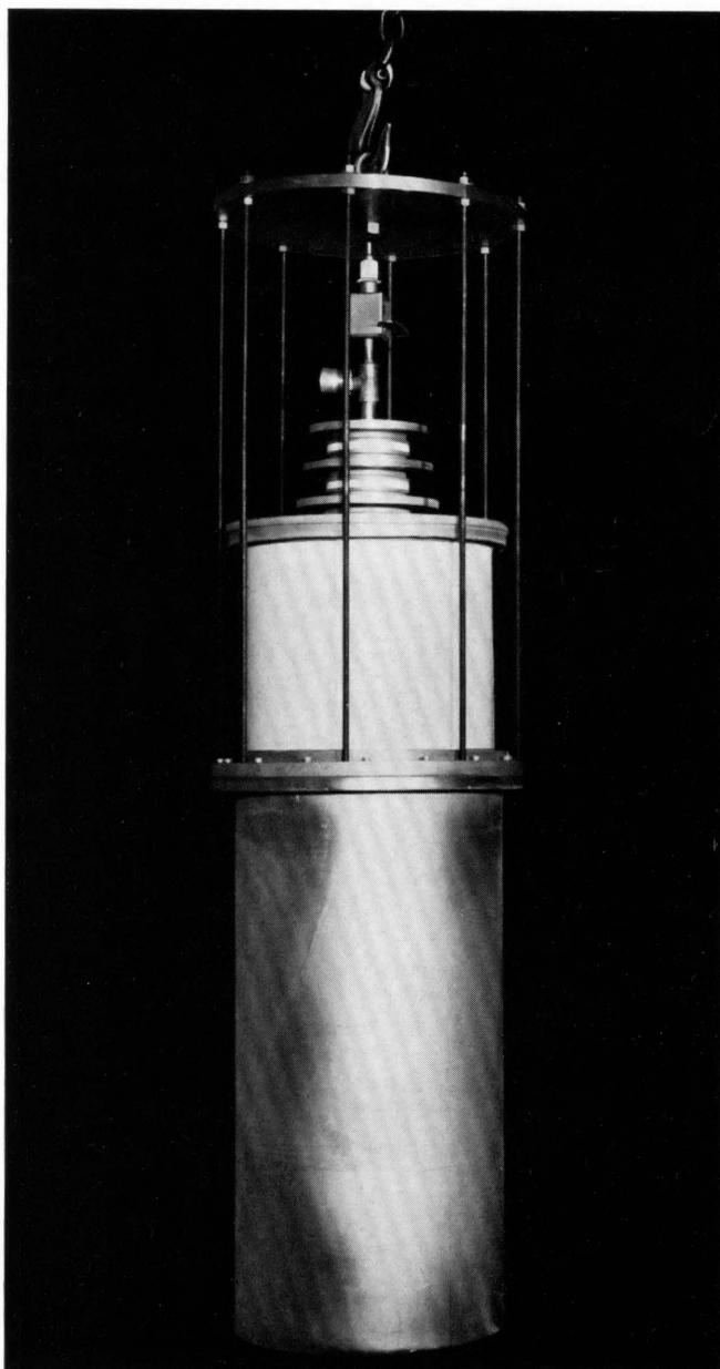
This powerful triode vacuum tube can dissipate 390 kilowatts in producing 90-megawatt pulses.
