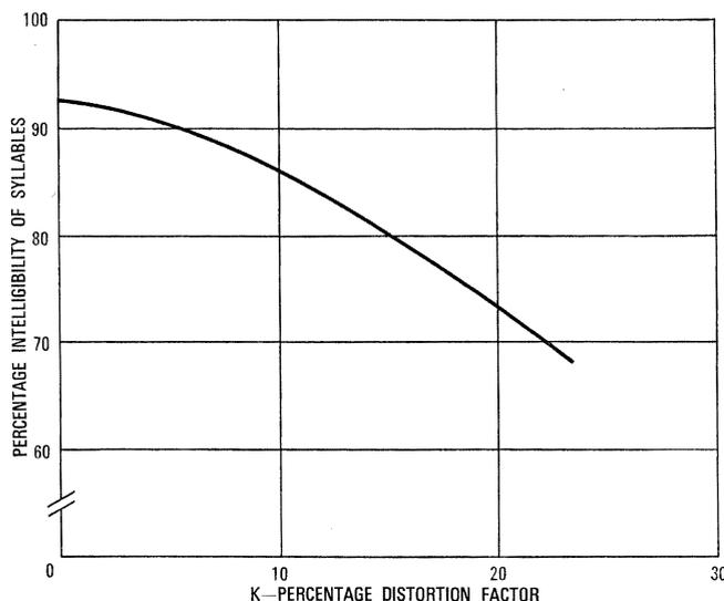
Figure 4 - Decrease of intelligibility with distortion factor *k* (according to K. Braun). The reduction of intelligibility at point *k* = 0 is caused by measuring equipment.
