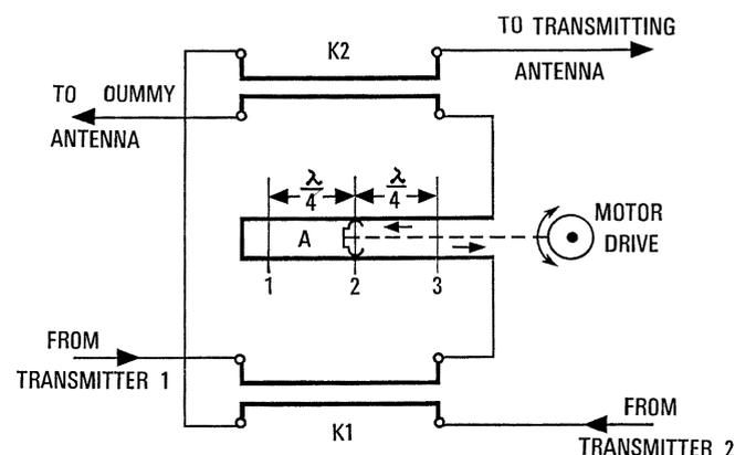
Figure 6 - Schematic of parallel transmitter operation.
