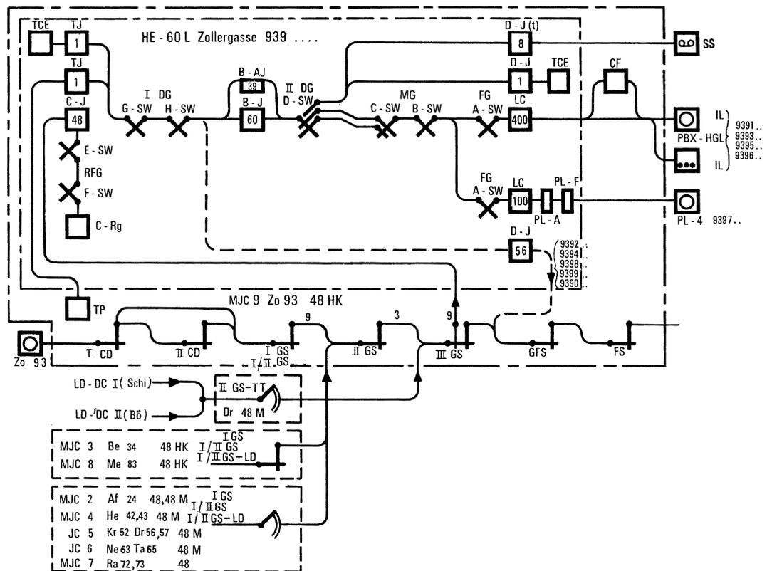
Figure 5 - System HE-60 L, Vienna-Zöllergasse. Incoming traffic (without internal traffic).
