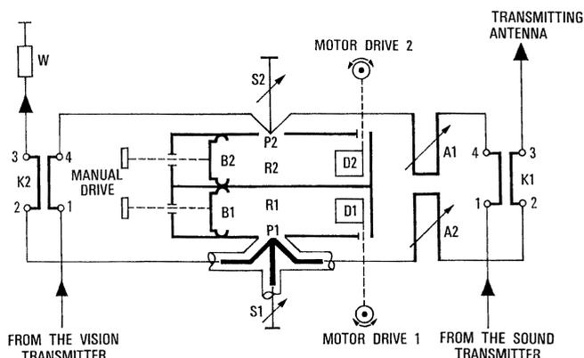
Figure 5 - Schematic of vision/sound combining unit.
