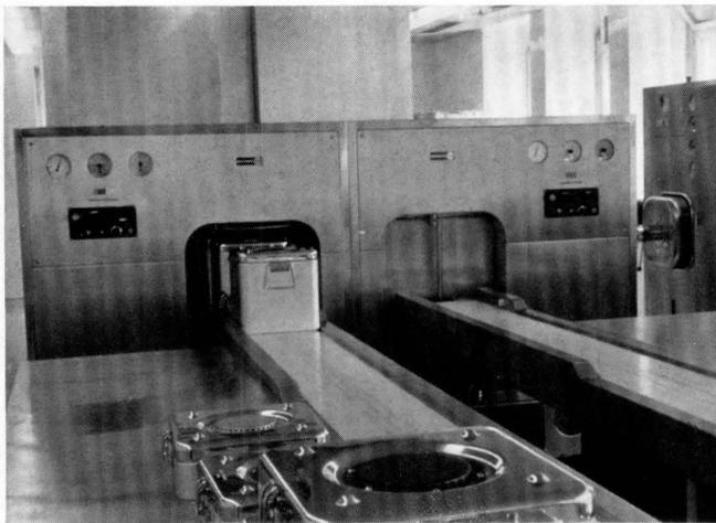
Conveyor system for moving containers of material into sterilizers.
