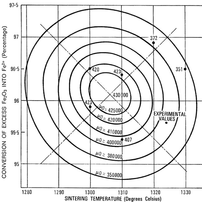
Figure 9 - Iso- $\mu Q$  curves for various sintering temperatures.
