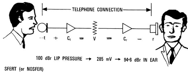
Figure 5 - Analogy of telephone circuit and SFERT.
