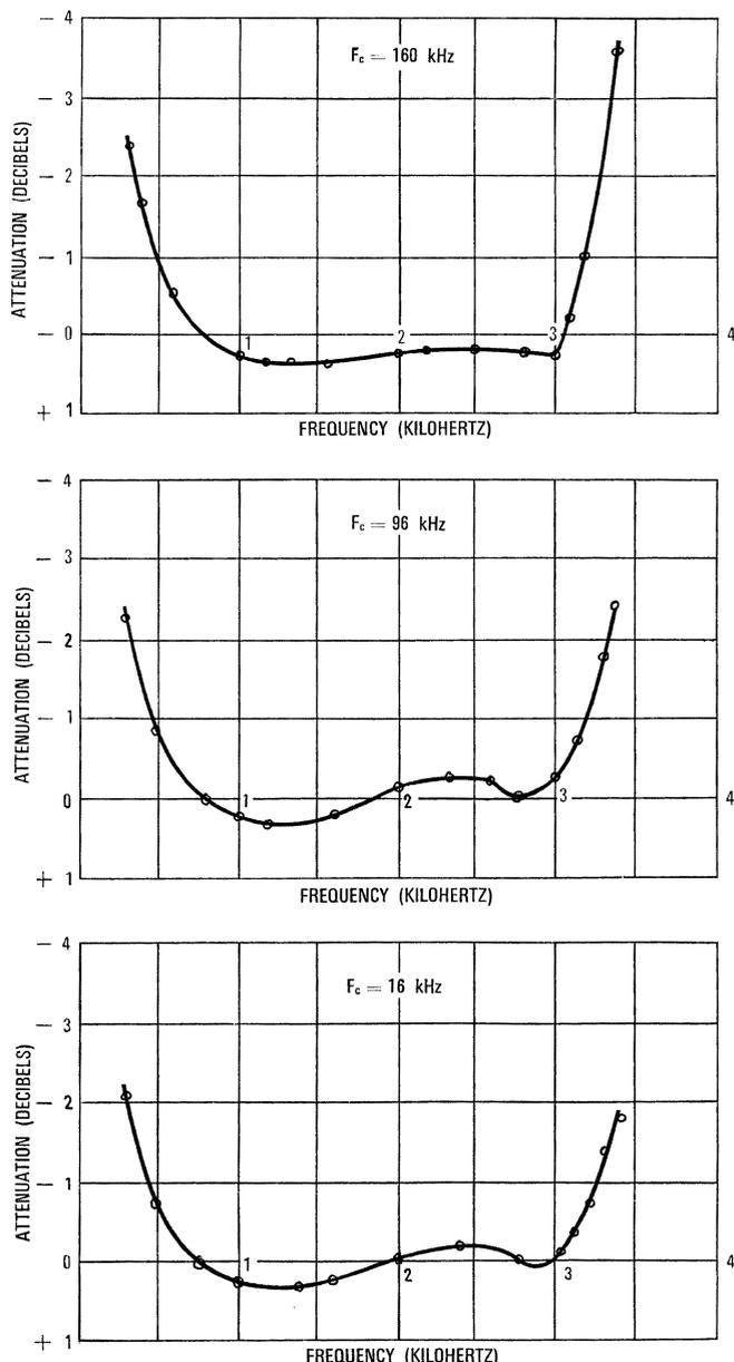
Figure 6 - Overall frequency-attenuation characteristic obtained in a back-to-back test for bottom, middle-range, and top channels.
