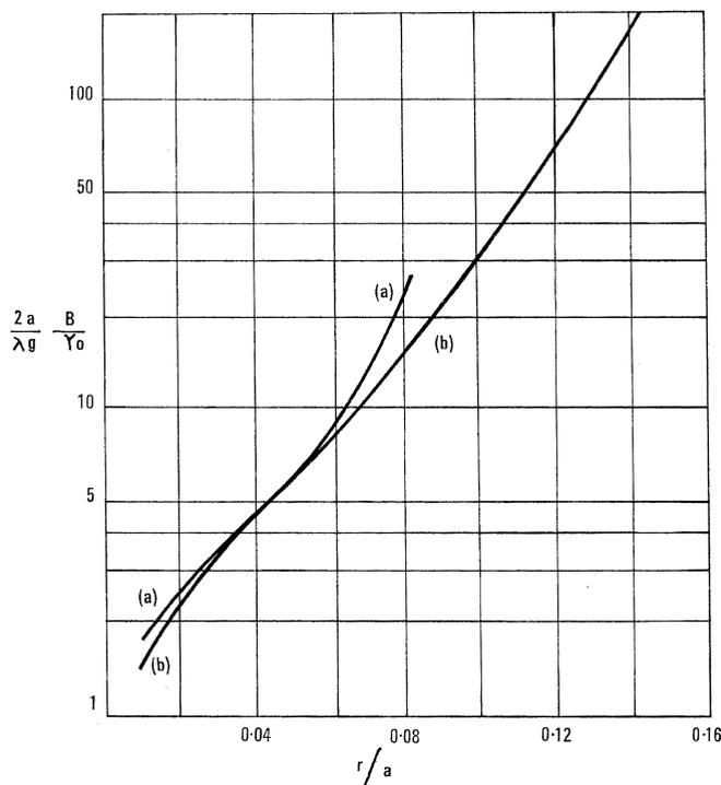
Figure 3 - Normalized susceptance of post doublets for  $\lambda_g = 2a$  and  $d = 1/2 a$ , (a) from Gruenberg's formula and (b) from (9).
