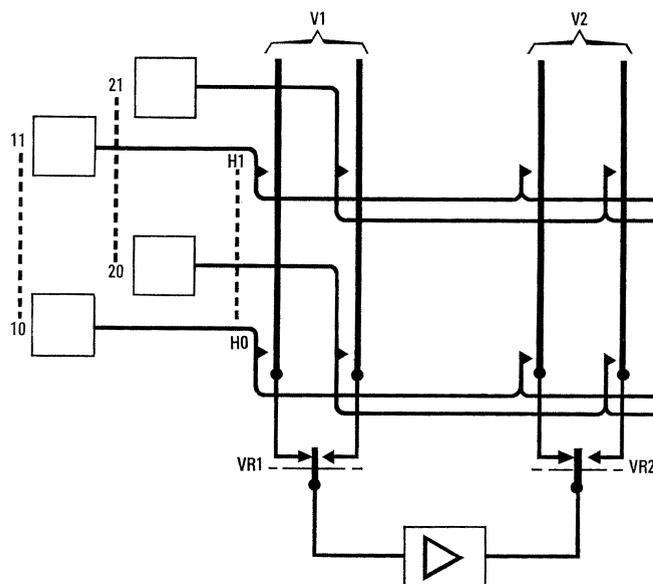
Figure 11 - Use of verticals in the crossbar switch unit.
