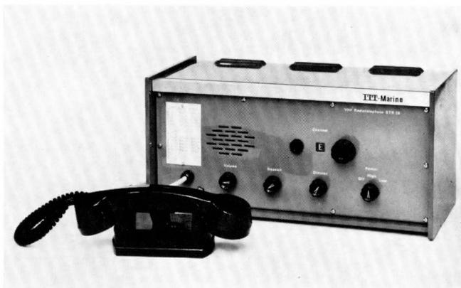
Marine very-high-frequency radiotelephone transceiver.
