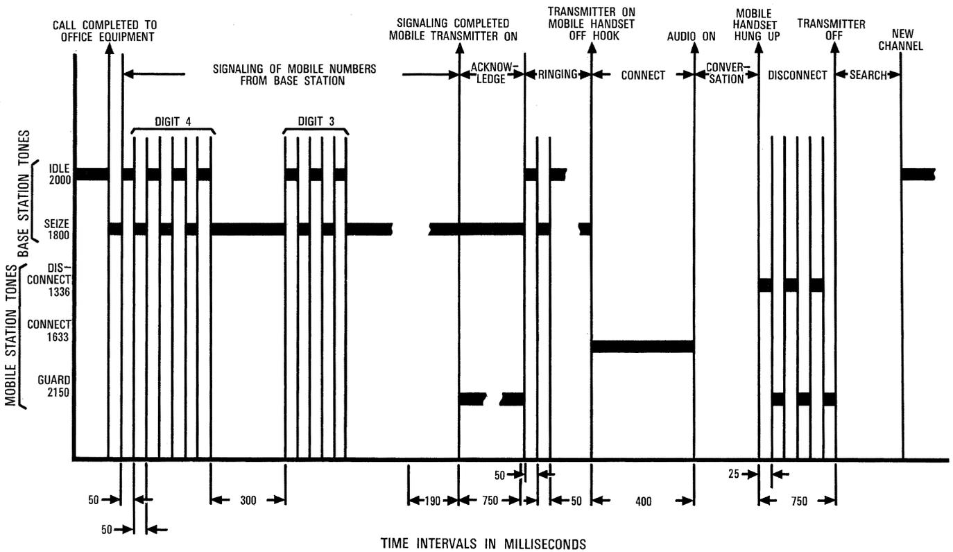
Figure 2 - Sequence of tone signals from base station to mobile subscriber set.
