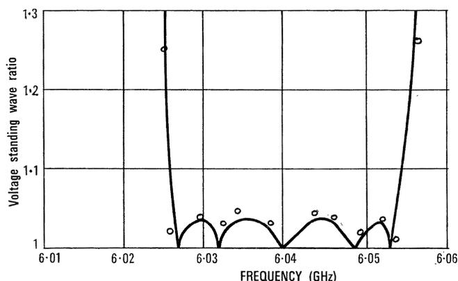
Figure 6 - Measured and calculated voltage standing wave ratio of filter (continuous curve is calculated voltage standing wave ratio).
