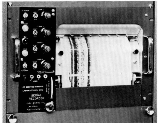
Paper recording using electrolytic marking for four channels.
