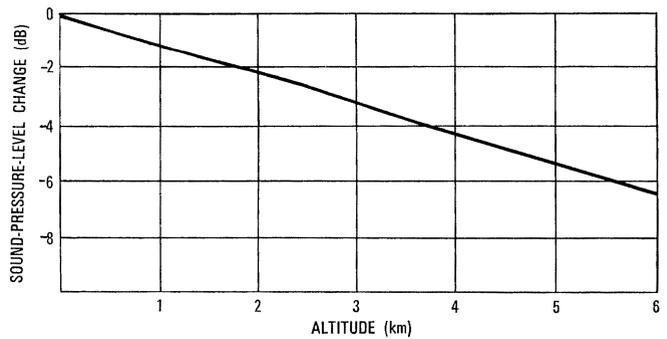
Figure 6 - Change in sound pressure level with altitude.
