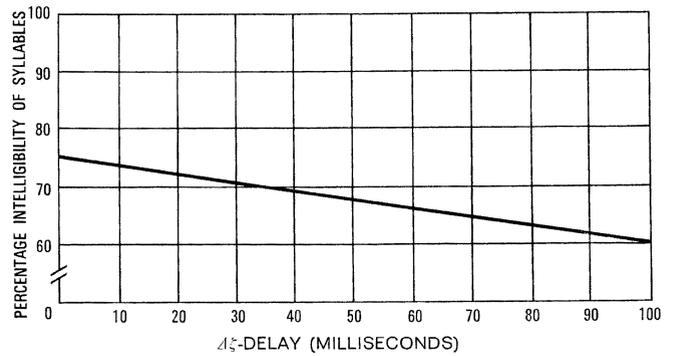
Figure 2 - Decrease in intelligibility with delay distortion (according to Lüschen, Küpfmüller). The reduction of intelligibility at point  $\Delta\tau = 0$  is caused by measuring equipment.
