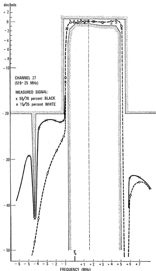
Figure 7 - Amplitude characteristic of sideband frequencies of a 10-kilowatt transmitter.
