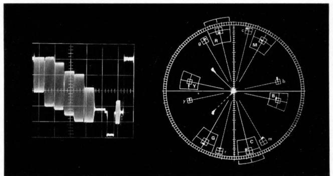
Figure 8 - Composite video with chrominance signal at the transmitter input.
