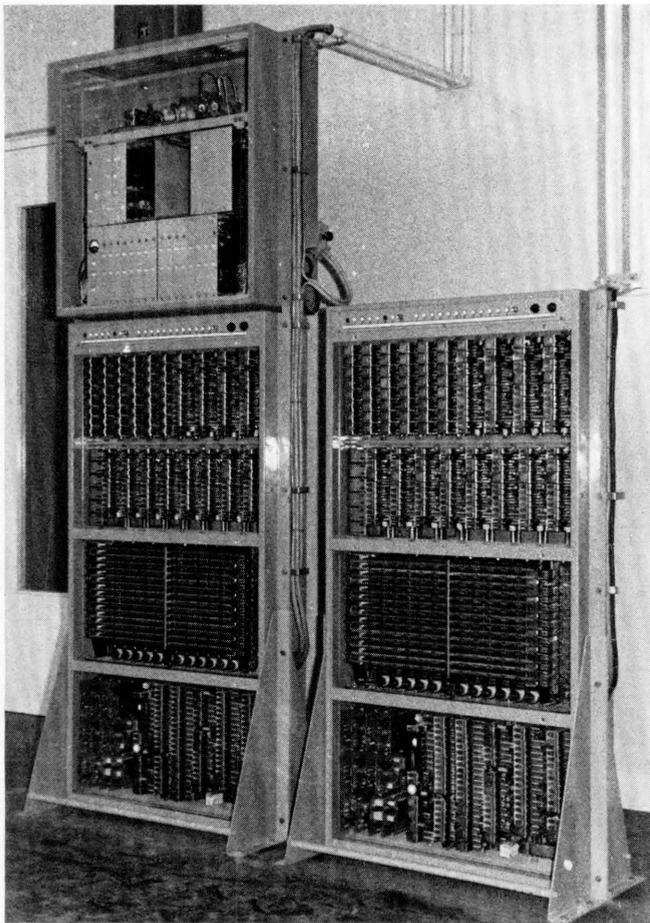
The two Pentaconta *CM 12* concentrators installed in the Paris regional telephone network.
