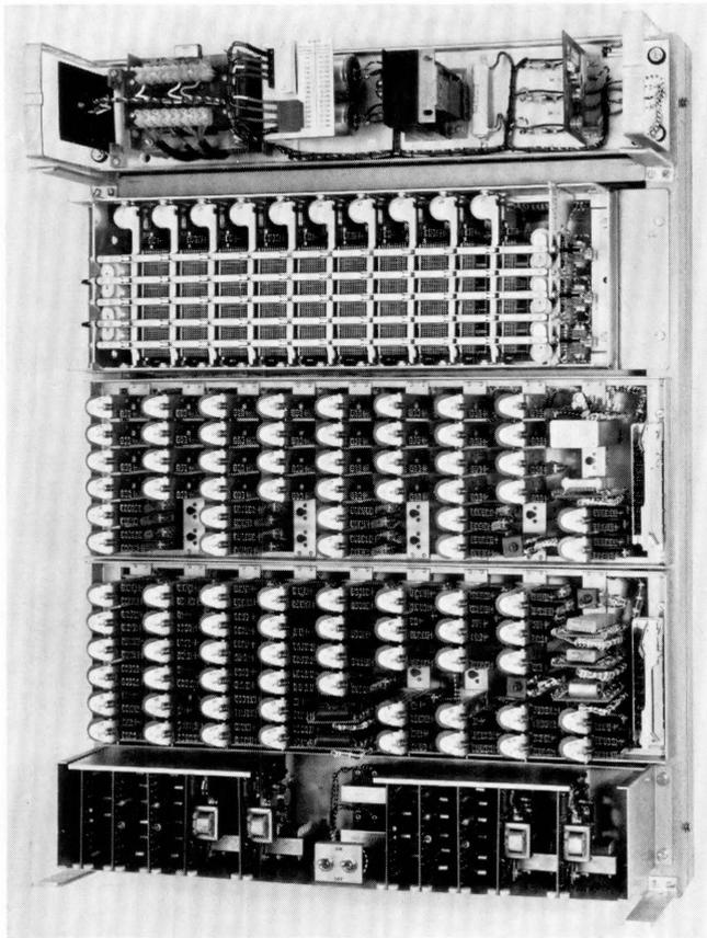
Figure 2 - A 32-line wall-mounted exchange with two cord circuits. Direct selection to 10 extensions and executive priority for one extension are included as standard features.
