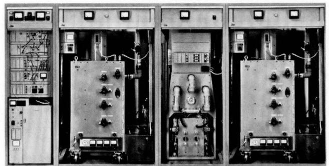
Figure 2 - The 40,8-kilowatt television transmitter (front row only — from left to right): vision/sound driver stage, klystron vision amplifier, combining unit, and klystron sound amplifier.
