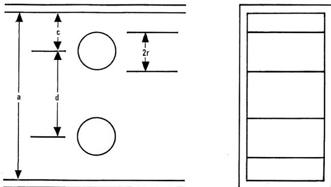
Figure 1 - Waveguide post doublets.
