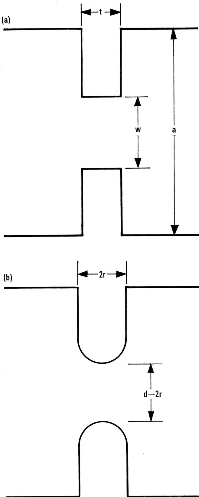
Figure 2 - Thick irises equivalent to a post doublet.
