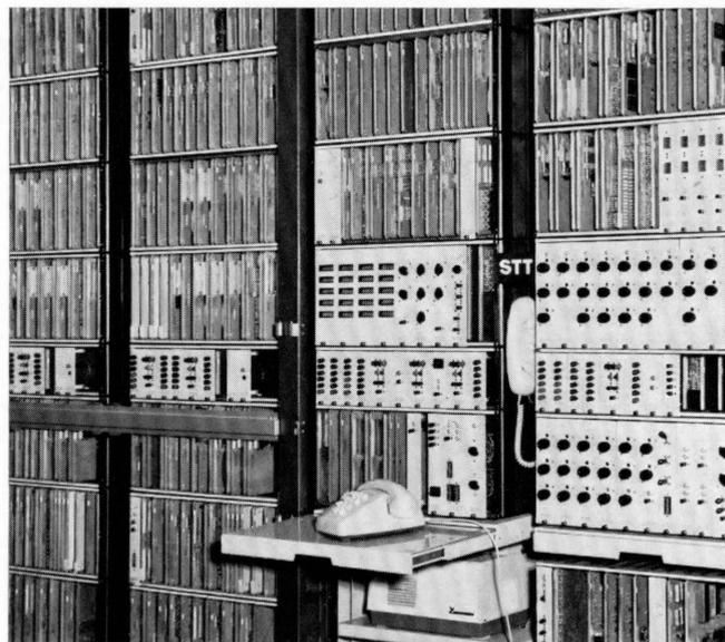
Figure 2 - Partial view of the quasi-electronic trial office; lower left, abbreviated-dialing translator units; push-button set.
