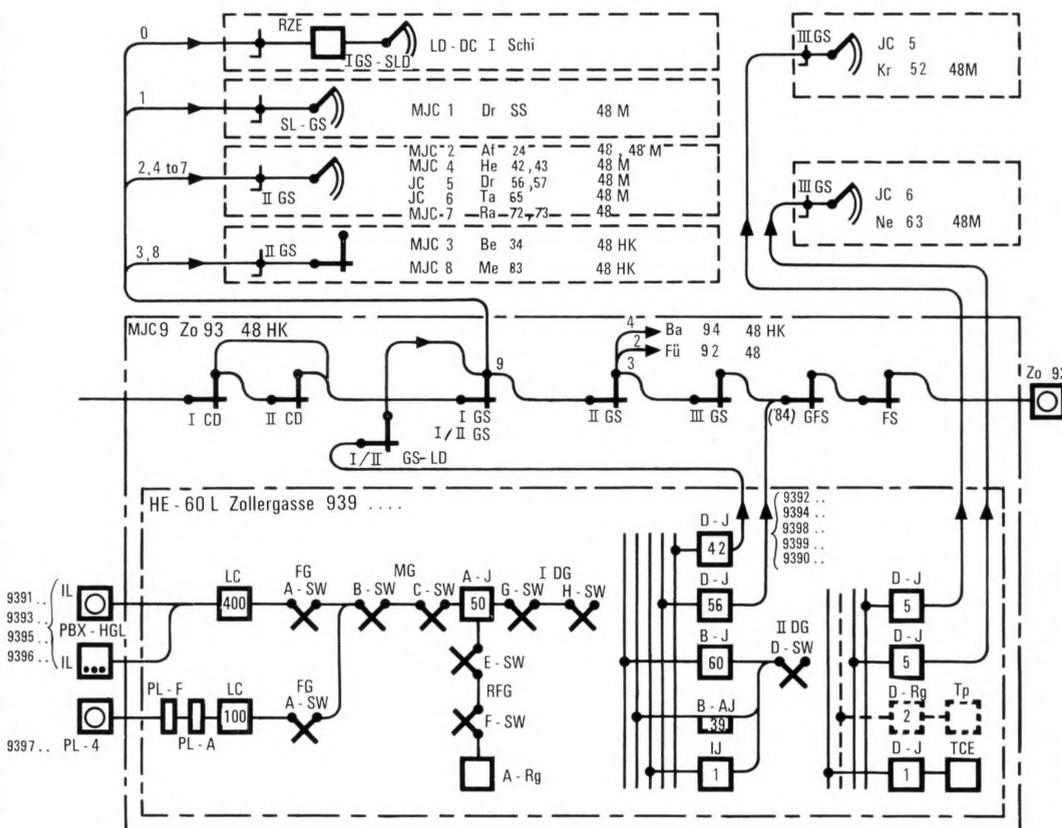
Figure 4 - System HE-60 L, Vienna-Zollergasse. Outgoing traffic (without internal traffic).
