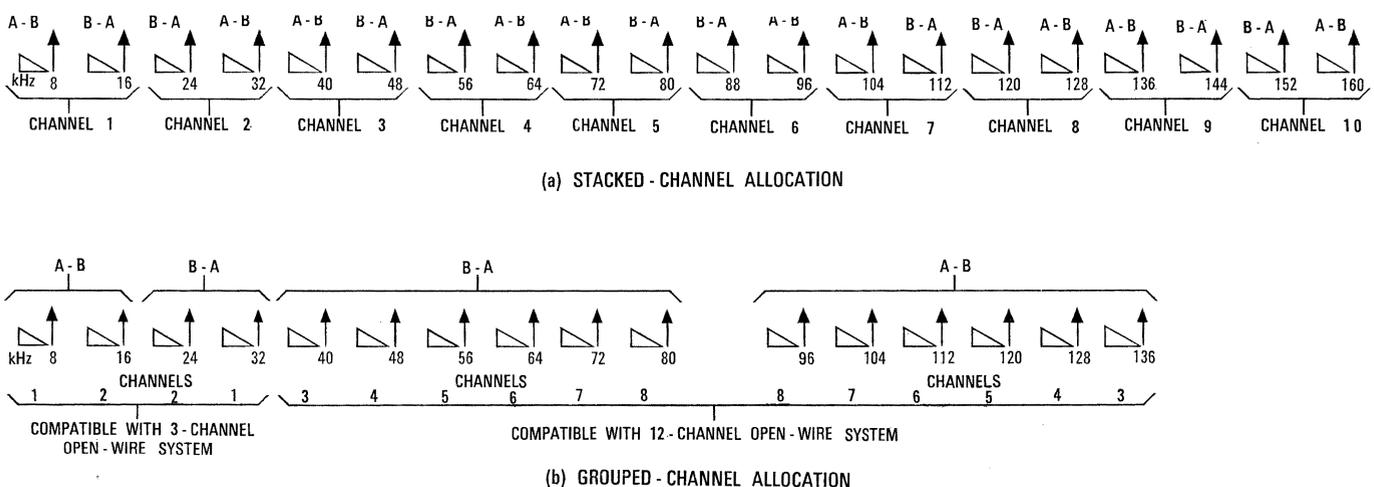
Figure 1 - Frequency allocation plans for stacked and grouped systems.
