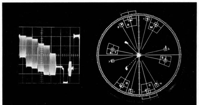
Figure 9 - Composite video with chrominance signal at the transmitter output.
