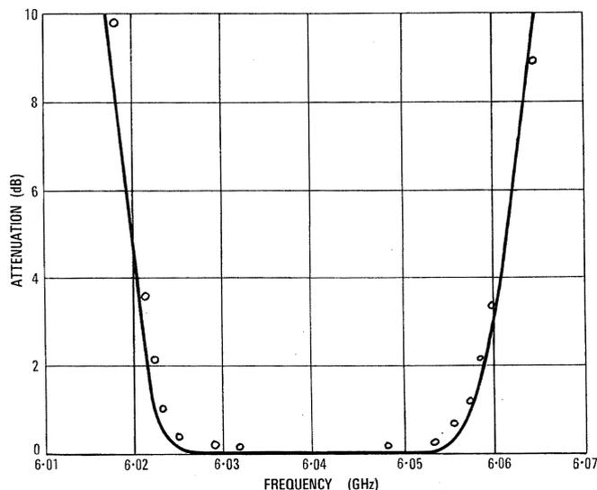
Figure 7 - Measured and calculated relative insertion loss of filter (continuous curve is calculated loss).
