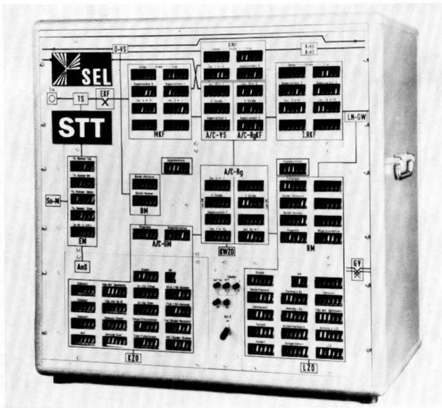
Figure 3 - Panel of memory for fault detection.
