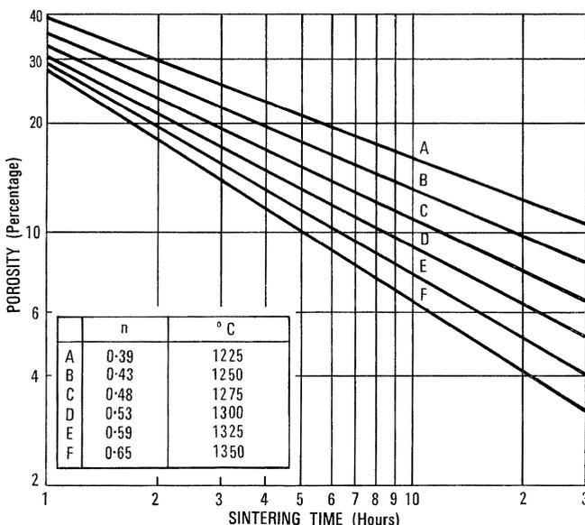
Figure 10 - Relationship between porosity and sintering duration at different temperatures and for a given amount of ferrous iron.
