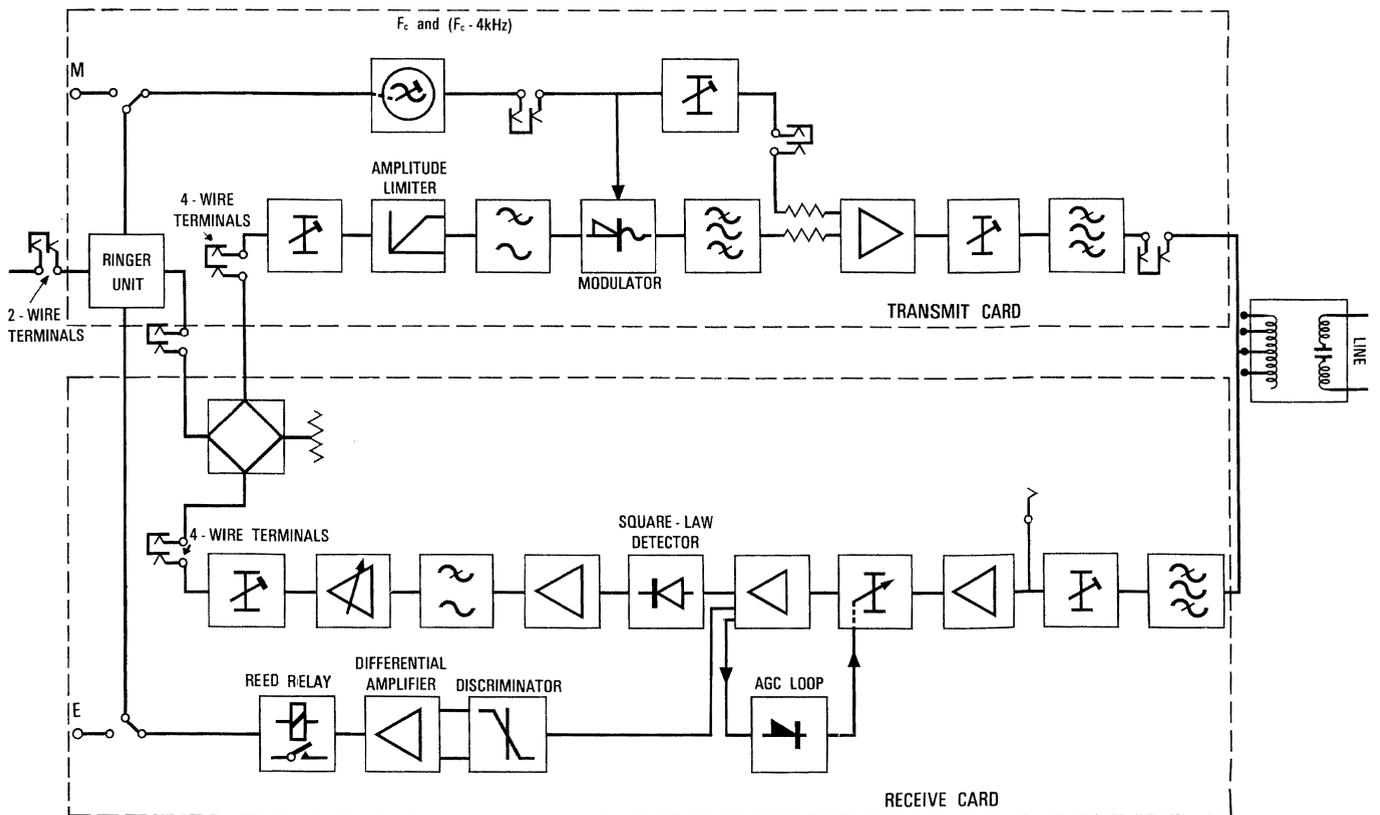
Figure 2 - Block schematic of receive and transmit terminal cards.
