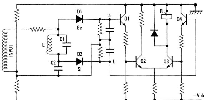
Figure 5 - Signaling receiver and discriminator circuit.
