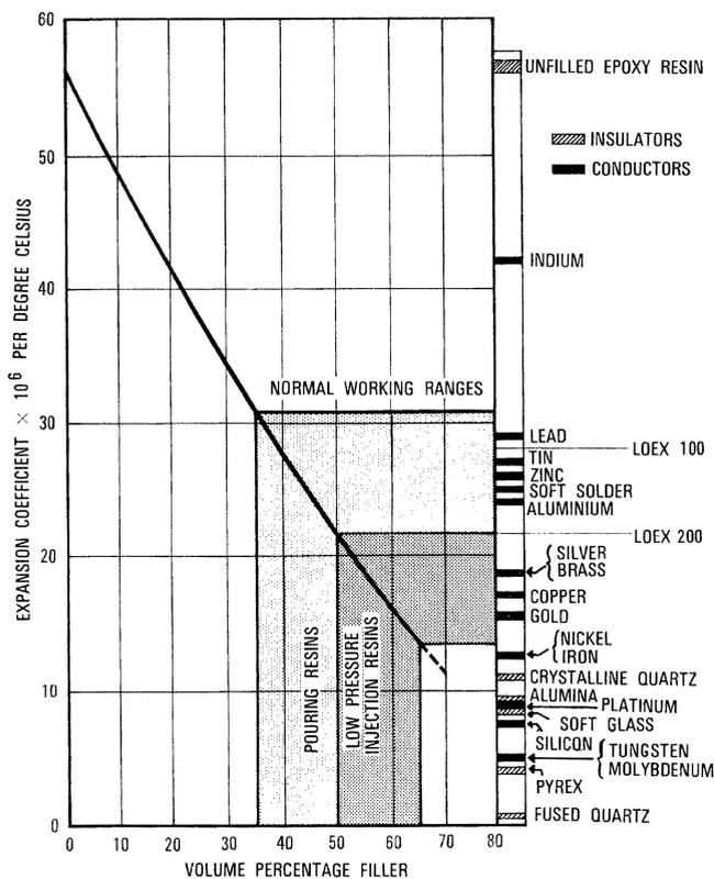
Figure 1 - Casting resins with matched thermal expansion.
