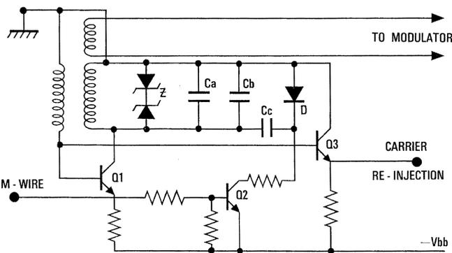
Figure 3 - Final oscillator circuit without biasing and matching details.
