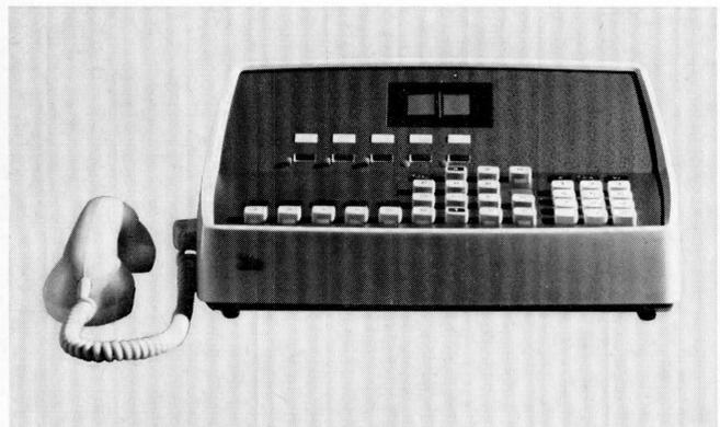
Figure 7 - Operator's desk of a Herkomat 5-50-6 exchange with push-button selection comprising meters and luminous-number extension identification.
