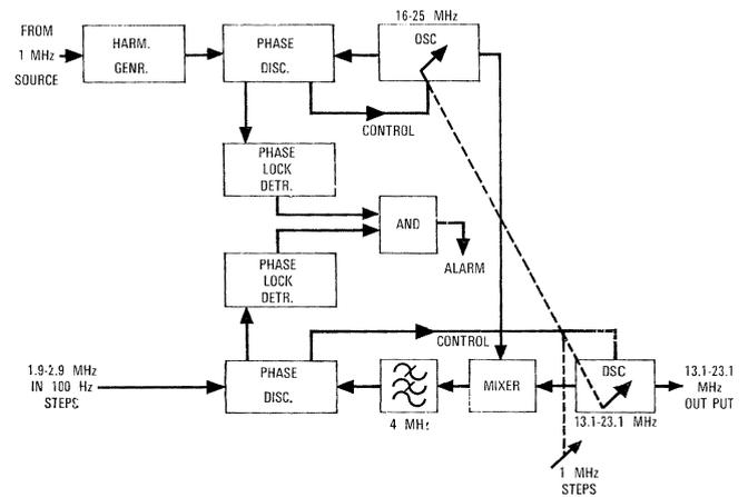
Figure 5 - High-frequency exciter, frequency synthesis, second stage.
