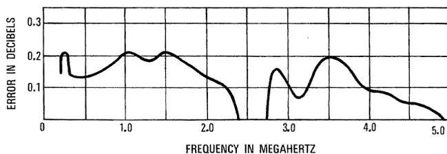
Figure 7 - Equalisation error of repeater compared to target gain.
