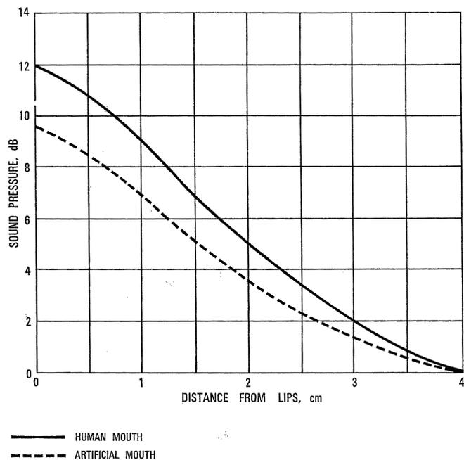
Figure 5 - Sound pressure at mid-band frequency on axis of mouth for B & K 4216 artificial mouth and human mouth. Relative to pressure at 4 cm from human lips.
