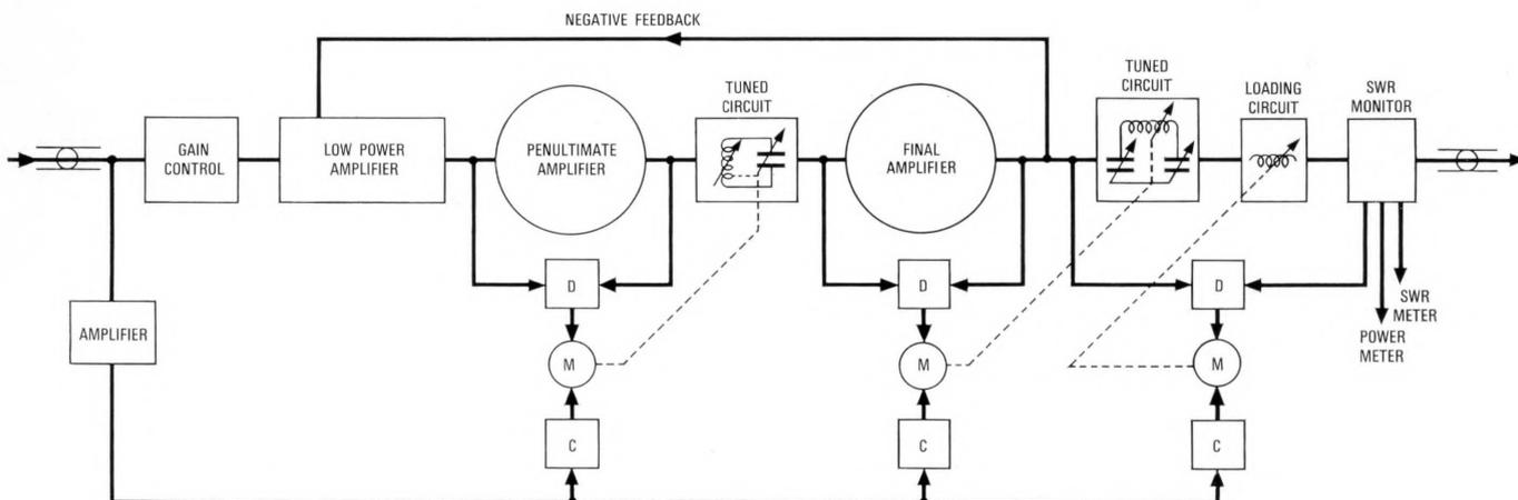
Figure 7 - High-frequency amplifier type QT8 block diagram.
