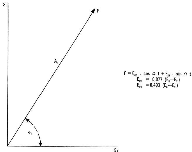
Figure 3 - Vector diagram of the modulated subcarrier.
