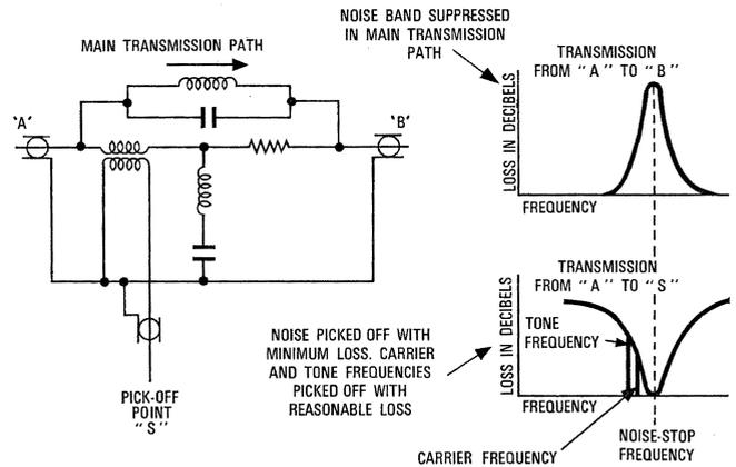
Figure 6 - Diagram illustrating supervisory pick-off method.
