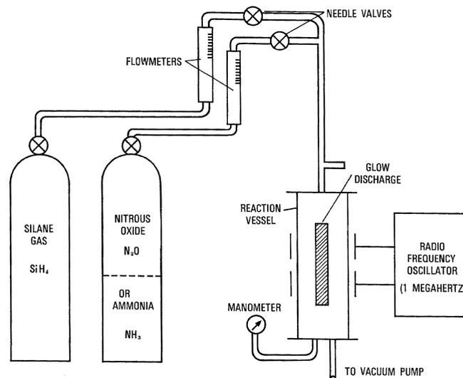
Figure 2 - Flow system for the coating apparatus.
