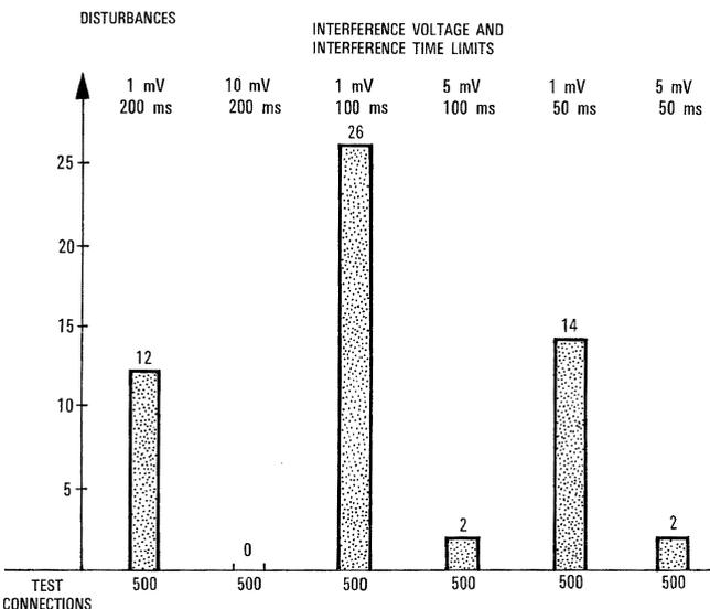
Figure 3 - Result of noise tests using the test connection equipment.
