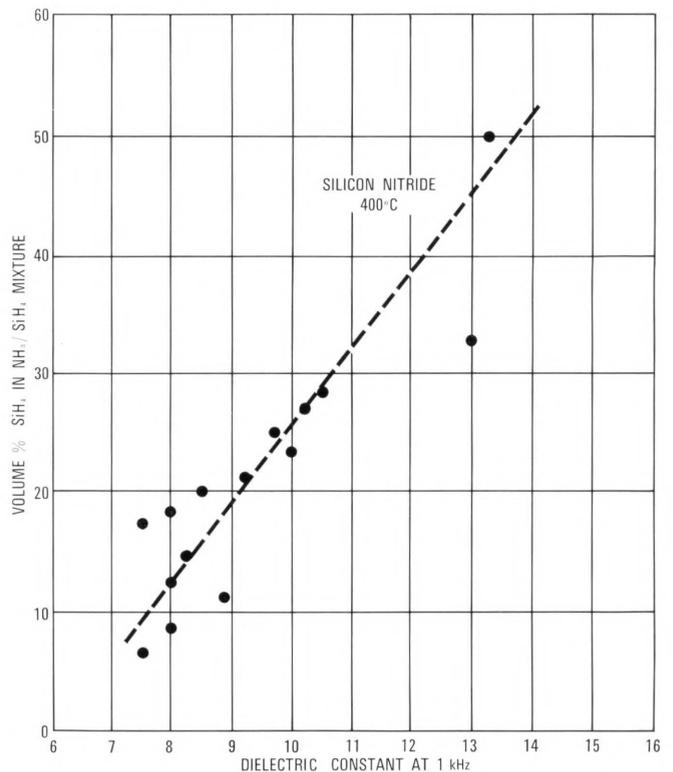
Figure 4 - Variation with gas composition of dielectric constant of silicon nitride deposited at 400 degrees Celsius.
