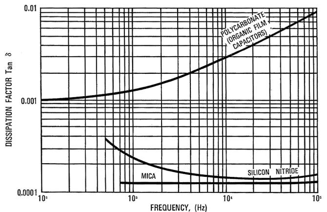
Figure 8 - Dissipation factor as a function of frequency.
