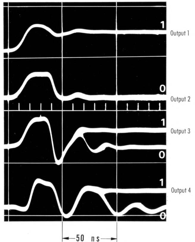
A typical switching process by which the 4 most significant digits of the equilibrium coder reach their correct output state. The ranges of samples giving rise to the outputs 1001 and 1010 are 38 to 40 and 40 to 42 quantum step units, respectively.
