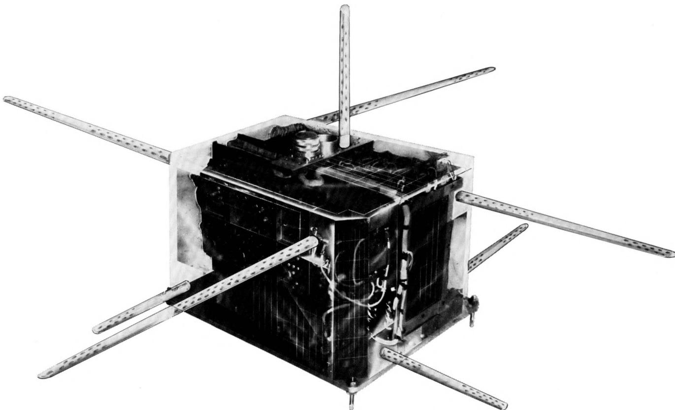
Figure 9 - Phantom view - ITT type II satellite.
