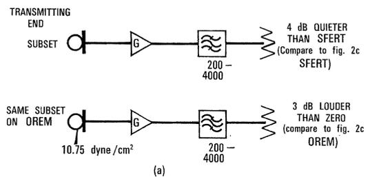
Figure 3 - a) Subset with gain "G" and band-pass filter.
