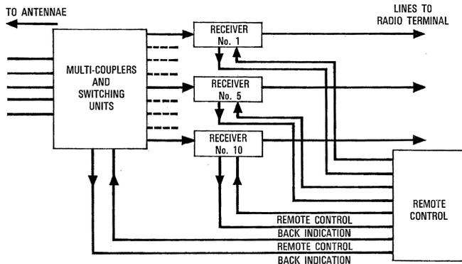
Figure 10 - Receiver station, block diagram.
