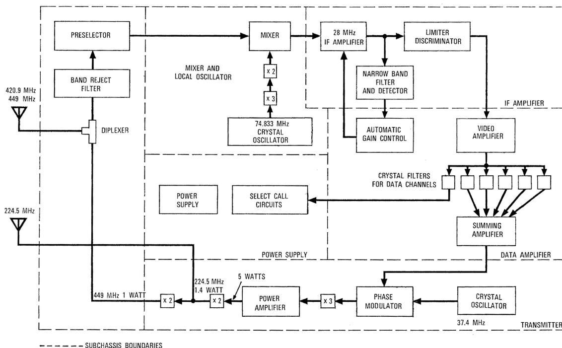
Figure 11 - Solid-state transponder model 102, block diagram.
