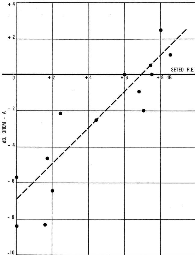
Figure 1 - a) Transmitting comparison of subjective and objective reference equivalents SETED (NOSFER) and OREM-A.
