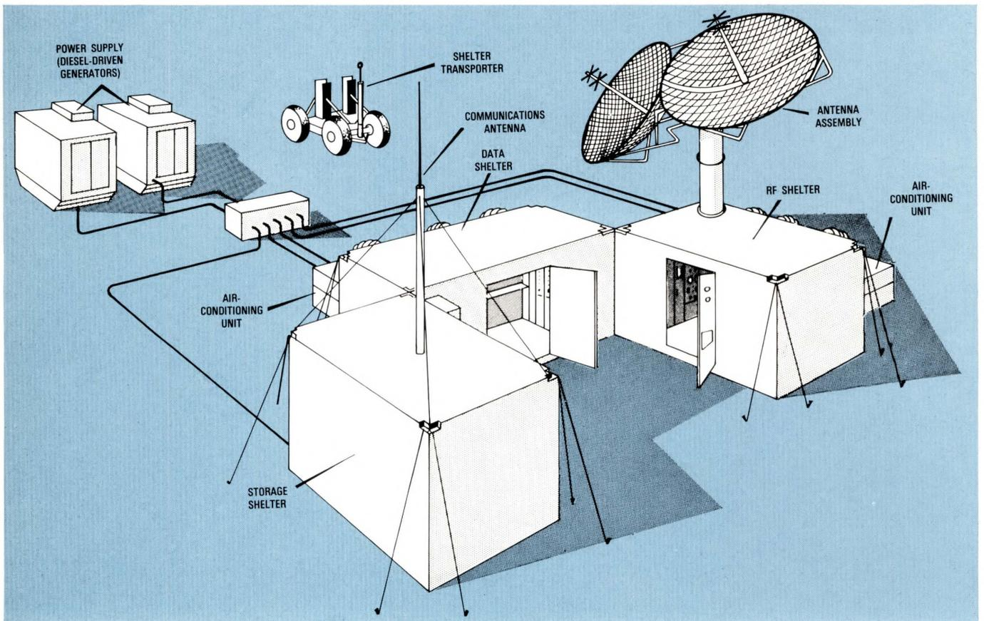
Figure 7 - Geodetic satellite ground station.
