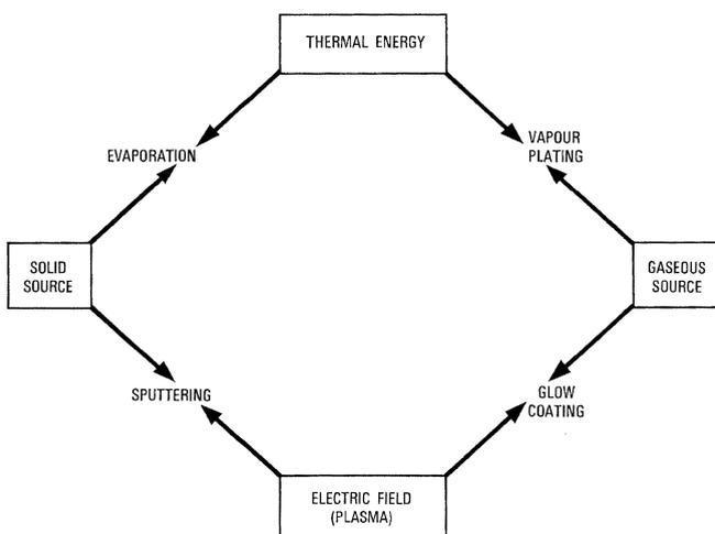
Figure 1 - Relationships of gas-phase deposition processes.
