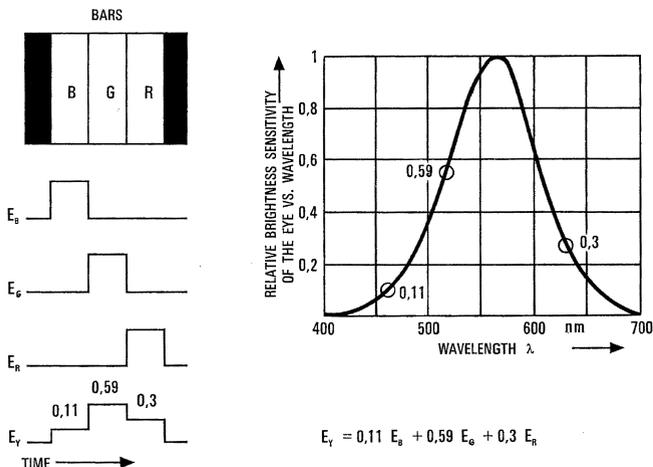
Figure 2 - Generating the luminance signal  $E_Y$ .
