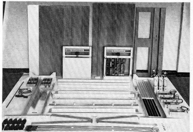
Figure 2 - Loose parts for building up a 2003 P toll board.
