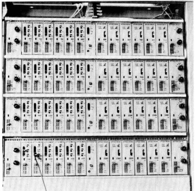
Subrack mounting of a 24-channel group. Each level comprises: a transmit line unit, 6 VF transmitters, a local voltage stabilizer, 6 VF receivers, and a receive line unit.
