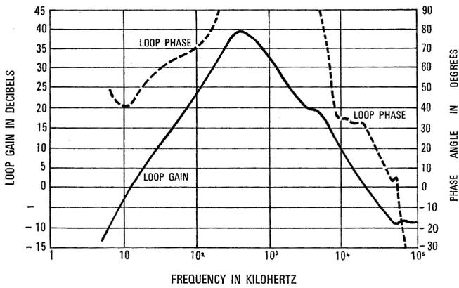
Figure 5 - Amplifier feedback loop characteristic.
