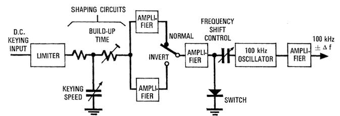
Figure 2 - Frequency-shift-keying modulator block diagram.
