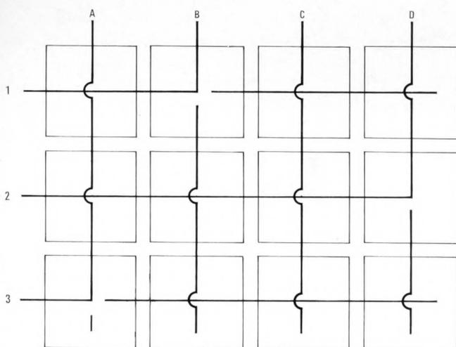
Figure 8 - Output crossbar switch, diagram.
