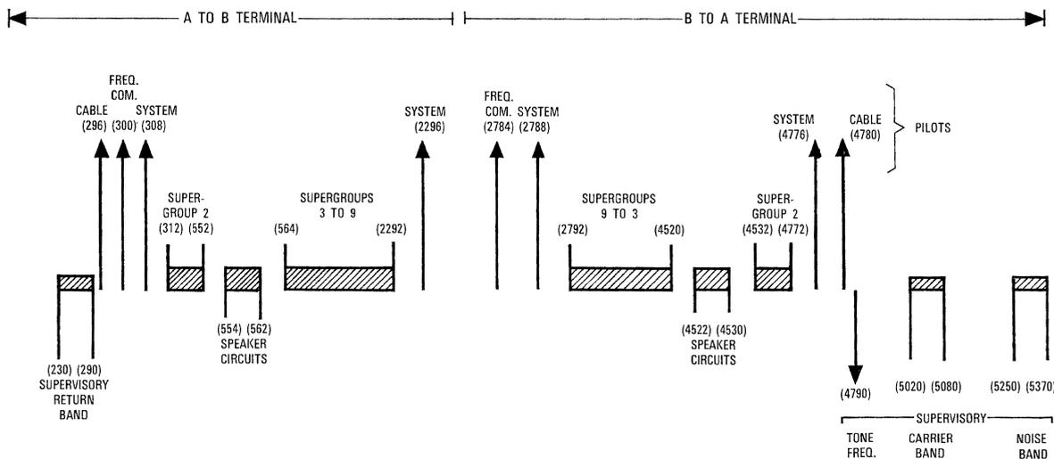
Figure 1 - System frequency spectrum (frequencies in kilohertz are given in parentheses).
