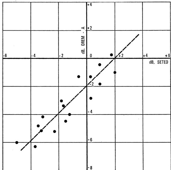
b) Receiving comparison of subjective and objective reference equivalents SETED (NOSFER) and OREM-A.
