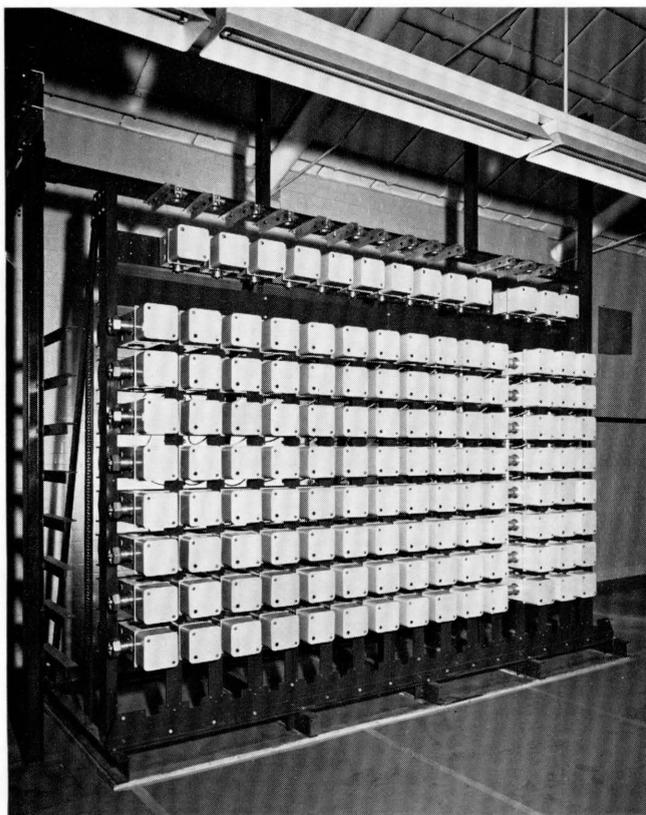
Figure 9 - Output crossbar switch, photograph.
