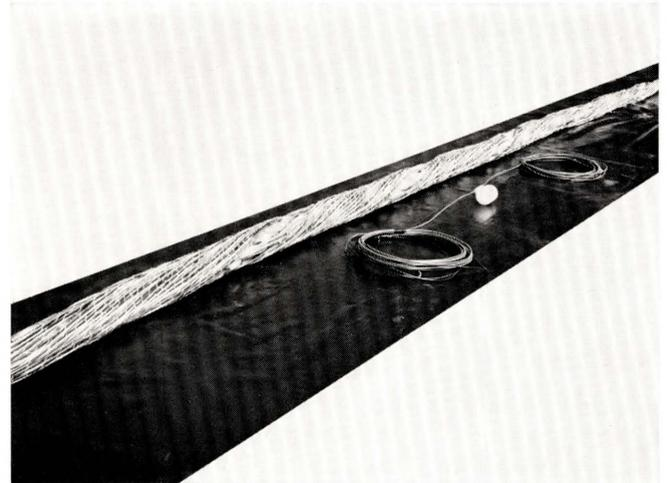
Figure 7 - Loading assembly containing 68 side circuit coils.
