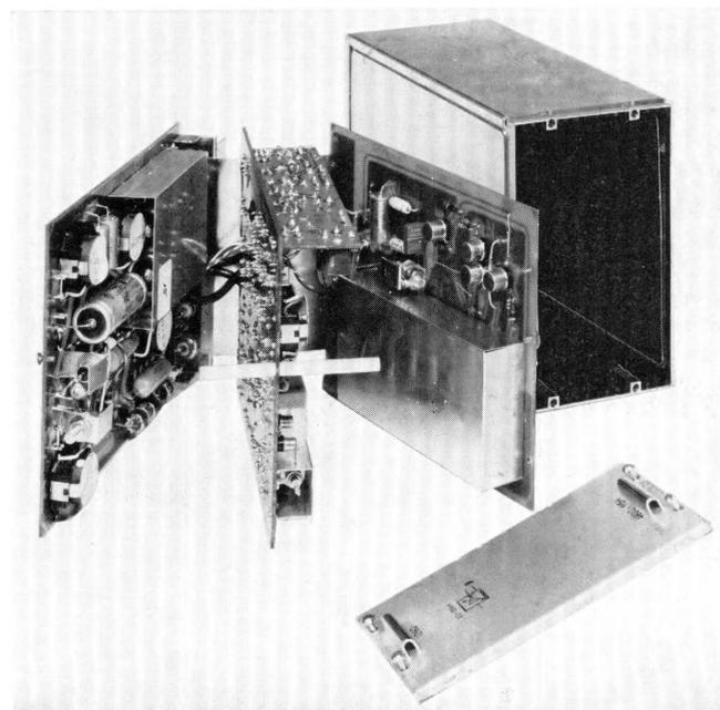
1260-channel equipment - 6 MHz bandwidth line amplifier with pilot-regulator and supply separator filter.
