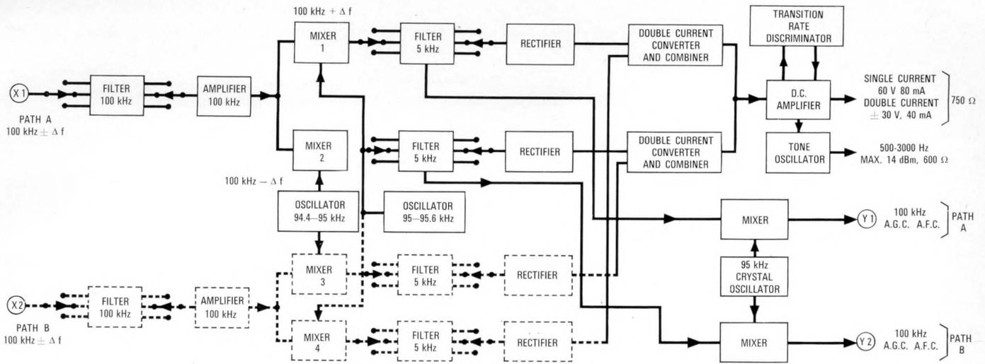
Figure 12 - RX 11 receiver, telegraph equipment, block diagram.
