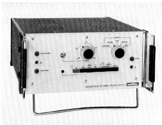
Pattern generator GX 951 A for the SECAM system.
