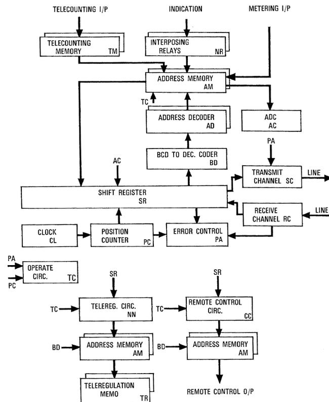
Figure 4 - Slave station - Block diagram.
