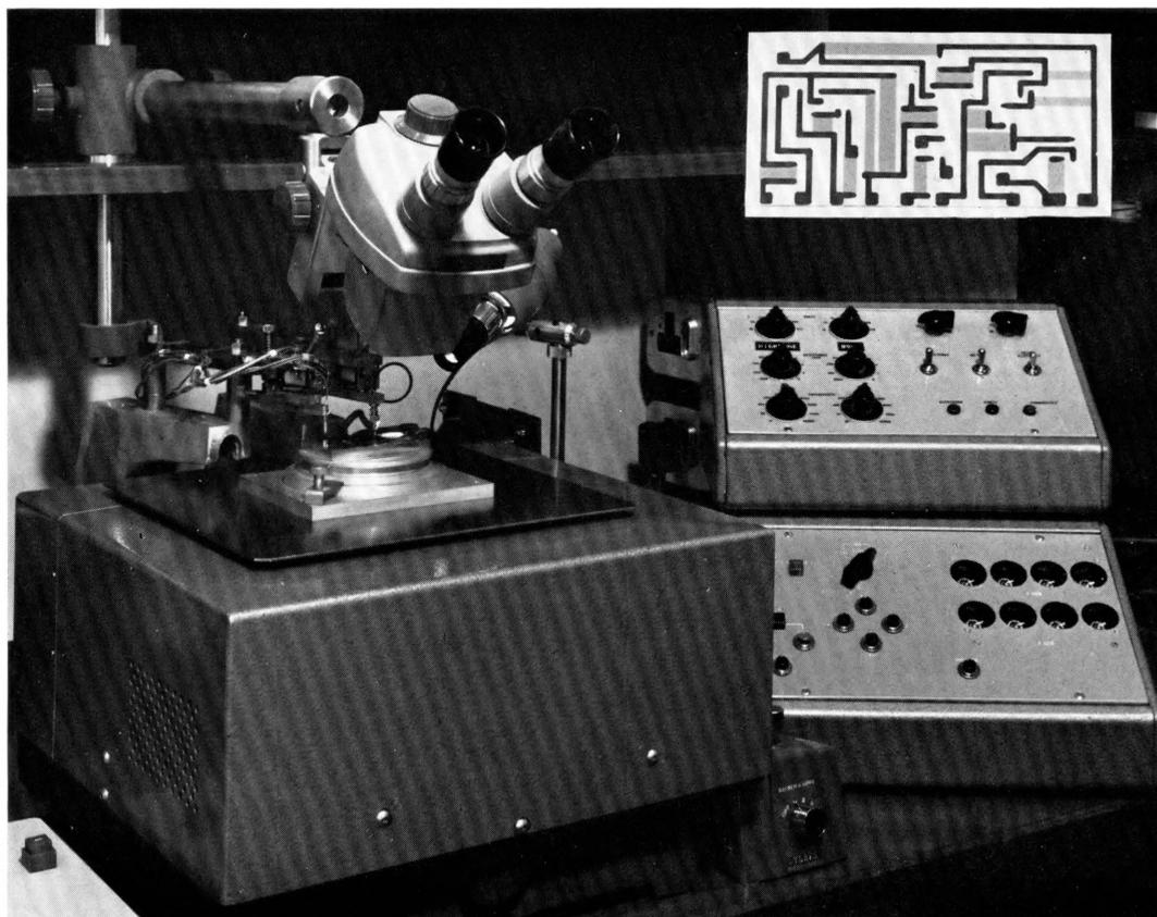
"Writing in" equipment for tape-controlled thin-film circuit, fabrication, with (inset) a typical thin-film resistor and interconnection pattern produced on a  $1 \times \frac{1}{2}$  inch ( $2.5 \times 1.25$  cm) substrate.
