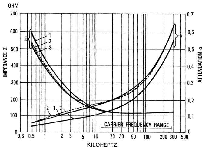
Figure 2 - Impedance and attenuation of land cables compared to those of "wet" submarine cables.
