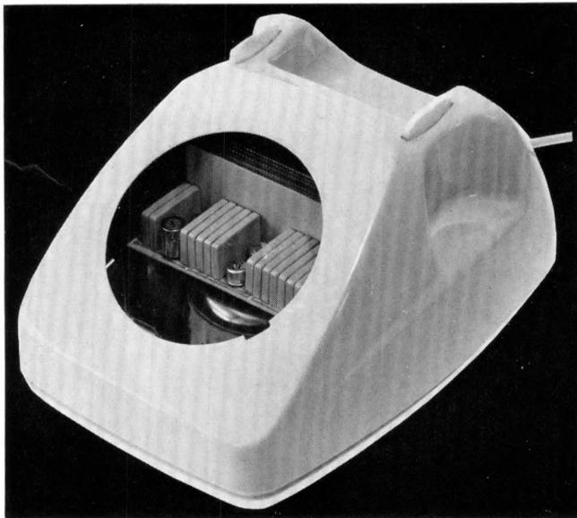
A telephone subset fitted with a model of a PCM coder-decoder.
