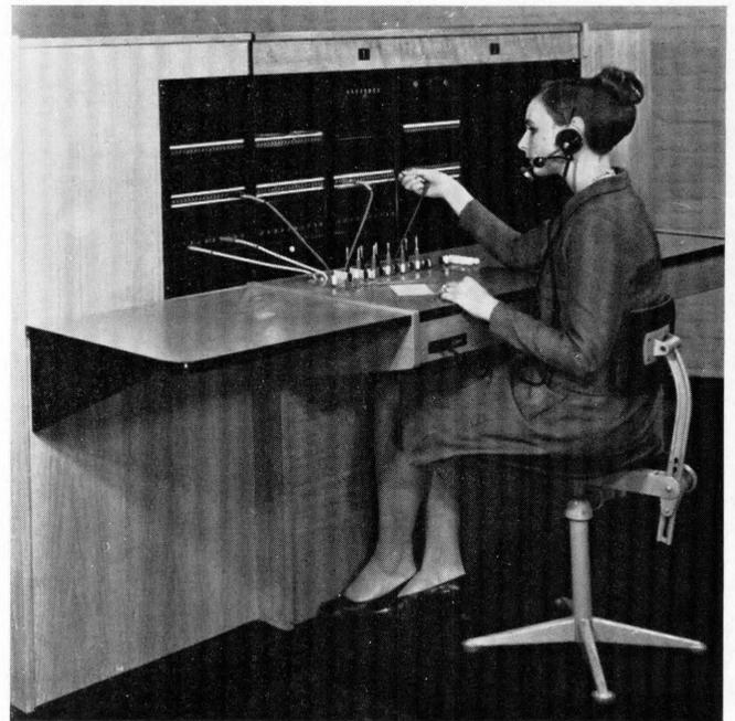
Figure 1 - Front view of the 2003 P toll board.
