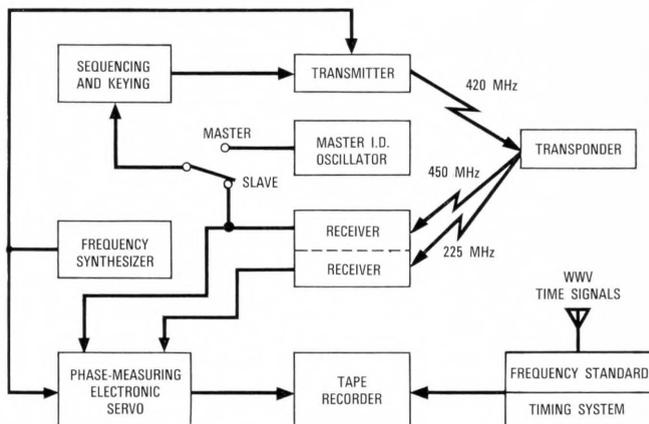
Figure 4 - Simplified block diagram of geodetic satellite system.
