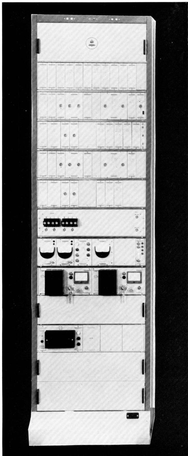
1260-channel equipment - Terminal equipment of the trial section.
