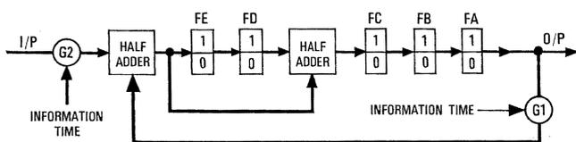
Figure 3 - Error control bits generator corresponding to  $1 + X^2 + X^5$
