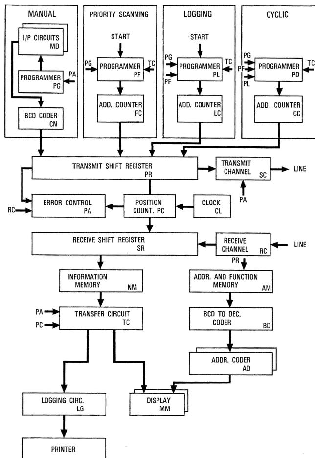
Figure 2 - Master station - Block diagram.
