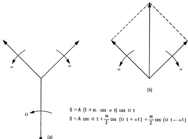
Figure 4 - Amplitude modulation.
