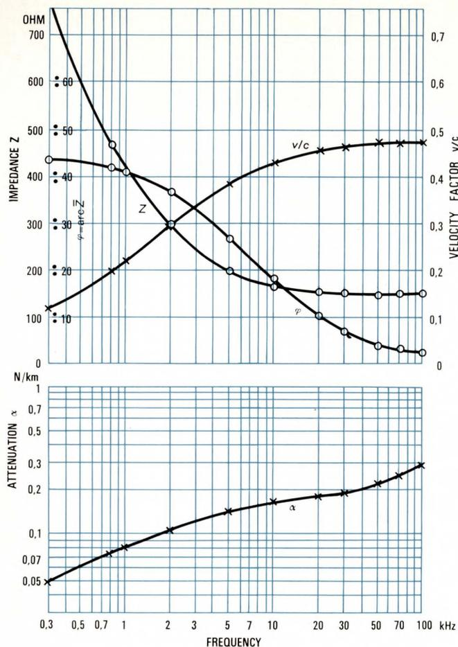
Figure 1 - Electrical characteristics of a typical "wet" submarine cable.
