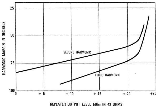
Figure 8 - Harmonic margins of repeater against fundamental output level.
