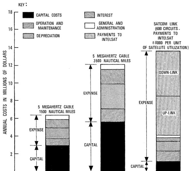
Figure 9 - Comparative annual cost mix for "heavy" transoceanic trunk routes (medium and long haul).
