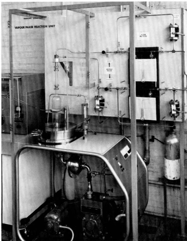
Figure 5 - Silicon nitride deposition plant.
