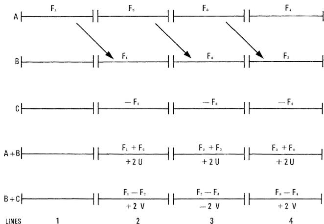
Figure 11 - Signal sequence in PAL — Decoder.
