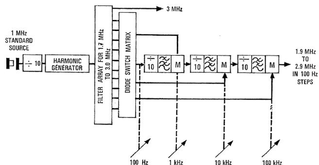
Figure 4 - High-frequency exciter, frequency synthesis, first stage.
