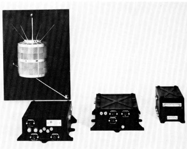
ESRO I Satellite and its electronic subunits RL 1446 A, B, and C.
