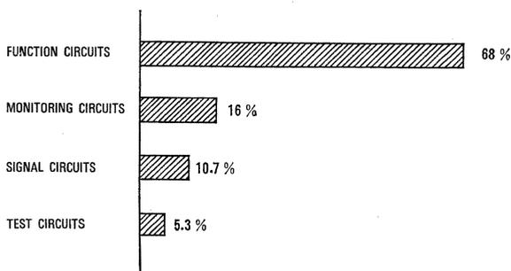
Figure 6 - Breakdown of failures by system parts.
