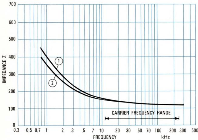
Figure 6 - Impedance matching of embedded "wet" submarine quad to DM land cable.
