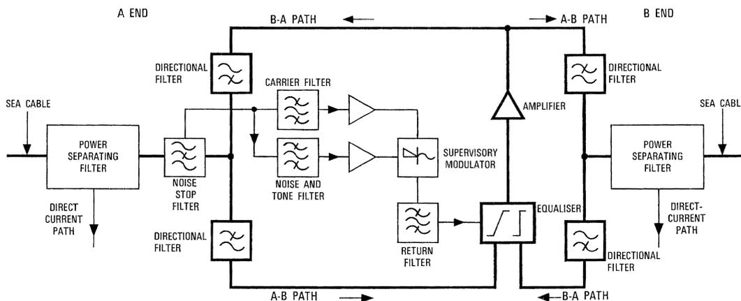
Figure 2 - Block schematic of repeater.
