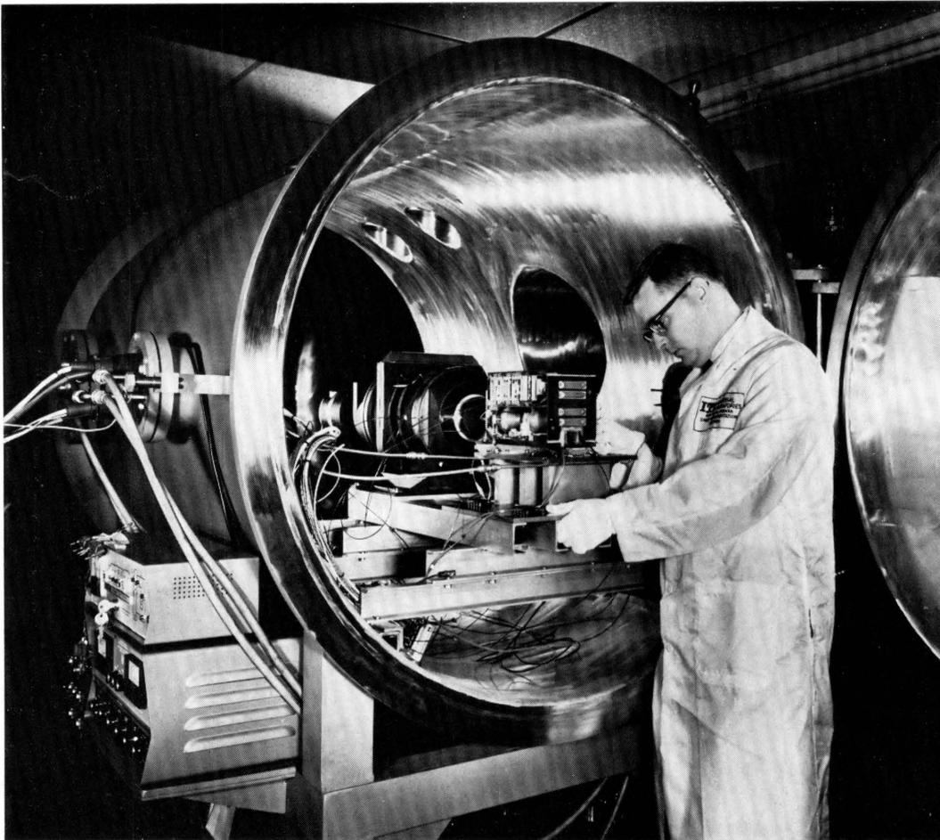
Daytime camera system for the Nimbus-D satellite being tested under conditions of outer space.
