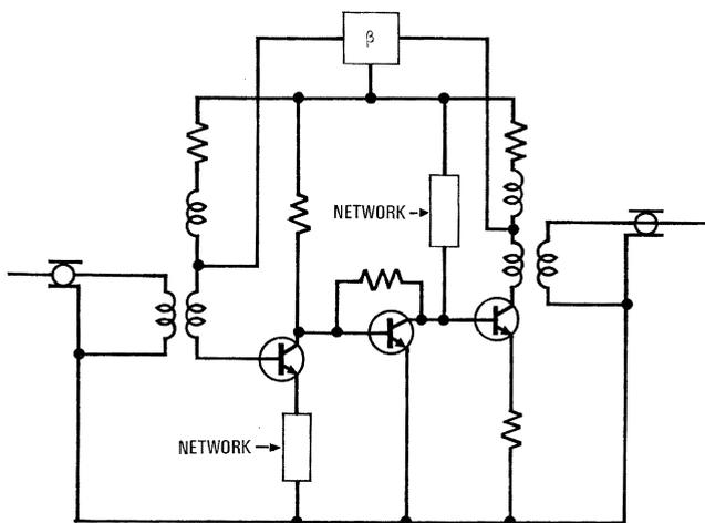
Figure 3 - Simplified amplifier schematic.
