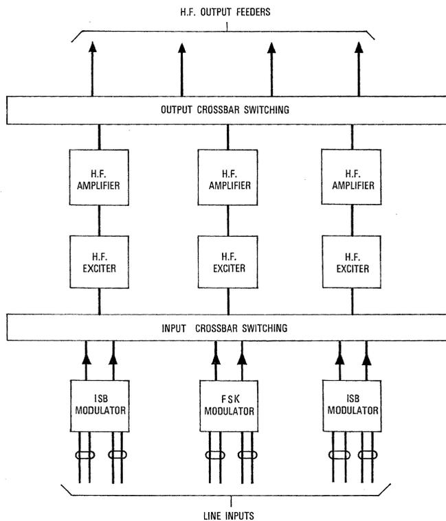
Figure 1 - Transmitter station, signal path.
