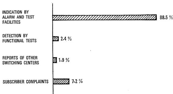
Figure 5 - Breakdown of failure reports.
