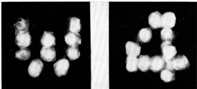
Figure 2 - Optical displays obtained from a 25-element array; the letter W and the numeral 4.
