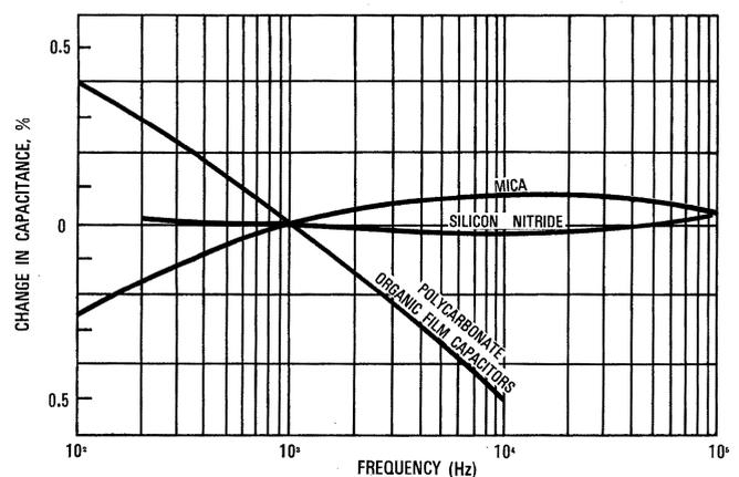
Figure 7 - Capacitance change with frequency.
