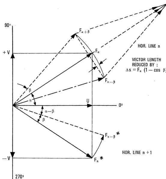
Figure 8 - PAL alternate line-switching principal (vectorial presentation).
