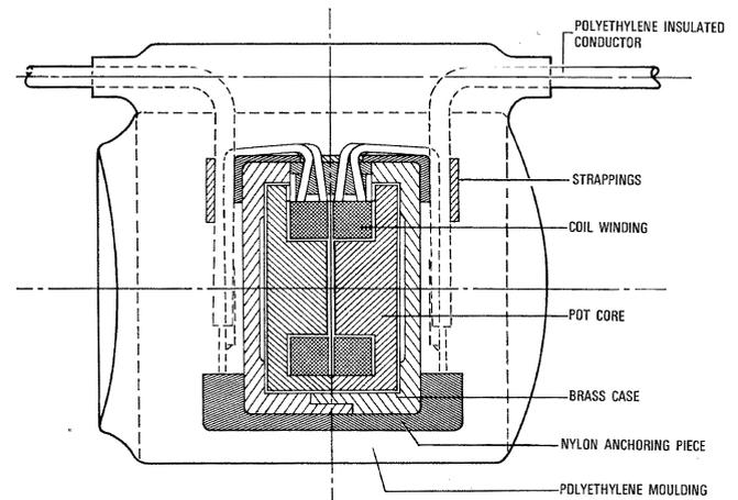
Figure 4 - Design of loading element.
