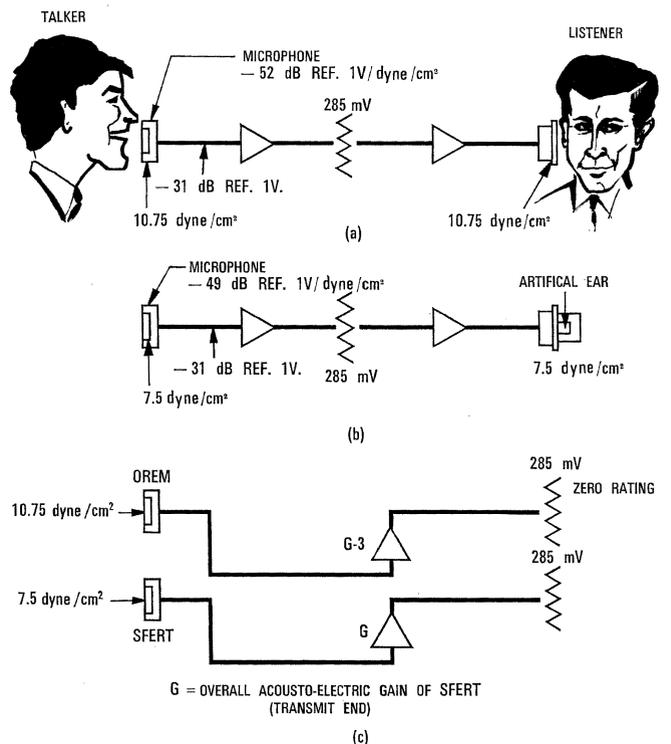
Figure 2 - a) SFERT - Thermophone calibration.
