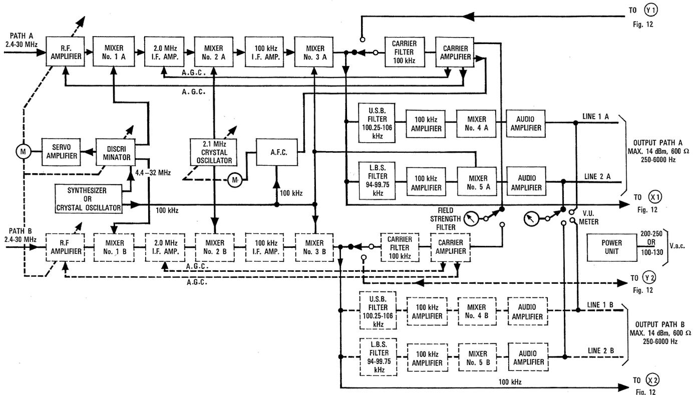
Figure 11 - RX 11 independant side-band receiver, block diagram.
