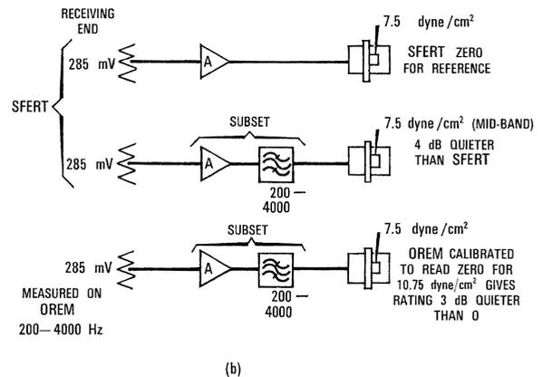
Figure 3 - b) Subset with gain "A" and band-pass filter.
