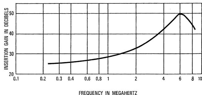
Figure 4 - Gain characteristic of repeater amplifier.
