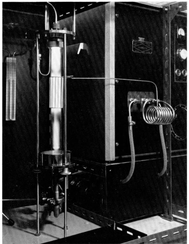
Figure 3 - Experimental apparatus for the formation of films by glow discharge.
