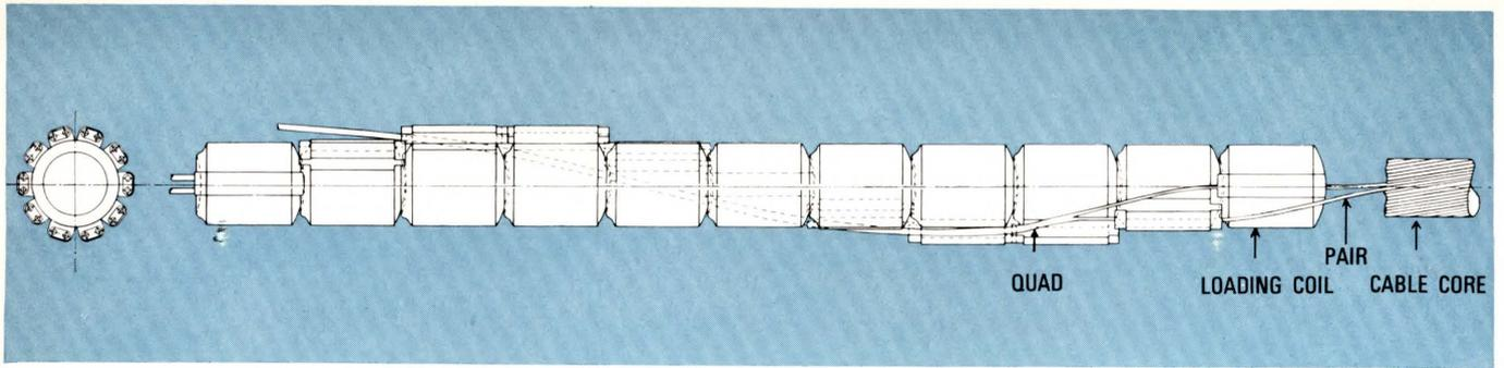
Figure 5 - Assembly of loading elements.
