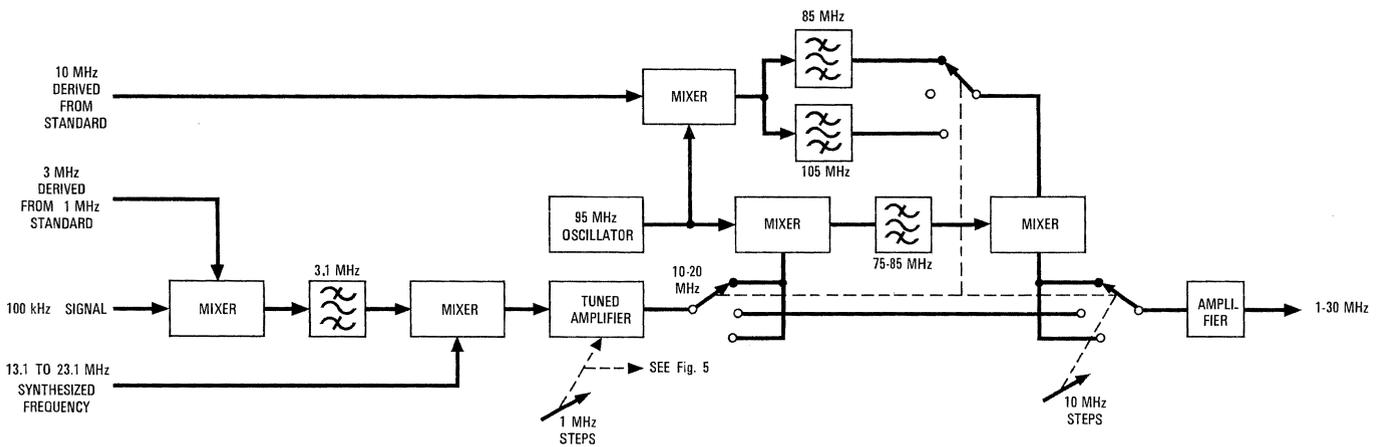
Figure 3 - High-frequency exciter, modulated signal path block diagram.
