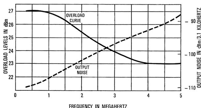
Figure 9 - Repeater output noise and overload level.
