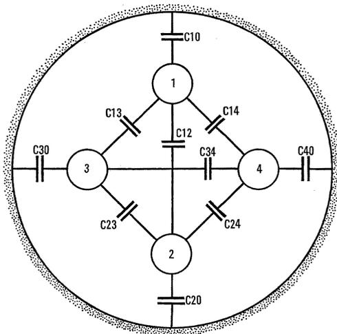
Figure 3 - Partial capacitances in a telephone cable star quad.
