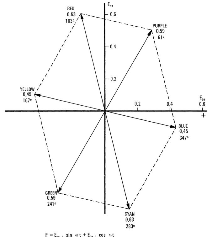
Figure 5 - Phase relations of subcarrier components.
