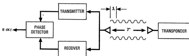
Figure 3 - Theory of range measurements.
