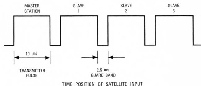
Figure 5 - Satellite interrogation cycle.
