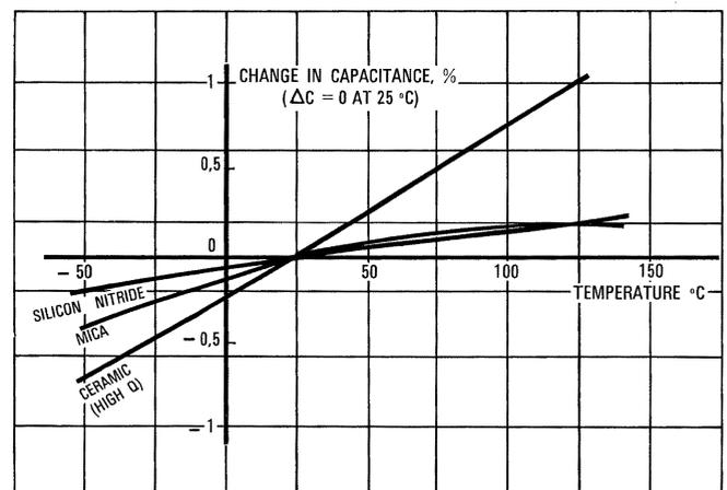
Figure 6 - Percent capacitance change with temperature from the capacitance value at 25 degrees Celsius.
