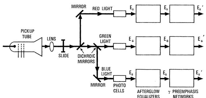
Figure 1 - Color Slide scanning (Schematic).
