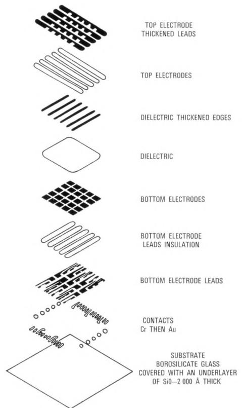
Figure 1 - Exploded view of 25-element array.
