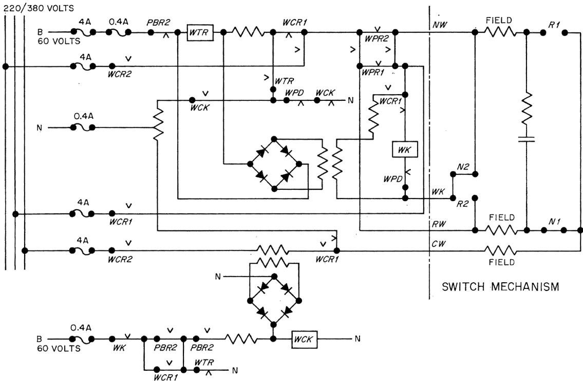
Figure 1—Switching machine is operated from 3-phase power supply.
