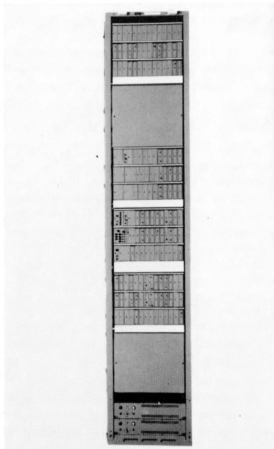
Figure 22—Master and supermaster groups for a 2700/1800-channel telephone system are mounted in this bay, which is 520 millimeters (21 inches) wide and 2750 millimeters (108 inches) tall. Design conforms with the standard equipment practice for ITT Europe.
