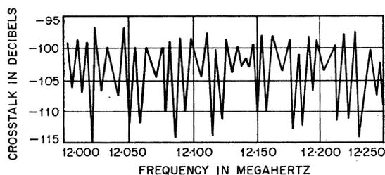
Figure 14—Crosstalk measured at close frequency intervals for the trial installation.
