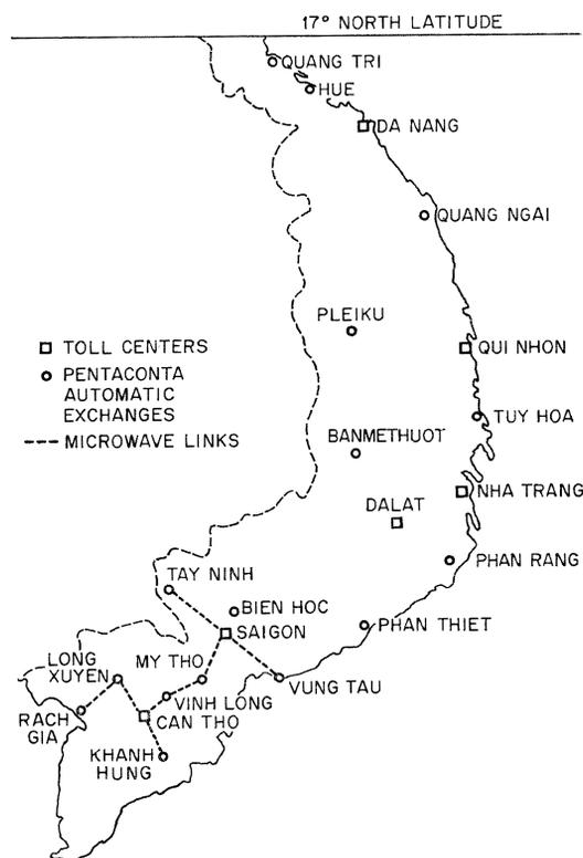
Figure 8—Installations in South Vietnamese nationwide telecommunication system.
