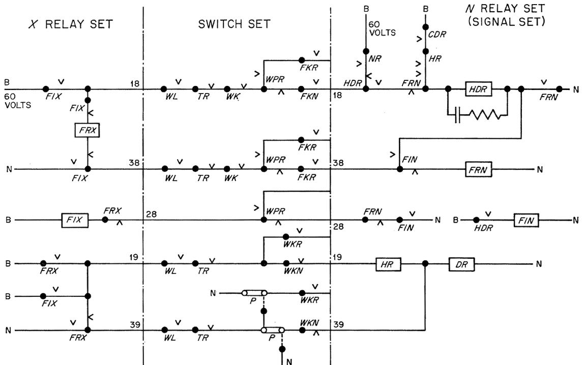
Figure 5—Signal control for geographic system.
