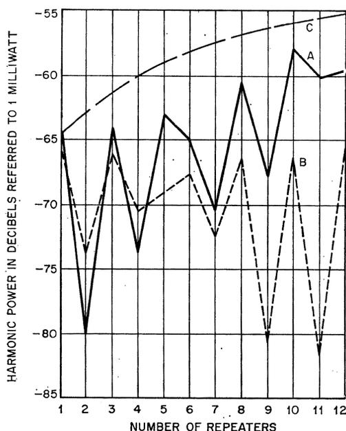
Figure 11—Second-harmonic distortion over the trial route for a fundamental of 6.25 megahertz at 0 decibels referred to 1 milliwatt at the transmit terminal output. *A* is measured, *B* is calculated allowing for section phase shift, and *C* is calculated assuming power addition.
