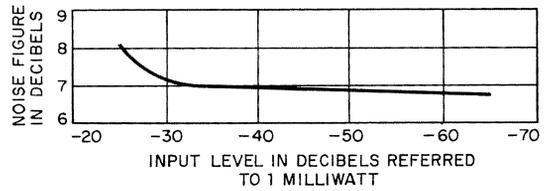
Figure 11—Receiver noise figure for super-high-frequency input.
