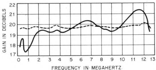
Figure 9—Gain-frequency characteristic over the trial route. The solid curve is before and the broken-line curve is after mop-up equalization, which limited the final spread to 0.55 decibel.
