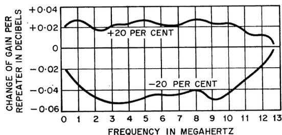
Figure 13—Variation of gain per amplifier with changes of 20 per cent in power-feeding currents.
