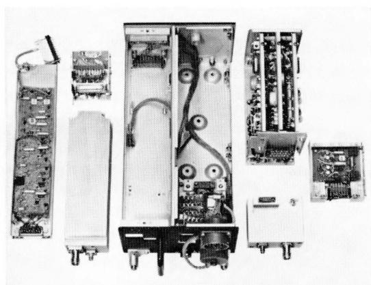
Figure 3—Modular construction of *STR 70-P*. From the left are the video unit, transmitter (front) and apparatus unit, chassis that has no active circuits but serves only for support and interconnecting, receiver (front) and power unit, and at extreme right the interface unit. The 3 units at the right are accommodated in the right half of the chassis unit.
