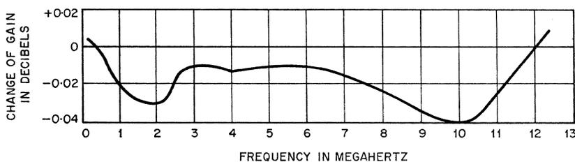
Figure 3—Change in gain for a 40-degree Celsius rise as a function of frequency.
