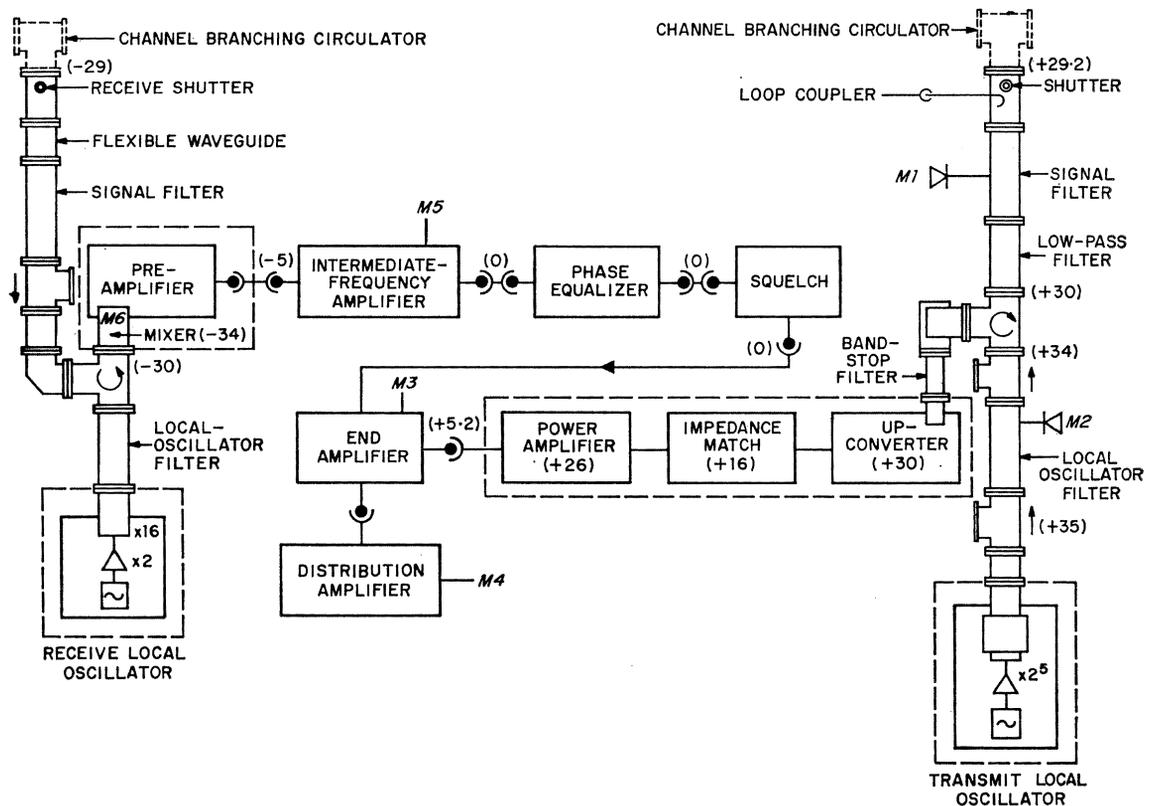
Figure 1—Block diagram. Nominal power levels are shown in parentheses in decibels referred to 1 milliwatt (dBm).
