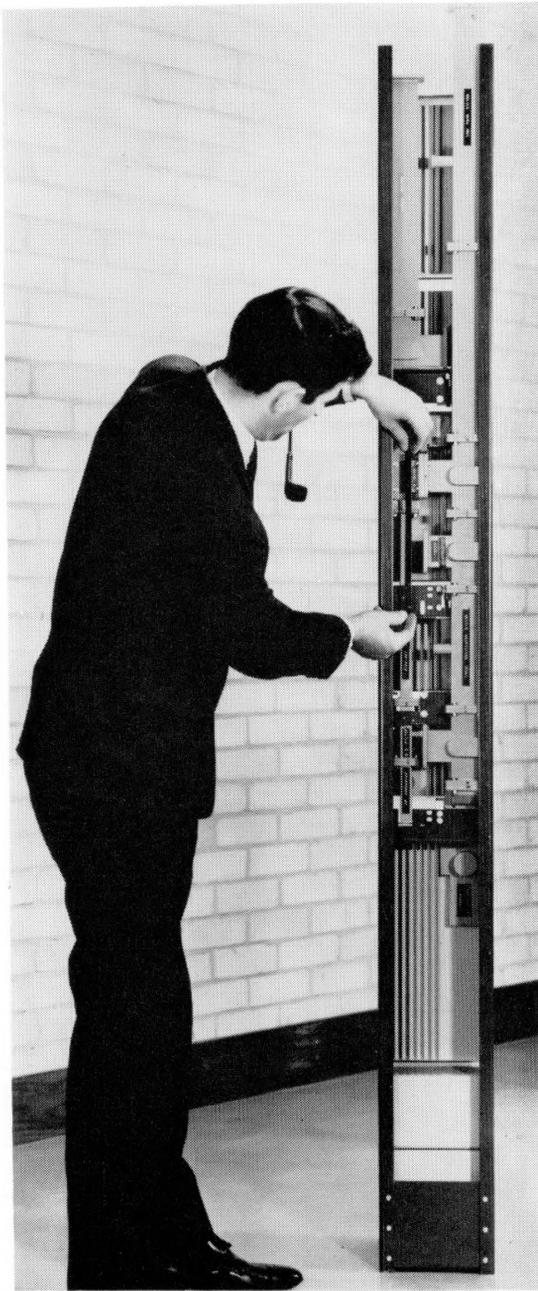
Figure 2—Rear view of the slimrack showing vertical waveguide runs.
