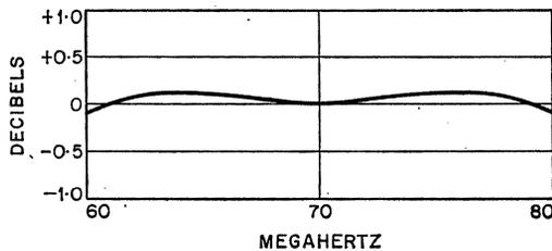
Figure 8—Transmitter-to-receiver response-frequency characteristic for an input level of -65 decibels referred to 1 milliwatt corresponding to a 35-decibel fade.
