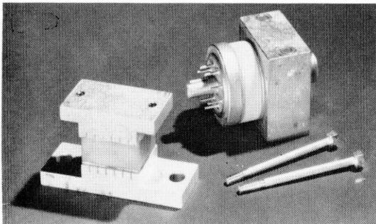
Figure 21—The *4KC/160M* ultra-high-frequency tetrode with its associated heat-sink mount.
