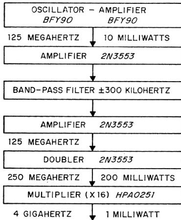
Figure 5—Receive local oscillator.
