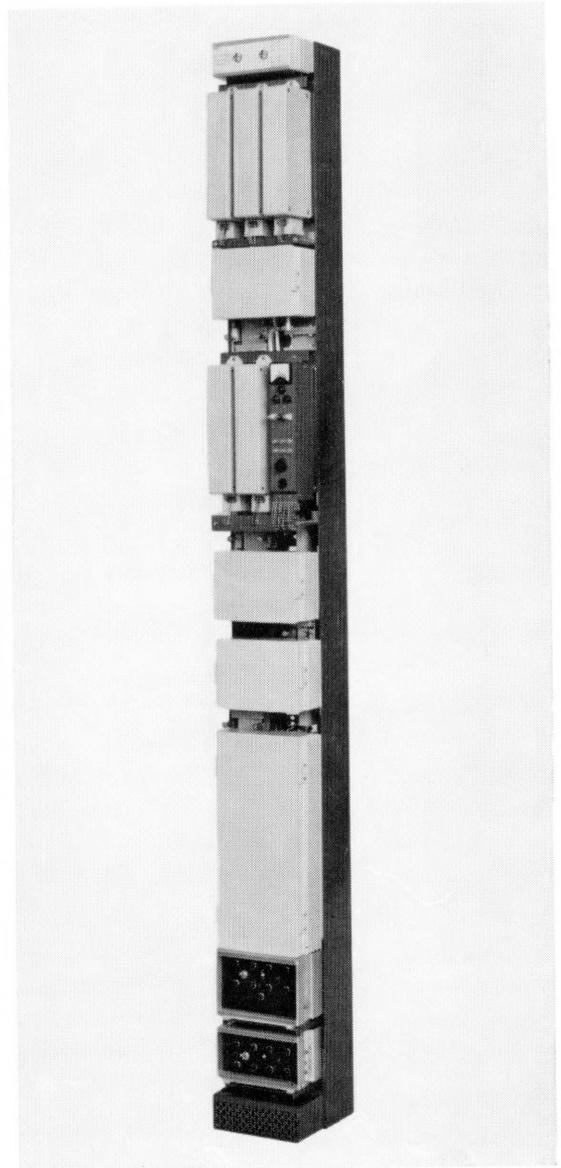
Figure 3—Front view of the slimrack. At the top is the alarm indicator while the 3 panels immediately below are the squelch, end amplifier, and distribution amplifier. The pre-amplifier is next and beneath it are the equalizer, intermediate-frequency amplifier, and meter panel. The next three units are the receive local oscillator, power amplifier, and transmit local oscillator. At the bottom are the transmit and receive power units.
