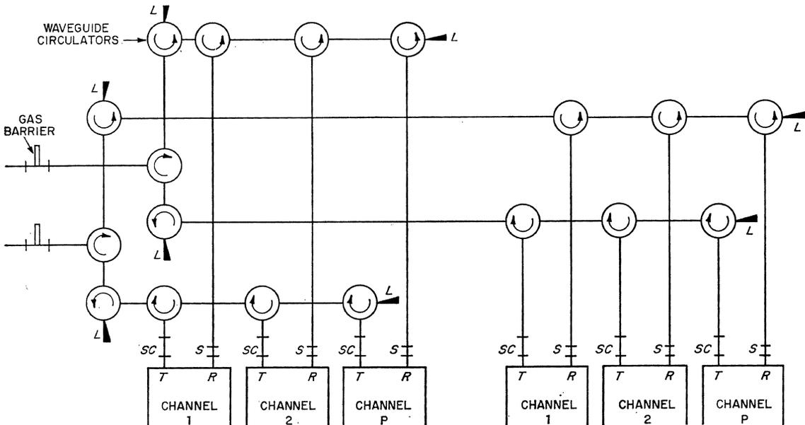
Figure 12—Channel branching scheme. *S* = waveguide shutter switch. *SC* = waveguide shutter switch with test point on transmitter side. *L* = waveguide load. *T* and *R* are transmit and receive halves of the indicated channels.
