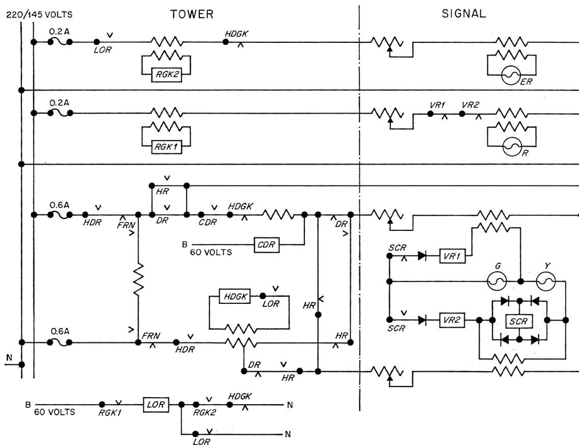
Figure 6—Light signal circuits.
