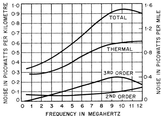
Figure 5—Computed system noise for a 280-kilometre (175-mile) route.
