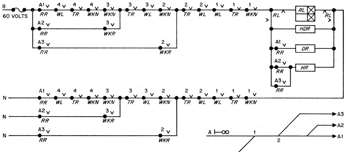
Figure 2—Signal control circuits with relay interlocking.
