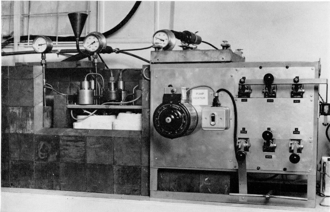
Figure 2—S.T.C. Semiconductors designed this equipment for pressurizing semiconductor devices in radio-active krypton to obtain ultra-fine leak measurements. Some of the lead bricks used for screening have been removed to reveal the test chambers.
