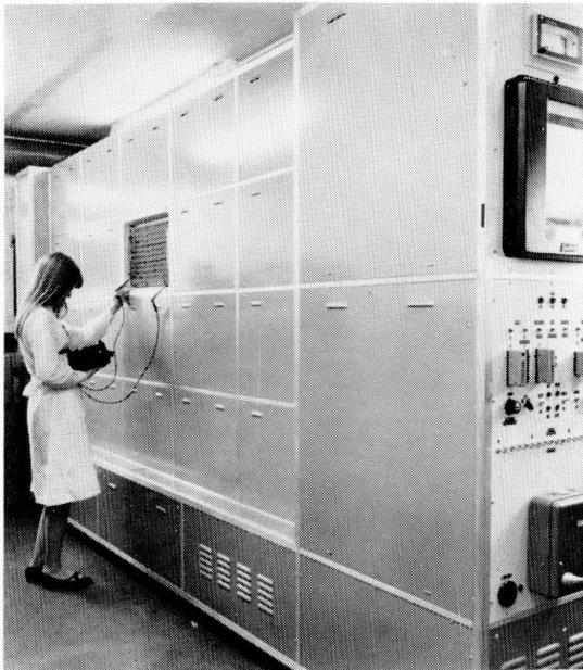
Figure 1—Life test rack on which 2557 transistors and 4743 diodes were burnt-in for three months, without any failures. The rack applies the submarine repeater operation conditions with an elevated device case temperature.
