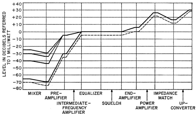
The final stage provides an available 400 milliwatts at 70 megahertz to act as the signal for the up-converter.
