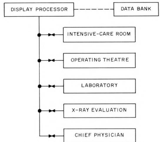
Figure 17—Hospital application of data display system. At each terminal there is a keyboard machine for inserting and requesting data and a console for visual display.
