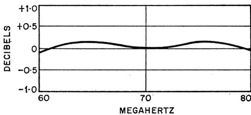
Figure 7—Transmitter-to-receiver response-frequency characteristic for a nominal input level of -30 decibels referred to 1 milliwatt.
