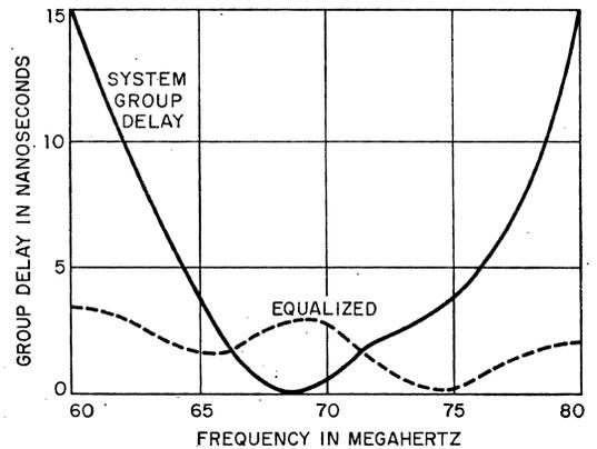
Figure 10—Group delay for a single hop at a super-high-frequency input of -65 decibels referred to 1 milliwatt corresponding to a 35-decibel fade.
