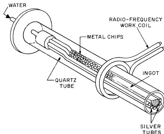
Figure 7—Consolidation of degassed metal chips in a silver boat.
