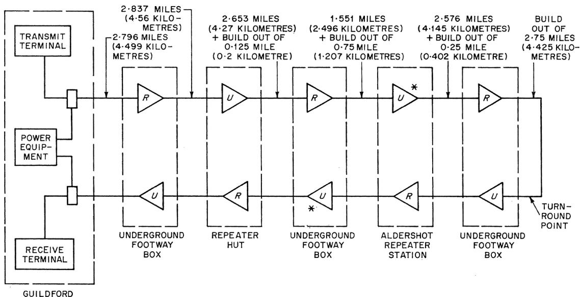
Figure 6—Route of field trial installation having a total looped length including build-out sections of 48 kilometres (29·8 miles). *R* indicates regulated line amplifier and *U* is for fixed-gain amplifiers.
