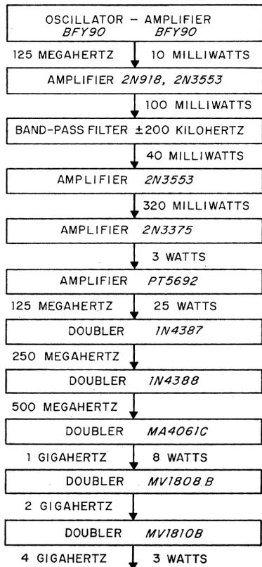
Figure 4—Transmit local-oscillator chain.
