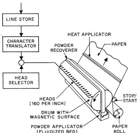
Figure 14—Arrangement of Ferrodot high-speed printer.
