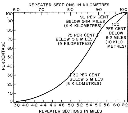
Figure 4—Percentage of repeater sections below the stated lengths for 30 routes of 4-megahertz 960-channel systems.
