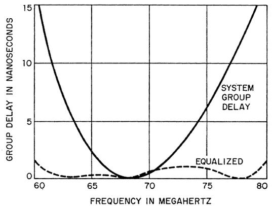
Figure 9—Group delay for a single hop at a super-high-frequency nominal input of -30 decibels referred to 1 milliwatt.
