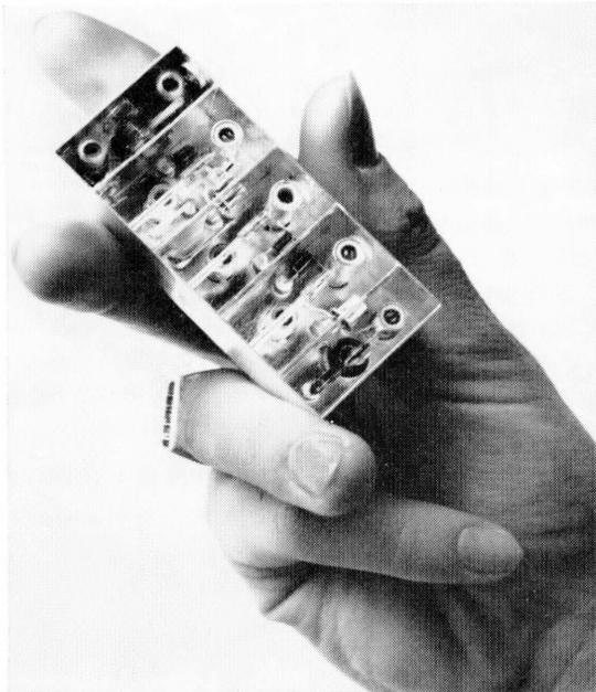
Figure 11—A television tuner using voltage-adjustable diode capacitors in *DO-7* glass mounts. The diodes may be seen in the centers of the three middle sections.
