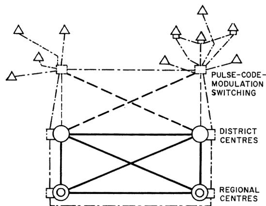
Figure 5—Typical hierarchical network showing beginnings of a national digital network which includes pulse-code-modulation switching for local tandem, toll, and pulse-code-modulation transmission and switching in long-haul backbone network.
