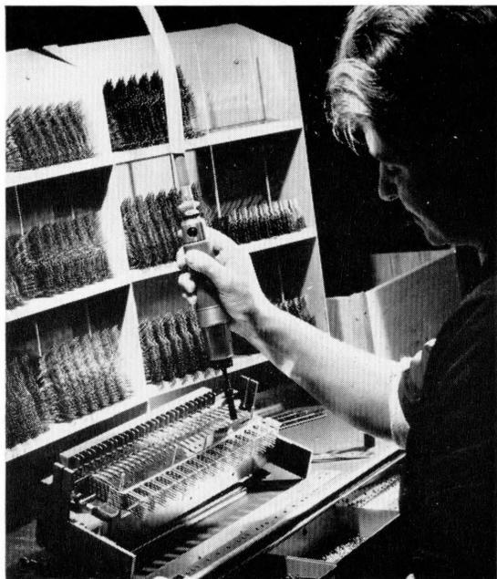
Figure 14—Operator using preset-torque pneumatic screwdriver in assembling crossbar telephone switches.
