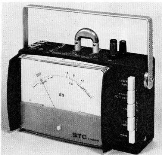
Figure 19—Milliwatt Test Set 74311-A.
