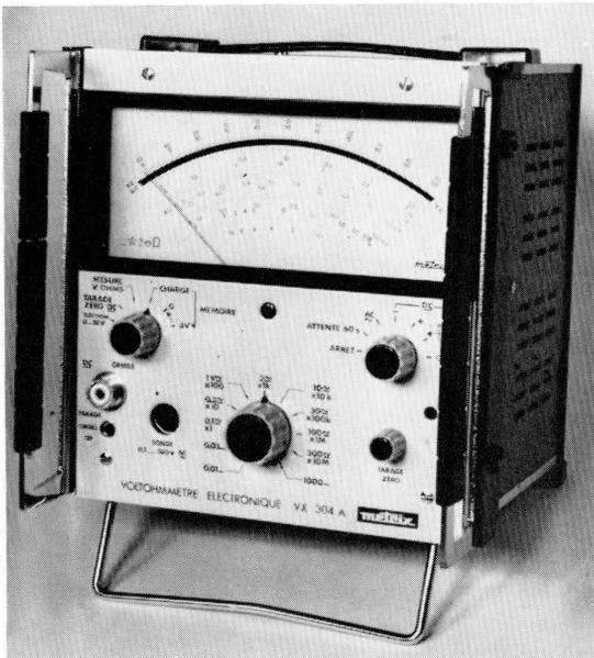
Figure 16—Electronic voltohmmeter *VX304A*.
