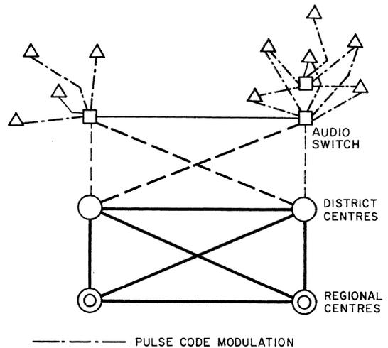
Figure 4—Typical hierarchical network showing first introductory phase in which pulse code modulation replaces physical circuits in the junction area.
