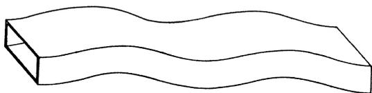
Figure 7—Sketch of periodically bent rectangular waveguide.
