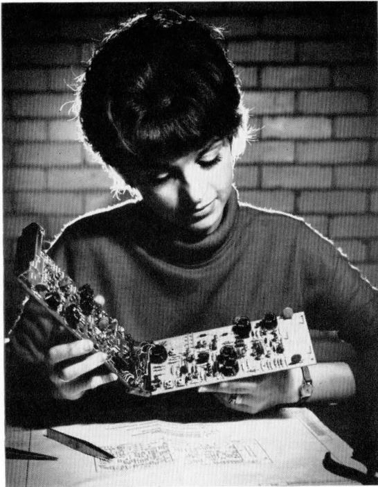
Figure 8—Complete 24-circuit 2-way repeater for pulse-code-modulation telephony.
