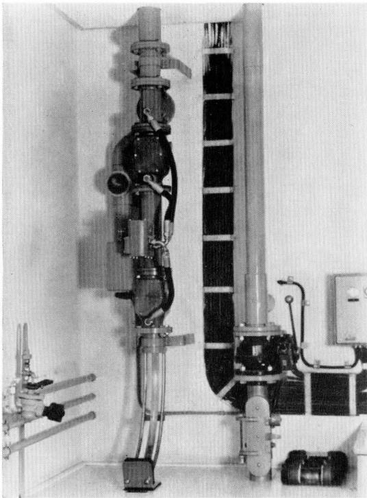
Figure 13—Transmitter (right) and receiver (left) of the long high-speed pneumatic tube system for transporting steel samples.
