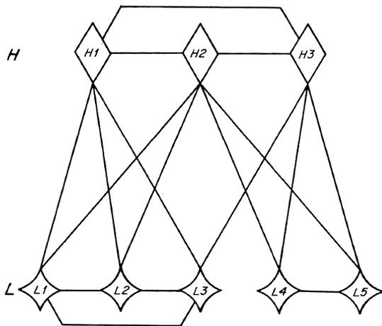
Figure 6—Computer network in which each low-level computer  $L$  is connected to two high-level computers  $H$ .
