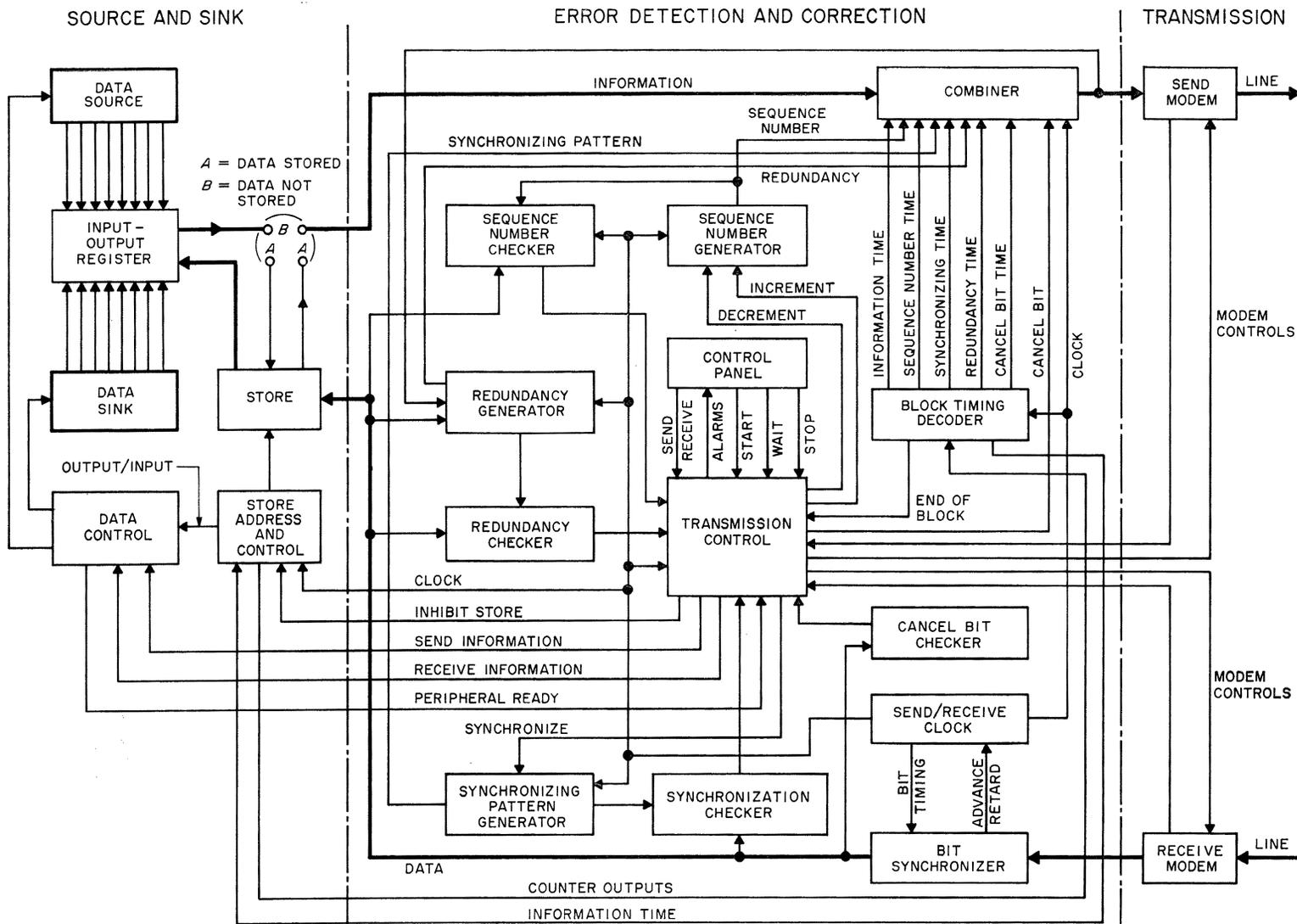
Figure 3—Block diagram of the GH 206 equipment.
