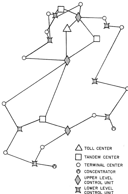
Figure 3—Remote-control network.
