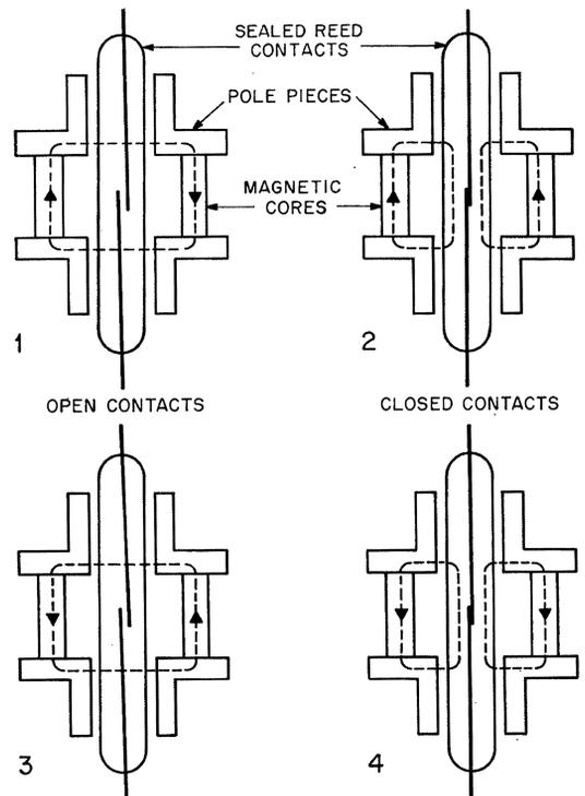
Figure 6—Of the 4 magnetic conditions shown, 2 open the reed contacts and 2 close them.
