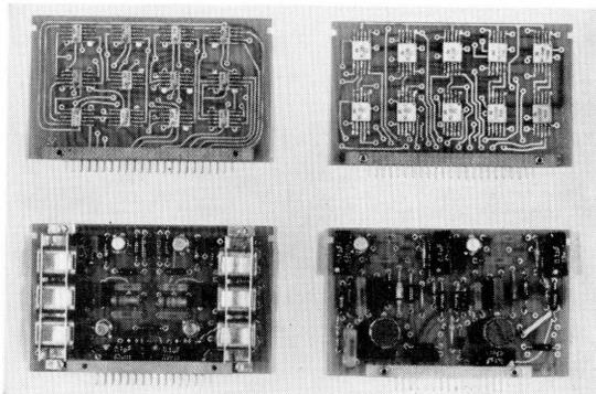
Figure 9—Sample circuit boards showing both integrated circuits and separate components.
