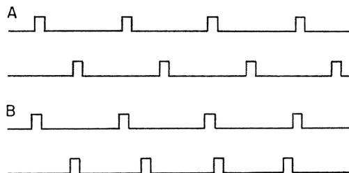
Figure 6—The pulses in the two series at *A* alternate. If as at *B* two pulses in the lower series are interpolated between two adjacent pulses in the upper series, the binary counter is stepped to change the frequency of the controlled oscillator.
