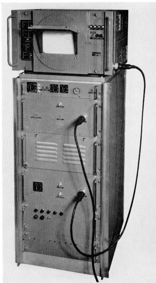
Figure 4—Equipment for the improved processing of information from a pulse coherent Doppler radar.
