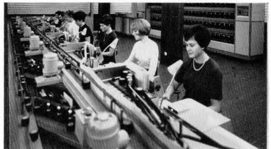
Figure 9—Coding desks in Wiesbaden postoffice for marking letters in fluorescent ink. These marks actuate electronic readers to determine the destination boxes into which the distributing machine behind the operators sorts the letters.
