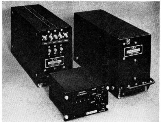
Figure 1—LMT 3527 A airborne transmitter-receiver for operation from 2 to 30 megahertz.
