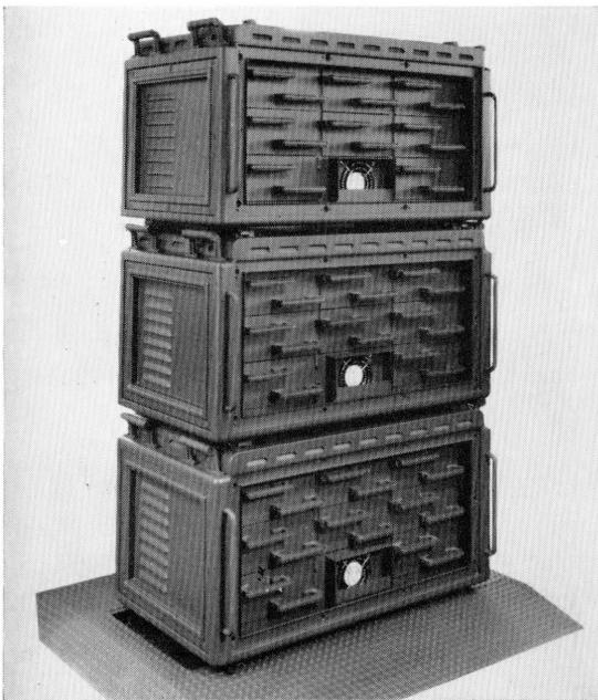
Figure 7—Front view of metal coffers in which the exchange equipment is mounted.
