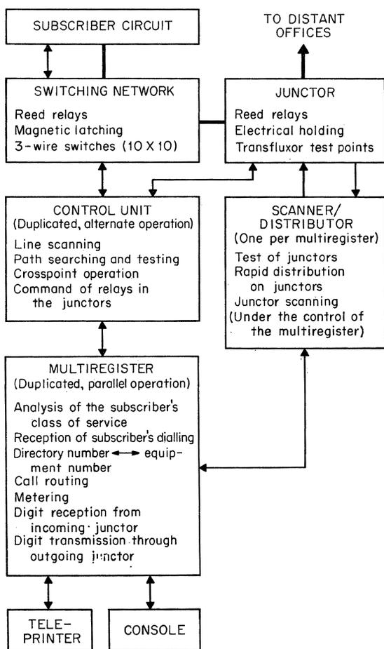
Figure 1—General arrangement of Artemis exchange.
