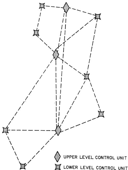
Figure 2—Control network of computers in two levels.
