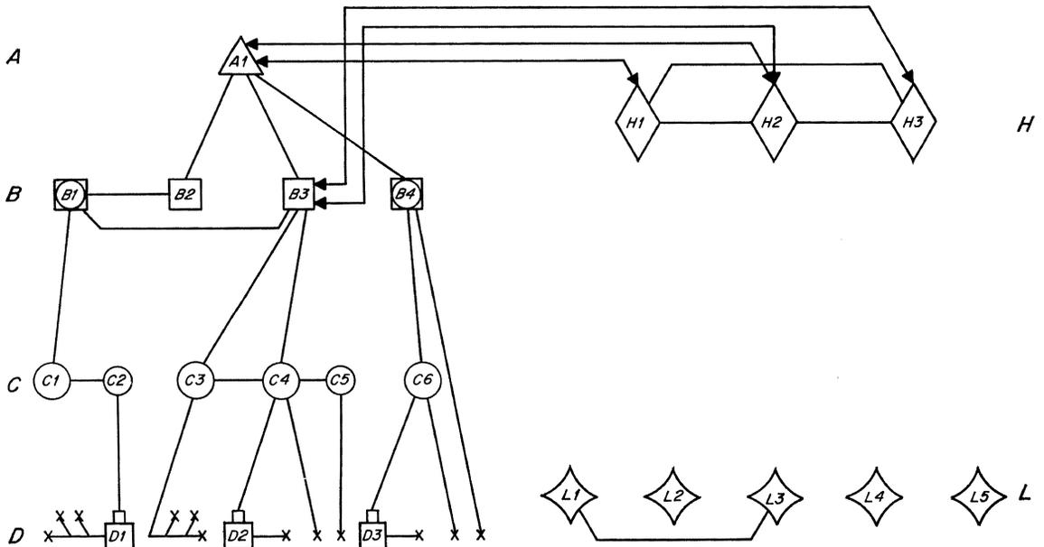
Figure 8—Control of A- and B-plane switching centers.
