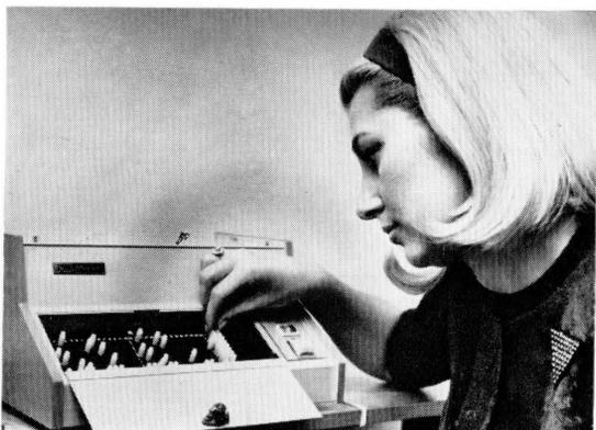
Figure 1—Cryptel 240 scrambler for commercial teletypewriter traffic uses pins in holes to determine the scrambling code. There are approximately  $2.5 \times 10^{26}$  possible settings.
