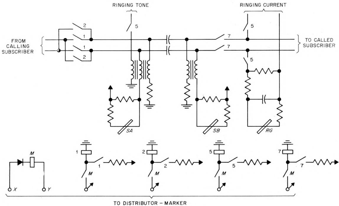
Figure 10—Principle of the local junctor.
