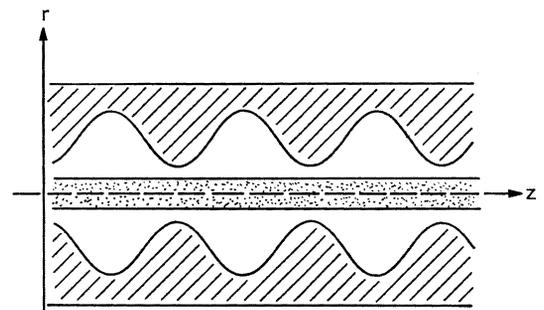
Figure 2—Longitudinal section of a traveling-wave tube having a solid electron beam, employing axially corrugated circular guide for its slow-wave structure.
