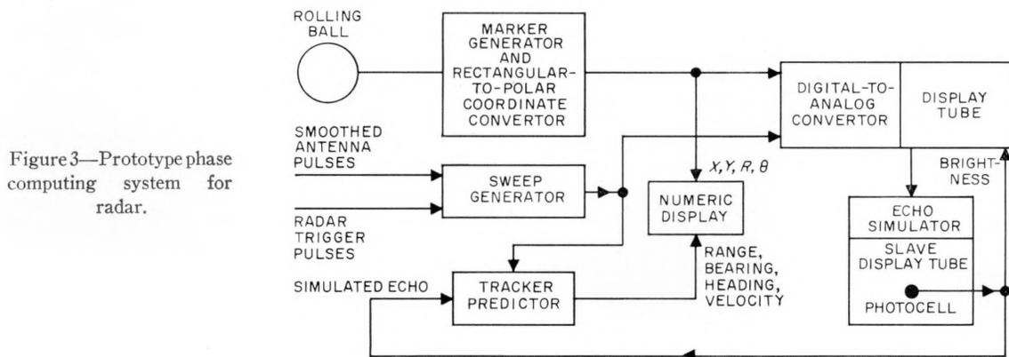
Figure 3—Prototype phase computing system for radar.
