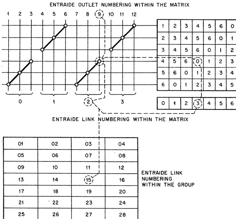
Figure 2—Entraide network details showing cyclical permutation.
