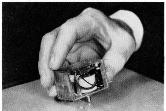
Figure 18—Type 26 relay.
