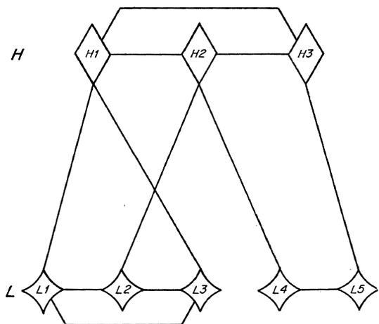
Figure 7—Computer network in which each low-level computer  $L$  is connected to only one high-level computer  $H$ . If  $H1$  fails,  $L1$  is connected to  $H2$  via  $L2$ .
