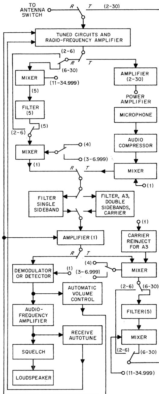
Figure 2—Transmitter-receiver diagram. Approximate frequencies are given in megahertz in parentheses. R indicates receive and T indicates transmit positions of switches.
