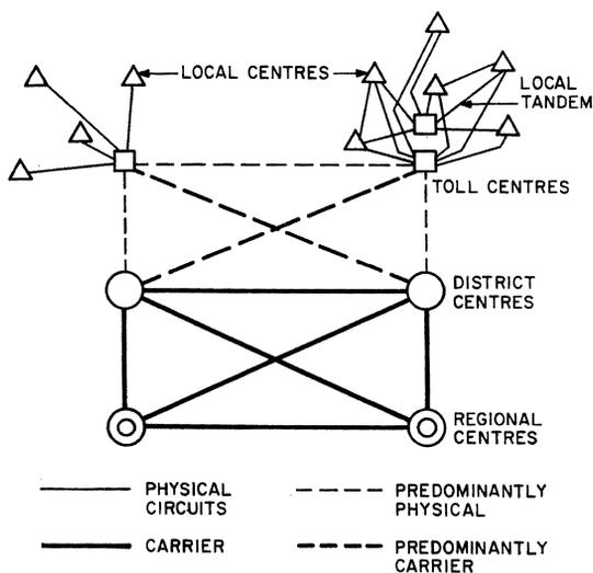
Figure 3—Typical hierarchical network.
