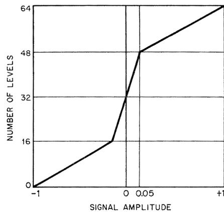
Figure 3—Compression curve of the encoder.
