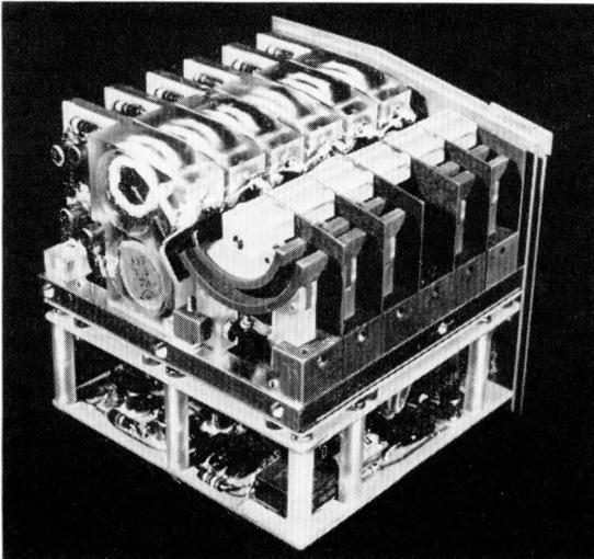
Figure 2—High-voltage generator and particle detector for *ESRO 1*.
