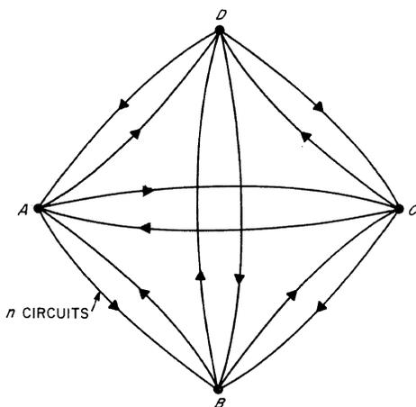
Figure 2—Simple 4-exchange network.
