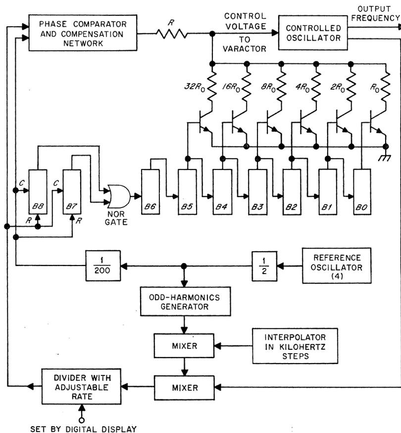
Figure 5—Method of adjusting the controlled oscillator.
