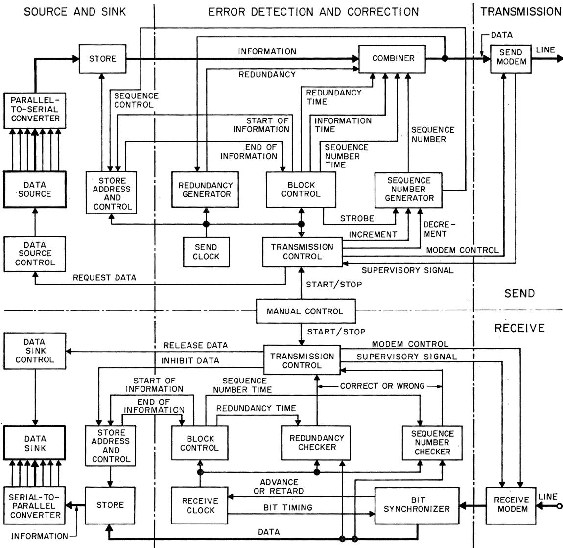
Figure 1—Block diagram of the GH 205 equipment.
