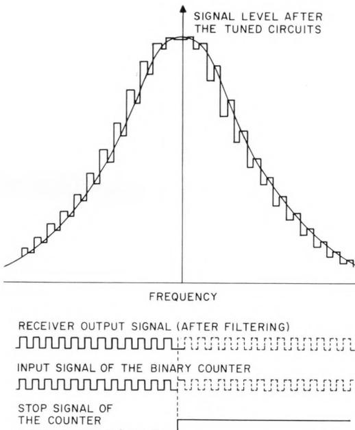
Figure 7—Varactor method of tuning the input receiver circuits to the desired signal frequency.
