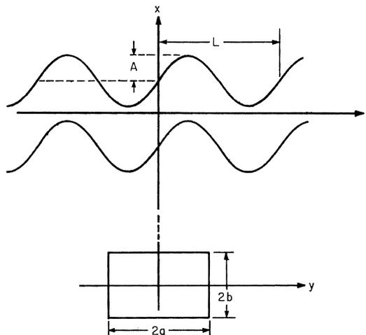
Figure 8—Longitudinal and cross sections of bent guide, showing the period  $L$  and amplitude of bending  $A$ . The dimensions of a cross section are  $2a$  and  $2b$ .
