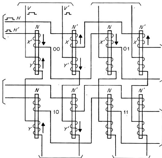
Figure 7—The pulses operating crosspoint  $00$  will open all other crosspoints in the vertical and horizontal coordinates of  $00$ .
