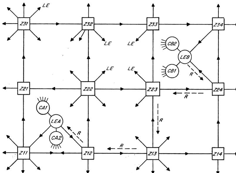
Figure 1—A typical mesh network having transit or zone exchanges  $Z$  at the nodes to which local exchanges  $LE$  are connected. Concentrators  $CA$  and  $CB$  are connected to the local exchanges.
