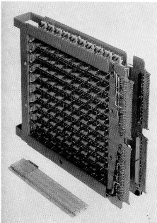
Figure 8—Plug-in drawer accommodating 100 crosspoints in a 10 by 10 array.
