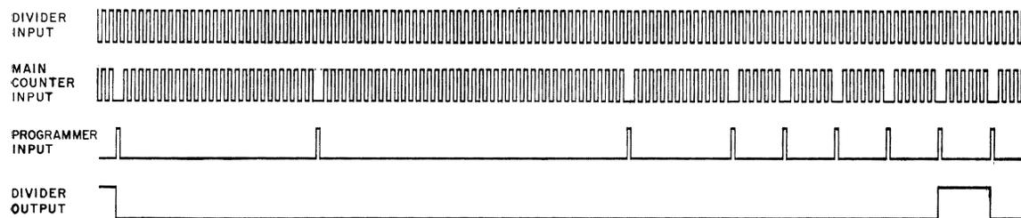
Figure 4—Waveforms in the adjustable divider.
