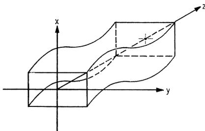
Figure 9—Sketch of bent guide referred to rectangular coordinates  $x, y, z$ . Parametric equations of the upper and lower faces are  $x = \pm b + A \sin (2\pi/L)\zeta, y = \eta, z = \zeta$ .
