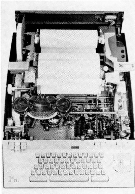
Figure 2—Teleprinter with silencing cover removed.
