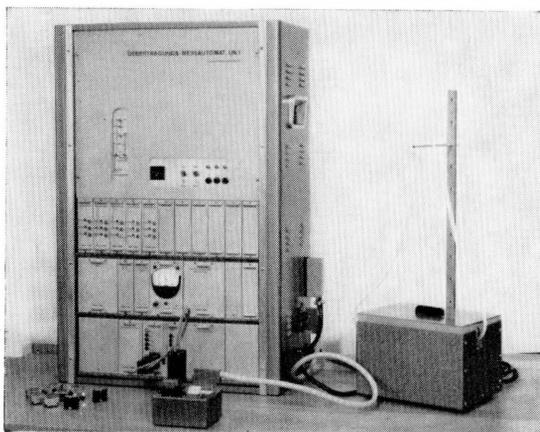
Figure 14—Automatic transmission test set UN2. To the right is the perforated tape reader; in front, the adapter with plug-in socket for the samples; and to the left are some samples.
