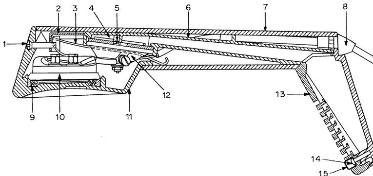
Figure 3—Sectional view of the handset.
