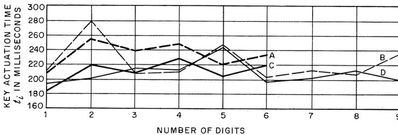
Figure 7—Arithmetic mean values of the key actuation times. Curves *A* and *B* were measured in 1964; they represent 7259 and 3188 key depressions, respectively. Curves *C* and *D* were measured in 1965 and represent 13 670 and 7259 key depressions.
