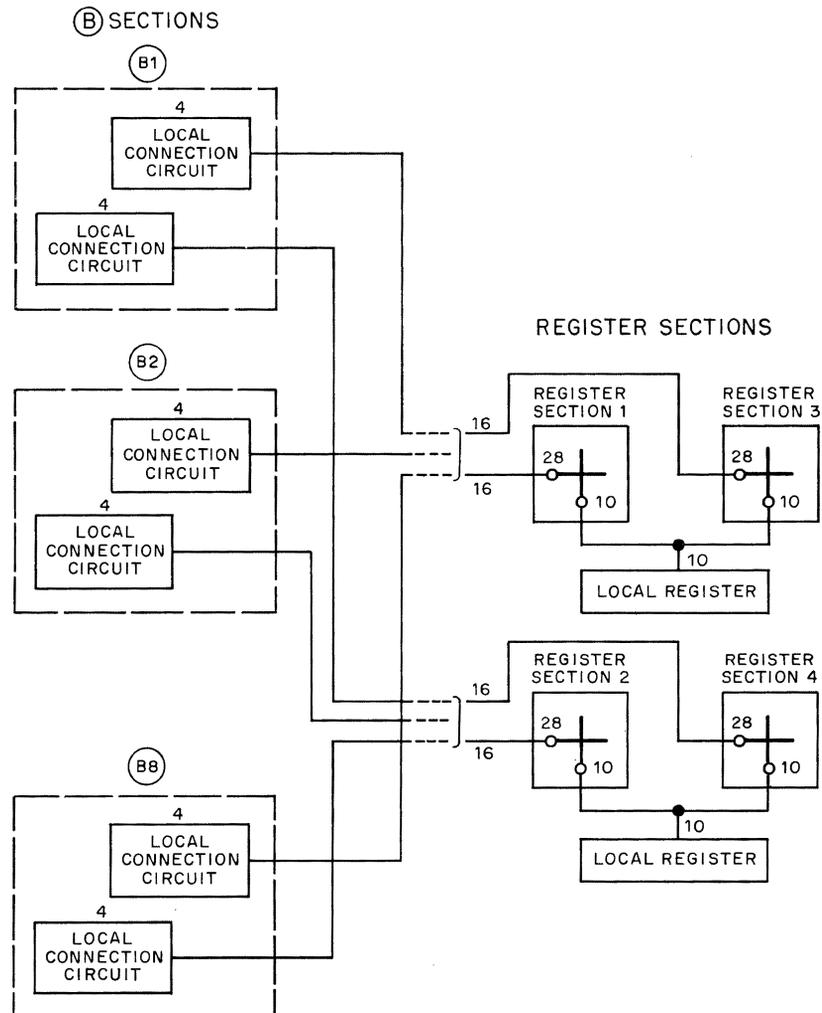
Figure 3—Access of local connecting circuits to local register circuits.
