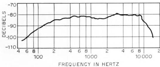
Figure 7—Response of the 4124 lavalier microphone. 0 decibels = 1 volt per dyne per square centimetre.
