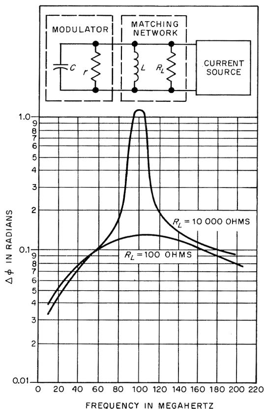
Figure 5—Performance characteristics of transverse-field modulator.  $L = 0.12$  microhenry and  $P_T = 5$  watts.
