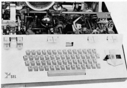
Figure 8—Machine with automatic shift to letters and figures.
