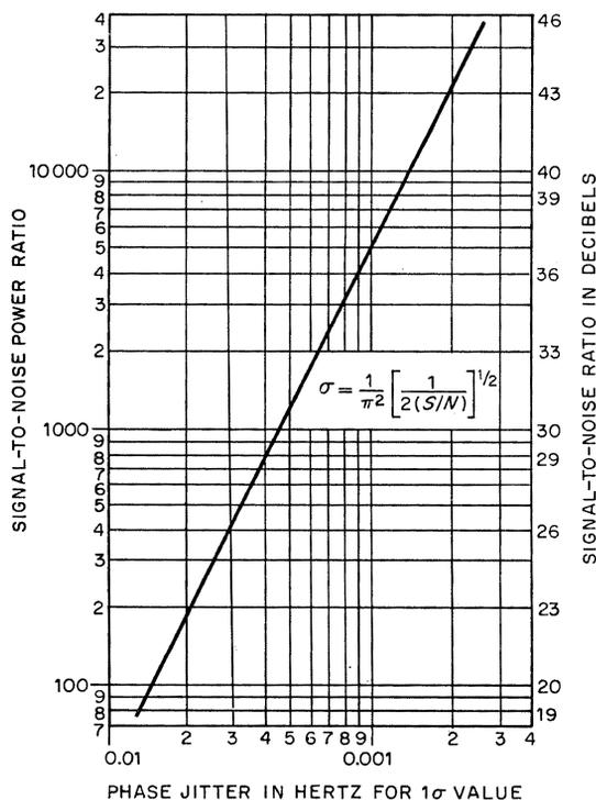
Figure 9—Phase jitter versus signal-to-noise ratio.
