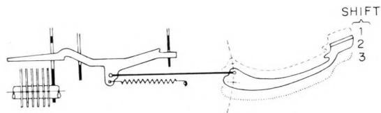
Figure 7—Shifting on the type basket.
