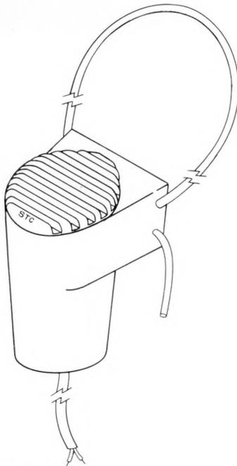
Figure 6—Type 4124 miniature lavalier moving-coil microphone.
