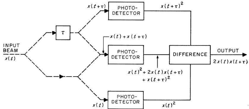
Figure 14—Optical autocorrelator with local modulator.
