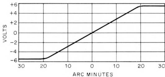
Figure 10—Error signal characteristics expanded at null.
