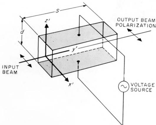
Figure 2—Electro-optical modulator using transverse field.
