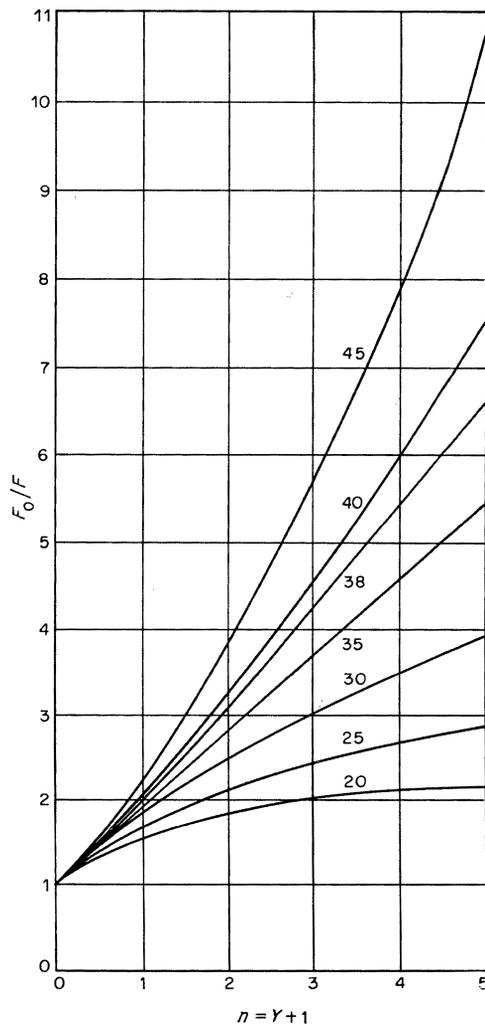
Figure 7—Transition frequency ratio versus class overlapping for values of  $X$  indicated on the curves.  $F$  = transition frequency,  $F_0$  = transition frequency for  $n = 0$  (disjoint classes),  $N = 50$ ,  $a = 37.90$  erlangs,  $B = 0.01$ , and  $h = 180$  seconds.
