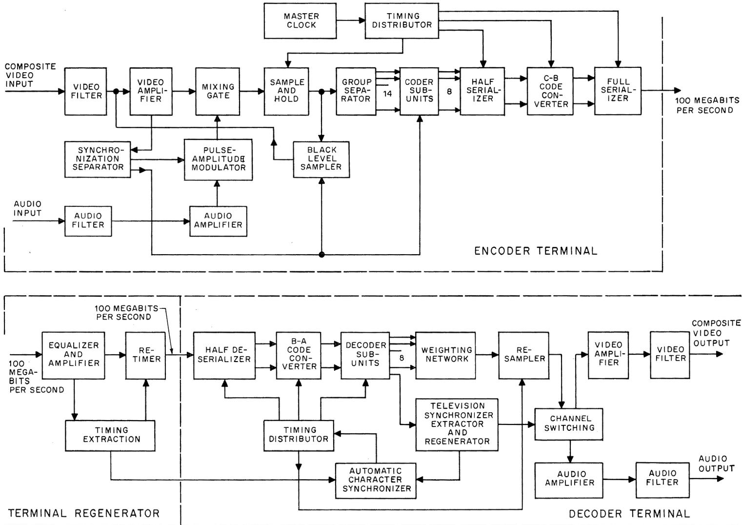
Figure 1—Schematic diagram of 81-level pulse-code-modulation system.
