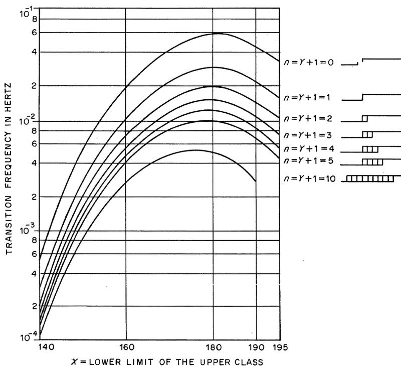
Figure 3—Average transition frequency versus occupation class limits.  $N = 200$ ,  $a = 179.74$  erlangs,  $B = 0.01$ , and  $h = 180$  seconds.
