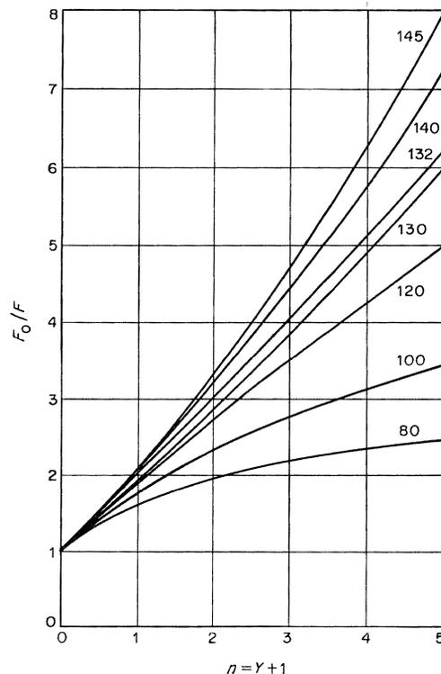
Figure 5—Transition frequency ratio versus class overlapping for values of  $X$  indicated on the curves.  $F$  = transition frequency,  $F_0$  = transition frequency for  $n = 0$  (disjoint classes),  $N = 150$ ,  $a = 131.58$  erlangs,  $B = 0.01$ , and  $h = 180$  seconds.
