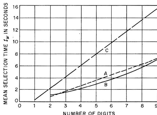
Figure 10—Mean selection times  $t_w$ . Curves A (1964) and B (1965) are for push-button selection, while curve C is for dial selection.
