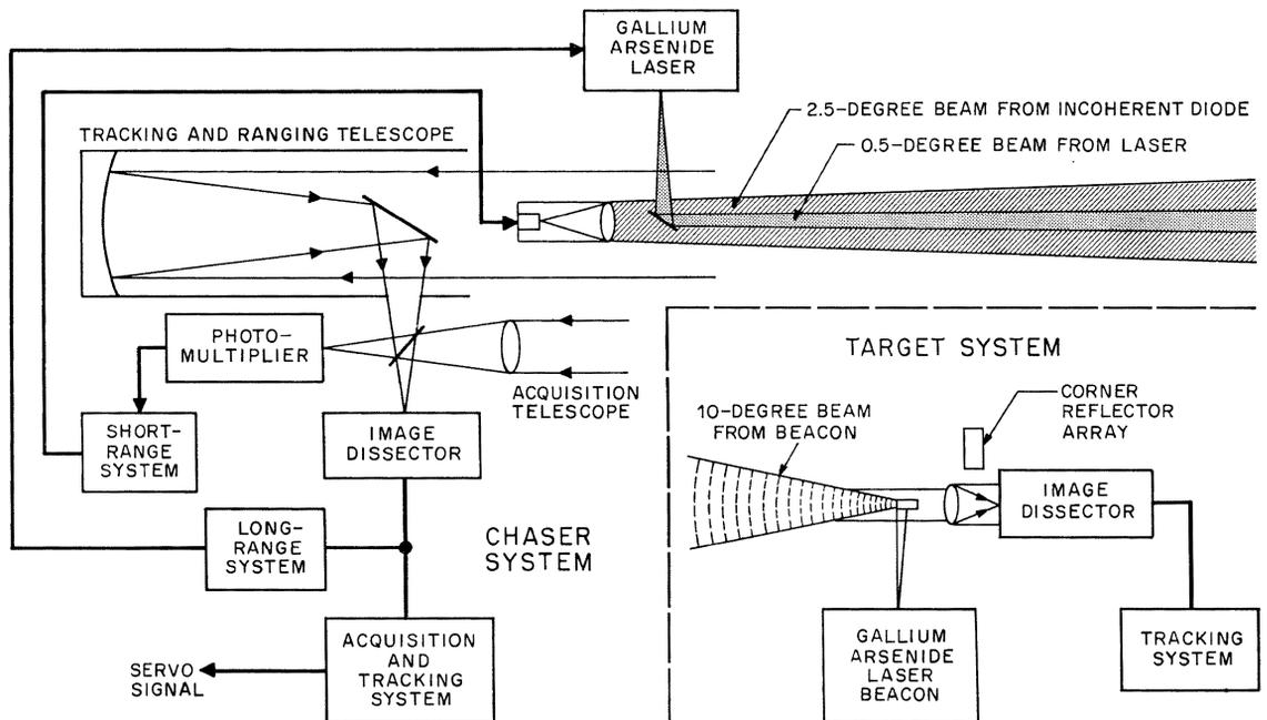
Figure 12—Diagram of rendezvous guidance system.
