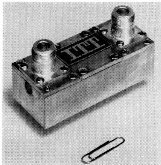
Figure 3—Transverse-field modulator.
