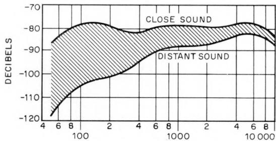
Figure 9—Response of the 4115 microphone to close and distant sound.
