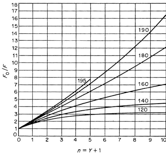
Figure 4—Transition frequency ratio versus class overlapping for values of  $X$  indicated on the curves.  $F$  = transition frequency,  $F_0$  = transition frequency for  $n = 0$  (disjoint classes),  $N = 200$ ,  $a = 179.74$  erlangs,  $B = 0.01$ , and  $h = 180$  seconds.
