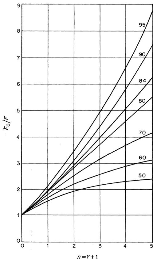
Figure 6—Transition frequency ratio versus class overlapping for values of  $X$  indicated on the curves.  $F$  = transition frequency,  $F_0$  = transition frequency for  $n = 0$  (disjoint classes),  $N = 100$ ,  $a = 84.06$  erlangs,  $B = 0.01$ , and  $h = 180$  seconds.
