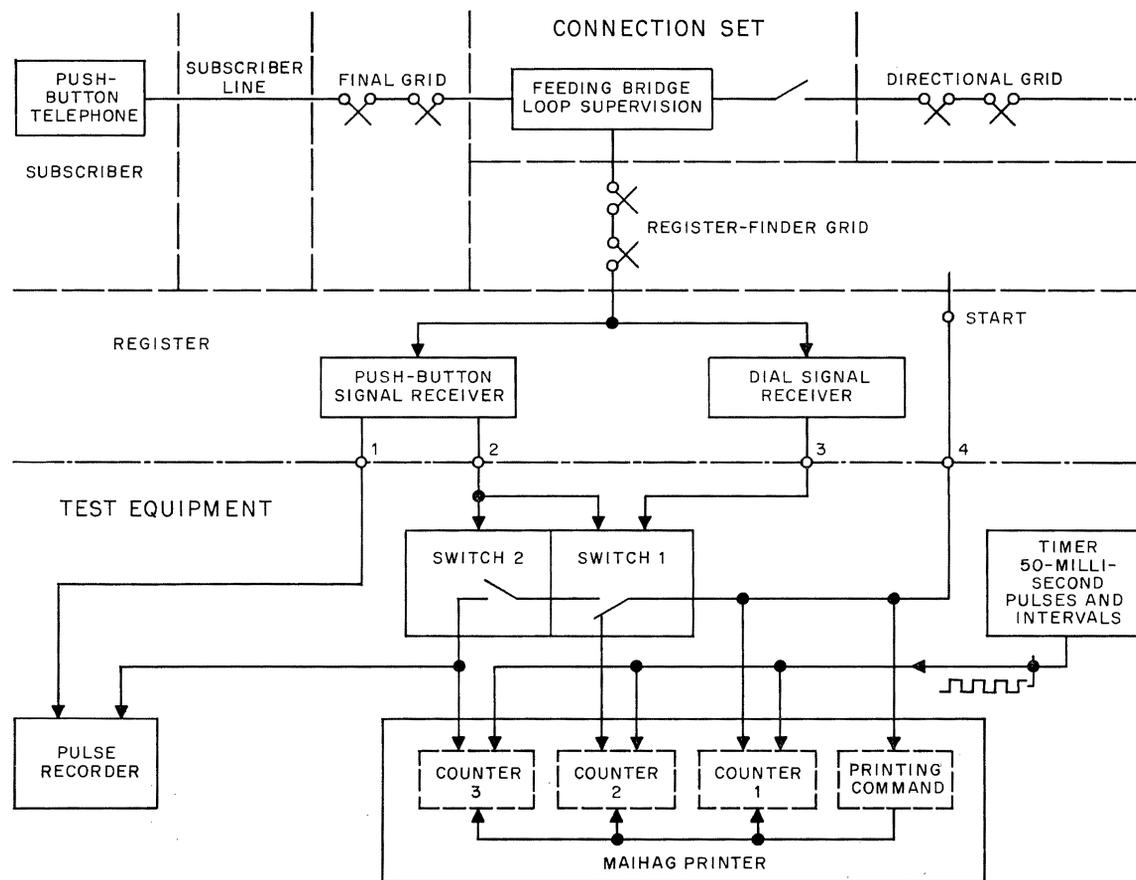
Figure 2—Block diagram of the test setup.
