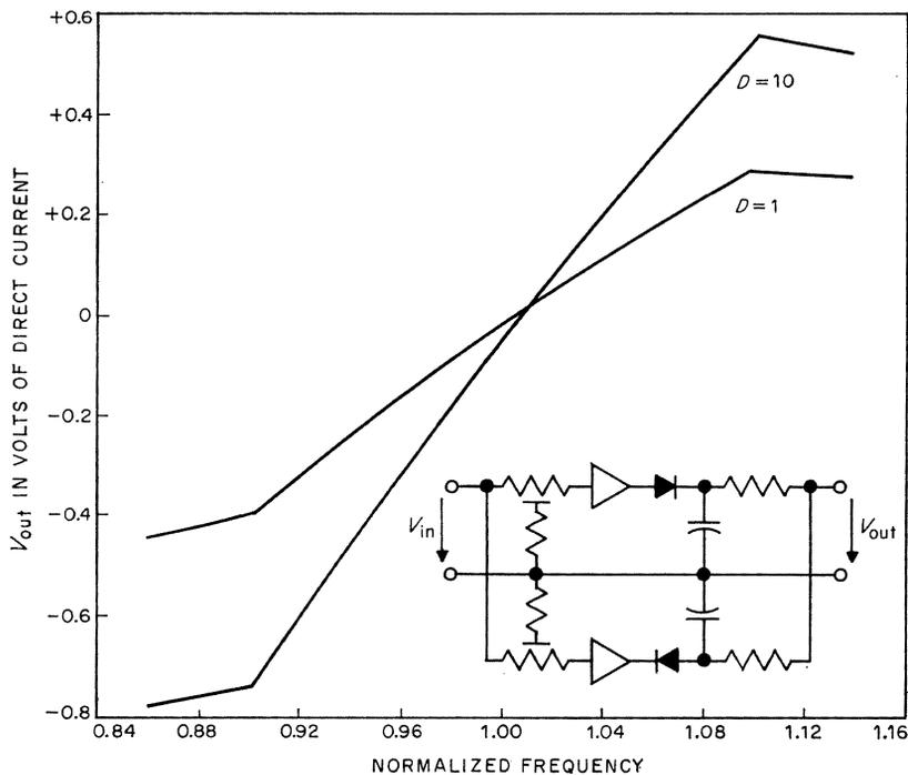
Figure 15—Frequency-modulation discriminator for wideband demodulation using two thin-film distributed resistance-capacitance null networks.  $D$  is the ratio of the width of the resistive film at the input and output of the network. The amplifiers have gains of 20 decibels and the input signal is 1 volt, root mean square.
