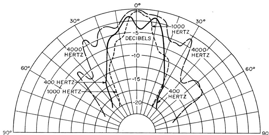
Figure 11—Polar response characteristics of column loudspeaker.
