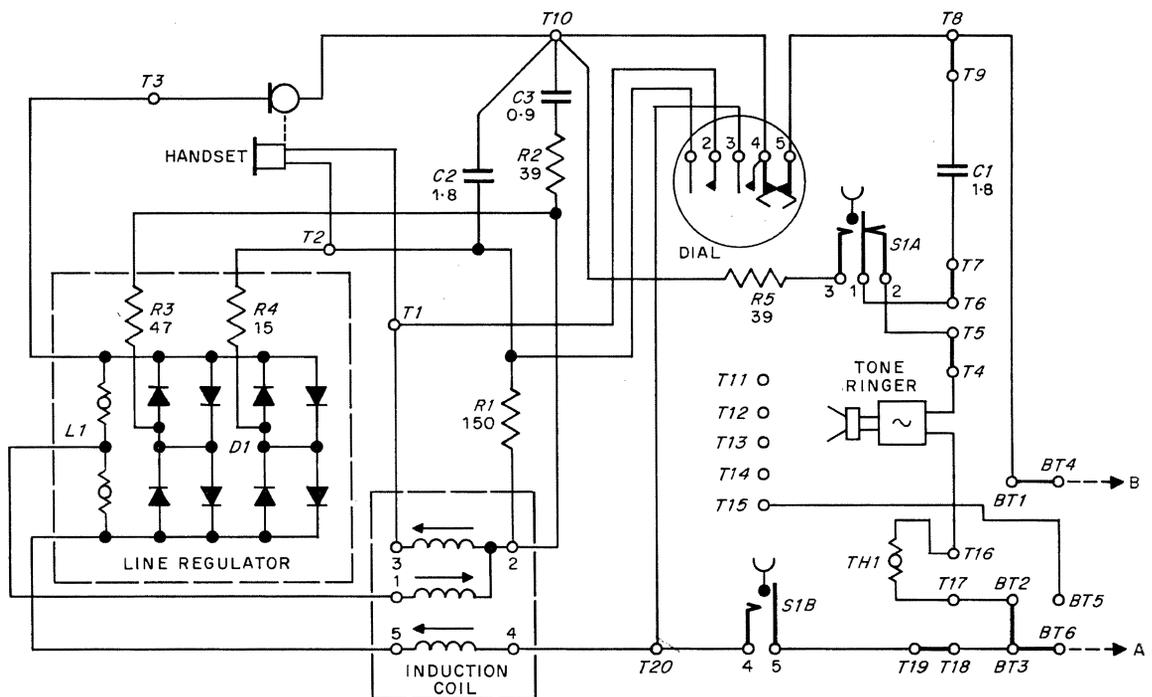
Figure 4—Transmission circuit. Values of resistance are in ohms and of capacitance in microfarads.
