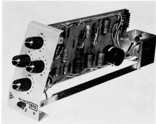
Figure 12—A microphone amplifier built into a single-width module unit. The method of construction combines adequate rigidity with ease of access for servicing.
