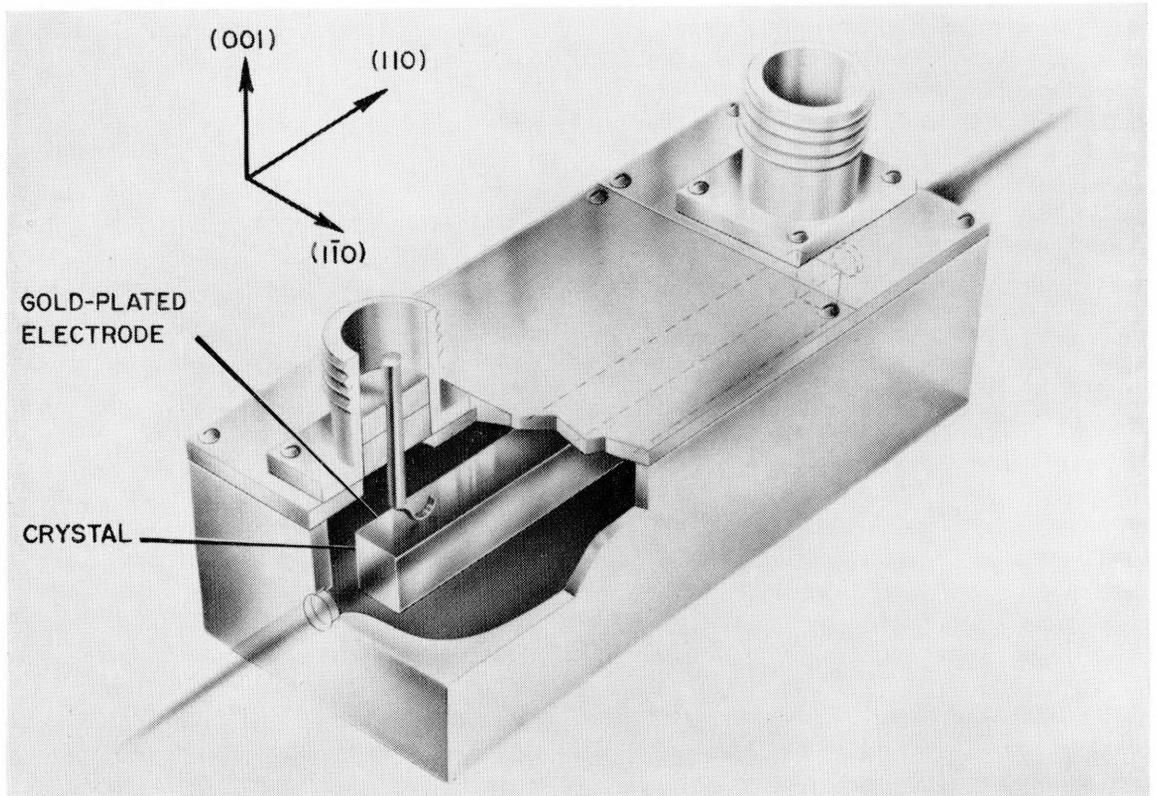
Figure 4—Internal arrangement of transverse-field modulator.
