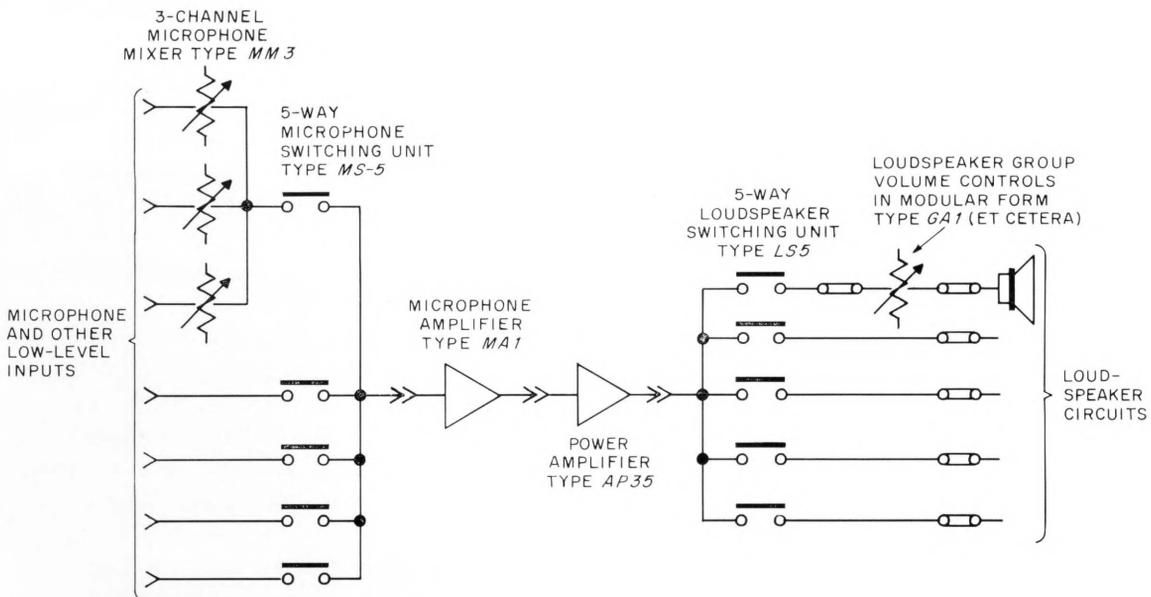
Figure 13—Diagram of a sound system engineered from standard elements of the modular public-address equipment.
