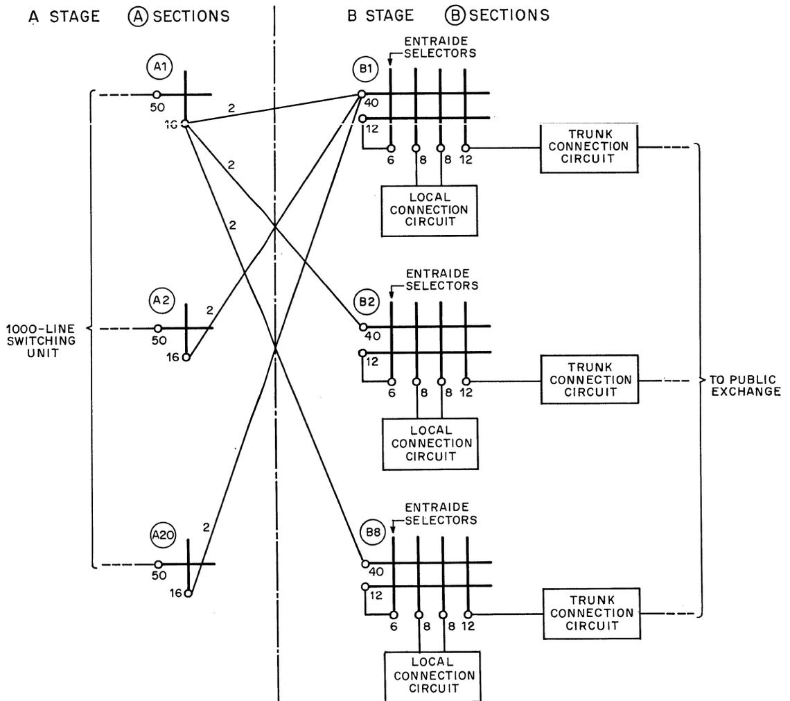
Figure 2—Link arrangement for 1000-line switching units.
