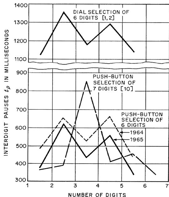
Figure 9—Arithmetic mean values of interdigit pauses  $t_p$ .
