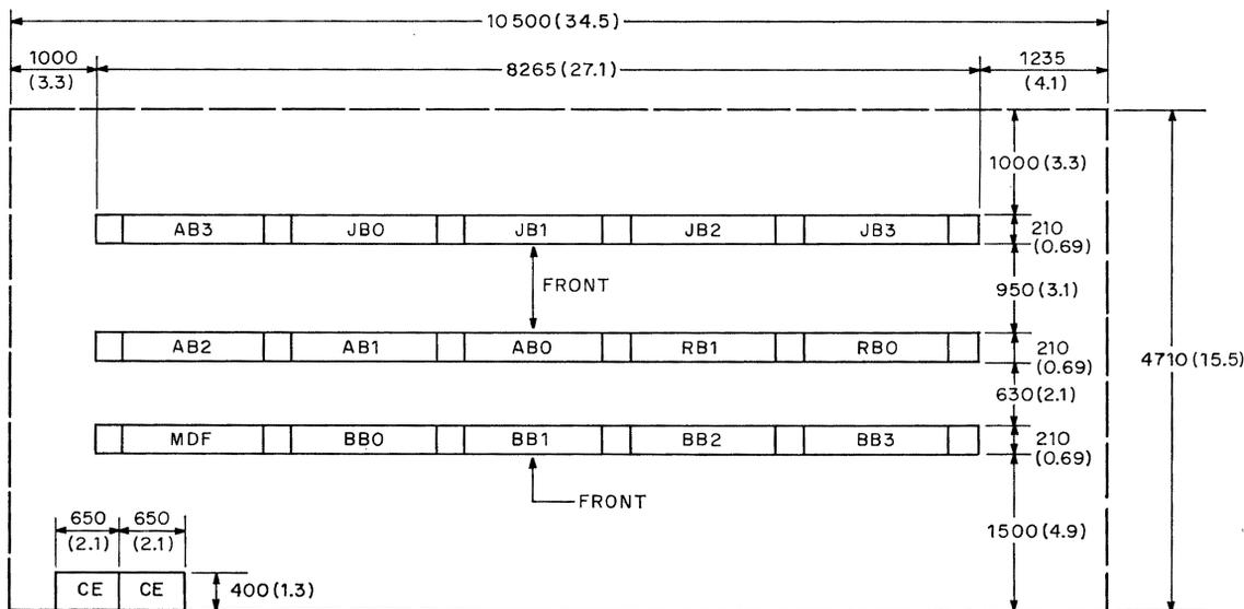
Figure 1—Floor plan for 1000-line exchange with 72 trunks and 64 local connecting circuits using fixed frames 2.81 meters (9.2 feet) high and weighing approximately 450 kilograms per running meter (300 pounds per running foot). Dimensions are in millimeters (feet). The functions of the frames are as follows:
