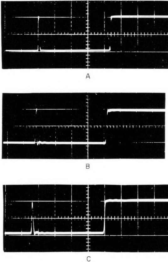
Figure 3—Pulse and bar response. *A* is the input, *B* the output of the encoder drive amplifier working into a resistive load, and *C* is the final output. The horizontal scale is 2 microseconds per division.
