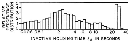
Figure 4—Percentage distribution of inactive holding times (failure to call after lifting handset) for 2977 seizures. There were 34.4 percent under 0.4 second and the 9.1 percent above 20 seconds corresponds to automatic forced release of the register for failure to call. Class width = 12 percent.
