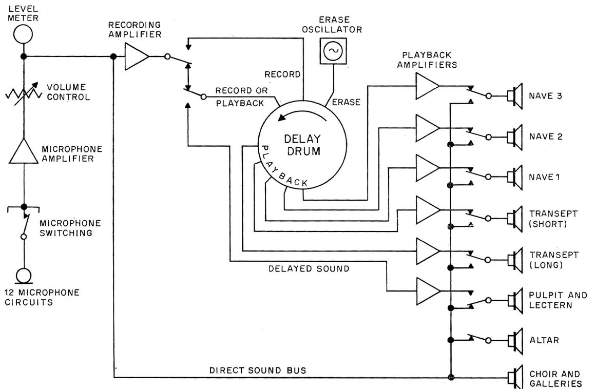
Figure 17—Layout of magnetic-drum delay unit.
