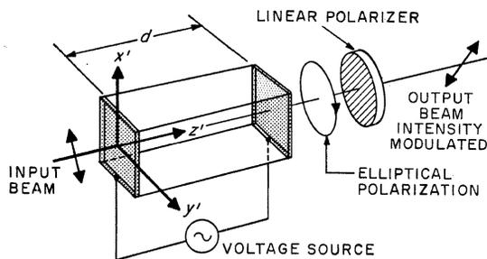
Figure 1—Electro-optical modulator using longitudinal field.
