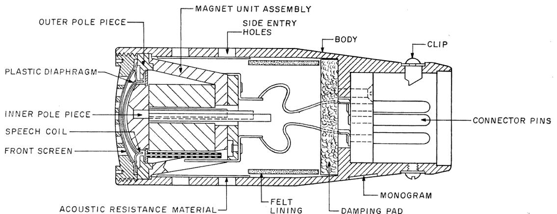
Figure 1.—Type 4105 unidirectional moving-coil microphone.
