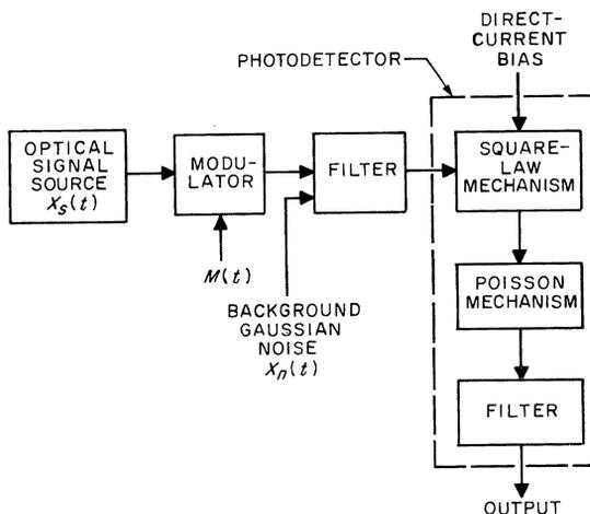
Figure 6—Model for deriving signal-to-noise ratio. The output power density spectrum includes signal  $\times$  signal, signal  $\times$  noise, noise  $\times$  noise, and shot noise caused by optical inputs and direct-current potentials.
