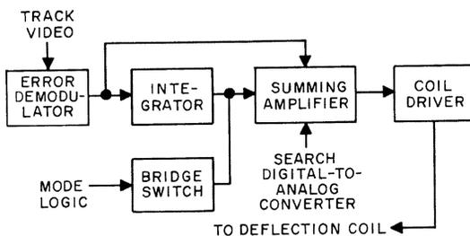
Figure 8—Single channel of tracking loop control circuits.
