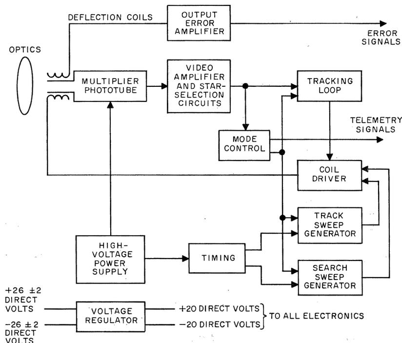
Figure 2—Block diagram of fine-guidance sensor.
