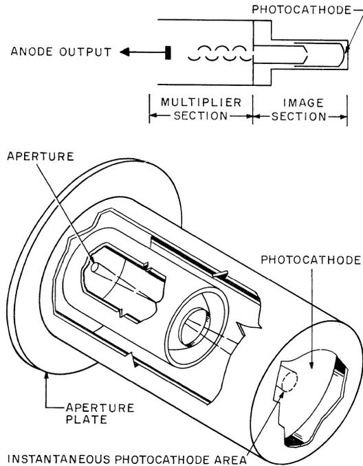
Figure 3—Multiplier phototube.
