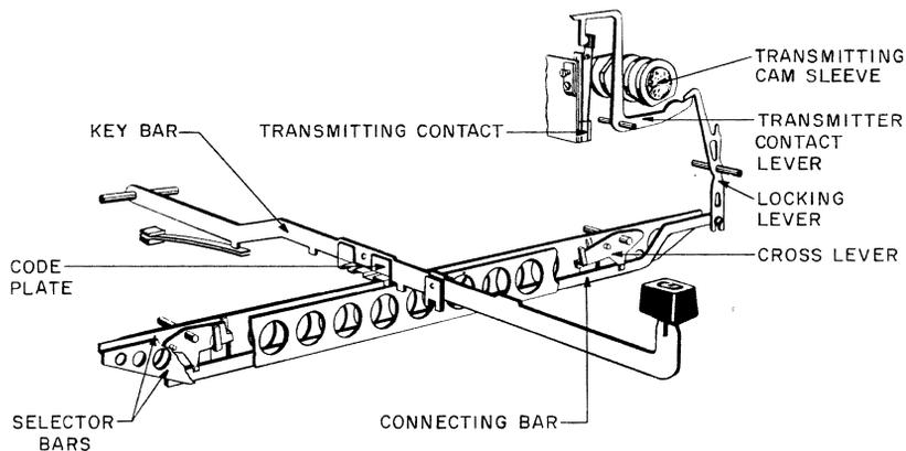
Figure 4—Principles of coding.
