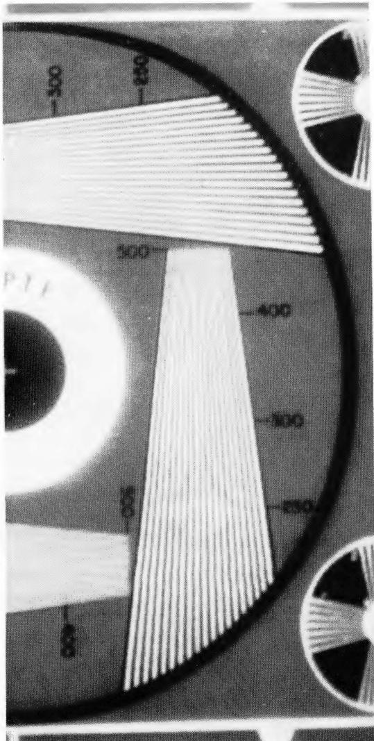
Figure 2—Part of test card of Society of Motion Picture and Television Engineers after transmission through a pulse-code-modulation system. Exposure is 1/15 second.
