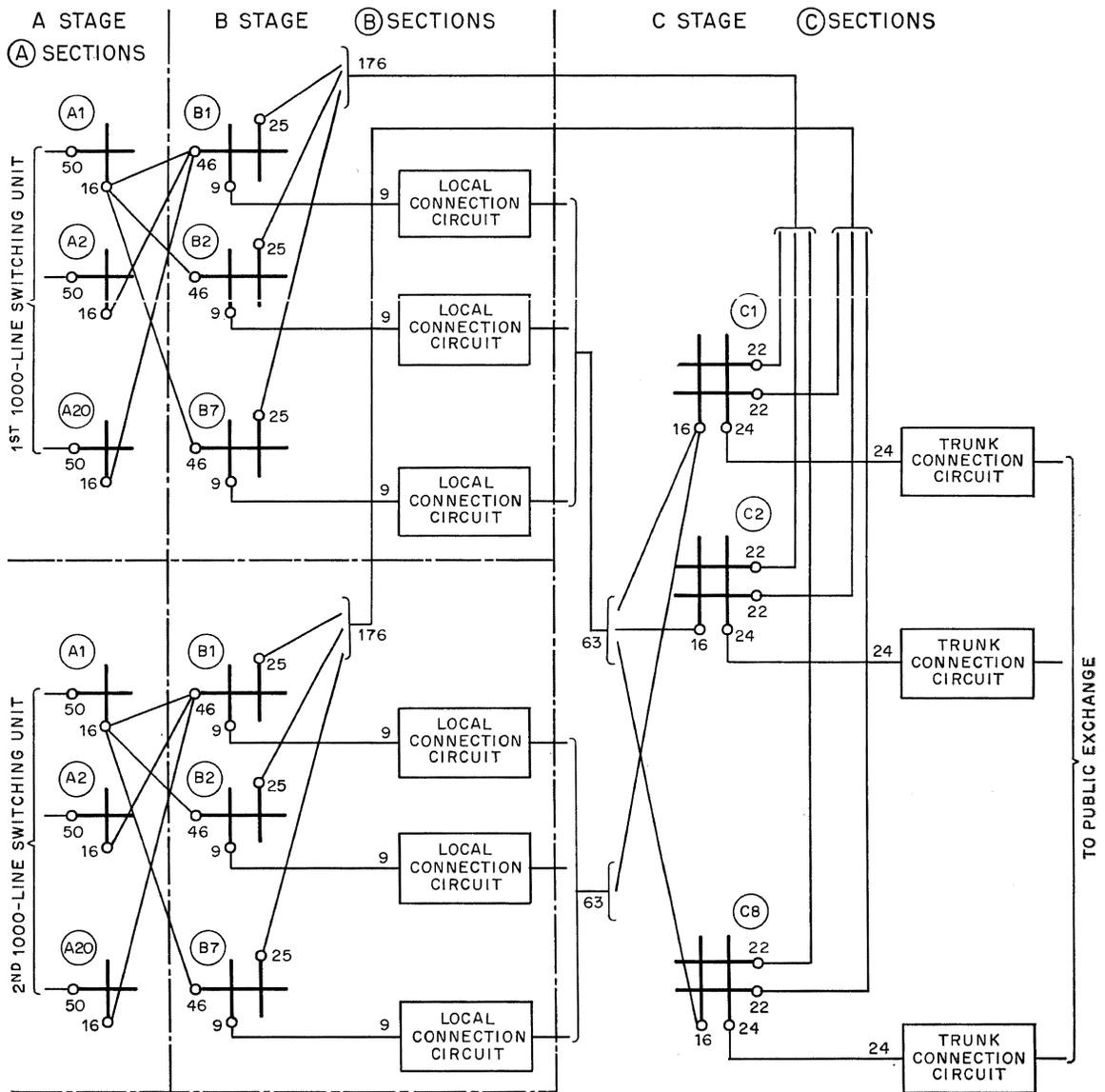
Figure 5—Link system arrangement for 2000-line conjugate switching unit.
