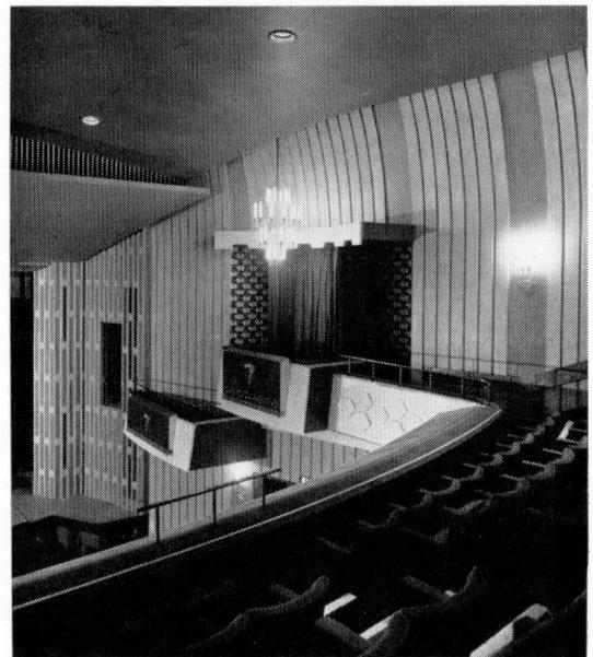
Figure 15—Column loudspeakers built into proscenium arch.
