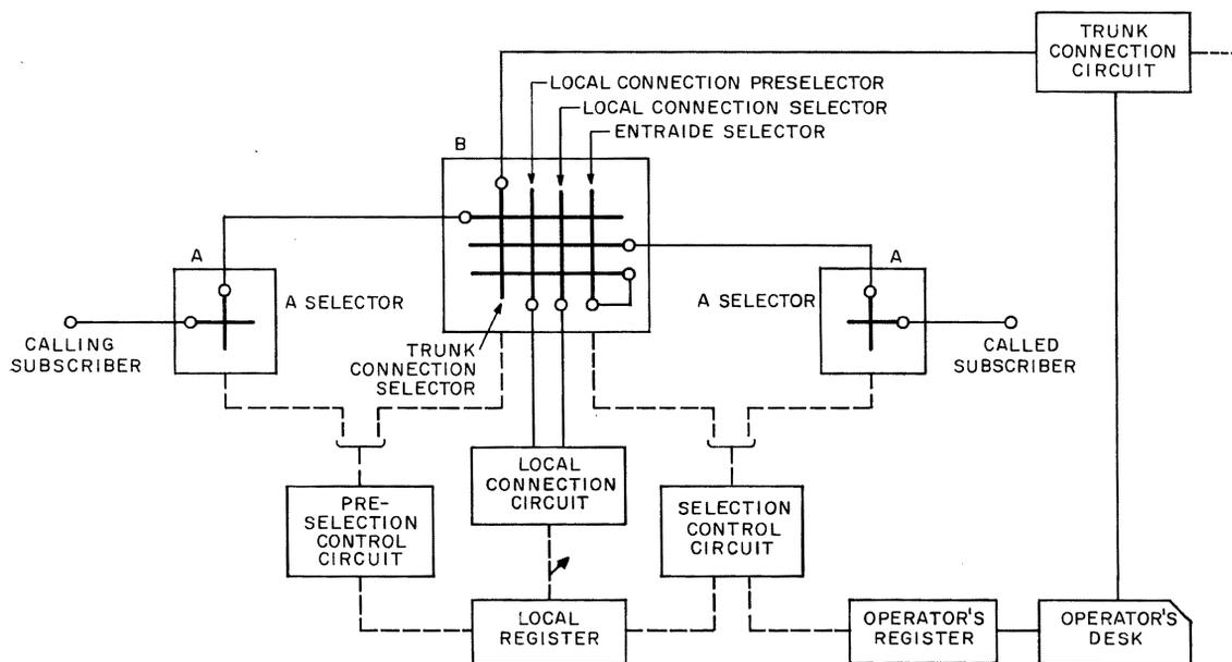
Figure 4—Simplified junction diagram for 1000-line switching unit.
