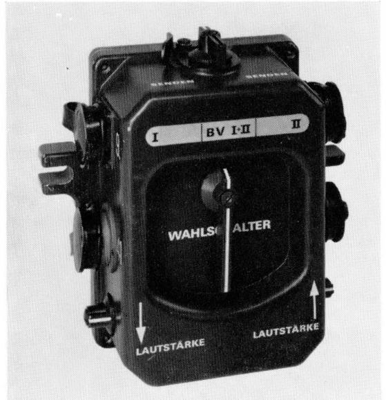
Figure 14—Intercommunication control unit.
