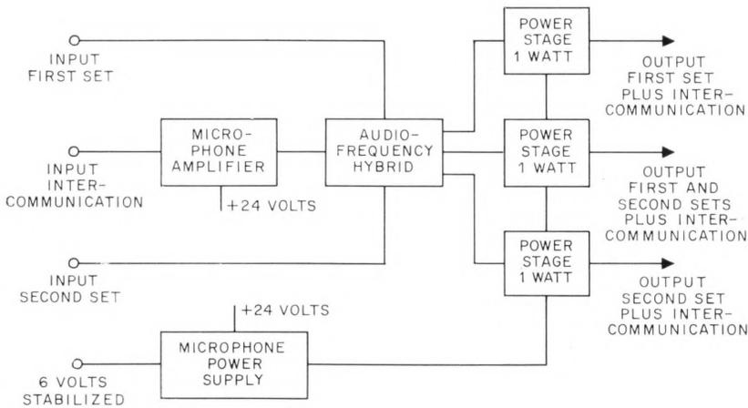
Figure 12—Intercommunication-amplifier arrangement.
