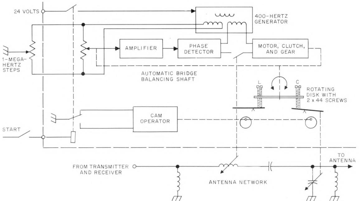
Figure 3—Antenna tuning unit. Adjustment for each of 44 steps of 1-megahertz each is by 2 screws that control the adjustable inductor and capacitor in the antenna network. The cams push the arms away from these setscrews and close the switch to the motor when the disk is to be rotated for a new channel.
