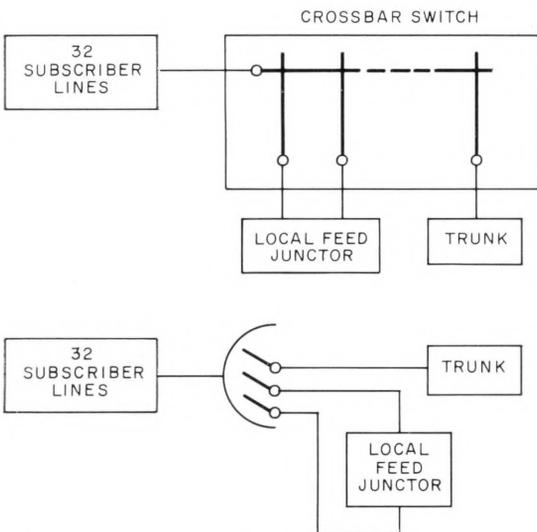
Figure 2—Single-stage version of primary switch.
