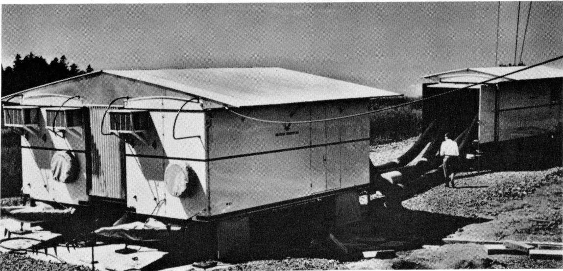
Figure 3—Mobile television transmitter.
