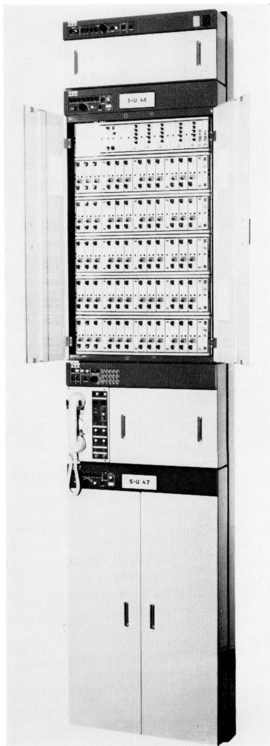
Figure 2—Multiplex telephone equipment for a 120-channel supergroup.
