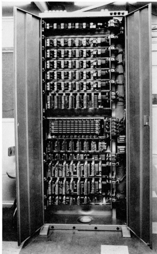
Figure 3—Small rural exchange with 32 subscriber lines connected.
