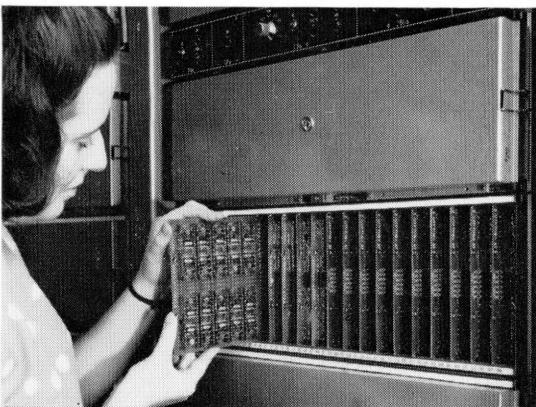
Figure 19—All parts are mounted on plug-in cards, and Minibell type paraplate modules are used.
