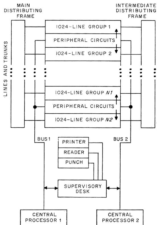
Figure 1—Modular network and central control of 10-CX system.
