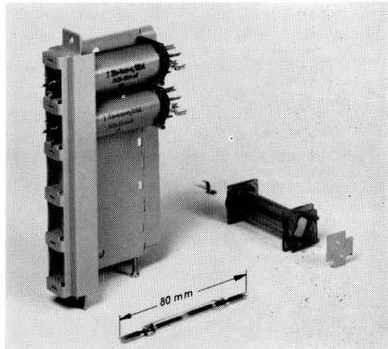
Figure 7—The coil form at the right holds 2 of the 80-millimeter (3.1-inch) reed-contact elements. A crosspoint strip to hold 5 complete reed switches is also shown.
