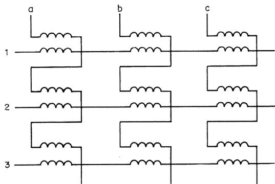
Figure 3—Crosspoint matrix using linear addition of electromagnetic energy distributed to two coordinate directions.
