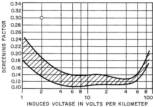
Figure 9—Production-control screening-factor curves for 1.2-millimeter 27-quad cables at 16 $\frac{2}{3}$  hertz (1.3-millimeter aluminum sheath). Refer to Table 4.
