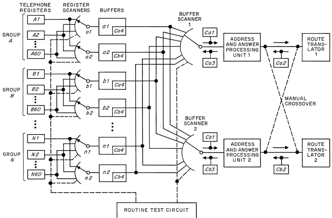
Figure 18—Block diagram of number analyzer.
