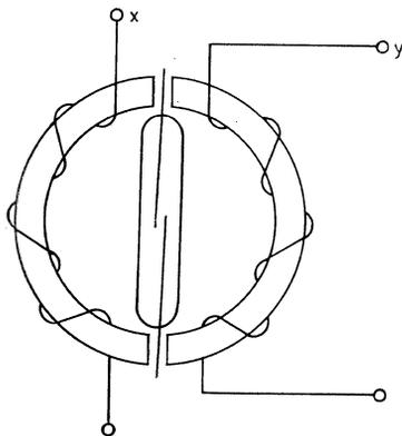
Figure 5—Principal structure of the ferreed.
