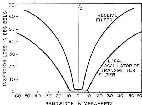
Figure 3—Insertion loss of waveguide filters as a function of bandwidth.
