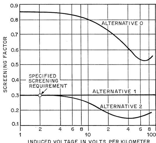
Figure 4—Calculated screening-factor curves of alternatives 0, 1, and 2 for 1.2-millimeter 27-quad cable at  $16\frac{2}{3}$  hertz. Refer to Table 3.
