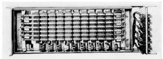
Figure 1—Crossbar switch used in Pentaconta 32 telephone switching system.
