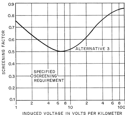
Figure 5—Measured screening-factor curve of alternative 3 for 1.2-millimeter 27-quad cable at 16 2/3 hertz.
