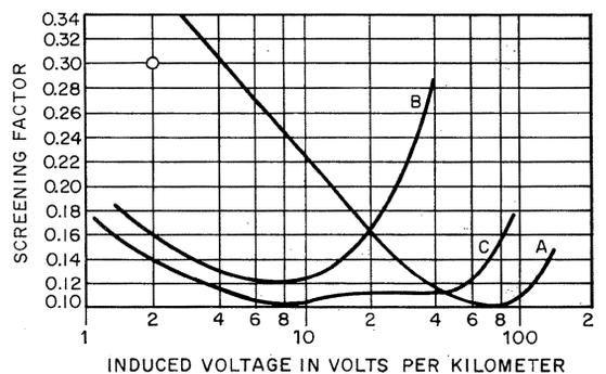
Figure 6—Measured screening-factor curves on hand-made samples of 1.2-millimeter 27-quad cable at 16 2/3 hertz. Refer to Section 3.2.
