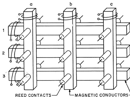
Figure 2—Crosspoint matrix with simple linear addition of the actuating energy distributed to two coordinate directions.
