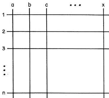
Figure 1—Crosspoint matrix with  $n$  inputs and  $x$  outputs.
