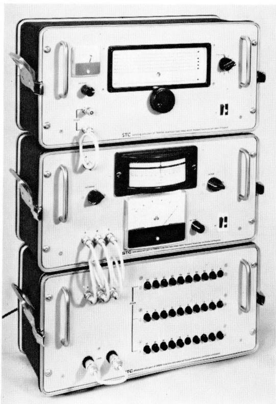
Figure 13—Insertion-loss measuring equipment type 74905.
