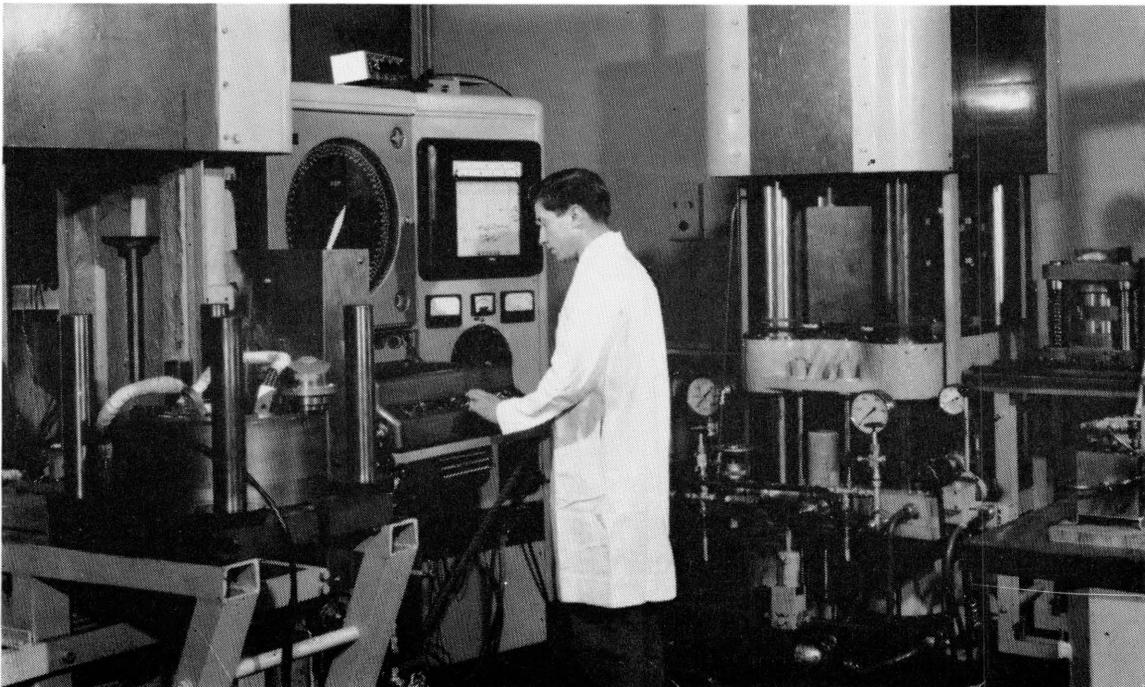
Figure 7—Tetrahedral anvil apparatus used in measurements of the Gunn effect at pressures up to 50 000 bars.
