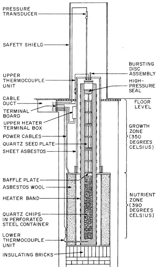
Figure 2—Diagrammatic cross-section of quartz-growing installation.
