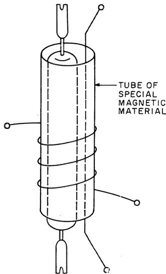
Figure 4—Crosspoint element using a tube of magnetic material having two directions of easy magnetization.
