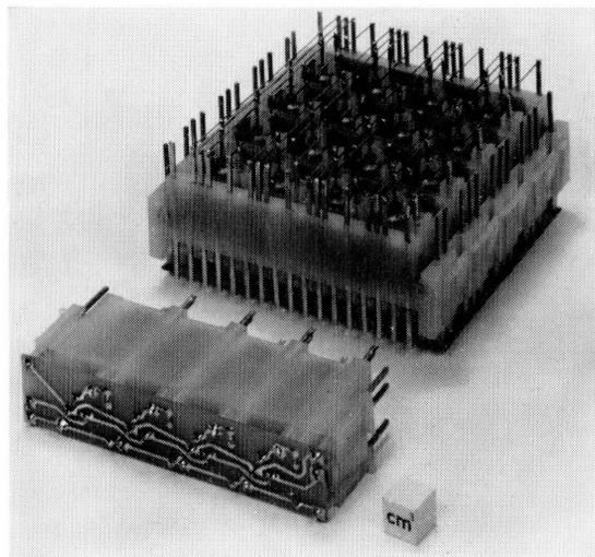
Figure 10—Crosspoint strip holding 4 crosspoint elements, each with 3 type *H 50* reed contacts for continuous hold current. The crosspoint matrix shown consists of 4 crosspoint strips with 4 crosspoint elements each.
