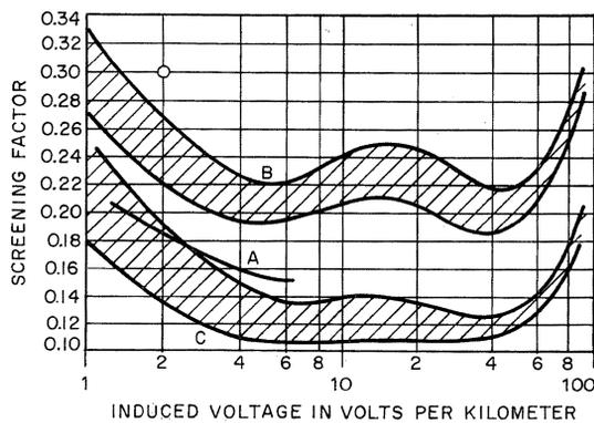
Figure 11—Curve A is the effective screening factor between Ål and Ustaoset. B and C are the factory measured screening-factor curves for 19-quad and 27-quad cables, respectively.
