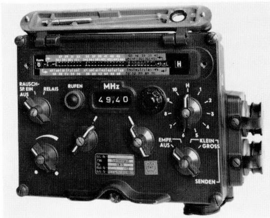
Figure 9—Remote-control unit, showing open cover for setting preset frequency.
