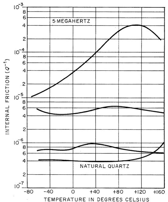
Figure 6—Internal friction ( $Q^{-1}$ ) as a function of temperature for 3 laboratory-grown crystals. The equivalent curve for natural quartz is also given.
