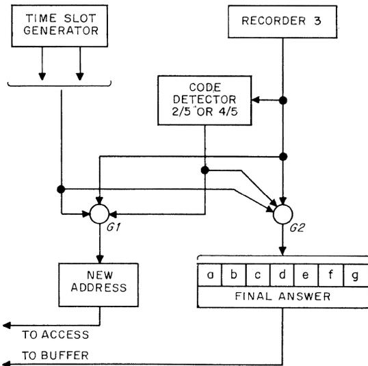
Figure 16—Transcoding and display.
