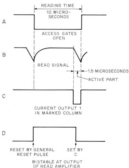
Figure 12—Read cycle of capacitor store.
