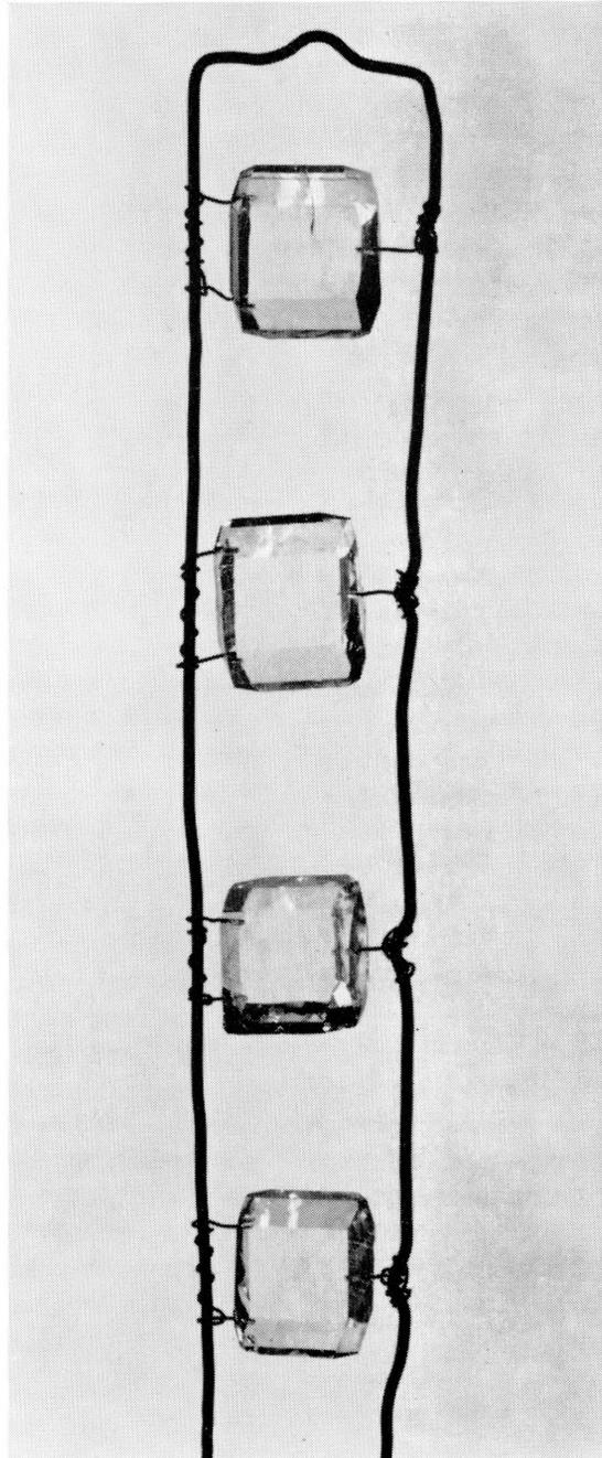
Figure 1—First crystals produced during project. These are approximately 2 centimetres square and 7.5 millimetres thick.
