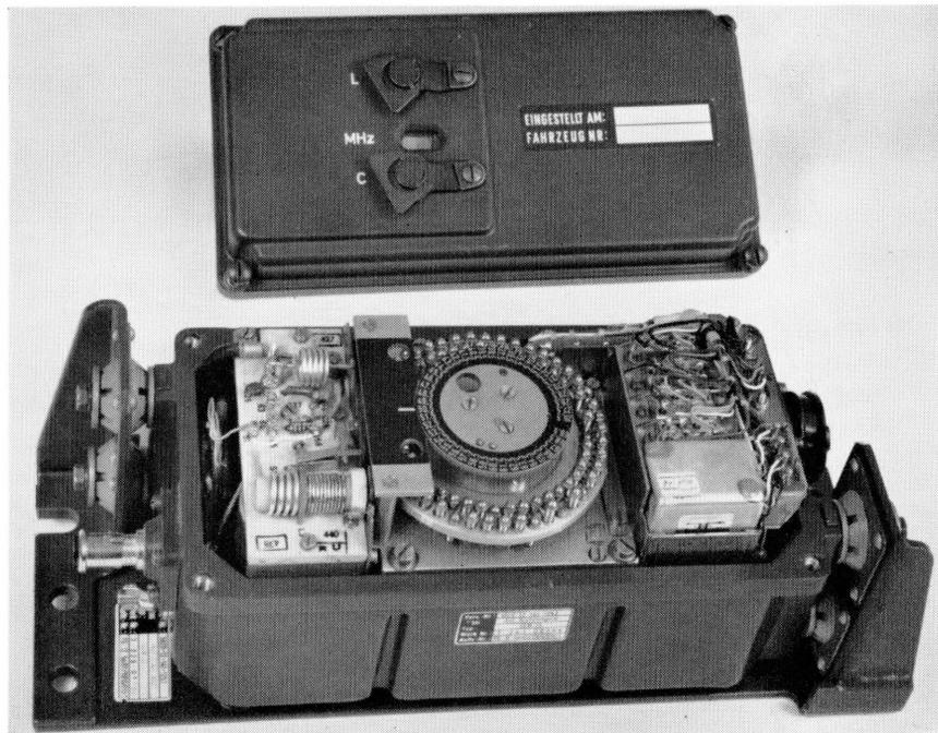
Figure 11—Automatic antenna tuning unit, cover removed.
