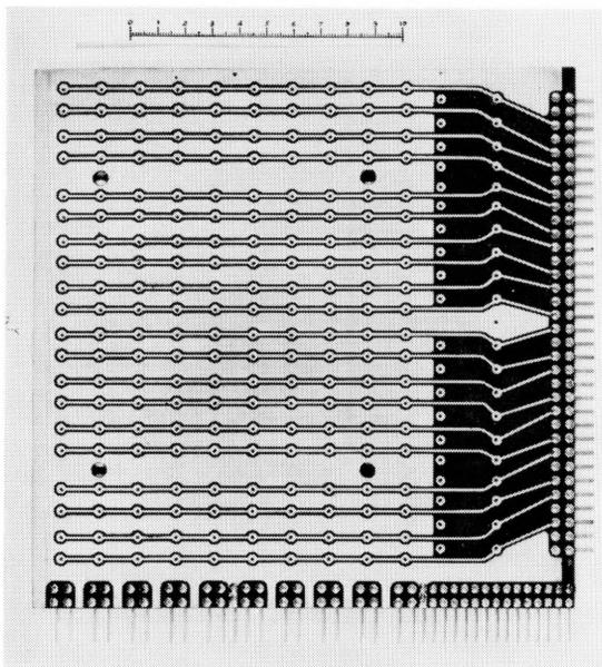
Figure 9—Bottom view of submatrix.
