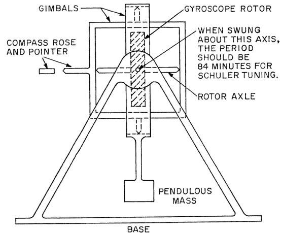
Figure 3—Schuler tuning employs a pendulum having a period of 84 minutes that when moved from its vertical position causes an oscillation about the indicated axis. The error does not continue to increase with time but oscillates back and forth at the Schuler period.
