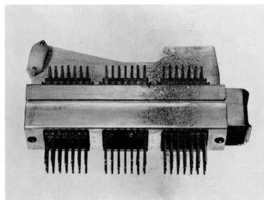
Figure 8—Plugs and jacks, separate and engaged.
