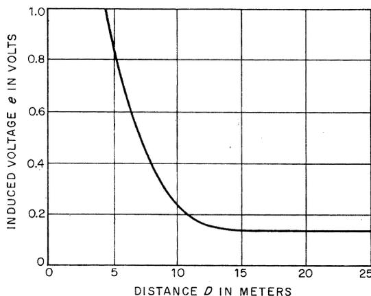
Figure 1—Induced voltage  $e$  per 100 ampere-kilometers as a function of distance  $D$  from middle of track (experimental results from southwest Norway on a stretch with booster transformers).
