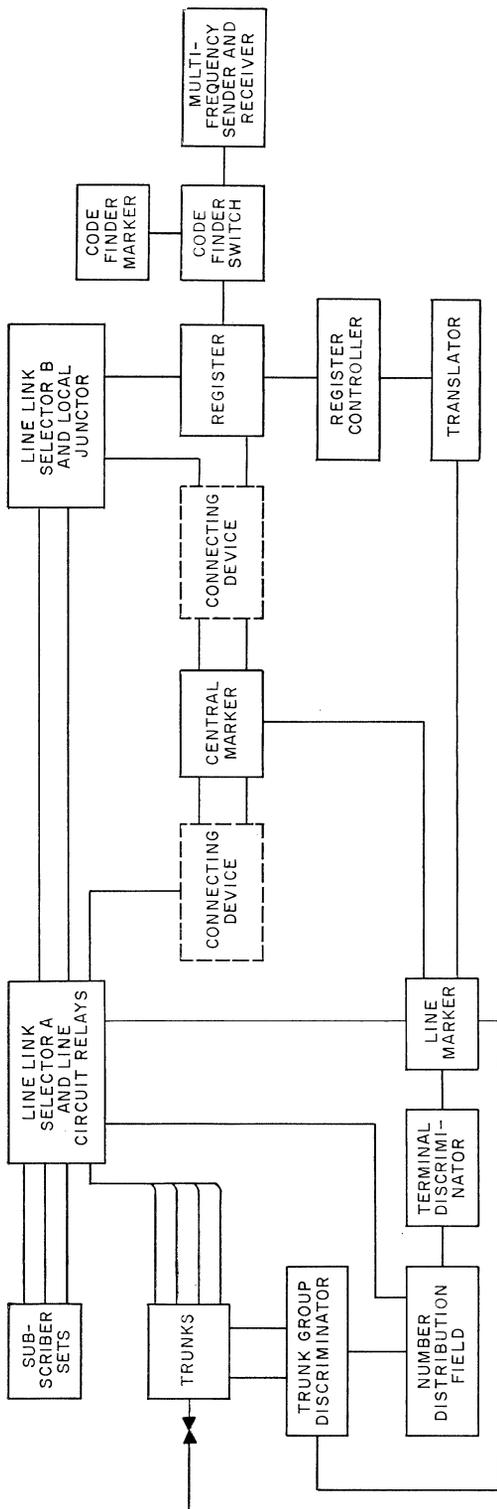
Figure 6—Block diagram of Pentaconta 32 system.
