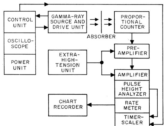
Figure 15—Arrangement of components in the Mössbauer spectrometer.
