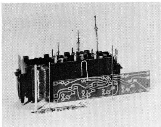
Figure 6—Standard building block containing 4 reed crosspoints.
