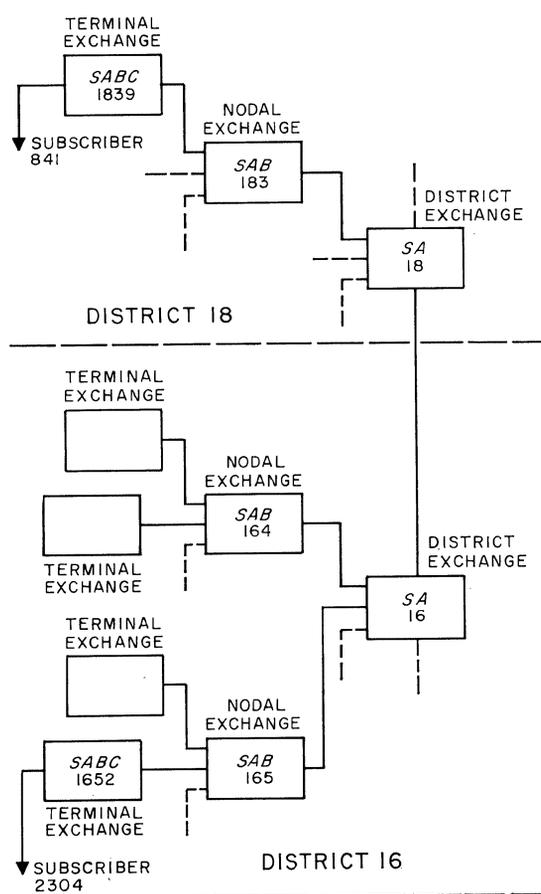
Figure 1—Star-shaped telephone network.
