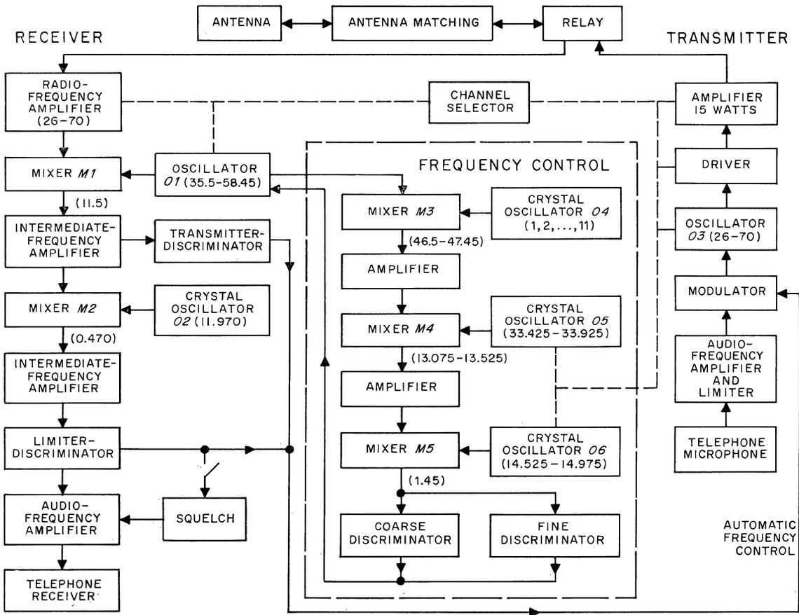
Figure 1—Block diagram of SEM 25. The numbers within parentheses are in megahertz.
