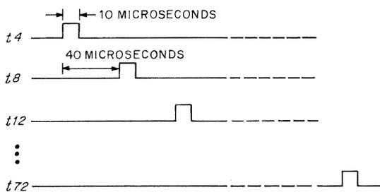
Figure 6—Clock pulses.
