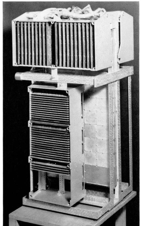
Figure 7—Model 3 memory with access electronics.
