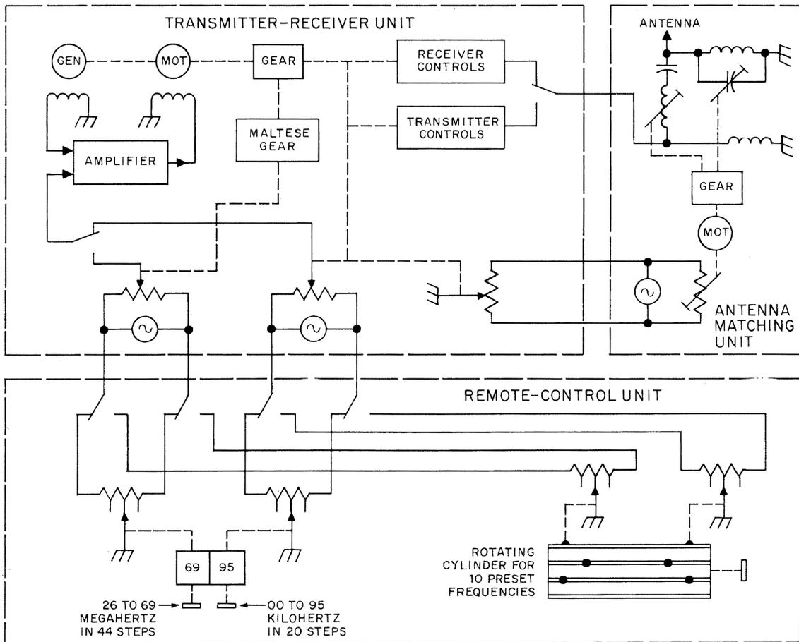
Figure 2—Remote-control system for channel selection and tuning.
