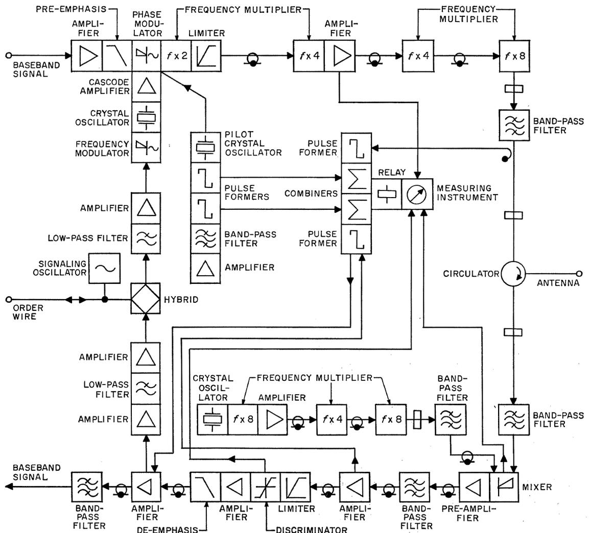
Figure 2—Block diagram of transmitter and receiver.
