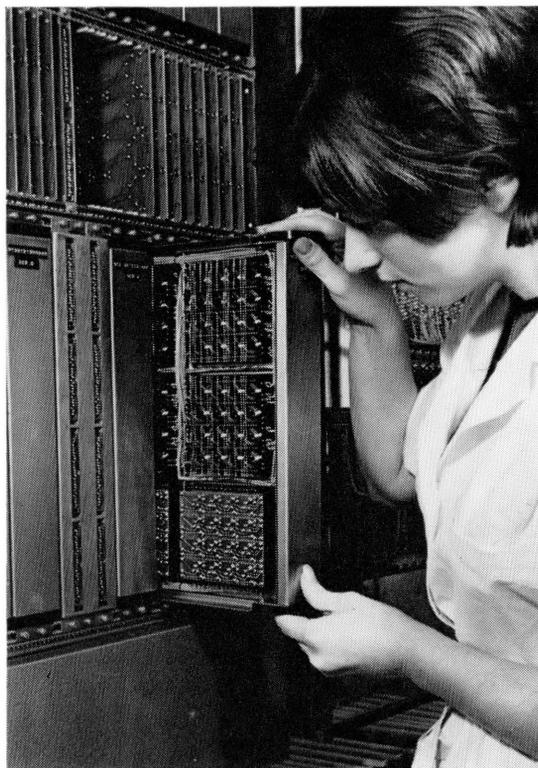
Figure 7—Plug-in line switch unit containing 6 sets of 4-by-4 crosspoint matrices.
