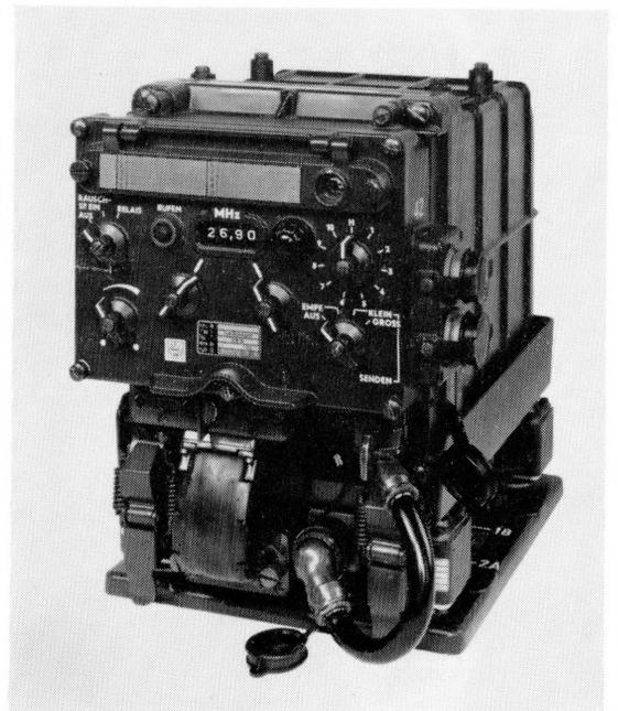
Figure 5—Receiver with control unit attached.
