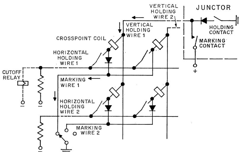
Figure 4—Marking procedure in a crosspoint matrix.
