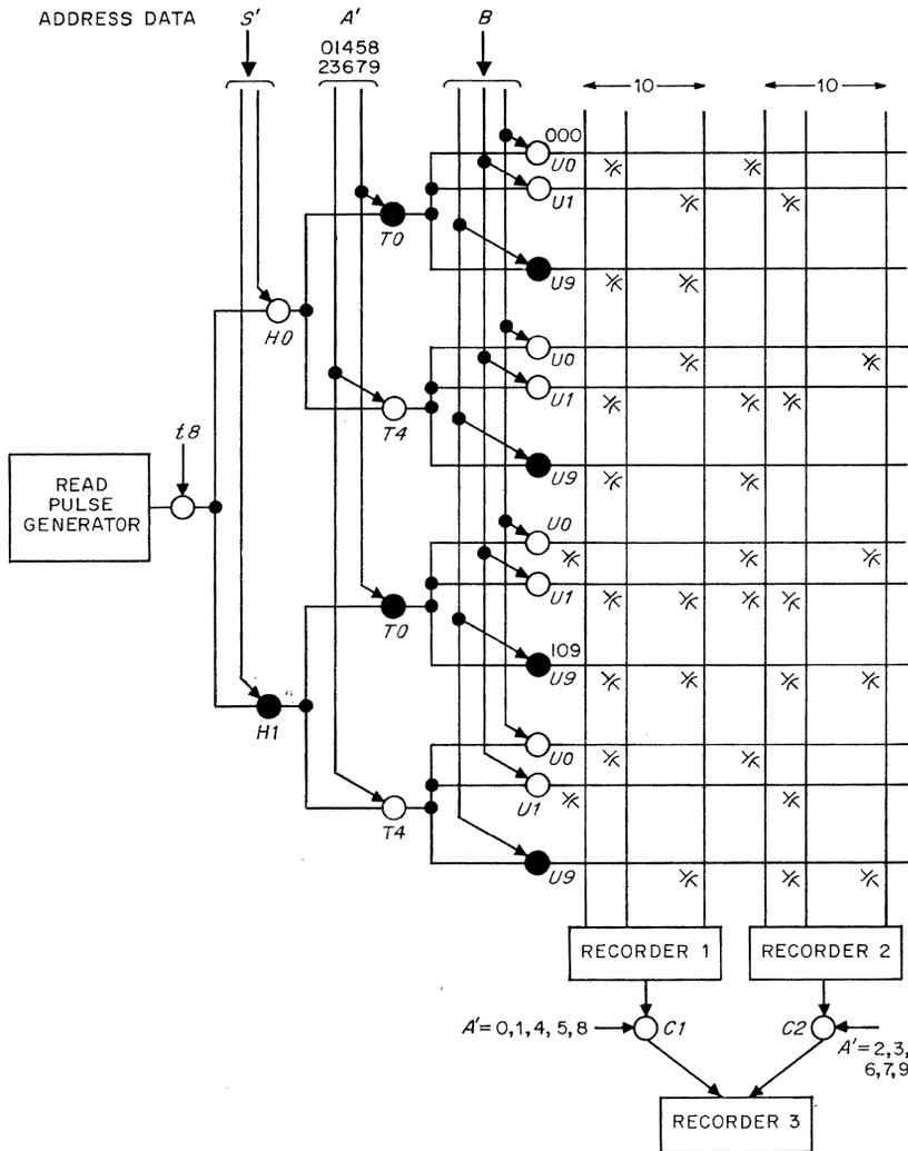
Figure 13—Principle of access gating for 160  $S'A'B$  combinations of the number-of-digits section.
