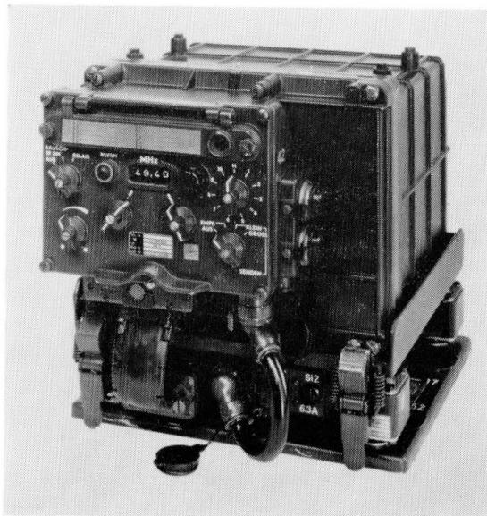
Figure 4—Transmitter-receiver with control unit attached.
