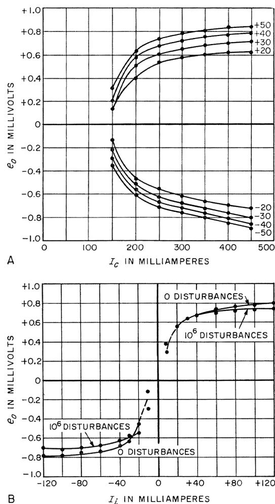
Figure 3—Typical output characteristics of the memory cell. A shows  $e_o$  as a function of  $I_c$  for the indicated values of  $I_i$  in milliamperes. B shows  $e_o$  as a function of  $I_i$  for  $I_c = 250$  milliamperes.
