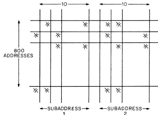
Figure 7—Capacitor matrix. The absence of a capacitor at a crosspoint gives a 0 output.
