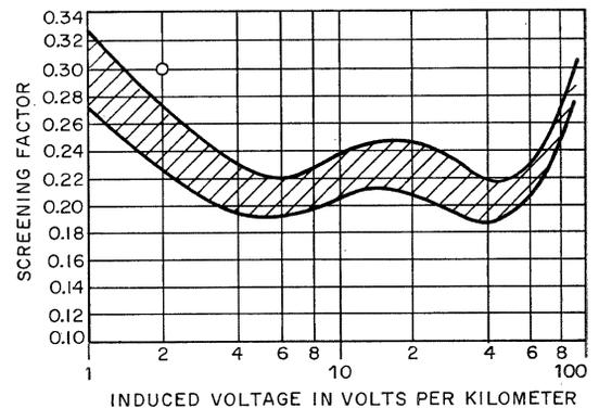
Figure 8—Production-control screening-factor curves for 1.2-millimeter 19-quad cables at  $16\frac{2}{3}$  hertz (1.1-millimeter aluminum sheath). Normal variations (gap approximately 45 percent). Refer to Table 4.
