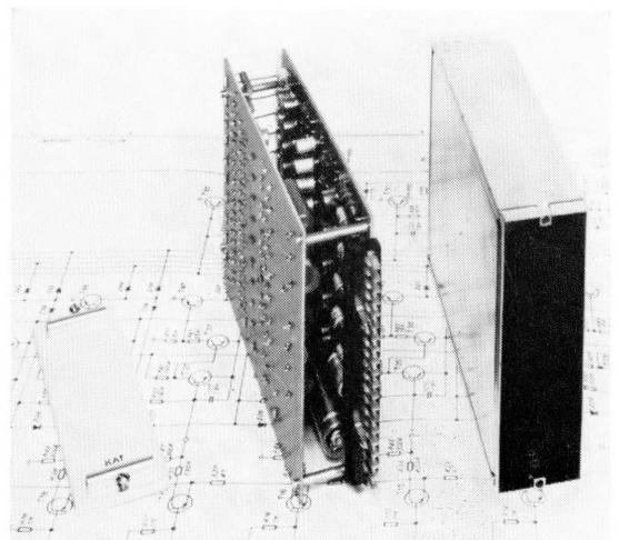
Figure 6—Electronic scanner for category identification in a Pentaconta exchange.
