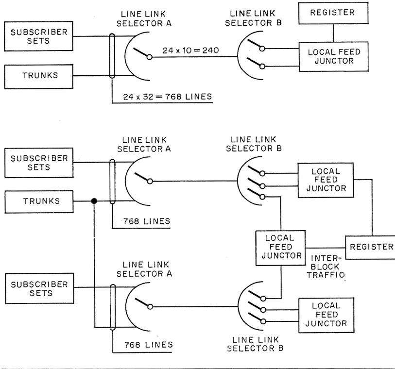
Figure 4—Two-stage version of primary switch. At top is the single-block exchange with a maximum of 768 terminals. Below it is a 2-block exchange.
