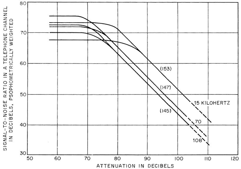
Figure 8—Influence on 15- and 70-kilohertz channels of a perturbing super-high - frequency signal modulated by white noise over the baseband from 6 to 108 kilohertz.
