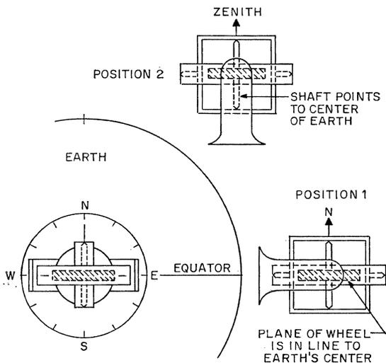
Figure 2—Gyrocompass pointing north when at the equator (position 1) will maintain its spatial orientation when moved to position 2 where it will point to the sky and be useless for azimuth indication.
