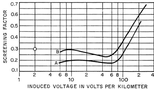
Figure 10—Production-control screening-factor curves at 16 $\frac{2}{3}$  hertz. *A* = 1.2-millimeter 12-quad cable with 1.0-millimeter aluminum sheath. *B* = 1.2-millimeter 4-quad cable with 0.9-millimeter aluminum sheath. Refer to Table 4.
