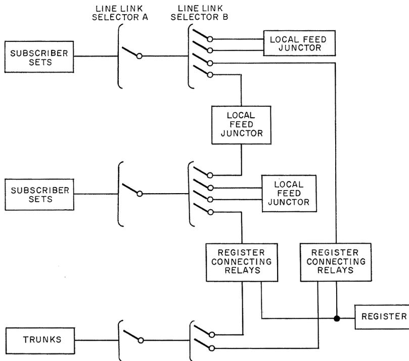
Figure 5—Multiblock exchange with separate trunk stage.
