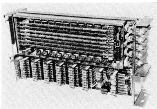
Figure 7—Line link selector *A* and line circuit relays.
