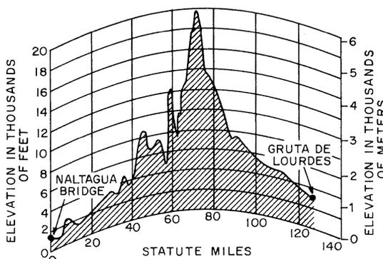
Figure 2—Profile of path 1 for  $K = 1.0$ .
