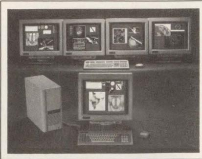
gle mouse and keyboard control all displays. A virtual screen mode treats multiple displays as a single large display surface. The unit has a thick and thin Ethernet interface and supports TCP/IP and DECnet network protocols. Terminal with 4 Mbytes of RAM, \$6500. **Jupiter Systems**, 1351 Harbor Bay Pkwy, Suite 200, Alameda, CA 94501. Phone (510) 523-9000. **Circle No. 447**
