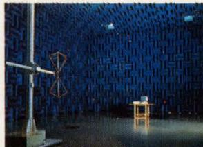
Anechoic chamber (FCC Filing and 10 m Regulations)
