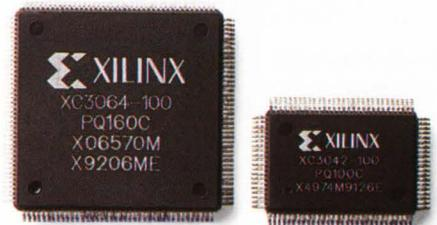
*Besides pushing speed, density and costs, we're also driving advancements in packaging, including the first programmable logic in QFPs.*
