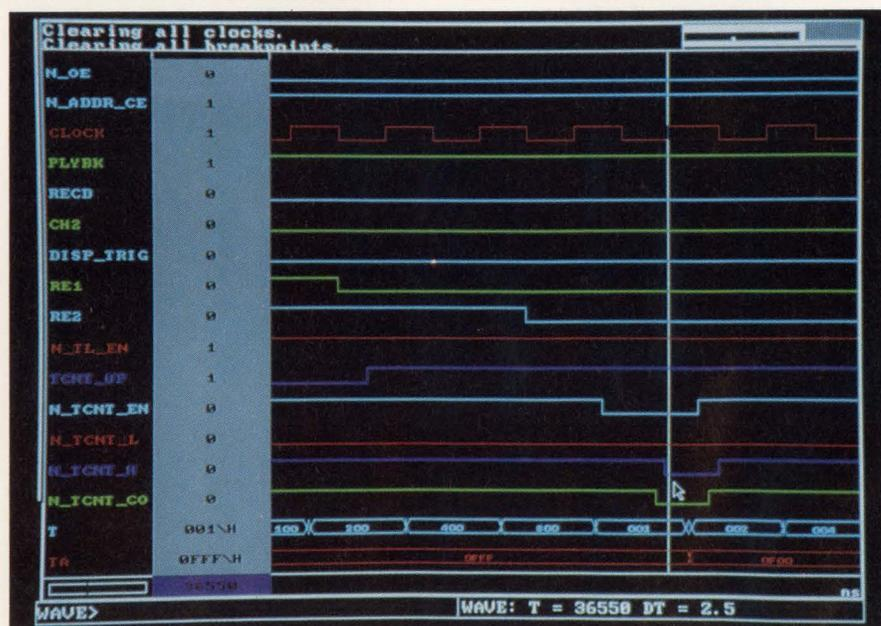
Here I pushed the clock up to see where the circuit fails. At 20 MHz the signal enabling the upper 7-bit counter for the horizontal trigger position (N\_TCNT\_H) has only 2.5-nsec setup time before the rising edge of the clock, insufficient for the counter. You can see the Trigger Address bus (TA) does not make the transition from OFFF to 1000 but goes to 0F00.
