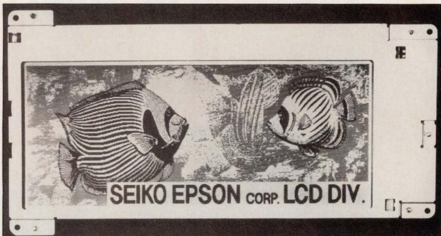
Designed for use in palm-top computers, the TCM-9108A from Epson has a CGA-compatible resolution of  $640 \times 200$  pixels. The LCD consumes 130 mW, weighs 190 grams, and is 6.3-mm deep.
