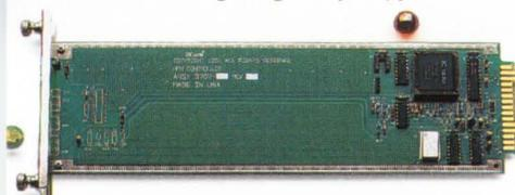
*Before Xilinx, this board was crawling with chips. We reduced chip count by 80%, power consumption by 75%, and cut out two board layers. That's what we call a good shrink.*
