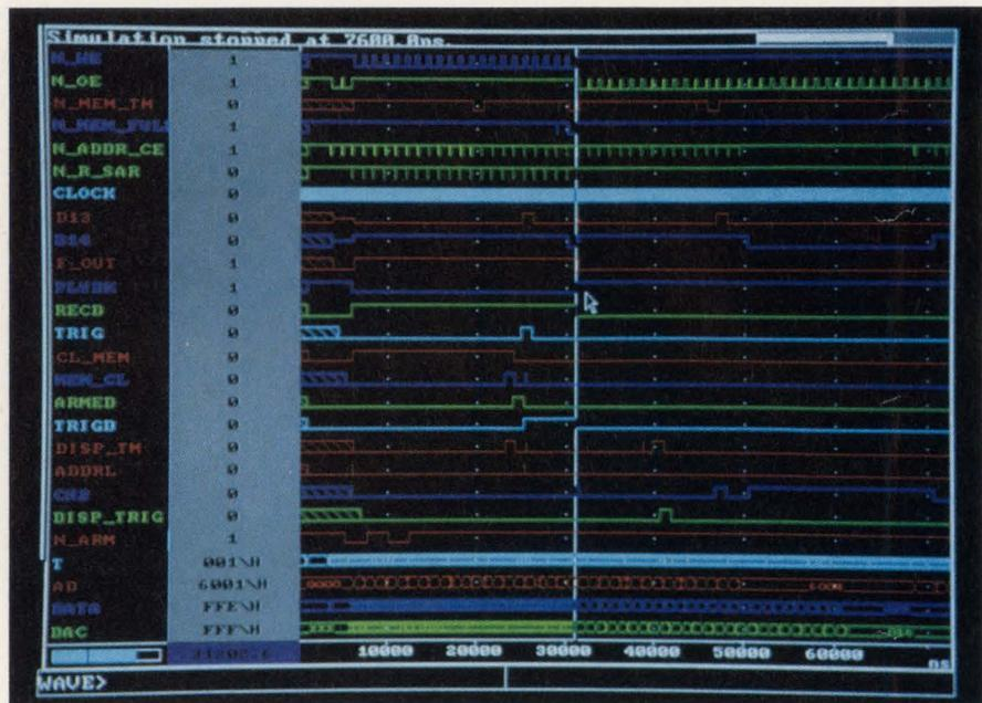
**Fig 2**—This sequence takes the design through reset, clearing memory, arming, triggering, completing data acquisition, playback with capture trigger marker, and end of data marker. To see more details, you need to zoom in as shown in Figs 3 and 4.
