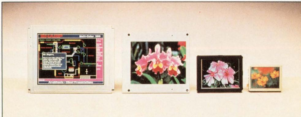
Several sizes of color LCDs are available from Sharp Electronics. The displays include both passive and active-matrix types.
