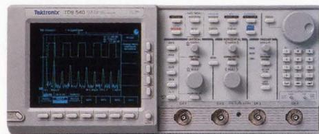
get 500 MHz bandwidth and up to 50k record lengths. A single-channel sampling rate of 1 GS/sec on the **TDS 540** and 500 MS/sec on the 520—combined with edge, pattern, state, glitch, runt & pulse width triggering—greatly simplifies debugging and fault isolation. What's more, both feature built-in
