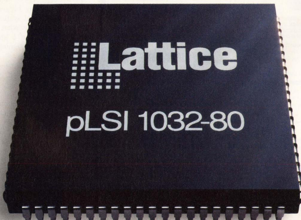
System clock rates up to 80 MHz. And a propagation delay of only 15ns pin-to-pin. That's the kind of performance you get with our new pLSI™ family of high density PLDs. Comprised of four devices ranging in density from 2,000 to 8,000 PLD gates, they give you absolute timing predictability, right from the data sheet. Lattice also offers the ispLSI™ family—an in-system programmable (isp) version of the pLSI family that delivers non-volatile, 5-volt only in-system programming capability.
