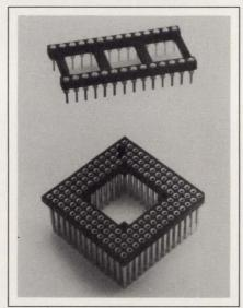
Both devices utilize glass-filled, molded polymer construction. The DIP sockets are supplied in open or closed versions that have center-to-center spacings of 0.300, 0.400, 0.600, and 0.900 in. The models with 0.300- and 0.600-in. spacings are compatible with automatic insertion equipment. The high-tem-
