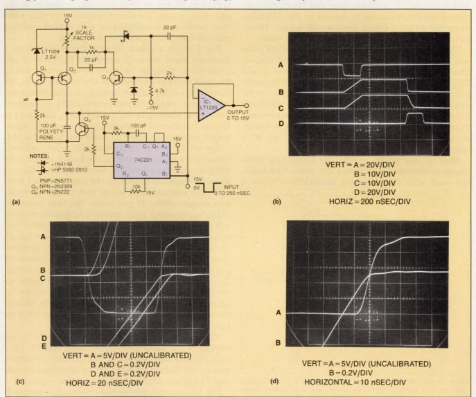
Fig 5—Changing pulse widths to voltages provides a convenient way to monitor changes in time intervals that occur as a function of time. The circuit in  $\bf{a}$  performs this function. In  $\bf{b}$  you see circuit waveforms. These waveforms appear in expanded form in  $\bf{c}$ . The current-source turn-off appears in  $\bf{d}$ .
