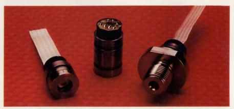
**Design flexibility is the primary advantage** offered by Novasensor's NPI pressure sensors. Capable of measuring pressures of 10,000 psi, the devices provide a 100-mV output, feature a  $\pm 2\%$  interchangeability, and are accurate to  $\pm 1\%$  over a 0 to 70°C operating range.
