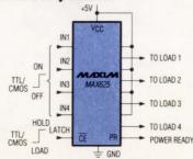
The MAX625 allows logic signals to switch four 1A loads (4A peak), simplifying load switching in low-voltage systems and extending battery life. It has a 4.5V to 16.5V input supply range and 70µA typical quiescent current. Ideal for battery-powered and distributed power applications requiring high efficiency and small size. Available in 24-pin narrow plastic DIPs.
