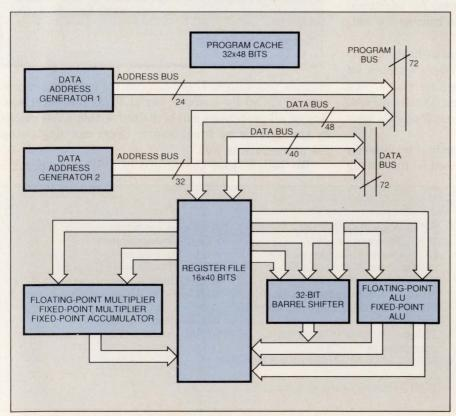
Fig 3—An on-chip cache lets Analog Devices' AD21020 do fast inner-loop processing. The processor caches complex instructions then uses the program bus as a second data bus.
