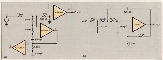
Fig 5—This unity-gain third-order Butterworth GIC filter has a 40-kHz cutoff frequency (a). The equivalent Sallen and Key realization requires twice the gain (b).
