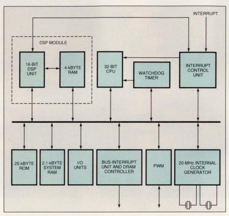
The 32AM160 microcontroller controls voice processing by combining a 32-bit CISC CPU with a dedicated DSP module.
