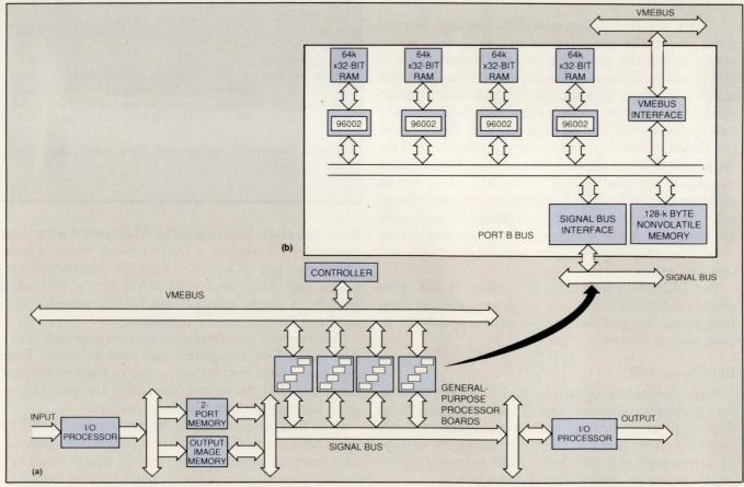
DSP chips are building blocks for large-scale processing systems. Spectrum's Vasp (a) is a scalable, multiprocessor system built around Motorola's 96002 (b). The system was designed for aperture radar applications.
