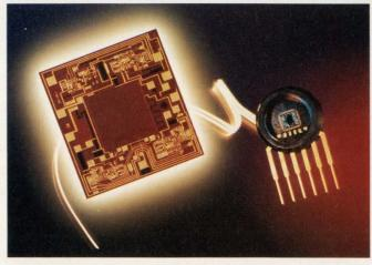
Signal conditioned to interface directly with a  $\mu P$ , Motorola's MPX5100A is a single-chip, 15-psi absolute pressure sensor. It has a 0.5 to 4.5V output and is temperature compensated for operation over a 0 to 85°C range.
