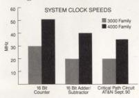
As measured by typical design benchmarks, the XC3000 family is the industry's fastest FPGA. Or at least it was until we introduced the 4000 family.
