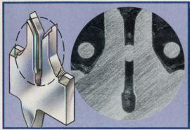
Contact-to-Conductor Relationship – Thomas & Betts' "coined-slot" contacts are designed to position the terminated conductors within a specified region for maximum conductivity and reliability.
