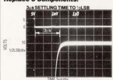
The monolithic MAX526 replaces 4 DACs and 4 op amps. Monotonic 12-bit performance quaranteed with ½LSB relative accuracy over temperature for all 4 outputs and 1LSB total unadjusted error with no zero-or full-scale adjustments at +25°C. Outputs settle to ½LSB in 3us.
