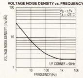
The MAX412 provides the best noise performance—even at very low supply voltages. <2.4nV/Hz@1kHznoise guaranteed! With a guaranteed output voltage swing of 7.3Vpp and greater than 97dB SINAD (Signal/THD+N) while operating from ±5V supplies, the MAX412 is ideal for 5V systems. 8-pin DIP/SO. (CIRCLE 282)
