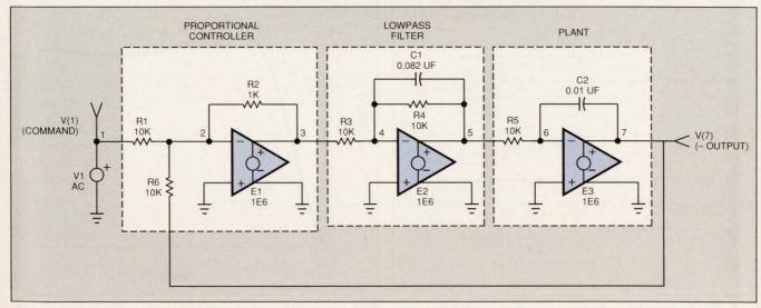
Fig 3-Op amps and other components model each of the three blocks-the controller, the filter, and the plant-of Fig 2's control system.
