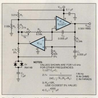
Fig 1—Based on a modified GIC bandpass filter, this 5-kHz sinewave oscillator runs off 5V.
