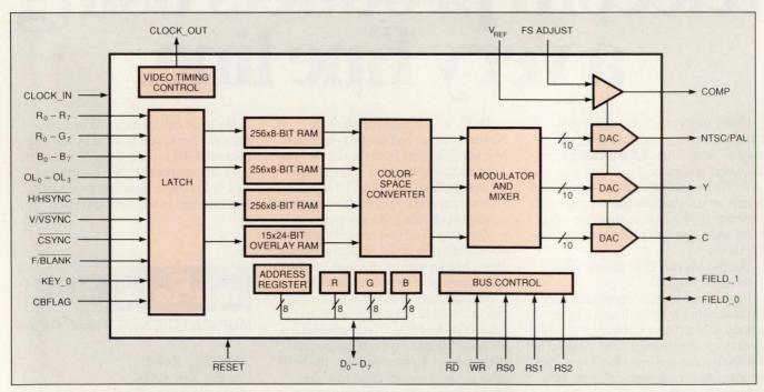
Fig 1—A choice of S-Video, NTSC, or PAL outputs makes the Bt858 video-encoder IC useful in applications that require compatibility with different international television standards.
