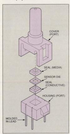
Fig 1—High reliability is a prime advantage provided by the simplified construction of 24PC Series sensors. The conductive seal also allows Micro Switch to employ a large diaphragm area, which improves sensor stability.
