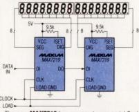
The new MAX7219 has an easy-to-use serial 3-wire interface and digital/analog brightness control. Only one external resistor is required to set the segment current for all LEDs. The MAX7219 has 1kHz per digit scan rate and is available in a compact 24-pin SO package. (CIRCLE 287)
