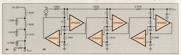
Fig 2—An LC ladder network generates any lowpass-filter polynomial (a). You can simulate the filter's transfer function by multiplying each element value by 1/s and realize the filter using GICs(b).
