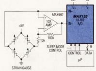
The **MAX135** low-noise, 5V-powered, multi-slope integrating ADC provides ±0.005% accuracy at 16 conversions per second, while requiring only 125µA of supply current over temperature (10µA in sleep mode). Resolution is extended to 18 bits with 3 sub-LSB bits and data averaging. 8-bit data bus and 3 logic control lines simplify µP interfacing. (CIRCLE 275)
