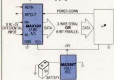
The **MAX190** converts rail-to-rail signals to either serial or parallel data in 7.5µs on battery power. Precision laser-trimmed reference, clock and track/hold included on-chip. The MAX190's already-low 15mW power consumption is reduced to 150µW during shutdown.
