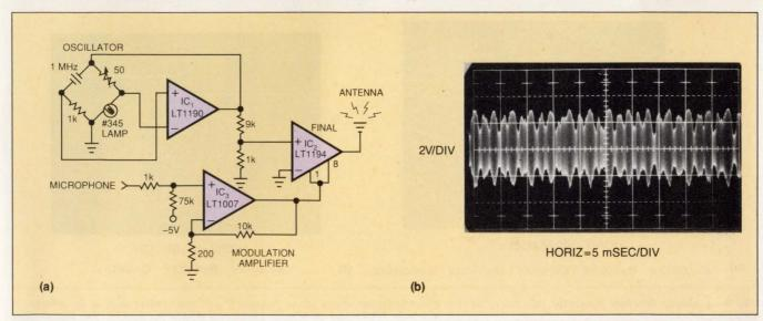
Fig 7—Though perhaps not worthy of Wolfman Jack or Dick Biondi, the circuit of **a** is still a complete AM radio station. When Chuck Berry picks his guitar and belts out "Johnny B. Goode," the modulated output looks like what you see in **b**.
