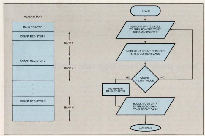
Fig 1—Creating N banks of memory extends an EEPROM write-cycle life by N times. The cost is the added memory.
