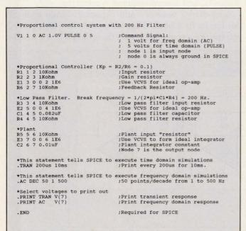
Fig 4—This Spice model, representing the circuit in Fig 3, has three types of lines—comments, components, and control lines.
