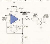
The MAX404 video op amp has 0.01° differential phase and 0.05% differential gain while operating from ±5V supplies. Featuring 80MHz gain-bandwidth and 500V/µs slew rate, this amplifier is ideal for video and other high-speed applications. 50mA continuous output current is guaranteed. (CIRCLE 281)
