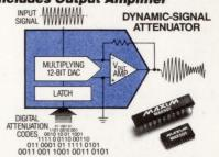
The **MAX501/502** combine a BiCMOS amplifier with ±10V drive capability and a laser-trimmed, thin-film-resistor DAC on a single chip. These DACs accept a DC or AC reference and have buffered input latches that are easily interfaced to both 8-bit (MAX501) and 16-bit-wide (MAX502) data buses.
