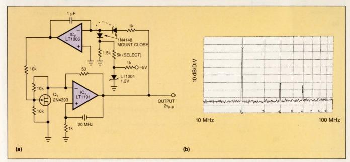
Fig 5—An electronic gain-control circuit that uses the voltage-controlled on-resistance of a FET stabilizes the output amplitude of this 20-MHz crystal oscillator (a). In b, you see that the output's harmonics are at least 47 dB below the fundamental.
