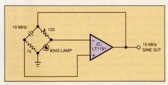
Fig 4—An incandescent lamp's current-dependent resistance stabilizes the oscillation amplitude of this 10-MHz crystal oscillator.
