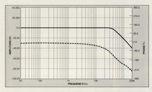
Fig 6—The amplitude (solid line) and phase response (dotted line) of the third-order Butterworth GIC filter are nearly constant throughout the audio-frequency band.
