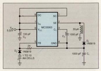
Fig 1—This switched-current regulator can charge anywhere from one to 10 1.5V NiCd cells using an input voltage of approximately 5.2V.
