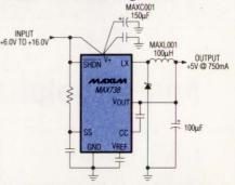
The MAX738 PWM step-down switching regulator is ideal for high-efficiency step-down applications. It has a 6V to 16V input voltage, up to 750mA output current, and 88% efficiency
