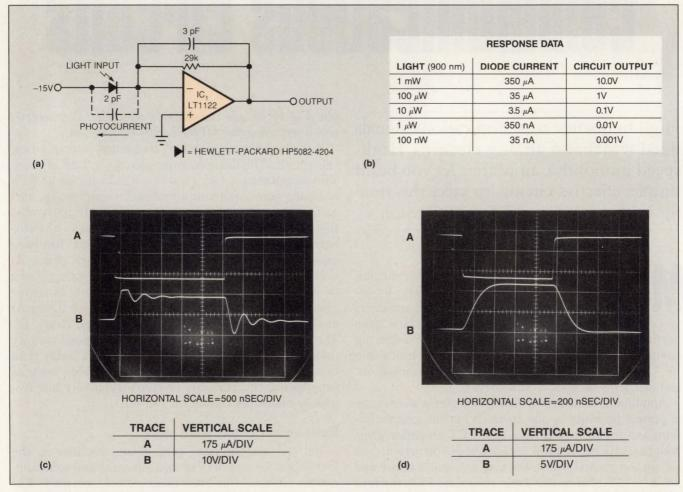
Fig 1—This basic photodiode amplifier circuit (a) handles 5 decades of light intensity. The table (b) details the circuit's operating characteristics with the HP5082-4204 diode. Parts c and d show the circuit's response (trace B) to an input signal (trace A) without and with compensation, respectively.
