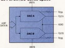
The MX7549 current-output, four-quadrant multiplying DAC features 1% resistance match between DACs, making many dual applications possible. The new DAC has ±½LSB max integral nonlinearity, ±5ppm/°C max gain temperature coefficient, and operates from a single +5V to +15V supply. Pin compatible to AD7549
