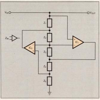
Fig 1—The topology of a Generalized Immittance Converter (GIC) can simulate the impedance of any passive component, including a frequency-dependent negative resistor (FDNR).
