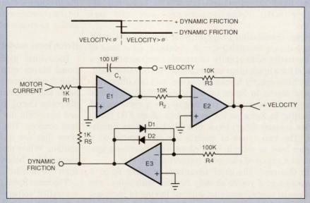
Fig A—This model of a servo motor with a frictional load uses an op amp with diodes in the feedback path to simulate dynamic friction.
