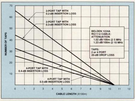
This graph illustrates the relationship between carrierband cable length and the number of taps in a 5-Mbps network. Developed by IEEE 802.4 LAN design engineers at Motorola, it also shows that a 0.1-dB difference in insertion loss at each tap will significantly affect the number of taps a given length of RG11/U cable can accommodate.
