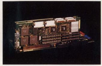
A typical multiprocessing DSP design is illustrated by the IBM GT4x graphics adaptor, which has six TI TMS320C30s in a 3-card subsystem. The adapter handles 2- and 3-D wireframes and 3-D surfaces with  $1280 \times 1024$ -pixel resolution.
