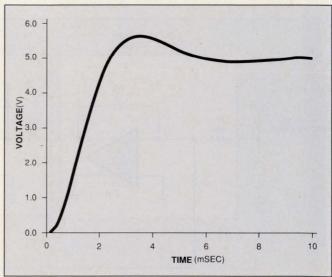
Fig 6—About half a volt of overshoot occurs in Fig 3's system when the cutoff frequency is reduced to 200 Hz ( $C1 = 0.082 \mu F$ ).
