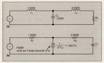
Fig 4—A normalized third-order Butterworth filter serves as a building block for the anti-imaging filter (a). You obtain the normalized GIC filter by multiplying each normalized element value by 1/s (b).
