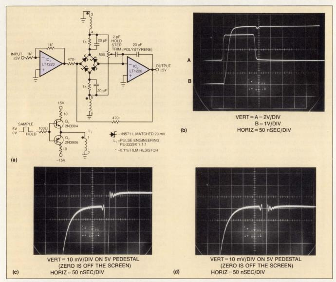
Fig 2—This very fast S/H circuit (a), acquires signals to 8-bit accuracy in 100 nsec. In  $\mathbf{b}$  you see the waveforms within the circuit. Accurate operation depends on cancellation of the switching signals that feed through the bridge. In  $\mathbf{c}$ , the compensation is disconnected. In  $\mathbf{d}$ , you can see the effect of the compensation.
