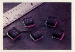
Accurate to better than ±0.25%, Model 1431 absolute pressure sensors from IC Sensors are housed in a surface-mount package measuring 0.3×0.3 in. They operate from either a constant-current or constant-voltage supply, measure pressure levels of 15 to 300 psi, and have a 60-mV typical output span.
