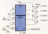
The MAX621/620 drive 4 low-cost 35A/0.028Ω N-MOSFETs from 4.5V to 16.0V inputs. It combines a power supply, four latched MOSFET drivers, protection circuitry — all in a single 18-pin IC. The MAX621 has internal charge-pump capacitors; MAX620 costs less and requires 3 inexpensive external components.
