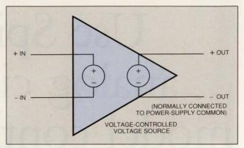
Fig 1—The voltage-controlled voltage source (VCVS) is the basic Spice tool for block diagrams. If the gain constant is large and -OUT is connected to power-supply common, the VCVS acts like an ideal op amp.
