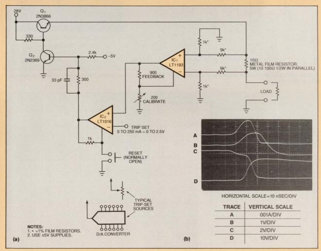
Fig A—This circuit breaker (a) trips in as little as 18 nsec. The circuit shuts down the load (b, trace C) when the load current (trace A) exceeds the trip point. Trace B represents  $IC_1$ 's output voltage; trace D represents  $IC_2$ 's output voltage.
