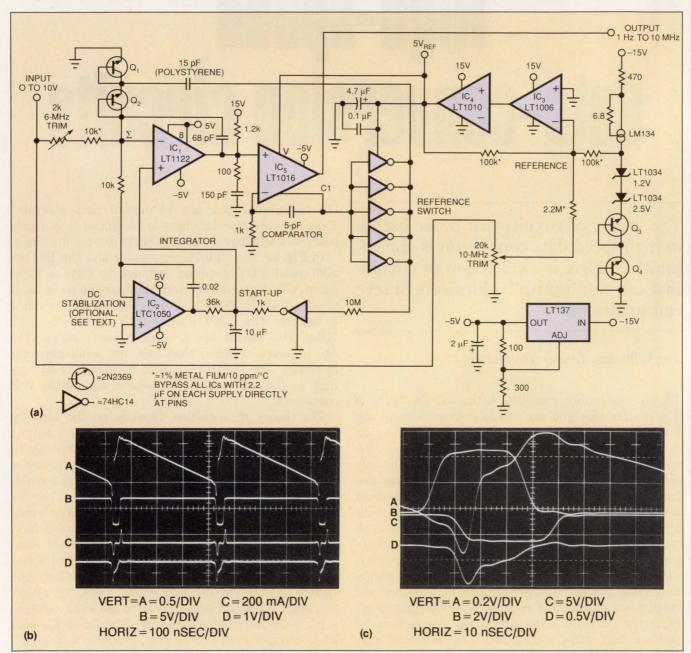
Fig 1—A voltage-to-frequency converter with a maximum output frequency of 10 MHz and a 140-dB dynamic range is only moderately complex (a). In b, you so the circuit waveforms; c is an expanded view of the discharge-reset sequence upon which the circuit performance depends.
