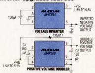
The MAX660 charge-pump voltage inverter converts a +1.5V to +5.5V input to a -1.5V to -5.5V output. It is a pin-compatible high-current upgrade of the ICL7660. 100mA is supplied with only a 0.65V voltage drop, compared to only 15mA with the ICL7660. Efficiency exceeds 90% for most applications.
