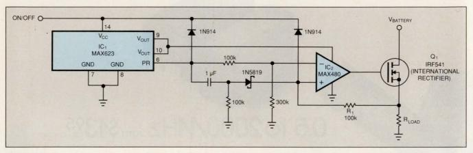
Fig 1—A regulated charge-pump IC generates a gate drive equal to  $V_{BATTERY} + 10V$  for the high-side power switch  $Q_1$ , an n-channel power MOSFET.
