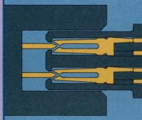
Precision Lead-In Design – assures that repeated connect/disconnect functions are consistently smooth and without pin damage.
