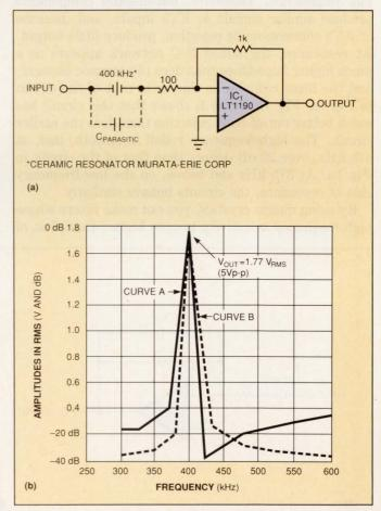
Fig 1—One amplifier and a ceramic resonator create a bandpass filter (a). The solid curve of b shows the filter's frequency response. Note the dip to -40 dB on the high side of resonance. The dip is the result of the resonator's parasitic capacitance.
