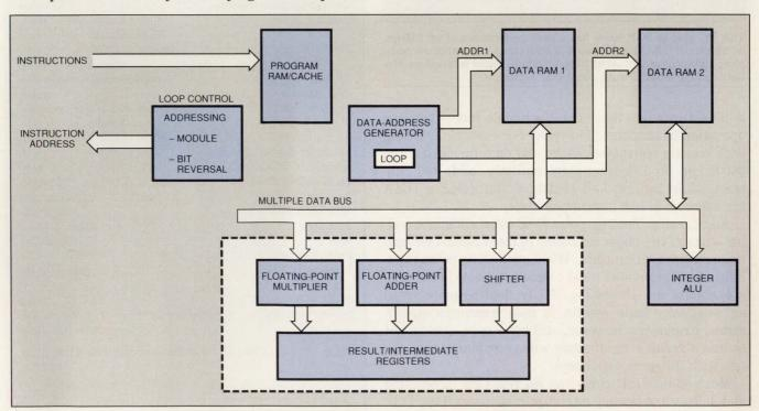
Fig 1—A generic 32-bit floating-point processor supports 3-memory addressing with automatic addressing and loop control. A low-overhead multiply/accumulate unit (MAC) calculates series
