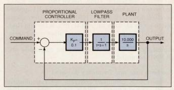
Fig 2—This simple control system consists of a proportional controller, a lowpass filter, and an integrating plant. The plant might represent an idealized motor or a mass in a frictionless system.  $K_P$  is the proportional gain, and  $\tau$  is the cutoff frequency in radians/sec.
