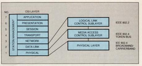
Fig 1—Based on the 7-layer ISO/OSI communications model, the Manufacturing Automation Protocol (MAP) was devised by system integrators at General Motors to unite the "islands of automation" created by the computerization of individual manufacturing processes. The IEEE 802 LAN standard provides the specific implementation of the first two layers of the model.
