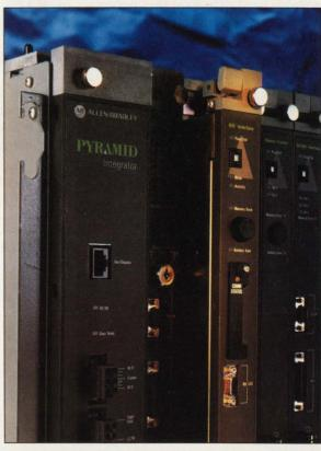
If you need to tap into a MAP LAN, many proprietary networks offer gateways like this Pyramid Integrator for Allen-Bradley's Data Highway Plus LAN. Using such gateways lets you eliminate "islands of automation" that arise when the controllers from competing vendors can't exchange data.
