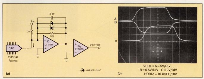
Fig 3—Only two ICs yield a fast summing comparator (a). In b, you can observe key waveforms as the circuit operates.
