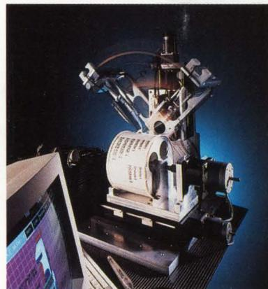
An automated system for testing bar-code scanners, from Hewlett Packard, combines Compumotor and Daedal technology.
