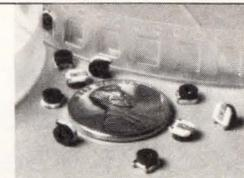
TMC4K "chip" trimmers feature a ceramic substrate, a metal glaze element, and an insulated knob for easy adjustment. The TMC4K can withstand operating temperatures of  $-30^{\circ}\text{C}$  to  $+125^{\circ}\text{C}$  and is rated at 0.2 watts of power at 20V. Its standard resistance range is 200 $\Omega$  to 1M $\Omega$ . Outside dimensions are 3.8mm wide x 4.5mm long (2.1mm height).
