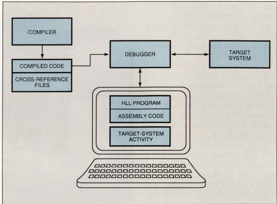
Fig 1—Debuggers have seen recent improvements at all three of their interfaces: compiler, human, and target-system.
