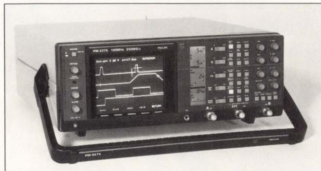
The 100-MHz, 250M-sample/sec PM 3375 is one of seven low-cost DSOs offered by Philips. This model performs nine automatic measurements in addition to cursor measurements.
