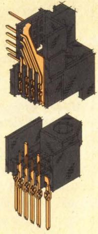
ing reference planes between pin columns to retain maximum pin counts in a controlled impedance interface.
