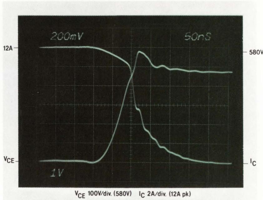
Turn-off characteristics of a single-ended forward converter with 300Vdc input. International Rectifier's IRGBC30U switches 12A at 50 kHz. Easily. (Actual unretouched photo.)
