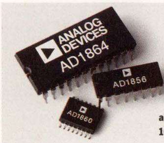
**Digital Audio Converters – The SOUNDPORT™ family of data converters comes complete with output amplifier, reference and digital logic interface. These mixed-signal ICs for high fidelity digital audio and multimedia applications achieve SNRs as high as 108 dB and THDs as low as 0.0025%.**
