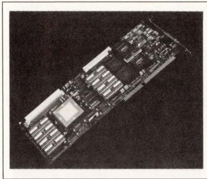
low partial signal reconstitution. Additional onboard logic and support software exercises the 96002's on-chip emulation facility for debugging work. Other backup consists of Intermetrics' 96002 C compiler, assembler, and high-level debugging tools. Support also includes an interface library to allow your Microsoft programs to control the board. £3495. Showing on Motorola's booth.
