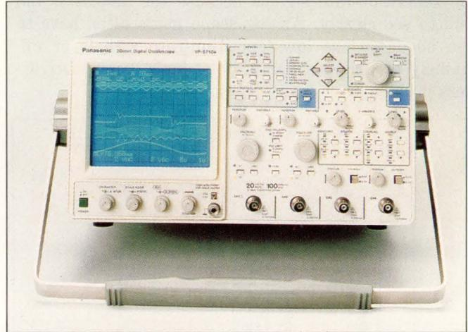
**With a 64k-point record length on one channel, the 20M sample/sec, 100-MHz VP-5710A from Panasonic can record long events. Two- or 4-channel operation results in proportionately shorter record lengths.**
