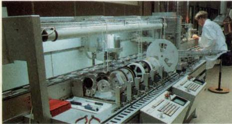
The PKA & PKC, DC/DC converters are produced on fully automated lines to guarantee consistently high quality and reliability
