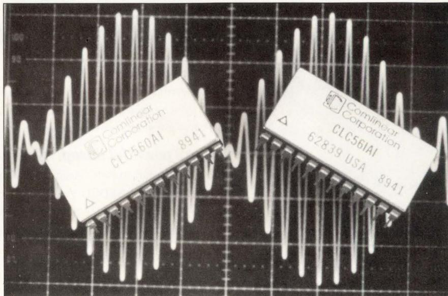
*Designed for output-driver applications, the CLC560 and CLC561 from Comlinear allow you to set both gain and output impedance by judicious choice of the feedback network. Because the impedance-matching maneuver entails no series resistor, the full output-voltage swing is available to the load.*
