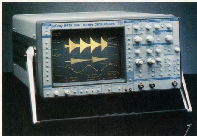
Extensive automatic-measurement features, a memory-card mass-storage system, and a 4000 × 4000-pixel display are key features of the LeCroy 9410 DSO. The 150-MHz unit provides 2% vertical accuracy and a 150M-sample/sec digitizing rate.
