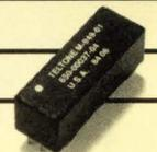
Line Sense Relays connect in series with Tip and Ring and provide a relay closure in response to loop current flow. For on-hook, off-hook monitoring, switchhook flash detection, and rotary dial pulse counting. Simple design, rugged construction.
