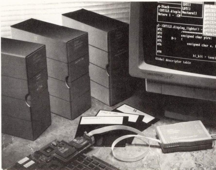
*Offering a subset of in-circuit-emulator features, Applied Microsystem's CodeTAP provides a fast, nonintrusive link between a debugger and a target system.*
