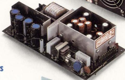
**Medical switchers and linears — designed to meet UL 544/IEC 601/CSA 22.2 No. 125.**
