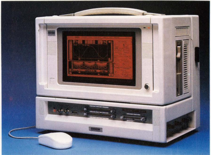
*Omnilab II is a good name for this multipurpose system from Orion Instruments. It is a logic analyzer, digital oscilloscope, and waveform generator combined with a PC.*
