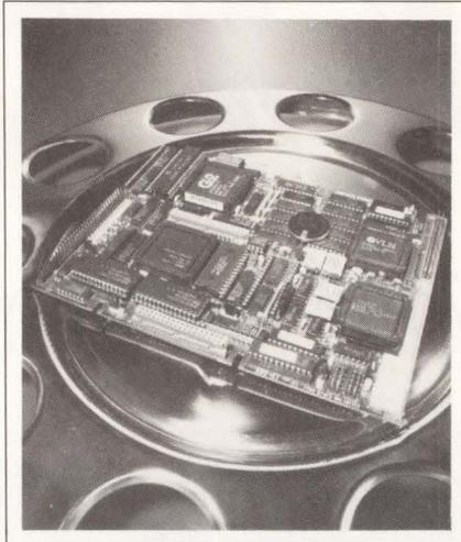
coprocessor. Memory capacity extends to 640k bytes. The board contains controllers for hard and floppy-disk drives, and supports CGA graphics. The board includes two RS-232C interfaces, one parallel port, and provisions for IBM PC bus and iSBX expansion. Additional items include a battery-backed
