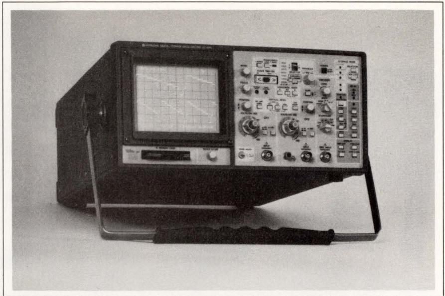
can read and write data on credit-card-sized RAM modules. Each module stores 15 waveforms. The connector that accommodates the RAM modules also lets you connect the scopes to a personal computer
