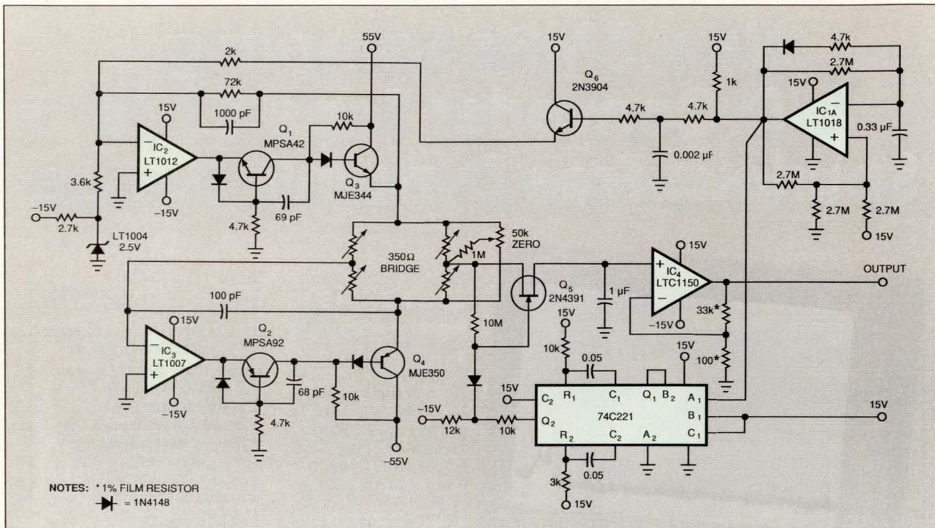
**Fig 17**—A special case of sampled drive, this circuit puts 100V across a 10V, 350Ω strain-gauge bridge for short periods of time. The circuit is intended for applications requiring high-resolution outputs from a bridge transducer.
