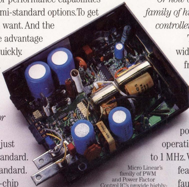
Micro Linear's family of PWM and Power Factor Control IC's provide highly-integrated solutions for a broad range of switching power supplies.
