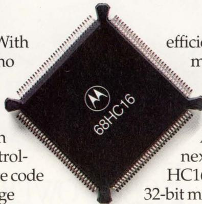
efficient. The HC16 can use any inter-module bus peripheral from our rapidly expanding 68300 Family.
