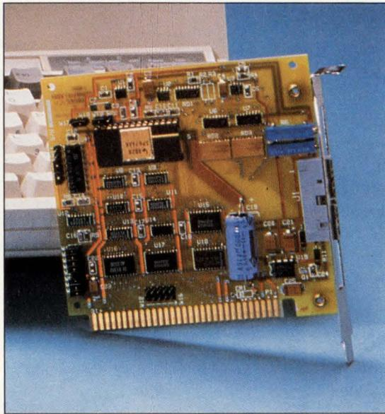
*Designed with portable PCs in mind, the DT2814 data-acquisition board from Data Translation requires minimal space and power. The board generates its own -12V power because many portable PCs don't.*
