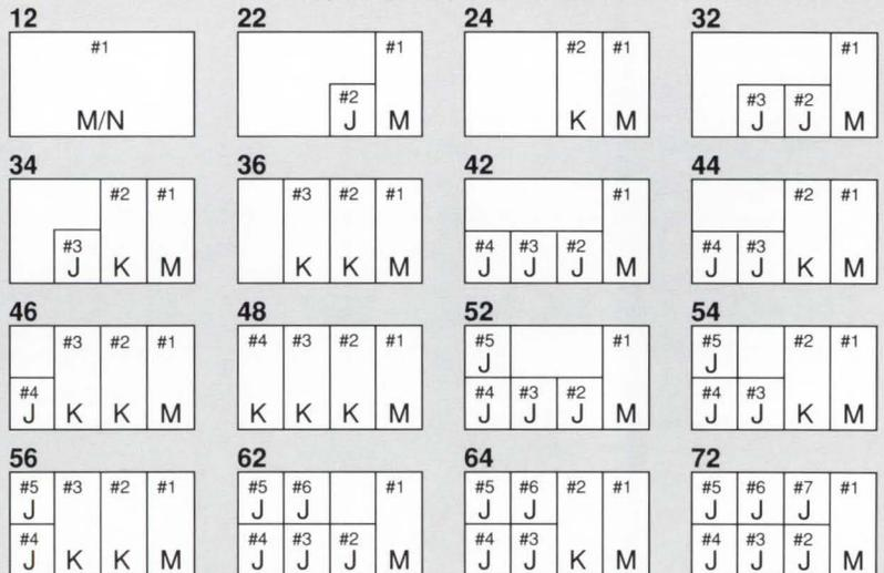
The boxes above are diagrammatic representations of the power supplies as viewed from the output end. The two digit numbers above the boxes are the configuration codes.
