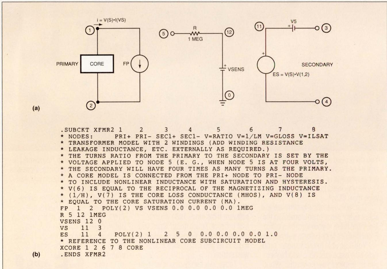
**Fig 1**—The voltage at node 5 controls the turns ratio of this 2-winding transformer equivalent circuit (a) and Spice model (b).
