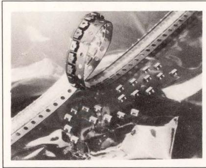
SOT23 package. Both types feature a  $V_{CESAT}$  of 0.3V typ at 1A  $I_C$ .  $H_{FE}$  is a minimum of 40 at the peak  $I_C$  rating of 2A, and increases to 100 at 0.5A  $I_C$ . At a 25°C ambient temperature and mounted on a 0.6-mm substrate of 80 mm<sup>2</sup>, the transistors can dissipate 425 mW. £0.14 (100).
