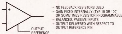
Figure 1. Conceptual Instrumentation Amplifier
