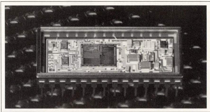
aged in a double-wide, side-brazed DIP, the MN6400 is available in four performance grades and three levels of reliability screening. Prices range from \$175.00 to \$293.25 (100).
