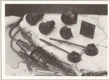
mountings. Pin counts of 2, 3, 4, 6, 7, and 9 and coaxial BNC inserts are optional. The connectors accept cables from 5 to 9 mm in diameter, and offer dust and moisture protection to IEC 529 specification. Maximum current rating is 10A at 250V. In-line 3-way versions have NATO stock numbers. Three-way in-line plug/socket, £8.23 (25).
