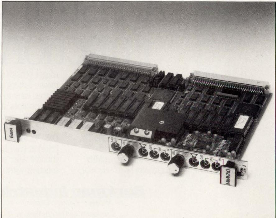
*ADPCM, PCM,  $\mu$ -law, and A-law data-encoding choices, and a programmable sampling rate allow users of the MMI-210 VMEbus audio board to trade off audio-data capacity and sound quality.*
