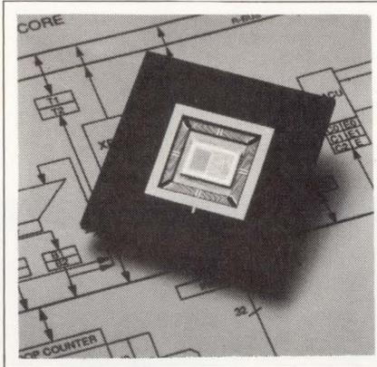
tiplications/sec. In a cycle time of 77 nsec, the device can read two operands, multiply and store, set three address pointers, and handle an I/O operation. The circuit has an operational power dissipation of 350 mW and a standby dissipation of 0.5 mW. The processor is compatible with the CB12000 library of standard cells. Development support includes an assembler/linker, C compiler, VHDL model, and real-time
