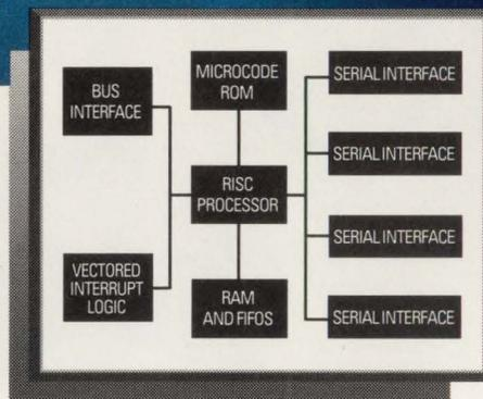
An on-chip 10 MIPS RISC-based processor handles transmit and receive functions, buffer management, flow control, and all special character processing. 84-pin FIFOs reduce host interrupts to give you more efficient interrupt handling. The result: faster system throughput, lower host overhead, and less waiting.
