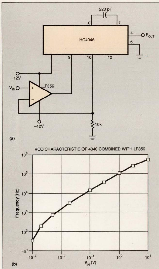
Fig 1—Using the HC4046's internal transistor (a) instead of an external component achieves the linearization in b.
