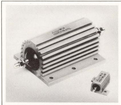
creases to 300W with additional heat sinking. You can specify inductive or noninductive windings and resistance tolerance from 1 to 10%. Terminations cater to solder, threaded, or fast-on connections. 300W type, DM 84 (100).
