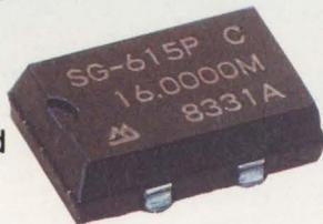
Epson has pioneered the first truly heat resistant crystal for use in its surface mount crystals and crystal oscillators. Capable of withstanding 260°C for 20 seconds... far above the demands of standard IR and vapor phase reflow processing systems... these labor-saving high-temp SMD crystals have become the accepted standard for surface mount crystal and oscillator components.
