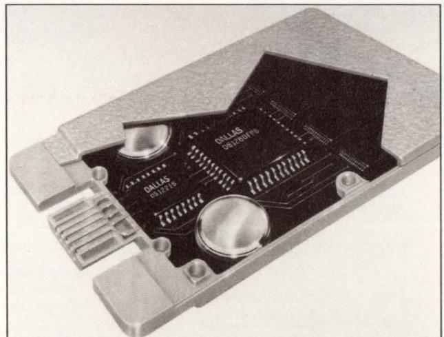
*Providing 10 years of nonvolatile static-RAM storage for as much as 4M bits of data, CyberCard withstands harsh environments and provides a connector life of 50,000 insertion/extraction cycles.*
