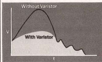
They're widely used for incoming AC protection and clamping circuits. And they're available in a wide range of packaging—axial leaded, radial leaded, leadless surface mount, high-energy modules and connector-pin configurations.
