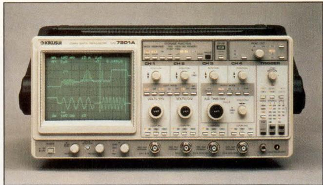
Both analog and digital operation are available on the 200-MHz 7201A from Kikusui. The 4-channel DSO also includes an IEEE-488 interface.
