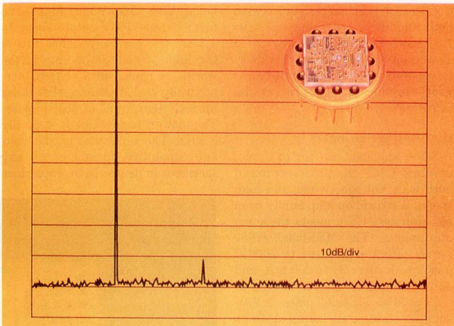
**Current-feedback architecture** takes the credit for the high speed of Comlinear's CLC207 op amp. The  $\pm 15\text{V}$  device delivers  $\pm 150$  mA to its load and slews at  $2400\text{V}/\mu\text{sec}$ .
