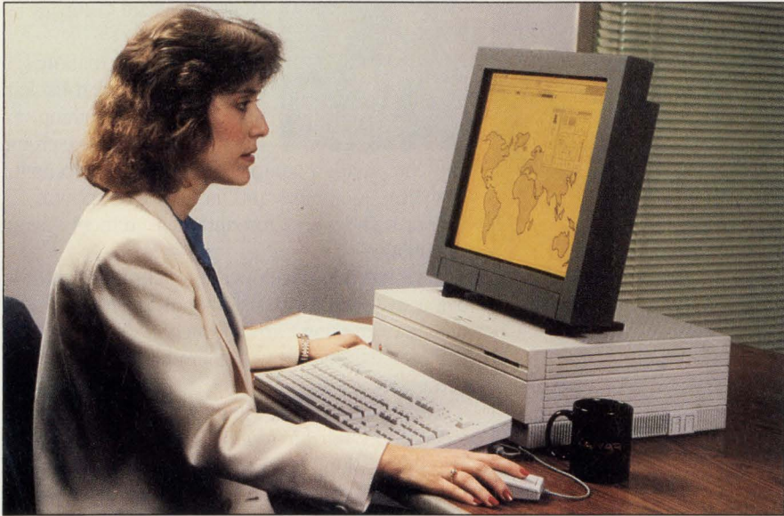
This electroluminescent display, the EL751214M from Planar Systems, features a diagonal measurement of almost 18 in. The monitor has a viewing angle of 160°, weighs less than 15 lbs, and takes up less than 50 in. 2 of work area.
