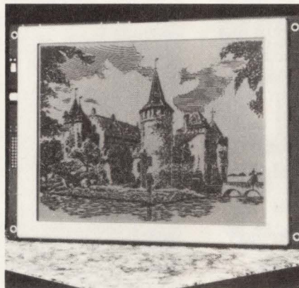
Using a 2-terminal active matrix, this monochrome LCD from Seiko Instruments has a 10-in. diagonal viewing area and a resolution of 640 x 400 pixels.
