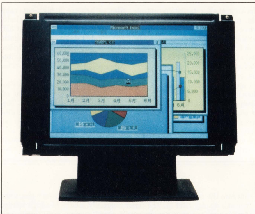
Containing 921,600 pixels, this 10-in. color LCD from Sharp Electronics has a VGA-compatible resolution of 640 \times 3 \times 480 pixels. The display uses an active-matrix technology with a thin-film transistor for each pixel.
