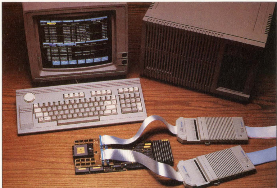
To support the 88100, Tektronix's DAS 9200 uses the 92DM35 support package. A single connector probes the 181-pin PGA. The analyzer monitors all cached and noncached program activity in real time at speeds as fast as 33 MHz.
