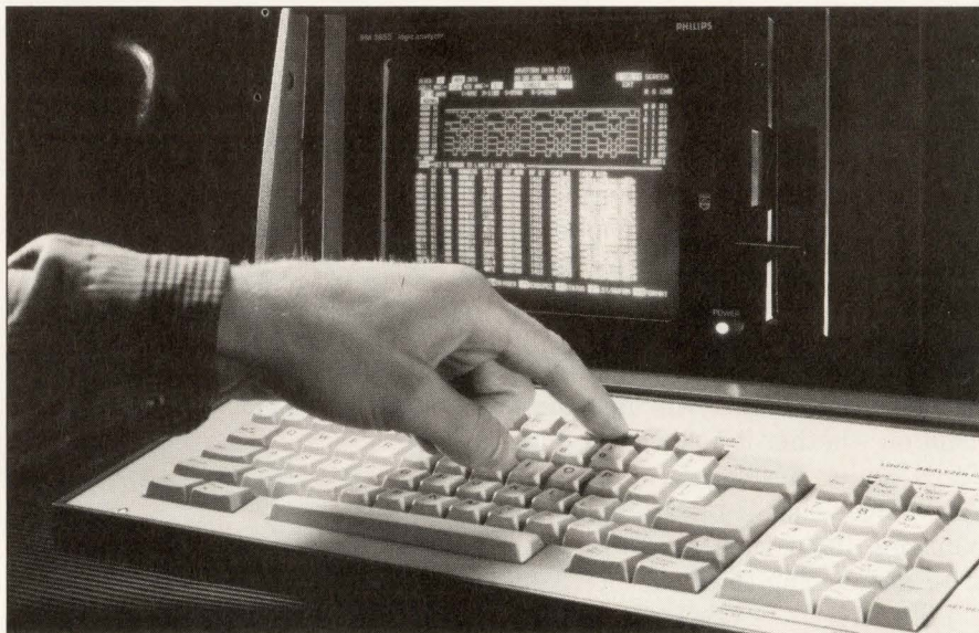
State-analysis at 100 MHz; capacitive loading of 8 pF max; custom disassemblers for RISCs, including Intel's i960CA; and an integral IBM PC/AT-compatible computer make the PM 3655 logic analyzer from Philips/Fluke an excellent choice for RISC debugging.
