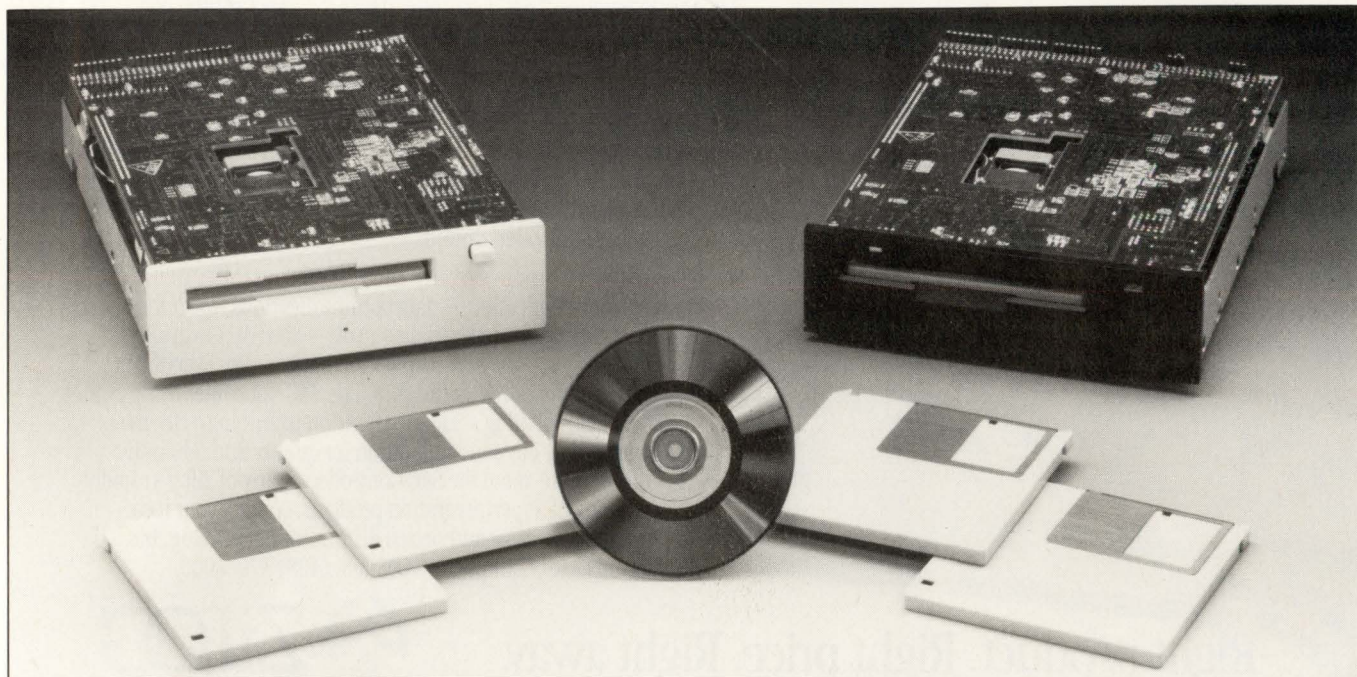
The 30-msec average seek time of the RMD-5100-S optical drive makes the unit competitive with magnetic drives. Furthermore, the 133M-byte unit employs ANSI-standard 3½-in. media and fits in a standard half-height 5¼-in. drive slot.
