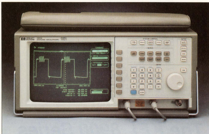
With a rate of 1G samples/sec, the HP54510A DSO makes accurate measurements of single-shot events using waveform reconstruction.
