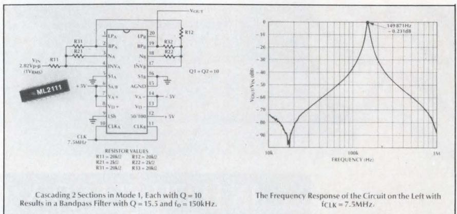
low-offset (15-mV max) voltage amplifier, a voltage summer, two integrators, and control logic. The filters maintain their specifications when operating from  $\pm 5\text{V}$  supplies with  $\pm 10.0\%$  tolerances. The device can also operate from a single  $5\text{V} \pm 10\%$  supply at a maximum operating frequency of 100 kHz. An
