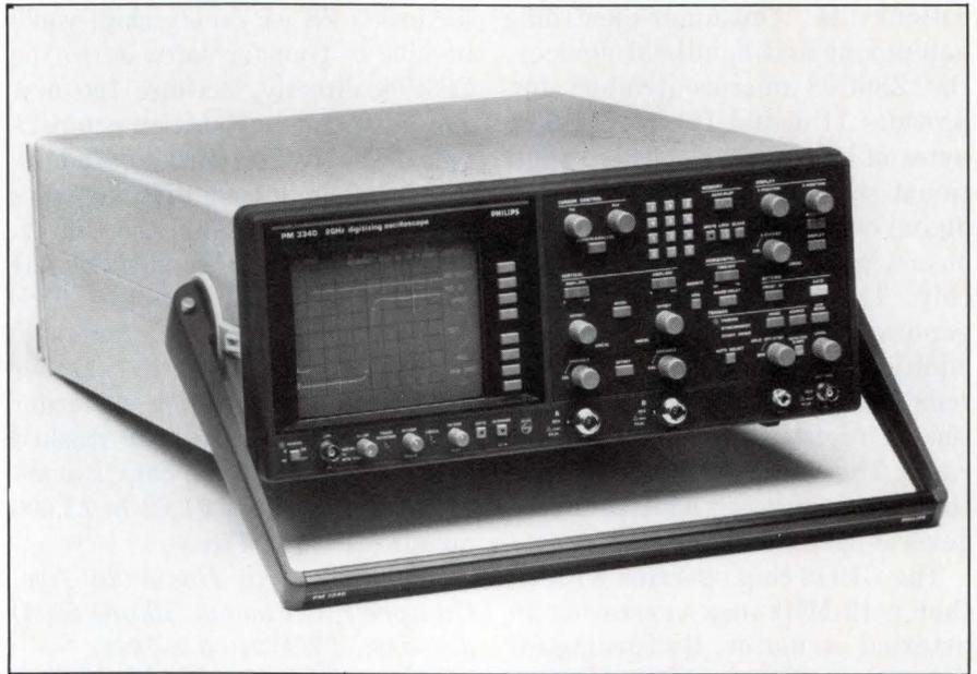
*The front panel of the PM 3340 resembles that of an analog scope, but the row of softkeys to the right of the screen and the keypad reveal its digital heritage.*
