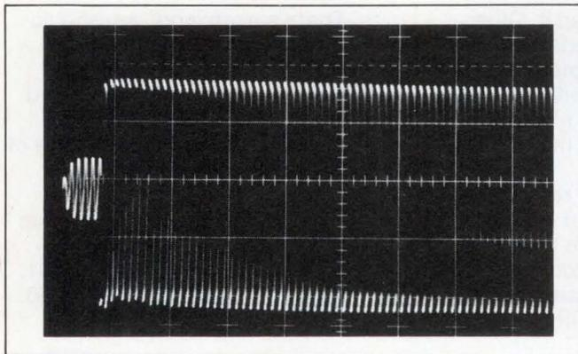
Fig 1—The ringing that follows excitation of a piezoelectric transducer can last for 20 msec, masking the echoes from targets within 10 ft of the transmitter. In this photo, scale is 5V/div in the vertical axis and 200  $\mu$ sec/div in the horizontal axis.
