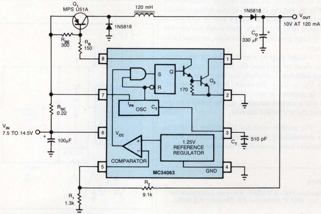
Fig 1—Using a single inductor, a switching-regulator IC, and a few external components, you can build a step-up/step-down switching regulator.
