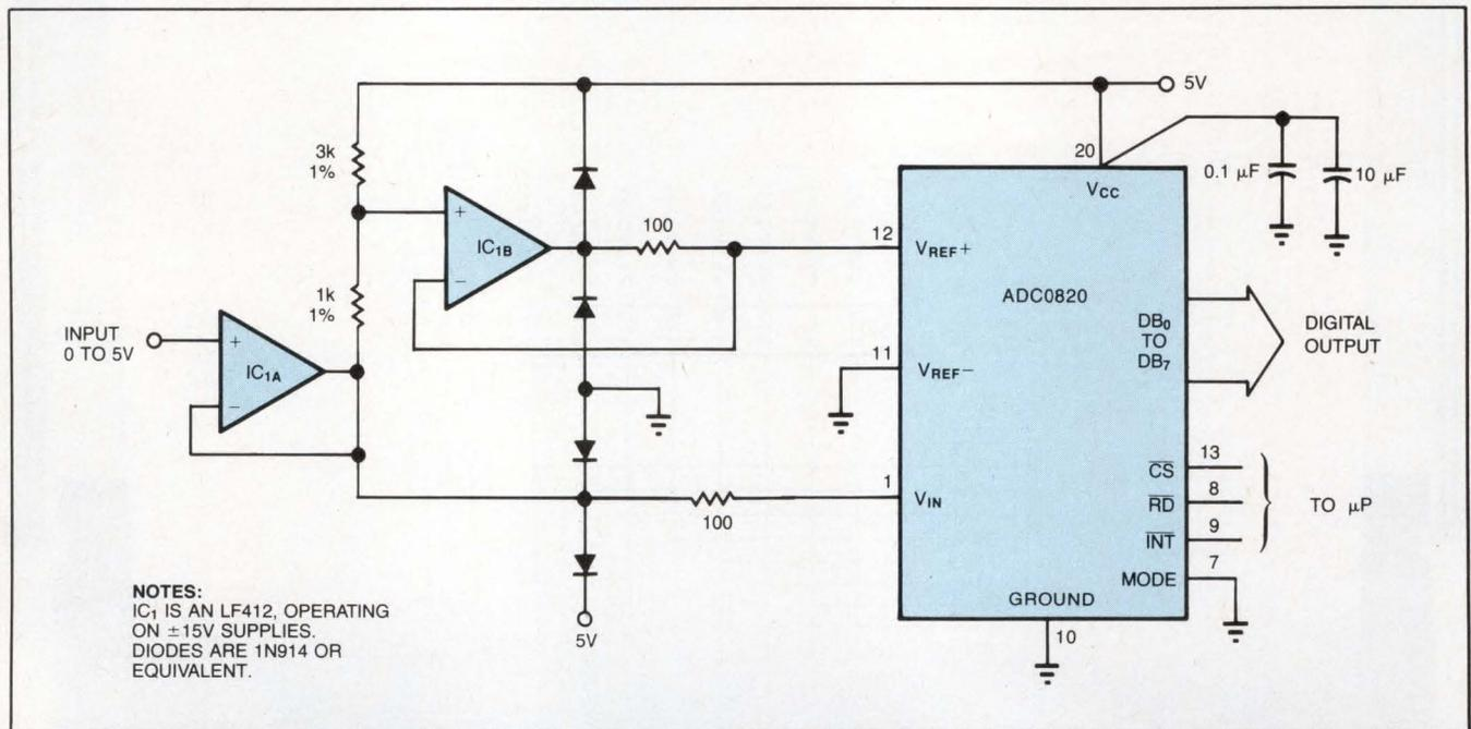
Fig 1—You can increase an A/D converter's apparent resolution by combining the input signal with a fixed reference voltage and feeding this sum to the converter's reference input.
