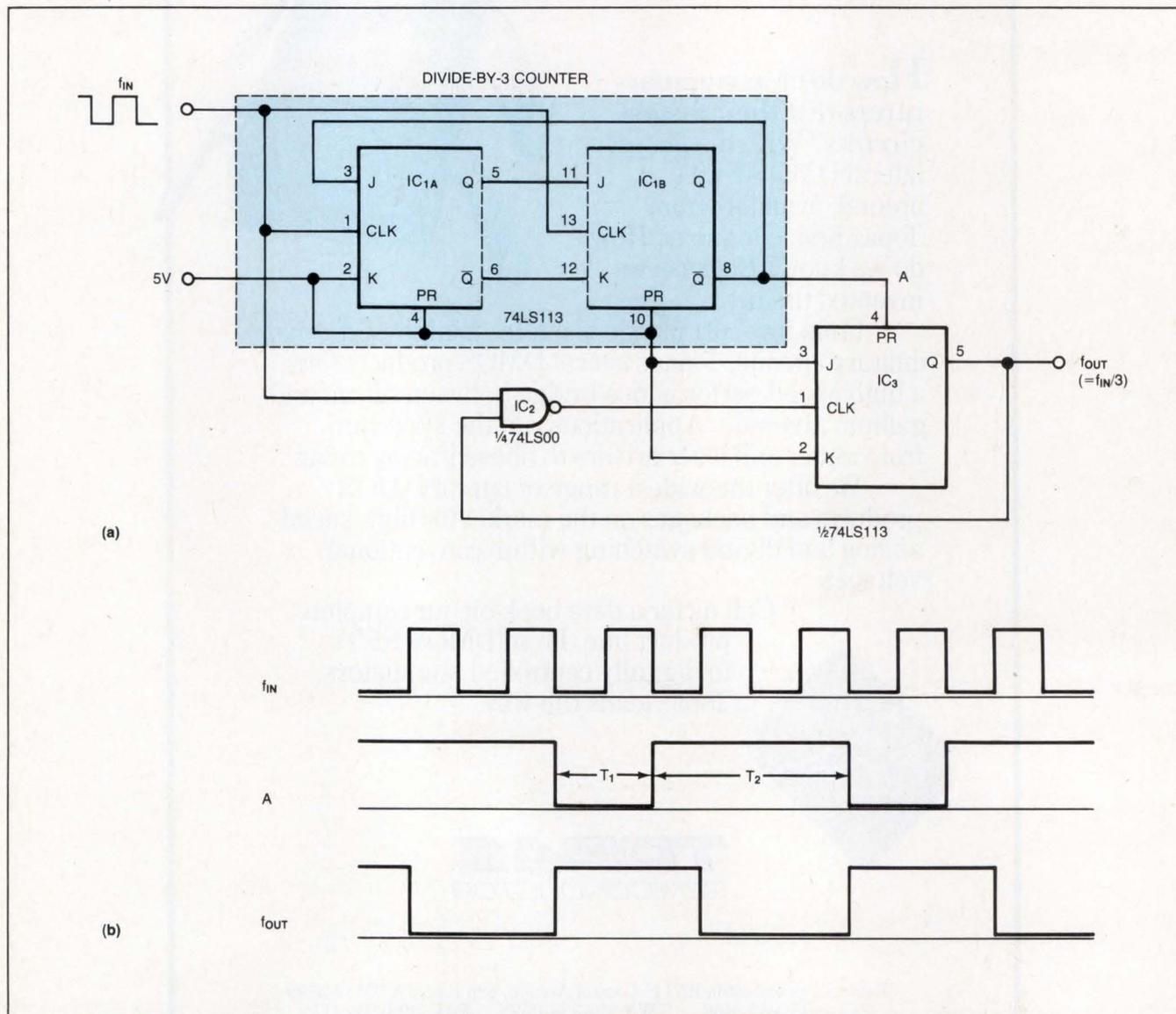
Fig 1—Odd-integer division performed using a divide-by-3 counter (a) produces the asymmetrical waveform (such as the one labeled A in part b), but you can add additional circuitry to generate a symmetrical f<sub>OUT</sub> signal.
