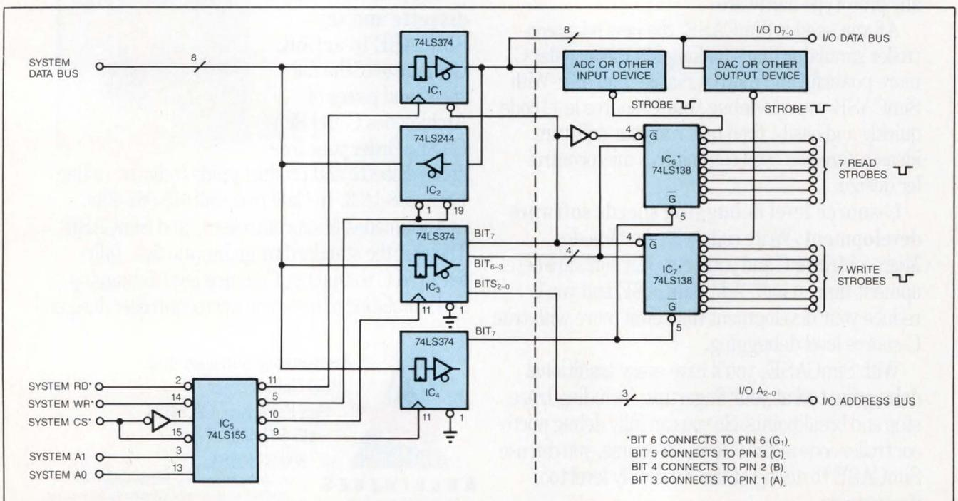
Fig 1—By adopting this foolproof, latched-I/O scheme as a standard for  $\mu$ P-based systems that must handle parallel I/O, you can quickly adapt it to different tasks.
