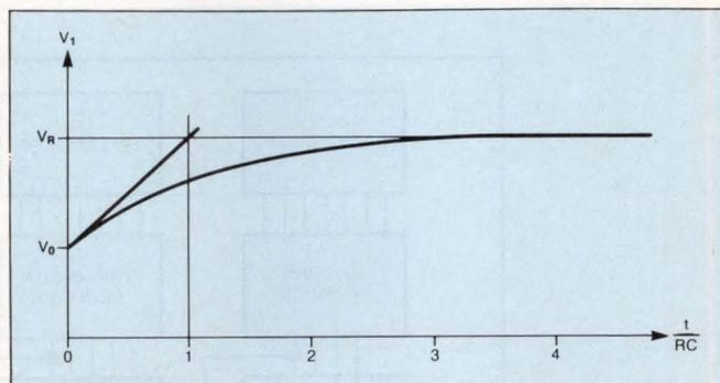
**Fig 3**—This curve shows the variation of  $V_1$  following closure of  $S_1$  and caused by the charging of capacitor  $C_1$ .
