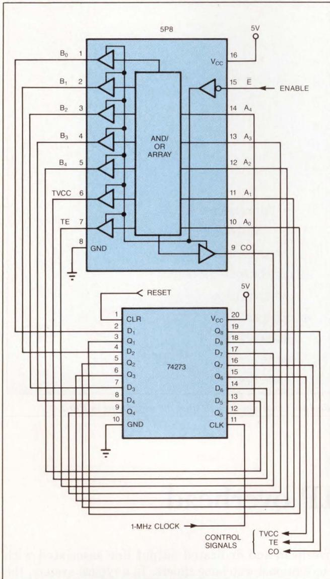
Fig 1—A state machine consisting of a 5P8 PAL and an octal flip-flop generates programming-timing control signals for programming common PALs.
