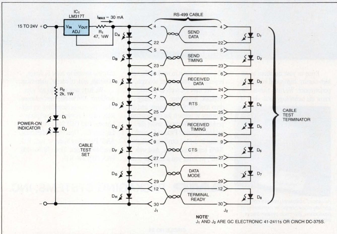
Fig 1—By driving two LED strings from a common current source, you can quickly check a cable of twisted-pair wires for short circuits, open circuits, and pair-to-pair shorts.
