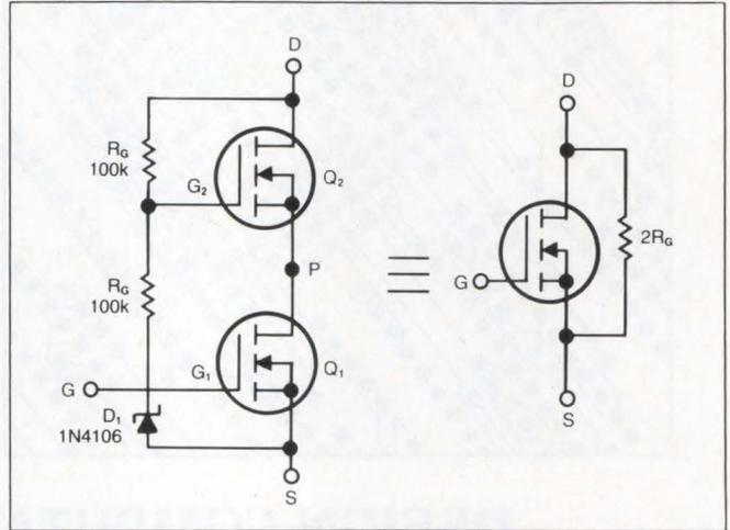
Fig 1—Double a MOSFET's  $BV_{DSS}$  by connecting two units in series. This composite device behaves as shown in the equivalent diagram.
