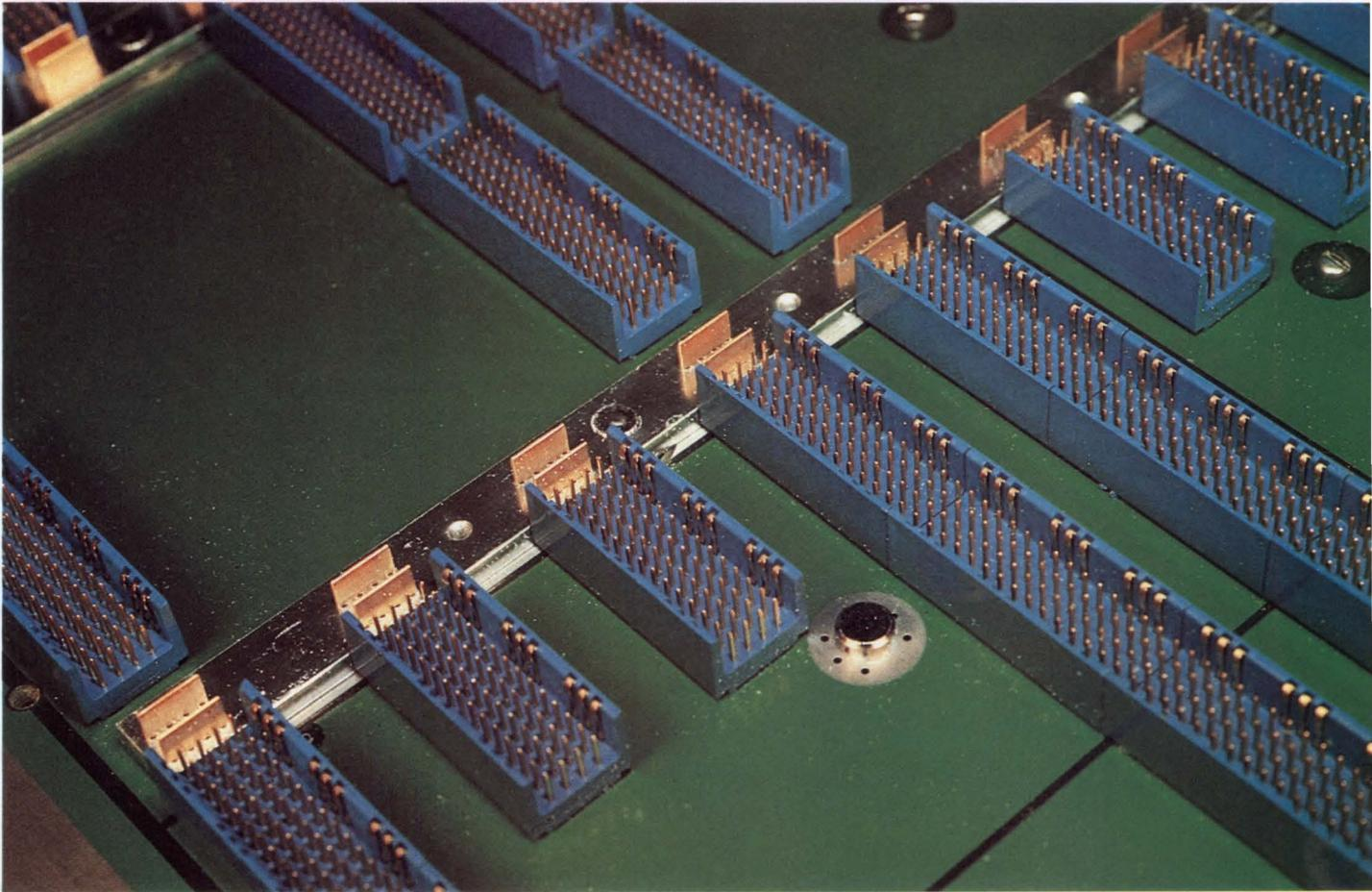
*Backplane with modular connectors (Teradyne Connector Systems)*
