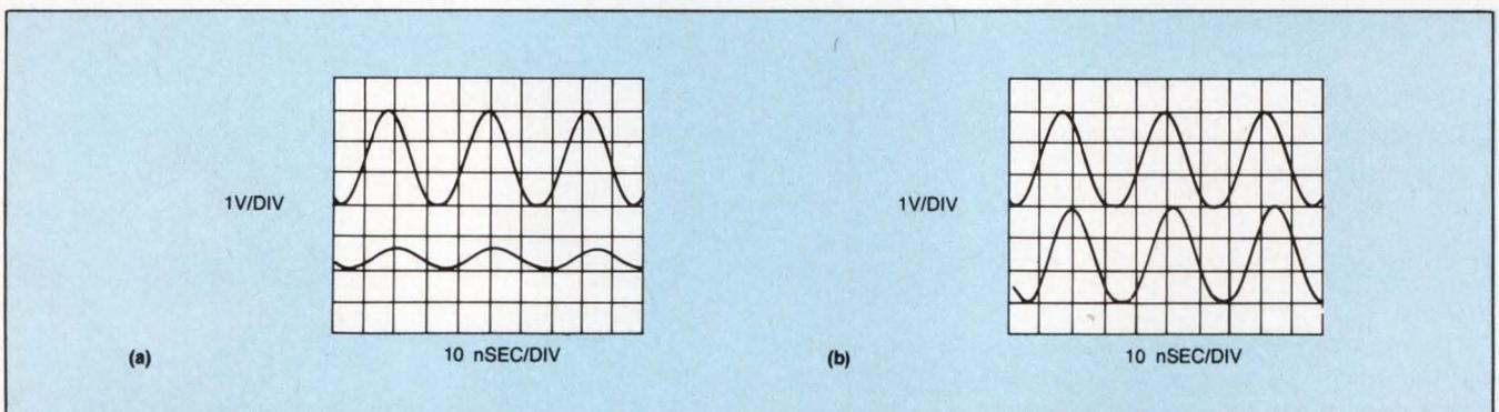
Fig 1—These input (top) and output (bottom) waveforms show the frequency-response improvement that results when you modify the LH0002 current amplifier (whose response is shown in a) by adding the external components in Fig 2. The improvement illustrated in b results when  $R_S=1$  k $\Omega$ ,  $R_L=50\Omega$ , and frequency equals 30 MHz.
