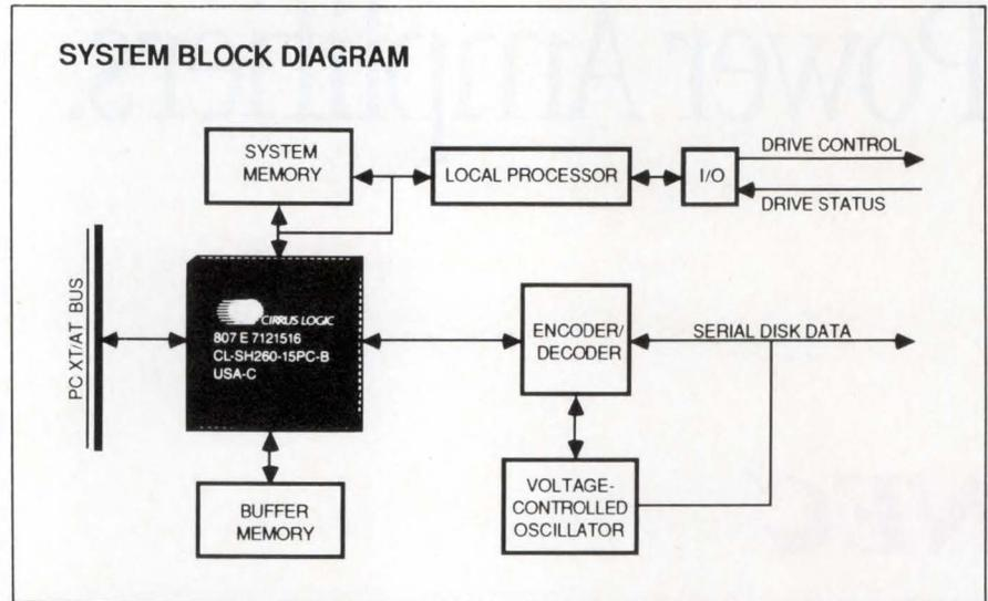
late the IBM Task File for the PC/AT and the IBM Command Descriptor Block for the PC/XT. The chip can sustain a 2M-byte/sec transfer rate to the disk and a 4M-byte/sec transfer rate on the host
