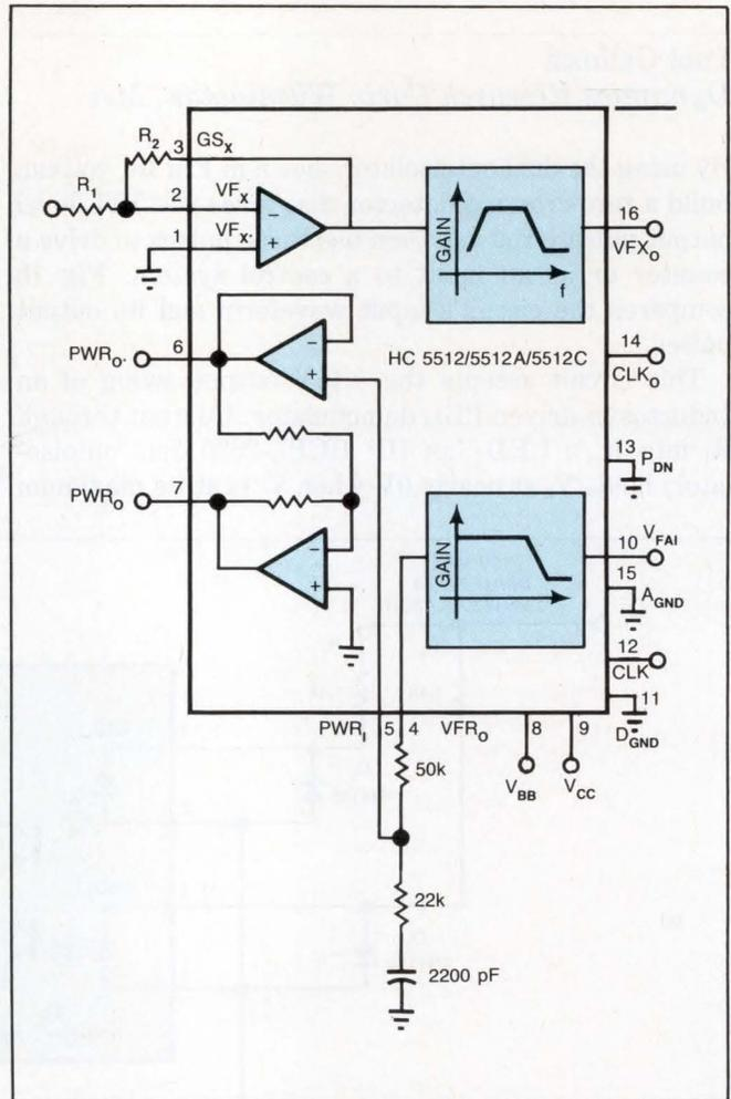
**Fig 1—You can program this PCM filter to act as either a lowpass or highpass filter. By varying the chip's external clock frequency between 300 kHz and 5 MHz, you can select filter cut-off frequencies between 200 Hz and 10 kHz.**
