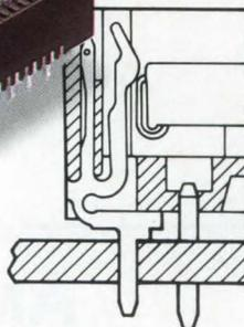
Controlled contact interface angle in AMP HPT sockets ensures positive chip carrier retention. Our exclusive removable housing allows direct inspection of solder joints, and fast repair/replacement of contacts.
