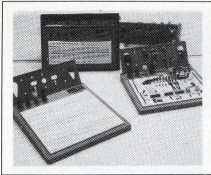
into DIP-spaced breadboard socket connections. The boards come in four models that offer from 810 to 2940 tie-points. Each model includes an area containing both distribution and terminal strips that accommodate all DIP sizes, lead components, and wire gauges of 20 to 29 AWG. The phosphor bronze, nickel-plated contacts provide a 3-mΩ initial contact resistance and a 10,000 in-out-cycle min lifetime rating. Each breadboard features four multipurpose binding posts. \$16.95 to \$59.95.
