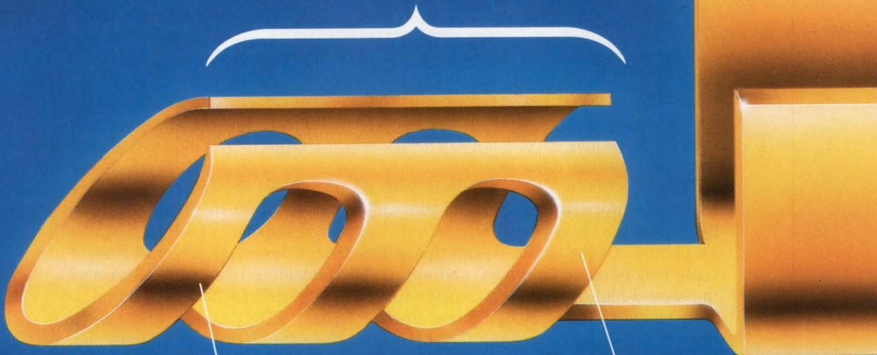
DuPont RIB-CAGE™ connectors feature a three-rib contact that delivers 100 grams of normal force.
