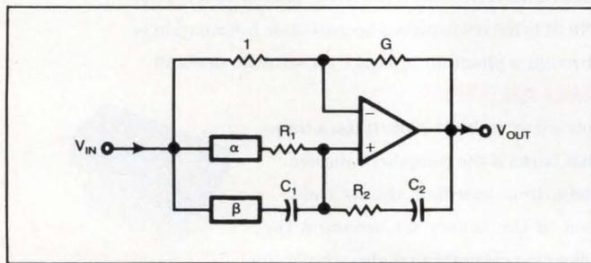
Fig 1—Use this building-block circuit to generate the pole-zero pairs used in bandpass-filter design.
