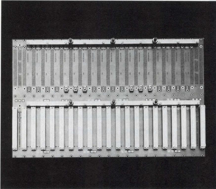
*Monolithic backplane with press-fit construction (Bicc-Vero Electronics)*
