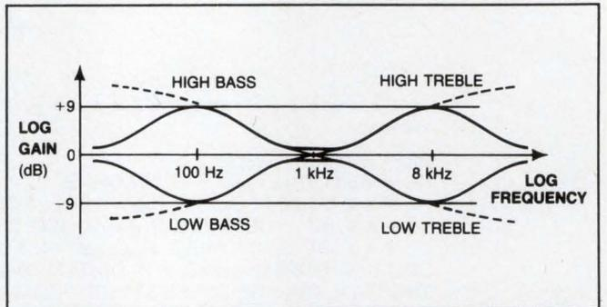
**Fig 2**—The frequency response of the dual-filter tone control (**Fig 1**) shows little effect at 1 kHz but  $\pm 9$ -dB variation in the treble and bass regions. For comparison, the dashed lines show the response of a Baxandall tone control.
