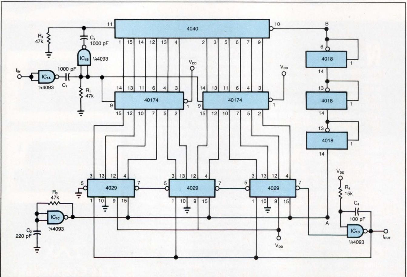
**Fig 1**—You can multiply frequency  $f_{IN}$  from eight to 1000 times by using 10 CMOS ICs and several passive components.
