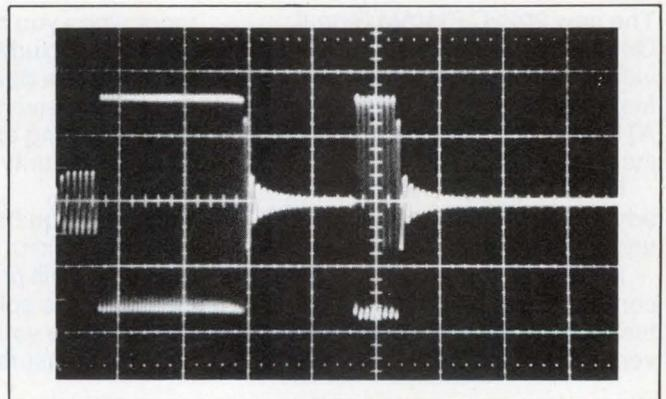
Fig 2—Ring duration for an electrostatic transducer is less than 1/20th that of a piezoelectric type, allowing easy recognition of an echo that occurs 800  $\mu$ sec after the transmit pulse begins. Here, scale is 5V/div in the vertical axis and 200  $\mu$ sec/div in the horizontal axis.
