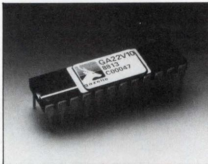
inputs and ten 3-state outputs that you can program for registered or combinatorial data with active-high or active-low polarities. It also has a
