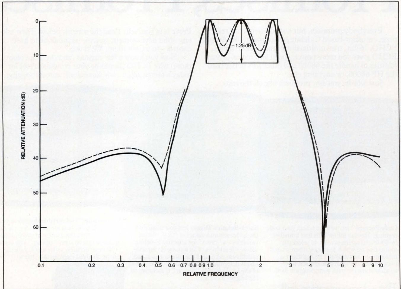
Fig 3—The bandpass filter's performance changes only slightly when you change its center frequency from 1.6 kHz (solid curve) to 16 kHz (broken curve) by scaling capacitor values.
