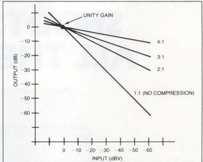
Fig 2—The input/output transfer-function curves of the circuit in Fig 1 show the four possible signal-compression slopes and the unity-gain point for each slope.
