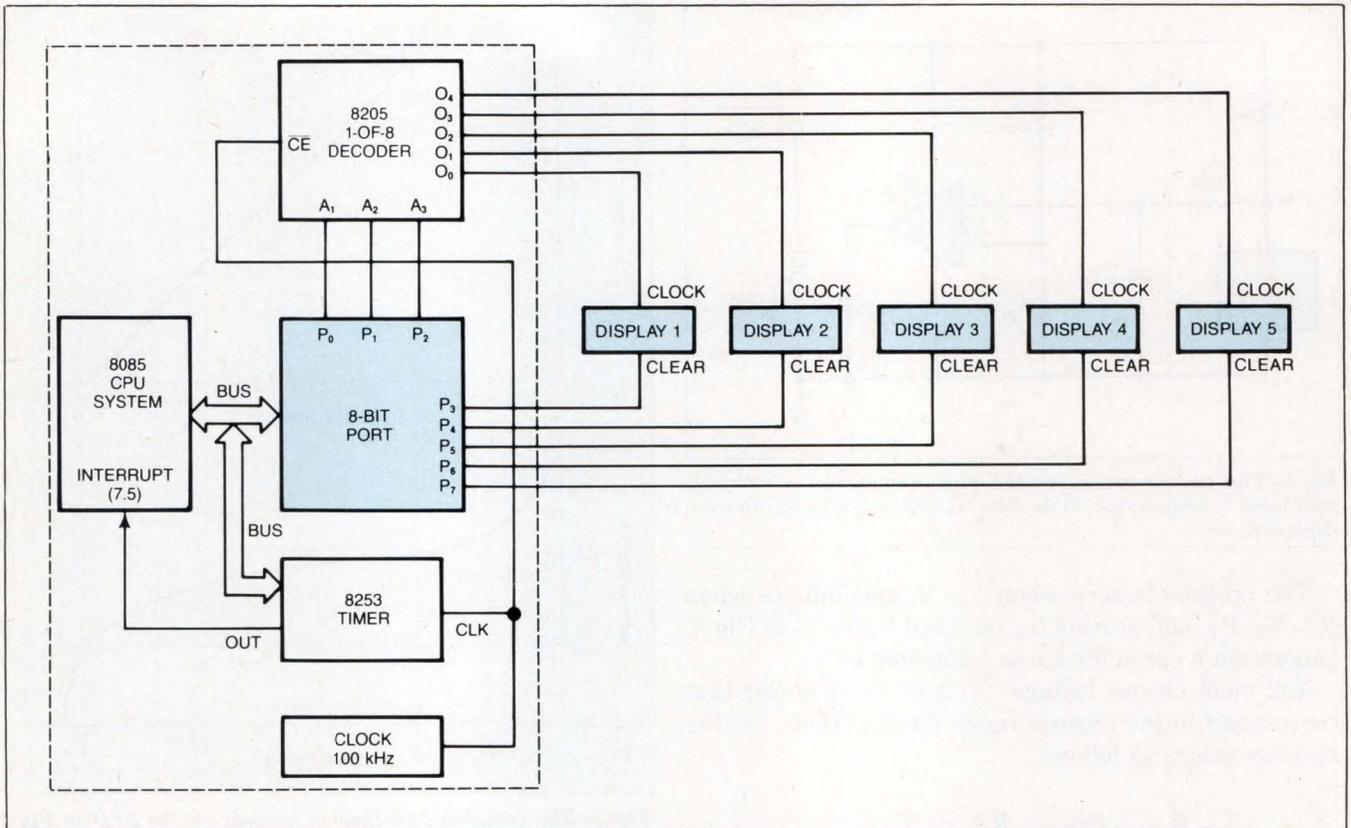
Fig 1—One 8-bit port drives five displays, each with an arbitrary number of digits. Each display requires only two signals, Clock and Clear.
