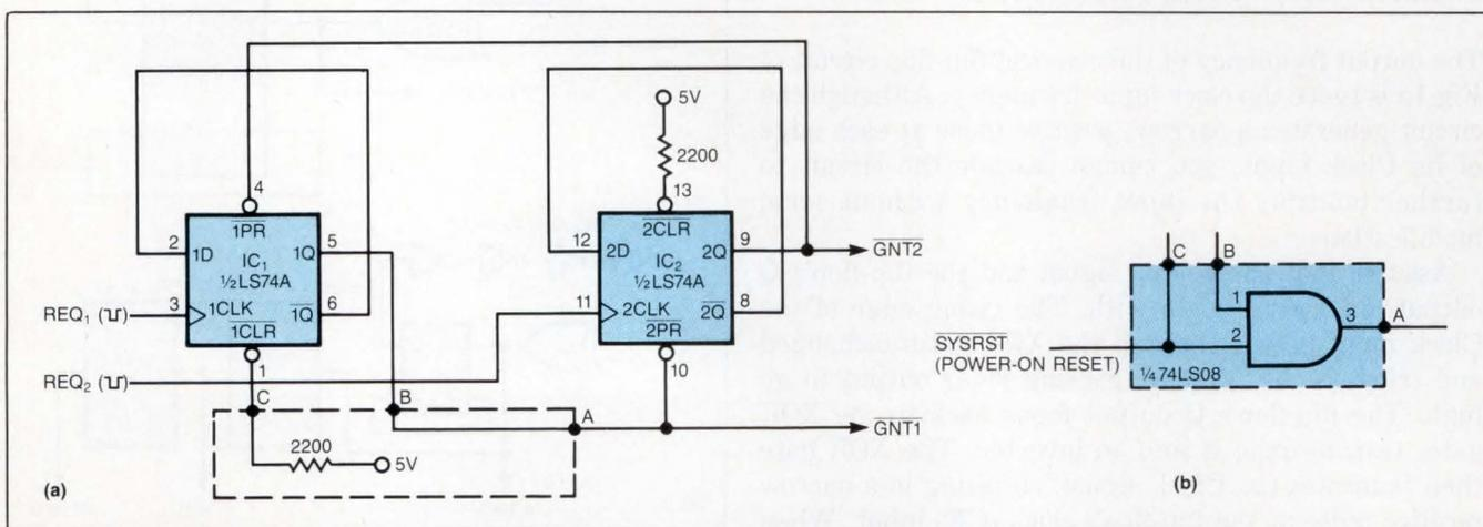
**Fig 1**—A pair of back-to-back flip-flops can arbitrate access to a shared resource. A master requesting access will be blocked until the second master relinquishes control because each resource-grant flip-flop, when active, engages the other flip-flop's preset input. The AND gate in **b** forces the circuit to a predetermined state upon power up.
