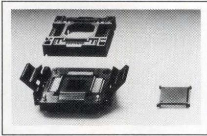
cepts devices with 52, 68, 84, 100, and 132 leads. The hinged-lid socket accepts devices with 84, 100, and 132 leads. The insulation material is polyethersulphone/polyetherimide. The contacts are made of beryllium-copper and feature gold-over-nickel plating. 132-pin socket and carrier, \$92.11 (100).
