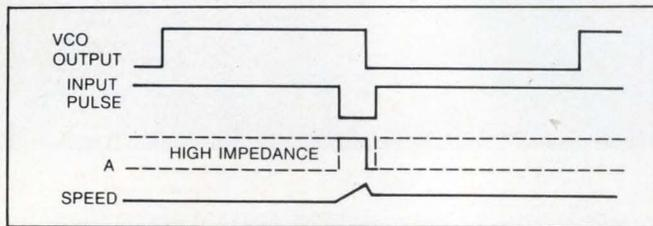
Fig 2—The output of Fig 1's VCO is high when an input pulse occurs; simultaneously, the 3-state buffer's output is high, and capacitor C charges. Then, the VCO's output goes low, the buffer's output goes low, and the capacitor discharges.
