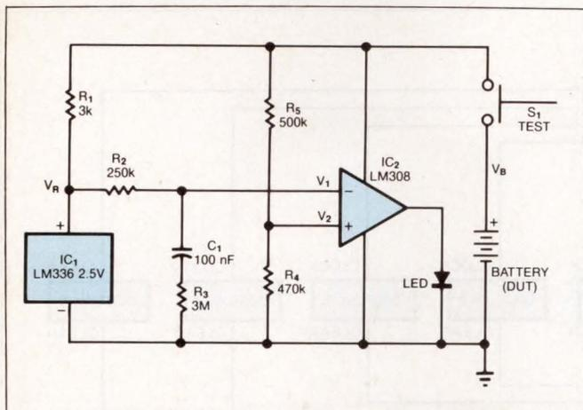
**Fig 1**—This test circuit checks the remaining charge in a battery; the charge is proportional to the time the LED remains on after you depress  $S_1$ .
