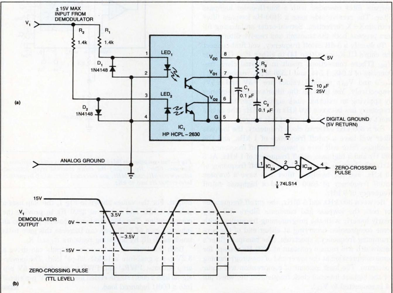
Fig 1—A dual optoisolator and a handful of components make up a circuit that provides a glitch-free pulse for each detected zero crossing.
