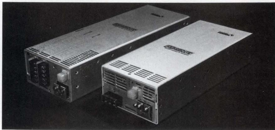
ture a modular design that provides one to seven outputs. Their line- and load-regulation performance is 0.2% or 10 mV max, and their switching frequency measures 100 kHz. The units' efficiency figures range from 70 to 85%. The maximum ripple and noise specs (for a 20-MHz bandwidth) are 1% or 50 mV for the main
