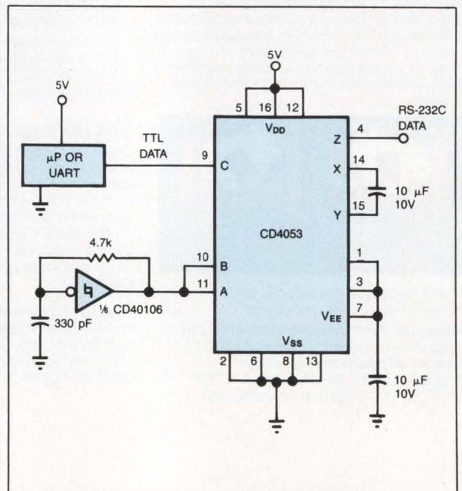
**Fig 1**—Two inexpensive ICs convert serial TTL data to a bipolar format suitable for transmission on RS-232C lines.
