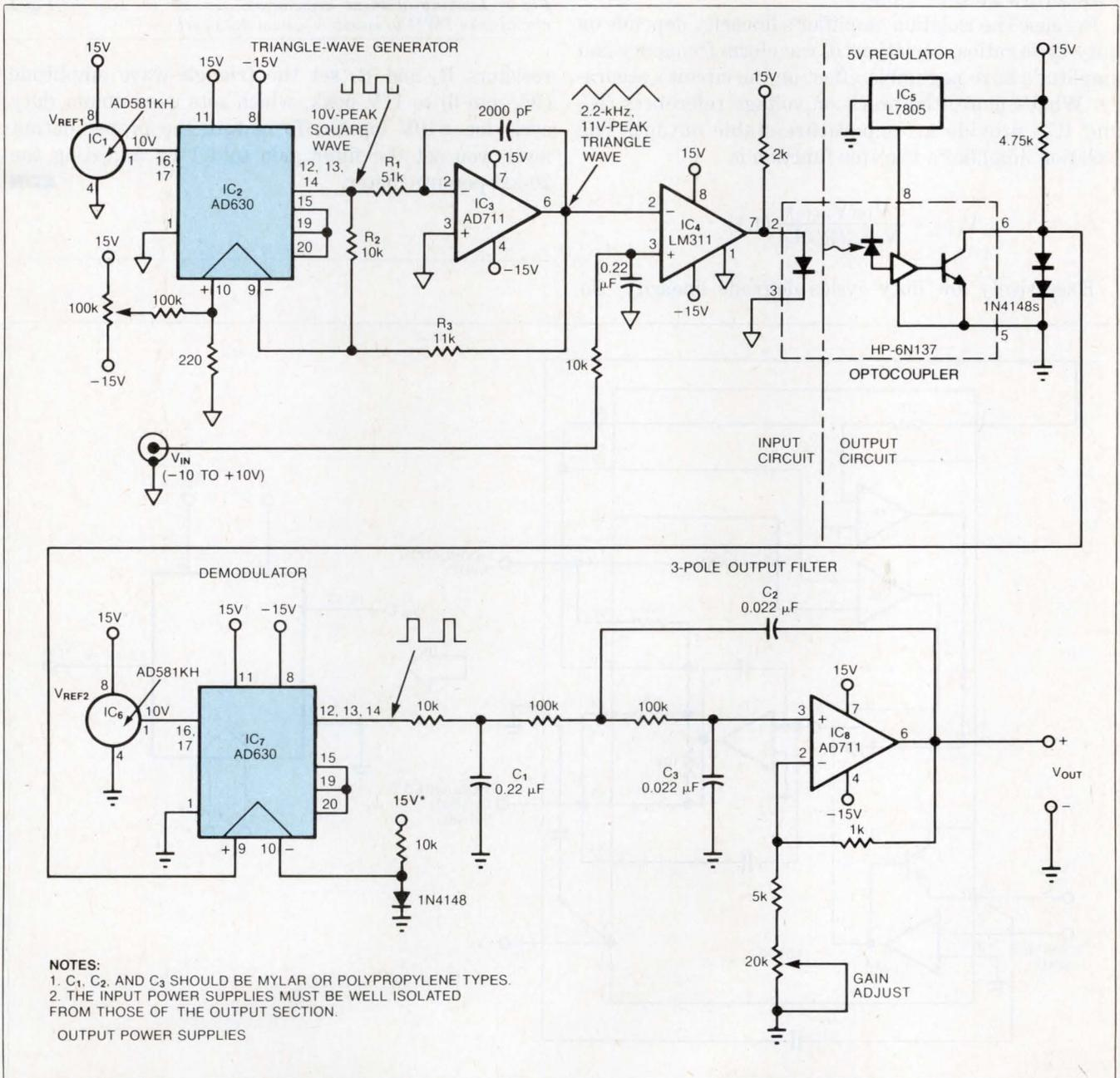
Fig 1—This isolation amplifier employs PWM and optocoupling to transfer low-frequency signals across a barrier of 3 kV or more.
