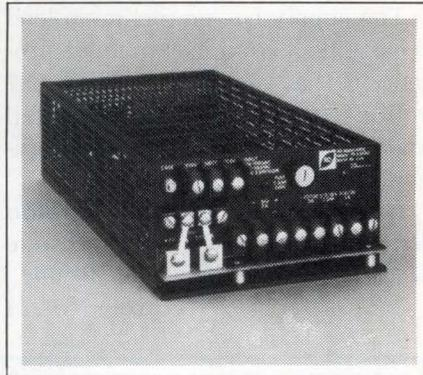
dary windings. The supply outputs are 5V at 20A, 12V at 3A, -12V at 2A, and 24V at 2A (for disk-drive applications).
