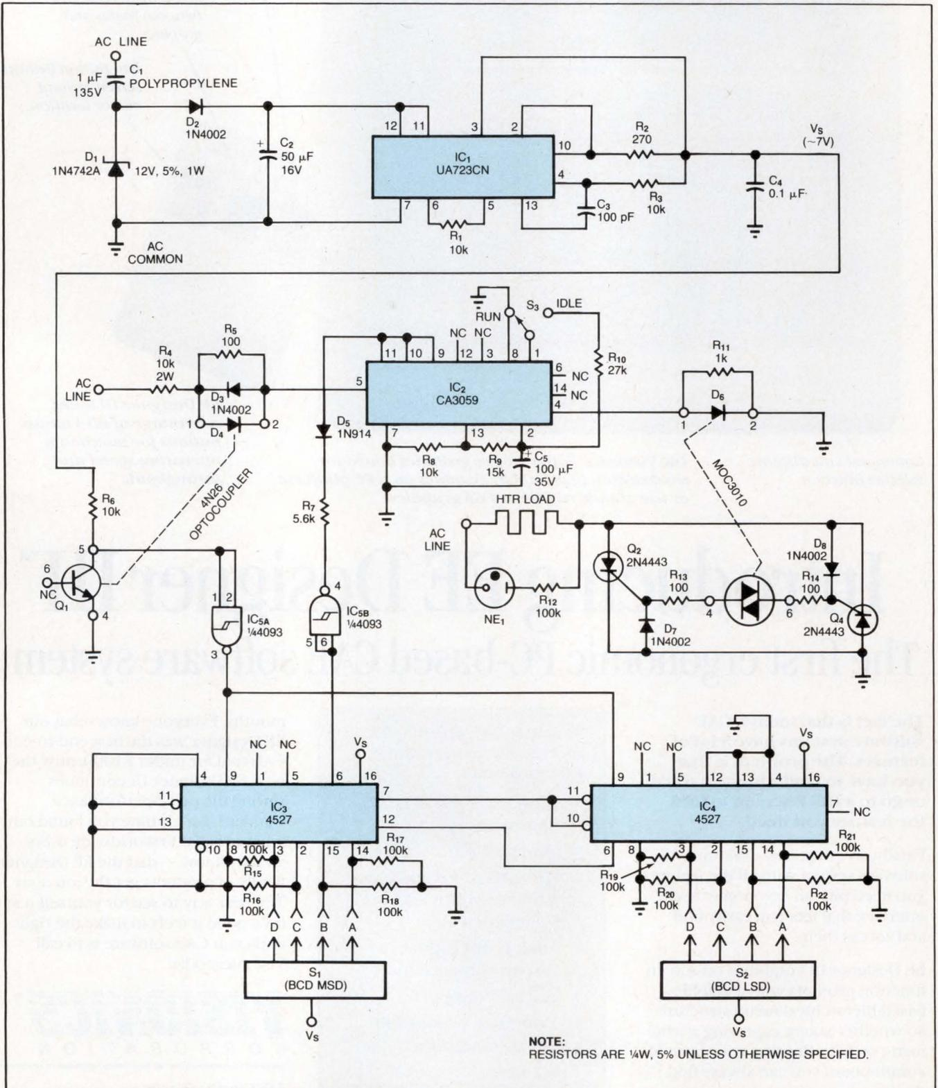
**Fig 1—A low-power circuit provides digital control of 1 kW, or more, in 1% steps. A zero-crossing detector ensures that only an integral number of full line cycles reach the load during any 1.67-sec control period.**
