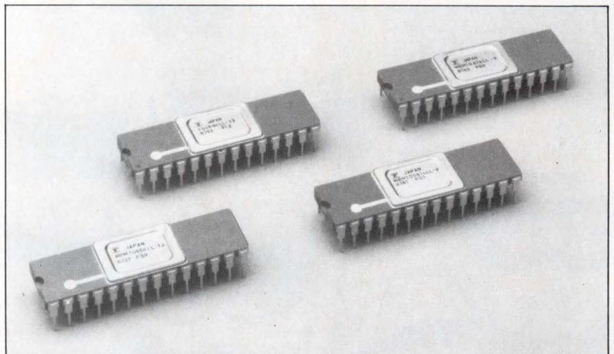
it's compatible with 100K ECL products. The devices come in 28-pin ceramic DIPs. The 1k×4-bit units cost \$55 (1000); the 4k×4-bit devices sell for \$75 (1000).
