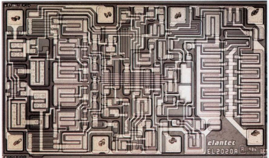
The settling-time performance of current-feedback op amps makes them equally attractive as an output stage for high-speed D/A converters. As a bonus, if you use the op amp in an inverting gain mode, the low input impedance of the op amp's inverting input effectively shorts out the output capacitance of the D/A converter, reducing the effect that this capacitance has on the overall settling time.
