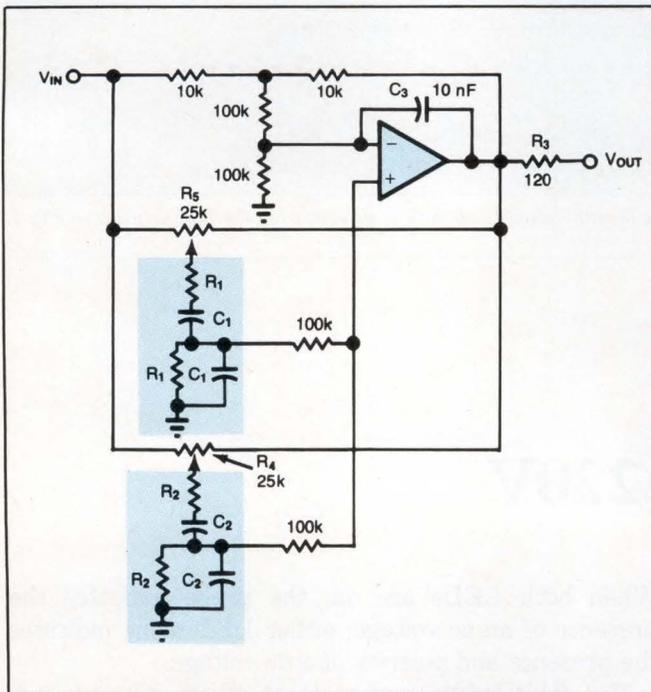
**Fig 1**—This audio filter's two Wien-bridge networks provide  $\pm 9$  dB of tone control for treble and bass frequencies.
