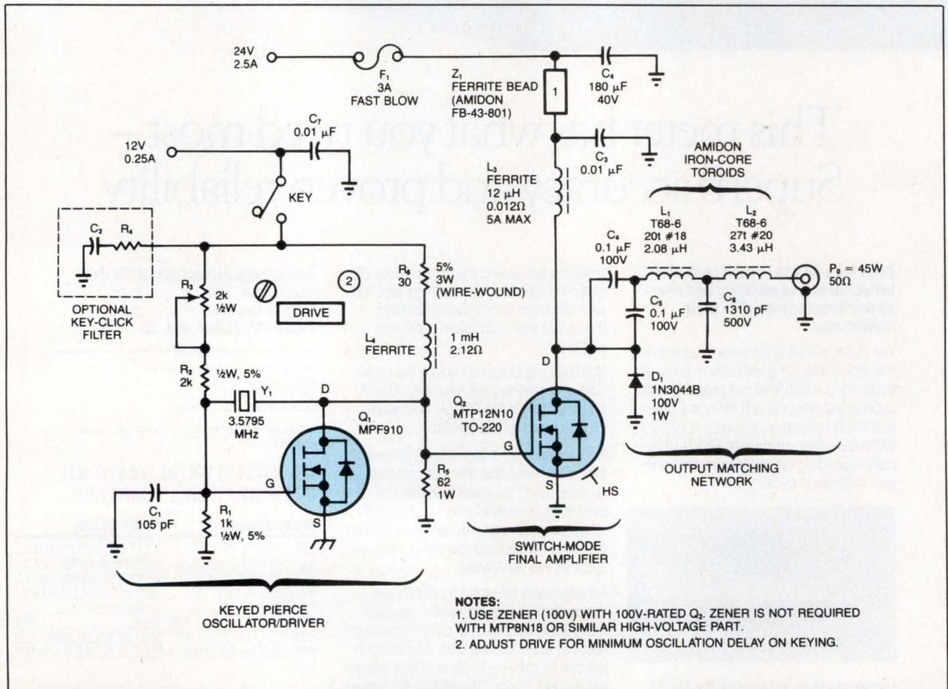
Fig 1—This 80m amateur-radio transmitter includes one MOSFET for the oscillator and a second MOSFET for the final amplifier.
