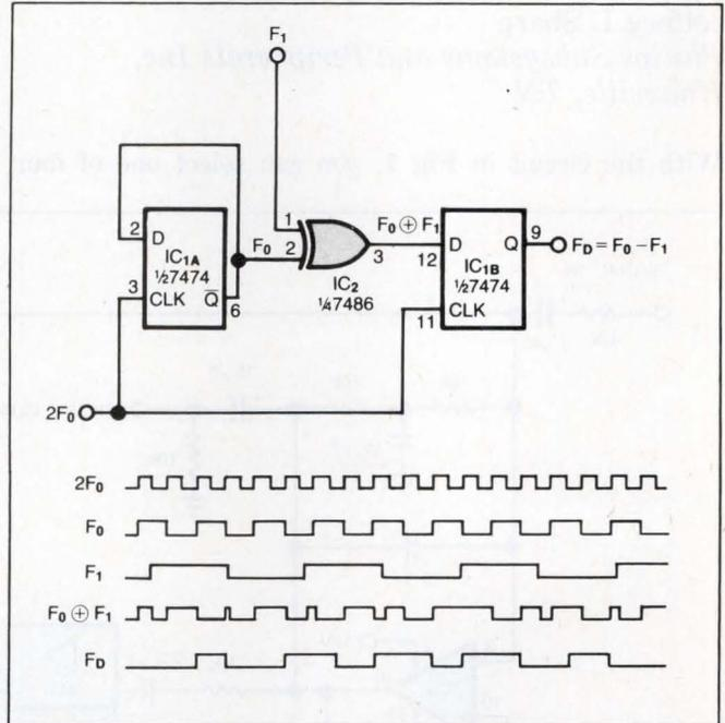
Fig 1—Two ICs generate the frequency difference between  $F_0$  and  $F_1$ .
