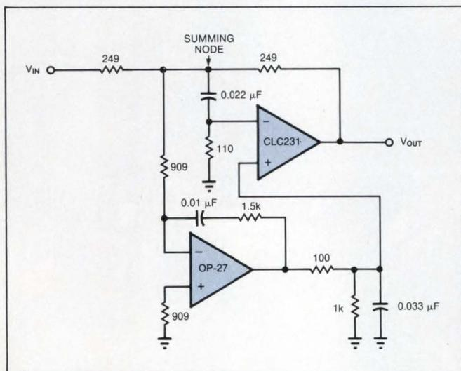
**Fig 1**—This composite op-amp circuit combines the low offset and drift of the OP-27 op amp with the high speed of the CLC231 current-feedback op amp to produce a circuit that settles to 0.1% in 17 nsec, yet maintains high dc accuracy. The OP-27 maintains the summing node at an accurate virtual earth potential; the CLC231 takes over at high frequencies to provide good ac performance.
