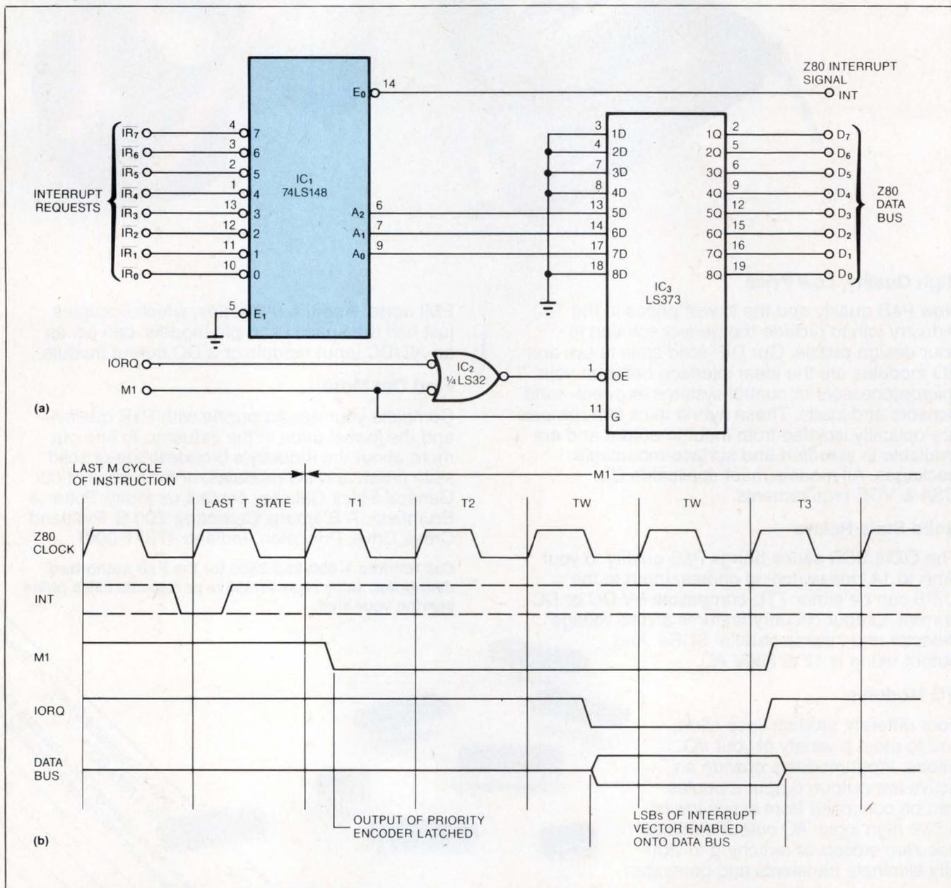
**Fig 1**—This circuit handles as many as eight interrupts in a Z80-based system without using specialized peripheral devices (a). The timing diagram (b) shows that the interrupting device must identify itself by supplying an 8-bit vector while  $\overline{M1}$  and  $\overline{IORQ}$  are low.
