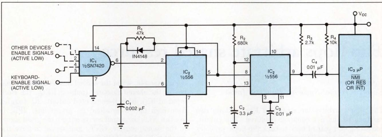
Fig 1—This watchdog timer saves  $\mu$ P overhead and eliminates a dedicated output line. It uses the  $\mu$ P's input-enable signals to retrigger its one-shot rather than employing a specific watchdog-timer command.
