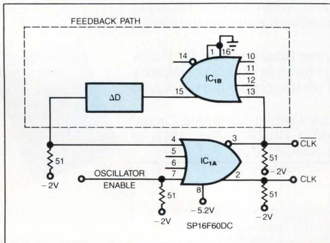
Fig 1—Two ECL gates and an optional delay line provide a 300-MHz gateable oscillator.
