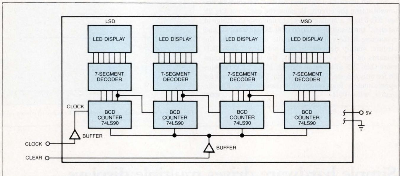
Fig 2—A typical display in Fig 1 includes a digit display, 7-segment decoder, and BCD counter for each digit.
