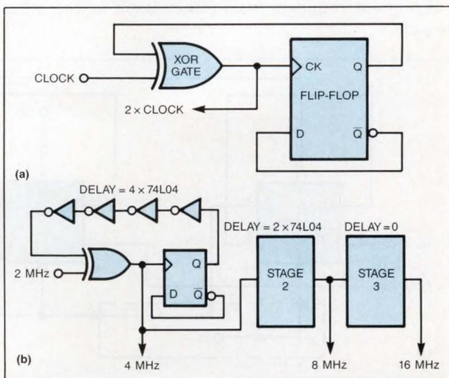
Fig 1—A simple circuit can double the clock input frequency (a). However, you cannot cascade such doublers unless you insert appropriate delays in the feedback paths as in b.
