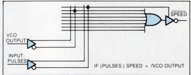
Fig 3—Using a PLD with 3-state outputs, you can implement Fig 1's circuit. Just connect the pulse source to a gate's output enable and the VCO's output to the gate's input. Because these PLDs have inverted outputs, you'll have to invert some signals.
