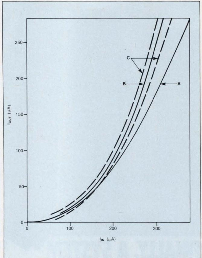
**Fig 2**—These curves illustrate the performance of **Fig 1**'s circuit. The curve labeled A represents the ideal squaring function, the curve labeled B shows the calculated function, and the two curves labeled C form an envelope for the results obtained using five different CA3096 arrays.
