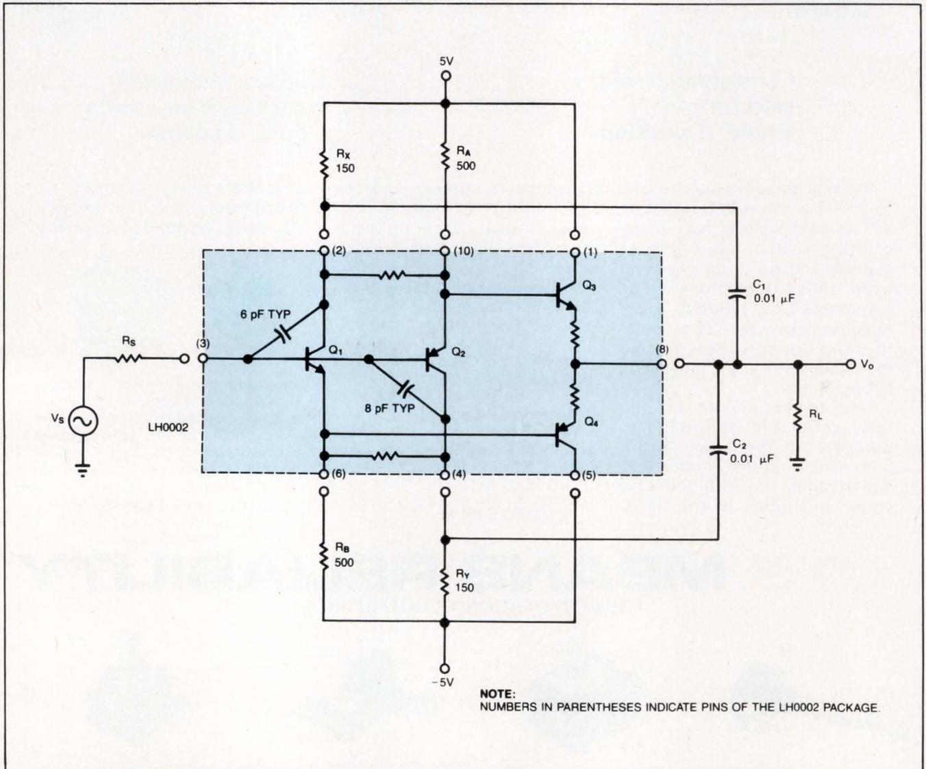
Fig 2—You can add components to extend the bandwidth of an LH0002 amplifier. This circuit increases the input-stage bias currents and bootstraps the amplifier's input capacitance.
