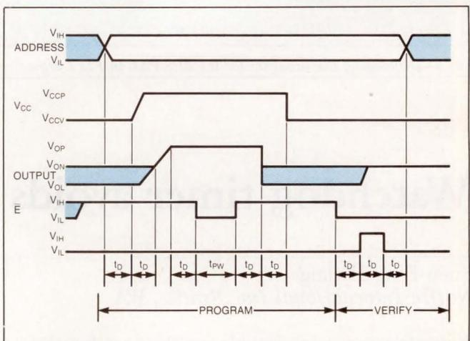
Fig 2—The state machine in Fig 1 generated these waveforms.
