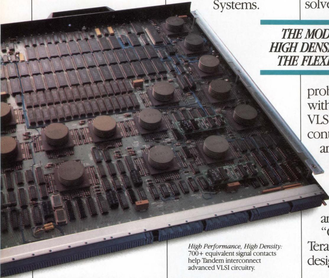
*High Performance, High Density:* 700+ equivalent signal contacts help Tandem interconnect advanced VLSI circuitry.
