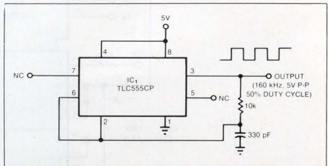
Fig 1—Based on a CMOS version of a 555 timer, this astable multivibrator's output symmetry depends on the tolerance of the internal switching thresholds.
