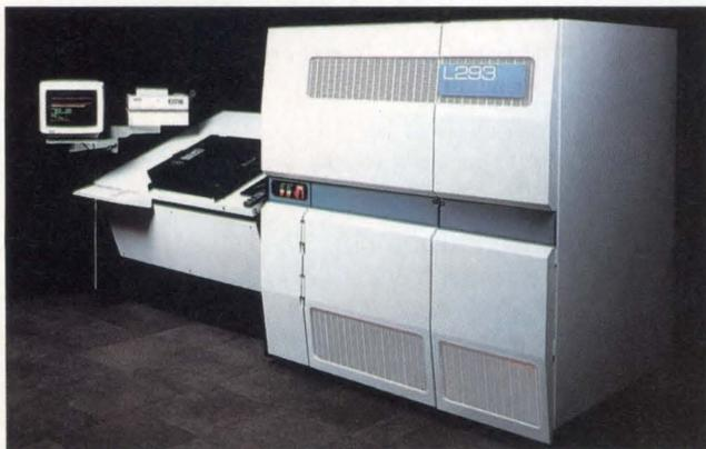
The L293 VLSI Module Test System.
