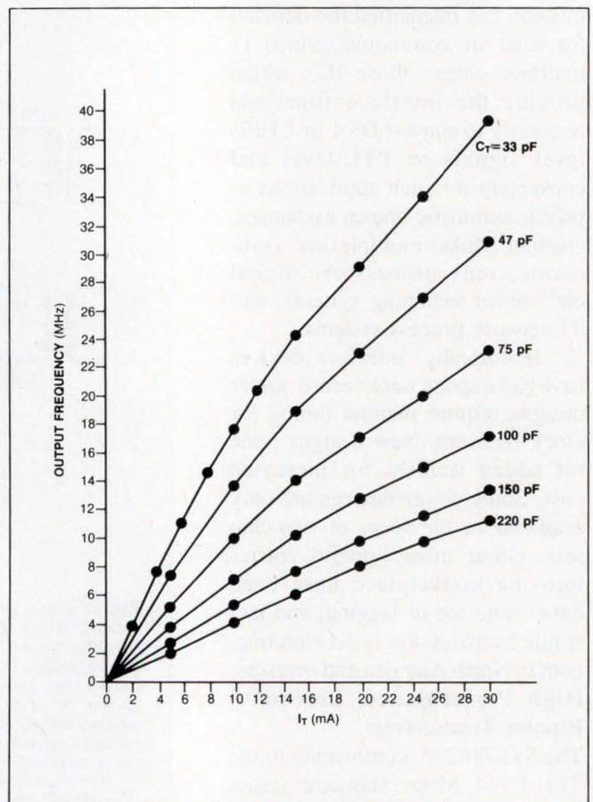
**Fig 2**—This graph illustrates how different values of **Fig 1**'s timing capacitor  $C_T$  provide different output frequencies for a given value of input current.
