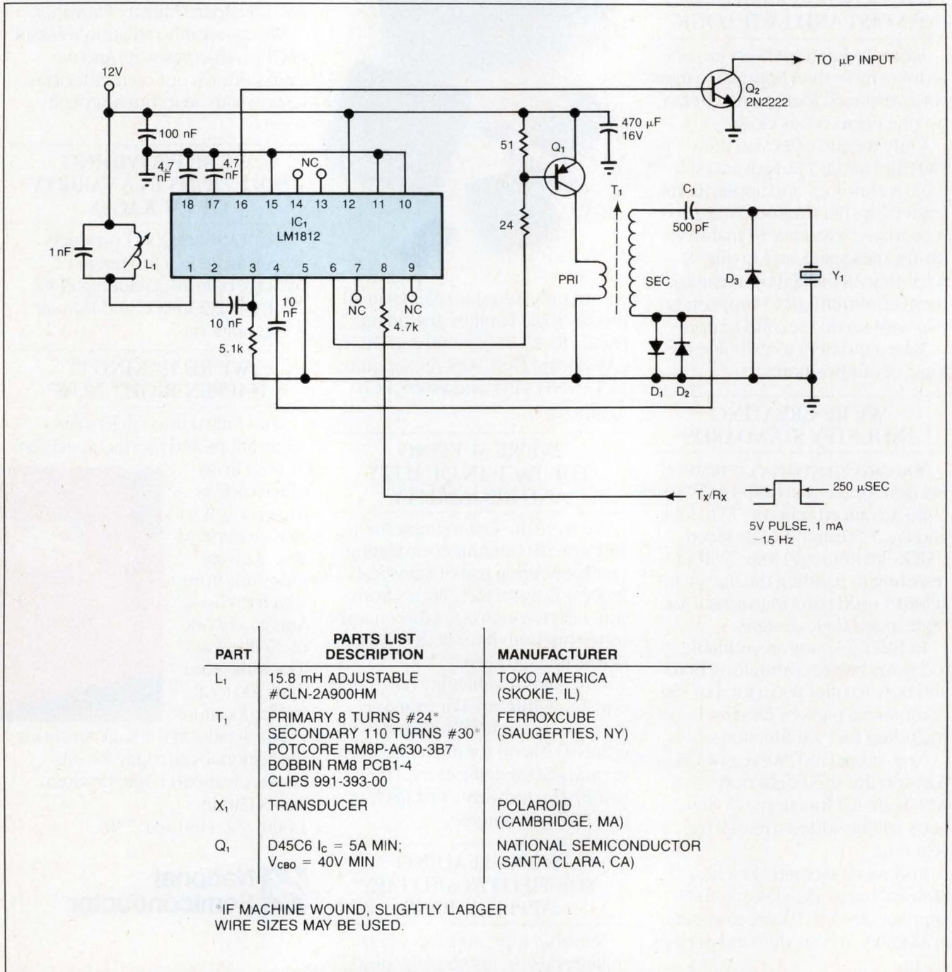
Fig 3—This ultrasonic ranging system features an ultrasonic transceiver ( $IC_1$ ) and an electrostatic transducer ( $Y_1$ ). Its sensing range is 4 in. to more than 30 ft.
