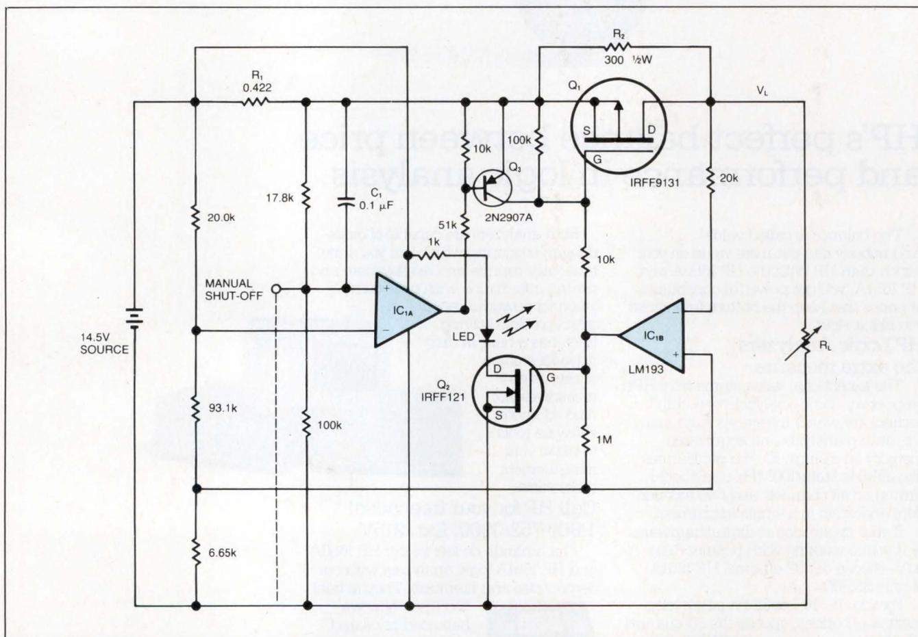
**Fig 1**—Load currents higher than 0.5A trip this electronic circuit breaker. The circuit resets automatically when the overload is removed.
