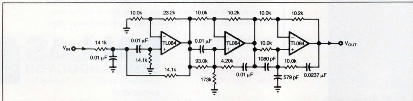
Fig 2—You can achieve a 39-dB stopband and 1.25-dB ripple using this bandpass filter. Scale the capacitor values to change its center frequency.
