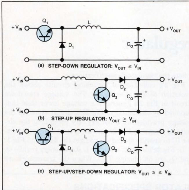
**Fig 2**—These three switching circuits show the evolution of Fig 1's circuit. The voltage step-down circuit in a generates a voltage lower than that supplied by the battery. The circuit in b steps up the voltage provided by a battery. By combining these circuits as shown in c and using a switching-regulator IC to provide the switching function and  $Q_2$ , you derive the design in Fig 1.
