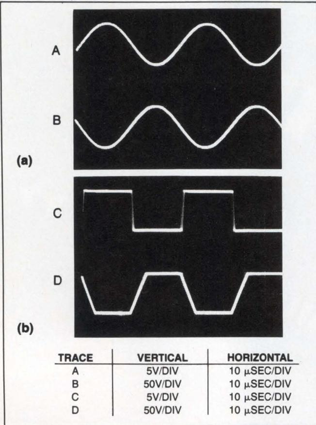
**Fig 2**—The **Fig 1** circuit produces 100V p-p sine- and square-wave outputs—**a** and **b**, respectively. Slew response to the square wave is a product of the OP-27 slew rate (2.8V/ $\mu$ sec typ) and gain of the booster stage (approximately 5.5).
