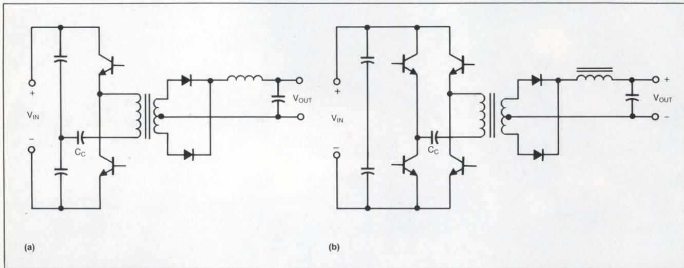
Fig 1—Most high-power switching supplies use either a half- or a full-bridge configuration. The half-bridge circuit (a) is the most popular for transistor currents to about 20A. At higher currents, designers usually switch to the full-bridge circuit (b), which nearly doubles the power output. Bridge circuits can use transistors that have about half the breakdown-voltage rating required for flyback or push-pull circuits.
