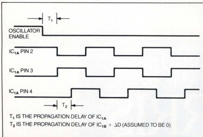
Fig 2—The Fig 1 oscillator always starts in the same state. Either IC<sub>1B</sub>'s internal propagation delay by itself or the delay and an optional feedback loop determine the frequency of oscillation.
