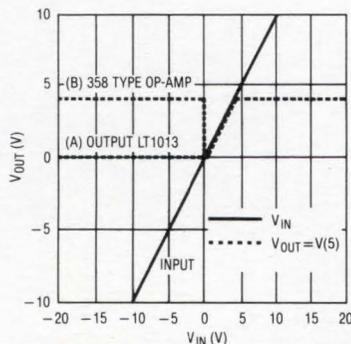
Figure 2. LT1013 Test Circuit: Single-Supply (+5V), Overdriven Follower
