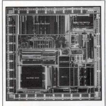
VAX MIPS performance. It has an 88100 RISC  $\mu P$  and an 88200 Cache/Memory Management Unit (CMMU). The  $\mu P$  employs fine-grain parallelism, using four pipelines that execute concurrently. Most of the 51 instructions operate in one machine cycle. It integrates an integer and two floating-point units to deliver 7M to 12M flops. It has a 32-bit combinatorial multiplier and separate 32-bit data and data-
