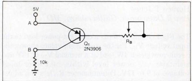
**Fig 2**—In this test configuration,  $R_{AB}=0.061R_B\pm 2\%$  as  $R_B$  varies from 34 to 825 k $\Omega$ .
