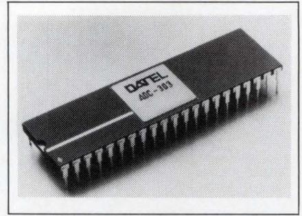
8-bit parallel outputs are buffered and have open-emitter arrangements. The chip dissipates 1.2W and has an integral and differential linearity of  $\pm$ 1/2 LSB over its operating range. You can select one of the following output codes: binary, complementary binary, 2's complement, and complementary 2's complement. The chip operates with an external clock and reference source, and comes in a 42-pin DIP. Its operating temperature ranges from -20 to +100°C. \$550.
