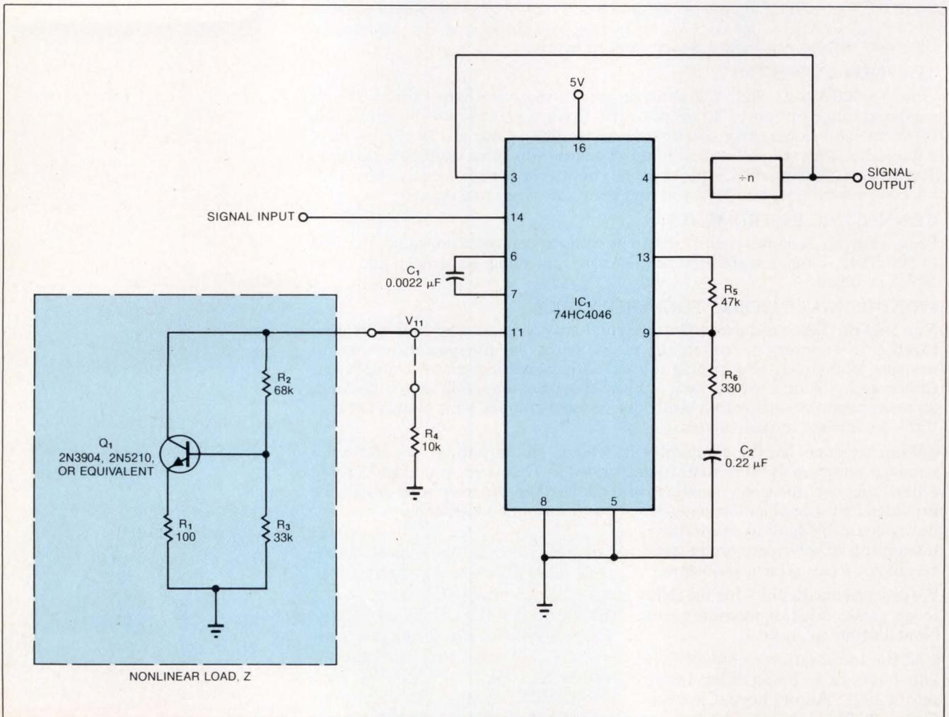
**Fig 1**—By connecting the nonlinear load  $Z$  to pin 11 of the PLL chip  $IC_1$ , you can extend the PLL's frequency range by a factor of 50, as compared with that possible by using a fixed resistor ( $R_4$ ).
