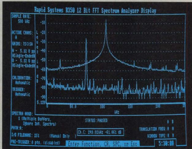
The R350 is a PC-based 12-bit, 2-channel, 500 KHz, real-time, FFT spectrum analyzer. Sample 2 channels simultaneously. 32K data buffers. Autosave spectrums to hard or floppy disk. Two modes of spectrum averaging. Fully differential inputs. Linear or log amplitude scaling. Amplitude and frequency cursor. Display spectrums 5 to 10 times a second. Print, store, retrieve and overlay spectrums. 500 KHz anti-aliasing filters on each channel, 80db of dynamic range.
