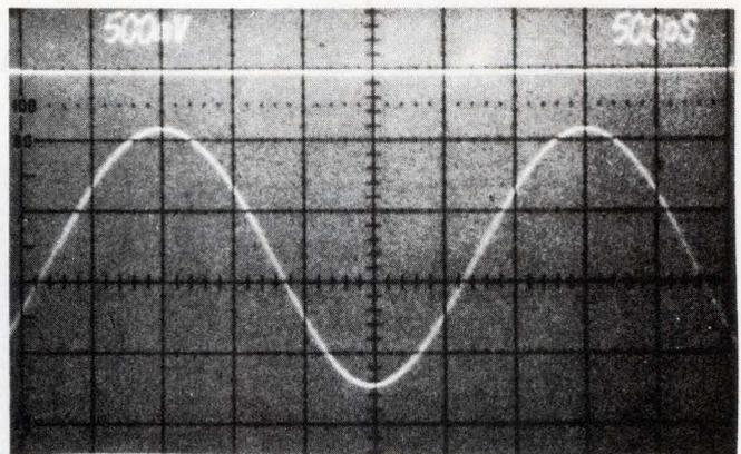
Fig 3—The Fig 1 free-running oscillator furnishes a clean output that varies between -0.5 and -2.25V. Here, the vertical scale is 500 mV/div; the horizontal scale, 500 psec/div. The horizontal line at the top of the display represents the zero level.
