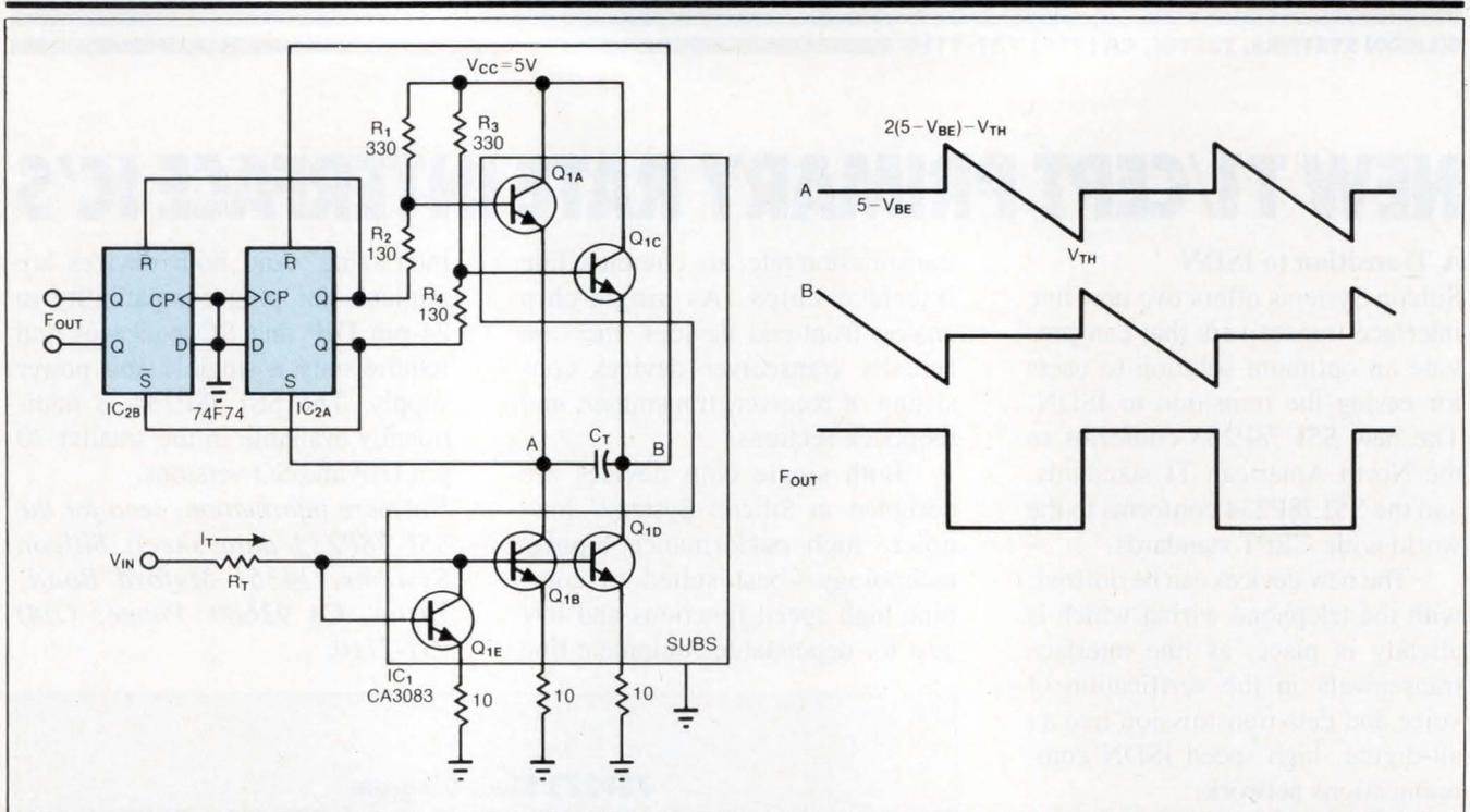
**Fig 1**—Two ICs form a voltage-controlled oscillator that generates TTL-compatible, complementary outputs with maximum frequency above 40 MHz.
