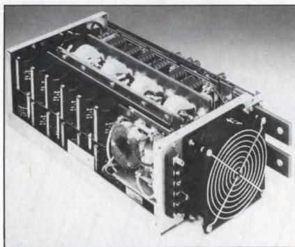
0.1% (whichever is greater) line regulation, and 10 mV or 0.2% (whichever is greater) load regulation; dynamic response of 4% max for a 25%-step load change; 200- $\mu\text{sec}$  output recovery to within 1% of nomi-
