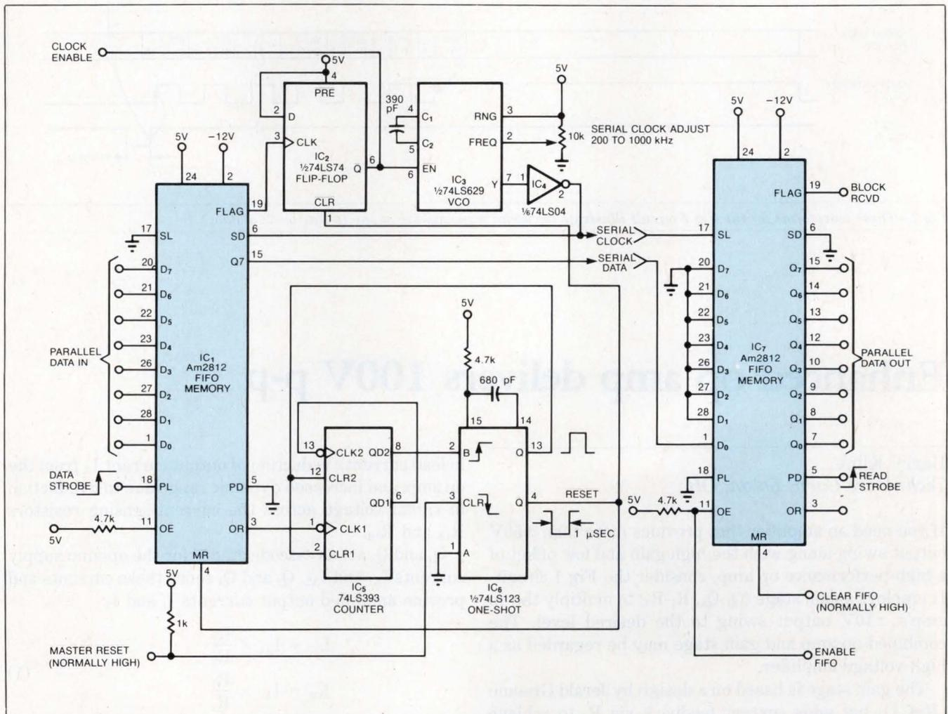
**Fig 1**—IC<sub>1</sub> provides a 16-byte buffer memory for parallel-input data and formats the data for serial transmission to IC<sub>7</sub>. IC<sub>7</sub> then reorganizes the data in byte-parallel format.
