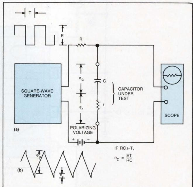
**Fig 1**—You can quickly determine a capacitor's series resistance by using the circuit in a. By looking at the relative magnitudes of  $e_r$  and  $e_c$  (b), you can decide whether the capacitor's resistance lies within acceptable limits.
