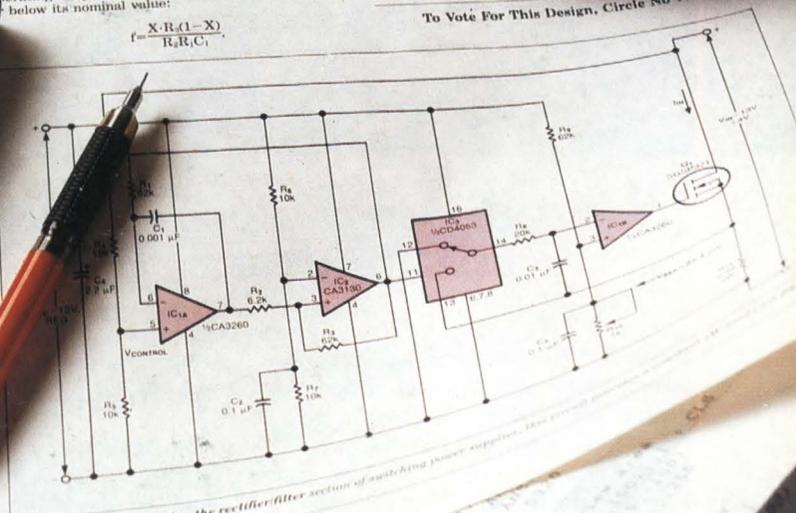
Fig 1—Developed for testing the rectifier/filter section of switching power supplies.
