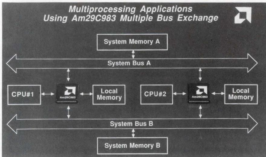
ance state. All the I/O lines go to a high-impedance state upon power-down. The device is available in a 68-pin PLCC or LCC, and it exhibits typical port-to-port delays of 9 nsec. The ports for each of these devices are TTL compatible and can sink 48 mA of output drive current.
