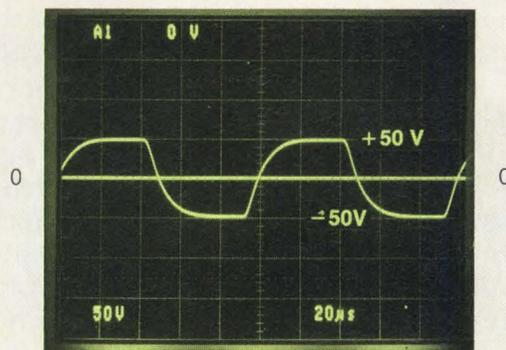
Reproduction of a 10KHz square wave by a Kepeco bipolar Power Manager Model BOP 50-2M, which actually has a 20KHz bandwidth in the voltage mode.
