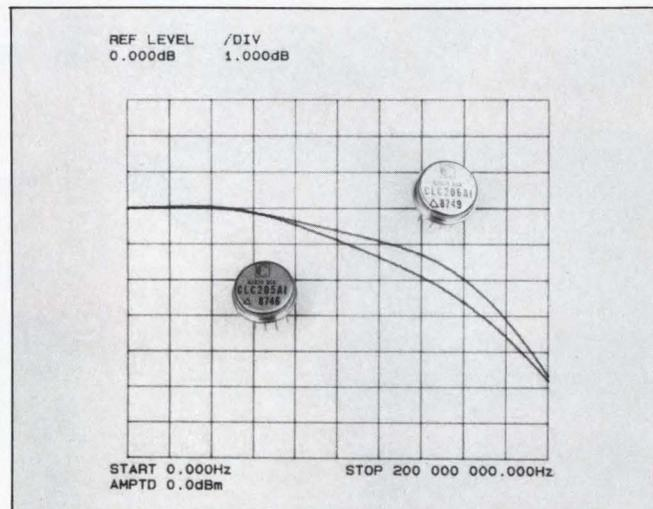
200-MHz, overdrive-protected op amps (Comlinear Corp)
