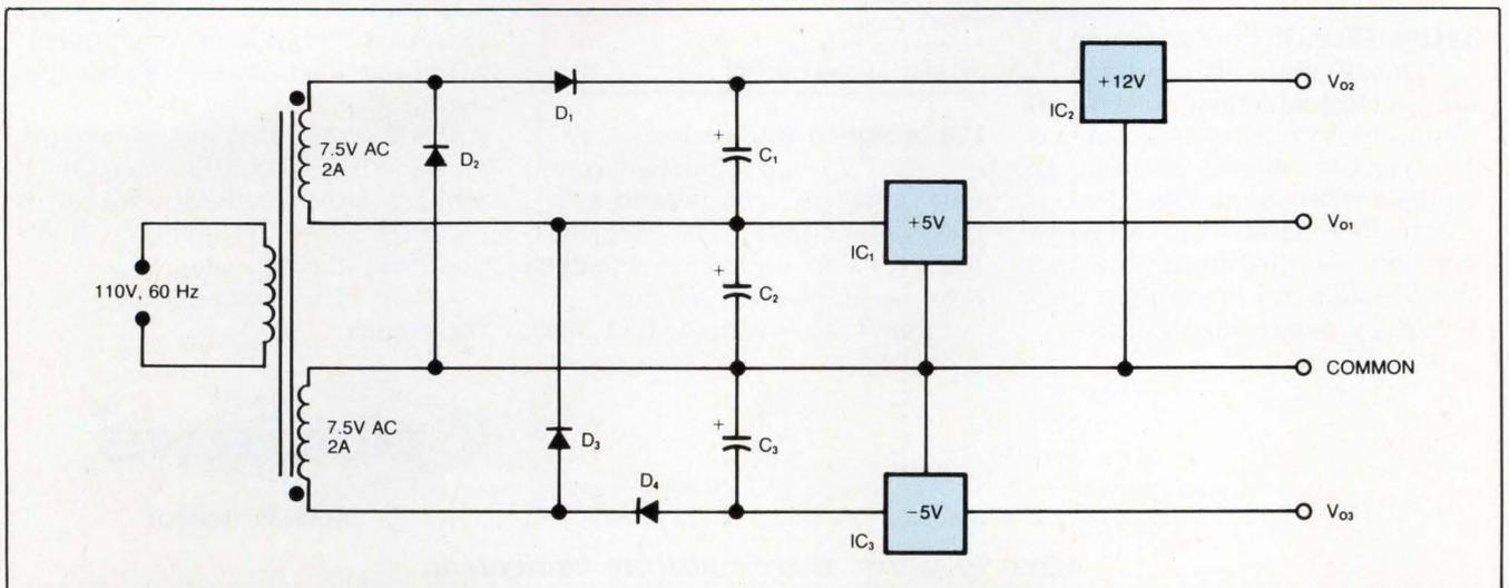
Fig 1—This simple power supply generates three regulated voltages using a minimum of components.
