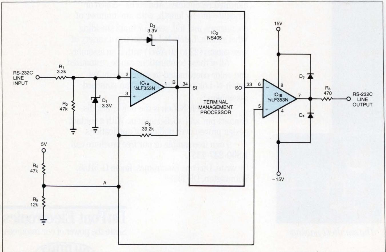
Fig 1—A dual op amp provides a single-channel interface between an RS-232C line and a MOS terminal-management IC.
