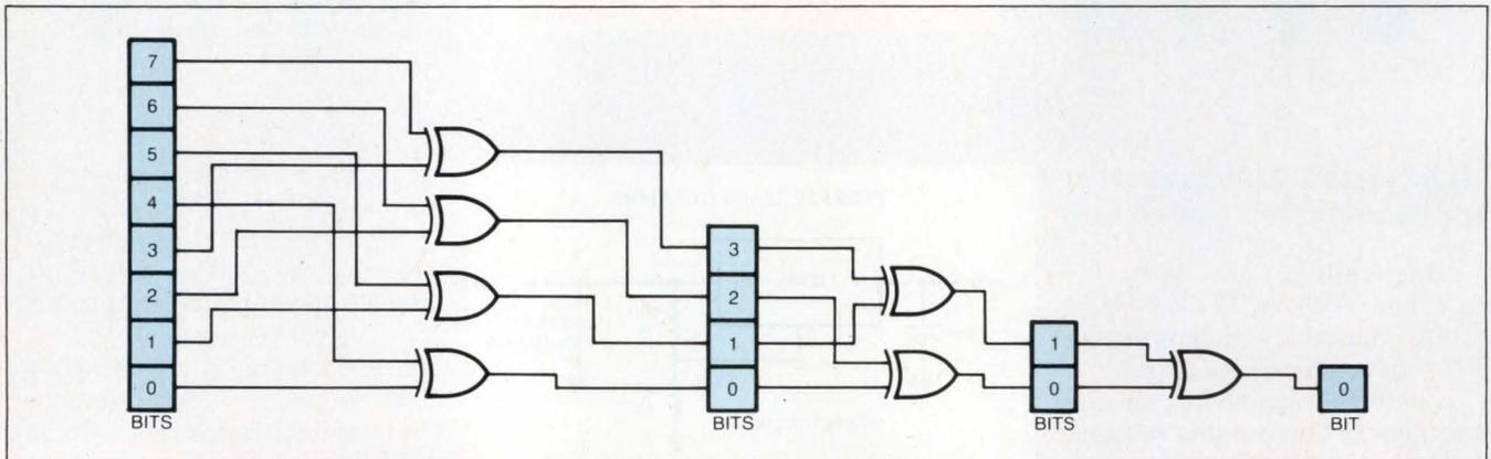
Fig 1—You can quickly test 8-bit character codes for parity by emulating this hardware in a software routine.
