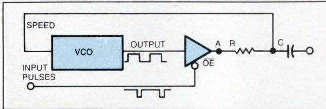
Fig 1—Using a 3-state buffer as a PLL's phase detector, you can keep the PLL synchronized with a pulse train—even when pulses are missing.
