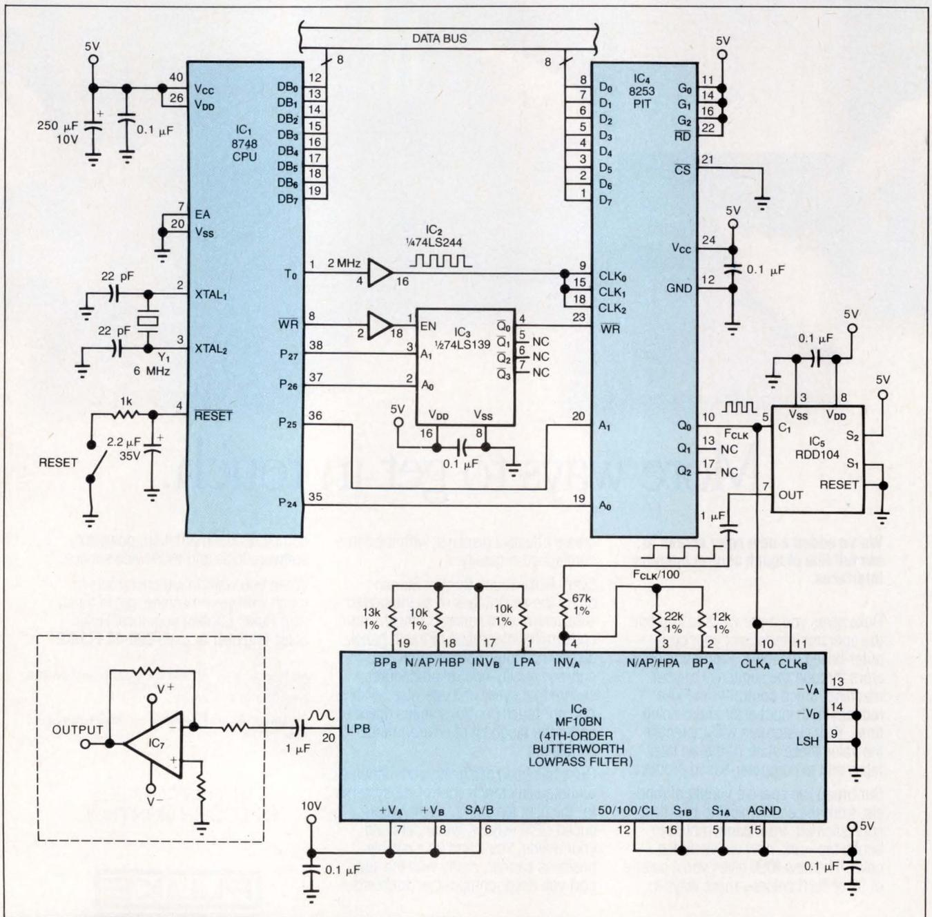
**Fig 1**—This microcomputer-controlled system produces a constant-amplitude, programmable-frequency audio output. Frequency range spans five decades to 20 kHz.
