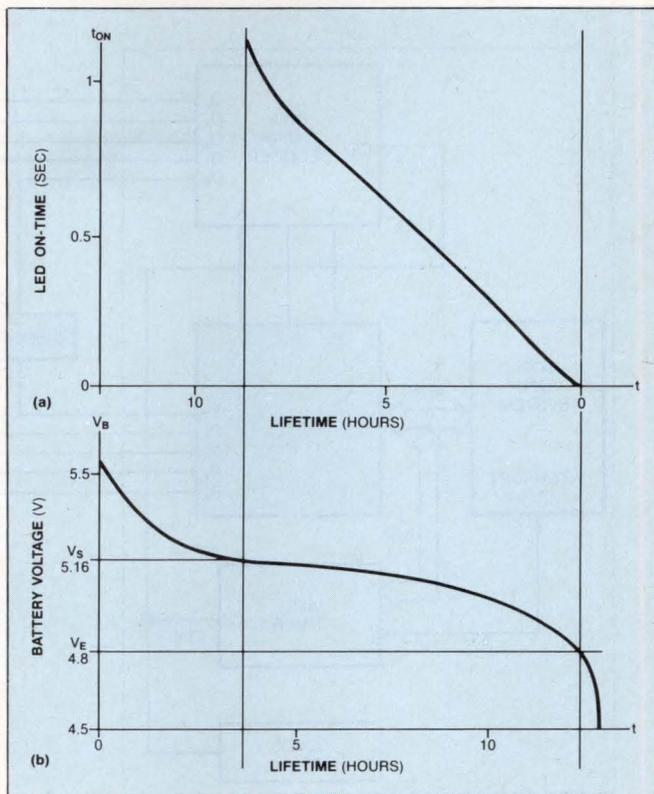
**Fig 2**—The calculated on-time in seconds for the LED in Fig 1 corresponds to the battery's remaining life in hours, based on a 100Ω load (a). The curve in b shows the measured rate of discharge for a NiCd battery (four Varta RS600 cells loaded with 100Ω).
