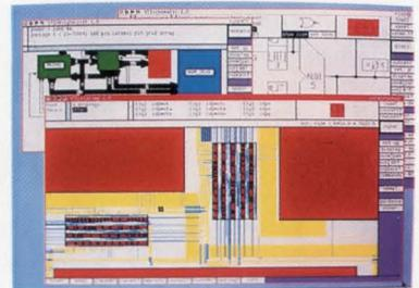
This design integrates all the peripheral chips for an AT computer with six megacells and control logic. Using the Silicon Express Design System, logic and physical designs like these can be implemented in under two man months.
