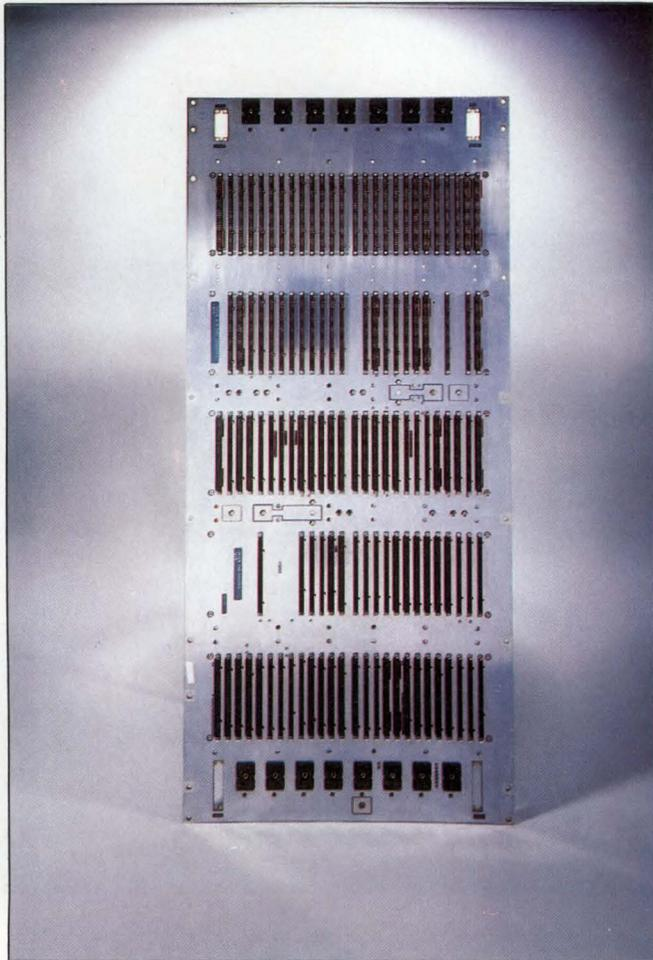
*MIL-spec backplane measuring 42x22 in. (Methode Electronics)*
