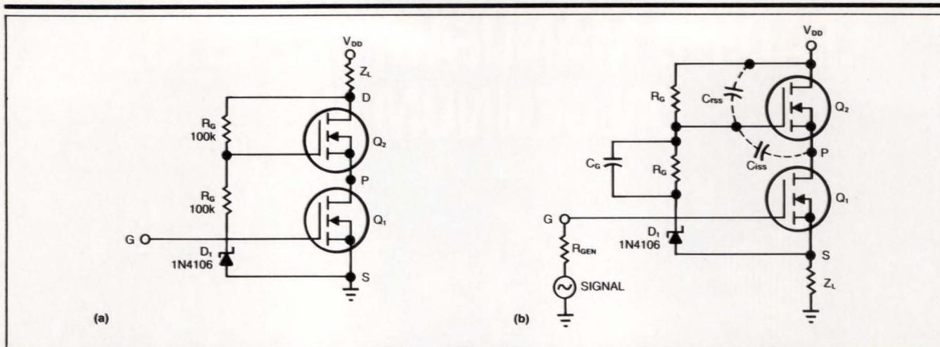
Fig 2—You can use the composite MOSFET in conventional high- $V_{DD}$  applications such as common-source (a) and source-follower (b) connections.
