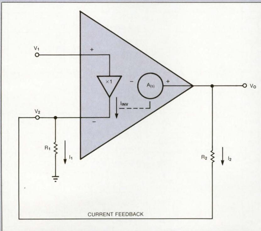
current-feedback op amp—unlike the conventional op amp—the position of the poles (contained within  $D(s)$ ), and hence the bandwidth of the current-feedback op amp, is not dependent on the closed-loop gain. Provided that you keep  $R_2$  constant, you can change the closed-loop gain of a current-feedback op amp—without
