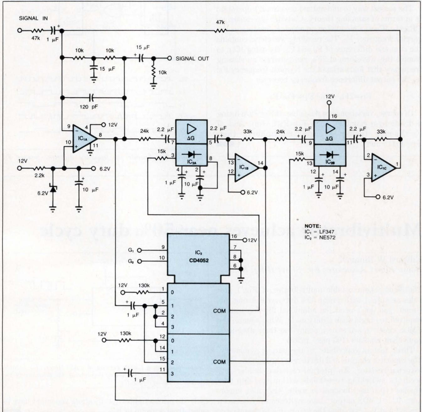
Fig 1—With this circuit, you can select gain-compression ratios of 1:1, 2:1, 3:1, and 4:1 without changing the unity-gain point. By changing inputs  $G_0$  and  $G_1$  of the analog multiplexer, you control the detector current in each half of the NE572 ( $IC_2$ ), and, therefore, the gain of each section.
