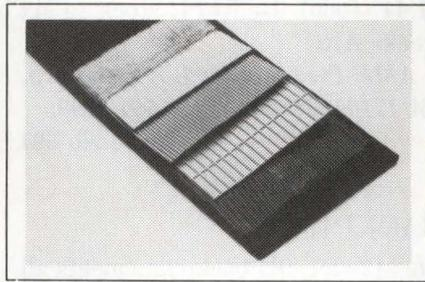
FCC regulations for EMI/ESD protection; it features a full 360° wrap of extended copper shield. Dielectric PVC material, located above and below the cable inside the shield, maintains precise shield-cable spacing, thus providing the high-impedance and low-capacitance values.
