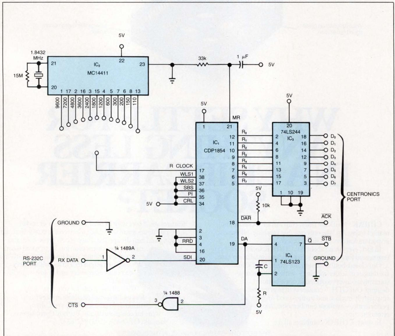
**Fig 1—The CDP-1854 UART assembles serial RS-232C data into bytes for a Centronics port. IC<sub>2</sub> provides a baud rate that matches the RS-232C transmission rate, and IC<sub>3</sub> buffers the data byte to the Centronics port. Signals DA and DAR control the timing of the two ports.**
