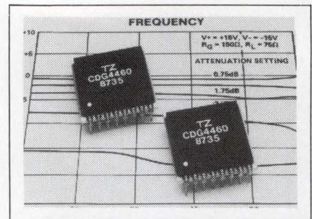
output resistance over the entire resistance range. An onboard data latch lets you set predetermined attenuation settings. It operates with power supplies ranging from  $\pm 6$  to  $\pm 15$ V and dissipates 0.5  $\mu$ W typ. The 16-pin hybrid package occupies 1 sq in. of board space. \$39.50.
