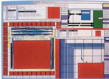
This highly-integrated design combines control logic, a register file, a refresh counter, and five peripheral chips onto a die size of 275x315 mils. The logic design, layout, and verification were completed in only 12 weeks.
