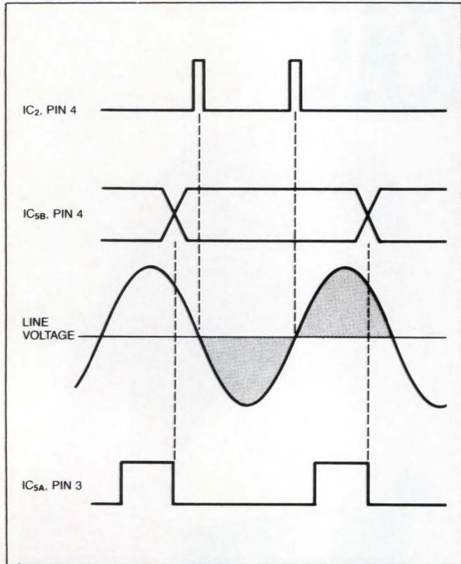
Fig 2—This circuit is timed to fire the SCRs Q<sub>2</sub> and Q<sub>4</sub> (Fig 1) so that only one full line cycle (highlighted area) is passed to the load for each pulse from IC<sub>5B</sub>, pin 4.
