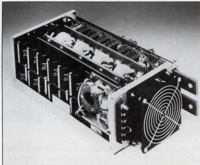
*Fan-cooled 3-kW supply in a 5x8x15-in. package (Powertec Inc)*
