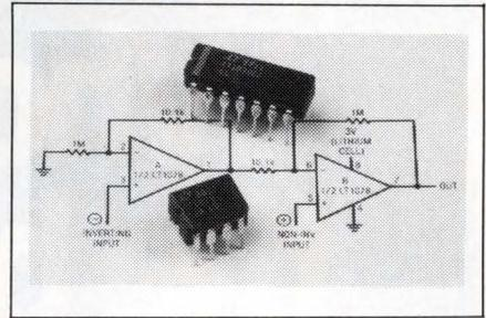
250-pA-max offset current, 0.4  $\mu$ V/ $^{\circ}$ C offset voltage drift, a 200-kHz gain-bandwidth product, and a 0.07V/ $\mu$ sec slew rate. The 1/f corner of the voltage noise spectrum is 0.7 Hz. This low frequency corner permits a voltage noise specification of 0.6  $\mu$ V<sub>p-p</sub> and a current noise specification of 3 pA<sub>p-p</sub> over the 0.1-Hz to 10-Hz frequency range. The outputs can source and sink 5 mA of load current. LT1078, \$2.80; LT1079, \$3.50 (100).
