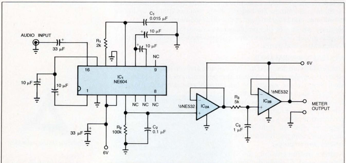
Fig 1—You can measure audio signal levels to  $\pm 1.5\text{-dB}$  accuracy using a dual op amp and an FM IF chip (normally used for cellular-radio and other RF applications). Sensitivity is  $10.5 \mu\text{V}$ ; power consumption is 30 mW.
