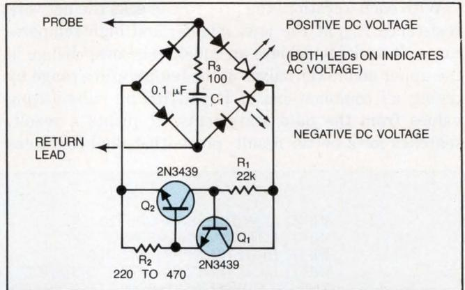
**Fig 1**—This simple test probe indicates ac or dc voltage over a 4 to 220V range. The current source ( $R_1$ ,  $R_2$ ,  $Q_1$ , and  $Q_2$ ) ensures a constant current in the LEDs for any acceptable test voltage.
