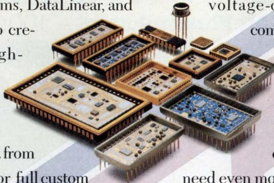
36 monolithic and hybrid devices ranging from 8 to 18 bits, including quads,  $\mu$ p-compatible, voltage-output, and current-output components.
