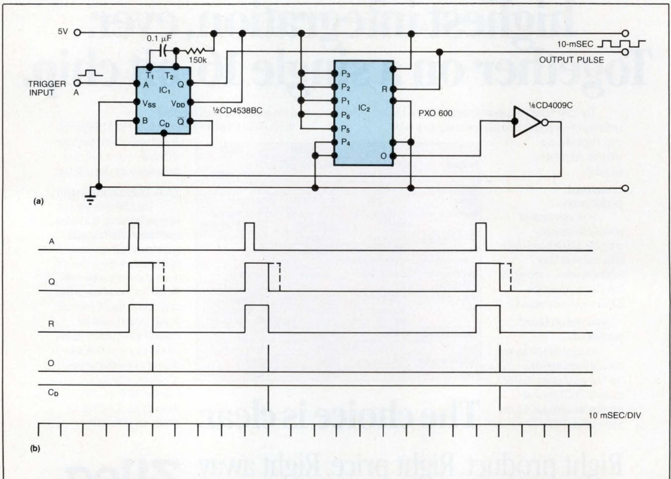
**Fig 1**—This circuit (a) lets you set precise pulse widths (b) that are independent of component aging, power-supply variations, and temperature. The monostable multivibrator ( $IC_1$ ) is configured in the nonretriggerable mode, and the RC time constant is greater than the desired pulse width.
