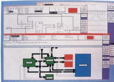
The Concept Express Design System's highly productive logic tools and silicon compilers were used to develop this very-large-scale ASIC. It incorporates a 2901 datapath, RAM, ROM, and over 3,400 gates of random logic.
