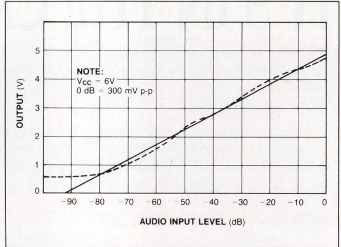
Fig 2—The dotted line indicates the response of Fig 1's circuit for the 100-Hz to 10-kHz audio range; the solid line indicates an ideal response. Full scale (0 dB) equals 300 mV p-p.
