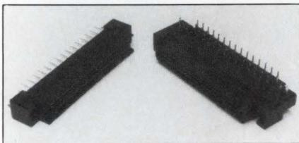
on pc boards. You can order 30-, 40-, 50-, or 60-pin versions of either style with as many as 200 contact positions. On pc-mounted connectors, alternate pairs of tails are staggered by 0.075 in. The insulators have clips to keep the connectors on the boards before soldering.
