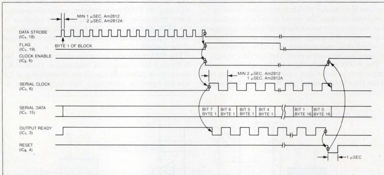
Fig 2—These waveforms for the Fig 1 circuit illustrate the serial transmission of one 16-byte block of data.
