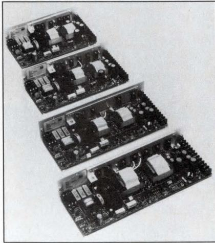
features of the switchers are built-in line filtering, 3750V ac safety isolation, shielded power transformers,
