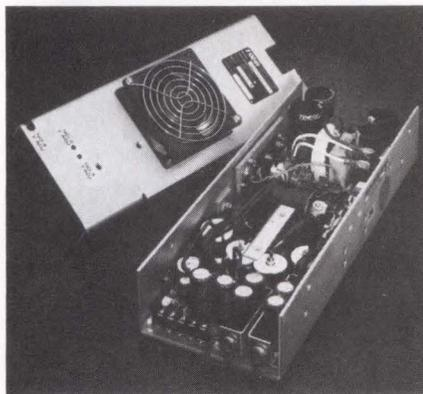
80% min, the vendor claims. The unit specs 0.2% rms max ripple and noise.
