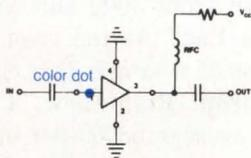
Unbelievable, until now... tiny monolithic wide-band amplifiers for as low as 99 cents. These rugged 0.085 in. diam., plastic-packaged units are 50ohm\* input/output impedance, unconditionally stable regardless of load\*, and easily cascadable. Models in the MAR-series offer up to 33 dB gain, 0 to +11dBm output, noise figure as low as 2.8dB, and up to DC-2000MHz bandwidth.
