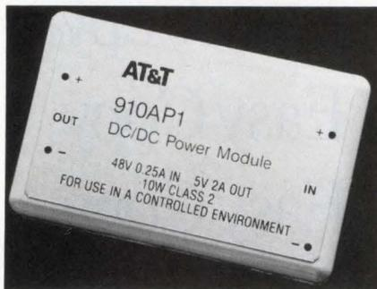
circuits located inside the module maintain the module's output ripple (from dc to 20 MHz) at 100 mV p-p max. The product needs no external components to attain this performance. The input and output sections of the 910AP1 are completely
