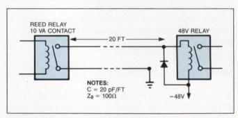
Fig 2—In Problem 2, a reed relay drives a power relay through 20 ft of cable. Are transmission-line effects significant?
