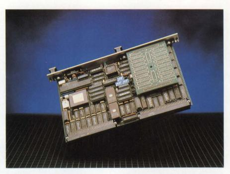
The TCP/IP protocol that executes on the CMC ENP-100 68020-based Ethernet board results in VME Bus application-to-application data rates in excess of 3M bps.
