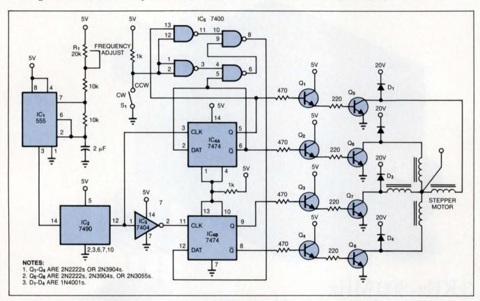
Fig 1—This stepper-motor controller lets you adjust motor speed using  $R_1$  and motor direction using  $S_1$ .
