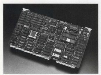
Supporting both link-layer and front-end modes of handling the TCP/IP protocol allows the Exos 301 Multibus I board from Excelan to work with varied third-party protocol software.
