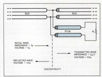
Fig 8—Without the use of matching transformers, stubs often present intractable reflection problems. The best advice is to keep stubs short.
