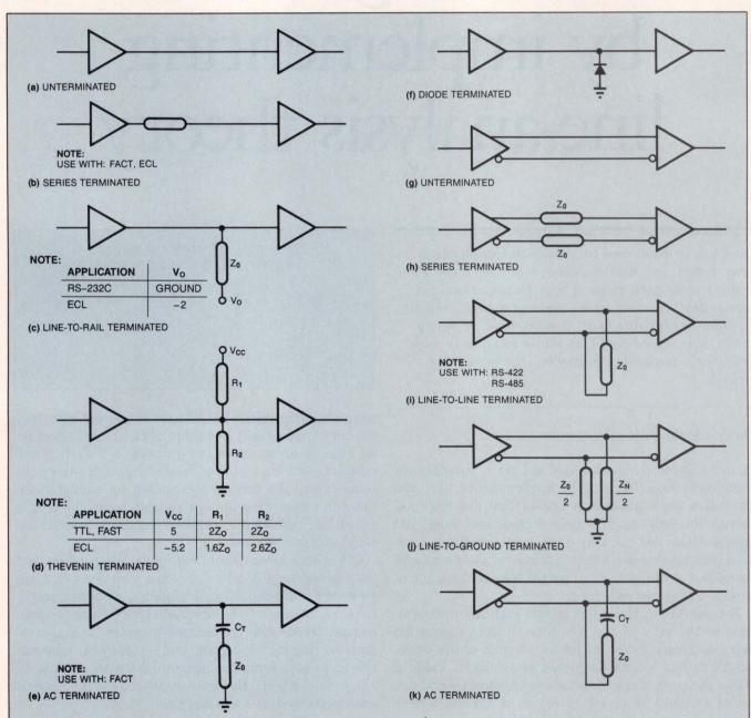
Fig 7—You can choose from numerous techniques for terminating single-ended and balanced transmission lines. Diode termination, shown in (f), usually doesn't require discrete diodes for digital logic. The diodes are within the gates that act as receivers.
