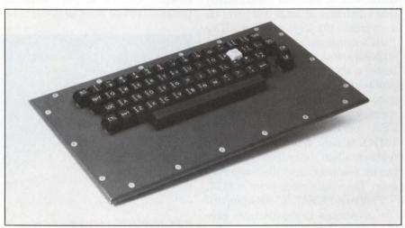
**Designed for military applications,** the Model 30498-05 keyboard from IEE meets MIL-STD-810C as well as EMI/RFI and Tempest specifications. Its keyswitches use conductive-rubber technology and are rated for a minimum of 20 million actuations.
