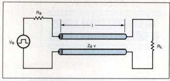
Fig 4—A classic transmission line receives a signal from a voltage source,  $V_S$ , by way of source impedance,  $R_S$ . The line delivers the signal to a load, represented here as  $R_L$ .
