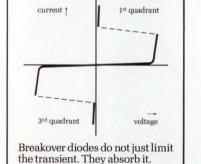
Dual Symmetrical; in a range from 100 to 280 volts. All designed for use as superior alternatives to any transient surge protectors you currently use.
