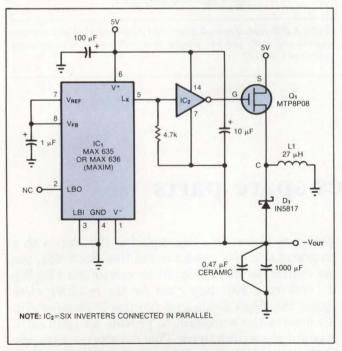
Fig 1—This negative regulator supplies -5V when using a MAX635 or -12V when using a MAX636.
