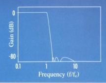
The SR640 offers a unique combination of filter specifications, preamplifier performance, and programmability at a price far less than other instruments. Featuring two fully independent 8-pole, 6-zero elliptic filters with less than 0.1 dB p-p passband ripple and 115 dB/octave rolloff, the SR640 is the ideal filter for general purpose signal processing as well as anti-aliasing for digital signal processing systems.
