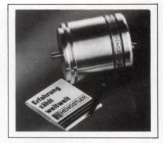
resolution is provided by a resolution of 12-bits per revolution for 4096 revolutions. The encoder is sealed to IP65 requirements and has an operating temperature range of -10 to +80°C. Its serial output can drive as much as 50m of coaxial cable. Interface circuitry, supplied with the encoder on a Eurocard sized pc board, processes the encoder output to produce either a binary or Graycode, TTL-level, parallel output. A version with open-collector outputs is also available. The
