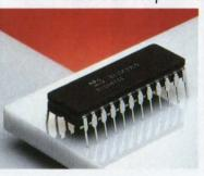
By using super-shallow junction transistors, trench isolation technology and Schottky diode clamp-type memory cells. Both ECL 10K (µPB10474A) and 100K (µPB100474A) interface devices are available.
