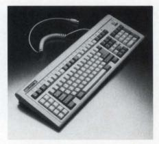
With its onboard, nonvolatile memory, the Memory Pro from Maxi Switch can retain over 80 user-defined macros. All keys are programmable and redefinable.
