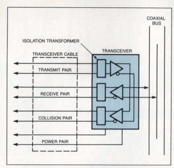
Fig 10—Ethernet is an example of a bus system that looks as if it could have problems with stubs. In fact, the active transceivers hold stub length effectively to zero.
