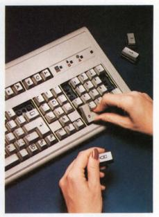
To maximize flexibility, the Modulkey EKT 109 keyboard from Advanced Input Devices allows you to use snap-in key modules to reconfigure the layout from 109 keys to 115.
