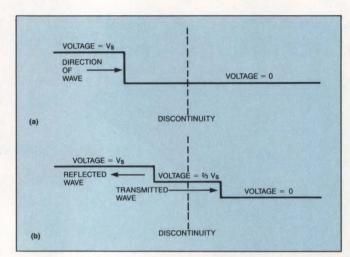
Fig 9—You may find it difficult to accept the notion, but you can't change the voltage along a transmission line instantaneously. If you apply a step at one end, it travels down the line and leaves a voltage change in its wake (a). When a wave encounters a discontinuity, wavefronts continue down the bus and the stub, and a reflection travels back toward the source (b).
