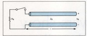
Fig 12—When the reed relay of Problem 2 closes, it shorts out the charged transmission line. The results are not the same as you would observe if you shorted out an equivalent lumped capacitor.
