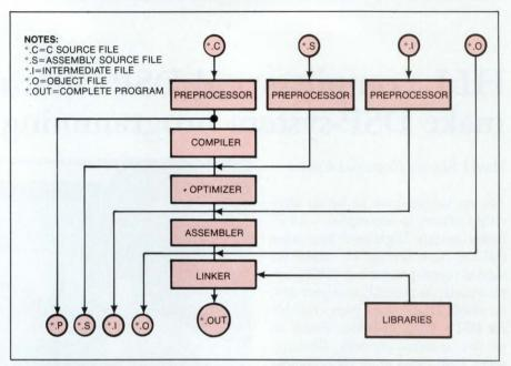
Optimizing compilers attempt to reduce the speed penalty inherent in high-level languages. The AT&T C compiler, for example, preprocesses the C source code, compiles it, optimizes it, and then assembles and links it.
