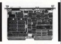
TVME 1612 (MVME 110-1 Compatible) System Control at 8 or 10 MHz
