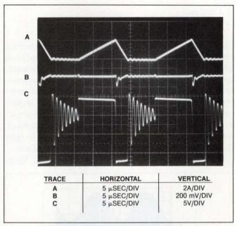
Fig 2—These Fig 1 waveforms show inductor current (trace A), output voltage (trace B), and flyback voltage across the inductor (trace C).
