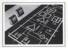
device provides a precision 5V reference output, useful for applications involving the excitation of a bridge or sensor. By means of pin connections, the 5V reference provides a half-scale offset for use with bipolar input voltages. The converter also features a maximum linearity error of ±0.02% FSR (full-scale resolution) at 100 kHz and a maximum gain-drift of ±40 ppm of FSR/°C. 20-pin PLCC, \$8.60 (100).
