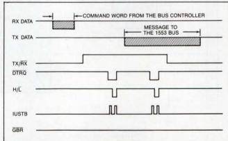
Fig 4—This diagram shows the timing requirements for the datahandshaking signals needed to transmit two data words over the 1553 bus. The 1553 controller doesn't set the GBR line during this operation.
