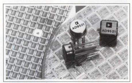
90 mW typ. It comes in two gaintolerance grades and in commercialand military-temperature range versions. The vendor offers the device in an 8-pin metal can and in a 20-pin LCC. Commercial-temperature range versions, from \$16; military-temperature range versions, from \$32 (100).
