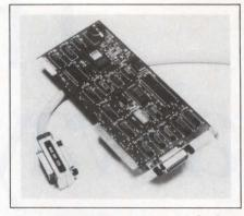
mnemonics and can drive 14 devices via a standard cable. Using DMA, it can transfer data to the computer at 300k bytes/sec; it also operates in programmed-I/O mode. The software resides in RAM on the board, and hence does not occupy any of the computer's memory. Support software enables you to write instrument-control programs in Basic, C, and Pascal. \$495.
