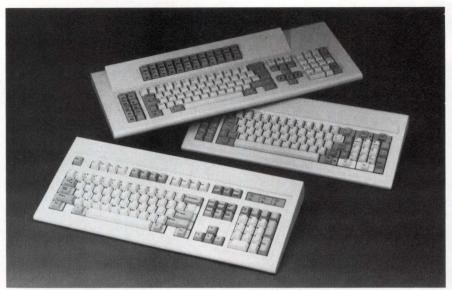
To make it easier to use software programs, the RT-101 keyboards from Hi-Tek feature an ergonomically placed cursor-control pad and dedicated screen-control keys.
