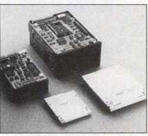
Removable, erasable, magneto-optic cartridges for the 5¼-in. Tahiti I and 3½-in. Fiji I optical-disk drives store 1G and 160M bytes, respectively.
