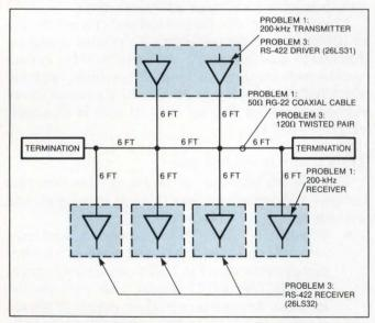
Fig 1—This multidrop data bus configuration is common in data communication and appears in two of the problems presented in this series. In Problem 1, the bus interconnects modems; in Problem 3, it joins drivers and receivers that conform to EIA standards.
