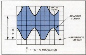
Fig 2—A different approach from Fig 1, this method allows a cursor scope to calculate percent modulation once you've measured the quantities C and D.
