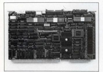
The Ethernet and WAN interfaces on the SBE MLAN-E Multibus I board can function as a bridge between LANs and WANs. Data passing over the bridge does not suffer from host-bus transfer delays.
