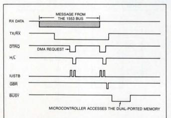
Fig 3—This diagram shows the timing requirements for storing two received data words in the dual-ported memory. The microcontroller places the remote-terminal hybrid in a busy state whenever the microcontroller accesses the dual-ported memory.
