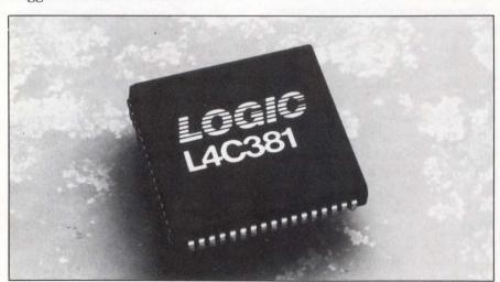
This 16-bit cascadable arithmetic logic unit has built-in latches for pipelining. It offers six arithmetic and logic functions and can be operated as an accumulator.
