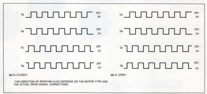
Fig 2—These transistor-collector waveforms of Fig 1 illustrate the drive signal you obtain with the CW/CCW switch closed (a) and open (b).
