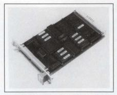
bytes/sec. The board performs many of the standard SCSI bus sequences without host CPU intervention. By allowing peripheral devices to disconnect from the SCSI bus after receiving commands, the board allows you to implement a degree of multitasking between various peripheral devices. Implemented largely with CMOS devices, the VSCSI board has a power consumption of 5W. Approximately DM 1000 (100).
