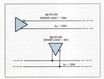
Fig 15—An RS-422 driver (a) can handle the load imposed by driving a line from one end, but it can't drive the lower impedance it sees when it has to drive a line from a tap in the middle. An RS-485 driver (b), can drive a line from a tap.
