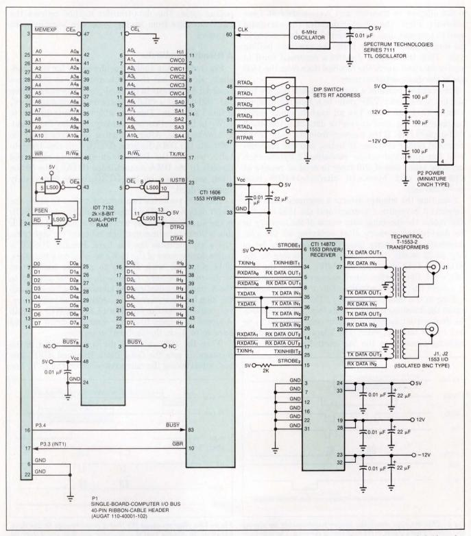
Fig 2—This schematic for the 1553 I/O board shows three major components: a 1553 controller, a driver and receiver hybrid, and a dual-ported memory.
