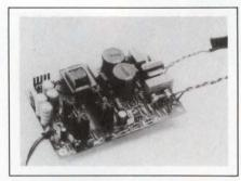
that complies with both FCC and VDE 0871 for level B equipment is also included in the supply. The supply features input voltage requirements from 85 to 132 or 170 to 264V ac. Standard features include overvoltage and overload protection on each output, and a 16-msec hold-up time. For full power output, the device operates over a temperature range from 0 to 50°C. \$25 (OEM qty).
