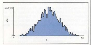
Fig 1—Listing 1 produced this near-Gaussian distribution using the mean values of 1864 batches of pseudorandom numbers. Each batch contained sixteen 16-bit samples.
