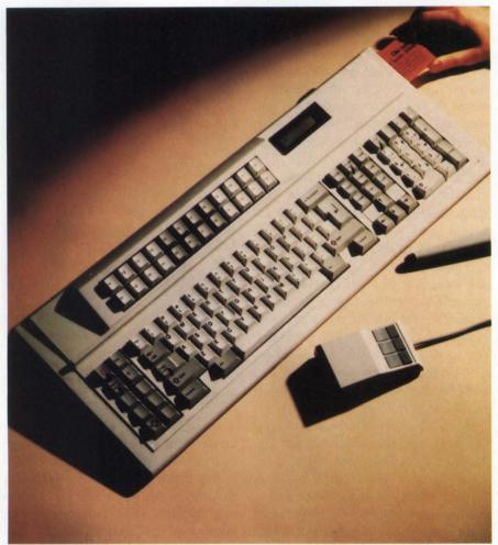
Offering a suite of options, such as a card reader, mouse, and remote bar code reader, Cherry's G80-2000 has a layout like the IBM 3270 terminal controller with 24 function keys along the top, in addition to the 10 at the left of the board.
