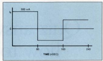
Fig 13—As a wave travels back and forth along an improperly terminated line, current polarity reverses. If there are any losses in the system, the oscillations eventually decay to zero. The losses determine the rate of decay.
