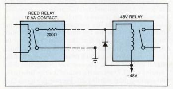
Fig 14—Adding a 200 $\Omega$  resistor to the circuit of Problem 2 limits the current through the reed-relay contacts to about 200 mA. You still have to select a reed relay that can handle the energy delivered by the charged transmission line.
