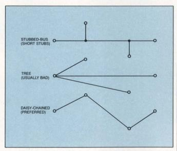
Fig 11—A daisy-chain bus can be difficult to install because you have to bring the bus, and not a stub, to each interconnected device. Electrically, though, the daisy-chain configuration presents the fewest complications.
