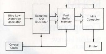
Frequency-Domain Testing of A/D Converters
