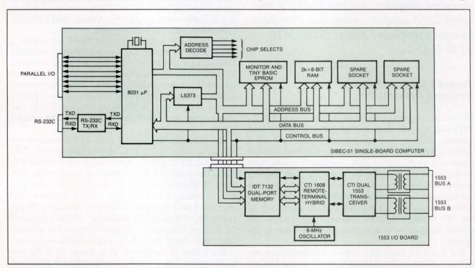
Fig 1—The universal 1553 adapter comprises a commercially available single-board computer (the Sibec-51) and a custom-designed 1553 I/O board.
