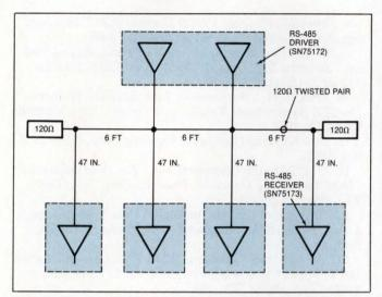
Fig 16—Reconfiguring the bus of Problem 3 by shortening the stubs from 6 ft to a little less than 4 ft, changing the drivers and receivers to RS-485-compatible ones, and selecting  $120\Omega$  terminators produces reliable operation.
