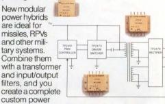
supply—in a fraction of the time, and at a fraction of the cost, it would take to start from scratch.
