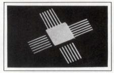
24-lead flat packs, include quad OR/NOR gates, quad AND/NAND gates, flip-flops, buffers, multiplexers, demultiplexers, shift registers, and counters. They feature ECL-compatible output levels and temperature compensation. The devices are fabricated in the company's ECL-3 process, a 1- $\mu$ m technology with a 10-GHz transition frequency and a 80-psec gate delay at 300  $\mu$ A. \$40 to \$150.
