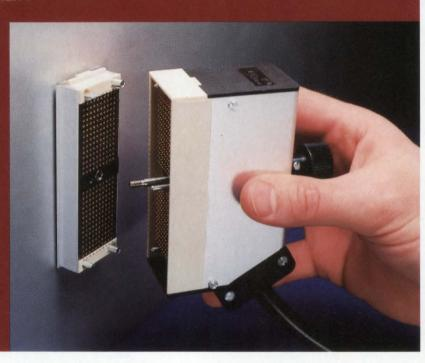
Only Hypertronics ends the compromise in multipin connectors—for heavy-duty power/signal applications—by replacing low wipe Zero Insertion Force (ZIF) contacts and expensive cams with lowforce, high-cycle reliability.
