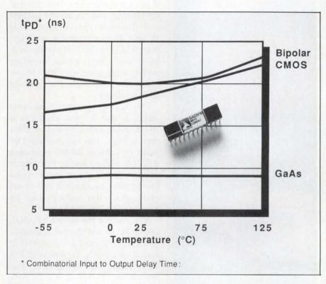
Wide temperature excursions have very little effect on the 10-nsec propagation delay of the laser-programmed GaAs GA22V10 PLD.
