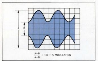
Fig 1—The traditional computation of percent modulation requires the measurement of quantities A and B, followed by subtraction, addition, division, and multiplication.
