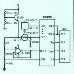
NOTE 1: YELLOW SPRINGS INSTRUMENT P/N 44201 NOTE 2: YELLOW SPRINGS INSTRUMENT P/N 44007
