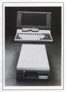
100+ laptop computer employs a 5¼-in. format, features a formatted capacity of 360k bytes, and offers 81-msec access time typ. The subsystem provides a convenient means of porting software between your laptop and desktop personal computers. Because it weighs 3.9 lbs
