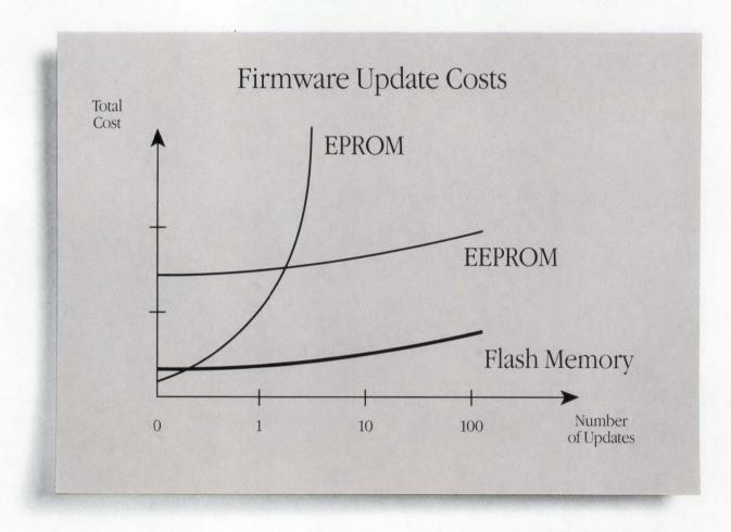
Until now, the only way designers could easily alter code in an embedded system was to upgrade from low-cost EPROM to expensive EEPROM.
