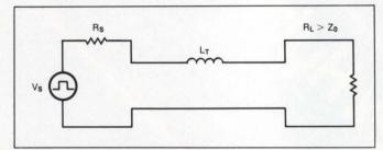
Fig 6—You can sometimes represent a transmission line as a single lumped element. Here the load resistance is lower than the line's characteristic impedance, and you can represent the line as an inductor.
