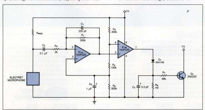
Fig 1—Speaking into this circuit's microphone drives the TX output low. The output remains low for about 0.7 sec following the last word spoken.
