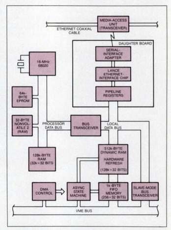
Because of concurrent operation of the  $\mu P$ , the Ethernet interface, and the DMA bus interface on the Interphase 4207 Eagle, VME Bus burst-data transfers faster than 35M bytes/sec are possible.
