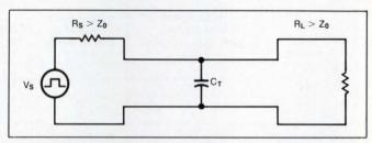
Fig 5—When the source impedance is large in comparison to the line's characteristic impedance you might be able to represent the line as a lumped capacitance.
