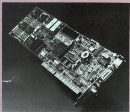
An onboard 80186  $\mu P$  handles the task of managing the Netbios protocol on the 3Com Etherlink Plus adapter for IBM PC/ATs and compatibles.
