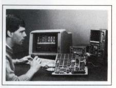
The board has both digital and analog interfaces. Two RS-232C ports connect the board to a terminal and host computer for program development. You can use an onboard codec, microphone port, speaker jack and amplifier, and a 12-bit D/A converter for linear predictive coding and echo cancellation. You can also add an A/D converter through an expansion port. \$1950.
