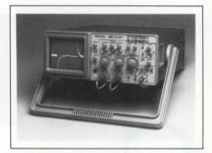
unit can display low frequency waveforms in the roll or triggered-roll modes, or it can freeze them on the screen. An external clock input, which accepts frequencies as high as 10 MHz, allows you to control data sampling and to synchronize sampling with occurrences in the equipment under test. You can collect 1k or 3k samples prior to triggering a sweep; in the pretrigger mode, a bright dot on the display denotes
