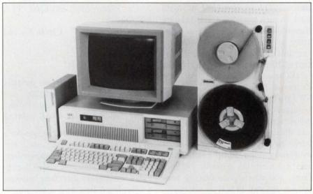
The streamer comes with standard or buffered Pertec interfaces, or with a SCSI, and it can write or read data at densities ranging from 1600 to 6250 bpi. The unit weighs 40 lbs. Standard Pertec version, \$6975;
