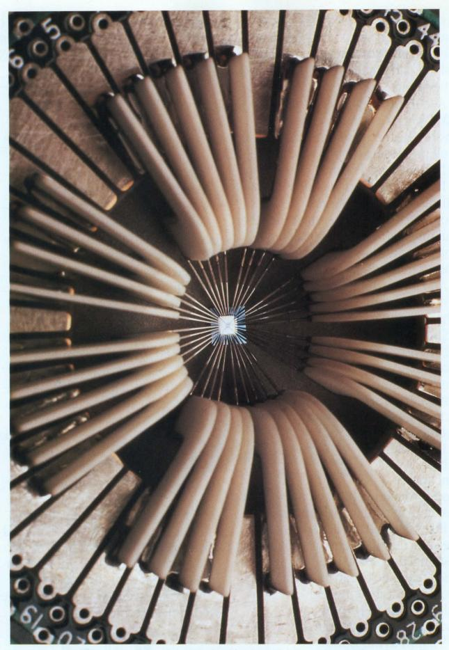
The world's smallest FETs, having feature sizes smaller than 0.1  $\mu$ m, undergo testing at IBM's T J Watson Research Center. Devices such as these minuscule transistors promise to revolutionize system design by making it possible to design ICs incorporating as many as 1 billion transistors per chip.
