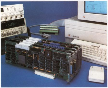
A ribbon cable connects the real-time system-integration bus on these data-acquisition and -control cards from National Instruments. The bus can link as many as five data-acquisition and -control cards, providing synchronization and DMA capability.
