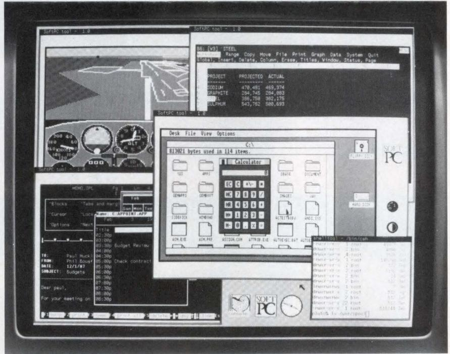
**Multiple MS-DOS-based programs can run on workstations.** The SoftPC program Insignia Solutions supplies pictorial representations of the IBM PC's monitor that indicate which programs are running. The screen shows Digital Research's GEM (including the calculator), as well as Lotus 1-2-3, Wordstar 2000, Sidekick, and Flight Simulator. Unix uses the window in the lower right corner of the screen to note its operations.
