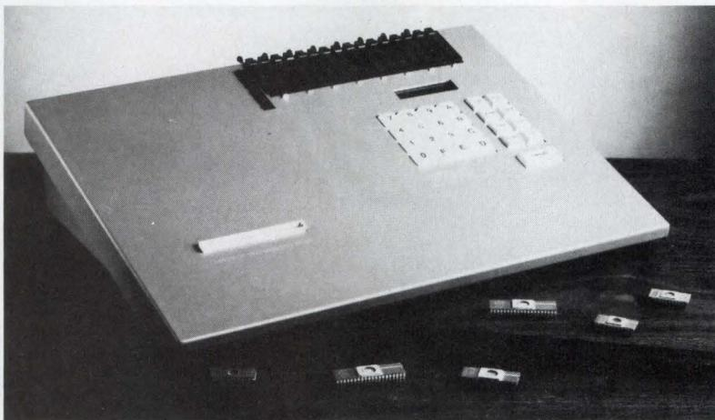
**THREE PROGRAMMERS IN ONE.** With the addition of the 135 MultiProgrammer™ BYTEK has provided a true Universal Programming Site. The 135 is a SET EPROM Programmer, a GANG EPROM Duplicator, and a UNIVERSAL DEVICE Programmer, designed for Engineering Development, Production and Field Service Environments.
