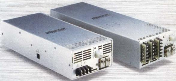
This new 250/400/600 Watt Series is designed for redundant power supply systems, providing current sharing for the main and auxiliary outputs. The modular design features one to seven outputs, 100 kHz switching, mag-amp regulation and efficiencies to 85%. Compactly packaged in a 2.75"H x 5"W format.
