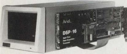
DSP-16 is a single card for the IBM PC or compatibles. Real-time 16 bit data acquisition on 2 input and output channels at up to 50 kHz simultaneously. User programmable TMS32020 or TMS-320C25. 512K or 2 Meg buffer. Concurrent sampling and anti-alias filters. Complete with software for applications and program development, common language interfaces.
