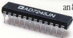
an 8-bit bus version of the AD7245 (the AD7248) that loads in two bytes.
