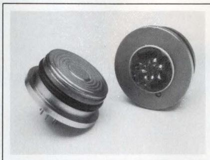
ranges from 5 to 300 psi and in absolute ranges from 5 to 50 psi. Its accuracy is  $\pm 0.5\%$ . The unit has a stainless-steel housing, which uses silicone oil to couple a diffused piezoresistive sensor to a convoluted, flush, stainless-steel diaphragm. The diaphragm interfaces with most harsh media. Integral laser-trimmed resistors provide tempera-
