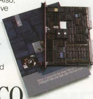
Another thing to take for granted is our R&D commitment to develop the highest performance controllers. One good example is our new Rimfire 3400. This intelligent VMEbus ESDI disk controller features a unique 512 Kbyte intelligent caching architecture and a command queuing software interface. For more information on all Ciprico controllers, for VMEbus and MULTIBUS I & II, contact us now.
