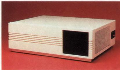
You do get a choice between two multiple-output power supplies: 190 Watts with 19A at +5V or 270 Watts with 30A at +5V. You can also choose a J2 backplane for VME extended addressing or iLBX II for a Multibus II system.
