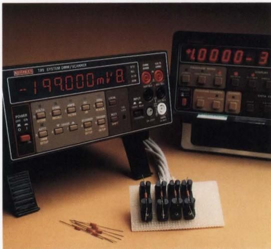
Use the Model 199 DMM/Scanner to evaluate multiple components, such as zener diodes, in a single test. Use the scanner in three different ways:
