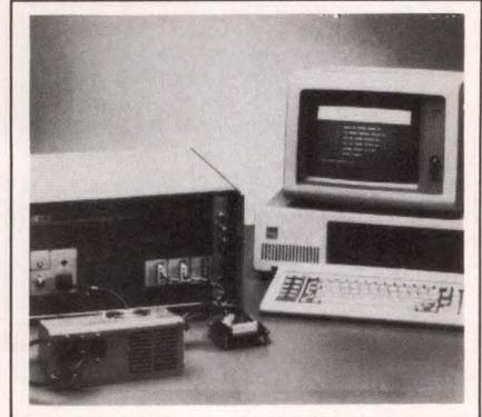
ible computer as a controller. The software supports 14 tests, which include current-limit and voltage adjustments, a p-p noise test, combined line- and load-regulation measurements, and, for multiple-output supplies, cross-regulation measurements. The programming language is Microsoft Basic. Including computer, \$11,950.
