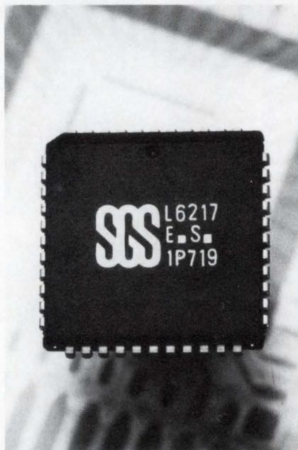
*Incorporating two H-bridge drivers, output-current regulators, and D/A converters, SGS-Thomson Microelectronics' L6217 and L6217A stepper-motor controllers allow you to microstep a 2-phase bipolar stepper motor. The plastic leaded chip carrier's special leadframe allows the devices to dissipate 2W.*
