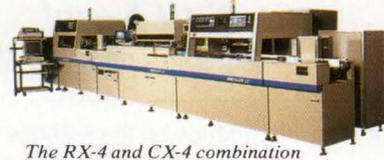
*The RX-4 and CX-4 combination mounts flat package ICs and standard chips onto double sided PCBs.*
