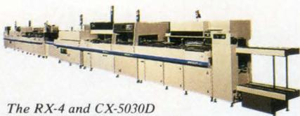
*The RX-4 and CX-5030D combination efficiently handles small batches and assorted PCBs.*
