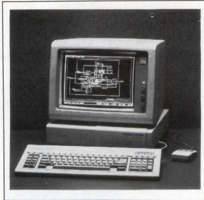
drive and a 40M-byte hard disk as options. Three AT-compatible expansion slots are standard. An AT-compatible ROM BIOS lets the computer run AT application programs. Diskless version, \$3299 to \$3499.
