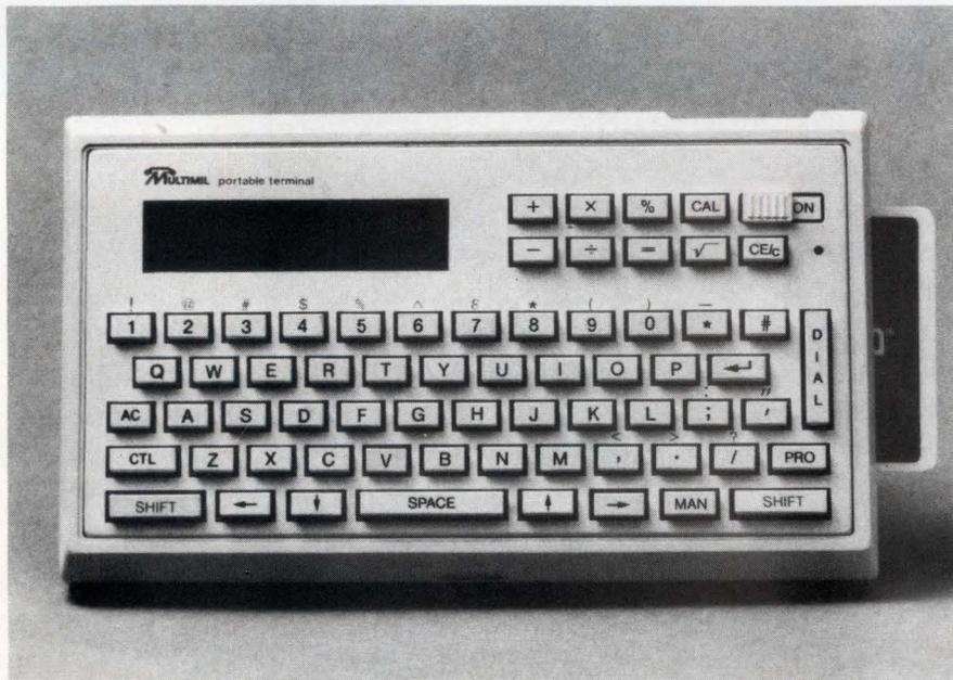
*Weighing 12 oz and measuring  $6\frac{1}{2} \times 3\frac{3}{4} \times 1\frac{1}{4}$  in., the Multiportable terminal lets you read, write, and program a Memocard smart card that contains an 8-bit  $\mu$ P and 2k or 8k bytes of EEPROM. An optional modem adds voice- and data-communication capabilities to the terminal's standard word-processing and calculating functions.*
