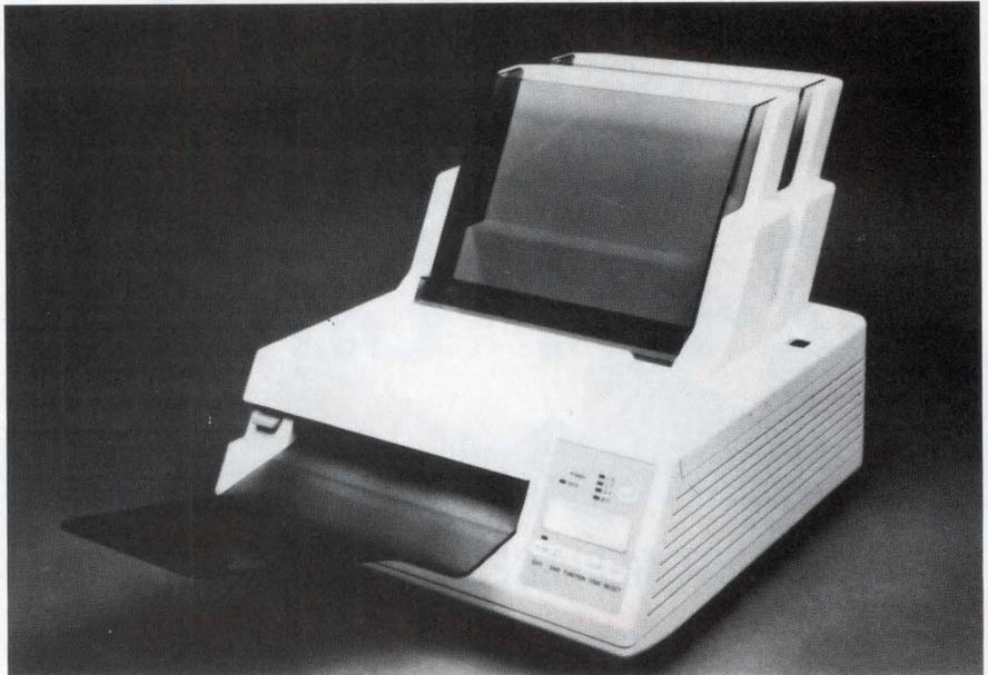
*The LED engine that Fujitsu uses in its 5-page/minute RX7100 proves to be a low-cost alternative to a laser-based engine.*
