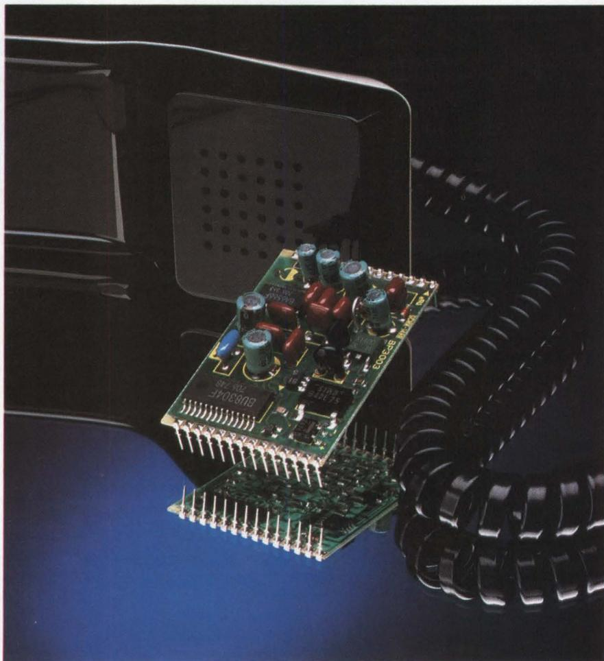
*Forming the basis for a complete telephone, this module from Rohm includes a DTMF dialer, a speech network, and a tone ringer.*
