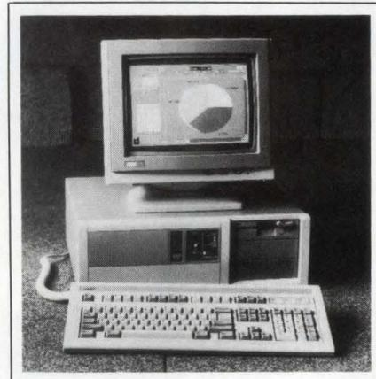
expansion slots, one 32-bit dedicated memory slot, three 16-bit PC/AT-compatible SmartSlots, one 8/16-bit standard PC/AT slot, and two 8-bit standard PC/XT slots. The SmartSlot architecture has three components: a dedicated 32-bit pathway from the processor to memory, a feature bus, and an arbitration bus. You can load coprocessors for graphics, communications, and disk control into the three
