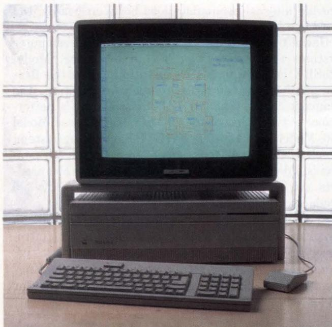
*The Macintosh II from Apple Computers is a 68020-based computer with an open architecture that has six 32-bit Nubus slots for expansion.*
