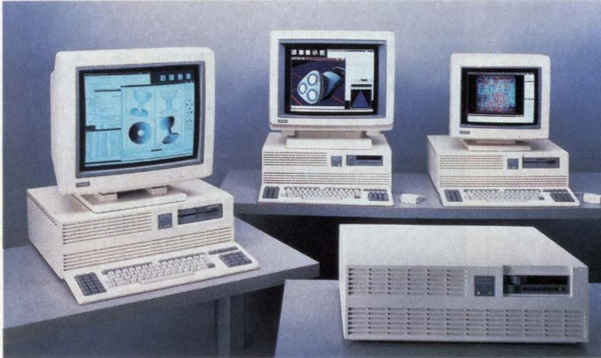
*Offering three display options—a 15-in. color, a 19-in. color, or a 19-in. monochrome monitor—the Apollo Computer Domain Series 4000 workstation is based on a Motorola 68020 running at 25 MHz.*
