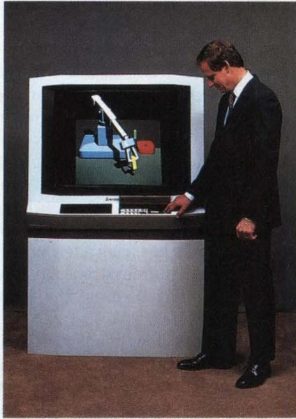
*Its flexible scan rate makes the XC-3710C color monitor compatible with the CGA, EGA, and PGA display generators. The 37-in. monitor, from Mitsubishi, offers a resolution of 640×480 pixels.*
