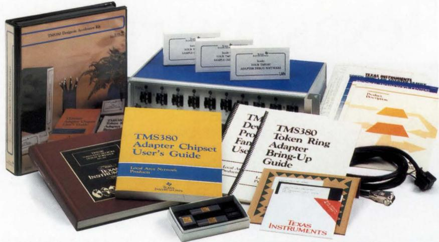
**TMS380 Bridge Design Kit** contains one TMS38021 Bridging Protocol Handler, one set of Bridge Options Adapter Software, and a TMS38021 Bridge Application Report to help you develop bridge or gateway products.
