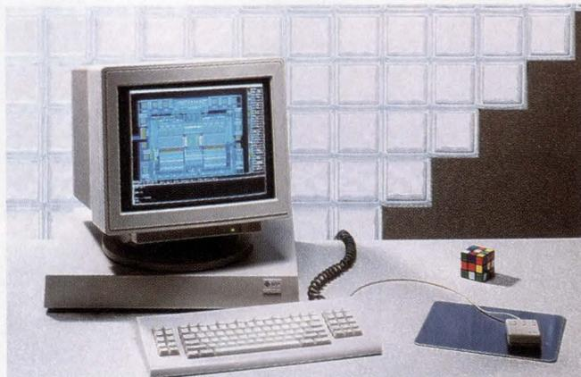
*This under-\$10,000 color workstation from Sun Microsystems uses a 20-MHz 68020  $\mu$ P. The Sun 3/60 offers a choice of five different monitors and has as much as 24M bytes of memory.*
