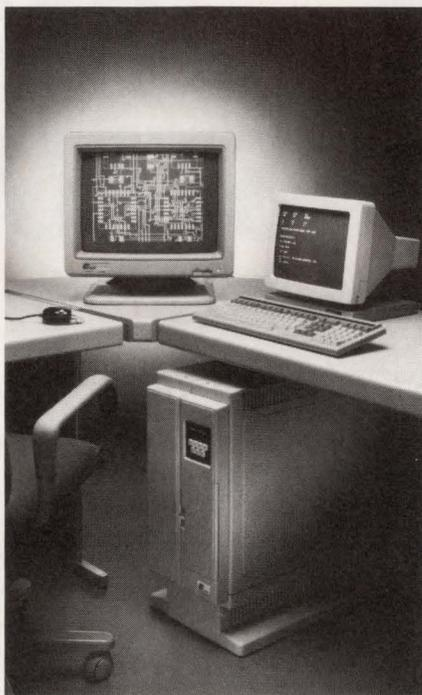
The Design Automation Series comprises the DA1000 basic workstation, the DA3000 intermediate-range workstation, and the DA5000 high-end workstation. The DA1000 is a complete design station that comes with interactive graphics; component-placement tools; a hardware, 100% autorouting package for multilayer boards; and postprocessing software.
