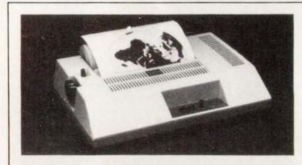
tion, fixed-array, thermal print head, which provides dot-for-dot reproduction of a screen image as dense as 1536×1024 pixels. The frame grabber captures an entire screen in 1/30 sec, so you don't need to freeze the display. The entire printing process takes 10 sec. You can choose any of 100 preset display types, which automatically set the display size, pixel resolution, and other display parameters. \$2995.
