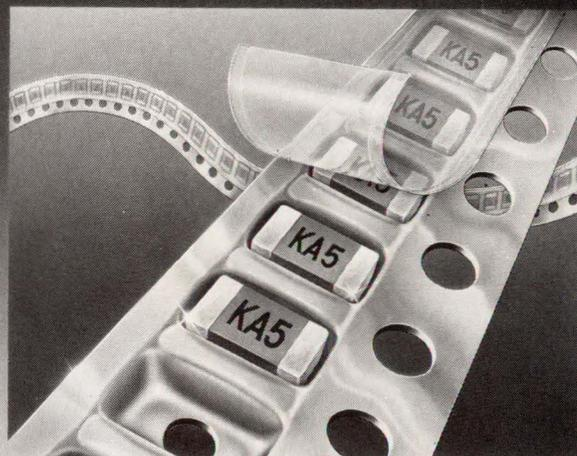
Order KEMET Multilayer Ceramic Chip Capacitors in cold-formed aluminum carrier tape packaging that works as fast as your placement machines. Easy-to-read marking. Sizes C0805 through C2225; capacitances 1.0 pF to 2.2 µF; 50 to 200 VDC. Standard, CDR and high-reliability grades.
