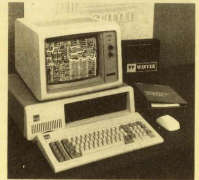
**smARTWORK® PCB Artwork Software.** In a fraction of the time hand taping requires, you can create double-sided printed-circuit boards with smARTWORK and your IBM PC. The program's features include interactive routing, continual design-rule checking, automatic pad shaving, a silkscreen, and text for all three layers. smARTWORK is \$895 and comes with a 30-day money-back guarantee. Write or call **Wintek Corporation**, 1801 South St., Lafayette, IN 47904. (800) 742-6809 or (317) 742-8428.
