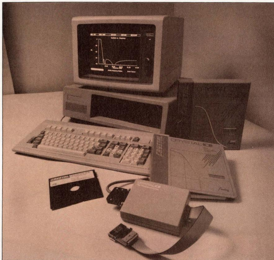
*Combining in-circuit emulation with menu-driven software, the Filter Development System from Crystal Semiconductor allows anyone who can describe the parameters of a filter to test the design. It's used in conjunction with the CS7008 universal active filter.*
