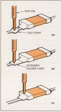
Test points need to be close to SMT devices (a). Test engineers do not recommend extending the solder pad (b) because of soldering problems. They also do not recommend probing on or near an SMT device (c) because of possible damage to the probe. (Illustrations courtesy Signetics SMD Technology)
