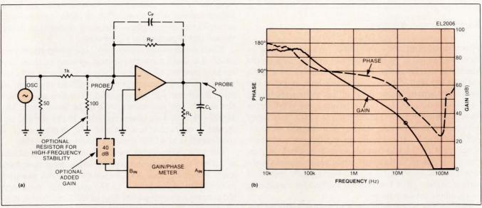
Fig 1—To measure an op amp's open-loop characteristics, you can connect the op amp in a "gain of -10" arrangement (a), in which most devices are stable. The gain/phase meter measures the  $V_{OUT}/V_{IN}$  of the amplifier. You can use the optional 40-dB gain block to increase the input signal to the meter. The plot (b) shows the gain and phase of the EL2006 op amp as a function of frequency. Where the gain is 34 dB, zero phase occurs at 15 MHz.
