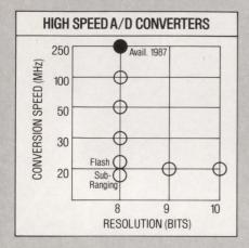
Our A/D converters include an 8-bit, 100-MHz device that was designed for the super-slow motion equipment used in the 1984 Olympics. A TDC-1048 replacement chip (CXA 1096 P) that requires just 25% of the 1048's power dissipation. A unique 20-MHz, 10-bit chip. And a 250-MHz, 8-bit converter that will be available in early 1987 (All 30-to 100-MHz A/D converters are available with extended temperature range, from -55°C to 125°C.)
