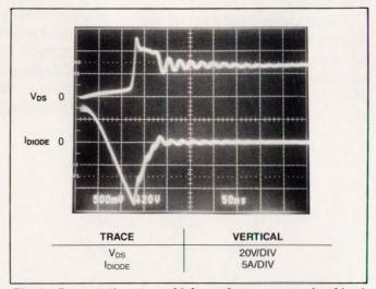
Fig 10—Commutation at very high speeds can cause avalanching in the device under test—an unreliable mode of operation.
