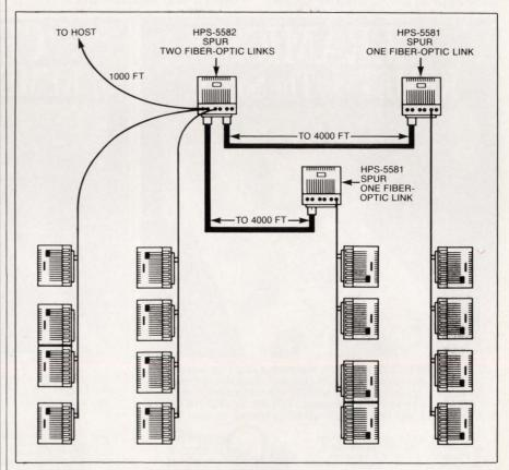
A combination of coaxial and fiber-optic links between the HPS-5581 and HPS-5582 repeaters (Spurs) and HPS cluster controllers provides electrical isolation and flexible fan-outs to terminals. The Spurs also allow you to extend your computer-communication links to as much as three miles.
