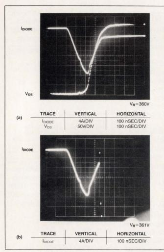
Fig 5—Instead of failing during peak dv/dt (a), the 4A/450V device that was tested to generate these waveforms failed when the reapplied voltage was increased from 360 to 361V (b).
