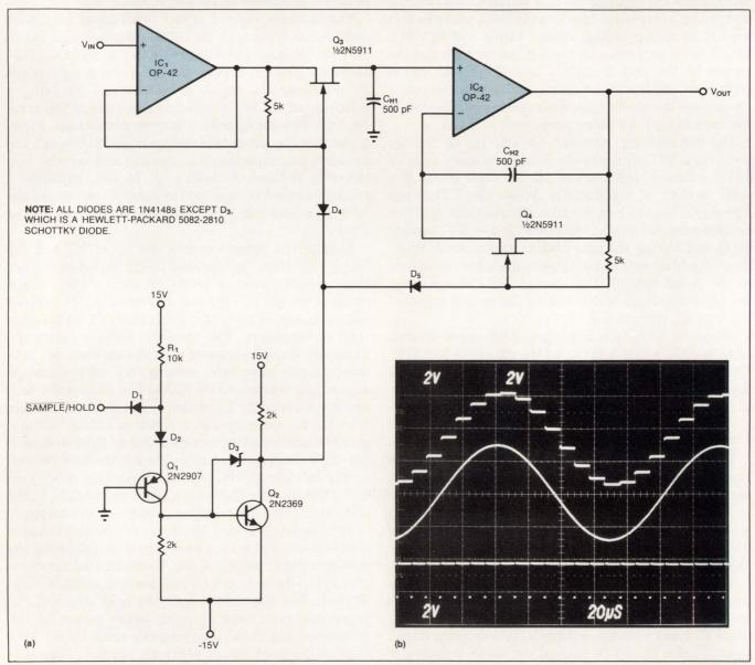
Fig 2—This fast sample/hold amplifier (a) uses two hold capacitors to minimize both the hold-step effect and the output droop. You can see the very small hold step and the absence of droop in the scope photo (b).
