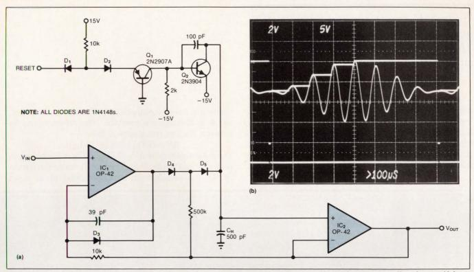
Fig 3—This peak detector (a) can capture a 10V peak that's only 2.5 µsec wide. After a reset it can detect very small peaks even if the ac signal has a negative dc offset. The detector's JFET-input amplifiers have very low input bias currents and therefore minimize leakage from the hold capacitor. This low leakage is responsible for the absence of droop (b).
