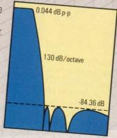
Passband ripple is 0.044 dB p-p, and there's 1° phase match up to the cutoff frequency.
