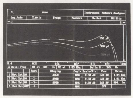
form of virtual instruments screen representations that mimic the format of real instruments. You can perform advanced calculations on the data acquired from the simulator, and you have tremendous flexibility in selecting the preParametric plotting allows you to optimize a circuit by changing component values and seeing the results of these changes. Here, FutureNet's Dash-Analog Workbench displays the frequency response of a circuit with various values of a capacitor.
