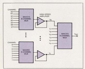
Fig 7—By adopting a 3-tiered approach and adding high-speed amplifiers, you can significantly improve the frequency response of the multiplexing circuitry.
