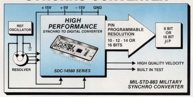
The SDC-14560 series S/D converters offer programmable resolution of 10, 12, 14 or 16 bits, tachometer-like high quality velocity output and accuracy to 1.3 arc minutes. In addition, a Built-In-Test (BIT), CT mode operation, transparent latch, and three-state output in two bytes are standard features.
