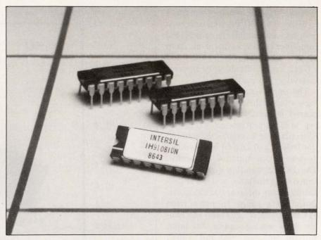
Capable of handling  $\pm 50V$  signals, the IH9108 8-channel multiplexer from GE-Intersil features a source off-state leakage of 2 nA and a drain off/on-state leakage of 15 nA.
