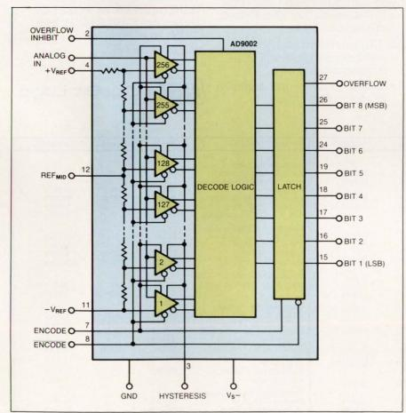
Featuring a sampling speed of 150M samples/sec and an analog bandwidth of 115 MHz, the AD9002 8-bit flash A/D converter includes 256 parallel comparator stages whose outputs are decoded to drive the ECL-compatible output latches.
