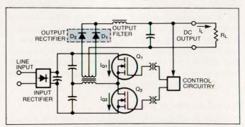
Fig 3—A MOSFET's intrinsic diodes generally do not experience commutating-dv/dt stress in a half-bridge switching power supply, even though they act as freewheeling rectifiers.
