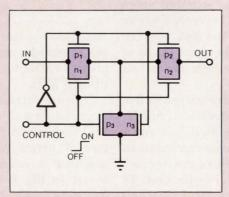
Fig A—A video switch's typical T configuration improves off-isolation.
