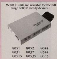
And, if you add our optional MetaICE-CHEST feature (included in MetaICE-80515), you can reach a full 64K of program and external data memories, 128,000 hardware breakpoints, 4K trace buffer and 15 break/trace conditions—for an additional \$1,495.
