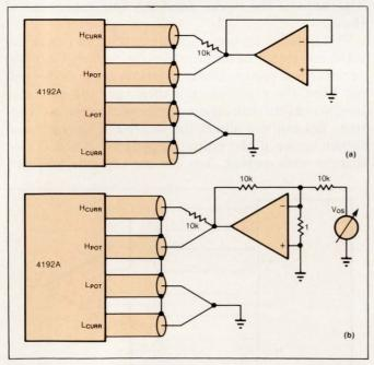
Fig 3—You can measure either the closed-loop or the open-loop output impedance of an op amp. The circuit in a is for testing an op amp connected as a unity-gain buffer. The circuit in b measures open-loop output impedance. You should operate the device at a frequency high enough to limit the open-loop gain to less than 10,000.
