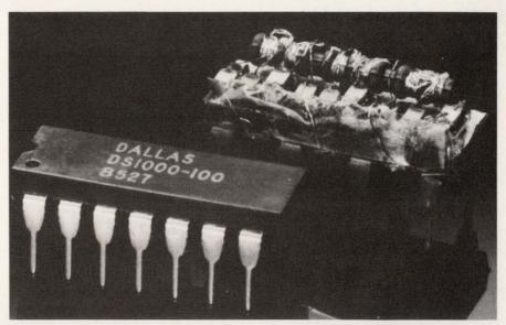
This monolithic CMOS delay line, a member of the DS1000 Series, has five delay taps, each laser-trimmed to within 1 nsec of the desired delay value. The manufacturer, Dallas Semiconductor, claims the device is more reliable than the conventional LC hybrid type shown in the background (without its cover).
