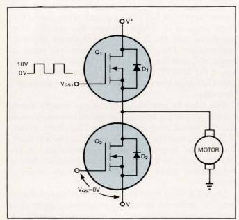
Fig 1—Commutating-dv/dt stress on the power transistors is a major problem in this PWM dc motor-controller system.
