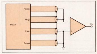
Fig 2—To measure an op amp's input impedance, you connect the 4-wire ac ohmmeter arrangement of the HP 4192A directly to the input of the amplifier. To obtain accurate measurements, you should use the smallest possible drive signal.
