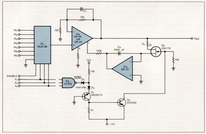
Fig 1—This autozeroing amplifier multiplexes seven inputs to a common output. The eighth input grounds the input of  $IC_2$  to zero the amplifier's offset voltage. Before you select a signal, hold the three address lines high for 200 usec to ensure proper zeroing.
