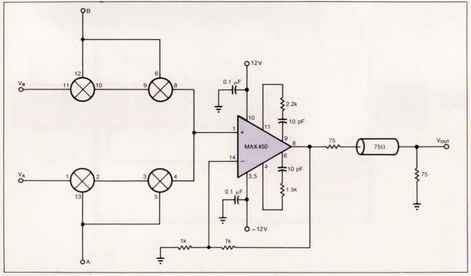
Fig 5—A CMOS-input amplifier such as the MAX450 presents a lighter load to your video switch.
