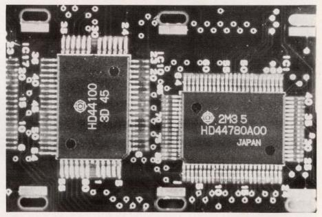
The finer lead pitches and high pin counts of SMT devices make pc boards bearing SMT devices harder to test than boards manufactured with older, less-dense technologies. (Photo courtesy Hewlett-Packard's Manufacturing Test Div)
