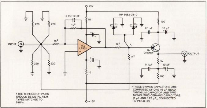
Fig 1—This circuit measures op-amp settling time by creating a false summing node (A) at virtual ground, which tracks the amplifier's output settling excursions.
