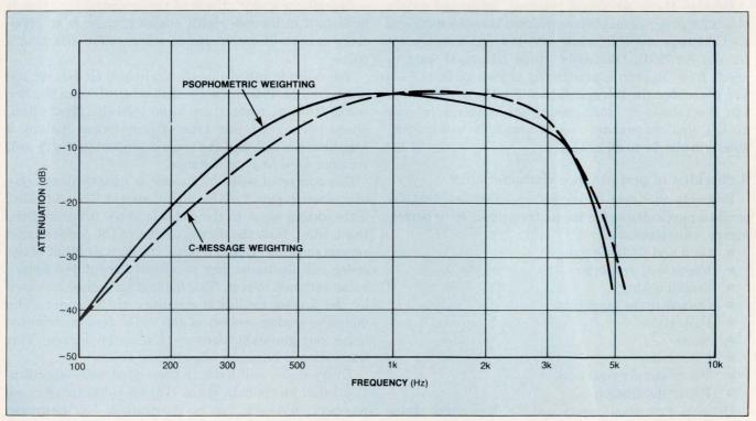
Fig 2—Telephone users are more irritated by noise at certain frequencies than noise at other frequencies. Consequently, the C-message weighting curve, which represents the response of the human ear to noise at different frequencies, was developed for use in the US, and the slightly different P-message weighting curve is used in Europe.
