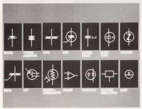
By consulting its tables of current-vs-voltage functions, the ACS System can simulate circuits that contain such devices as SCRs, triacs, and lamps.
