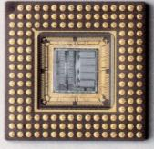
Channel-free Compacted Arrays combine logic and memory functions with up to 129,000 available (up to 70,000 utilized) gates.
