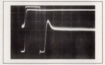
Fig 4—This settling waveform shows that Fig 3's circuit has clipped the undershoot (off the screen in Fig 2) at -250 mV, allowing accurate measurement of the amplifier's 310-nsec settling time. Horizontal scale is 100 nsec/div; vertical scale is 2V/div for top trace, 50 mV/div for bottom trace.
