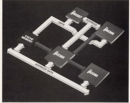
A 20-MHz 80386 µP and its three 16-MHz support peripherals form the core of a 32-bit computer. The support chips use the same microinstruction set that the  $\mu P$  uses.
