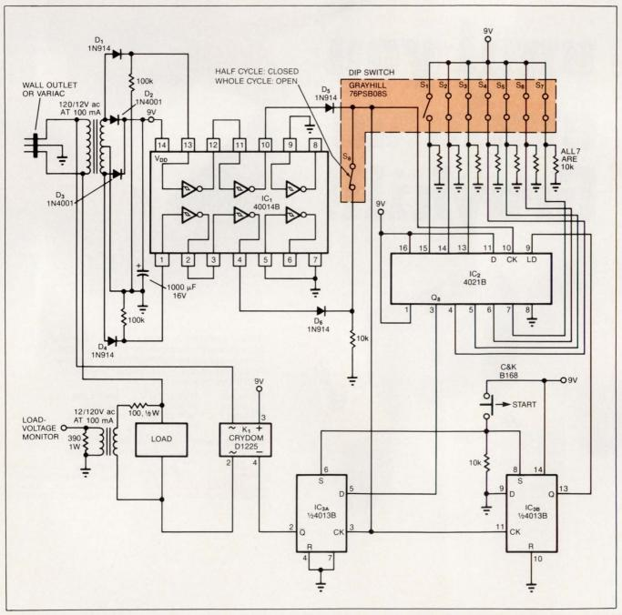
Fig 1—This circuit deletes a sequence of whole or half cycles from the line voltage applied to the load according to a 7-cycle pattern that you program using the DIP switch's sections  $S_1$  through  $S_8$ .
