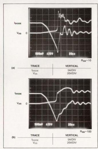
Fig 8—Increasing  $R_{GS}$  slows the reverse-recovery process and increases commutation power losses. However, the higher impedance reduces peak instantaneous stress and may also keep the device from avalanching.
