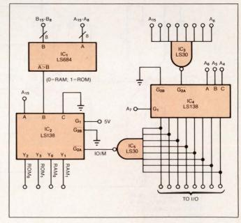
Fig 3—These ICs control Fig 1's memory. IC, and IC, select the RAM and EPROM chips according to the fence-address position, and IC, and IC, decode I/O addresses. IC, generates an IO/M signal.
