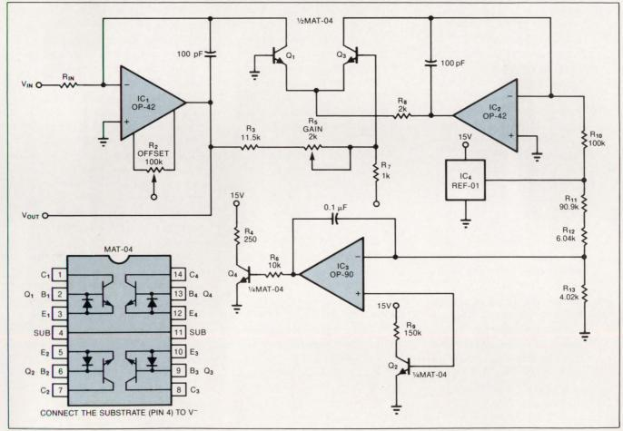
Fig 4—This logarithmic amplifier eliminates temperature effects by ensuring that the two log-conversion transistors are always at the same temperature. The conversion transistors are on the same substrate as a heater transistor and a temperature sensor, which are connected to each other in a feedback loop.
