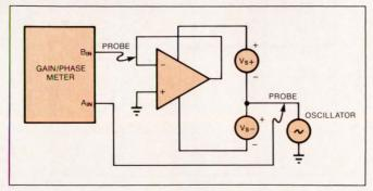
Fig 5—This circuit provides a common method of measuring an op amp's CMRR. The oscillator drives the supplies with respect to the noninverting input of the op amp. Supply variations cause a  $V_{\rm OS}$  variation at the amplifier's input; this variation is measured at the B input of the gain/phase meter. The problem with this approach is that the op amp's output also sees the supply-voltage variations.
