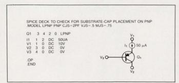
Fig 2—By representing a pnp transistor as shown, you can determine whether your Spice program is modeling it correctly.
