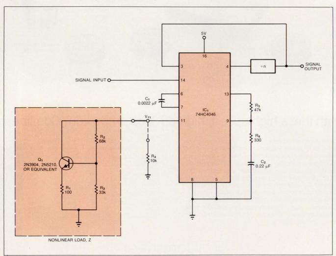
Fig 1—By connecting the nonlinear load Z to pin 11 of the PLL chip  $IC_i$ , you can extend the PLL's frequency range by a factor of 50, as compared with that possible by using a fixed resistor  $(R_i)$ .
