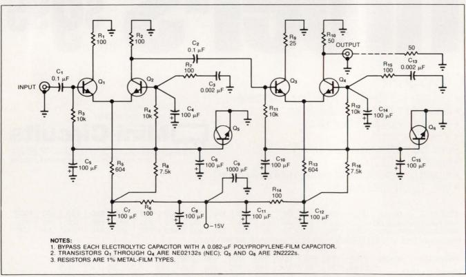
Fig 3—This 2-stage RF amplifier amplifies and clamps the output of Fig 1, letting you observe the final settling waveform at a resolution of  $\pm 1$  mV without overdriving the oscilloscope's vertical amplifier.
