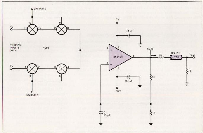
Fig 3-By adding an amplifier to the circuit of Fig 2, as shown here, you can drive the video cable properly.
