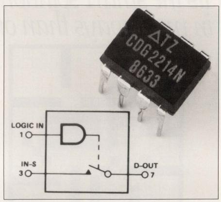
A 3-dB bandwidth of 250 MHz distinguishes the CDG2214 spst analog switch from Topaz Semiconductor. The device also specs off-state isolation figures of 100 and 200 MHz at 37 and 22 dB, respectively.
