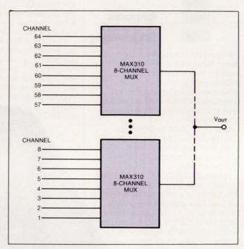
Fig 6—This method of ganging multiplexers degrades the bandwidth of your video circuitry.
