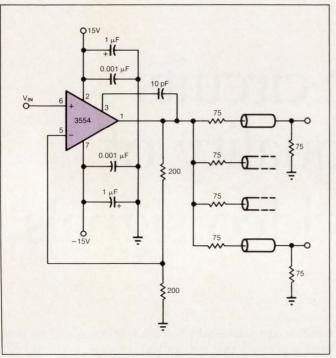
Fig 1—The 3554 amplifier has the drive capability to drive several video cables; it's shown here configured as a distribution amplifier.
