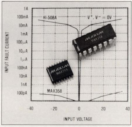
Analog inputs of  $\pm 35V$ , when applied to unpowered MAX358, -359, -368, or -369 8-channel (SE) and 4-channel (differential) multiplexers from Maxim Integrated Products, typically result in less than 200 pA of input current.
