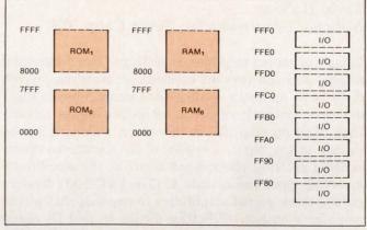
Fig 1—This 64k-byte memory system provides 64k bytes of physical RAM virtually overlapped by 64k bytes of physical EPROM.
