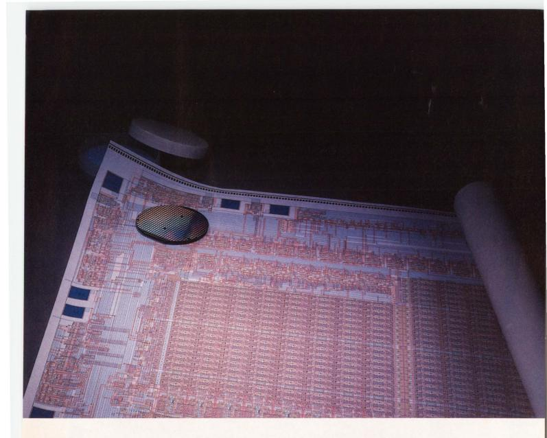
Structured Chip Design (SCD), a hierarchical approach to physical layout, removes much of the unnecessary and confusing mask data, while retaining correct functionality and interfaces.
