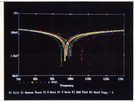
Using Monte Carlo analysis to determine the effect of component variations on circuit operation, MicroSim's PSpice can help you create designs that are tolerant of manufacturing inconsistencies.
