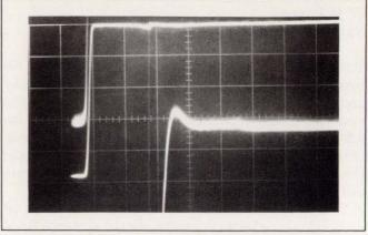
Fig 2—Fig 1's response to an approximate 10V-step input shows an undershoot on the lower trace that overloads the scope. The resulting scope-recovery time produces an apparent 500-nsec settling time for the amplifier under test. Horizontal scale is 100 nsec/div; vertical scale is 2V/div for top trace, 5 mV/div for bottom trace.
