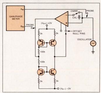
Fig 6—This circuit measures an op amp's CMRR. The setup uses the  $V_{\rm OS}$  balance pins of the amplifier as a feedback path. You connect the inputs and drive them with the oscillator. Thus, you can measure a CMRR greater than the open-loop gain over a wide frequency range.
