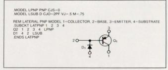
Fig 3—If your Spice program is incorrect, substitute this pnptransistor model, which uses a diode to model the junction-substrate capacitance for the model in Fig 2.
