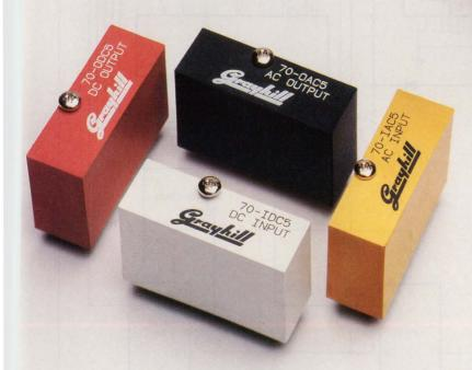
You'll find outstanding specs, performance, pricing and availability in these new I/O Modules...from Grayhill or your local Grayhill distributor, in all standard configurations. All are compatible with 5, 15 or 24V logic circuits.
