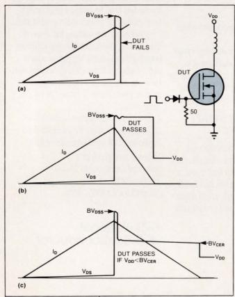
Fig 9—Because of defects in the present UIS test method, a device may fail in one of three ways. Some devices fail immediately in avalanche (a), while others can maintain their  $BV_{DS}$  during the entire transient period (b). In the third case (c), the drain-to-source voltage of some devices may collapse to a lower level.
