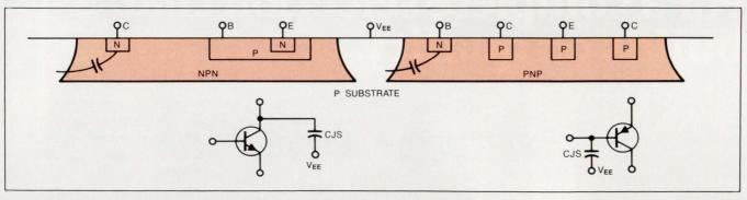
Fig 1—This wafer cross-section shows the structure of npn and pnp transistors used in bipolar-IC processes. As shown, the models for the junction-to-substrate capacitance (CJS) should connect to the npn's collector and to the pnp's base, respectively.
