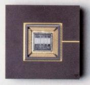
Structured Arrays combine high-density memories with up to 41,000 logic gates.
