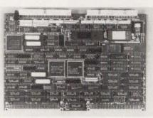
By employing read-ahead and sectorpacketizing techniques, the 752 single-board disk controller achieves an aggregate DMA transfer rate of 10M bits/sec.
