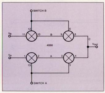
Fig 2—You can configure a 4066, with its bilateral switches, as a video multiplexer.
