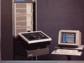
Available in desktop and rackmount versions, the DAS9200 mainframe can be augmented with up to three expansion mainframes for a total of 28 card slots.
