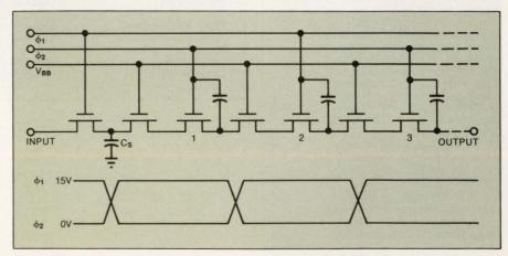
Fig 2—This structure is a bucket-brigade-type of analog delay line, in which a signal in the form of discrete charge packets shifts one stage along the chain with each cycle of the clock waveforms  $\phi_1$  and  $\phi_2$ . ( $V_{BB}$  is a dc voltage that biases the interstage transistors, which minimize the Miller capacitance between stages.)
