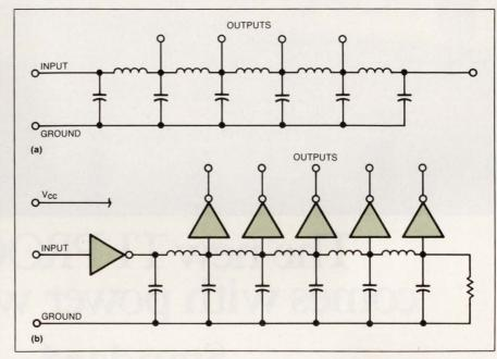
Fig 1—A passive LC delay line (a) consists of sections in cascade, each containing a series inductor and a shunt capacitor. An active, digital delay line (b) includes inverter gates.
