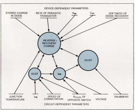
Fig 4—Many parameters affect total device stress during commutating dv/dt, and it can be difficult to select the meaningful and convenient independent variables for CSOA testing. The CSOA spec begins with  $I_{FM}$ , the reapplied voltage, and the commutation speed.
