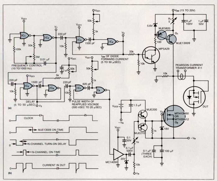
Fig 6—To determine the characteristics of just the transistor under test, this CSOA test circuit's design and layout minimize the effects of circuit parasitics.
