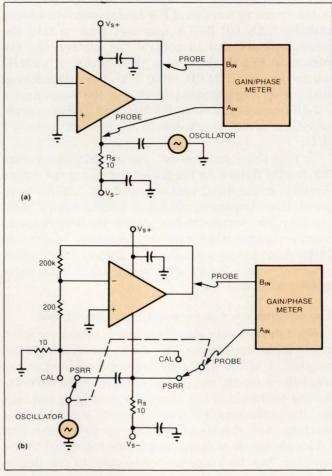
Fig 4—A simple way to measure an amplifier's PSRR is shown in a, in which a small ac component from the oscillator is superimposed on the supply voltage. The quantity B/A on the gain/phase meter provides a direct reading of PSRR. The circuit in b provides an improved method of measuring PSRR. In this circuit, the op amp provides a gain of 1000. This gain enhances the low-frequency PSRR range by some 60 dB, and you must normalize B/A readings.
