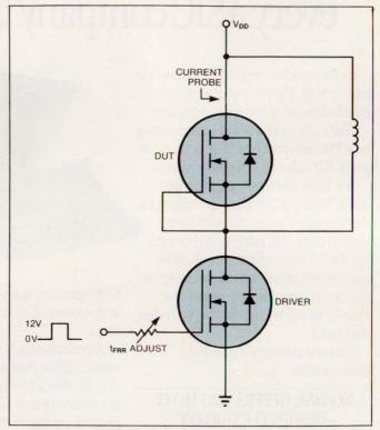
Fig 7—Although it's simpler and more convenient than Fig 6's circuit in some aspects, this CSOA test circuit lacks flexibility. The biggest problem is that circulating current is a function of supply voltage, so it's difficult to change these parameters independently of one another.
