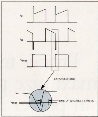
Fig 2—All three conditions for commutating-dv/dt failures are evident in these motor-controller waveforms.  $I_{D2}$  shows the effect of the diode's conducting during the switching cycle,  $I_{Q1}$  reflects the need to remove stored charge rapidly during reverse recovery, and  $V_{DSQ2}$  shows the need to extract the stored charge through a high reapplied voltage.
