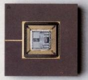
High Performance cell-based 1750 CPU combines logic, ROM and processors.
