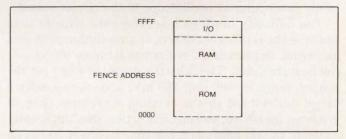
Fig 2—The logical organization of Fig 1's memory locates memorymapped I/O space at the top of the RAM and lets you set the boundary between the RAM and EPROM by manually setting a fence ad-
