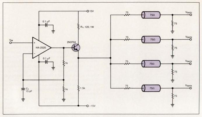
Fig 4—An emitter-follower allows you to boost the output drive of your video circuitry.
