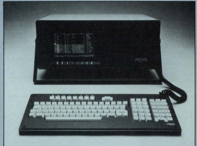
*You can develop software for many microcontrollers on this 8-bit development system, the Echo from Arium. The system lets you test your software right on the target machine with the aid of an emulator and a personality board that control the execution of your programs and trap errors.*
