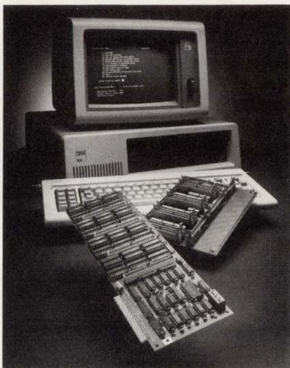
*Providing a low-cost means of developing microprograms, this microprogram-memory emulation card and target-interface board, which come with software, comprise the AG-11B microprogram development tool. The product lets you quickly load and test microcode in your target system; it also provides a hardware breakpoint signal for test purposes.*
