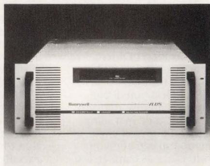
*Storing 5.2G bytes on a VHS tape cassette, the VLDS sustains a data-input rate of 4M bytes/sec and features a bit-error rate of 1 error in 10<sup>12</sup> bits.*
