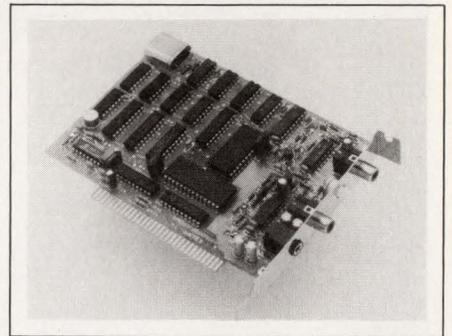
range and a 4- or 8-kHz sample rate. When you use a 4-kHz sample rate, the board requires 7.2M bytes to store one hour of digitized signal. \$345.
