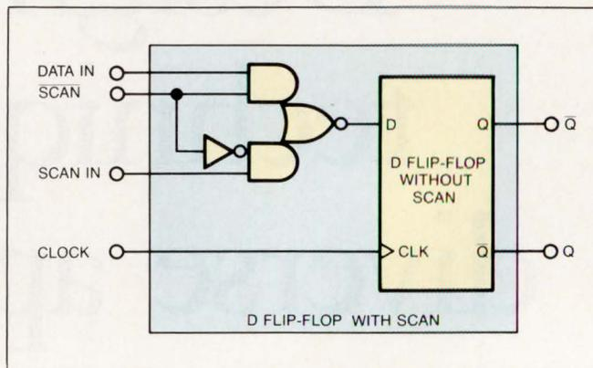
**Fig 1—When you use the structured technique, your circuit overhead increases in proportion to the number of gates required to implement the scan capability within a sequential device. For example, it might take three or four extra gates to perform the scan function for a D-type flip-flop.**
