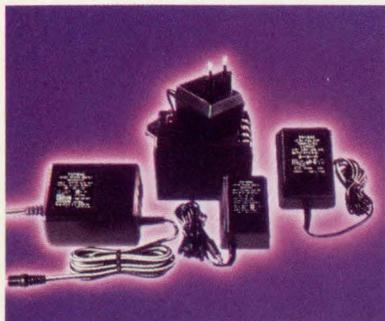
Linear wall-plug-in supplies like these are suitable for applications requiring less than 25W; switching versions are offering outputs approaching 100W (pg 107).
