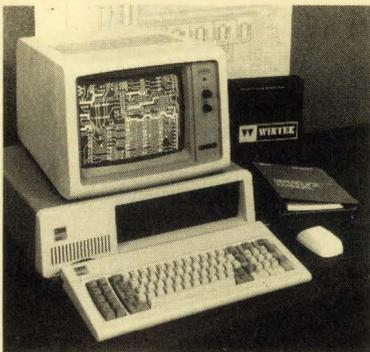
**smARTWORK® PCB Artwork Software.** In a fraction of the time hand taping requires, you can create double-sided printed-circuit boards with smARTWORK and your IBM PC. The program's features include interactive routing, continual design-rule checking, automatic pad shaving, a silkscreen, and text for all three layers. smARTWORK is \$895 and comes with a 30-day money-back guarantee. Write or call **Wintek Corporation**, 1801 South St., Lafayette, IN 47904. (800) 742-6809 or (317) 742-8428.
