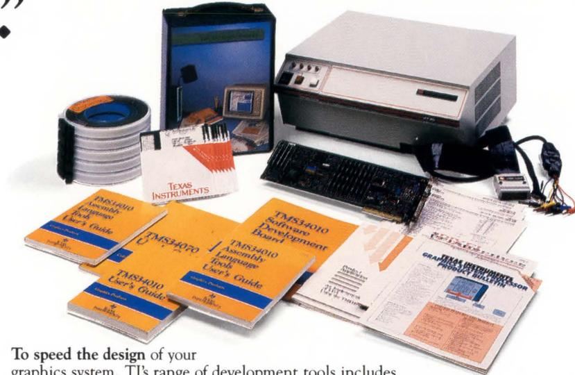
To speed the design of your graphics system, TI's range of development tools includes a comprehensive design kit (left rear), a realtime emulator, and a plug-in software development board. On floppy and magnetic disks: "C" compiler, assembler package, and function and font libraries. User's guides, development books, product bulletins and data sheets, and TI's newsletter, *Pixel Perspectives*, are all readily available.
