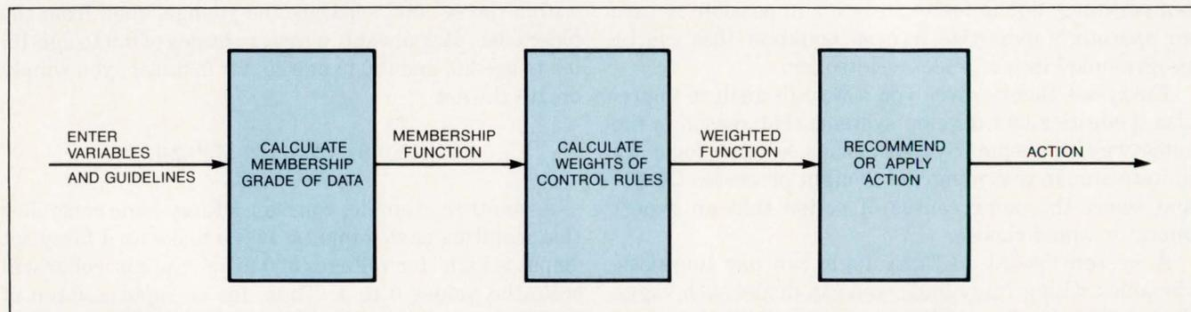
Fig 2—By following these steps, a fuzzy-logic controller can analyze a set of process variables, find the weighted average of all control rules in the process, and perform the same action that an expert operator would.
