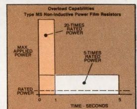
For even higher overload situations, Type MS resistors can be subjected to 20-times the rated power for one second.
