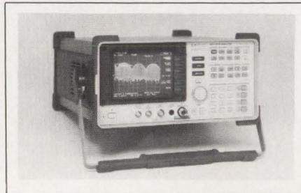
analyzers, cover a 1-kHz to 22-GHz frequency range. The HP 8562A provides tracking preselection from 2.75 to 22 GHz; the HP 8562B provides no preselection. The instruments have a 1-dB/division scale factor, and their synthesized tuners sport 100-Hz tuning steps. The analyzers' frequency response is  $\pm 1.2$  dB at 2 GHz and  $\pm 4.3$  dB at 22 GHz. The ratio of signal to harmonic distortion is 100 dB max; the ratio of signal to intermodulation distortion
