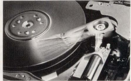
*A servocontrolled, rotary voice-coil actuator gives this 53.3M-byte, half-height, 5¼-in. Winchester disk drive its high capacity and speedy (25-msec) average access time.*
