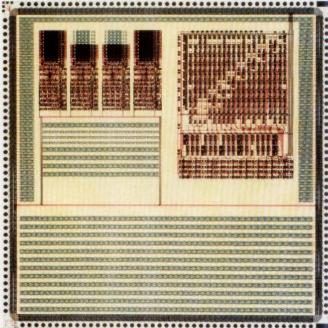
*You can integrate an entire microprogrammable system onto one piece of silicon using semicustom or gate-array ASIC products like this LSA2011 structured array from LSI Logic. The device incorporates four 2901 ALUs, a 16×16-bit multiplier/accumulator, and 5000 uncommitted logic gates.*
