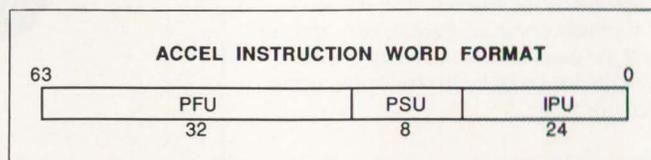
**Fig 4—That a fixed-architecture processor can be microprogrammable** is evident in the 64-bit instruction word in Weitek's Accel  $\mu$ P Series devices. The family's 8032 and 8064 processors use the full 64-bit microword, divided into a 24-bit field for the integer processing unit (IPU), an 8-bit field for the program sequencing unit (PSU), and a 32-bit field for the floating-point unit (FPU).
