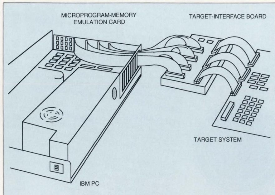
*The target-interface board supplied with the AG-11B links the product's microprogram-memory emulation card with your target system by using four shielded, 50-conductor ribbon cables between the memory card and the target-interface board and three user-supplied, 50-conductor cables between the target-interface board and the target system.*
