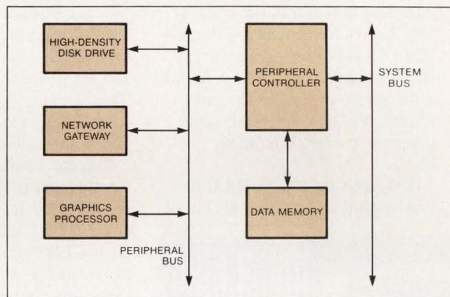
**Fig 1**—This block diagram depicts the architecture of the system that employs the peripheral controller. The controller receives commands and data from the host processor and then responds with status and data.
