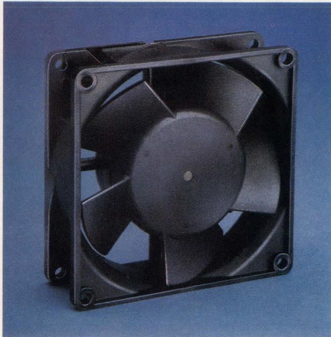
MULTIFAN uses 1/3 of the power required for AC motors and can be used interchangeably with an AC voltage or frequency when operating from secondary circuitry. Featuring a maintenance-free life expectancy in excess of 40,000 hours, locked rotor and reverse polarity protection, minimize noise level, permanently lubricated ball bearings, and extremely low weight. Available in four series.
