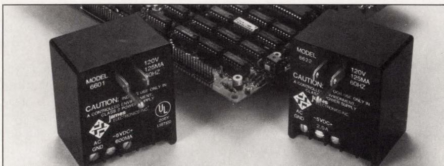
*Five-volt designs are best suited to a hybrid wall plug-in supply such as one of these from James Electronics. A hybrid supply has a linear front-end to reduce and rectify the line voltage to an 8 to 9V range, followed by a switching regulator to translate the unregulated 8 to 9V to 5V.*
