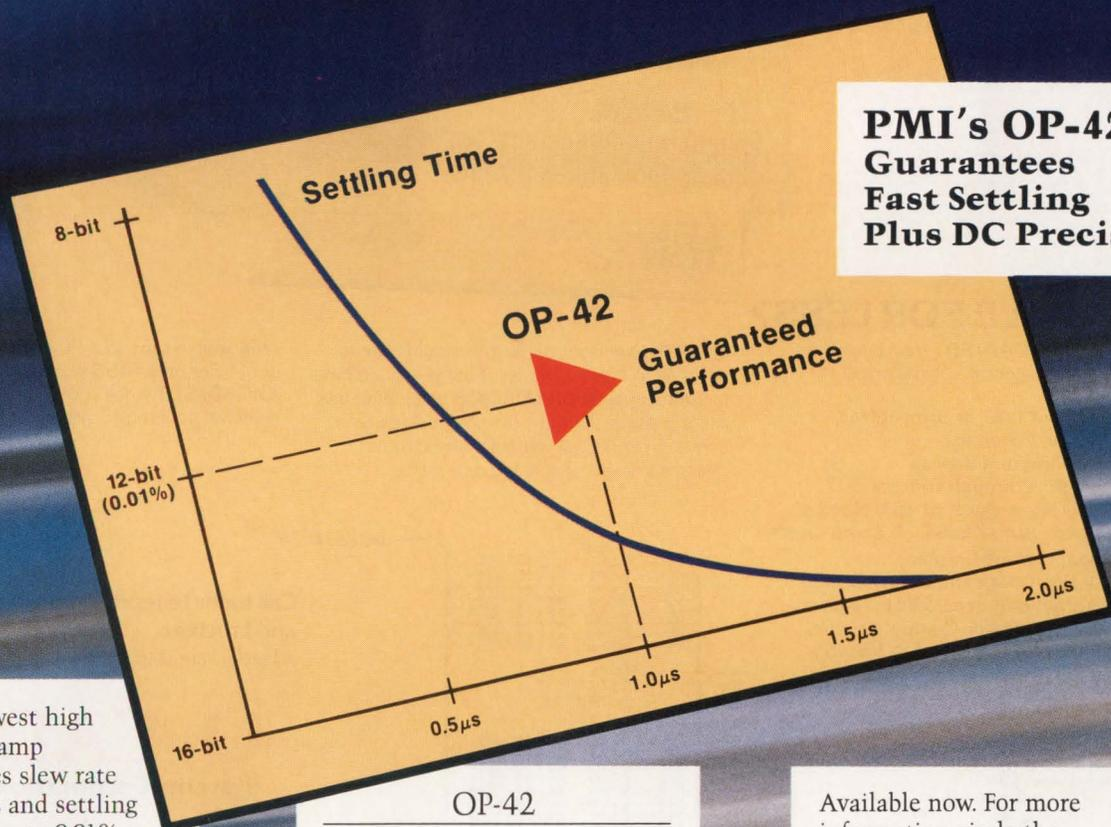
PMI's newest high speed op amp guarantees slew rate of  $50V/\mu s$  and settling time of  $1\mu s$  to 0.01%. With its 10MHz gain bandwidth and 850kHz full power BW, the OP-42 combines high speed with accurate DC performance.
