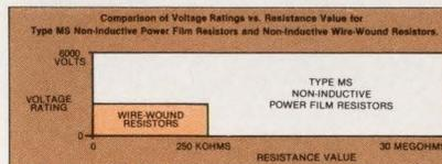
The higher voltage rating of Type MS resistors also overcomes the resistance value limits imposed on wire-wounds by the minimum wire size and spacing.
