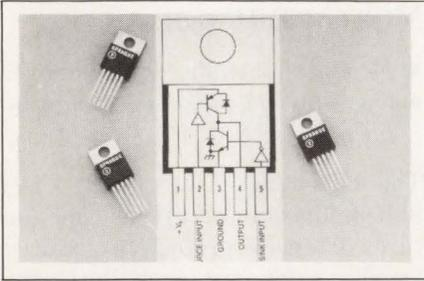
crossover-current protection, short-circuit protection, transient suppression, and input-logic lockout, which prevents source drivers and sink drivers from turning on simultaneously. The motor driver operates via pulse-width modulation, and it has saturated outputs. The 24V/1A bipolar device is available in a modified 5-lead, power-tab, TO-220 plastic package. \$1.35 (100). Delivery, 10 to 12 weeks ARO.
