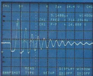
Waveform Parameter Extraction allows you to make specific measurements on the windowed portion of a waveform. Here, frequency and peak-to-peak voltage measurements are made on two cycles of a damped sine wave. The cursors set the limits of the window.
