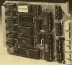
The 890 Z80A Multifunction CPU card is an integrated hardware/software solution for industrial control applications.
