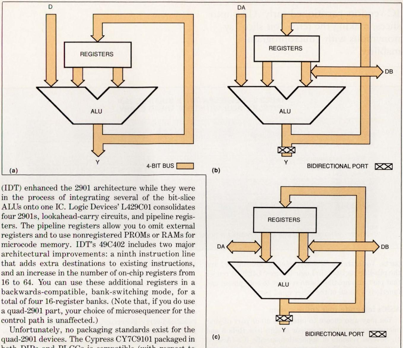
**Fig 2—Today's microprogrammable ALU/register files trace their lineage back to AMD's venerable 2901 (a), which had one input (D) and one output (Y) data port. Data movement became much easier in the 2903 (b), which gained a bidirectional DB data port and an improved, bidirectional Y port. The 29203 (c) completed the evolution of the ALU/register-file IC by rendering all three data ports bidirectional.**
