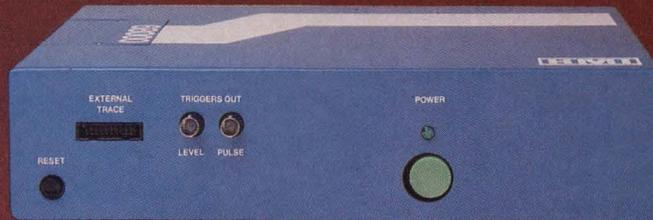
The HMI-200 series of microprocessor in-circuit emulators combine all of the features of an emulator and a powerful logic analyzer while utilizing your own IBM PC family or UNIX-based computer. These emulators are a result of HMI's years of experience in the design and application of emulators for all popular microprocessors and offer performance and capability that is unexcelled. Units are
