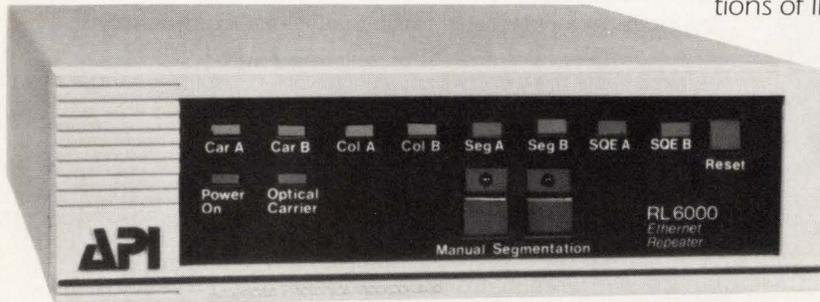
Connections can be made with either coax cable (Local) for segments greater than 50 meters apart or with fiber (Remote) for segments up to 1km.
