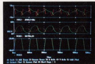
Also, our PSpice analog circuit simulator gives you more than just voltages (for example, *group delay* for filter design). Probe shows the answers you need, quickly and accurately.
