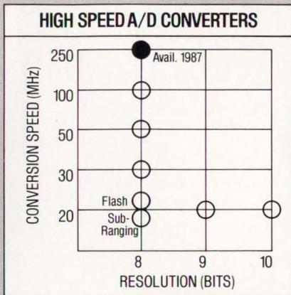
Our A/D converters include an 8-bit, 100-MHz device that was designed for the super-slow motion equipment used in the 1984 Olympics. A TDC-1048 replacement chip (CXA 1096 P) that requires just 25% of the 1048's power dissipation. A unique 20-MHz, 10-bit chip. And a 250-MHz, 8-bit converter that will be available in early 1987. (All 30- to 100-MHz A/D converters are available with extended temperature range, from  $-55^{\circ}\text{C}$  to  $125^{\circ}\text{C}$ .)
