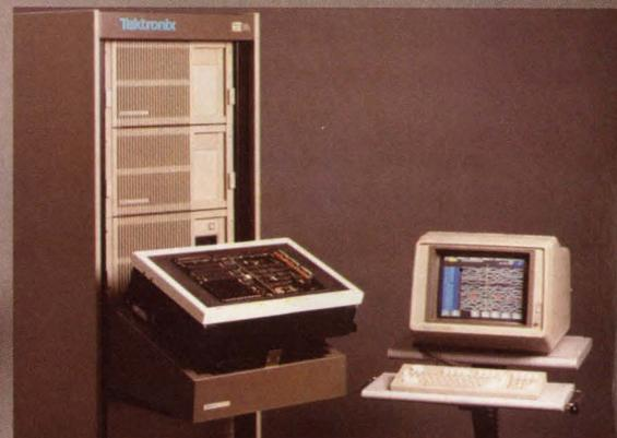
Available in desktop and rack-mount versions, the DAS9200 mainframe can be augmented with up to three expansion mainframes for a total of 28 card slots.
