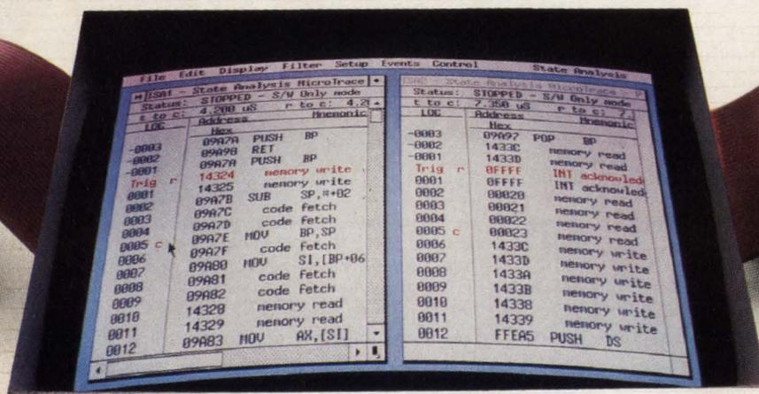
Since so many embedded microcomputer designs employ more than one processor, you'd think there would be many tools to trace multi-processor dialog in both assembly-level and high-level code. And then time-align the results.
