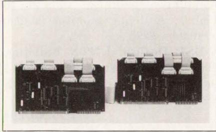
tween a Multibus computer system and a VME Bus computer system. The translator disguises the Multibus system as a typical VME Bus board by performing all the necessary VME Bus-to-Multibus signal and timing conversions. The Multibus repeater 2000 allows you to expand a Multibus system along the bus. The VME/VME system provides the same expansion capability for VME Bus systems. \$1495 each.
