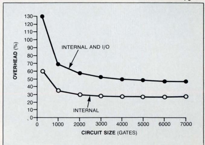
**Fig 2—Although BIST techniques require more silicon overhead than do the other design-for-testability techniques, the percentage of circuit overhead required by the BIST circuitry decreases as you increase the size of the circuit.**
