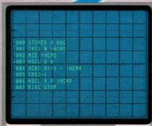
Waveform Processing —Key stroke programming enables user to design measurement routines tailored to individual tests or experiments. System: 7854 with Waveform Calculator Keyboard.
