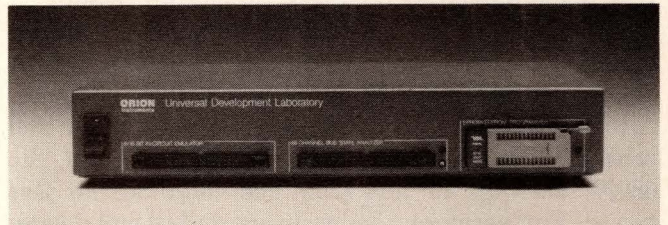
Because the instruments are designed for emulating ROMs in 8- and 16-bit systems, you would need a pair of Orion's $2395 UDLs to work with 32-bit \mu Ps.
