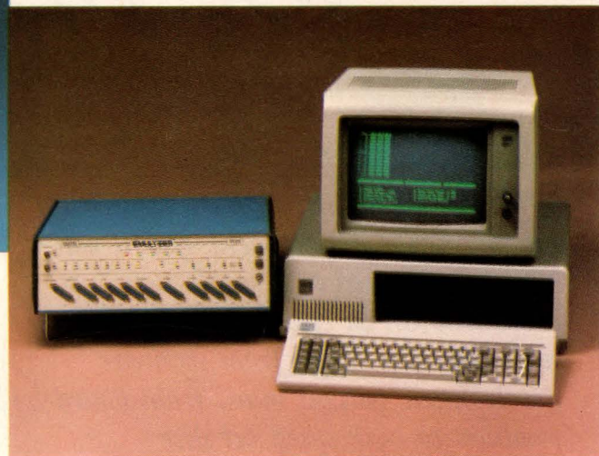
The NCR32 32-bit \mu P is a microprogrammed processor and, hence, mandates a development tool like the Hilevel DS370 ROM emulator and logic analyzer rather than an in-circuit emulator. However, because of their high speed and flexibility, ROM emulators also suit nonmicroprogrammed \mu Ps like the 68020 and 32032.
