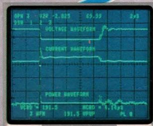
Multi-Waveform Storage and Calculation —Simplifies circuit design. Allows simultaneous viewing of calculated results and acquired waveforms. System: 7854 with 7A22 differential amplifier and 7B87 Time Base.
