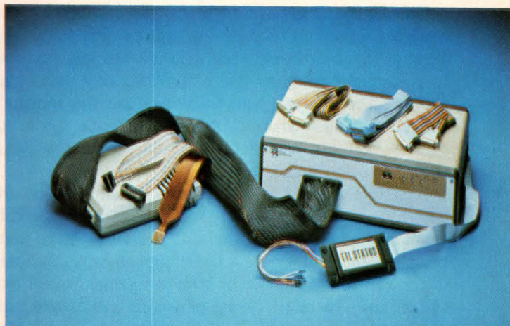
Because of the multichip architecture of the 32032, National's ICE32 emulator has a cable for the \mu P, the memory-management unit, and the clock chip.
