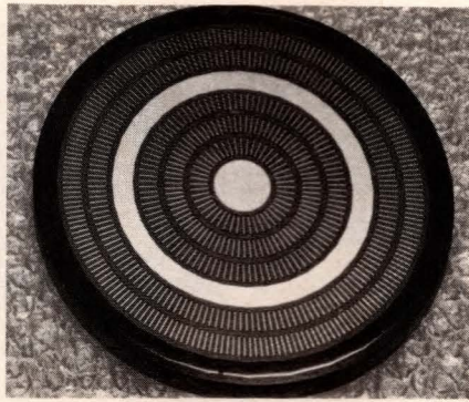
This 50-mm GTO thyristor wafer from Marconi Electronic Devices Ltd shows the highly interdigitated gate/cathode structure of a gate-turn-off thyristor.
