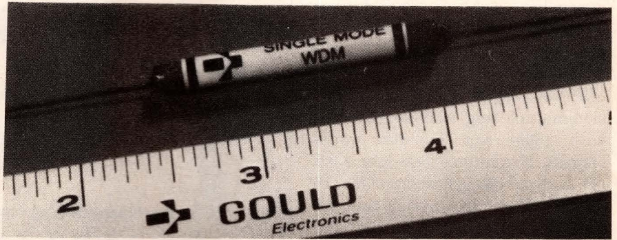
Employing fused-fiber technology, Gould's 2-channel wavelength-division-multiplexing (WDM) couplers operate with 1300- and 1550-nm wavelengths. They feature an excess loss of <0.5 dB and a wavelength isolation of -16 dB min.
